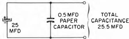
(B) Single polarized electrolytic capacitor shunted with an oil- or paper-dielectric capacitor.
