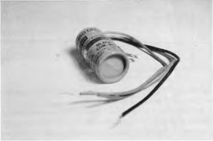
**Fig. 3-10. A typical dual electrolytic capacitor using a common negative connection.**
