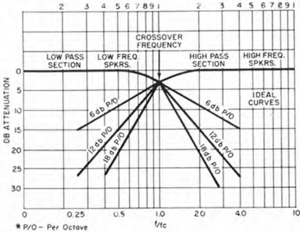
Fig. 1-4. Typical frequency characteristic for ideal 6-, 12-, and 18-db-per-octave crossover networks.
