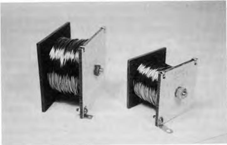
**Fig. 3-4.** 8.5- and 3.5-millihenry coils.
