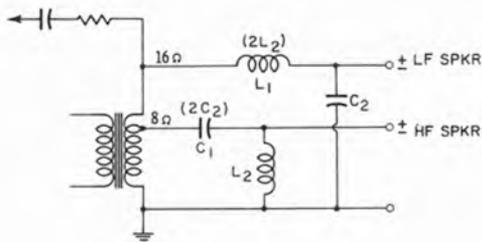
Fig. 2-1B. Circuit when higher impedance speaker is used for low-frequency work.
