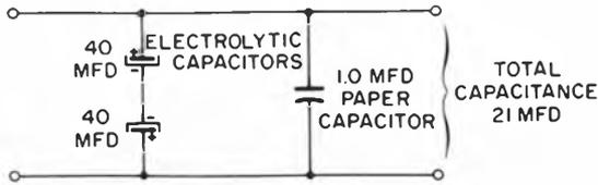
(A) Connected back-to-back in parallel with oil- or paper-dielectric capacitor.
