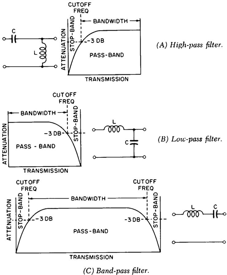
Fig. 1-2. Three basic filter configurations and their response curves.
