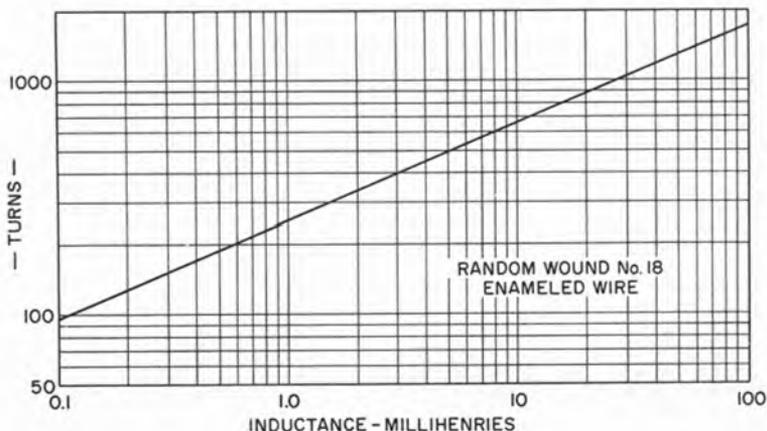
Fig. 3-1. Inductance versus turns of wire, using the form in Fig. 3-2.
