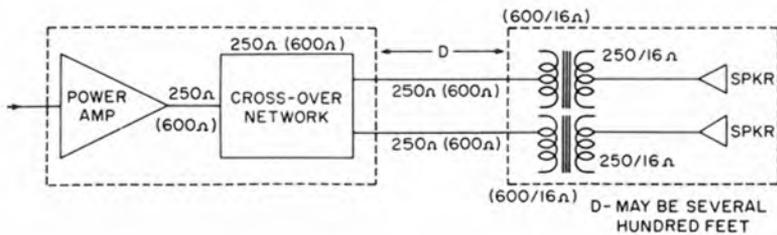
Fig. 1-7. 250-ohm crossover network with 250-ohm transmission line.
