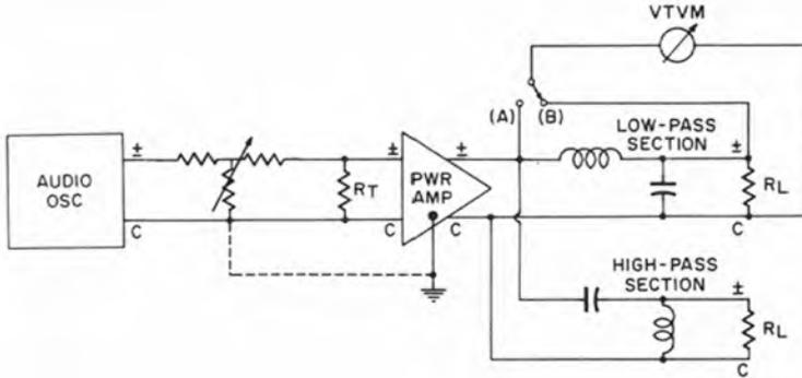
Fig. 4-6. Connections for measuring the insertion loss of a two-way network. (Series-type networks are measured in a similar manner.)
