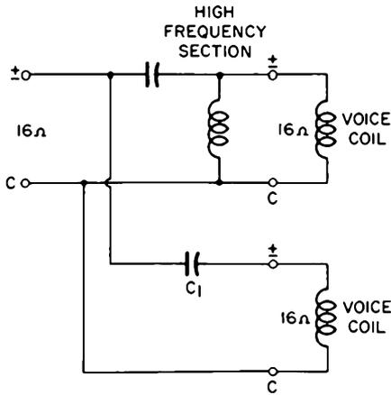
Fig. 2-8. Method of connecting a second high-frequency unit in parallel with the high-frequency section of the network.
