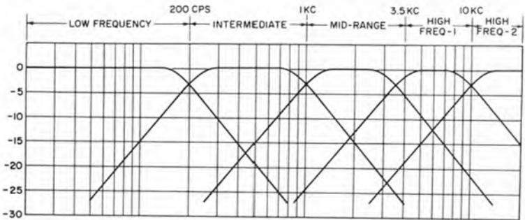
**Fig. 2-7. Typical frequency-response characteristics of a five-way, constant-k crossover network.**
