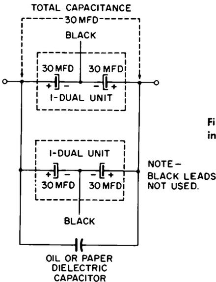
Fig. 3-12. Method of connecting the electrolytic capacitors to obtain the proper capacitance.
