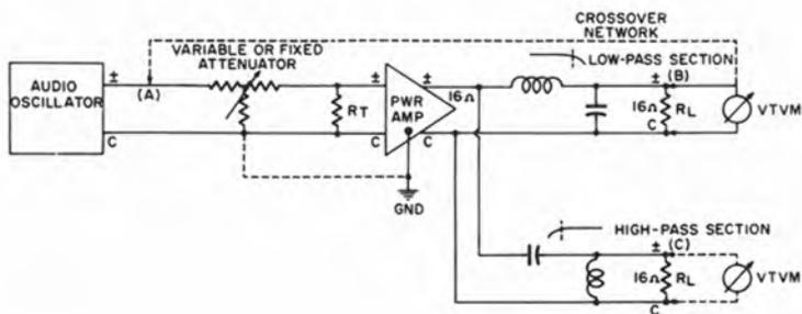
Fig. 4-2. Connections for measuring the frequency characteristics of a two-way crossover network with a 16-ohm impedance.
