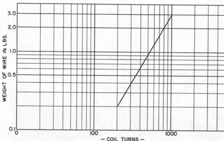
Fig. 3-7. Coil turns versus pounds of wire.
