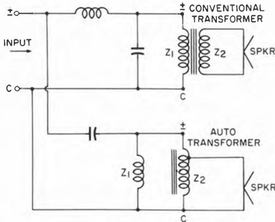
Fig. 2-2. An alternate method of matching speakers of unequal impedances.
