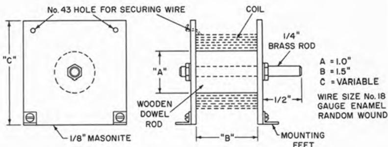
Fig. 3-2. Coil form for winding speaker crossover-network inductors.
