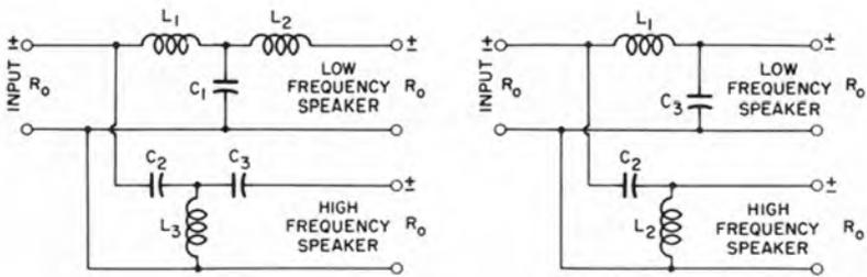
(A) Parallel type, 18 db per octave. (B) Parallel type, 12 db per octave.
