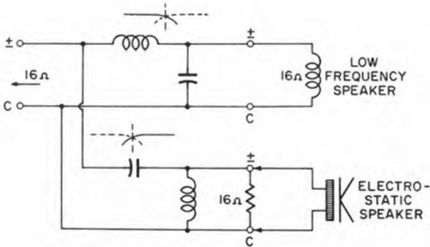
**Fig. 4-8. A two-way crossover network using a compression and an electrostatic speaker.**
