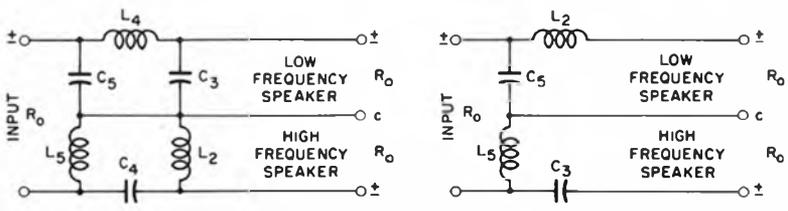
(C) Series type, 18 db per octave. (D) Series type, 12 db per octave.
