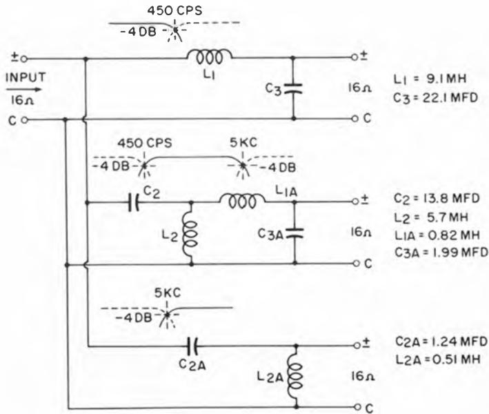
Fig. 2-10. A three-way, 12-dB per-octave, *m*-derived crossover network for a circuit impedance of 16 ohms.
