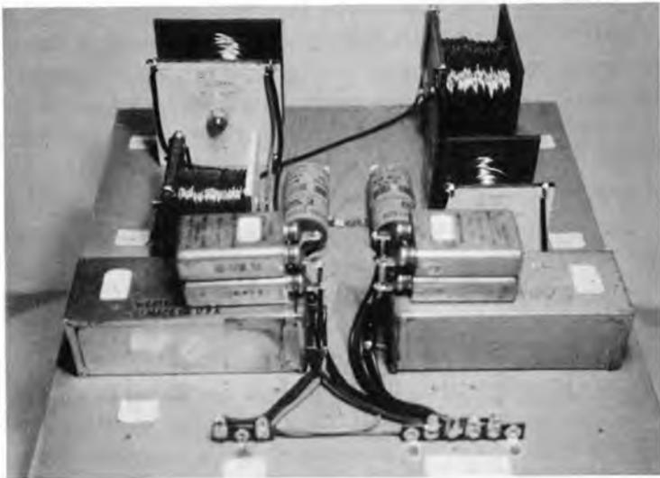
Fig. 3-9. A three-way, 16-ohm, 12-db per-octave crossover network. Crossover is at 450 and 5000 cps.
