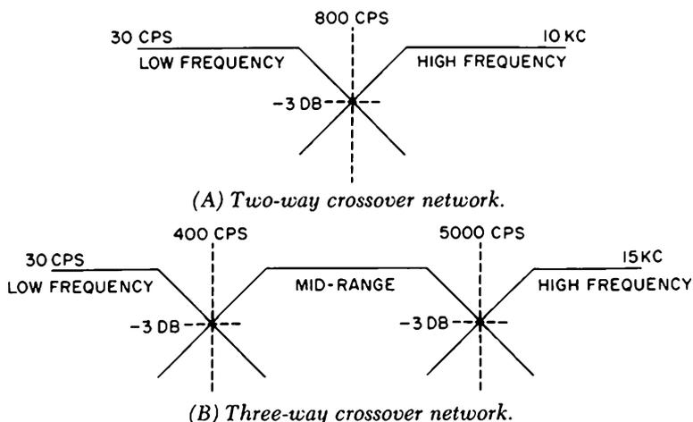
Fig. 1-3. Typical frequency-response characteristics of crossover networks.
