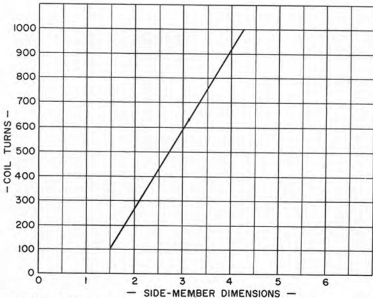
Fig. 3-5. Coil turns versus side-member dimensions. Random-wound No. 18 enameled wire.
