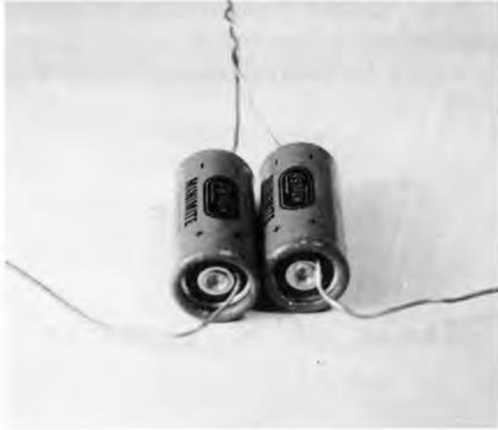
**Fig. 3-13. Two single electrolytic capacitors connected back-to-back to form a nonpolarized capacitor.**
