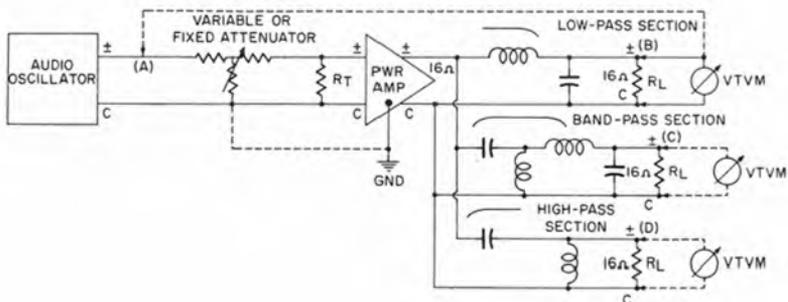
Fig. 4-4. Connections for measuring the frequency characteristics of a three-way crossover network with a 16-ohm impedance.
