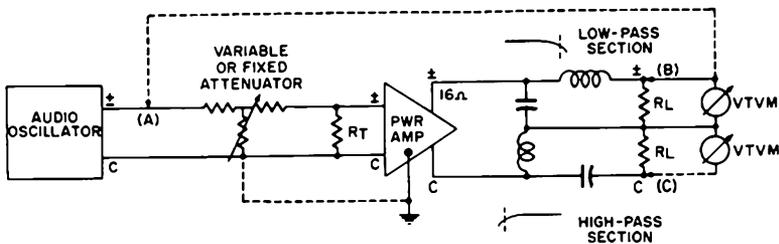
Fig. 4-5. Connections for measuring the frequency characteristics of a two-way, series-type network with a 16-ohm impedance. (The procedure for the measurement is the same as for a parallel network.)
