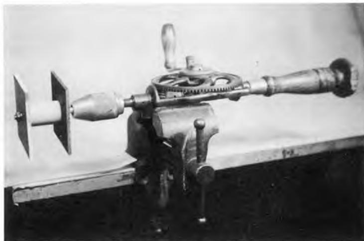
**Fig. 3-6. Coil form mounted in hand drill for winding.**
