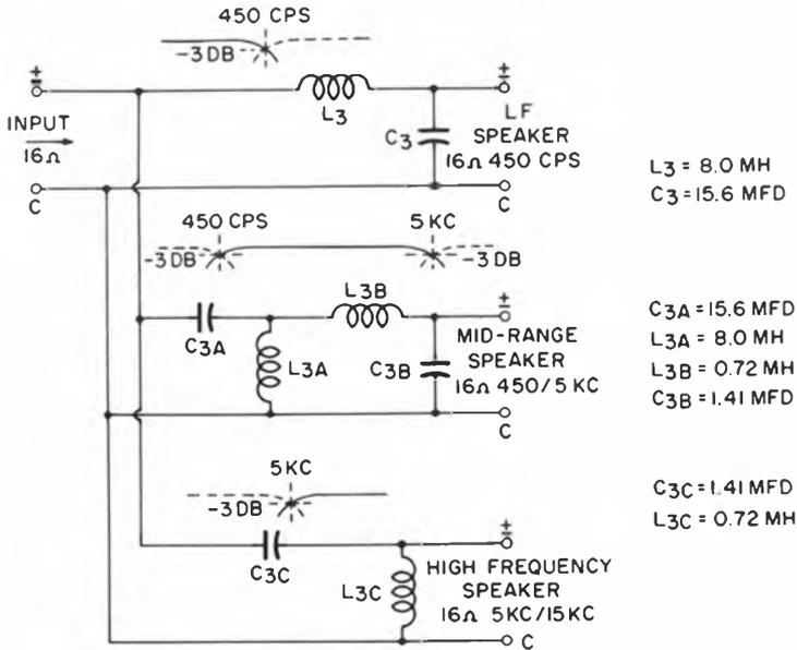
Fig. 2-4. A three-way, 12-db per-octave, 16-ohm impedance, constant-k crossover network.
