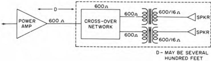
Fig. 1-8. 600-ohm crossover network with 600-ohm transmission line.
