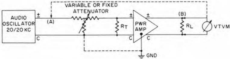
Fig. 4-1. Connections for measuring the frequency response of an amplifier.
