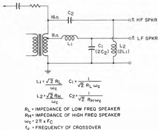
Fig. 2-1A. Method of matching speakers of unequal impedances.
