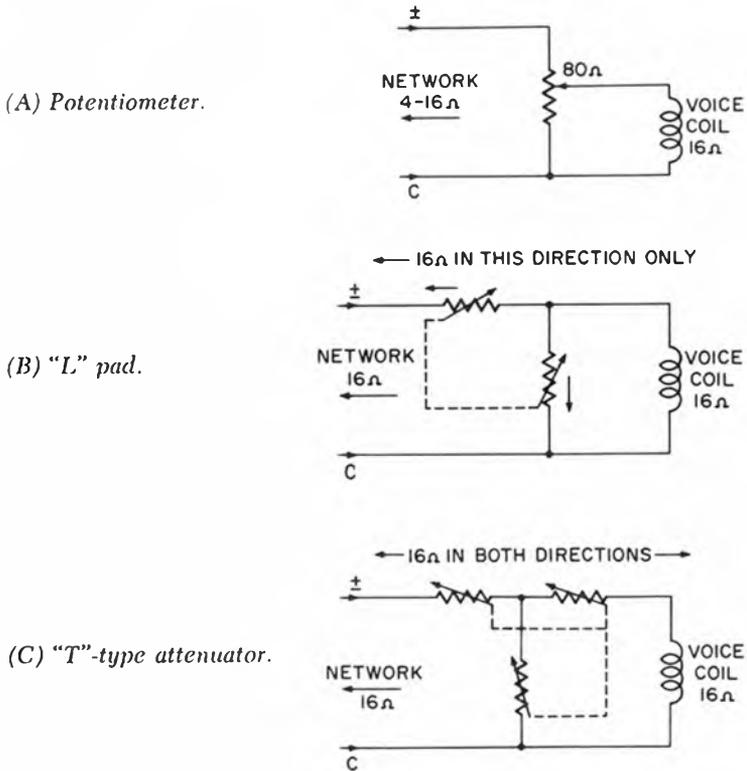
Fig. 4-7. Three types of controls for adjusting the acoustical output level of the midrange and high-frequency units.
