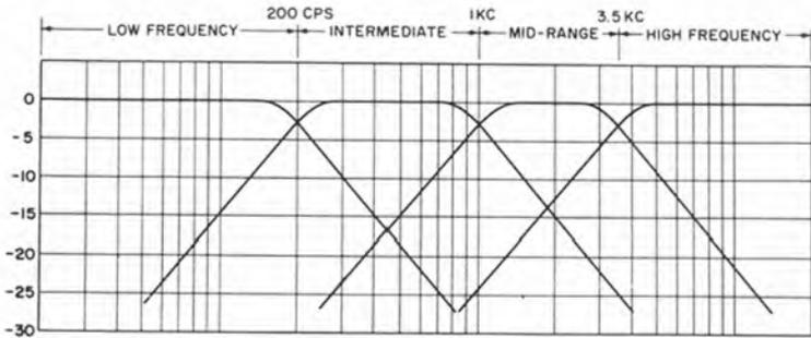
**Fig. 2-6. Typical frequency-response characteristics of a four-way, constant-k crossover network.**
