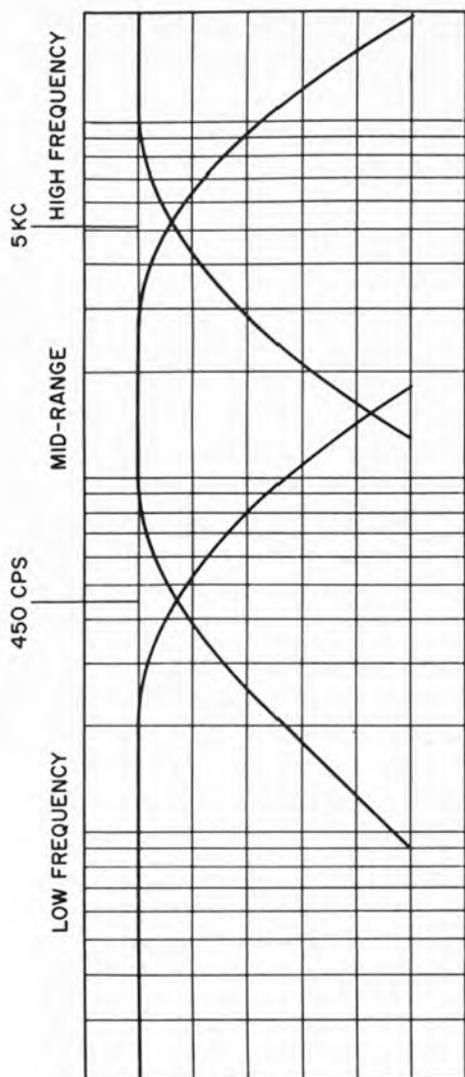
Fig. 2-5. Frequency characteristics of a three-way, 12-db per-octave, 16-ohm parallel network.
