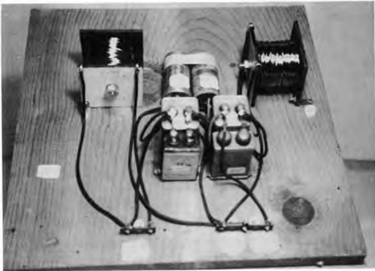
Fig. 3-8. A two-way, 800-cps, 16-ohm, 12-db per-octave crossover network.
