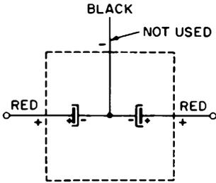
Fig. 3-11. Internal connection of a dual electrolytic capacitor.
