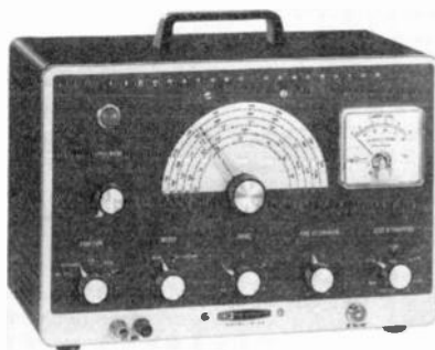
Fig. 2-7. A quality signal generator available in kit form. It covers 100 kHz to 9.5 MHz in four bands. The output meter provides calibrated r-f output
