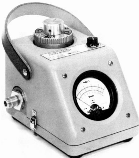
Fig. 6-12. The Sierra Bidirectional Power Monitor reads forward power and SWR directly on the meter scale. Plug-in units, on top, are multipliers for reading power in watts into a 50-ohm load.
