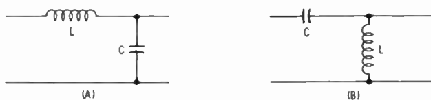
Fig. 2-19. Constant- k filter sections. A is a low-pass, and B a high-pass filter.
