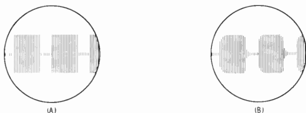
Fig. 5-14. Observing uniformly spaced c-w dots on a scope. With no keying filter they will be perfectly rectangular as in A. Proper filtering results in rounding the corners, which reduces key clicks, as in B.
