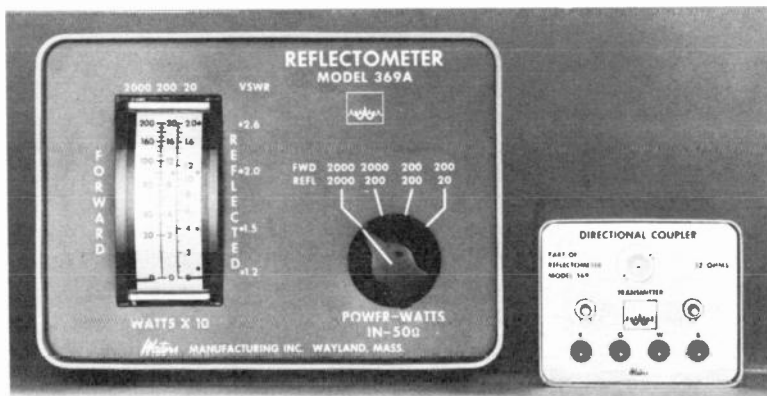
Fig. 6-10. This reflectometer has a meter with two pointers. One reads forward power and the other reflected. When loaded with exactly 50 ohms, the power readings are actual. VSWR is shown in the vertical panel scale to the right of the meter.
