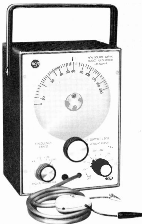
Fig. 2-8. A sine-/ square-wave audio oscillator. It covers the range from 20 Hz to 200 kHz. Output is a choice of pure sine wave or a square wave, which has value in hi-fi measurements.
