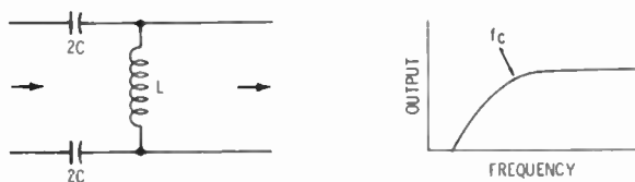
Fig. 2-28. A simple high-pass filter as used at the input of TV sets. The sketch at the right shows approximate response.
