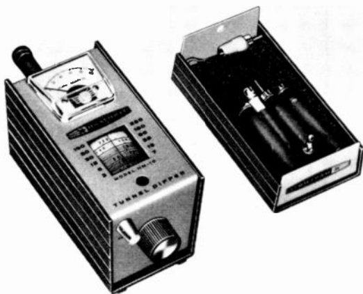
Fig. 7-21. A tunnel-diode GDO made from a kit. Plug-in coils cover the range from 3 to 260 MHz.
