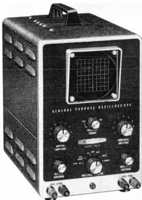
Fig. 7-22. Any inexpensive oscilloscope will serve as a modulation monitor. This one is available in kit form.
