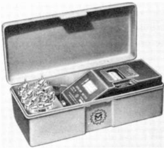
Fig. 2-5A. A commercial high-quality grid-dip oscillator. Its accuracy is much higher than is normally available from a kit or home-built unit.
