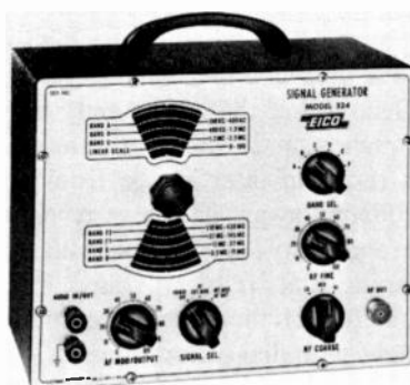
Fig. 4-1. The Eico Model 324-K signal generator has output from 150 kHz to 145 MHz on fundamentals. The built-in 400-Hz modulator is variable up to 50 percent.
