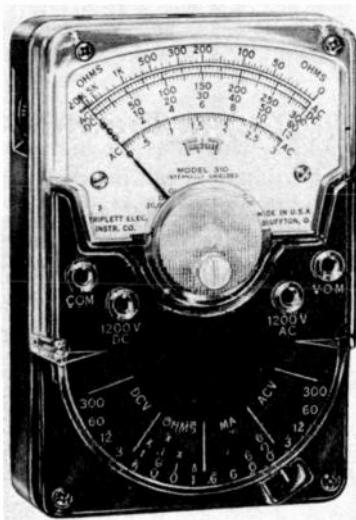
Fig. 7-1. This pocket-sized VOM measures only 2-3/4" x 4-1/4" x 1-5/16". It has 20,000 ohms-per-volt sensitivity.
