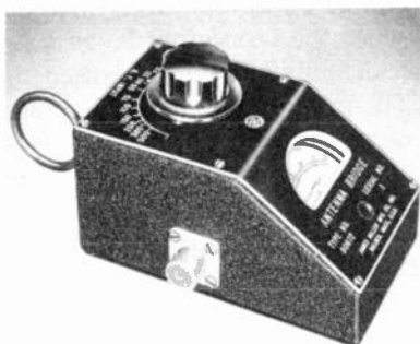
Fig. 7-13. An impedance bridge for use up to 140 MHz. It has a variable capacitor for a bridge arm instead of a variable resistor. Note the loop on back for coupling to a GDO for signal source.
