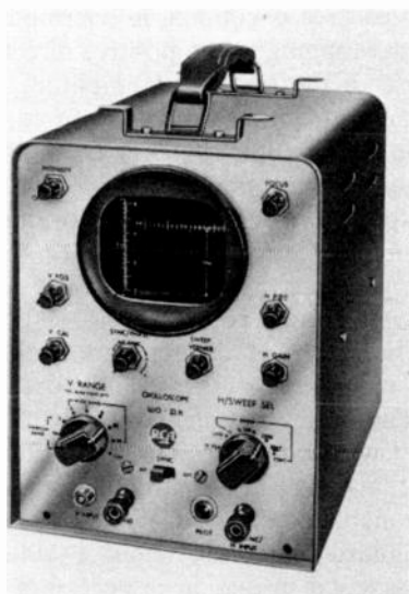
Fig. 5-9. A medium-priced oscilloscope available in kit form or wired. The Model WO-33A is switchable from a medium-gain, wideband (to 5.5 MHz) amplifier to a high-gain, medium-bandwidth (to 150 kHz) amplifier.
