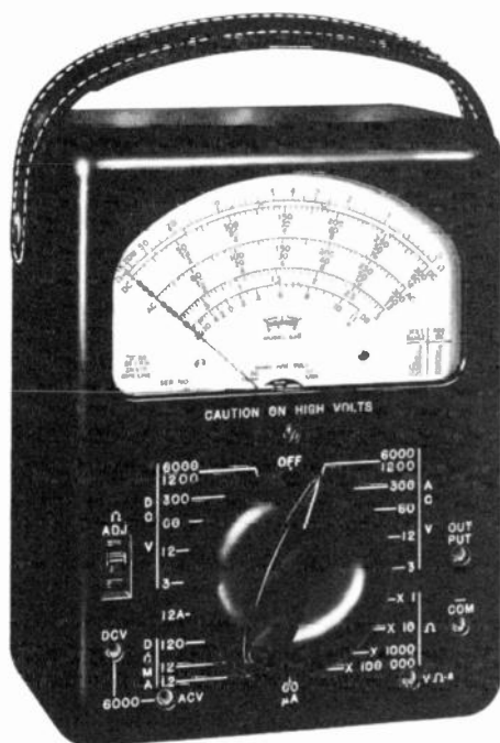
Fig. 1-1. The Triplet Model 630 VOM is typical of many of the better 20,000 ohms/volt VOM's.
