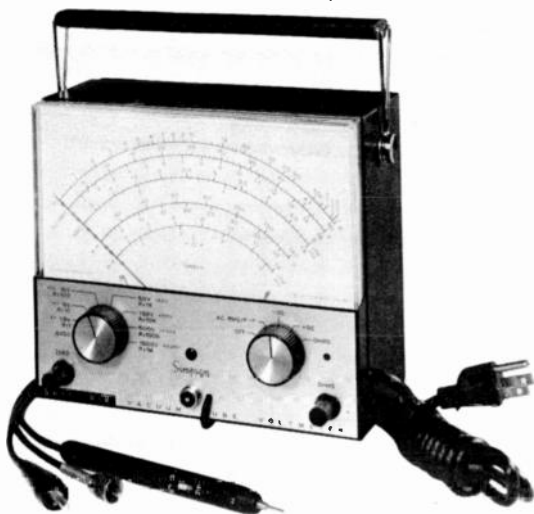
Fig. 7-3. This VTVM features an unusually large meter scale. The d-c input resistance is 16 megohms, as compared to the usual 11.
