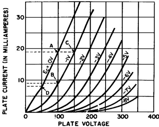
Fig. 1-4. Plate characteristic curves of a typical triode.
