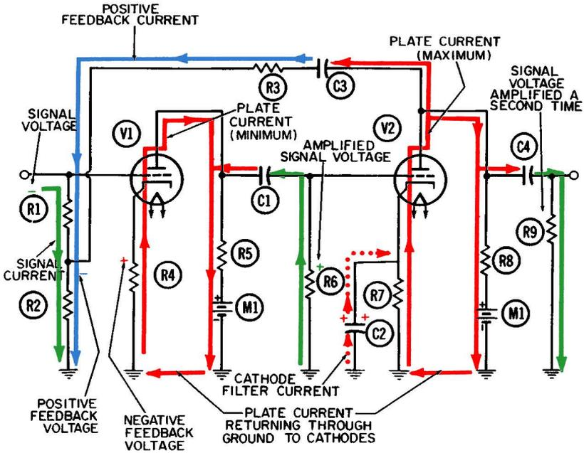
Fig. 2-9. An R-C coupled audio amplifier utilizing both positive and negative feedback—negative half-cycle.
