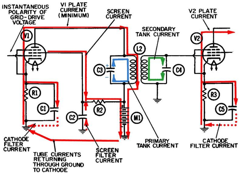
Fig. 7-5. Operation of the tuned-primary—tuned-secondary RF amplifier —first half-cycle at resonance.
