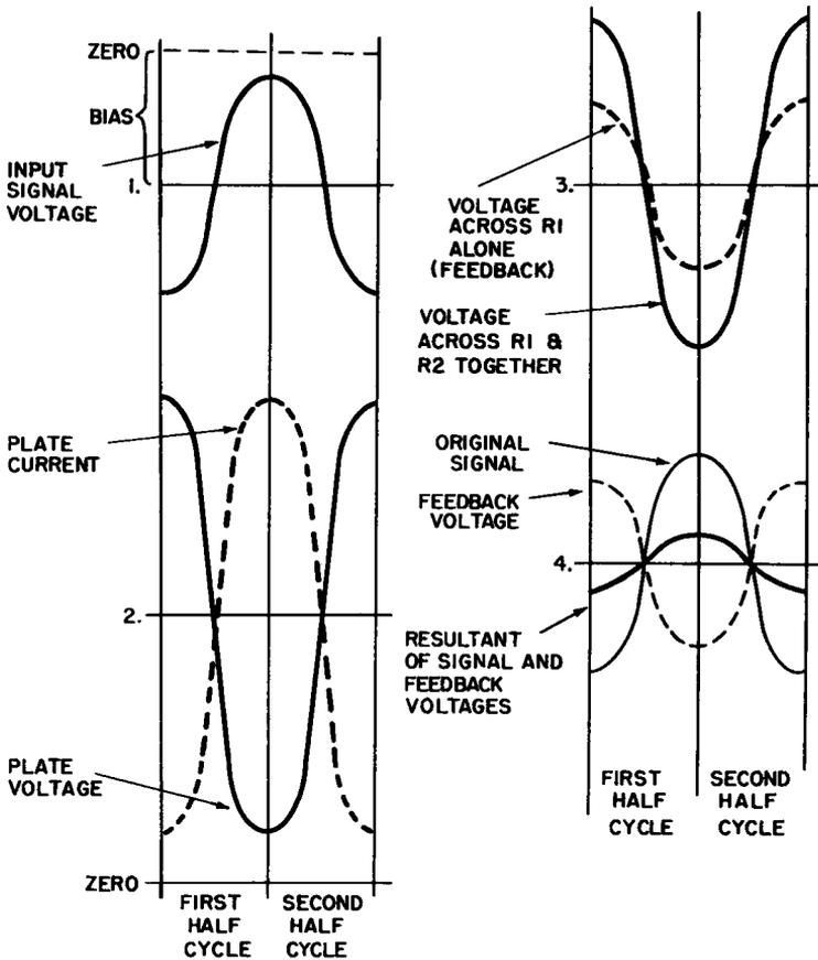
Fig. 3-9. Voltage and current waveforms in negative-feedback amplifier circuit.
