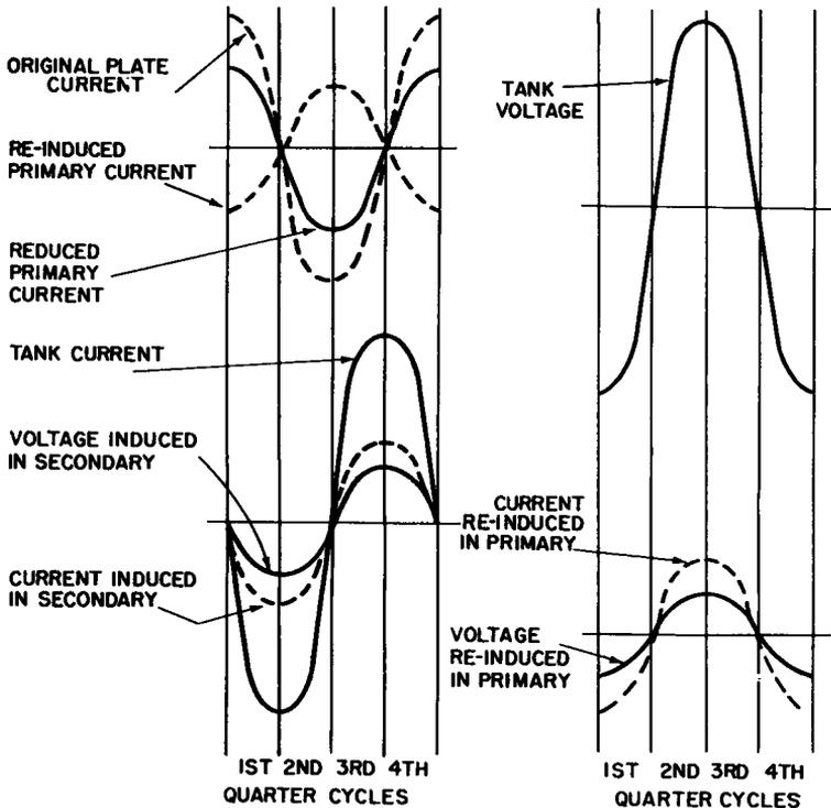
Fig. 7-4. Voltage and current waveforms in the tuned secondary circuit at resonance.
