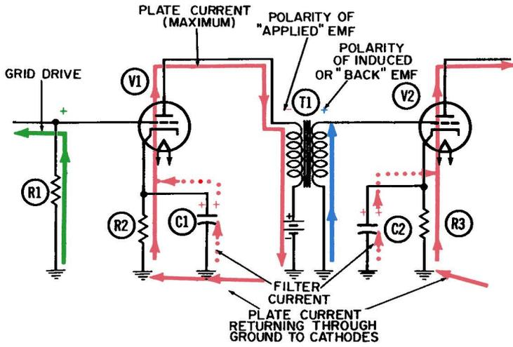
Fig. 3-1. The transformer-coupled AF amplifier—first half-cycle.
