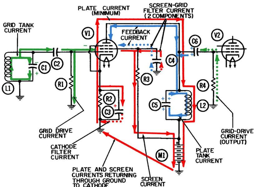
Fig. 6-3. Operation of the tuned impedance-coupled amplifier—first half-cycle.
