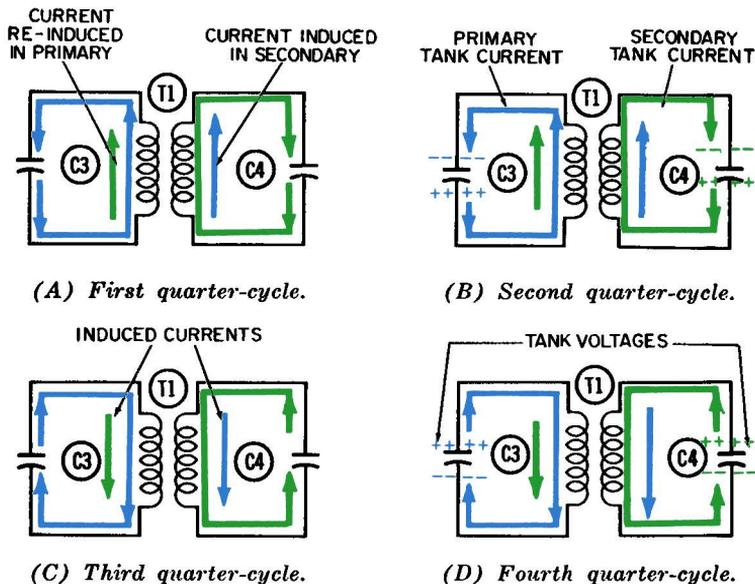
Fig. 7-12. The four quarter-cycles of operation of the bandpass tank circuit at a frequency below resonance.
