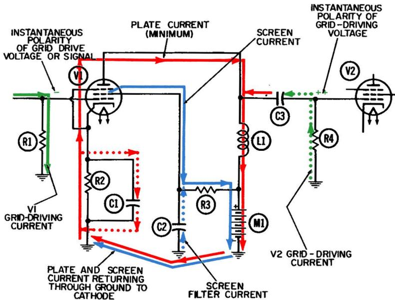
**Fig. 6-1. Operation of the untuned impedance-coupled amplifier—first half-cycle.**
