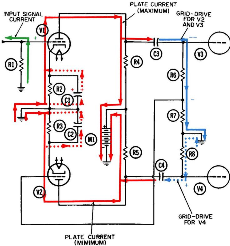
**Fig. 5-4. Operation of a two-tube phase-inverter circuit—second half-cycle.**
