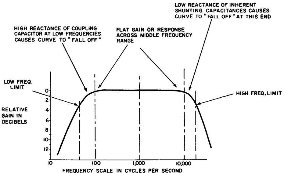
Fig. 2-5. An R-C coupled audio amplifier response curve.
