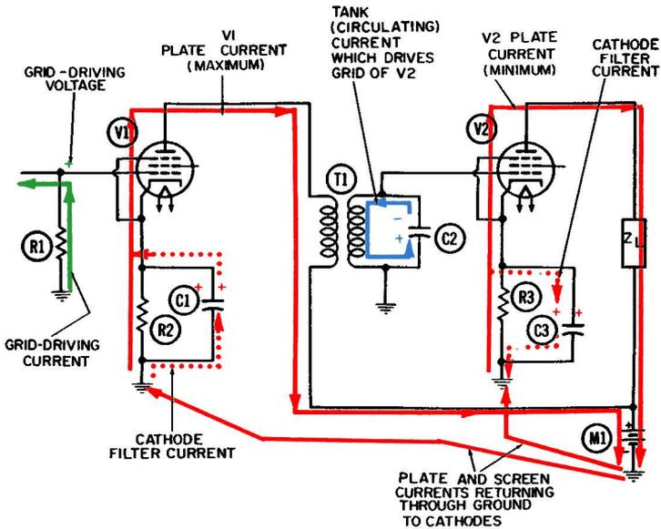
Fig. 7-2. Operation of the untuned-primary-tuned-secondary RF amplifier—second half-cycle.
