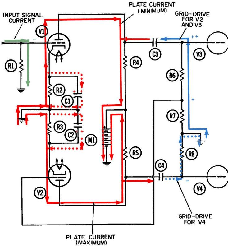
Fig. 5-3. Operation of a two-tube phase-inverter circuit—first half-cycle.
