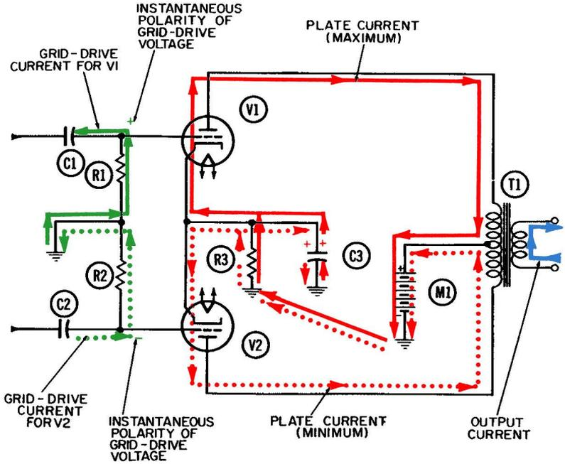
**Fig. 4-6. Operation of a push-pull AF power amplifier using cathode bias—first half-cycle.**
