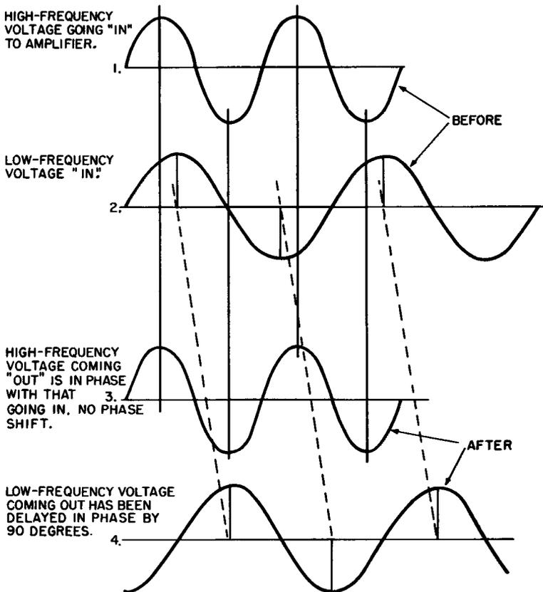
Fig. 2-11. The effect of phase distortion on a waveform.
