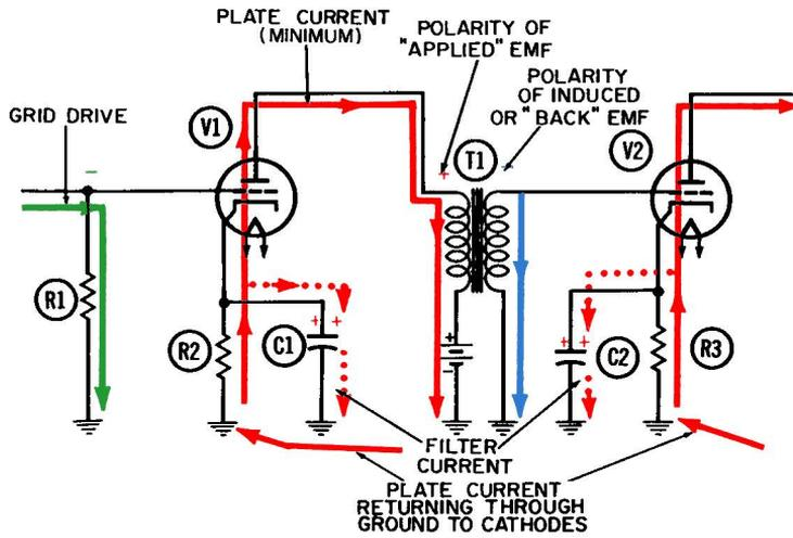
Fig. 3-2. The transformer-coupled AF amplifier—second half-cycle.
