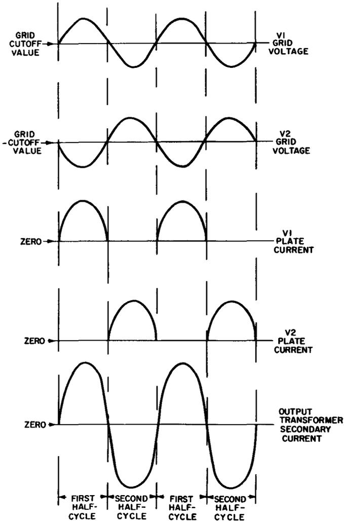
Fig. 4-8. Voltage and current waveforms in a Class-B power amplifier.
