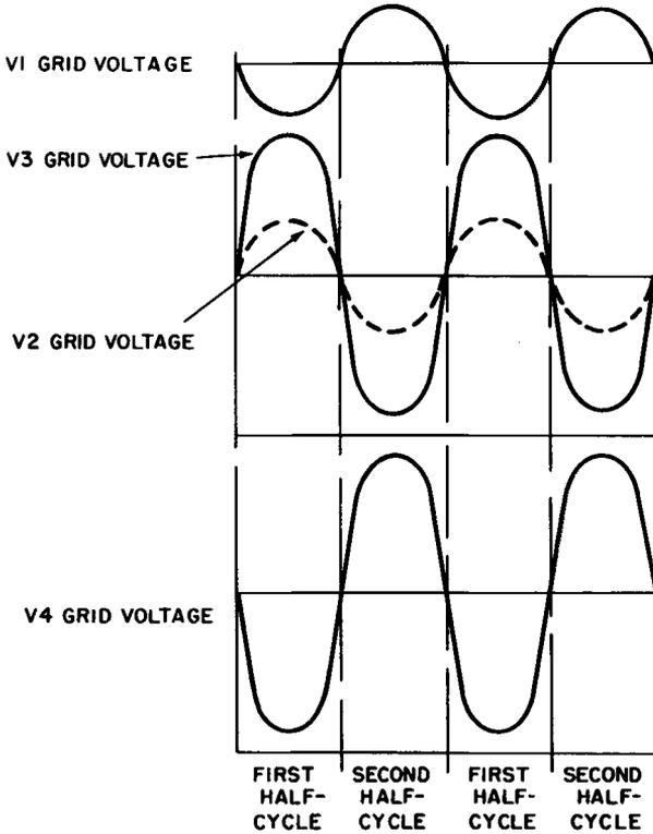
Fig. 5-5. Grid-voltage waveforms for the circuit in Figs. 5-3 and 5-4.
