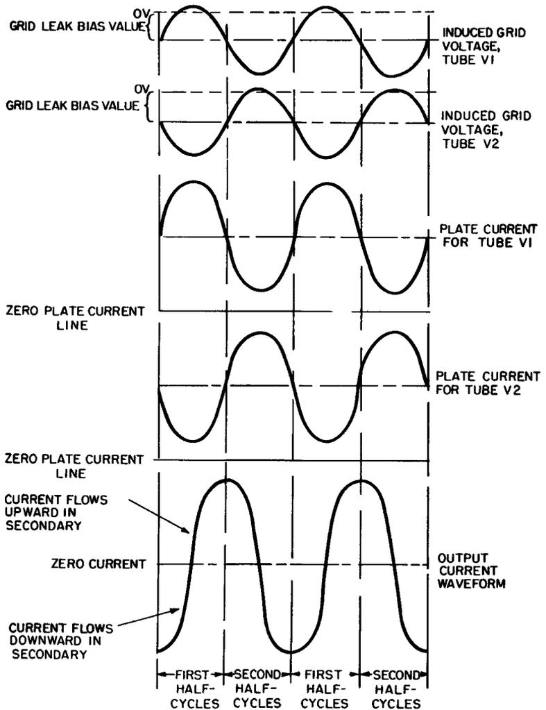
Fig. 4-5. Voltage and current waveforms in the amplifier of Figs. 4-3 and 4-4.
