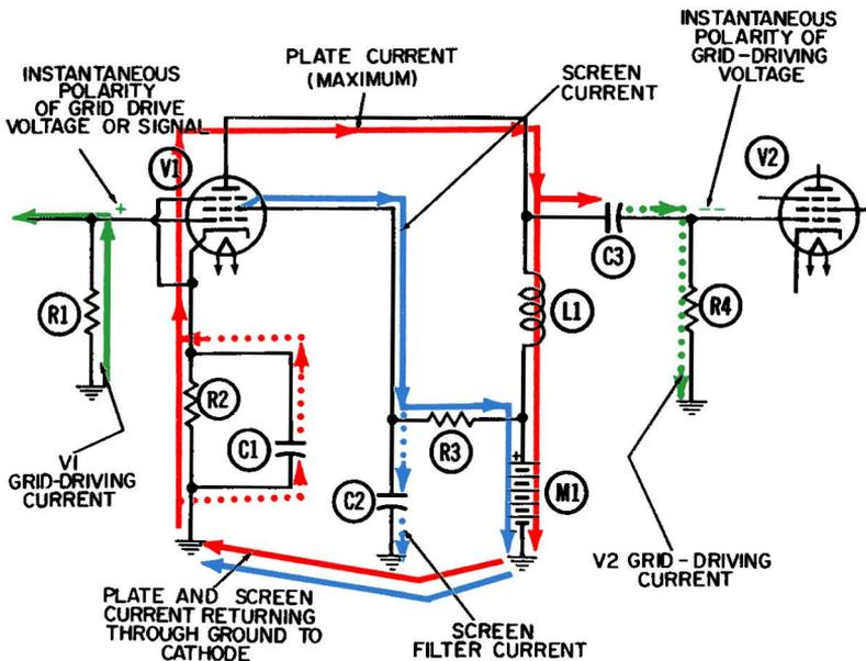
**Fig. 6-2. Operation of the untuned impedance-coupled amplifier—second half-cycle.**
