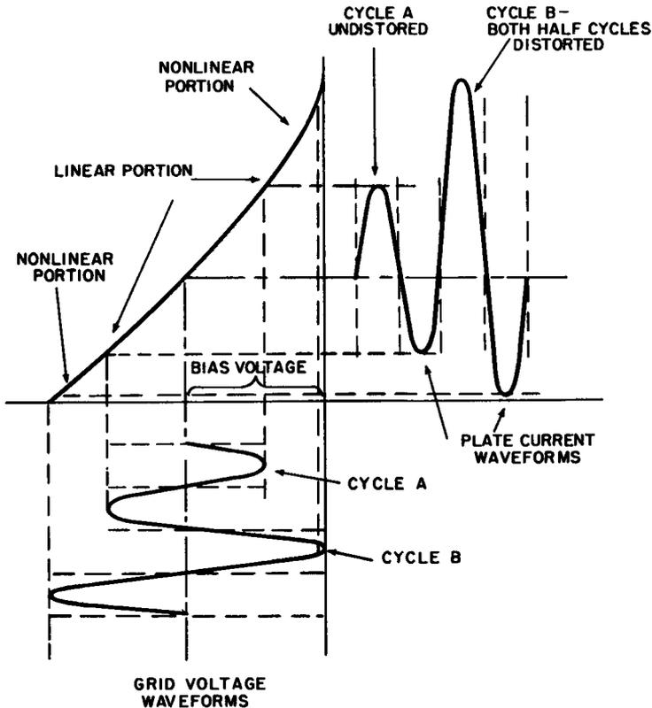
Fig. 2-10. How amplitude distortion is introduced when tube is operated on nonlinear portion of transfer characteristic curve.
