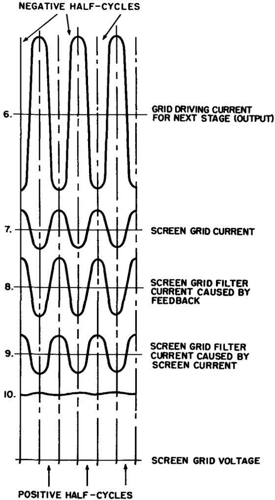
in the tuned impedance-coupled amplifier.
