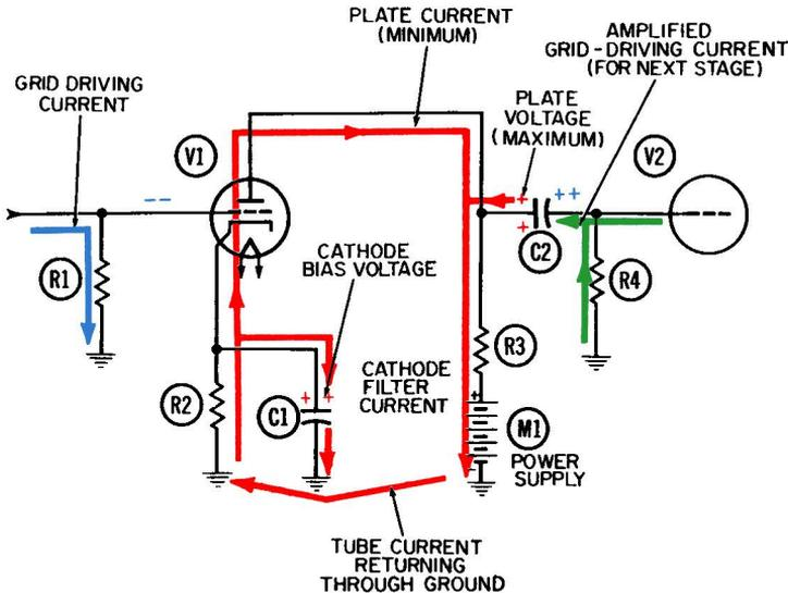
Fig. 2-1. The R-C coupled audio amplifier—negative half-cycle.
