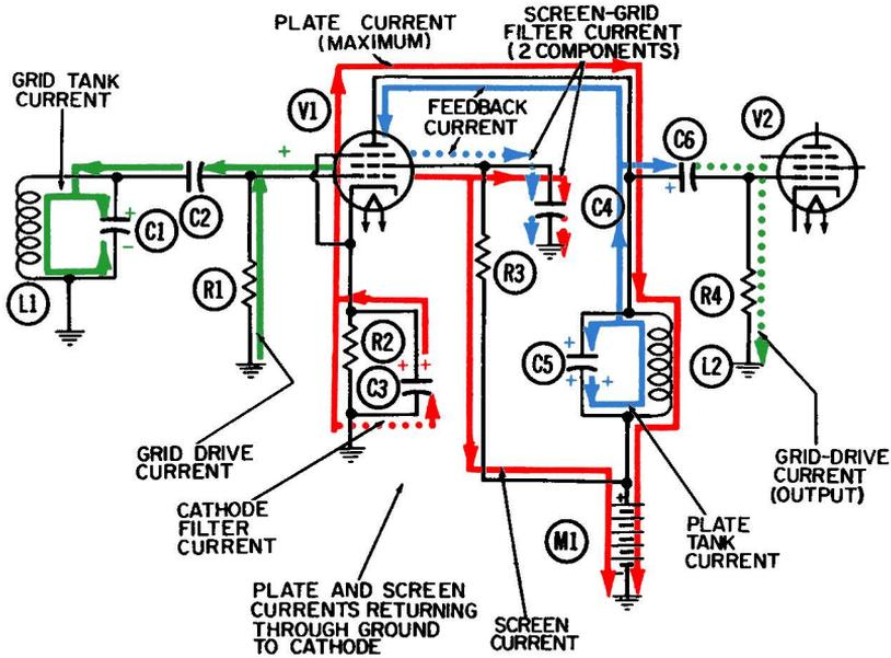
Fig. 6-4. Operation of the tuned impedance-coupled amplifier—second half-cycle.
