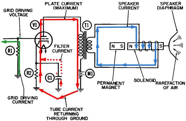
Fig. 4-1. Operation of an AF power amplifier—first half-cycle.
