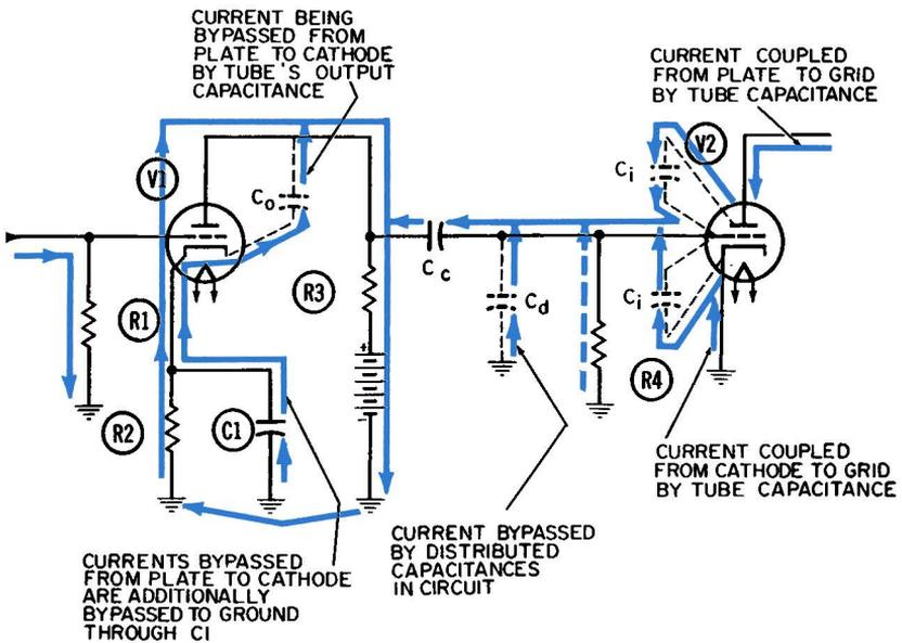
Fig. 2-7. Equivalent circuit at high frequencies in the R-C coupled audio amplifier—negative half-cycle.
