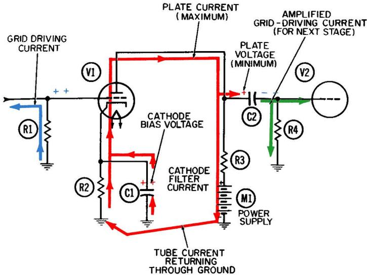
Fig. 2-2. The R-C coupled audio amplifier—positive half-cycle.
