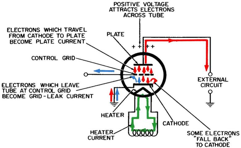
Fig. 1-3. The triode vacuum tube.
