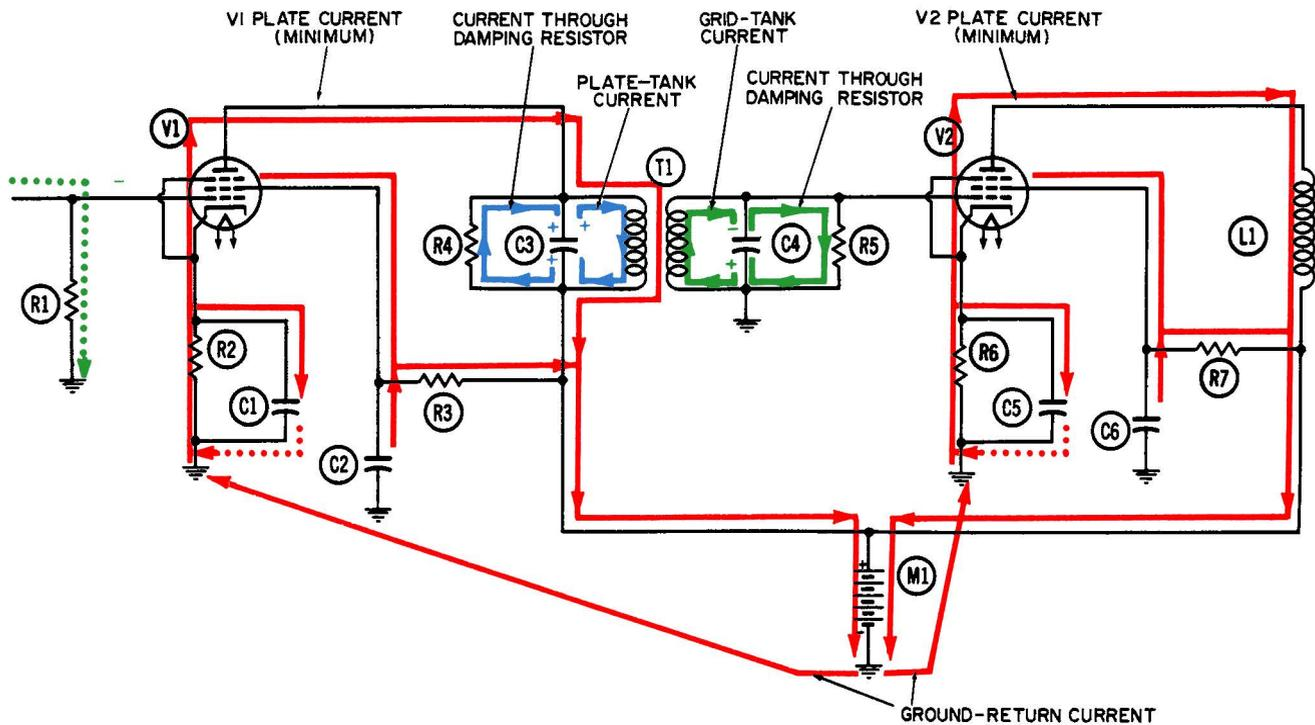
Fig. 7-8. Operation of the bandpass RF amplifier—second half-cycle.
