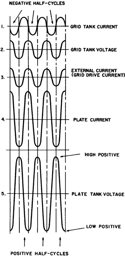
Fig. 6-5. Voltage and current waveforms
