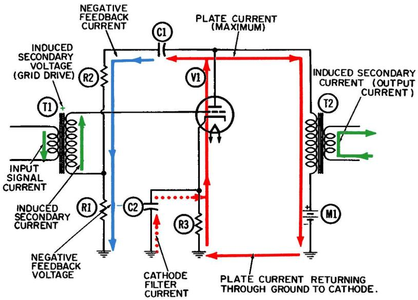
Fig. 3-7. Negative feedback amplifier circuit—first half-cycle.
