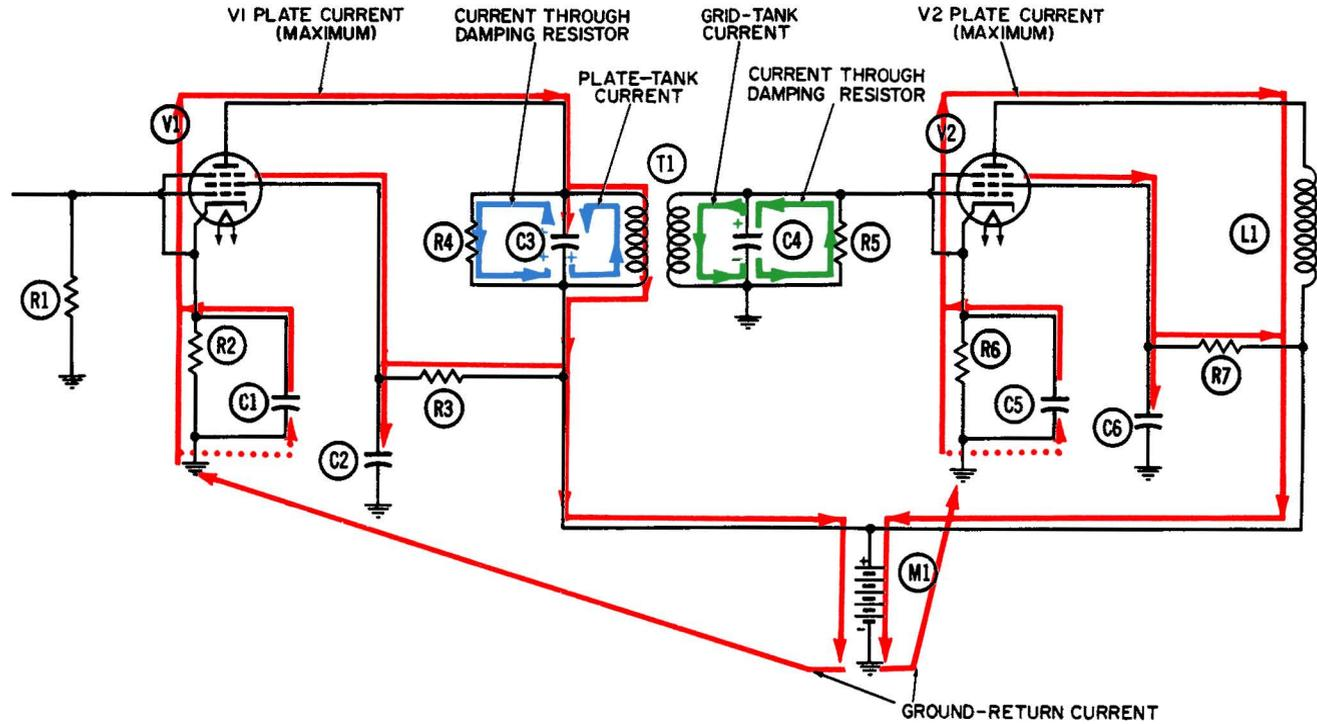
Fig. 7-7. Operation of the bandpass RF amplifier—first half-cycle.
