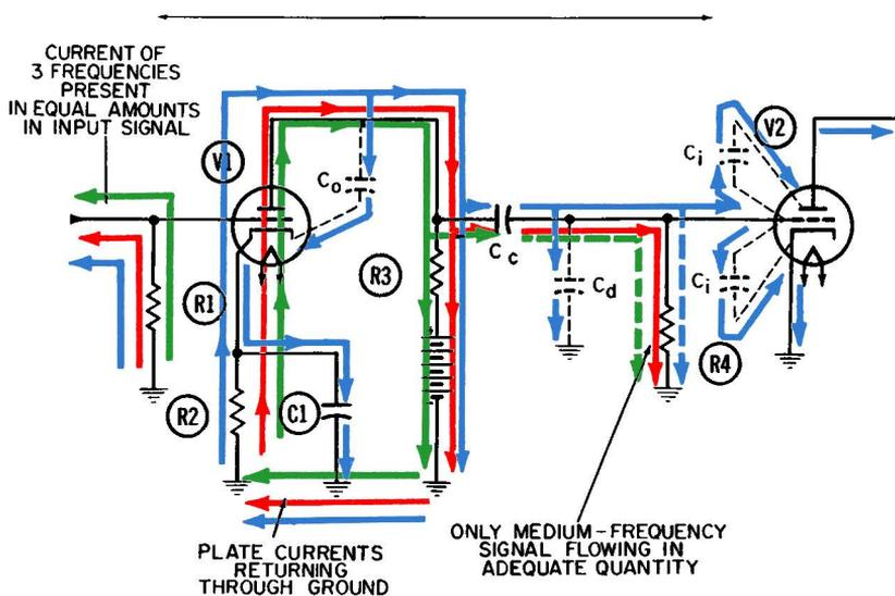
Fig. 2-6. Current flow at low, medium, and high frequencies in the R-C coupled audio amplifier—positive half-cycle.
