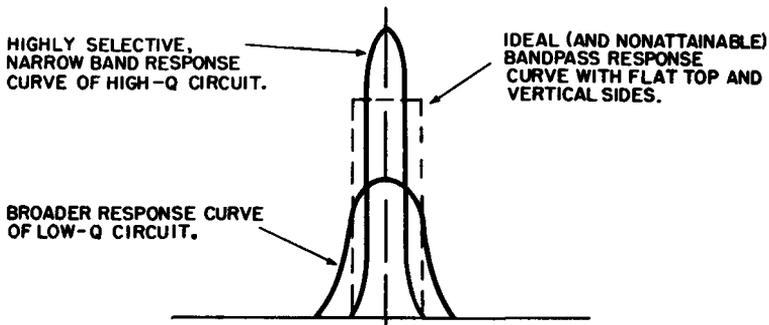
Fig. 7-9. Response curves of high- and low-Q circuits at resonance.
