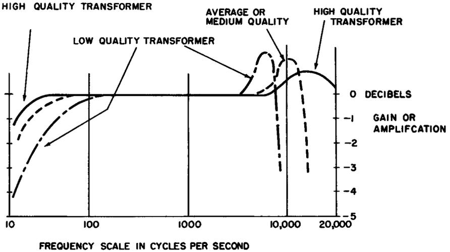
Fig. 3-4. Response curves of transformer-coupled AF amplifiers.
