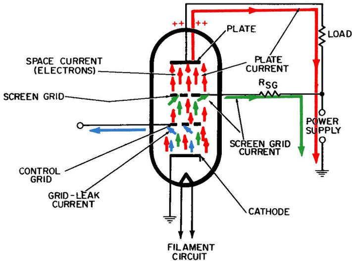
Fig. 1-5. The tetrode vacuum tube.
