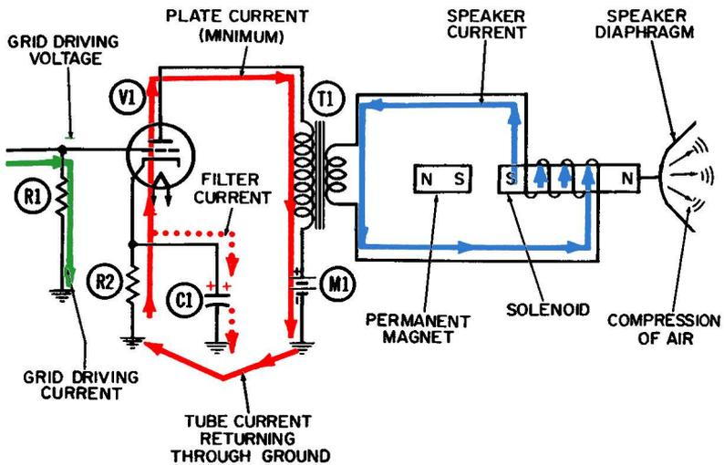
Fig. 4-2. Operation of an AF power amplifier—second half-cycle.
