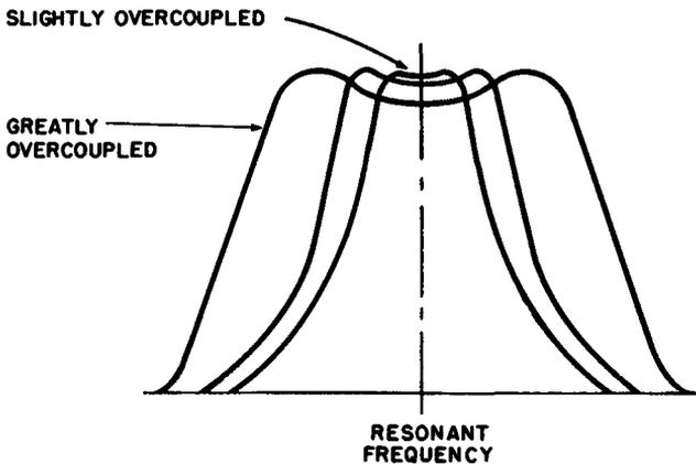
Fig. 7-10. Response curves of over-coupled tuned circuits.
