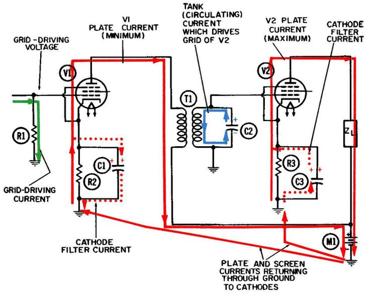
Fig. 7-1. Operation of the untuned-primary-tuned-secondary RF amplifier—first half-cycle.
