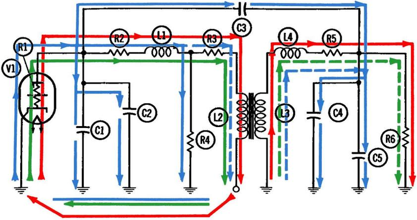
Fig. 3-5. Equivalent circuit of transformer-coupled AF amplifier—first half-cycle.
