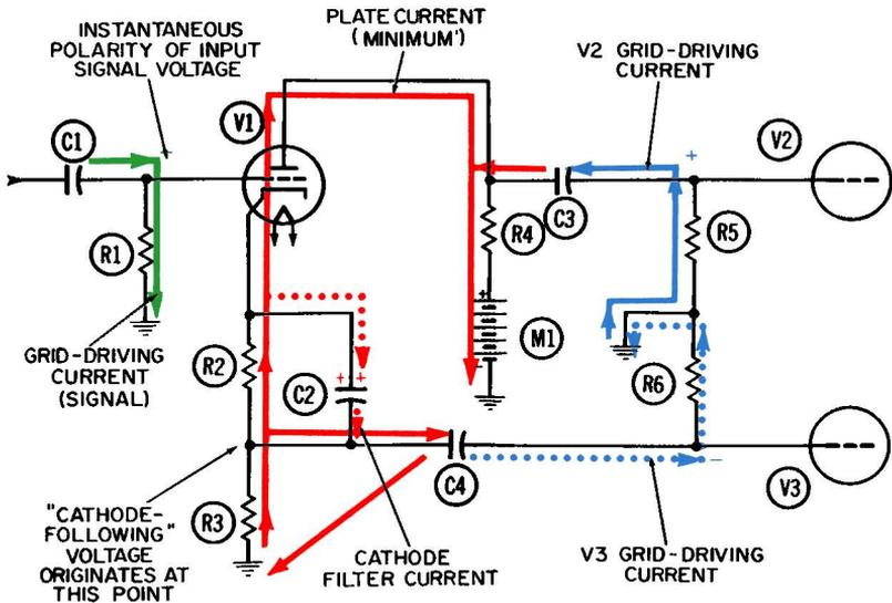
Fig. 5-2. Operation of a cathode-follower phase-inverter circuit—second half-cycle.
