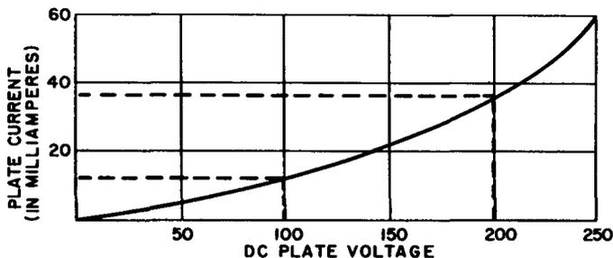
FILAMENT HEATING VOLTAGE - 2.5 VOLTS.
