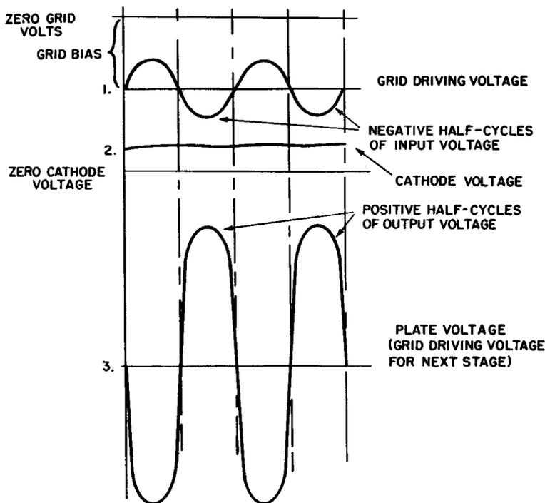
Fig. 2-4. Relationship between grid, cathode, and plate voltages in an R-C coupled audio amplifier.
