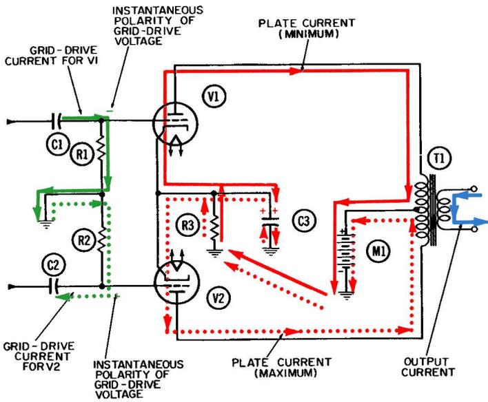
**Fig. 4-7. Operation of a push-pull AF power amplifier using cathode bias—second half-cycle.**
