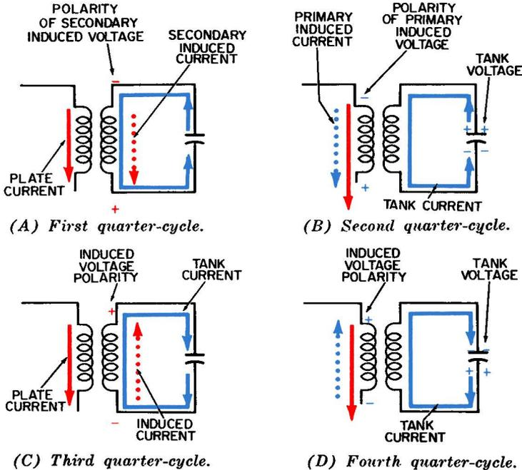
Fig. 7-3. The four quarter-cycles of operation of the tuned secondary circuit at resonance.
