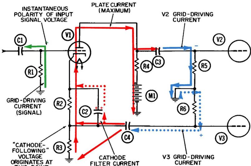
Fig. 5-1. Operation of a cathode-follower phase-inverter circuit—first half-cycle.
