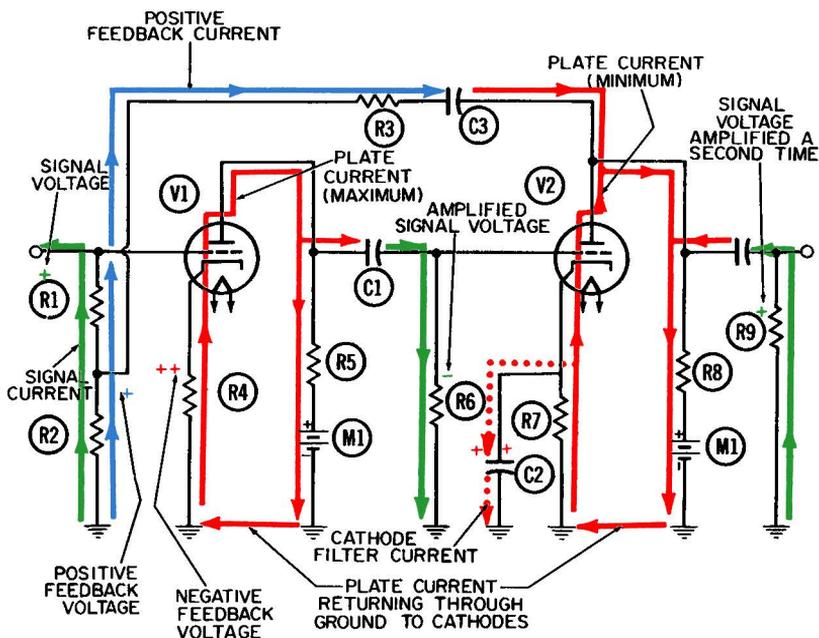
Fig. 2-8. An R-C coupled audio amplifier utilizing both positive and negative feedback—positive half-cycle.
