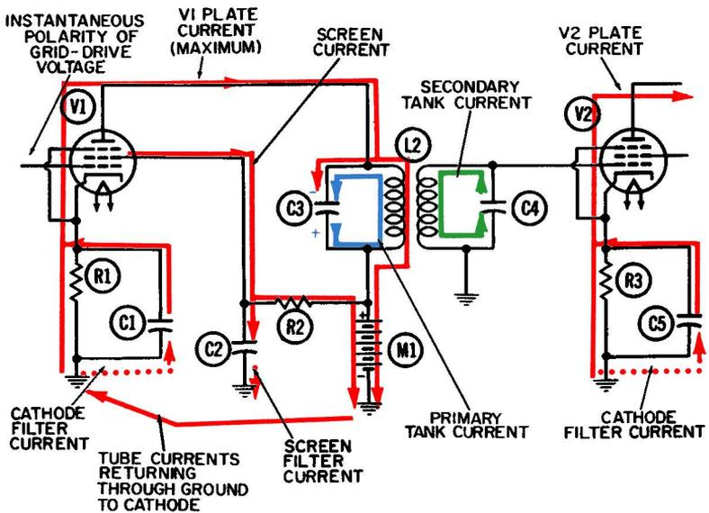
Fig. 7-6. Operation of the tuned-primary—tuned-secondary RF amplifier —second half-cycle at resonance.
