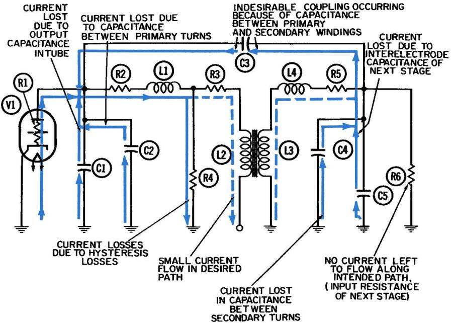
Fig. 3-6. Equivalent circuit of transformer-coupled AF amplifier at high frequencies—second half-cycle.
