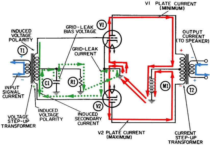
Fig. 4-4. Operation of a push-pull AF power amplifier using grid-leak bias—second half-cycle.
