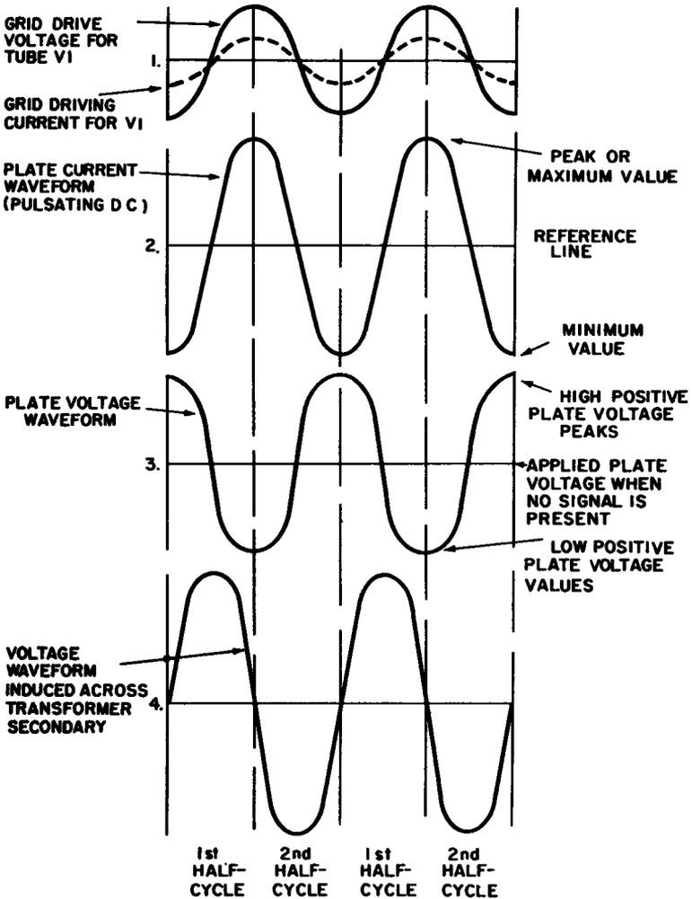
Fig. 3-3. Voltage and current waveforms in the transformer-coupled AF amplifier.
