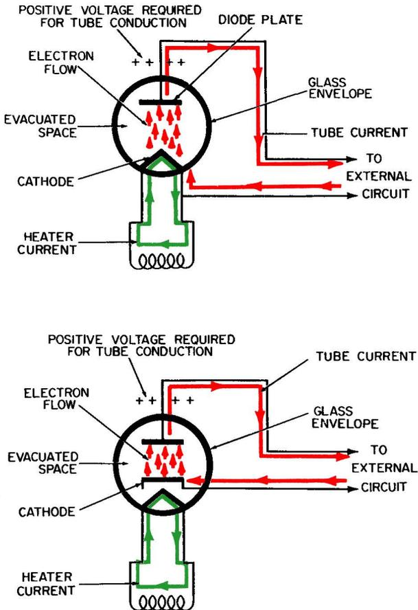
Fig. 1-1. The diode vacuum tube.
