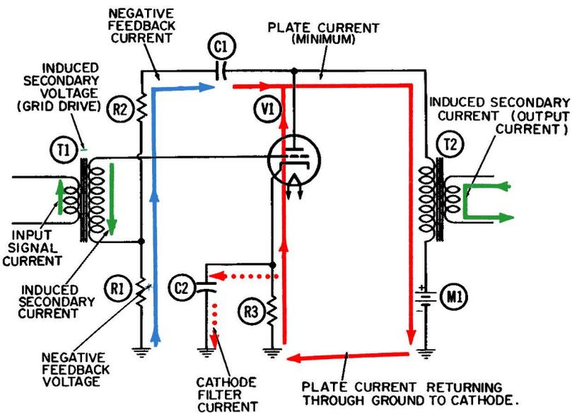
Fig. 3-8. Negative feedback amplifier circuit—second half-cycle.
