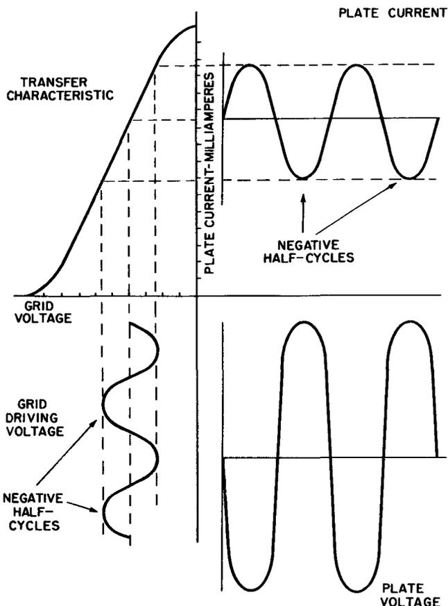
Fig. 2-3. Grid and plate waveforms for an R-C coupled audio amplifier.
