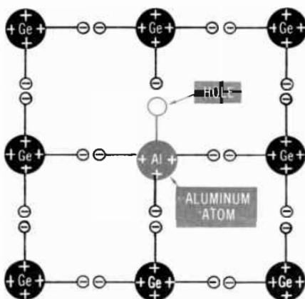
**Fig. 3-9.** Germanium doped with aluminum.
