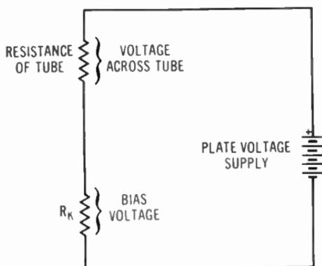
and the dc plate resistance of the tube. The plate voltage as seen by the tube is only that part of the supply voltage appearing across the plate resistance. Therefore, the plate-voltage supply must provide the bias voltage in addition to the plate voltage.
