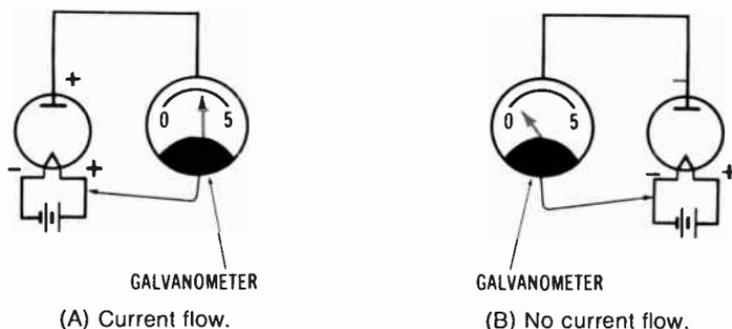
**Fig. 1-10. Circuit for demonstrating unidirectional conduction of a diode.**
