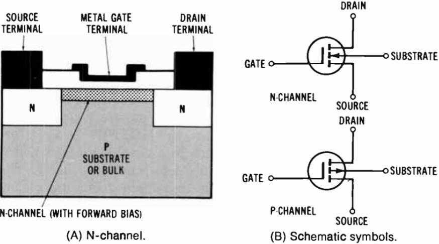
**Fig. 8-5. Enhancement type MOSFET.**
