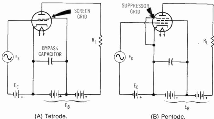
**Fig. 5-5. Amplifiers with multigrid tubes.**
