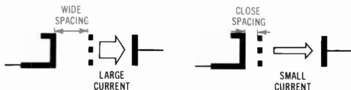
Fig. 2-5. Effect of cathode-grid distance on plate current.
