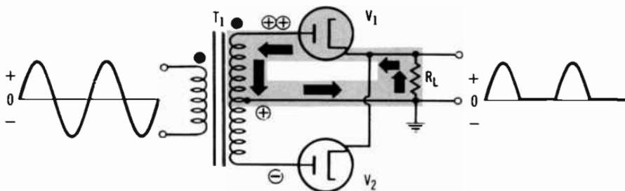
Fig. 4-11. Full-wave rectifier (positive half cycle).
