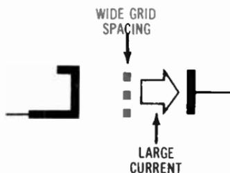
Fig. 2-6. Effect of wide grid spacing on plate current.
