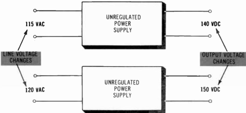
**Fig. 4-7. Unregulated power-supply action.**
