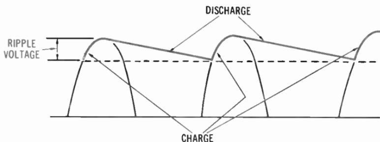
**Fig. 4-18. Capacitive filter charge and discharge.**
