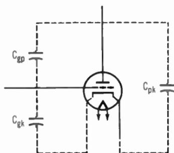
Fig. 2-21. Triode interelectrode capacitances.
