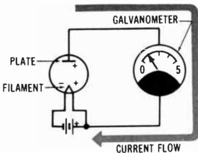
Fig. 1-9. Circuit for demonstrating Edison effect.
