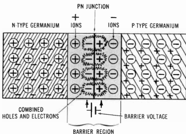
**Fig. 3-15. Action in a pn junction.**
