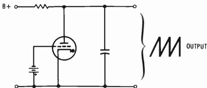
Fig. 7-6. A thyatron sawtooth generator.
