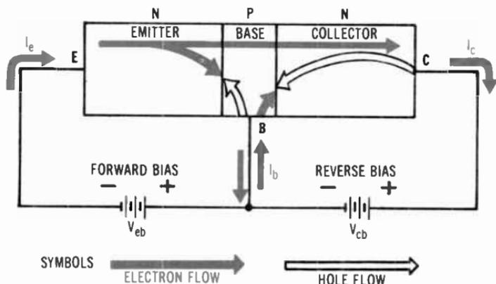
**Fig. 3-23. Current in a biased npn transistor.**
