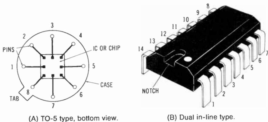
**Fig. 8-21. Pin numbering systems.**
