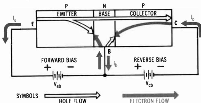
**Fig. 3-24.** Current in a biased pnp transistor.
