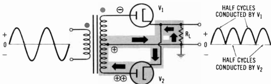
**Fig. 4-12. Full-wave rectifier (negative half cycle).**
