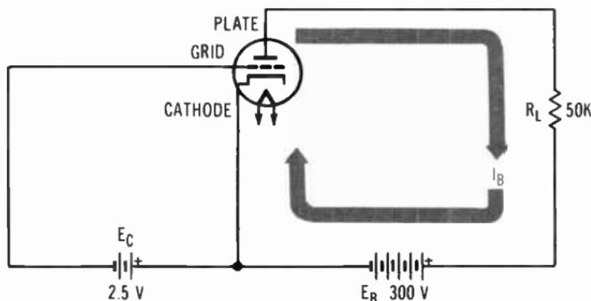
Fig. 5-2. Basic triode amplifier circuit.
