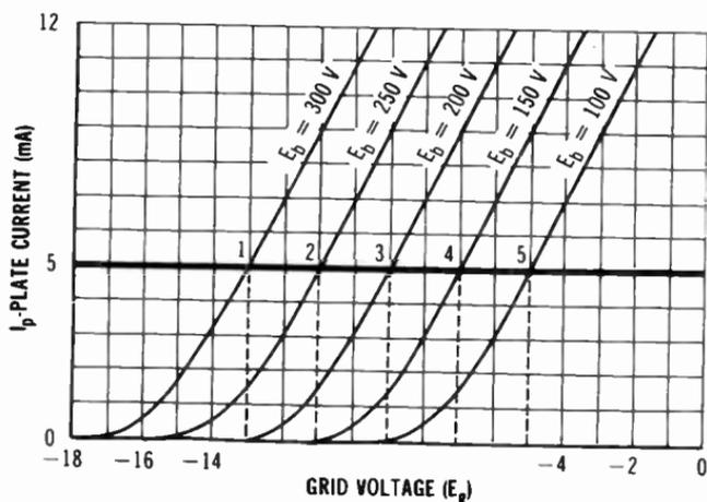
Fig. 2-13. Grid family of characteristic curves.
