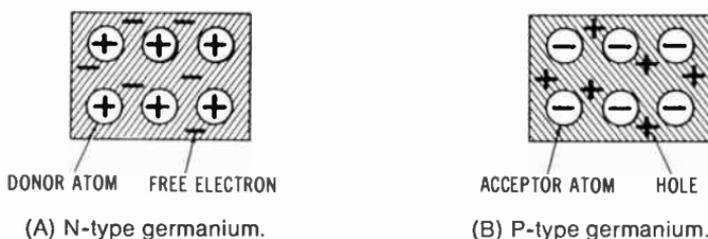
**Fig. 3-14. Doped germanium is electrically neutral.**
