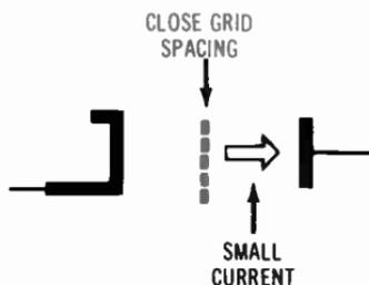
Fig. 2-7. Effect of close grid spacing on plate current.
