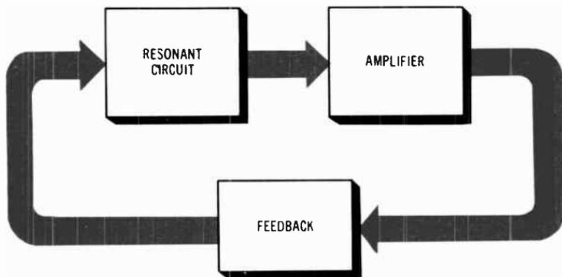
**Fig. 5-22. Feedback oscillator.**
