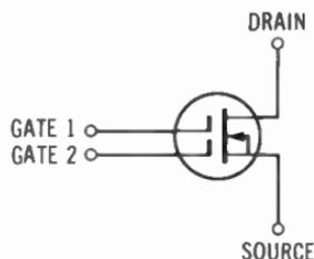
(B) Schematic symbol (includes substrate and case).
