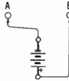
**A1-3.** The battery should be connected as shown.
