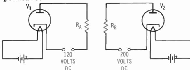
Q1-23. Moving the plate away from the cathode (increases, decreases) the current flow through the diode.
