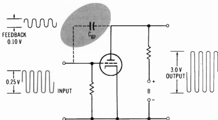
**Fig. 2-23.** Effects of grid-plate capacitance at a higher frequency.
