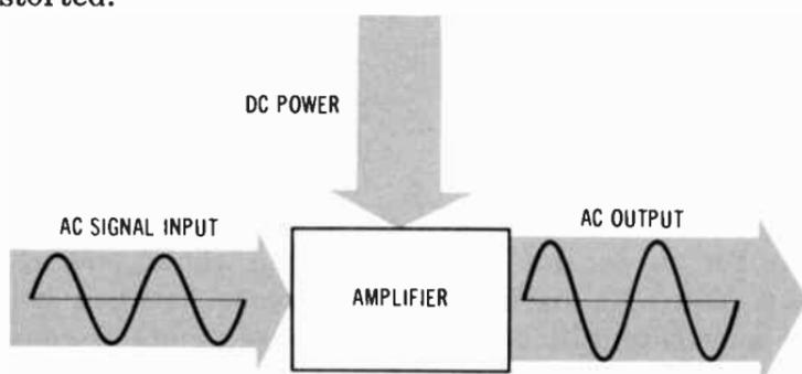
**Fig. 5-1. Basic amplifier principle.**
