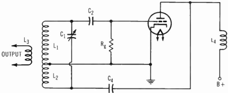
**Fig. 5-23. Shunt-fed Hartley oscillator.**
