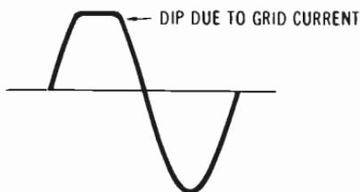
**Fig. 5-6. Distorted plate-current waveform.**
