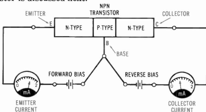
Fig. 3-22. Bias for npn transistor amplifier.
