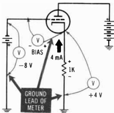
Fig. 2-19. Measuring bias voltage.
