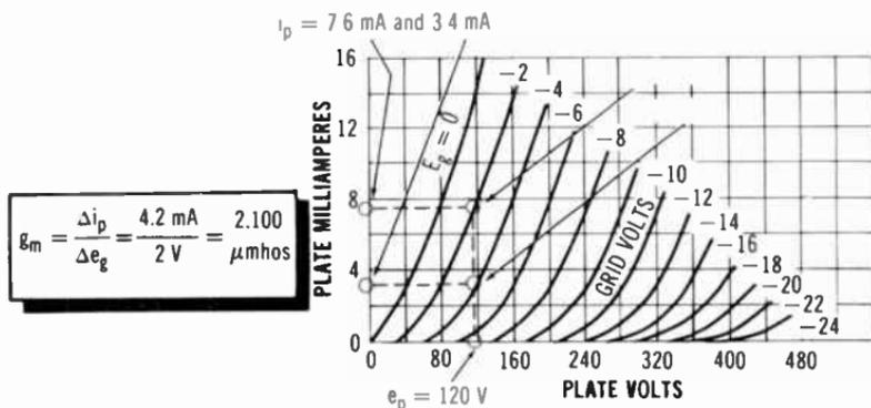
**A2-35.** Grid bias is the difference in potential between the grid and the cathode (not cathode to grid).
