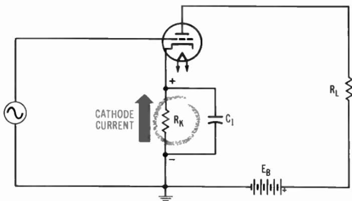
Fig. 5-12. Circuit using cathode-bias resistor.
