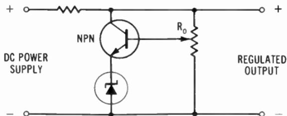
**Fig. 4-25. Shunt-type voltage regulator.**
