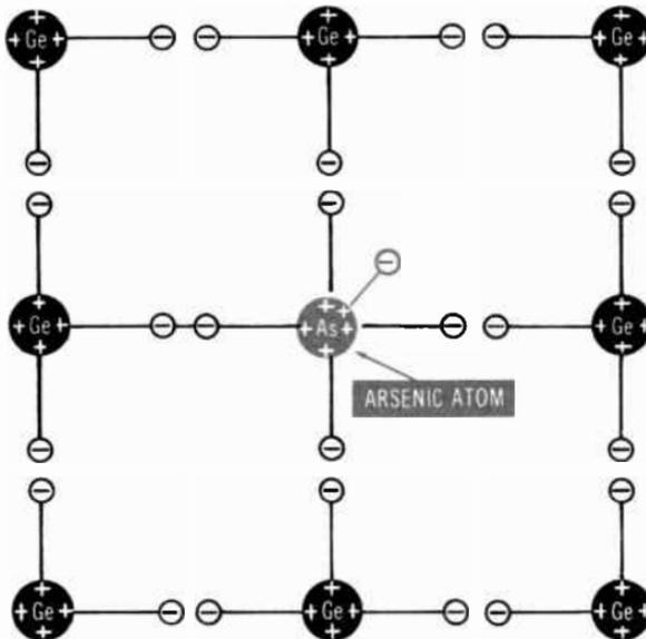
**Fig. 3-7. Germanium doped with arsenic.**
