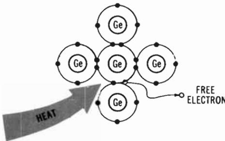
Fig. 3-4. Covalent bond broken by heat.
