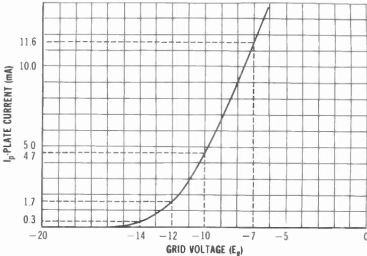
Fig. 2-12. Triode plate current versus grid voltage.
