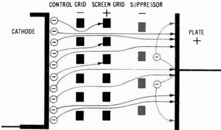
**Fig. 2-27. Action of a suppressor grid.**
