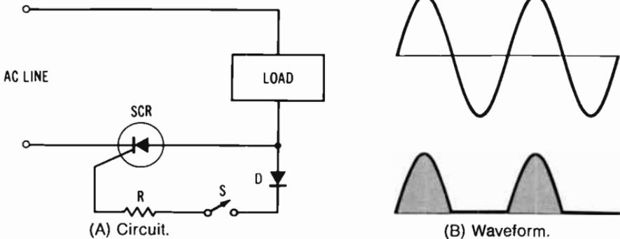
Fig. 8-15. Use of SCR to control ac load and waveform.
