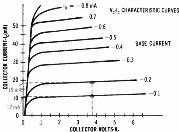
$$\beta = \frac{\Delta I_c}{\Delta I_b} = \frac{19 - 12 \text{ mA}}{0.2 - 0.1 \text{ mA}} = \frac{7 \text{ mA}}{0.1 \text{ mA}} = 70$$
