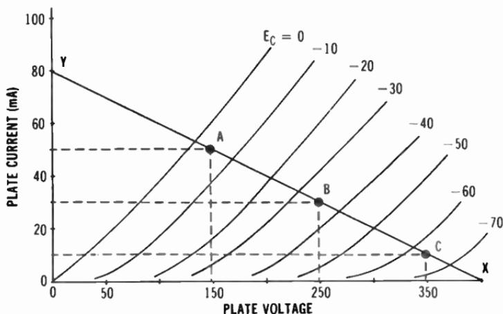
**Fig. 5-9.** Points on a load line.
