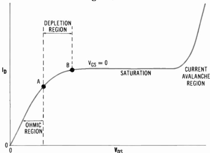
Fig. 8-7. JFET response curve, zero gate-source bias.
