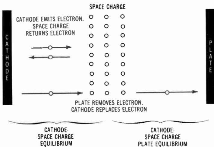
**Fig. 1-17. Two equilibrium conditions in a diode.**
