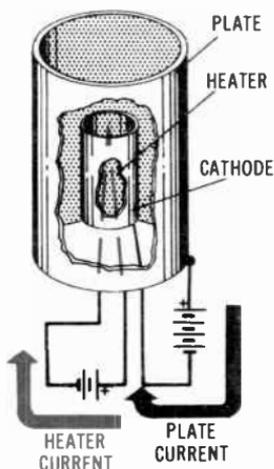
(A) Indirectly heated cathode.
