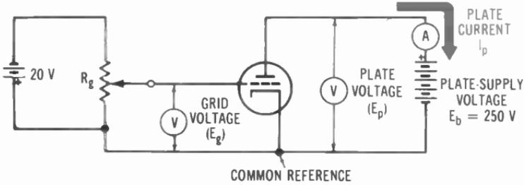
Fig. 2-11. Circuit to obtain data for triode characteristic curve.
