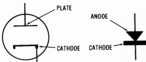
**Fig. 3-12. Comparison of diodes.**
