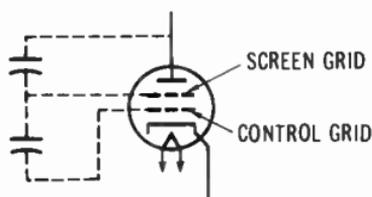
**Fig. 2-24.** Grid-plate capacitances in a tetrode.
