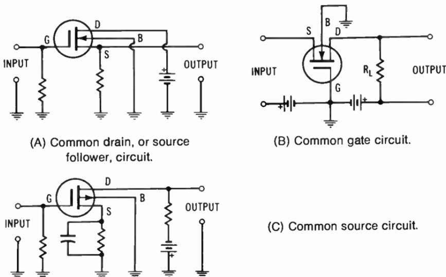
Fig. 8-6. Basic MOSFET circuits.
