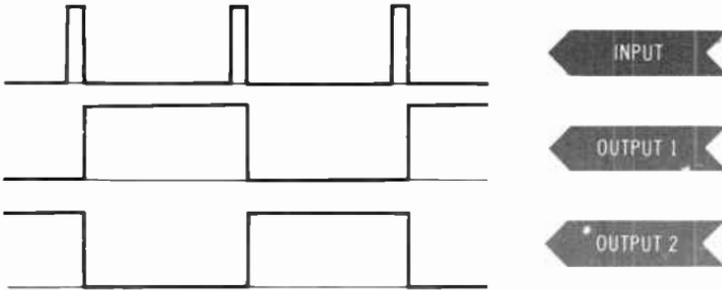
**Fig. 7-12. Bistable-multivibrator pulses.**
