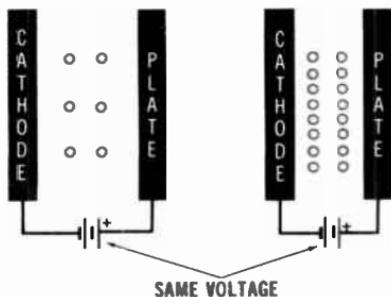
Fig. 1-14. Current flow is affected by tube-element spacing.
