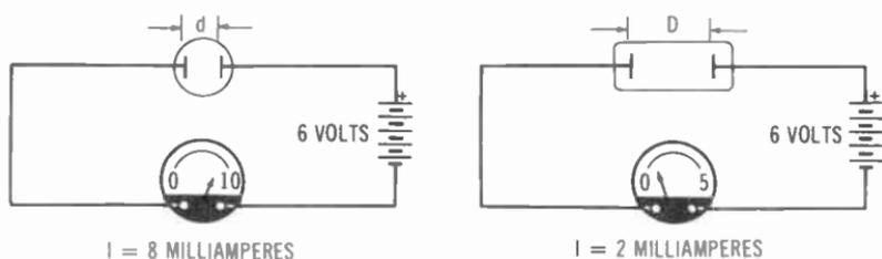
**Fig. 1-3. Variation of current with plate spacing.**
