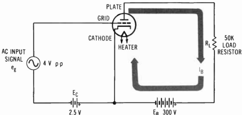
Fig. 5-3. Amplifier with input signal.
