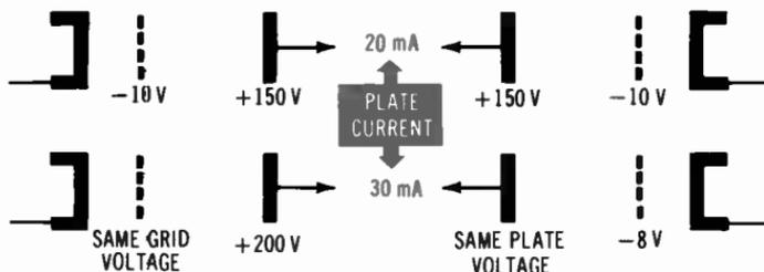
**Fig. 2-9. Relative effects of changes in grid and plate voltage.**
