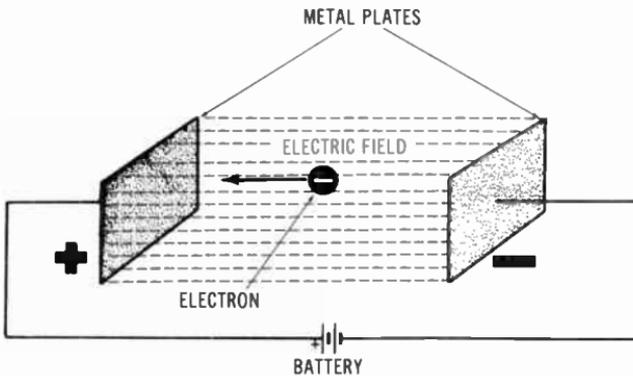
Fig. 1-1. Electron movement in an electric field.
