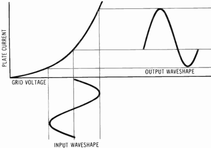
**Fig. 5-7. Distortion due to nonlinear operation.**
