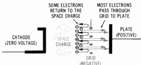
Fig. 2-4. Electron movement in a triode.
