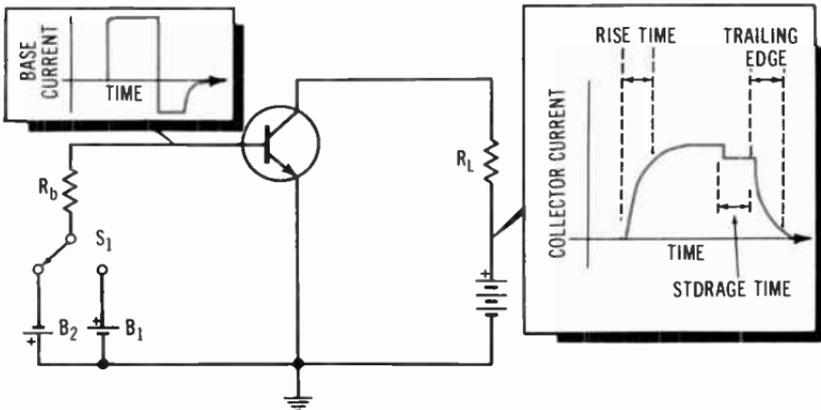
**Fig. 7-2. Transient response of a circuit.**
