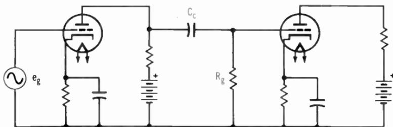
**Fig. 5-14. Resistance-capacitance coupled amplifier.**
