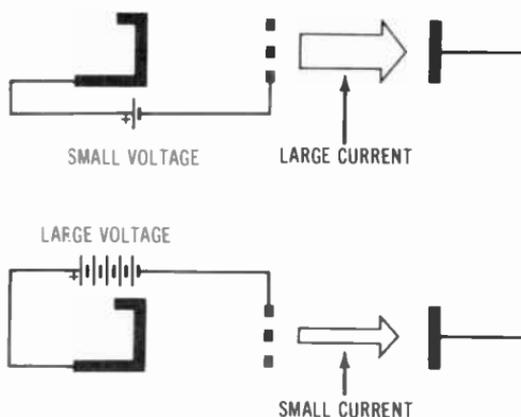
Fig. 2-8. Effect of grid voltage on plate current.
