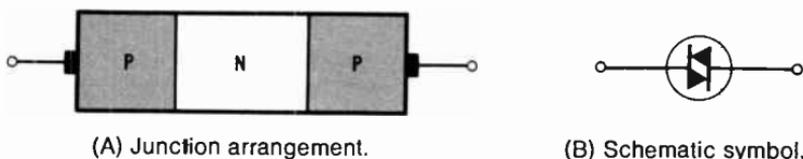
Fig. 8-19. Diac junction arrangement and symbol.
