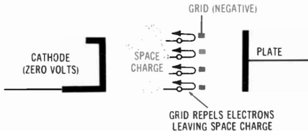
Fig. 2-3. Effect of the grid in a triode.
