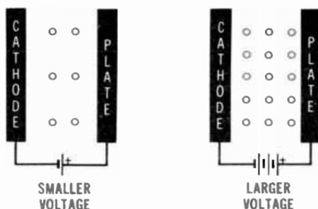
**Fig. 1-13.** Current flow is affected by plate voltage.
