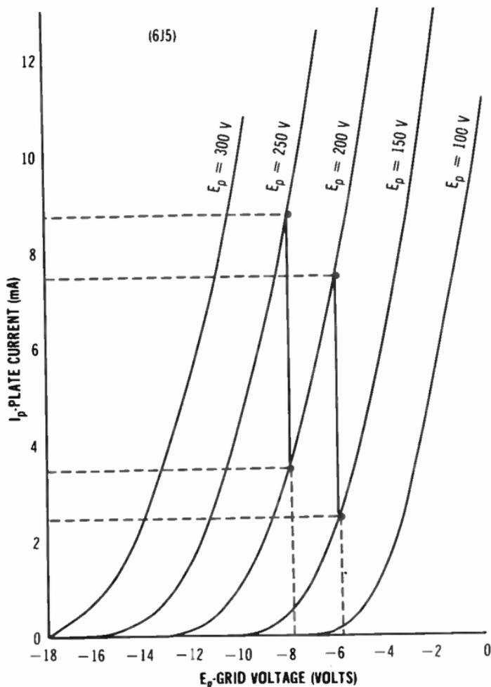
Note that these values (9,259, 10,000, and 9,090 ohms) are all fairly close to each other. When compared to the changes in  $R_p$  (from thousands of ohms to hundreds of thousands of ohms), the ac plate resistance ( $r_p$ ) may be considered almost a constant for a particular triode.
