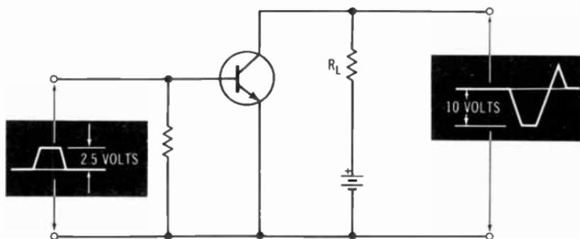
Fig. 7-3. A pulse-amplifier circuit.
