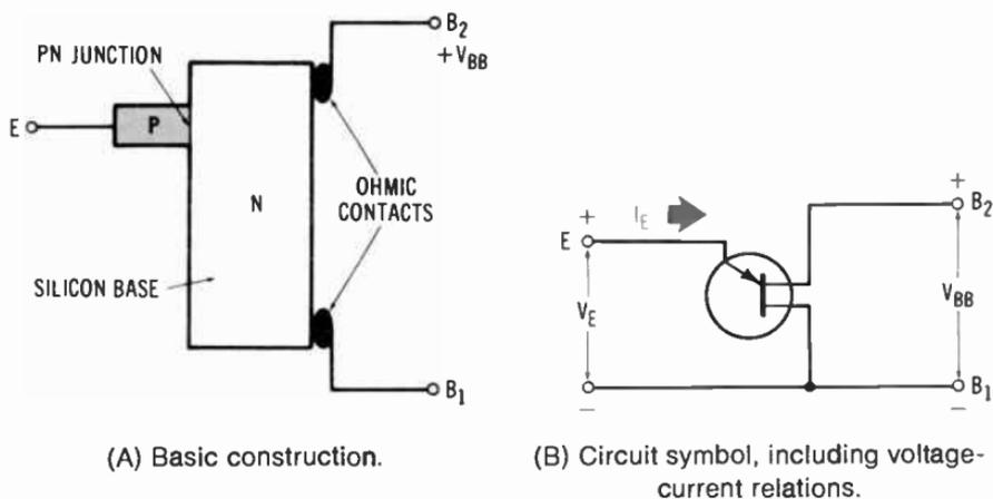
Fig. 8-10. Basic construction of unijunction transistor.
