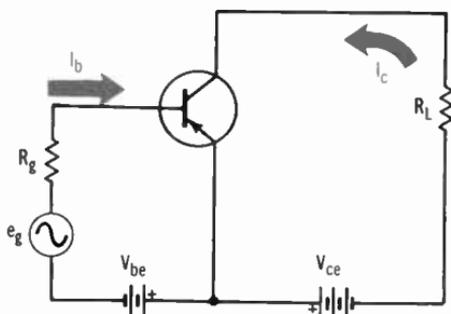
The voltage across load resistance  $R_L$  (which is a separate property of the circuit) is  $\Delta I_c R_L$ , where  $\Delta I_c$  is the signal current in the collector circuit. The term  $R_c$  (collector resistance) is often used interchangeably with  $R_L$ .
