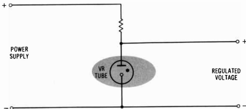
**Fig. 4-23. Simple vr-tube voltage regulator.**
