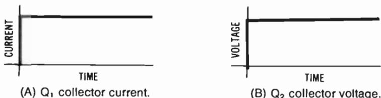
**Fig. 7-8. Ideal switching in a multivibrator.**
