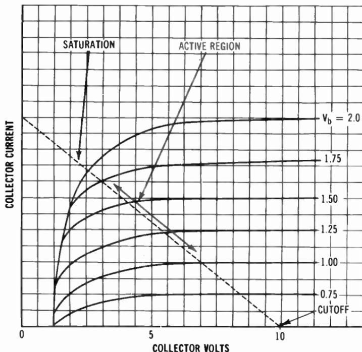
Fig. 7-4. Transistor characteristic curves.
