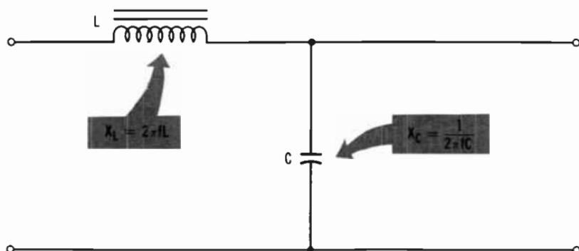
Fig. 4-20. L-section filter with series inductor.
