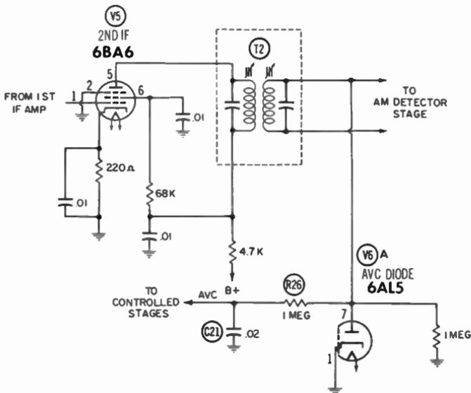
Fig. 3-16. An AVC system employing a separate rectifier tube.
