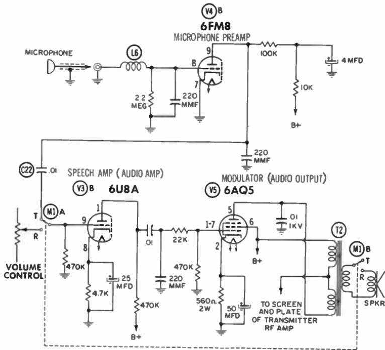
Fig. 3-21. The transmitter audio-amplifier section.
