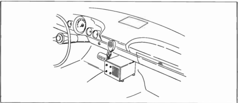
*Fig. 5-7. A floor mounting can be used if no space is available under the dash.*
