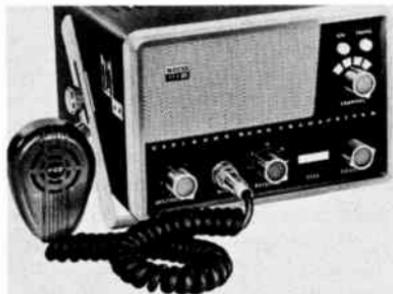
*Fig. 2-16. The EICO Model 772 Class-D transceiver is available in kit or factory-assembled form. It features a crystal-controlled transmitter and superhetrodyne receiver with automatic noise-limiter and squelch.*
