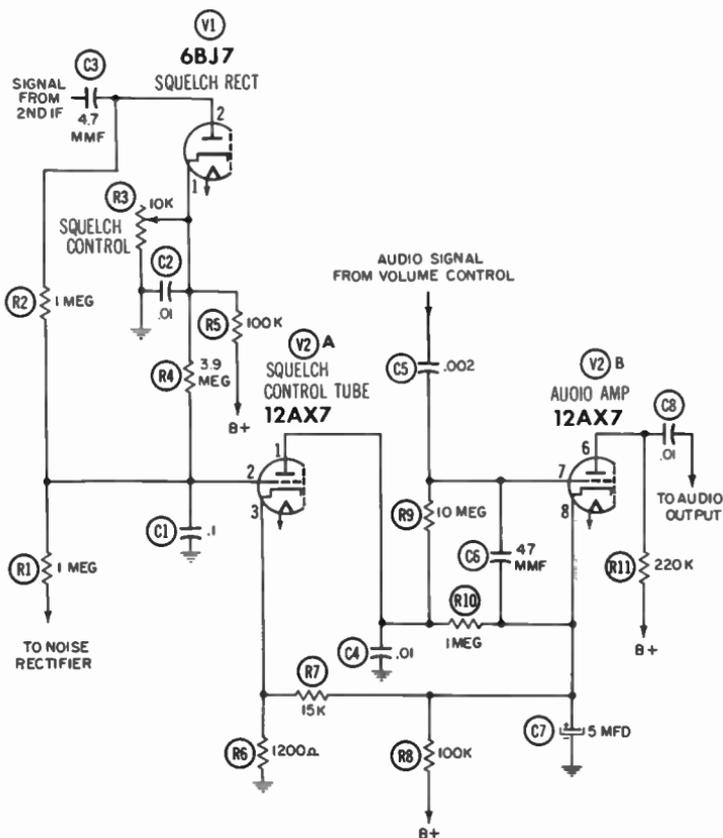
Fig. 3-17. A typical signal-operated squelch circuit.
