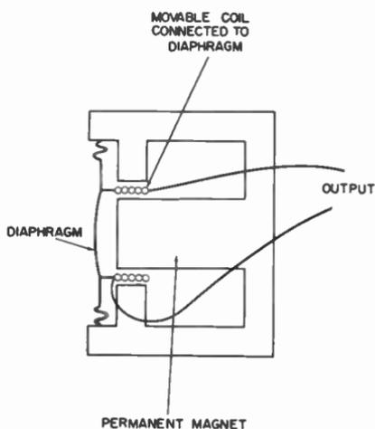
Fig. 2-25. Cross-sectional view of a dynamic microphone.
