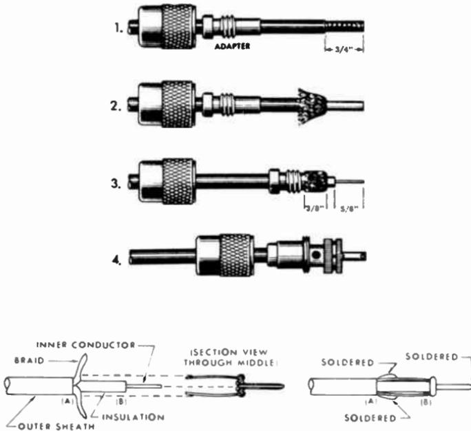
Fig. 5-3. Two methods of fastening the antenna connector to the cable.
