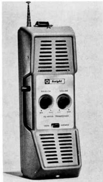
*Fig. 2-17. The Knight-Kit Model KG-4000A all-transistor Class-D walkie-talkie employs a crystal-controlled transmitter and superhet receiver with adjustable squelch and an automatic noise limiter.*
