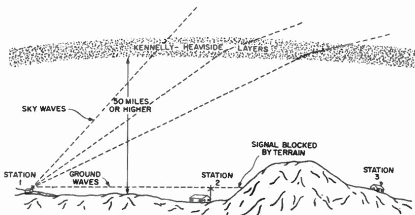
Fig. 4-4. Characteristics of ultra-high frequency (UHF) signals.
