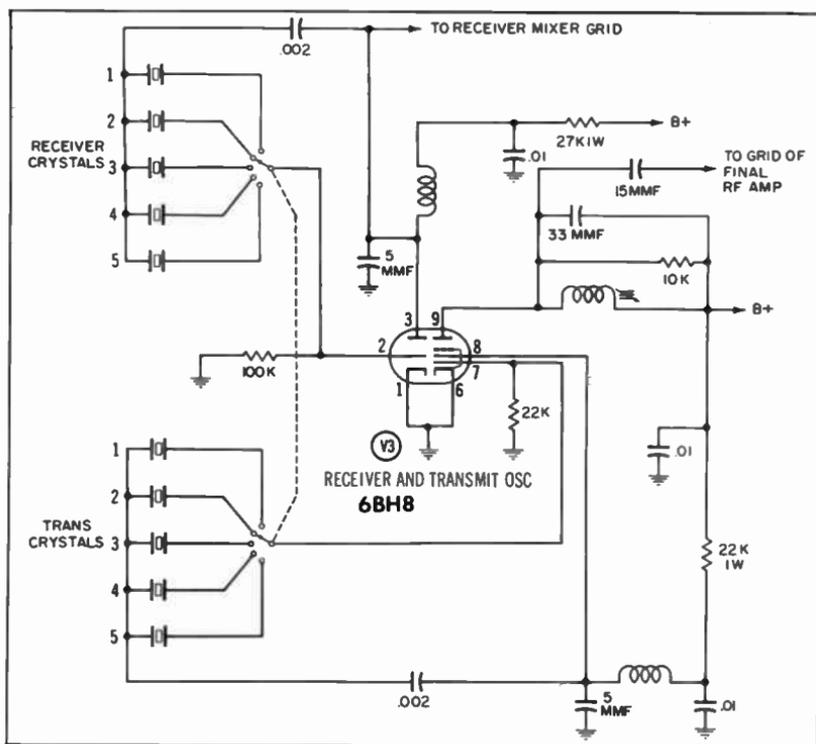
Fig. 3-23. A circuit incorporating the transmitter and receiver oscillators in the same tube.
