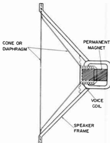
Fig. 2-26. Cross-sectional view of a PM dynamic speaker.
