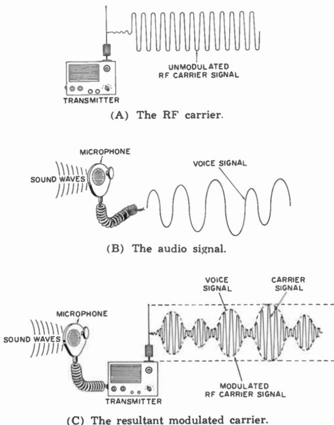
Fig. 8-4. Producing an amplitude-modulated carrier.
