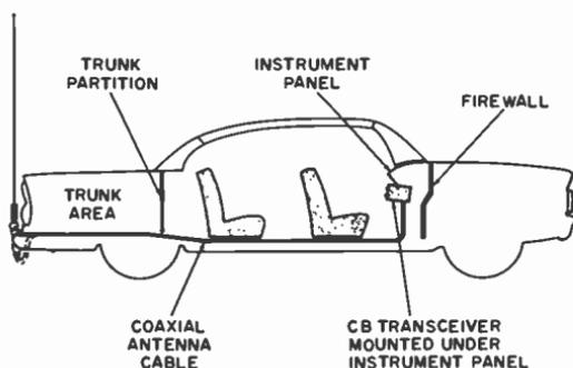
Fig. 5-8. One method of routing the antenna cable in an automobile installation.
