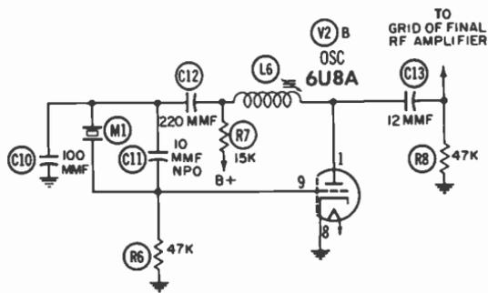
Fig. 3-22. A crystal-controlled transmitter oscillator circuit.
