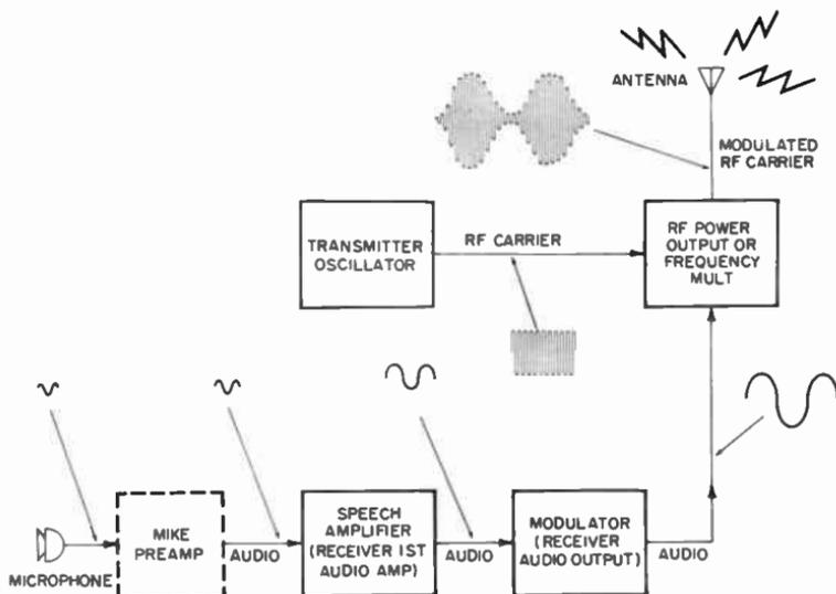
Fig. 3-20. Functional block diagram of a typical Class-D transmitter.
