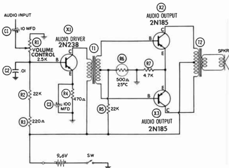
Fig. 3-14. A typical transistorized push-pull audio-output circuit.
