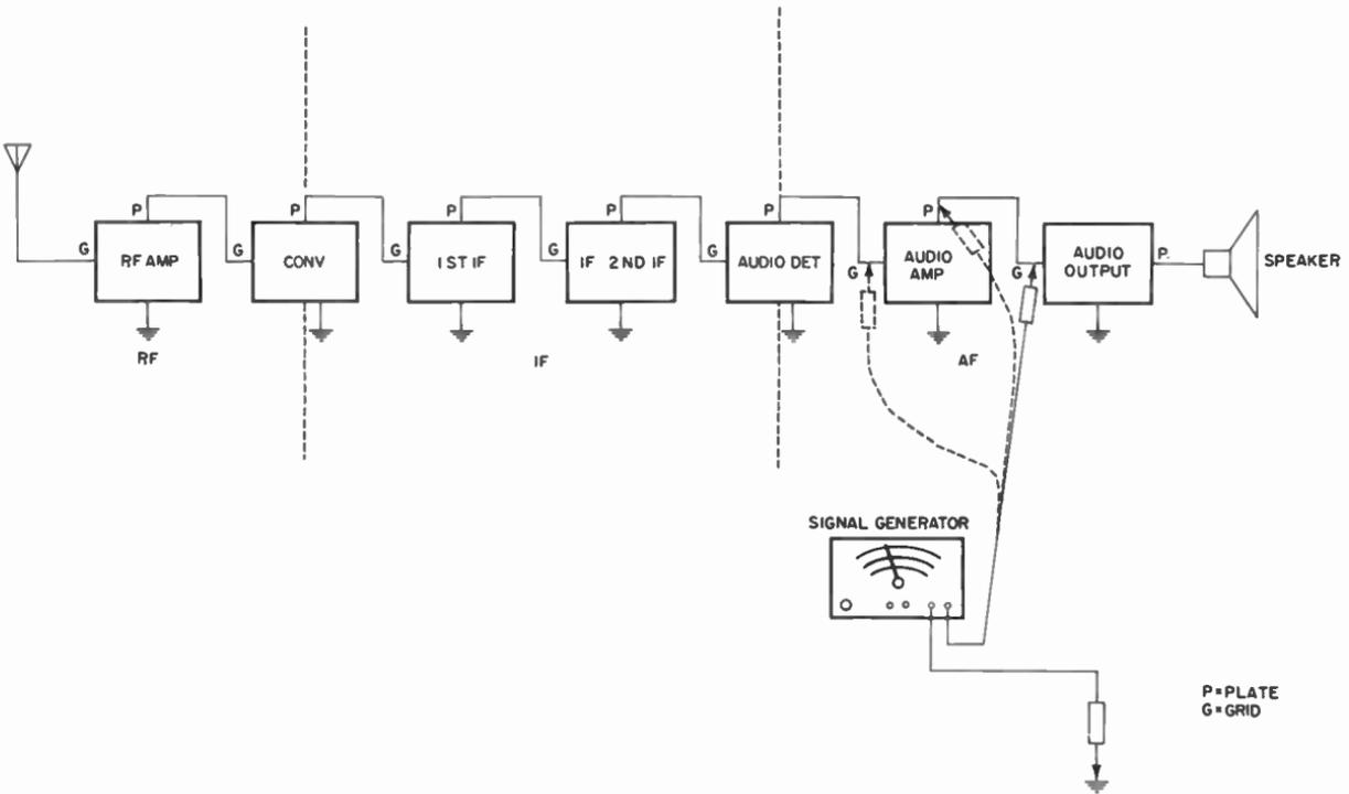
Fig. 6-10. Method of localizing a defective stage by signal injection.
