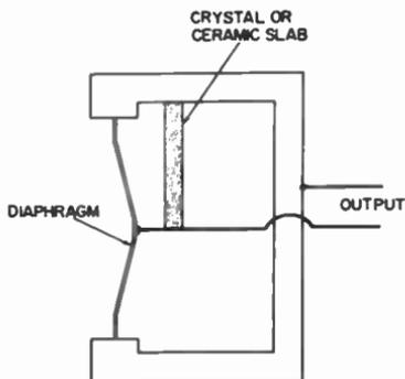
Fig. 2-27. Basic construction of a crystal or ceramic microphone.
