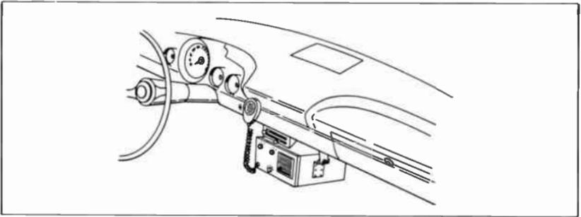
*Fig. 5-6. Suitable brackets permit transceiver to be mounted below interfering objects.*
