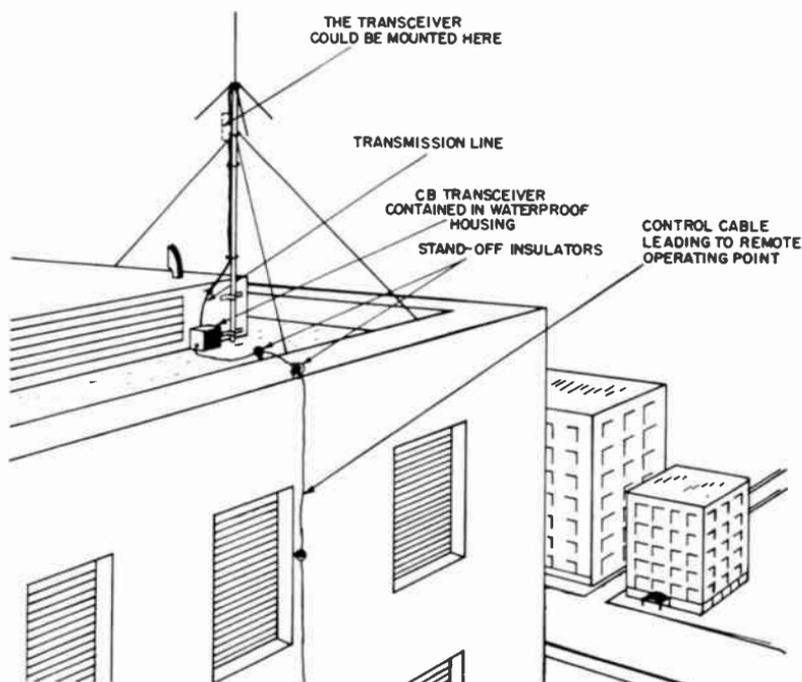
Fig. 4-17. A remote transceiver installation.
