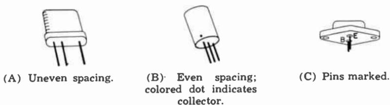
Fig. 6-7. Methods of identifying transistor leads.
