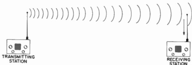
Fig. 4-1. Electromagnetic waves from the transmitter induce similar waves in the receiving antenna.
