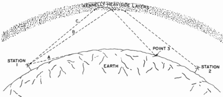
Fig. 4-3. Characteristics of high-frequency (HF) signals.
