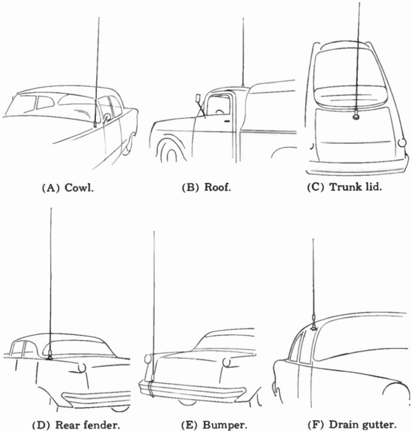
Fig. 4-18. Typical mobile whip mounting locations.
