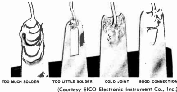
Fig. 3-8. Properly soldered connections are a must in kit construction
