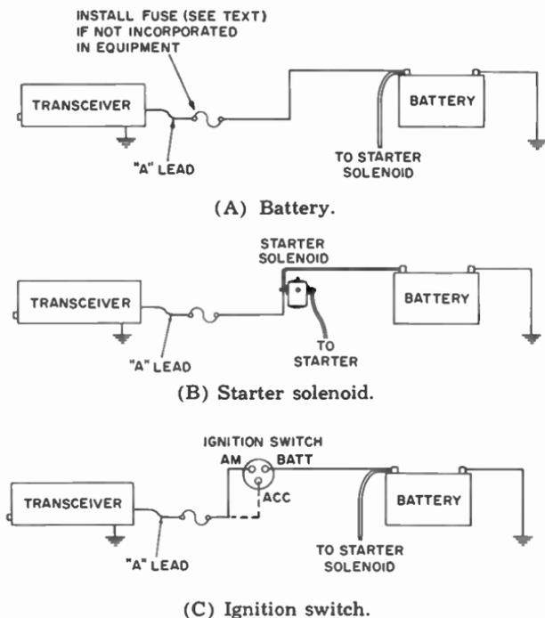
Fig. 5-9. Various points where a transceiver can be connected to the automobile source voltage.
