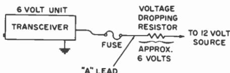
Fig. 5-10. Method of connecting a 6-volt transceiver to a 12-volt source.
