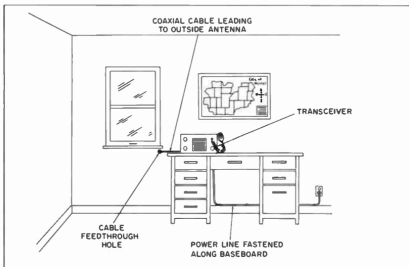
Fig. 5-1. A typical Class-D fixed-station installation.
