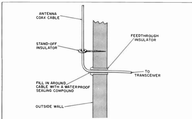
Fig. 5-2. Method of feeding the antenna cable through a wall.
