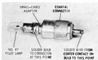
*Fig. 6-9. A home-made dummy antenna made from a PL259 connector and a No. 47 pilot lamp.*
