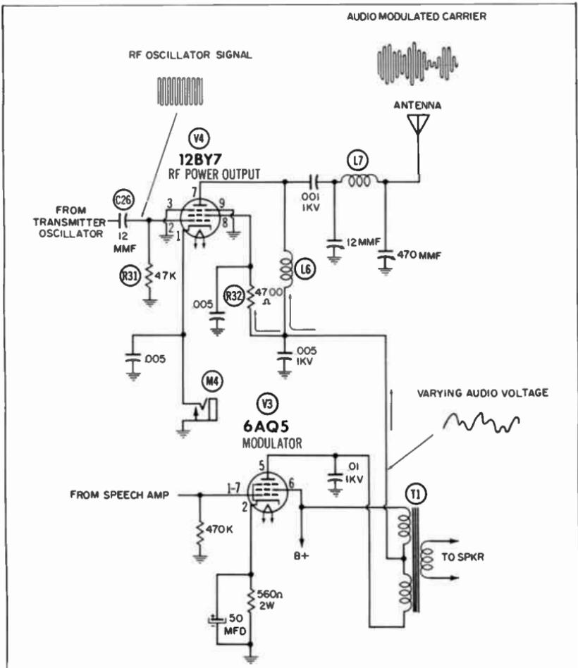
Fig. 3-24. A typical RF power-output stage.
