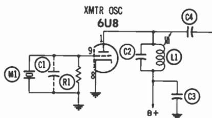
Fig. 7-3. Crystal-oscillator circuit.
