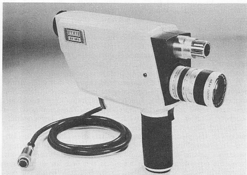
Fig. 2-13. An unusually compact color camera with electronic viewfinder.
