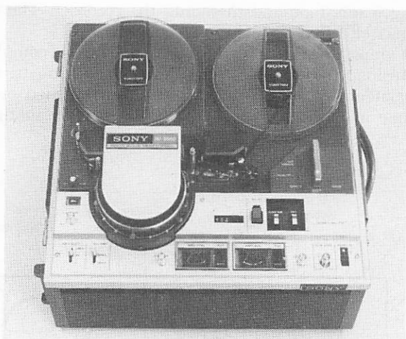
Fig. 5-12. A color ac-operated model that uses \frac{1}{2} -inch tape.
