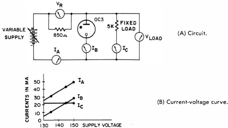
Fig. 2-9. Regulator circuit action when load is fixed and the source voltage is variable.
