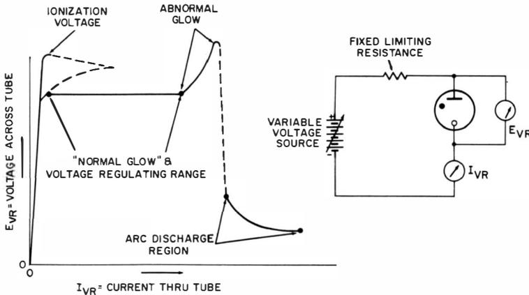
Fig. 2-3. The voltage-current characteristics of a gaseous VR tube.
