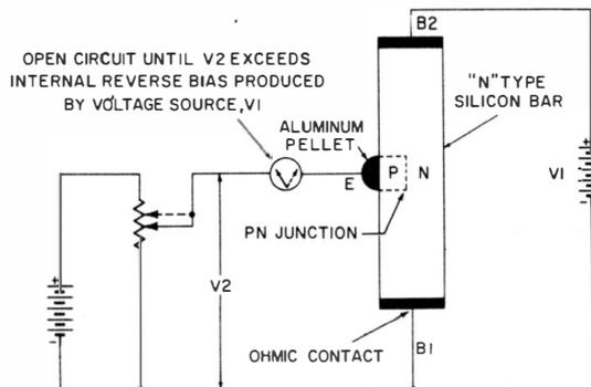
Fig. 6-7. Circuit for demonstrating switching of conductive states in unijunction transistors.
