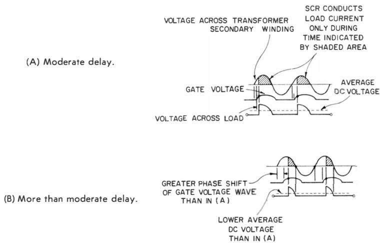
Fig. 6-5. Effect of gate firing-voltage delay on average DC output of circuit in Fig. 6-4.
