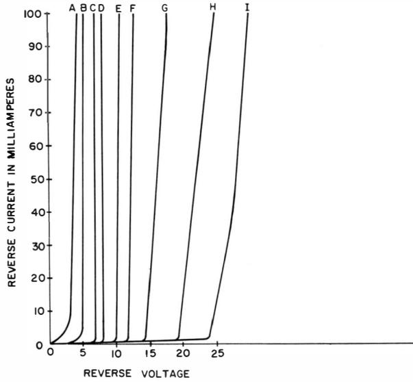
**Fig. 3-3. General trend of reverse-conduction characteristics for zener diodes with different breakdown voltages.**
