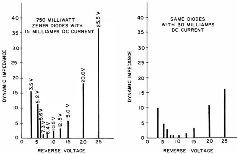
**Fig. 3-4. Effect of operating current on dynamic impedance of various zener diodes.**
