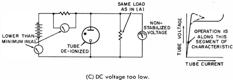
Fig. 2-8. Effects of source voltage variations on voltage-regulator circuit.
