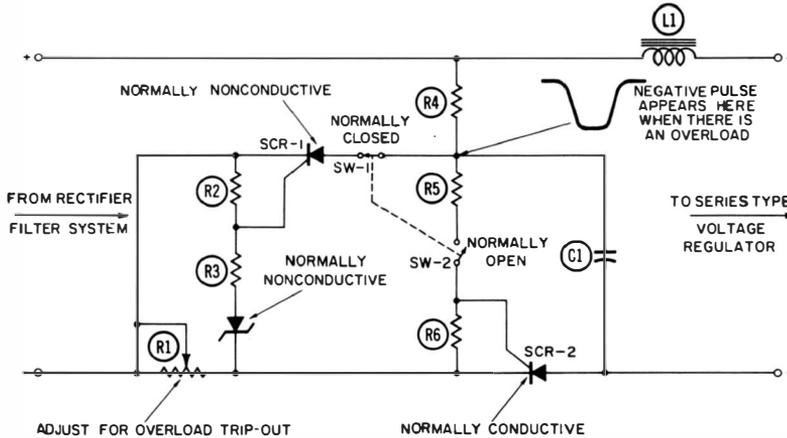
Fig. 6-17. SCR protective circuit diagram.
