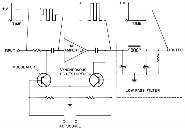
Fig. 6-2. Basic configuration of a transistor chopper.
