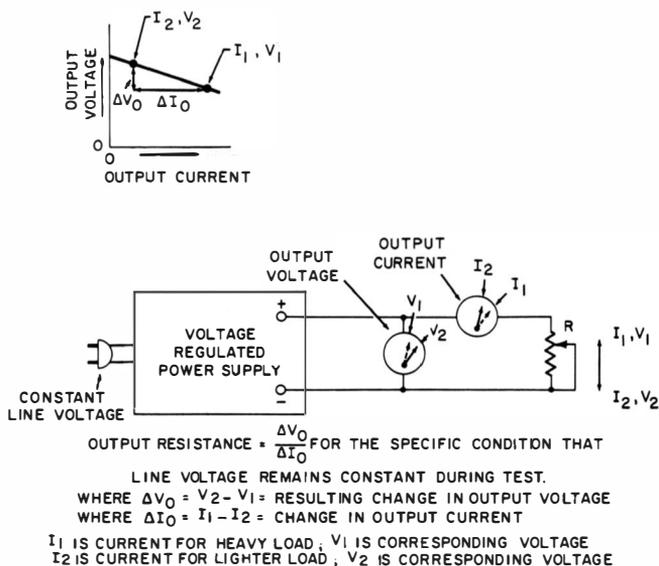
Fig. 1-4. Test setup for illustrating concept of output resistance.
