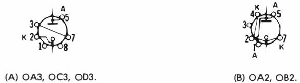
Fig. 1-20. Voltage-regulator tube pin connections.
