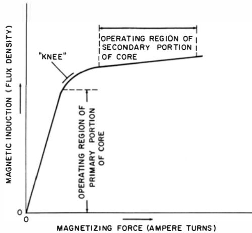
Fig. 1-16. Curve showing operating regions of primary and secondary core sections in a static-magnetic regulating transformer.
