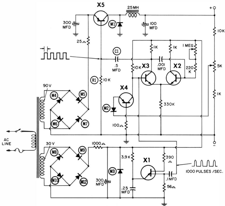
Fig. 6-13. Schematic of typical DC switching-type voltage regulator with an 80-volt, 500-milliampere output rating.
