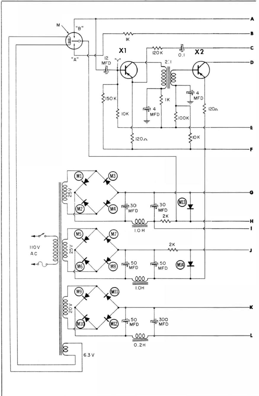
Fig. 6-1. A chopper stabilized voltage regulator
