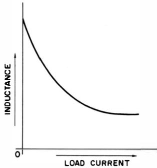
Fig. 1-24. Graph showing inductance versus load current of a swinging choke.
