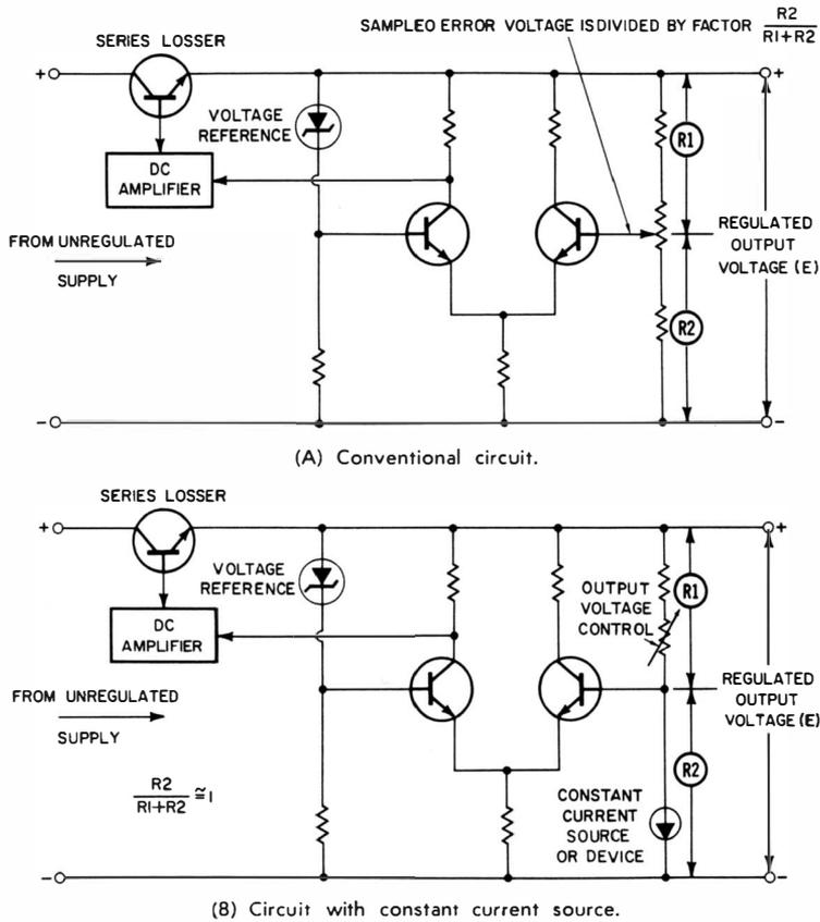
**Fig. 4-10. Simplified sampler/comparator circuits showing advantage of constant current source in comparator section.**
