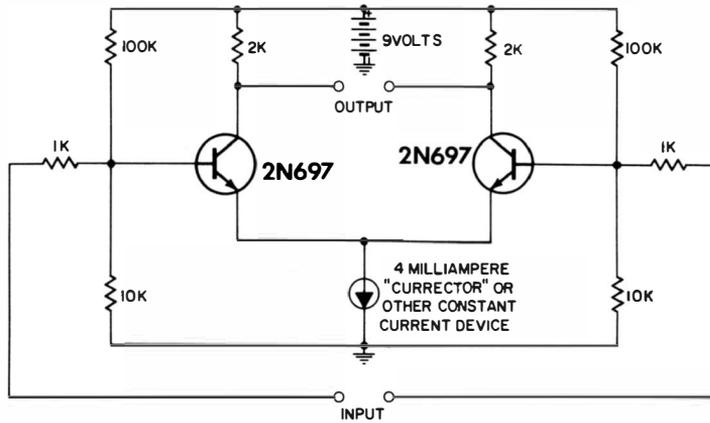
Fig. 4-7. Representative differential amplifier with constant current source in place of resistance.
