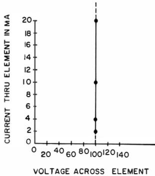
(C) Curve in B turned around to indicate current as function of voltage.
