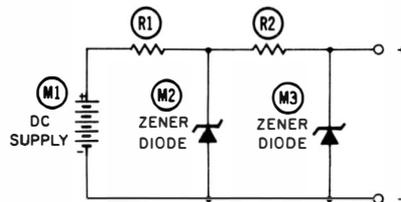
bilization voltage of about 25 volts. The dynamic impedance of the combination will be approximately the same as for a single diode, but the permissible power dissipation will be three times as much. Any number of low-impedance diodes can be series-connected to provide stabilization at a higher voltage.
