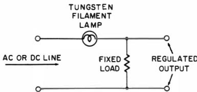
Fig. 1-11. Regulation against line-voltage variations by means of a series varistor.
