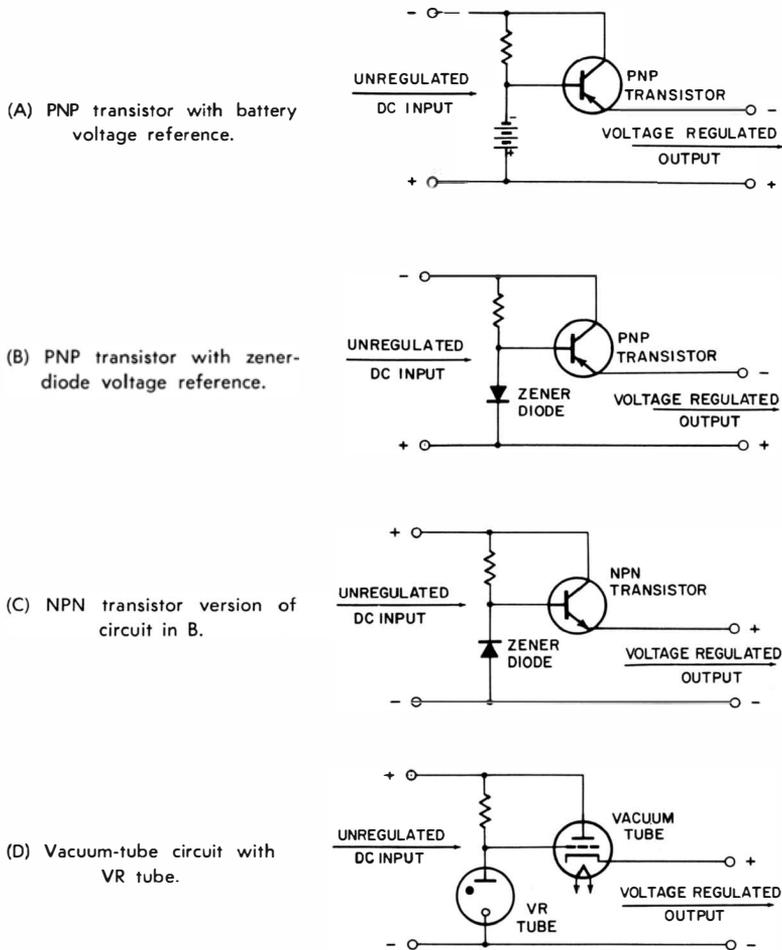
Fig. 4-1. Basic emitter- or cathode-follower voltage-regulator circuits.
