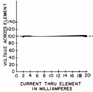
(B) Voltage as function of current through element.
