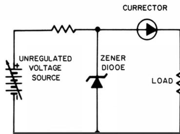
Fig. 4-9. Improvement of current regulation by means of zener diode preceding the Currector element.
