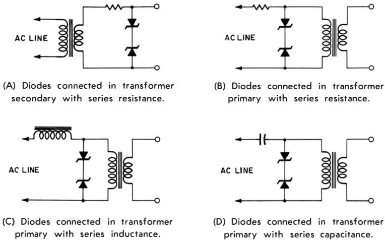
**Fig. 3-7. Methods of obtaining AC regulation with zener diodes.**
