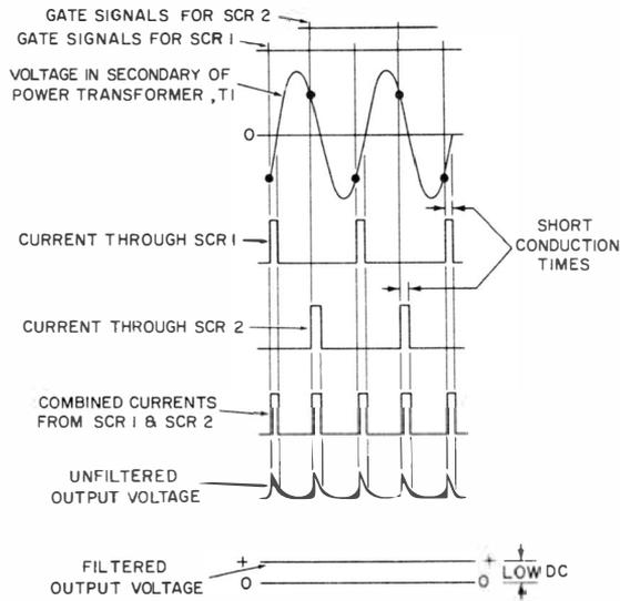
**Fig. 6-10. Conditions in circuit of Fig. 6-9 when phasing of gate signal allows short conduction time.**
