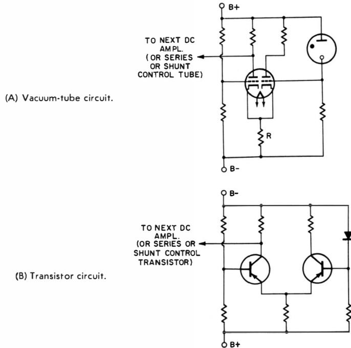
Fig. 4-12. Typical examples of differential amplifiers with input voltage reference connected to one input.
