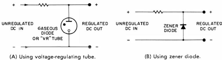
Fig. 2-1. Shunt-type voltage-regulator circuits.
