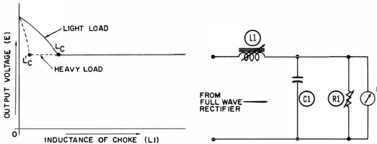
Fig. 1-25. Graph showing the effect of choke inductance on the output voltage for light or heavy loads.
