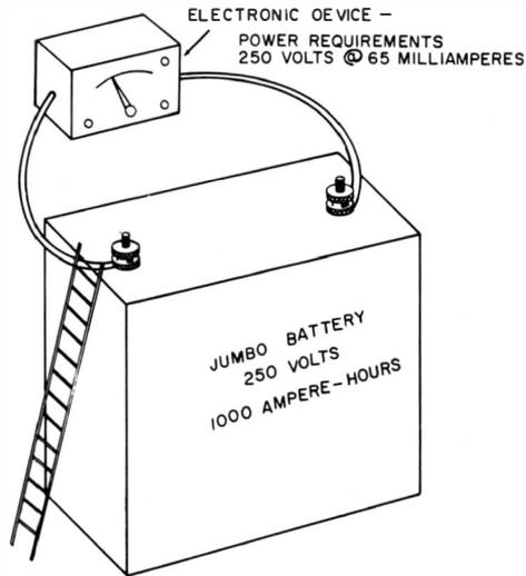
**Fig. 1-5. A voltage-regulated power supply appears to the load as a tremendous source of current, although actually it is not.**
