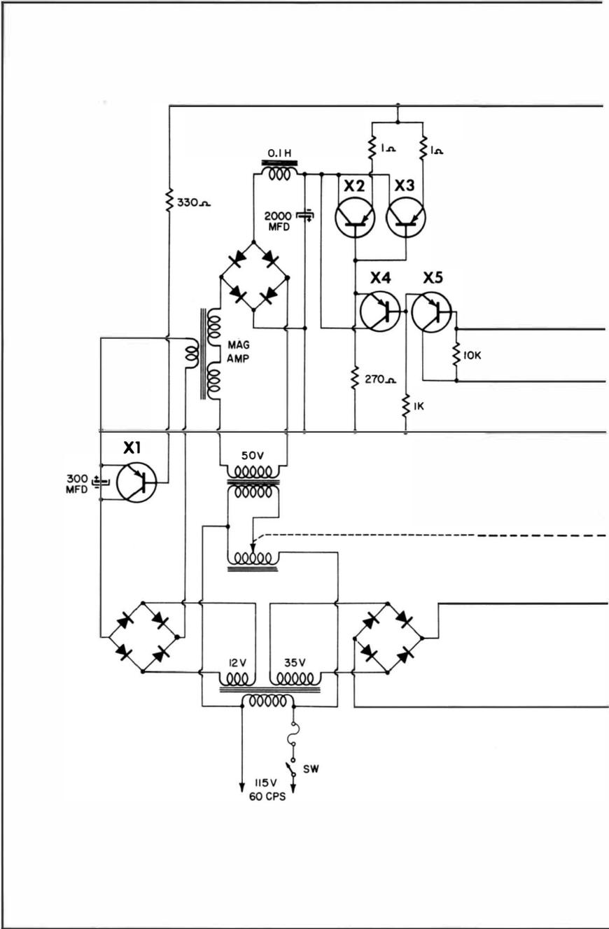
Fig. 5-6. A transistorized series regulator with
