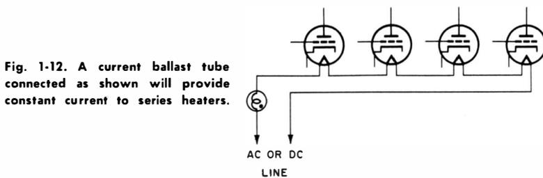
Fig. 1-12. A current ballast tube connected as shown will provide constant current to series heaters.
