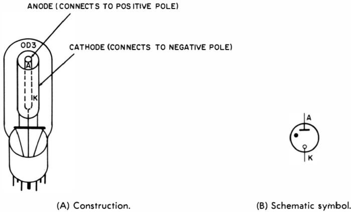
Fig. 1-19. The voltage-regulator tube.
