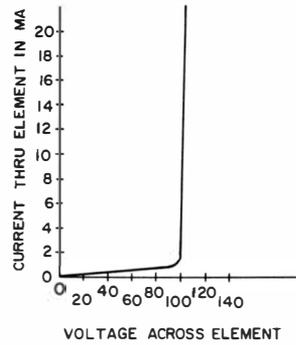
(D) Curve of zener diode or gaseous VR tube.
