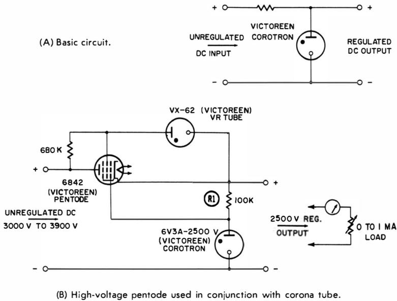
Fig. 2-14. High-voltage corona-tube regulator circuits.
