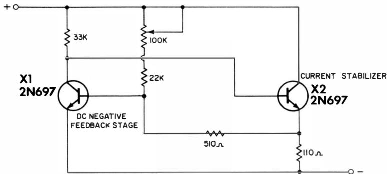
Fig. 4-5. Representative current regulator using DC negative feedback stage.
