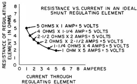
Fig. 1-21. Typical open-loop regulating circuit utilizing a shunt element to stabilize the output voltage.
