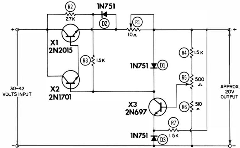
Fig. 6-15. Representative schematic of protective device with instant recovery feature.
