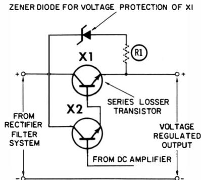
Fig. 6-16. Technique for over-voltage protection of the series losser transistor.
