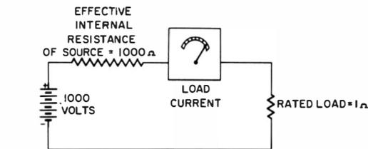
$$\text{LOAD CURRENT AT RATED LOAD} = \frac{1000}{1000+1} = .9990 \text{ AMP.}$$
