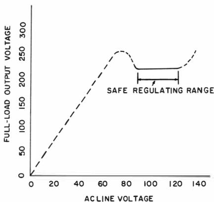
Fig. 1-8. The line-voltage range is an important consideration with regulated power supplies.
