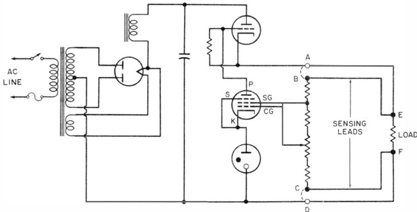
Fig. 5-8. Basic output-terminal arrangement for remote sensing.
