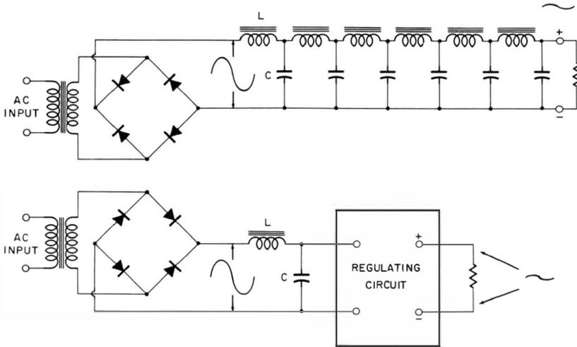
**Fig. 1-9.** The regulating circuit has a ripple smoothing ability equivalent to a complex network of filter elements.
