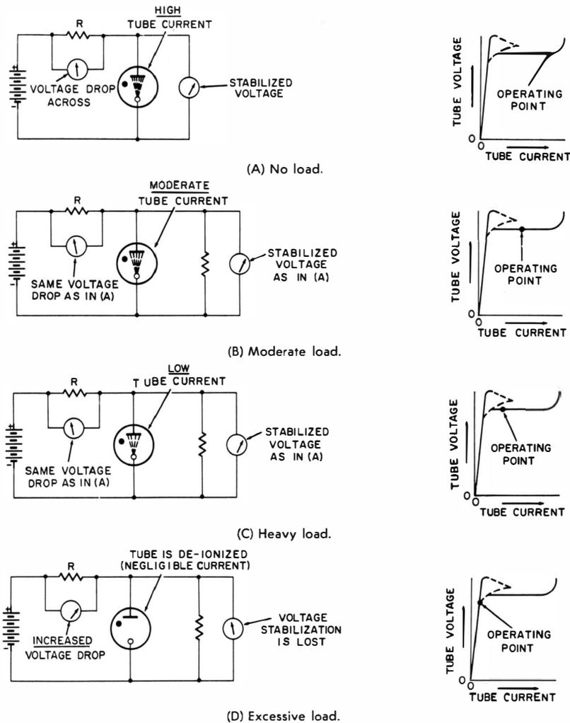
Fig. 2-5. Effect of various loads on regulator circuit voltages.
