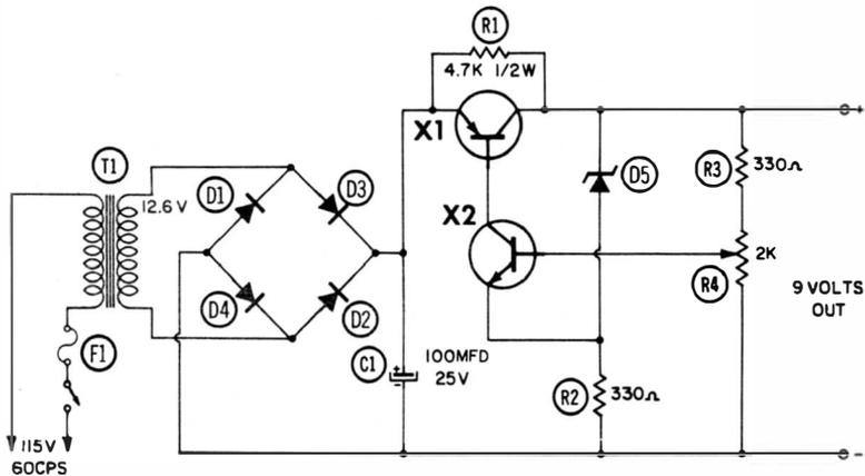
Fig. 5-11. Representative complementary symmetry voltage regulator power supply.
