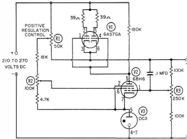
Fig. 5-9. A 180-volt, 150-milliampere voltage regulator that has provision for positive regulation.
