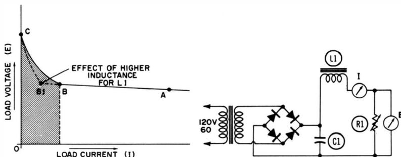
Fig. 1-23. Graph showing poor regulation region at low currents with choke input filter.
