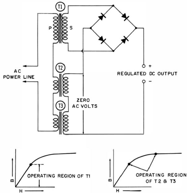
Fig. 1-18. A transformer regulating arrangement using the variable saturation method.
