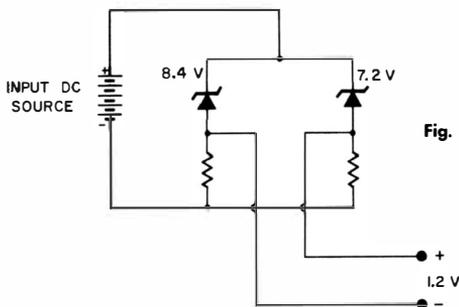
Fig. 3-6. Parallel network for obtaining low-voltage stabilization.
