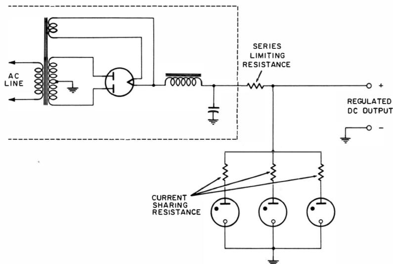
Fig. 2-11. Method of connecting VR tubes in parallel.
