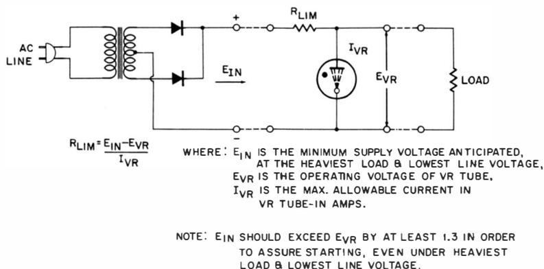
Fig. 2-4. Calculating the series limiting resistance of a shunt regulating circuit.
