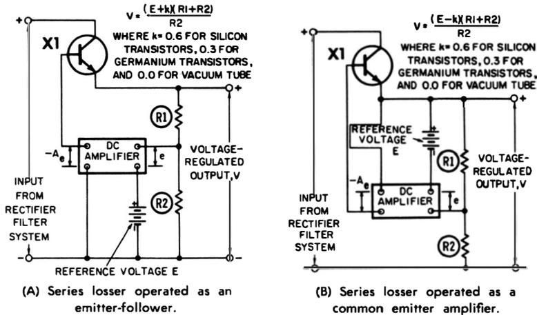
Fig. 4-2. Two basic circuit arrangements for series losser regulated power supplies.
