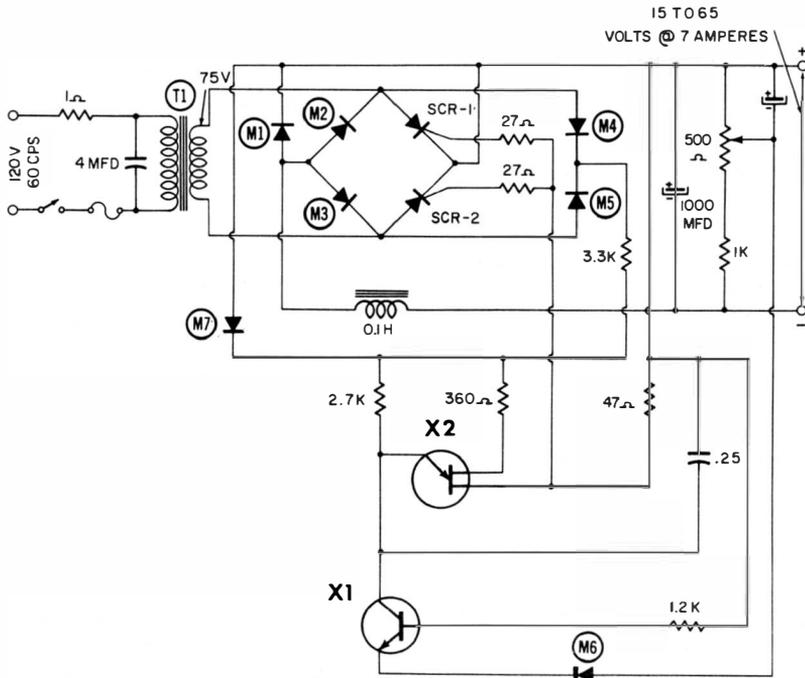
Fig. 6-9. Silicon controlled rectifier (SCR) voltage-regulated supply using variable-conduction time technique.
