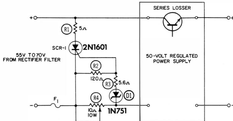
Fig. 6-14. Schematic of protective device in which deliberate blowing of a fuse removes over-current condition.
