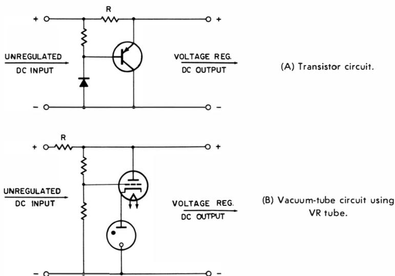
Fig. 4-3. Shunt voltage regulators.
