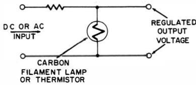
Fig. 1-10. Voltage regulation obtained by using a varistor in a shunt arrangement.
