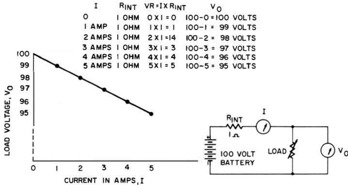
Fig. 1-3. Example of regulation due to resistance in series with load current.
