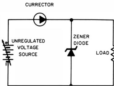
Fig. 4-8. Replacement of series loss resistance by Currector element in zener-regulated constant-voltage supply.
