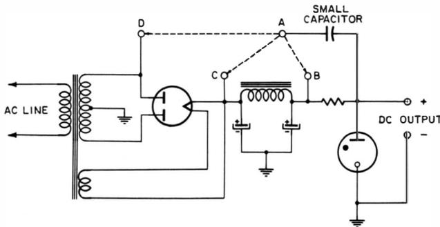
Fig. 2-10. Methods of connecting a small capacitor to aid in initial ionization of VR tube.
