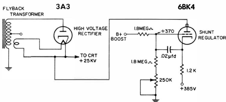
Fig. 5-12. Simplified schematic of a high-voltage regulator circuit in a color television circuit.
