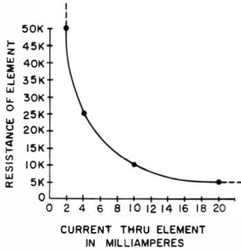
(A) Theoretical resistance variation in element capable of dissipating 2 watts.
