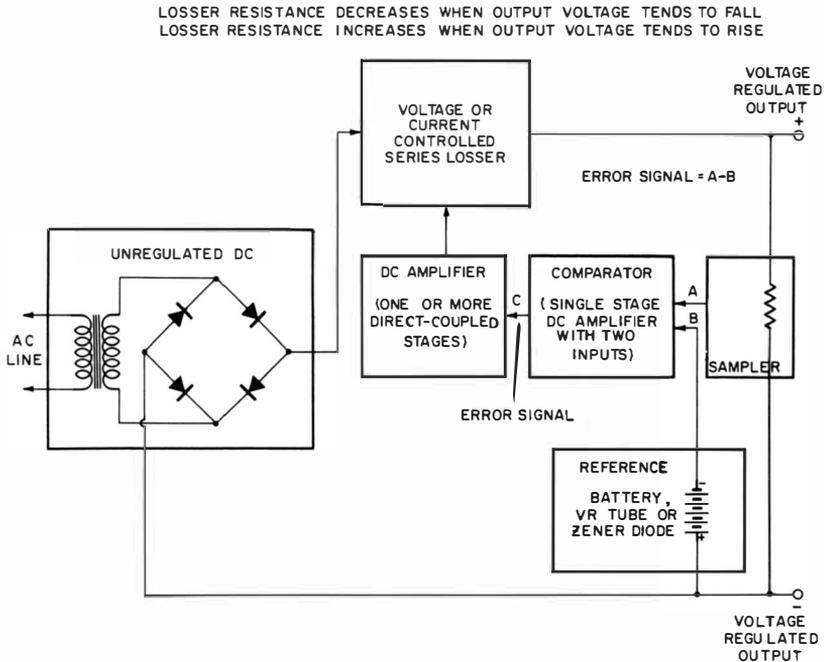
Fig. 1-22. Typical closed-loop arrangement for producing automatic voltage stabilization.
