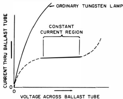
Fig. 1-13. Characteristic curve of a current ballast tube.
