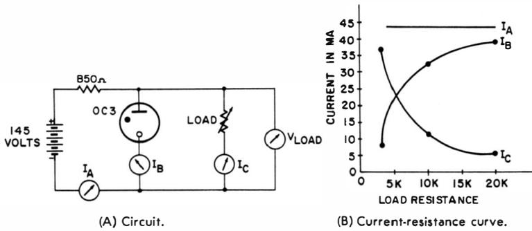
Fig. 2-7. Regulator circuit action when source voltage is fixed and load is variable.
