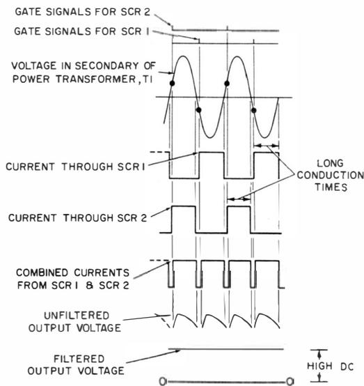
**Fig. 6-11. Conditions in circuit of Fig. 6-9 when phasing of gate signal allows long conduction time.**
