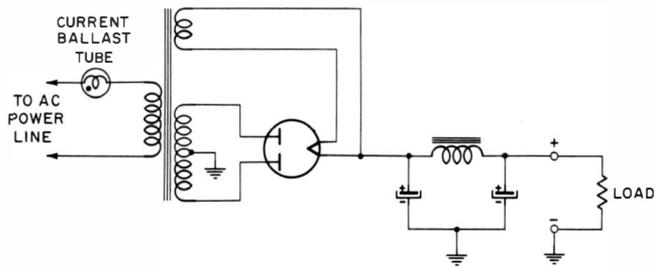
Fig. 1-14. Current ballast tube used in conjunction with a power supply.
