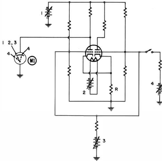
Fig. 4-11. Effect of operating voltage variations on output of differential amplifier.
