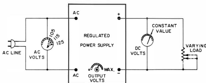
**Fig. 1-1. A voltage-regulated power supply can maintain a constant load voltage despite variations in line voltage or load resistance.**
