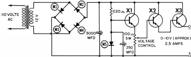
Fig. 5-4. A series regulator with a continuously variable output voltage from 0 to 10 volts and a current rating of 2.5 amperes.
