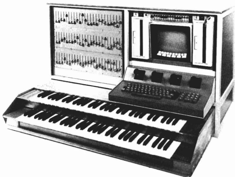
**Fig. 1-9. A digital synthesizer capable of linear fm.** (Courtesy Bell Laboratories)
