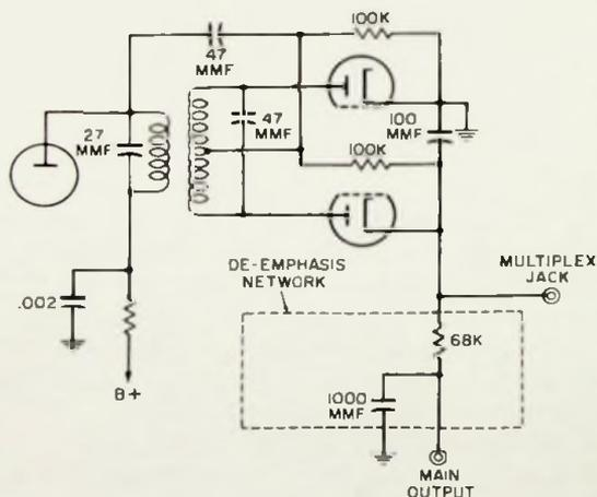
Fig. 3-7. Partial schematic of typical discriminator circuit.
