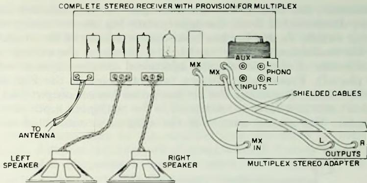
Fig. 3-21. Interconnection after addition of multiplex adapter.
