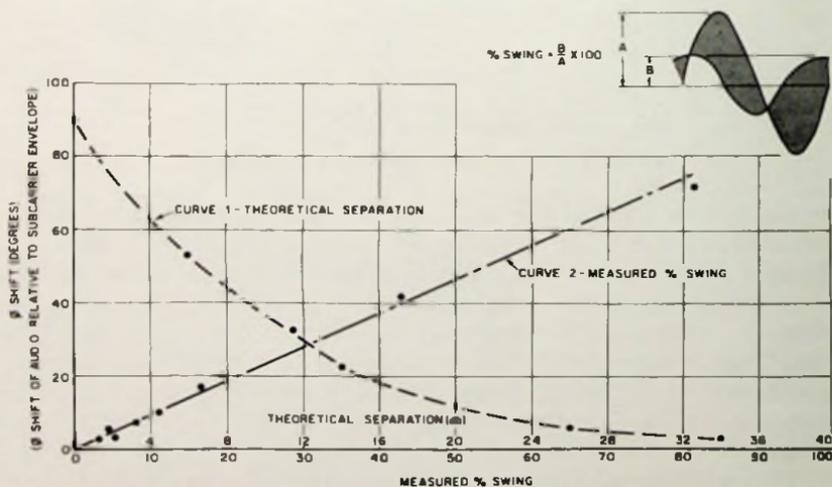
Fig. 5-13. Effects of phase shift on separation.
