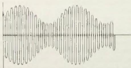
Fig. 2-6. Modulated subcarrier.
