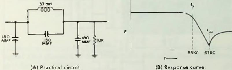
Fig. 4-19. Practical low-pass filter for switching demodulators.
