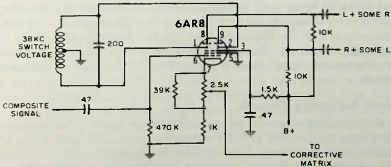
Fig. 4-25. Altec Lansing 359A demodulator circuit.
