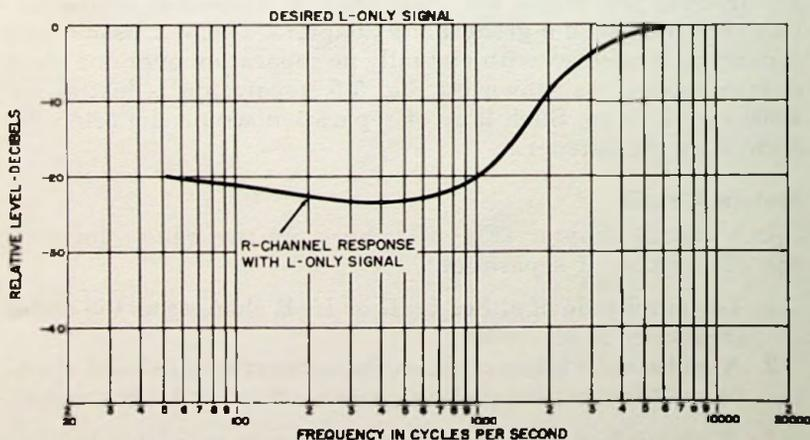
Fig. 5-5. Separation at high audio frequencies.
