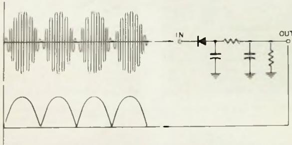
Fig. 2-10. Waveform obtained by rectifying sidebands without subcarrier.
