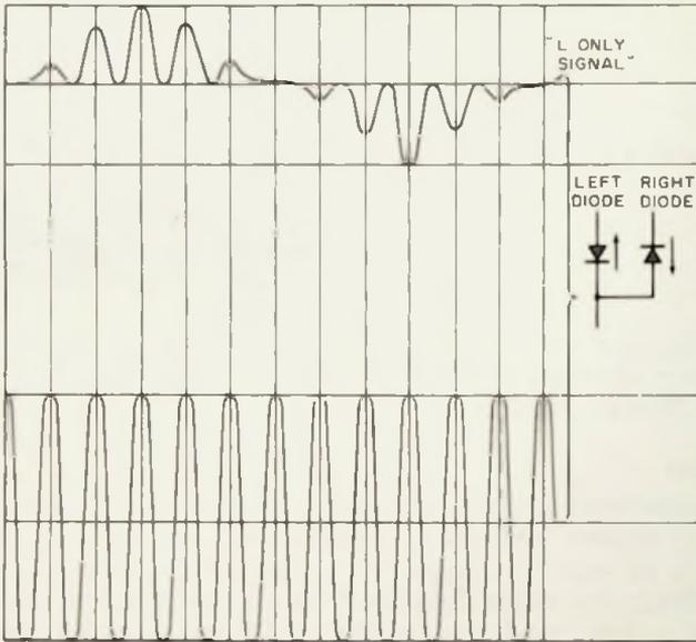
Fig. 4-23. Left-only signal (above) and switching voltage (below).
