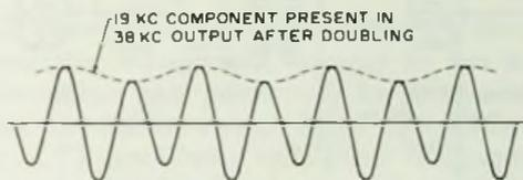
Fig. 4-13. Typical 38-kc output after single-stage doubling.
