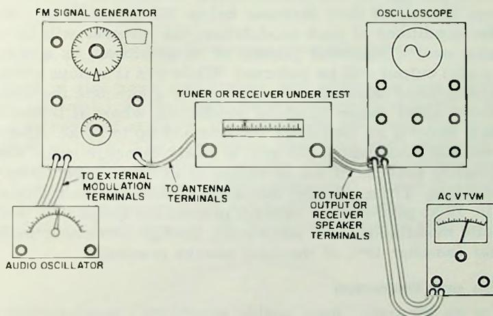
Fig. 3-1. Setup for performing quieting sensitivity measurements.
