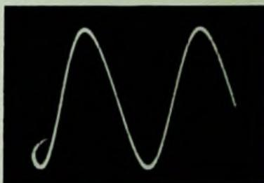
Fig. 2-4. Main-channel waveform when  $L=R$ .
