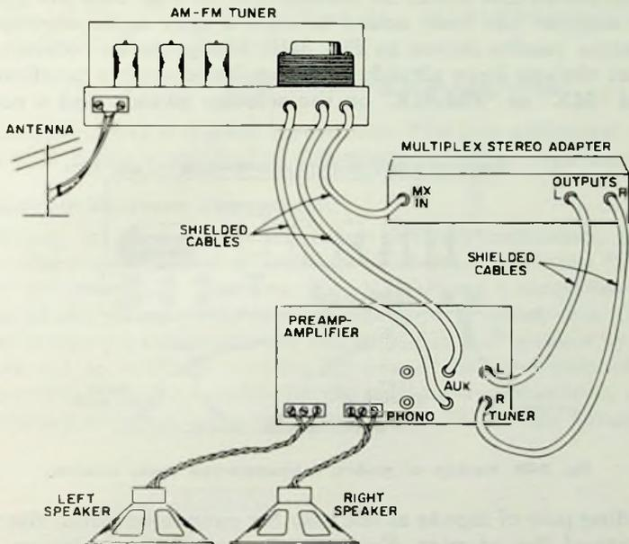
Fig. 3-19. System after multiplex adapter has been added.
