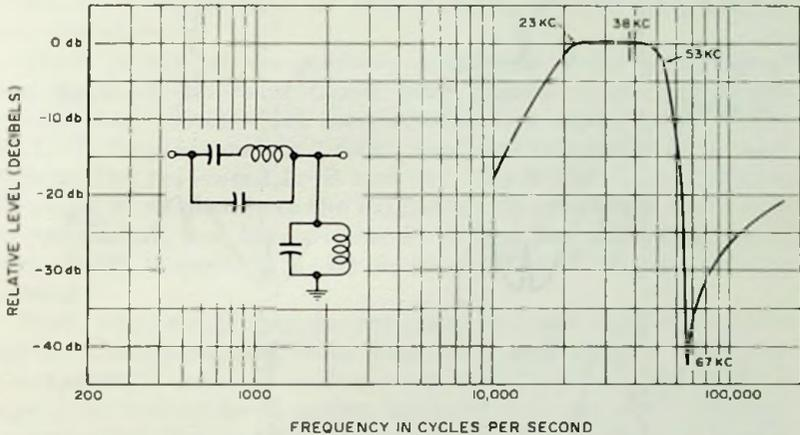
Fig. 4-3. Response of bandpass filter.
