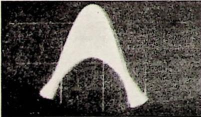
Fig. 3-13. Oscilloscope showing unbalanced recovery of main and sub-channel sidebands.
