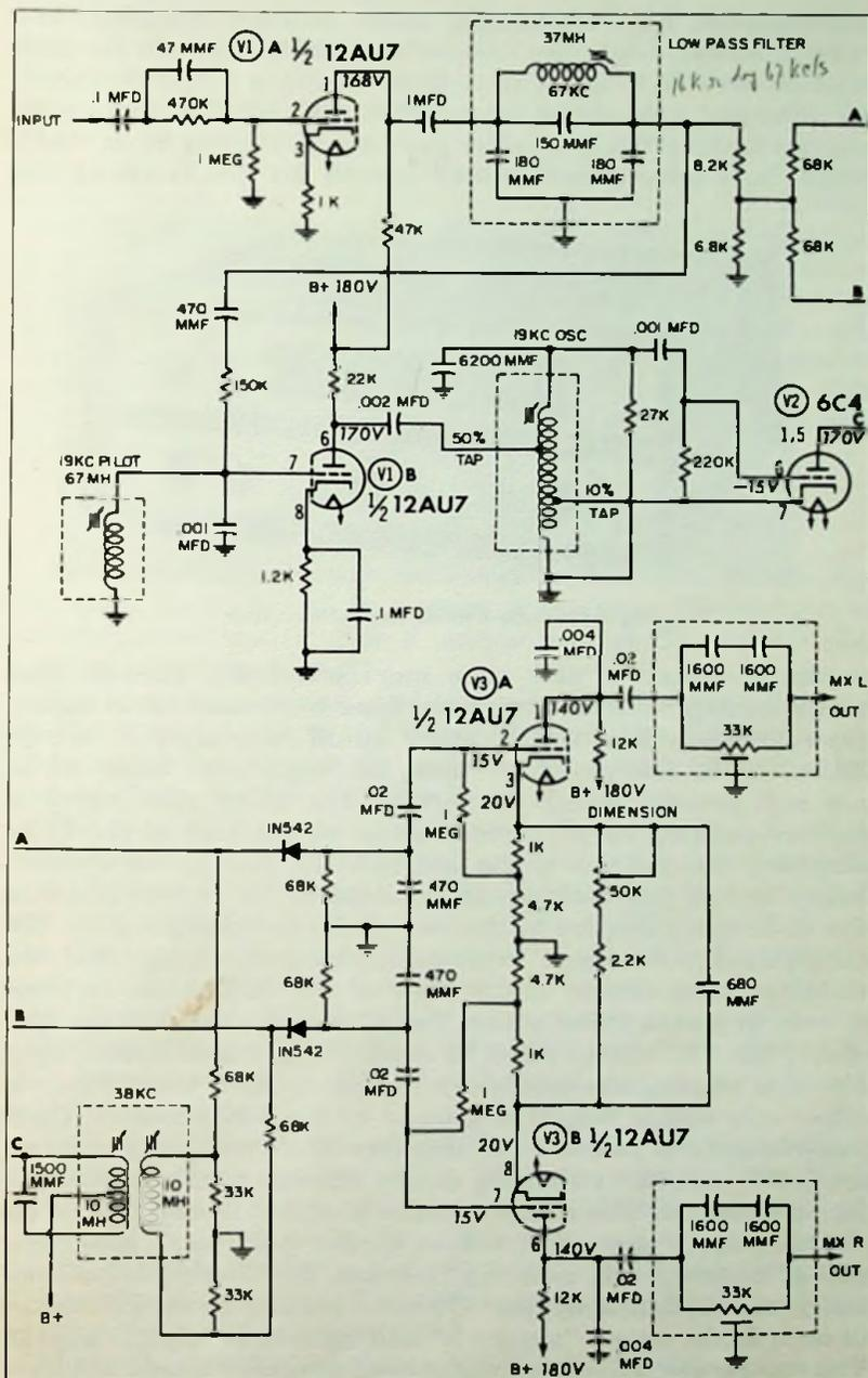
Fig. 7-8. Crosby RMX-30 multiplex section.
