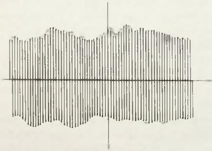
Fig. 5-2. Random modulation at junction of diodes X1 and X2 of Fig. 5-1.
