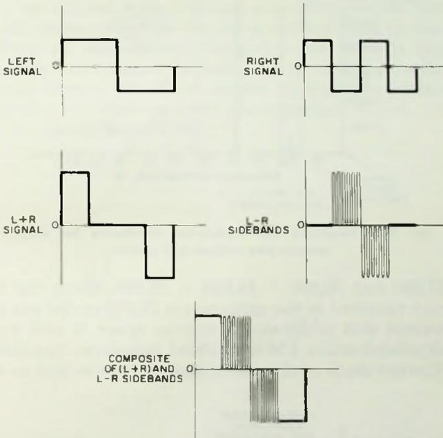
Fig. 2-14. Development of interleaving principle.
