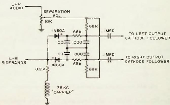
Fig. 4-29. Heath AC-11 detection and adding circuit.
