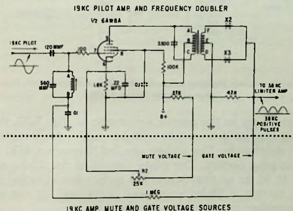
Fig. 7-21. Zenith 12H26 multiplex pilot amplifier and frequency doubler.
