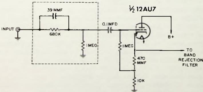
Fig. 5-6. Partial circuit of first stage of Pilot 100 and 200.
