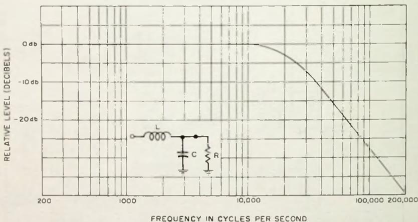
Fig. 4-2. Curve of low-pass filter
