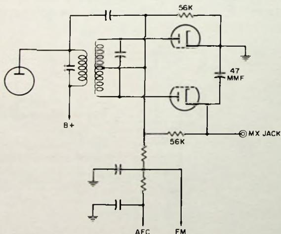
Fig. 3-16. Modified discriminator circuit.
