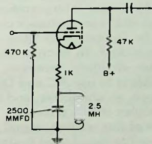
Fig. 4-34. Trap (67 kc) for reducing SCA interference.
