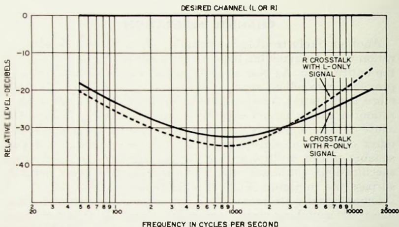
Fig. 5-4. Channel-separation curves.
