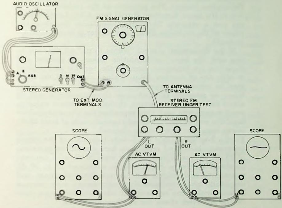
Fig. 6-9. Setup for checking performance of FM stereo receiver system.
