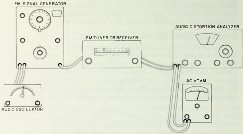
Fig. 3-2. Setup for measuring least usable sensitivity.
