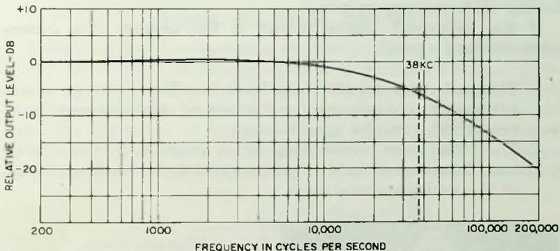
Fig. 3-11. Discriminator response with severe rolloff at subcarrier frequencies.
