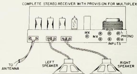
Fig. 3-20. Hookup of modern component-type stereo receiver.
