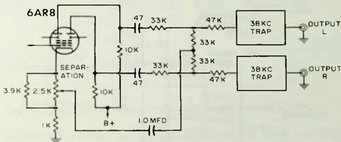
Fig. 4-28. Portion of Altec Lansing 359A demodulator circuit.
