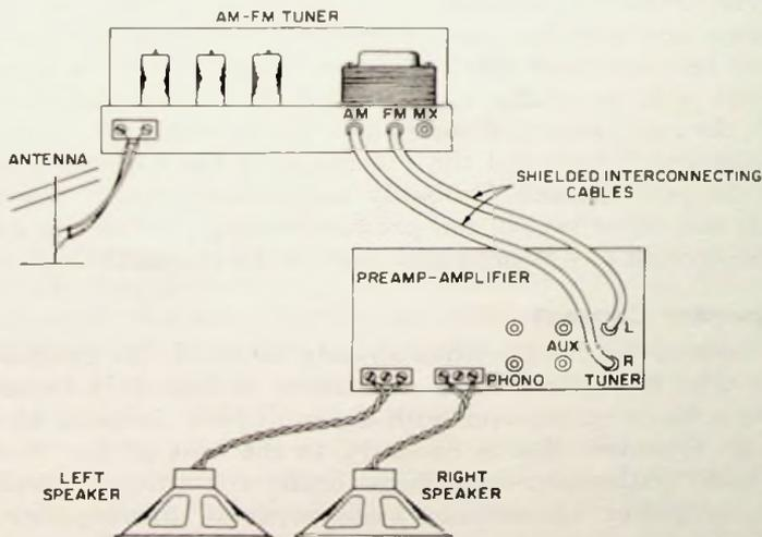
Fig. 3-18. Typical stereo component setup.
