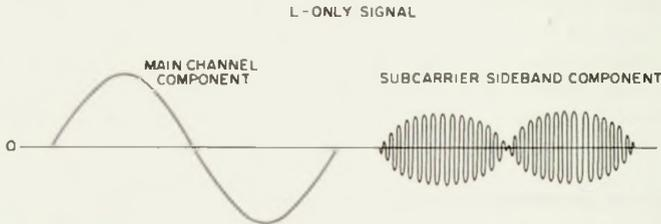
Fig. 3-12. Sidebands recovered in a receiver with discriminator response of Fig. 3-11.
