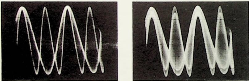
Fig. 2-13. Composite modulating signal with L = 400 cps and R = 800 cps.
