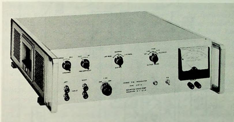
Fig. 6-1. Boonton Radio 219-A stereo FM modulator.
