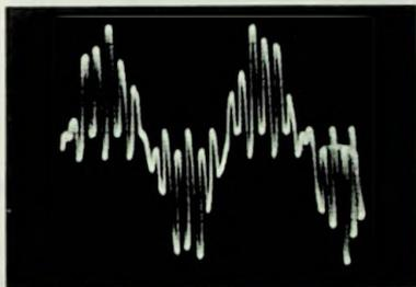
Fig. 2-12. Waveform using higher-frequency modulating tone.
