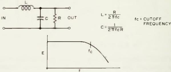
Fig. 4-17. Constant-K low-pass filter.
