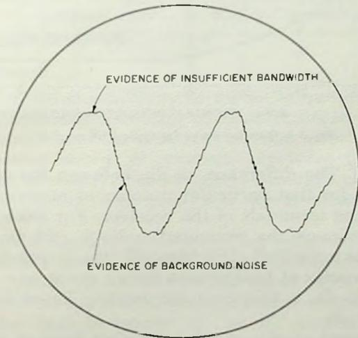
Fig. 3-3. Harmonic distribution in sine wave.
