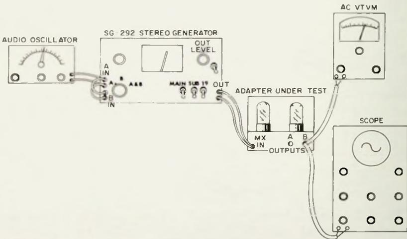
Fig. 6-6. Setup for aligning and testing multiplex equipment.
