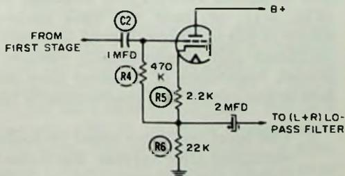
Fig. 4-10. Second stage of Heath AC-11.
