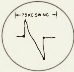
Fig. 5-10. Waveform indicating regeneration.
