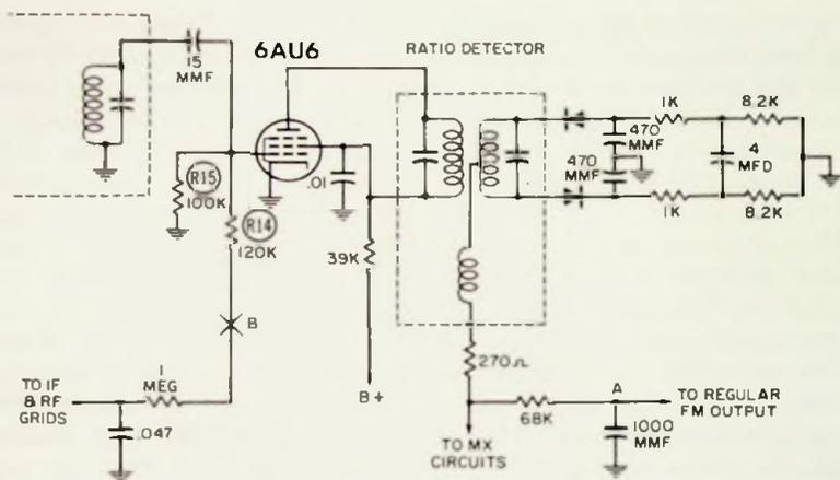
Fig. 3-5. Partial schematic of last IF stage and ratio detector of Bogen TP-60 tuner.
