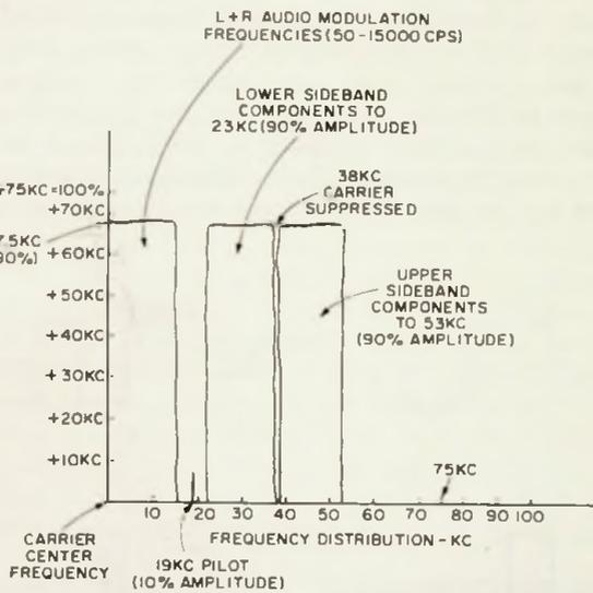
Fig. 2-15. Frequency and modulation distribution for stereo broadcasting without SCA service.
