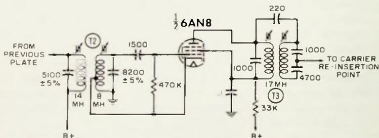
Fig. 4-12. Bogen TP-60 oscillator circuit.
