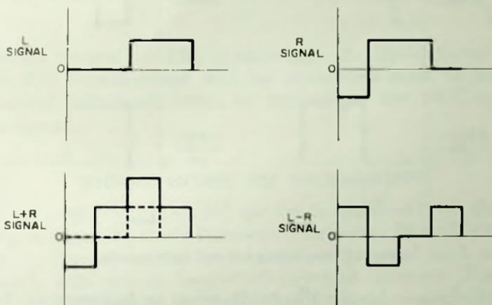
Fig. 1-1. Combining signals to obtain  $L+R$  and  $L-R$ .
