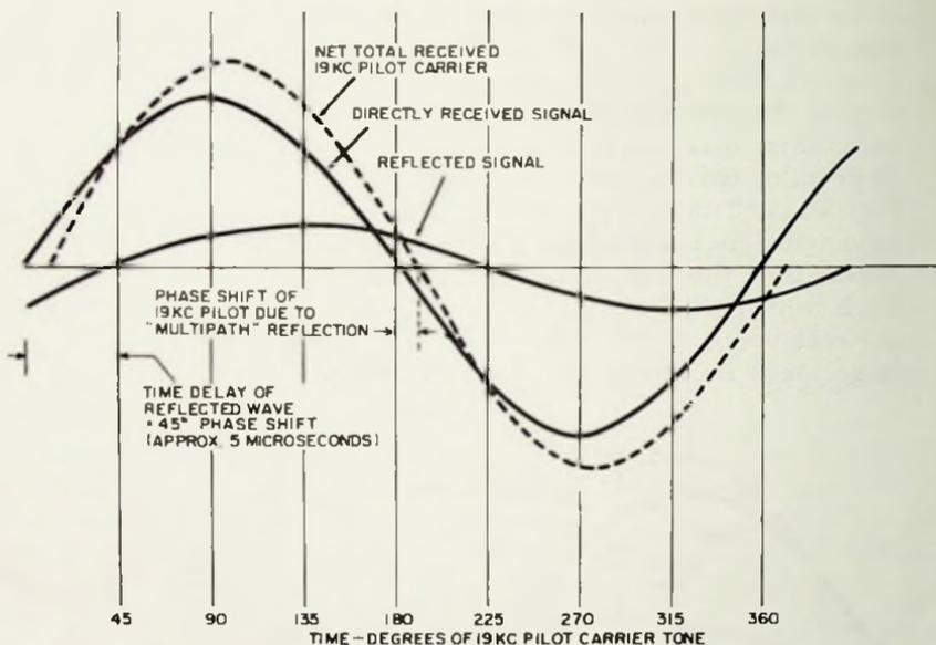
Fig. 5-12. Effect of multipath on 19-kc pilot carrier.
