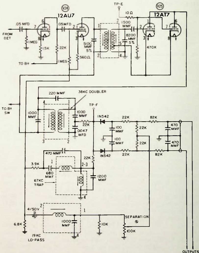
Fig. 7-3. Bogen RP-40A multiplex section.
