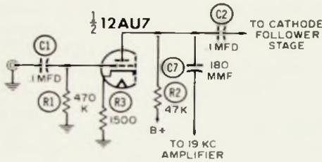
Fig. 4-6. First stage of Heath AC-11 adapter.
