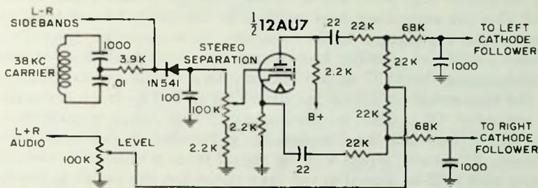
Fig. 4-30. Bogen PX-60 additive matrix circuit.
