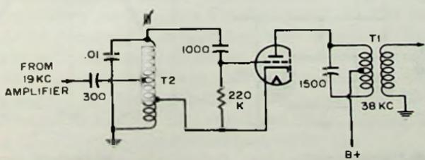
Fig. 4-16. Heath AC-11 oscillator circuit.
