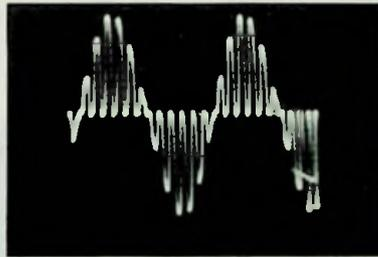
Fig. 2-9. L-only signal with higher-frequency tone.
