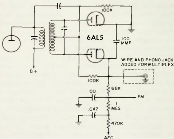
Fig. 3-15. Typical discriminator circuit.
