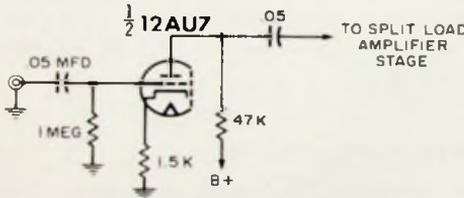
Fig. 4-7. First stage of Bogen PX-60 adapter.
