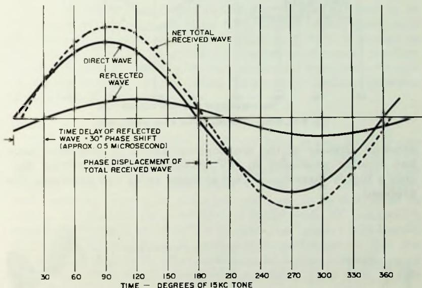
Fig. 5-11. Effect of multipath on 15-kc signal.
