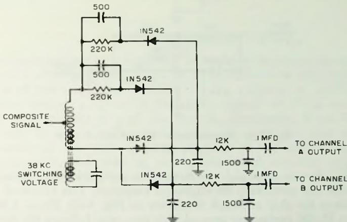
Fig. 4-31. Pilot Radio 100 and 200 demodulator circuit.
