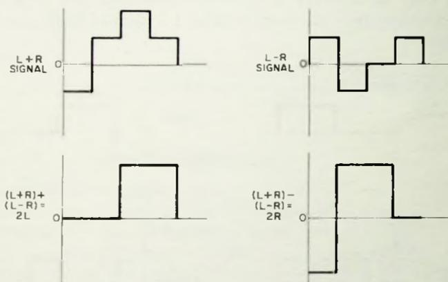
Fig. 1-2. Recovering left and right signals.
