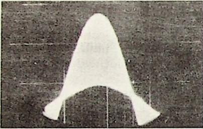
Fig. 4-26. Left-only signal attenuated 4 db.
