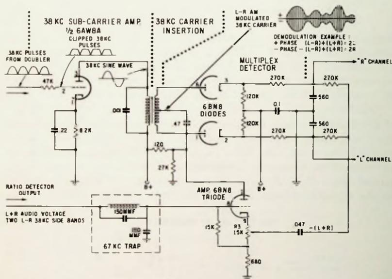
Fig. 7-22. Zenith circuitry showing subcarrier amplifier and reinsertion, L and R signal demodulation and matrixing.
