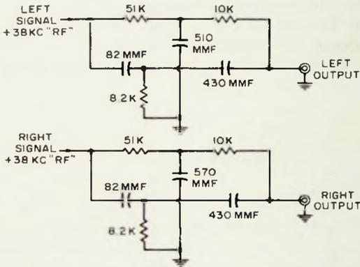
Fig. 4-32. Harmon-Kardon MX-500 twin-T notch filter (38 kc).
