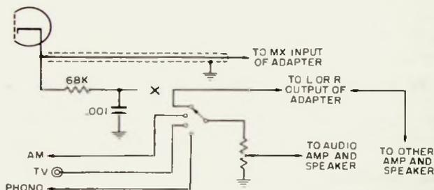
Fig. 3-23. Switch rewired to accommodate multiplex adapter.
