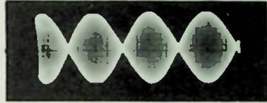
form of Fig. 2-3 will now be added to the “double-sideband, suppressed-carrier” waveform of Fig. 2-7. This will produce the waveform in Fig. 2-8. Except for one minor missing element, it is all that will be used to transmit a left-channel-only, 400-cycle tone over the air. This will be done by modulating the RF carrier  $\pm 90\%$  of 75 kc.
