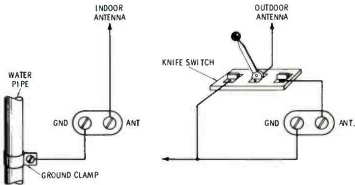
Fig. 3-2. Connections for single-wire antenna.
