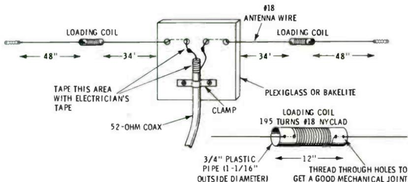
Fig. 10-9. Three-band antenna using loading coils.
