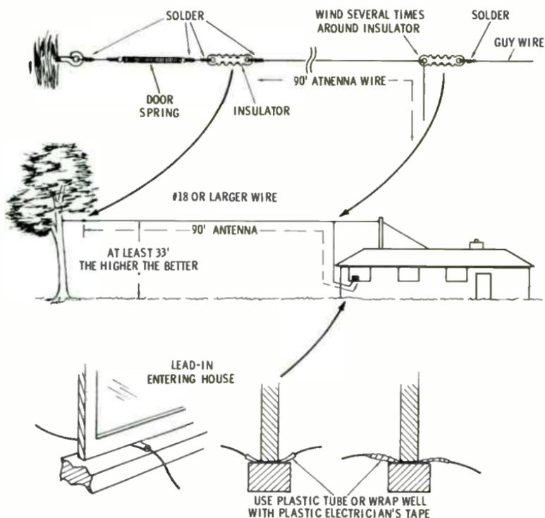
Fig. 9-3. Antenna installation for basic Novice station.
