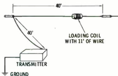
Fig. 9-4. Using a loading coil to shorten antenna length.
