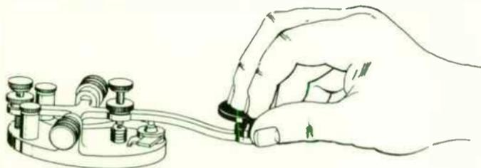
Fig. 8-3. Conventional grip used with a hand telegraph key.
