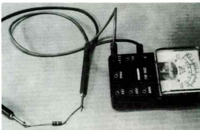
Fig. 4-4. Checking the resistance of a resistor.
