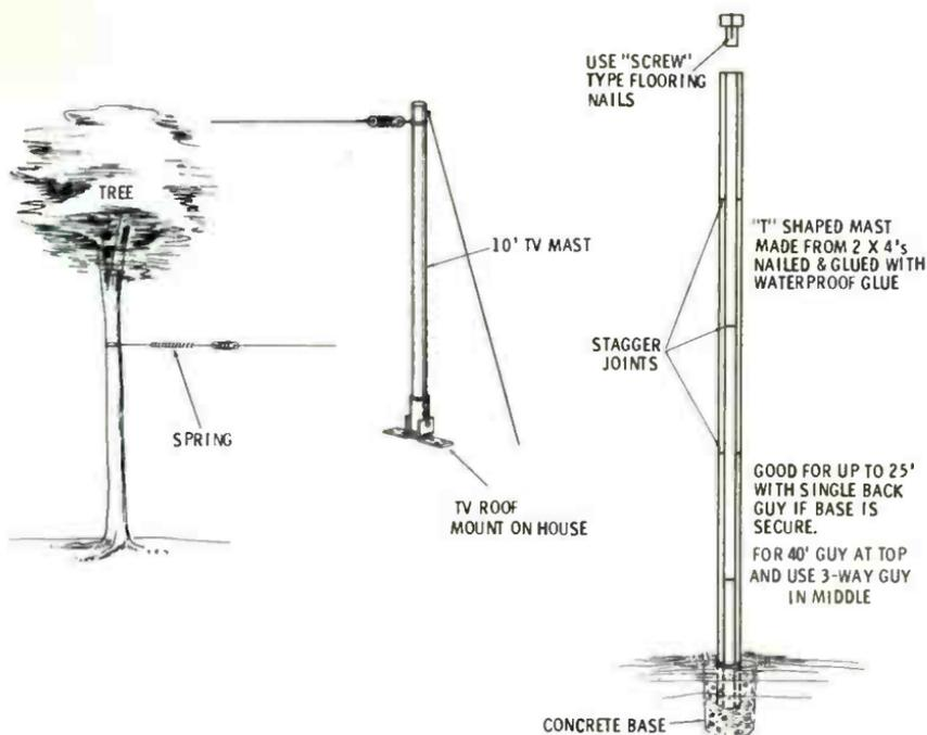
Fig. 10-1. Supporting the antenna.
