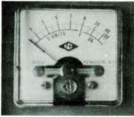
**Fig. 2-3.** An 5-meter on a communications receiver.
