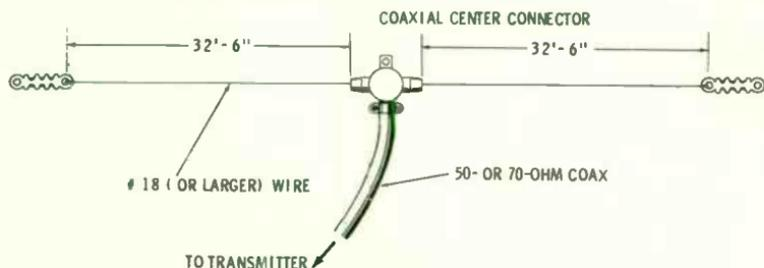
Fig. 10-7. The 40- and 15-meter antenna.
