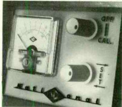
Fig. 3-12. Dial can be shifted with set control.
