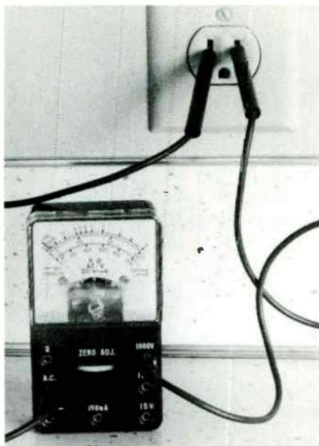
Fig. 4-11. Measuring ac line voltage.
