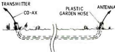
Fig. 10-13. Running coaxial cable underground.
