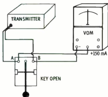
Fig. 9-12. Hookup for measuring plate current.
