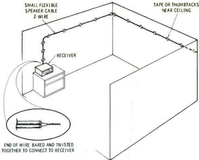
Fig. 3-1. A temporary room antenna.
