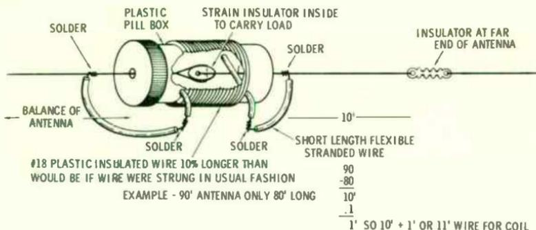
Fig. 9-5. Construction details for a loading coil.
