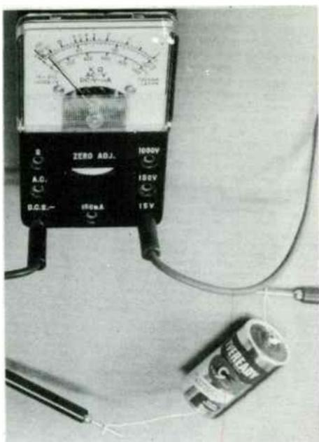
Fig. 4-10. Measuring battery voltage.
