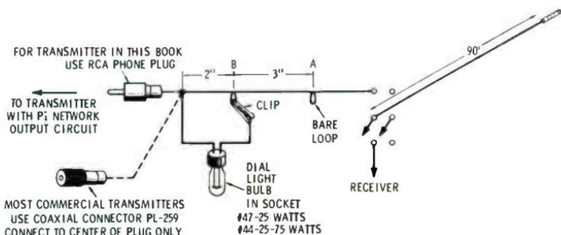
Fig. 9-10. Tuning indicator for single-wire antenna.
