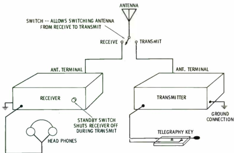
Fig. 5-1. Block diagram of a simple Novice station.
