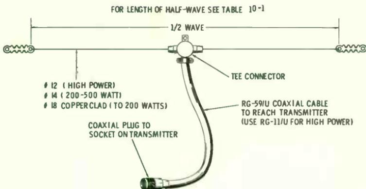
Fig. 10-2. Typical half-wave dipole.
