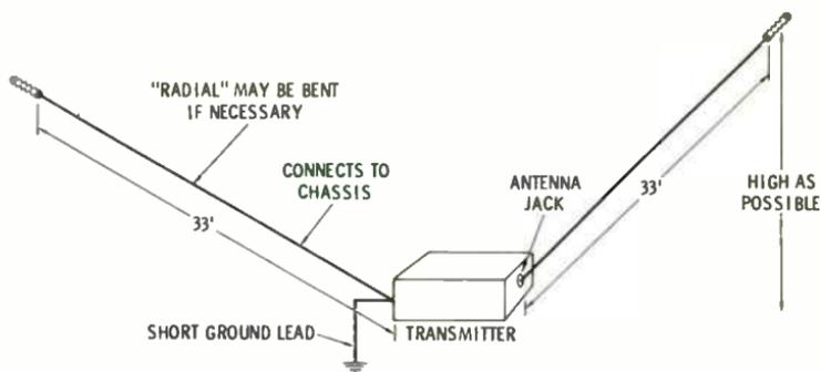
**Fig. 9-7. Improving the short 40-meter antenna.**
