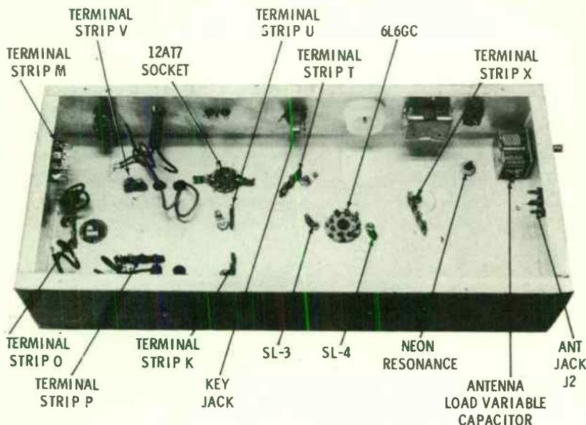
Fig. 6-3. Bottom view of chassis.
