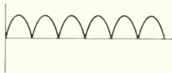
Fig. 4-8. Output current from a full-wave rectifier.
