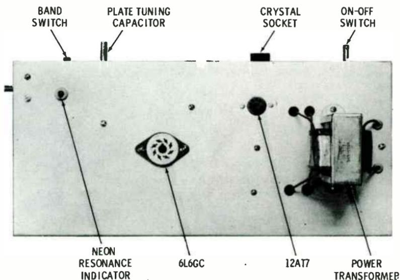
Fig. 6-2. Top view of chassis.
