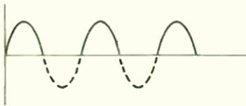
Fig. 4-7. Representation of output current of a half-wave rectifier.
