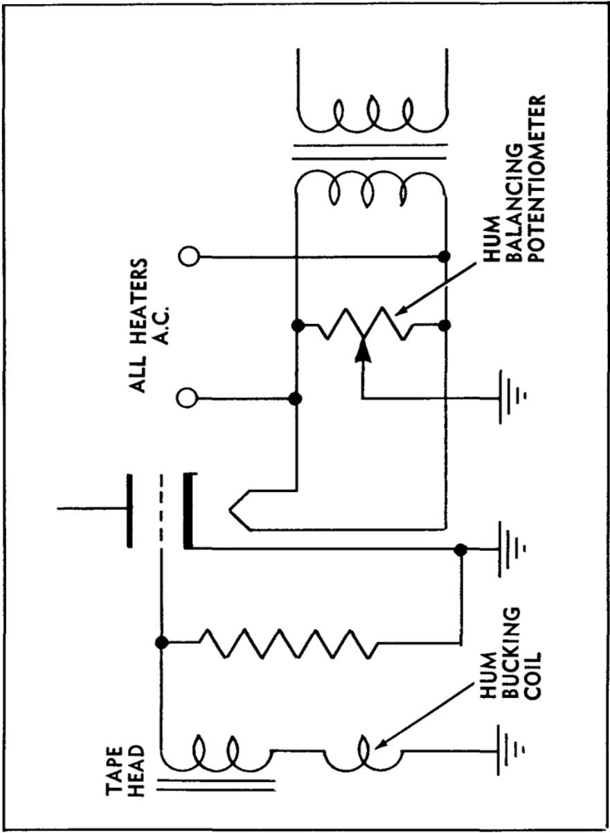
Fig. 3-2. A circuit with hum bucking and hum balancing.
