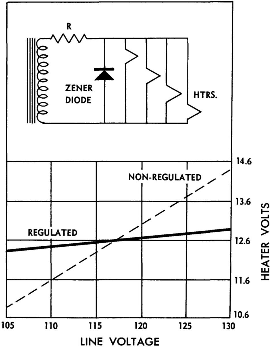
Fig. 10-1. Zener-diode regulator and chart, showing the improvement of the voltage stability.
