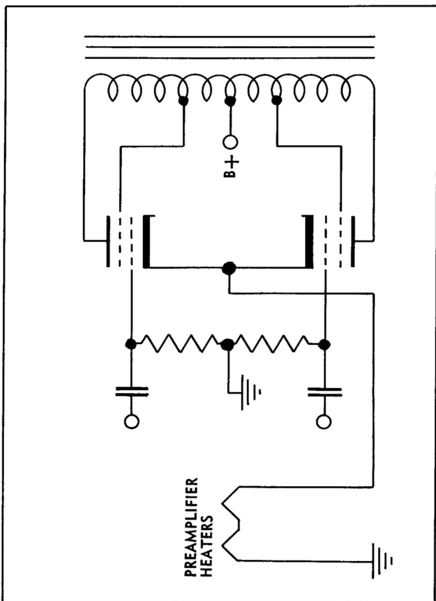
*Fig. 3-3. Using amplifier cathode current for heaters. The heater voltage drop provides the necessary bias for the output stage.*
