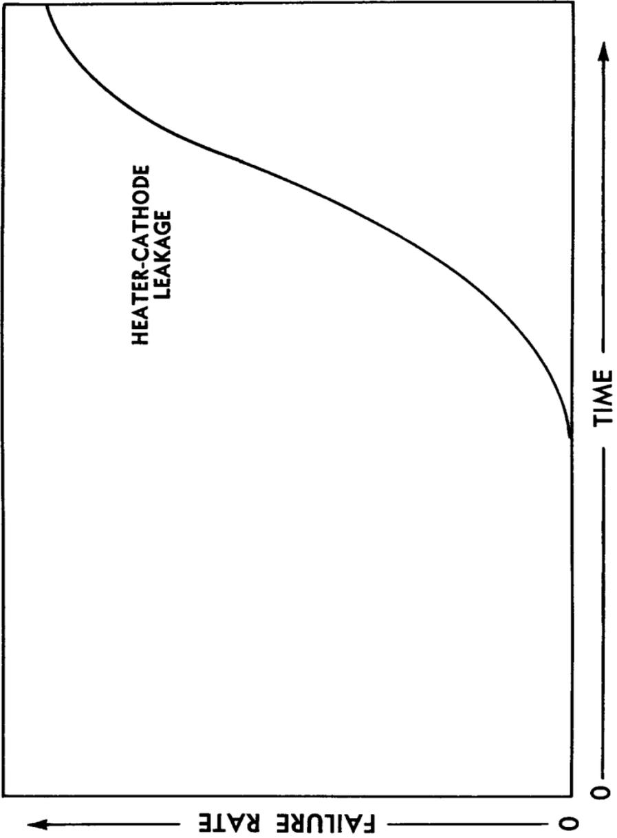
*Fig. 2-3. Heater-to-cathode leakage increases sharply with age.*
