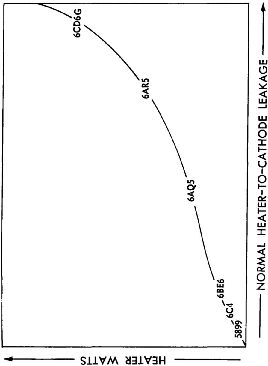
Fig. 8-3. A chart of heater power versus the normal leakage of a number of well-known tube types.
