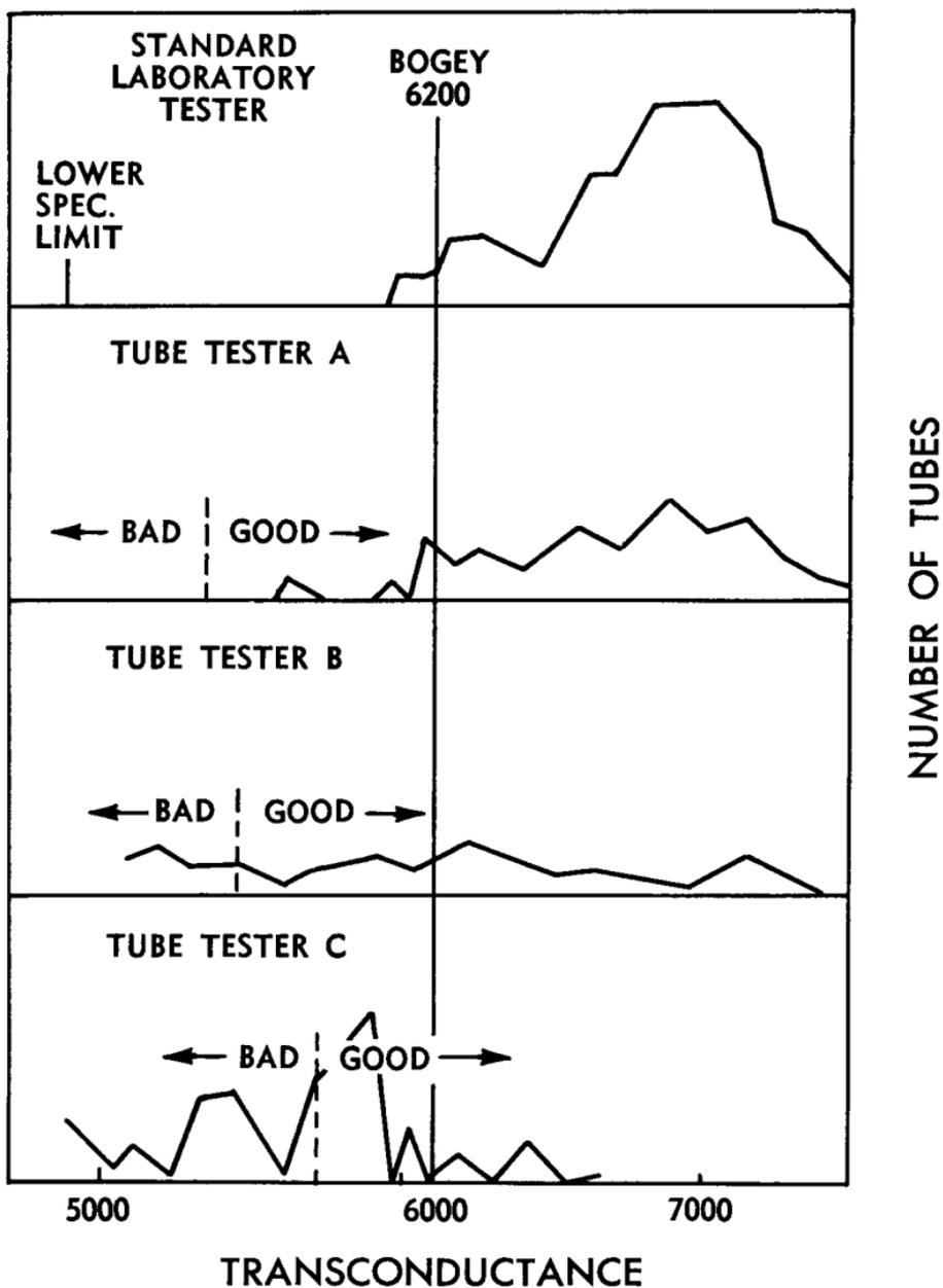
Fig. 8-1. Comparison of results obtained when a number of tubes were tested in three commercial tube testers and in a standard laboratory tester.
