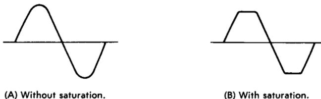
Fig. 5-12. Waveform of a transformer in which the core is saturating.
