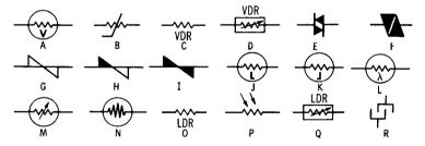
Fig. 2-13. Voltage- and light-dependent resistor symbols.
