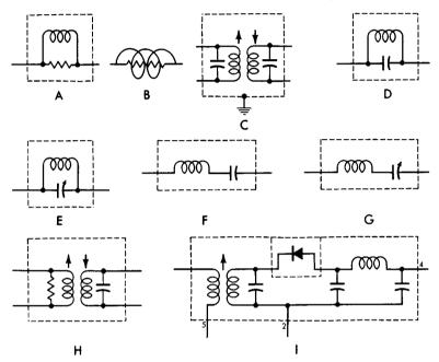
Fig. 9-13. Various coil and transformer combination symbols.
