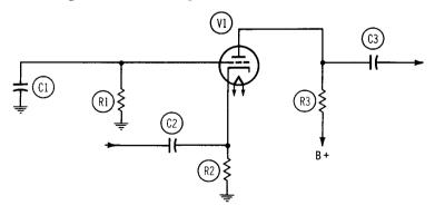
Fig. 10-6. A grounded-grid amplifier circuit.
