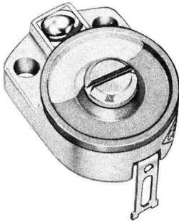
Fig. 3-9. A ceramic trimmer capacitor.
