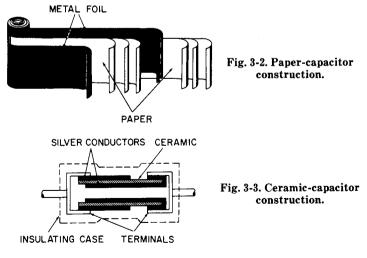
space. This method is shown in Fig. 3-2. This assembly can then be enclosed in plastic or wax-impregnated paper.
