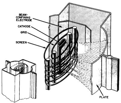
Fig. 5-9. Construction of beam-power tube.
