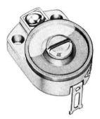
Fig. 3-9. A ceramic trimmer capacitor.
