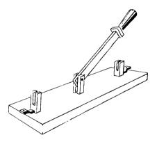
Fig. 7-3. A SPDT knife switch.
