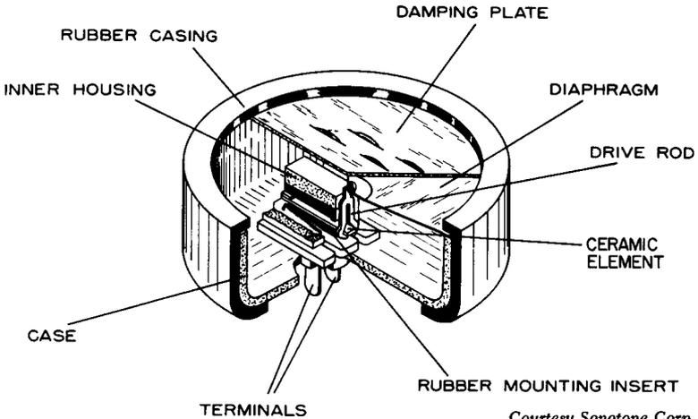
**Fig. 8-19. Construction details of a ceramic microphone.**
