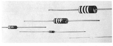
Courtesy Ohmite Manufacturing Co. Fig. 2-1. An assortment of carbon resistors.
