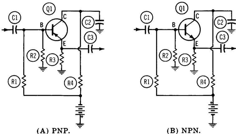
Fig. 10-9. Common-collector circuits.
