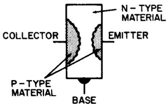
Fig. 6-8. Elementary construction of a transistor.
