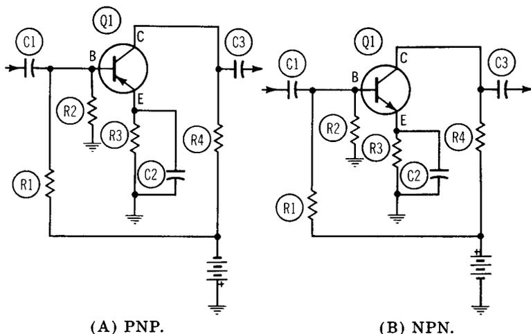
Fig. 10-7. Common-emitter circuits.
