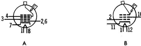
Fig. 5-17. Electromagnetic cathode-ray tube symbols.
