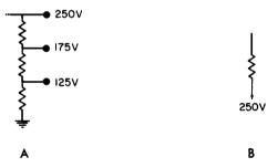
Fig. 9-3. A common method of showing connections to voltage sources.
