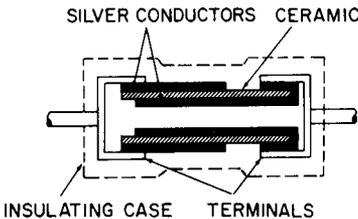
Fig. 3-3. Ceramic-capacitor construction.
