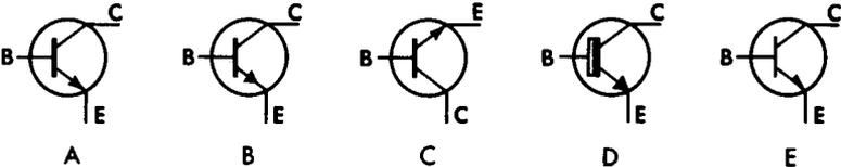
Fig. 6-10. NPN-transistor symbols.
