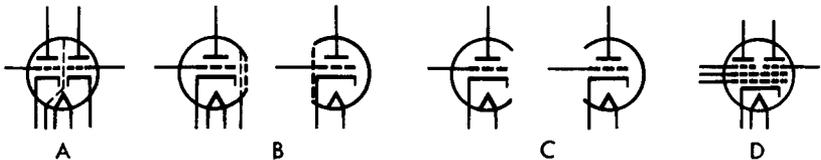
Fig. 5-11. Dual-section tube symbols.
