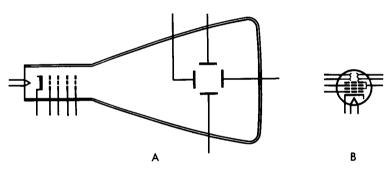
Fig. 5-16. Electrostatic cathode-ray tube symbols.
