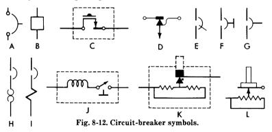
The symbol for a thermal unit is given by H in Fig. 8-12. It is a combination of symbol A and two partial circles which designate the thermal action. If the action is magnetic, the zigzag line in I is used instead. A coil and a switch symbol are combined to depict a magnetic circuit breaker in J, and resistor symbols are used in the thermal unit designated by symbols K and L.
