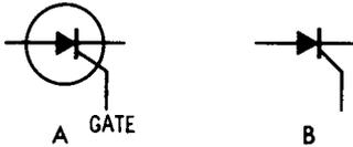
Fig. 6-13. Silicon controlled rectifier symbols.
