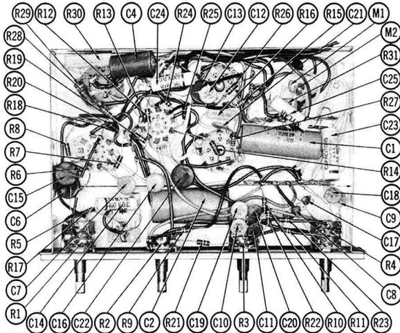
**Fig. 1-5. Photo of underside of phono-amplifier chassis.**
