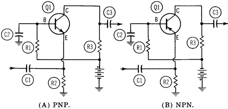
Fig. 10-8. Common-base circuits.
