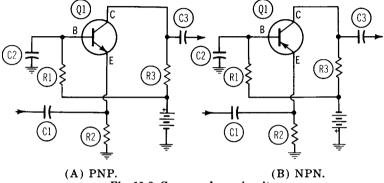
Fig. 10-8. Common-base circuits.
