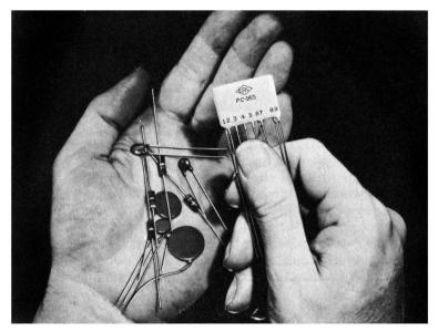
Courtesy Centralab, Electronics Division of Globe-Union Inc. Fig. 9-15. A packaged electronic circuit and the components it replaces.
