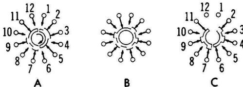
Fig. 7-11. Wafer-switch symbols.
