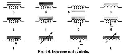
Adjustable iron-core chokes are comparatively rare. Usually, instead of being continuously variable, a series of taps and a switch are employed to make connection to the desired portion. When a continuously variable iron-core unit is used, however, it may be indicated by any one of the symbols at H, I, J, K, or L. These are the same as for a conventional choke, but with an arrow added to signify the inductance can be varied.
