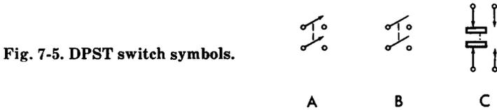
*single-throw* (DPST) knife switch consists of two blades, each of which can be connected to one set of terminals. The two blades are connected, or ganged, together (by an insulating material) so that when one is moved, the other automatically follows. Fig. 7-5 shows the symbols used to denote DPST switches. The dashed line indicates that the two arms are mechanically but not electrically connected.
