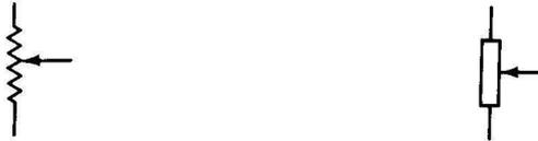
Fig. 2-7. Symbols sometimes used for adjustable resistors.
