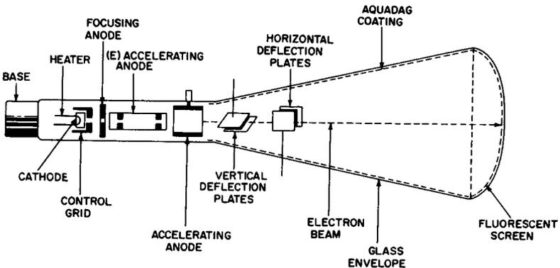
Fig. 5-15. Construction of an electrostatically-deflected cathode-ray tube.
