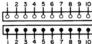
numbering and arrangement is usually included on the schematic also. Instead of the arrangement of Fig. 9-8, individual connections may be shown, as in C, D, and E of Fig. 9-7. Each is then labeled with the plug or socket number, followed by a dash and a number denoting the pin. Most of the time, plugs
