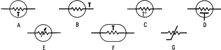
Fig. 2-12. Temperature-compensating resistor symbols.
