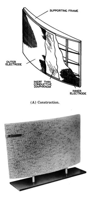
Courtesy of Pickering & Company, Inc. (B) Photograph. Fig. 8-5. An electrostatic speaker. rent flows through the coil, the core becomes magnetized, making the operation essentially the same as for the permanent-magnet speaker.
