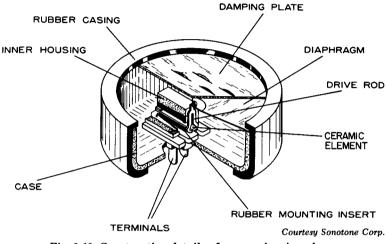
Fig. 8-19. Construction details of a ceramic microphone.
