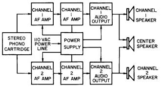
Fig. 1-2. Block diagram of the phono amplifier in Fig. 1-1.
