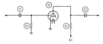
Fig. 10-3. An R-C-coupled grounded-cathode amplifier circuit.
