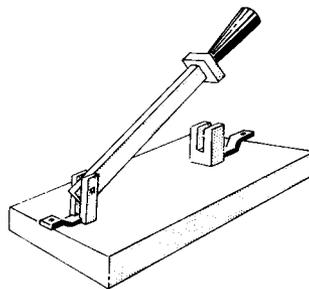
a device is called a *single-pole, single-throw* switch (abbreviated SPST). It can make connections for only one line, and at only one point. The symbols for SPST switches are given in Fig. 7-2. All look alike except B, differing only in the arrow-
