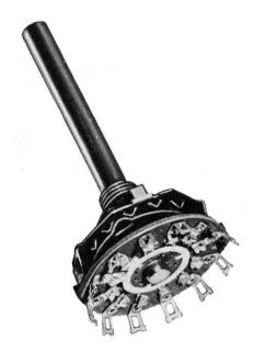
Courtesy of Centralab, Electronics Division of Globe-Union, Inc. Fig. 7-7. A typical wafer switch.
