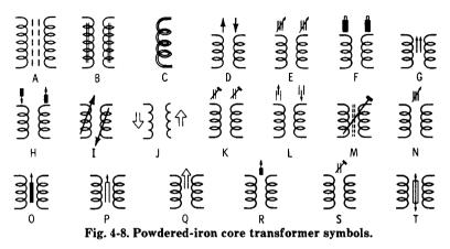
Fig. 4-8 shows the symbols for designating a powderediron core transformer. In this type the individual coils are usually wound on a single form (Fig. 4-9). In Fig. 4-9A the unit is shielded by a metal cover (called a *can*); the one in Fig. 4-9B has no such covering. Both units have capacitors connected across their windings for tuning.
