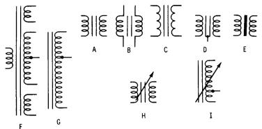
Fig. 4-11. Iron-core transformer symbols.
