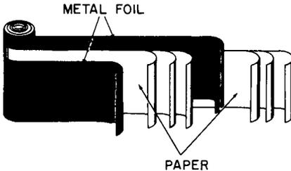
Fig. 3-2. Paper-capacitor construction.
