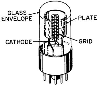
Fig. 5-4. Construction of a triode tube.
