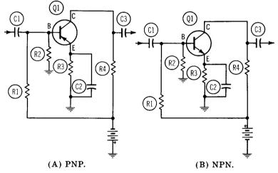
Fig. 10-7. Common-emitter circuits.
