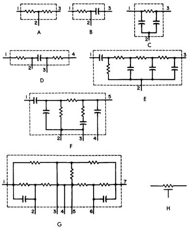
Fig. 9-16. Packaged electronic-circuit symbols.
