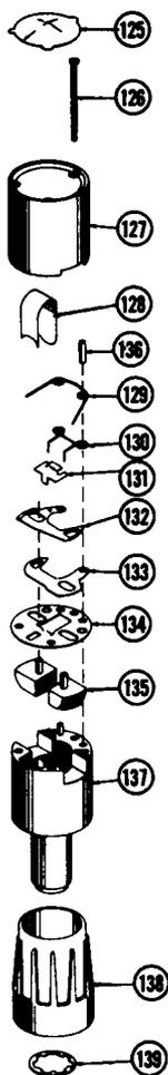
Fig. 1-7. Exploded view of the 45-rpm spindle for a record changer.
