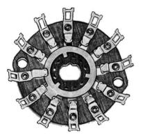
Fig. 7-9. A typical wafer.
