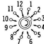
terminals 8 and 10 to terminal 11. Any number of connections can be made by such switches, each depending on the construction of the shorting ring. Two other possibilities are shown in symbols B and C.
