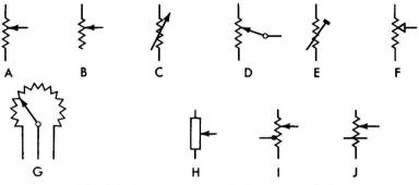
Fig. 2-9. Potentiometer and rheostat symbols.
