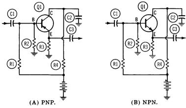
Fig. 10-9. Common-collector circuits.
