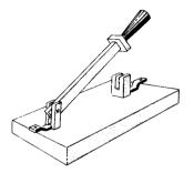
a device is called a *single-pole*, *single-throw* switch (abbreviated SPST). It can make connections for only one line, and at only one point. The symbols for SPST switches are given in Fig. 7-2. All look alike except B, differing only in the arrowheads (which indicate the movable contact) and the small circles (which indicate the connection points).
