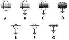
Fig. 9-4. Cable and shielded lead symbols.
