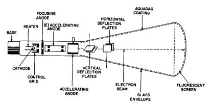
Fig. 5-15. Construction of an electrostatically-deflected cathode-ray tube.
