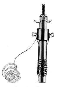
Fig. 8-2. A ferrite-loop antenna.
