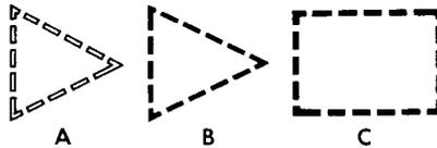
Fig. 9-19. Integrated-circuit symbols.
