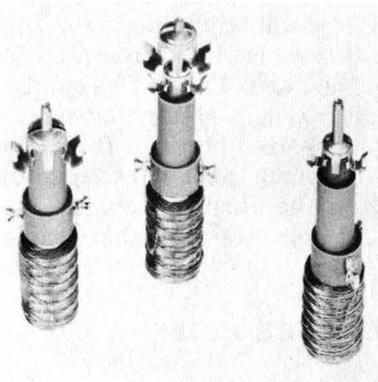
Fig. 4-4. Permeability-tuned coils.
