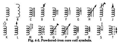
the desired shape. When such a core is brought near or inserted into a coil, it offers a more convenient path for the magnetic lines of force than does air. Hence, more lines cut the other conductors in the coil, increasing the inductance. The same symbols used for the air-core type—A and B in Fig. 4-3—may also be used for powdered-iron core coils. The symbol at C is also popular. The core may be represented by either two or three dashed lines.
