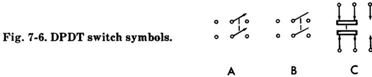
By adding another set of terminals to the two-bladed knife switch so that the two mechanically-connected blades make contact in either of two positions, it becomes a *double-pole double-throw* (DPDT). Fig. 7-6 shows the symbols for this type.
