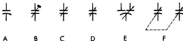
Fig. 3-10. Variable-capacitor symbols.
