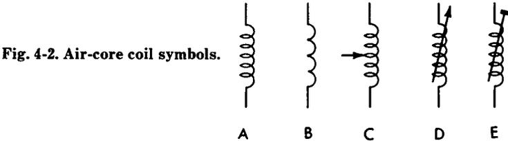
**Adjustable Air-Core Coils**
