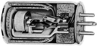
Courtesy P. R. Mallory & Co., Inc. Fig. 8-17. Cutaway view of a typical vibrator.
