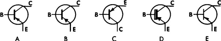
Fig. 6-11. PNP-transistor symbols.
