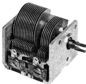
Fig. 3-11. A two-gang variable tuning capacitor.
