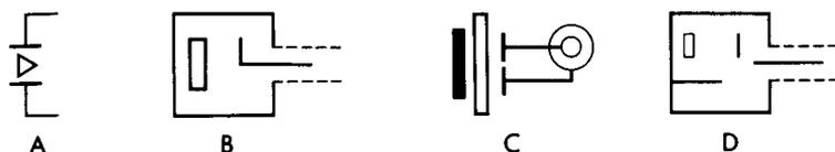
Fig. 8-21. Ultrasonic-transducer symbols.
