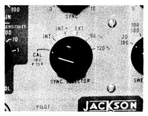
Fig. 6-3. Sync selector includes CAL position for interternal calibrating voltage.
