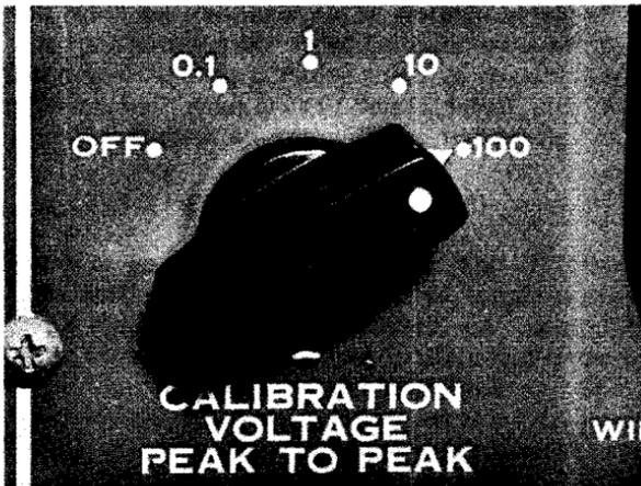
Fig. 6-4. This scope permits the use of four different calibrating voltages.
