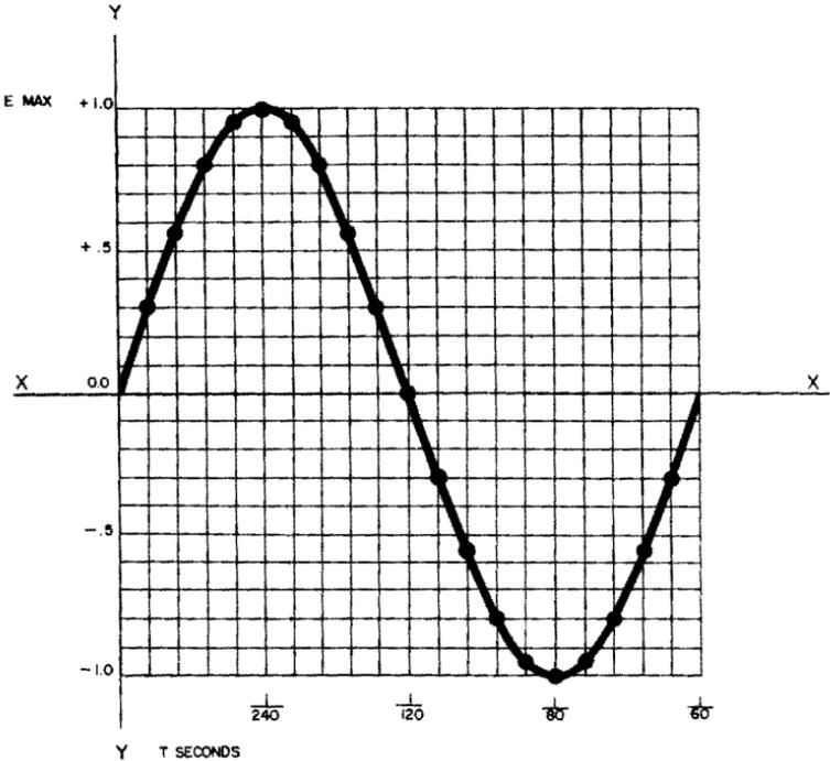
**Fig. 1-1. Graph of one cycle of power-line voltage. Frequency is 60 cycles per second.**
