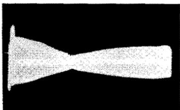
**Fig. 10-19.** Response curve obtained with correct adjustment of 4.5 megacycle trap.
