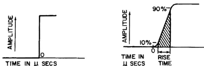
Fig. 5-6. Diagram illustrating rise time.
