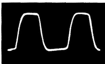
**Fig. 10-6.** High frequency attenuation is shown by rounded corners of square wave.
