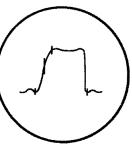
Since the sweep signals for the receiver response curve and marker adder are both taken from the same sweep generator, the marker will appear at its proper location when combined with the response curve. The marker signal does not pass through the receiver circuits and, therefore, is not attenuated by the trap circuits or amplified at peak response frequencies. The marker remains at the same amplitude on the oscilloscope screen as it is tuned across the entire response curve.
