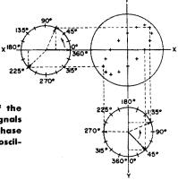
Fig. 9-10. Graphical illustration of the manner in which two sine-wave signals of identical frequency but different phase develop a phase indication on an oscilloscope.
