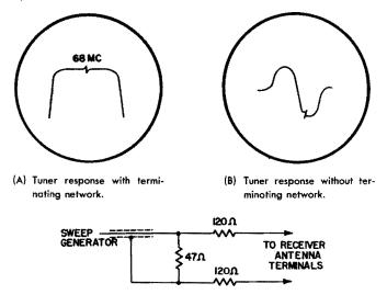
(C) Schematic diagram of terminating network.
