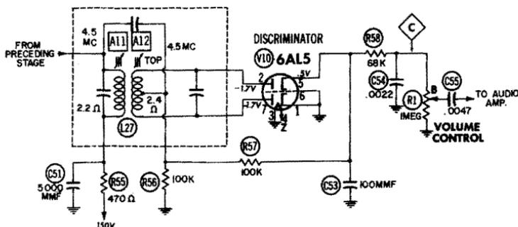
Fig. 11-7. Typical FM discriminator circuit.
