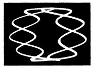
Fig. 9-5. 6 to 1 crown wheel pat- Fig. tern.
