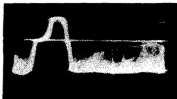
**Fig. 8-7. Oscilloscope response using amplifier of 2-megacycle bandwidth.**
