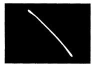
Fig. 12-13A. Triode operating characteristic with small overload.
