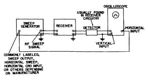
Fig. 11-3. Minimum equipment necessary to obtain a response curve.
