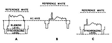
Fig. 5-3. Video signals at the picture tube; viewed on oscilloscope having DC amplifiers.
