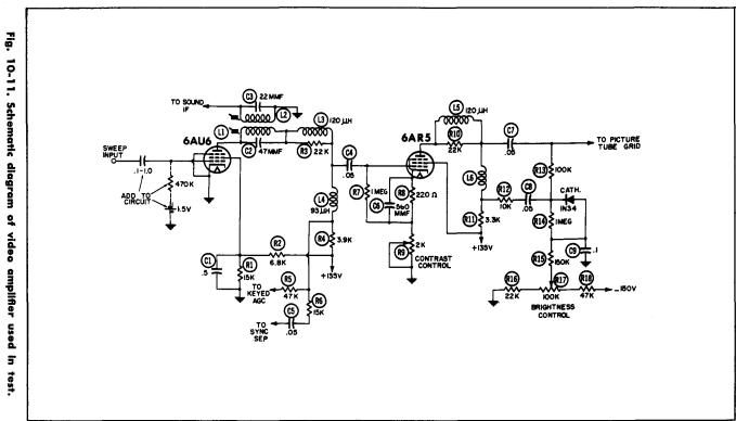
470K-ohm resistor and a 1.5-volt battery are connected in series from the video-amplifier grid to ground. The coupling capacitor should be as large a value as possible (.1 to 1.0 mfd). In circuits where fixed bias is applied to the video-amplifier grid and capacitive coupling is used, only the detector-load circuit need be disconnected.
