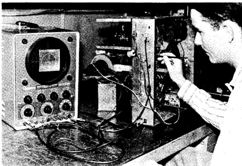
**Fig. 7-9. "Pic-Probe" and scope together substitute for picture tube.**
