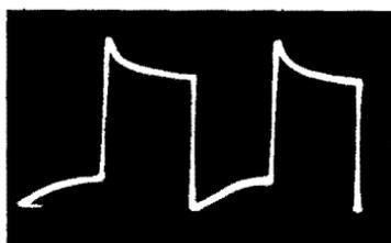
**Fig. 10-3.** Treble emphasis applied to a square wave signal.
