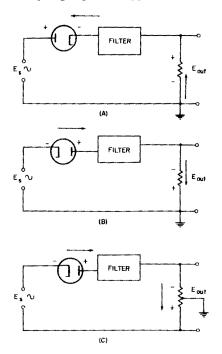
Fig. 2-4. Several variations of half-wave rectifier circuits.
