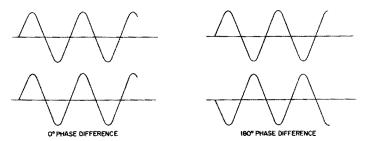
Fig. 9-14. Phase comparisons using an electronic switch.
