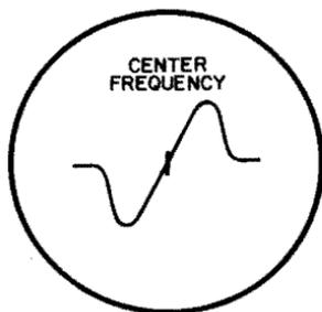
Fig. 11-14. FM discriminator or ratio detector response curve.
