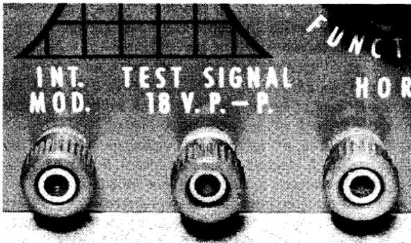
**Fig. 6-1. Source of calibration voltage located on front panel of oscilloscope.**
