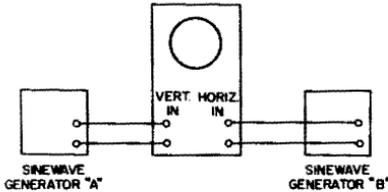
**Fig. 9-1. Method for generating Lissajous figures.**
