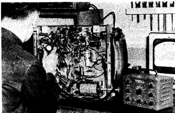
**Fig. 6-8. Probescope Model PO-1 being used to view waveforms in a TV receiver.**
