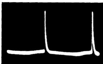
**Fig. 12-6.** Vertical pulses from the output of the vertical integrator network.
