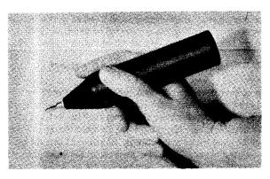
Fig. 6-7. Probe assembly of the Probescope Model PO-1.
