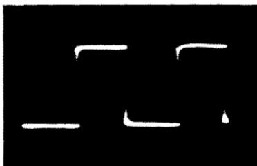
**Fig. 10-1.** A 1-kc square wave applied directly to the oscilloscope input.
