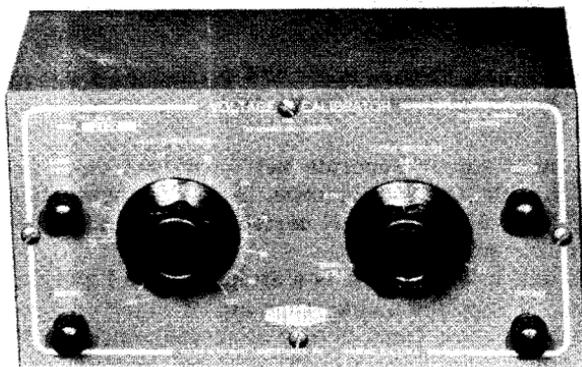
**Fig. 7-12C. Dumont Type 264-B voltage calibrator.**
