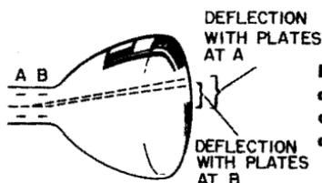
**Fig. 1-8. Given equal deflection voltages, deflection plates nearer the base of the cathode-ray tube will have the greater deflection sensitivity.**
