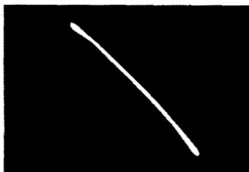
**Fig. 12-13A.** Triode operating characteristic with small overload.
