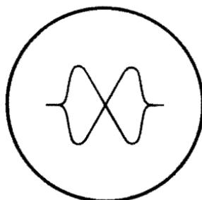
Fig. 11-15. Double response curve of FM detector.
