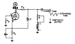
Fig. 3-4. Basic Thyratron sawtooth oscillator.
