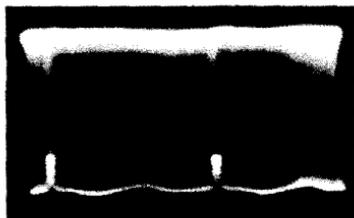
**Fig. 12-5.** Video signal after one stage of sync separation. Most of the video information has been removed.
