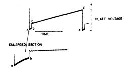
Fig. 3-21. Waveform at plate of vertical blocking oscillator in a TV receiver.
