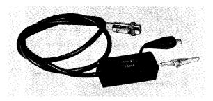
Fig. 7-7. The Simpson chromatic probe.
