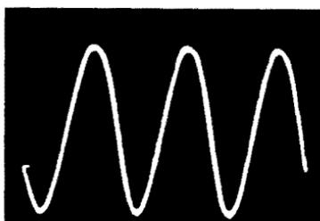
**Fig. 12-12B.** Sine-wave output of triode.
