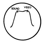
Fig. 11-12. Idealized tuner response curve.
