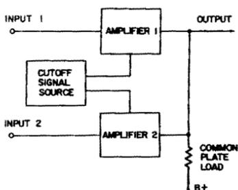
Fig. 7-16. Block diagram of an electronic-switch circuit.
