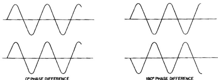
**Fig. 9-14. Phase comparisons using an electronic switch.**
