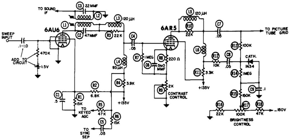
Fig. 10-11. Schematic diagram of video amplifier used in test.
