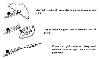
Fig. 11-9. RF (or marker) generator signal may be injected by being loosely coupled to receiver circuits.
