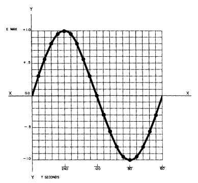
Fig. 1-1. Graph of one sycle of power-line voltage. Frequency is 60 cycles per second.
