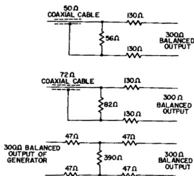
Fig. 11-5. Sweep generator attenuator pads.
