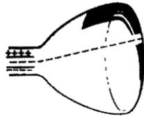
toward the positive plate and repelled from the negative plate (Fig. 1-6) because unlike electron charges attract and like charges repel each other. The electron beam is always negative and, therefore, is always attracted to the positive plate.
