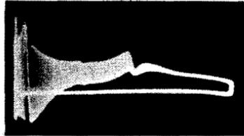
**Fig. 10-13.** Response curve showing distortion introduced by input capacity of oscilloscope.
