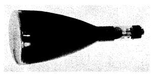
Fig. 1-3. Modern 5-Inch cathode-ray tube.
