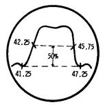
When the receiver is aligned for reception of normal strength TV signals, RF and video IF stages should be maintained at the same bias level that would be obtained with signals of this strength. In some amplifiers, the over-all response may change as the operating bias is changed. Therefore, to insure best response during actual reception, the receiver is aligned with normal operating bias. This also helps avoid adjustment of any stage to an overload condition.
