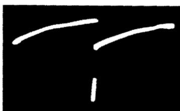
**Fig. 12-7.** Vertical deflection waveform from vertical output stage.
