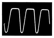
Fig. 12-14B. Greatly distorted output.
