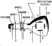
Fig. 2-1. Control elements in a 5UP1 cathode-ray tube.
