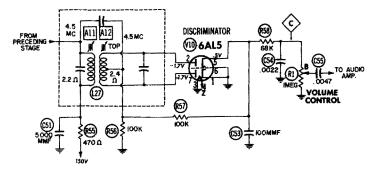
Fig. 11-7. Typical FM discriminator circuit.
