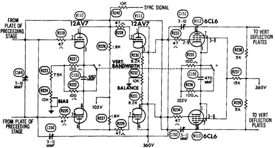
Fig. 5-2. Partial schematic diagram of the vertical amplifier of the Hickok Model 770 oscilloscope.
