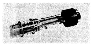
Fig. 1-4. Electron gun of cathode-ray tube.
