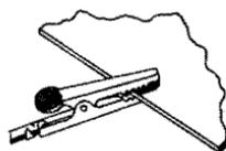
Clip "hot" lead of RF generator to chassis at appropriate point.
