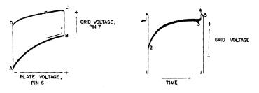
Fig. 3-19. Cyclogram comparing plate voltage variations on pin 6 with grid voltage variations on pin 7 for circuit of Fig. 3-12.
