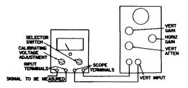
STEP 1 Connect scope, scope calibrator, and signal source as shown.
