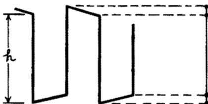
Fig. 7-14. Correct reference height of calibrating voltage.
