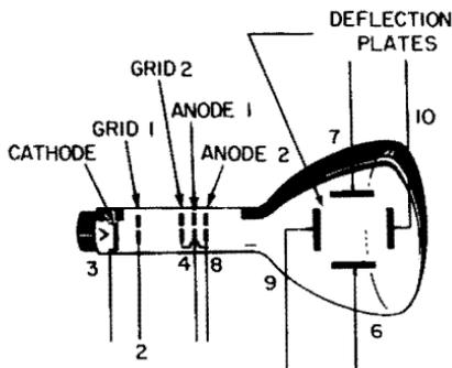
**Fig. 2-1. Control elements in a 5UP1 cathode-ray tube.**
