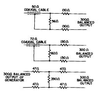
Fig. 11-5. Sweep generator attenuator pads.
