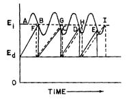
In Fig. 4-2 we have used a sine-wave signal in order to simplify the explanation. The signal is assumed to be taken from a point in the vertical amplifiers and therefore is exactly like the signal to be viewed on the oscilloscope screen, except for amplitude.
