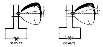
Fig. 1-7. The amount of deflection is directly proportional to the voltage applied to the plates.
