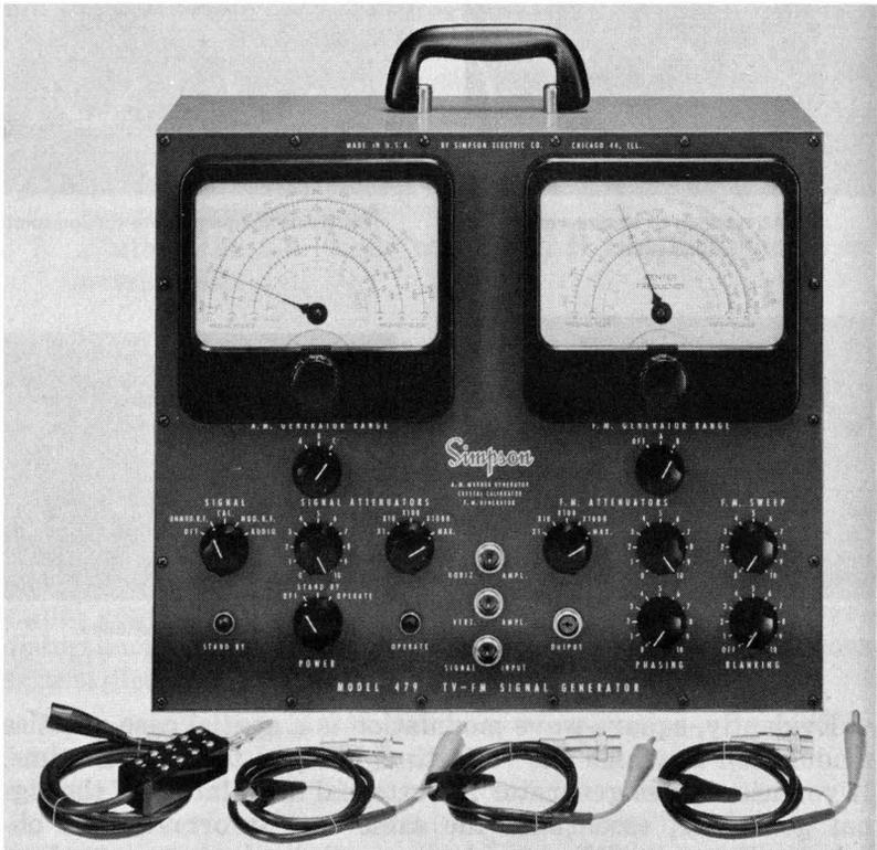
Fig. 3-17. Typical fm/am generator.
