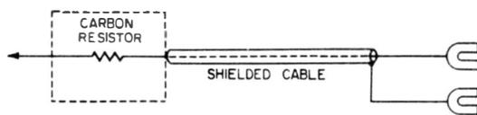
**Fig. 7-1. A simple isolation probe.**
