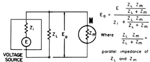
(B) External impedance connected across voltage source.
