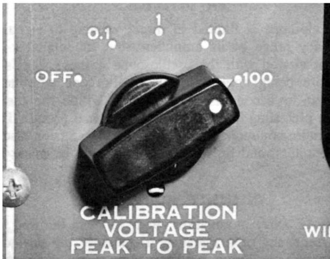
**Fig. 6-4. This oscilloscope permits the use of four different calibrating voltages.**
