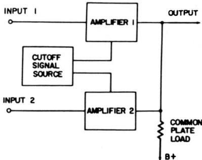
Fig. 7-17. Block diagram of an electronic-switch circuit.
