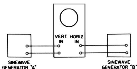
Fig. 9-1. Method for generating Lissajous figures.
