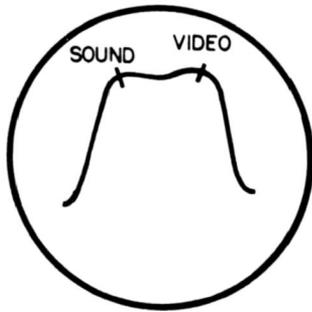
Fig. 11-14. Idealized tuner response curve.
