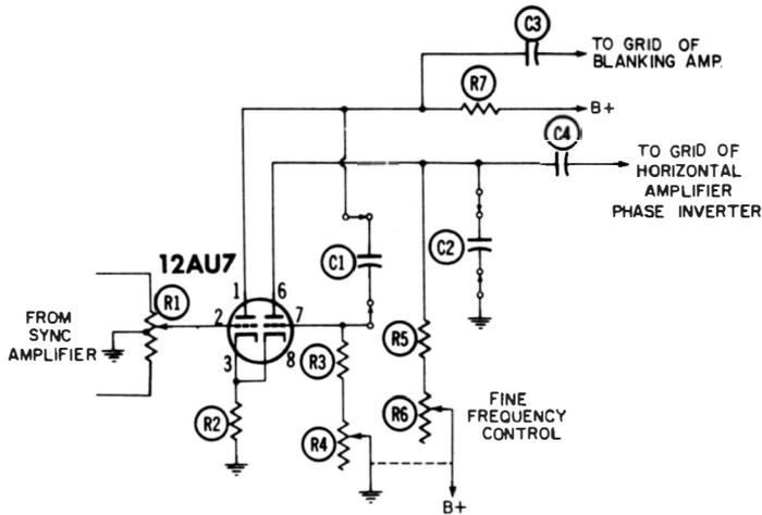
Fig. 3-16. Multivibrator sweep generator used in Simpson Model 466 Handiscope.
