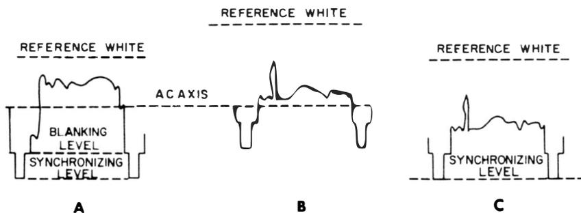
Fig. 5-3. The appearance of video signals at the picture tube as viewed on oscilloscope having d-c amplifiers.
