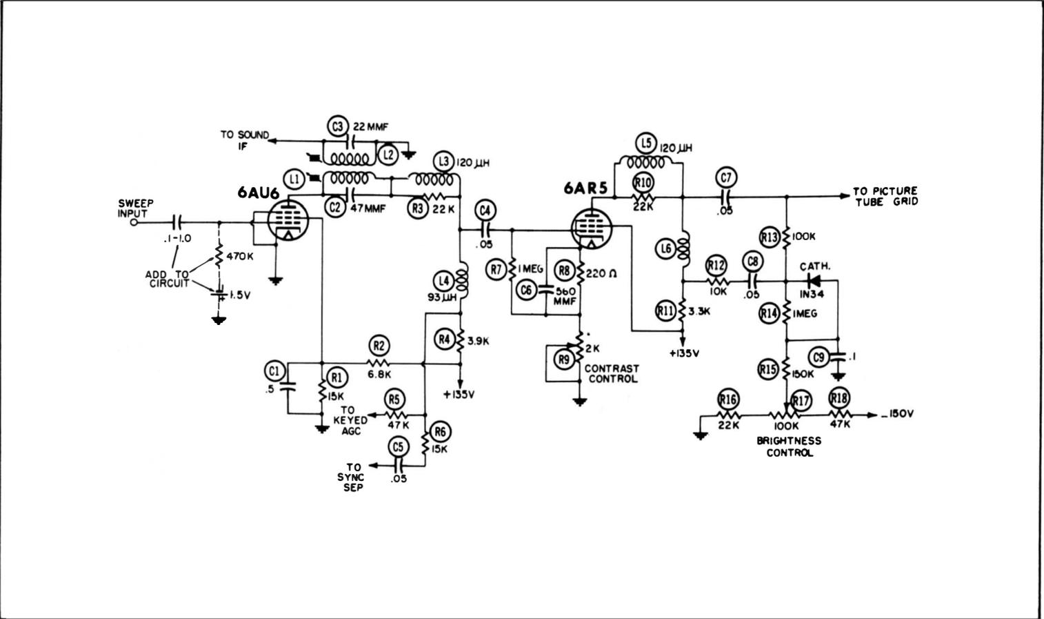
Fig. 10-11. Schematic of video amplifier used in test.
