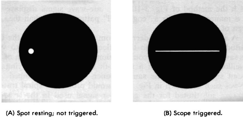
**Fig. 3-13. Trigger control of the cathode-ray tube beam.**
