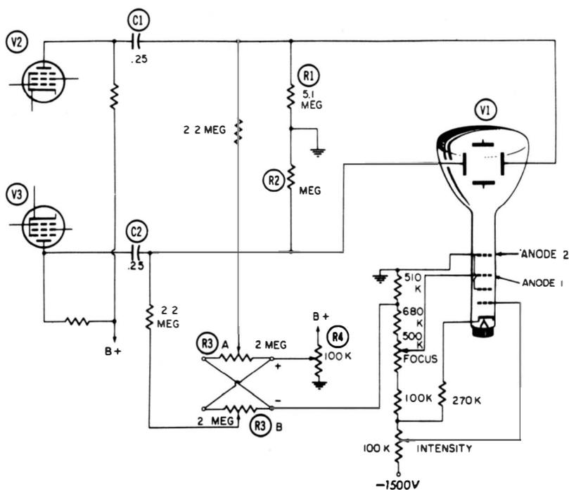
**Fig. 2-6. Partial schematic showing the positioning control and high-voltage divider network of an oscilloscope (Triplet Model 3441).**
