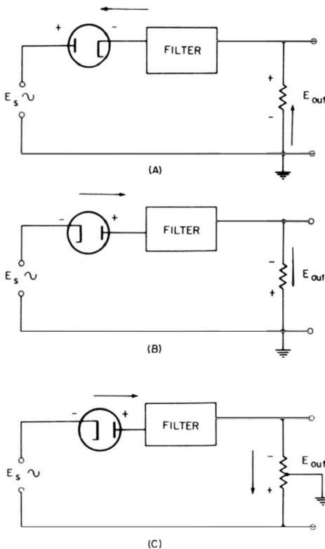
**Fig. 2-5. Several variations of half-wave rectifier circuits.**
