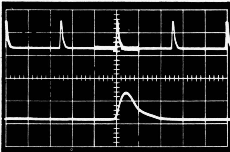
**Fig. 6-11. Illustrating a dual-beam display.**
