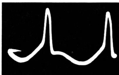
**Fig. 12-9. Waveform obtained at the second grid of the horizontal multivibrator stage.**
