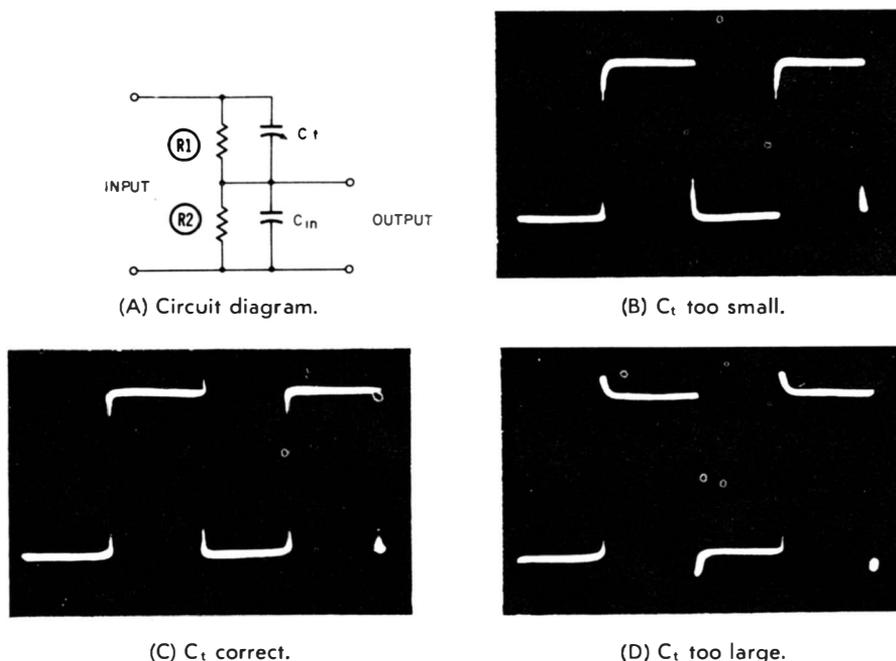
**Fig. 8-3. A frequency compensated attenuator and the effect of various degrees of adjustment on a square-wave signal.**
