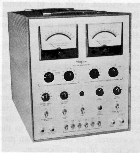
Fig. 7-22. A lab-type pulse generator.
