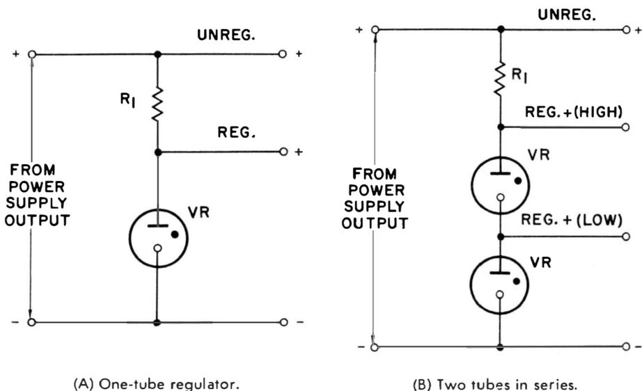
Fig. 2-3. Basic configuration for voltage regulator tubes.
