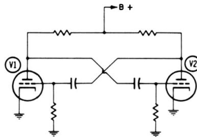
Fig. 3-7. Basic multivibrator circuit.
