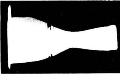
Fig. 10-20. Response curve showing misadjustment of 4.5-megahertz trap.
