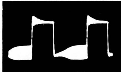
Fig. 10-8. Instability shown by continuous oscillation when square wave is applied.
