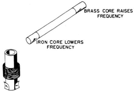
composition, similar to the tuning slugs. When the iron end of the wand is brought next to a coil, the inductance of the coil is increased, lowering the resonant frequency. Conversely, when the brass slug is placed next to the coil, the inductance of the coil decreases, raising the resonant frequency. The response curve is ob-
