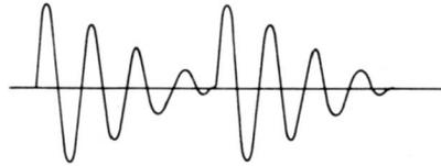
ing the signal must have a voltage rating high enough to withstand the voltage from the high-voltage supply. A much higher value of signal voltage is required for this method as compared with the method of Fig. 3-10. A square-wave signal displayed in this manner results in a “cog wheel” pattern rather than the pattern of Fig. 3-10.
