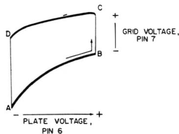
**Fig. 3-23. Cyclogram comparing plate voltage variations of pin 6 with grid voltage variations on pin 7 for circuit of Fig. 3-16.**
