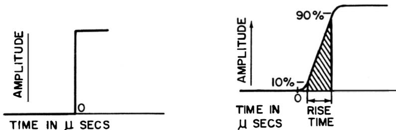
Fig. 5-6. Diagram illustrating rise time.
