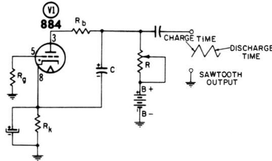
Fig. 3-4. Basic thyratron sawtooth oscillator.
