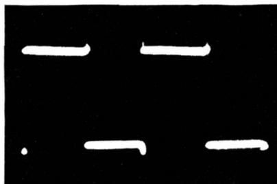
control, variously called BALANCE, AXIS SHIFT, POSITIONING, or the like, provides for separation or merging of the two traces on base lines. This is illustrated in Fig. 7-19. Thus, two waveforms can be displayed, one directly above the other, or they can be caused to merge into one trace for more exact comparison.
