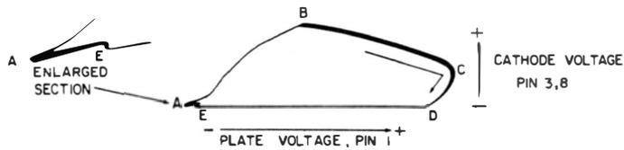
**Fig. 3-22. Cyclogram comparing plate voltage variations on pin 1 with cathode voltage variations for circuit of Fig. 3-16.**
