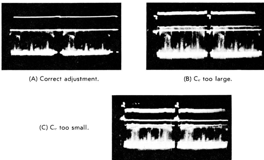
**Fig. 8-4. Video signal used in adjusting a low-capacitance probe.**
