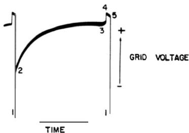
**Fig. 3-24. Waveform at grid of vertical blocking oscillator in a tv receiver.**
