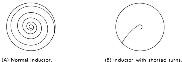
**Fig. 7-10. Test waveforms obtained with Doss probe.**
