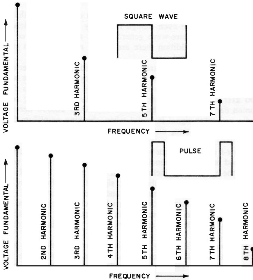
Fig. 7-23. Comparison of harmonic amplitudes in square waves and pulses.
