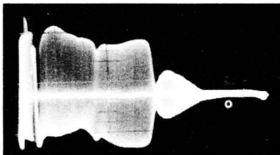
Fig. 10-12. Normal response of video amplifier.
