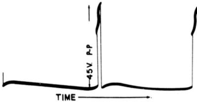
Fig. 3-17. Waveform at pin 1 (first plate) of the multivibrator of Fig. 3-16.
