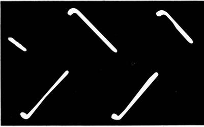
Fig. 10-5. 50-hertz square wave shows low frequency attenuation and phase shift.
