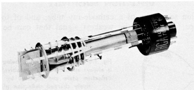
**Fig. 1-6. Electron gun of cathode-ray tube.**
