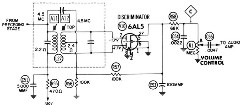
Fig. 11-8. Typical f-m discriminator circuit.
