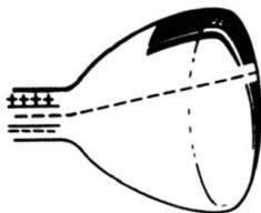
**Fig. 1-8. The electron beam, being negative, is always attracted by the positively charged deflection plate and repelled by the negatively charged deflection plate.**
