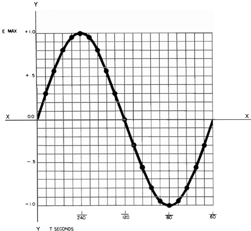
**Fig. 1-1. Graph of one cycle of power-line voltage. Frequency is 60 hertz.**
