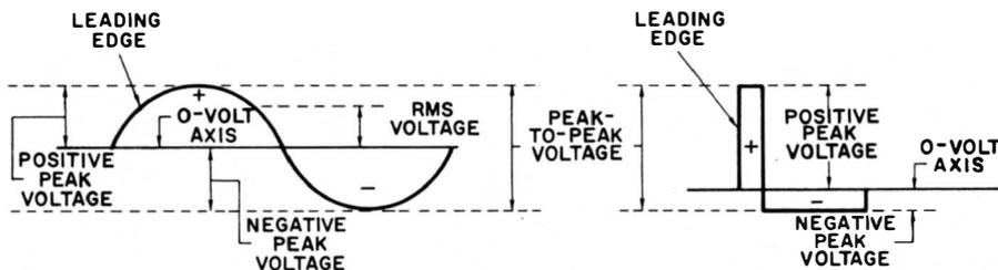
Fig. 3-12. Leading edges in sine and pulse signal waveforms.
