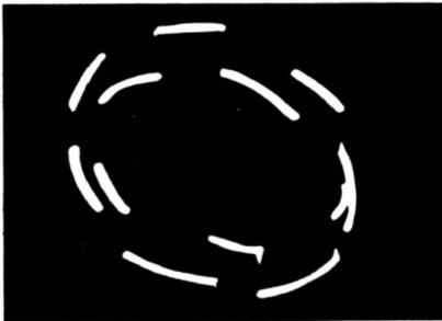
Fig. 9-5. 6-to-1 crown wheel pattern.
