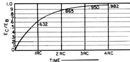
Fig. 3-3. Graph showing the rise in voltage as a capacitor is charged through a resistor.
