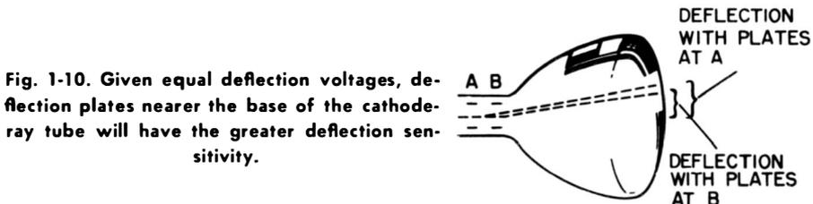
**Fig. 1-10. Given equal deflection voltages, deflection plates nearer the base of the cathode-ray tube will have the greater deflection sensitivity.**
