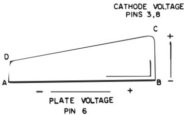
Fig. 3-21. Cyclogram comparing plate voltage variations on pin 6 with cathode voltage variations for circuit of Fig. 3-16.
