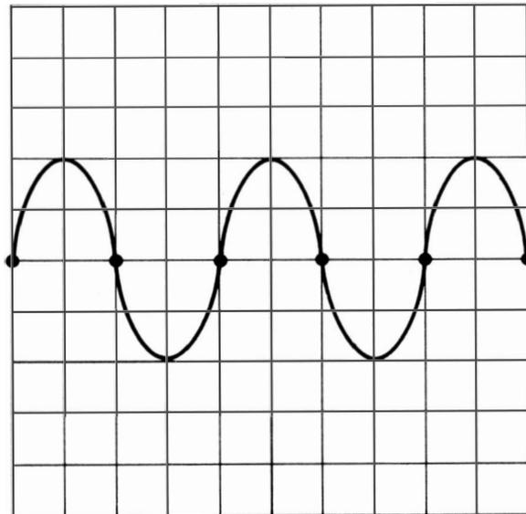
**Fig. 8-10. Checking scope sweep timing.**
