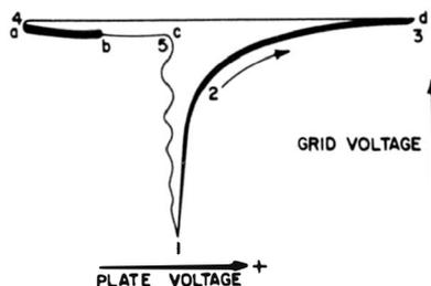
**Fig. 3-26. Cyclogram comparing plate voltage variations with grid voltage variations at the vertical oscillator of a tv receiver.**
