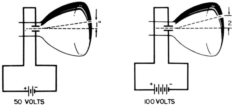
**Fig. 1-9. The amount of deflection is directly proportional to the voltage applied to the plates.**
