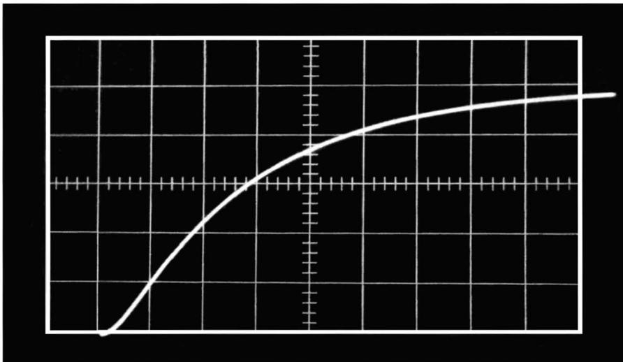
**Fig. 3-14. Expansion of the leading edge of a waveform.**
