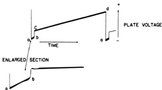
**Fig. 3-25. Waveform at plate of vertical blocking oscillator in a tv receiver.**
