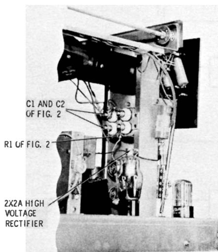
**Fig. 2-4. The high-voltage filter network in the Triplet Model 3441 oscilloscope.**
