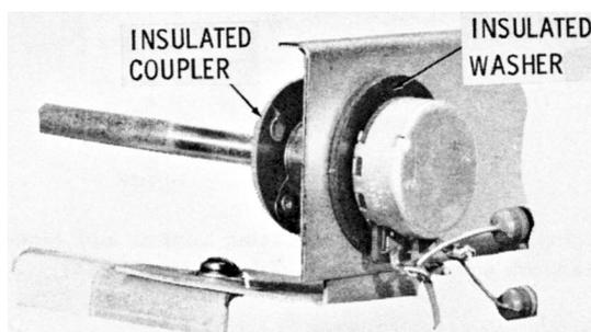
Fig. 2-7. One method of insulating between a control and the chassis.
