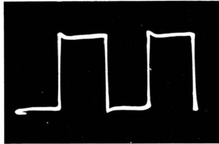
Fig. 10-2. Preamplifier response to the 1-kilohertz square wave. Tone controls were adjusted for flat response.
