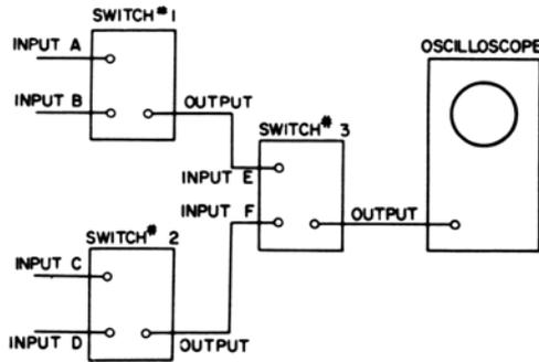
**Fig. 7-20. Electronic switch arrangement for viewing four signals simultaneously on an oscilloscope.**
