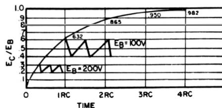
63 volts, and the deionization potential is 40 volts. Two effects of the higher value of  $E_{f1}$  can be noted: (1) a more linear sawtooth waveform, and (2) an increased frequency of the sawtooth signal. If  $E_{f1}$  were only slightly higher than the firing potential of 63 volts, the sawtooth would shift to a position near the top of the curve, the frequency would be lowered, and the waveform would become very nonlinear.
