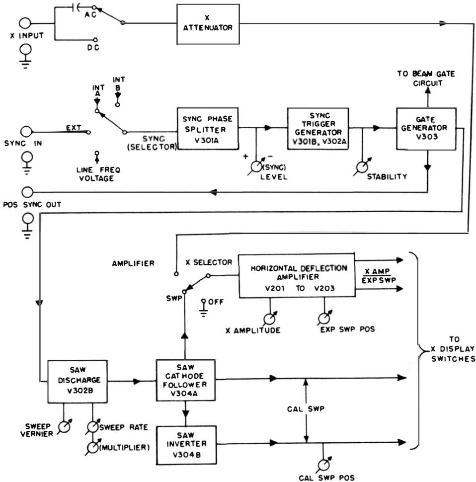
Fig. 4-5. Block diagram of a triggered-sweep system.
