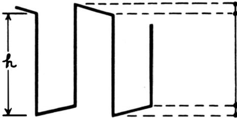
Fig. 7-15. Correct reference height of calibrating voltage.
