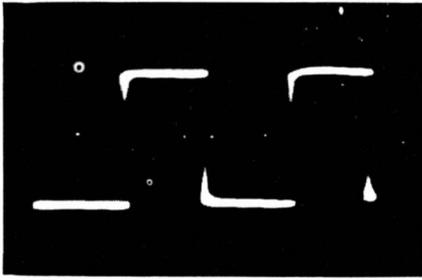
Fig. 10-1. A 1-kilohertz square-wave applied directly to the oscilloscope input.
