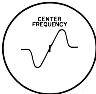
Fig. 11-16. F-m discriminator or ratio detector response curve.
