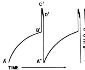
Fig. 3-20. Waveform at pin 7 (second grid) of multivibrator of Fig. 3-16.
