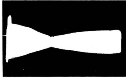
Fig. 10-19. Response curve obtained with correct adjustment of 4.5-megahertz trap.
