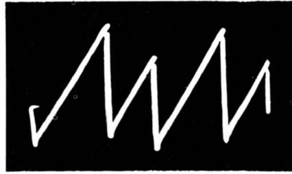
(B) Sawtooth signal developed at second section.
