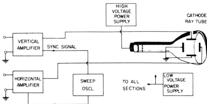
Fig. 1-4. Simplified block diagram of general-purpose oscilloscope.
