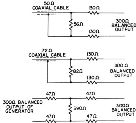
Fig. 11-6. Sweep generator attenuator pads.
