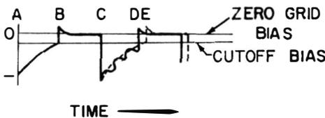
Fig. 4-4. Synchronization of a multivibrator sweep circuit.
