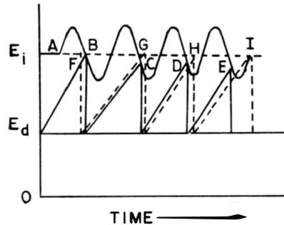
**Fig. 4-2. Synchronization of a thyatron sweep generator by means of a sine-wave signal.**
