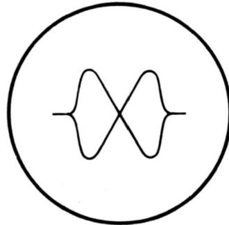
Fig. 11-17. Double response curve of f-m detector.
