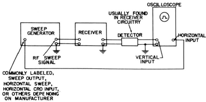
Fig. 11-4. Minimum equipment necessary to obtain a response curve.
