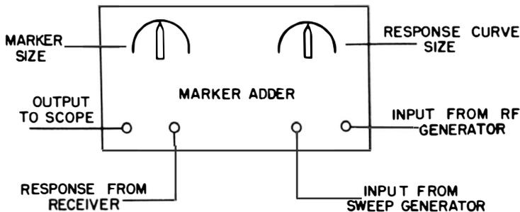
**Fig. 11-11. Block diagram showing connections when using marker adder unit.**
