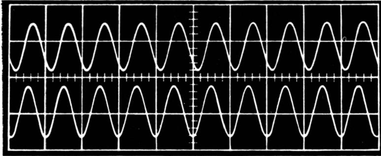
Fig. 9-15. Phase measurement with a dual-trace scope.
