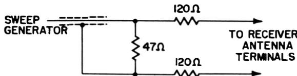
(C) Schematic of terminating network.
