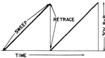
Fig. 3-19. Waveform at pin 6 (second plate) of multivibrator of Fig. 3-16.
