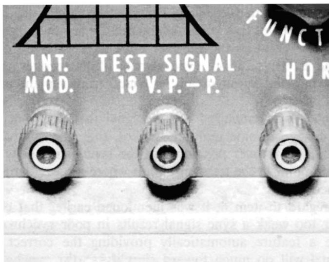
Fig. 6-1. Source of calibration voltage located on front panel of oscilloscope.
