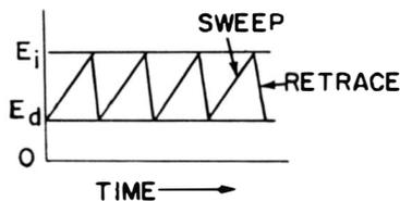
Fig. 4-1. Free-running operation of a thyatron sweep oscillator.
