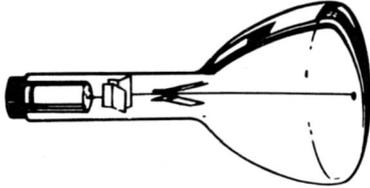
**Fig. 1-7. Path of electron beam through deflection-plate assembly.**
