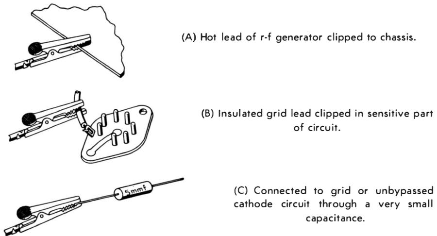
**Fig. 11-10. R-f (or marker) generator signal may be injected by being loosely coupled to receiver circuit.**
