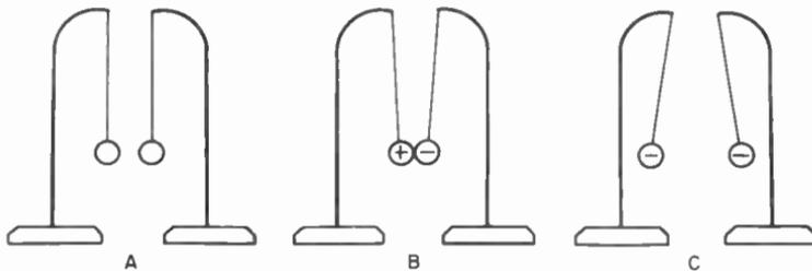
Fig. 3-4. If two pith balls are used, the same law of attraction and repulsion applies.
