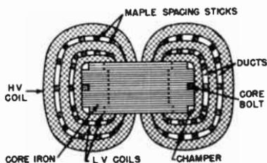
Fig. 11-22. Details of a core-type transformer winding.
