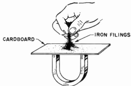
**Fig. 8-8.** The pattern of the lines of force can be shown by sprinkling iron filings over a cardboard placed over a magnet.
