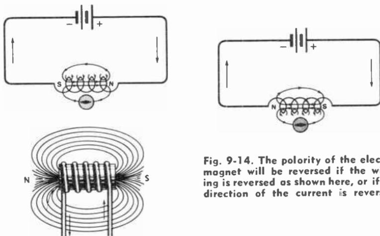
Fig. 9-14. The polarity of the electromagnet will be reversed if the winding is reversed as shown here, or if the direction of the current is reversed.
