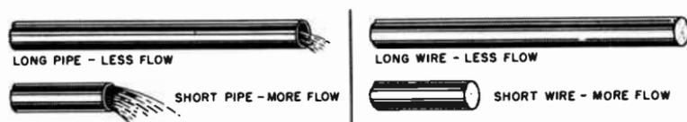
**Fig. 4-8. Water meets less resistance in a short pipe than in a long one. In like manner electricity finds less resistance in a short conductor than in a long one.**
