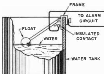
Fig. 14-15. A "Float" switch for controlling the level of water in a tank.
