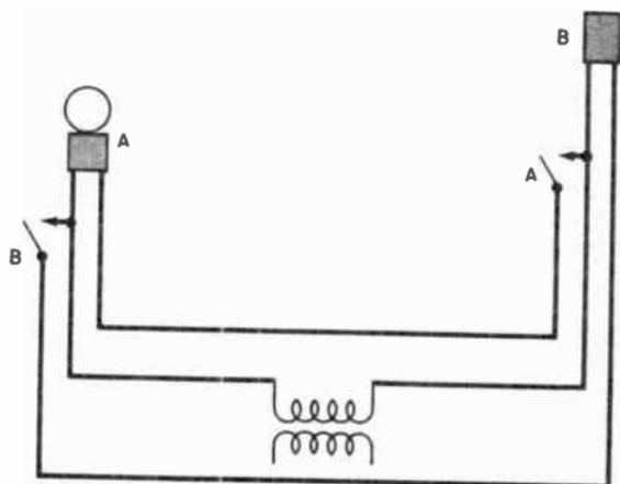
Fig. 14-25. A return-call system circuit.
