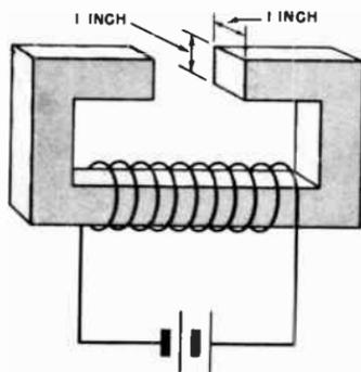
Fig. 9-22. How the cross-sectional area of magnetized iron is measured.
