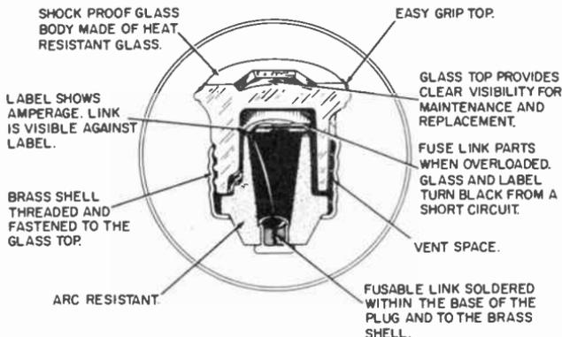
**Fig. 5-1. Cross-sectional view of a fuse plug showing its various parts.**
