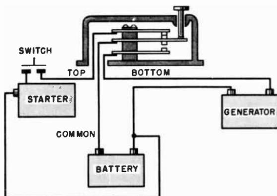
**Fig. 14-8.** How the principle of the two-contact switch can be applied to the automatic control of an automobile electric system.
