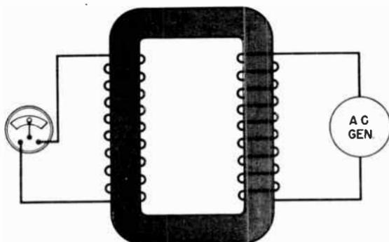
**Fig. 11-30.** By connecting the first coil to a source of AC voltage, we can cause the magnetic lines of force in the iron to keep continually moving, and continually inducing a voltage in the second coil.
