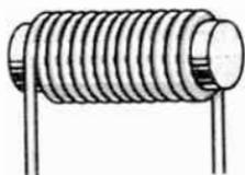
Fig. 9-13. The solenoid will draw the bar of iron within itself.
