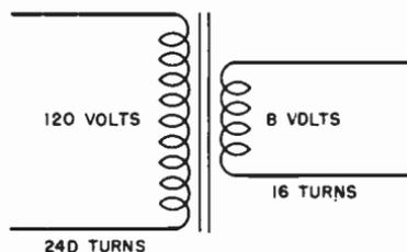
**Fig. 11-36.** How the 8 volts for a door bell are obtained from the 120-volt house-circuit voltage by using a transformer.
