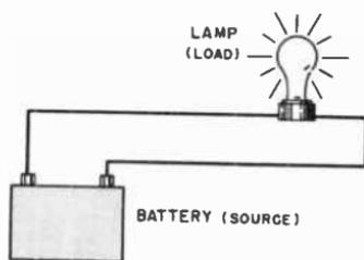
Fig. 4-13. An electric circuit showing the source and the load.
