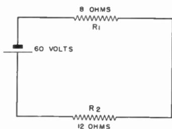
$$\begin{aligned} \text{TOTAL RESISTANCE} &= 12 + 8 = 20 \text{ OHMS} \\ \text{TOTAL CURRENT} &= \frac{60}{20} = 3 \text{ AMPERES} \\ \text{VOLTAGE DROP ACROSS } R_1 &= 8 \times 3 = 24 \text{ VOLTS} \\ \text{VOLTAGE DROP ACROSS } R_2 &= 12 \times 3 = 36 \text{ VOLTS} \\ \text{TOTAL VOLTAGE DROP} &= 24 + 36 = 60 \text{ VOLTS} \end{aligned}$$
