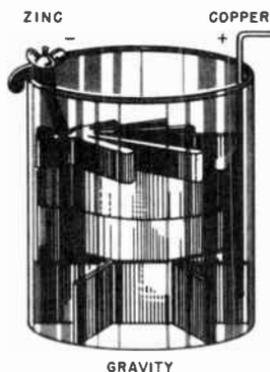
Fig. 4-18. A "crow's foot" electric cell such as was once widely used in telegraph work.
