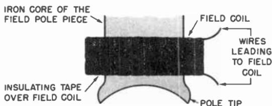
**Fig. 12-24.** How the field coil is mounted on the iron core.
