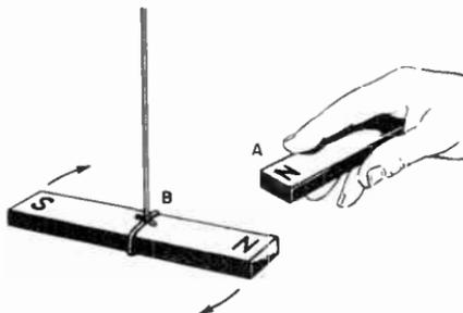
Fig. 8-5. The north pole of one magnet will repel the north pole of another magnet.
