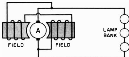
**Fig. 12-26.** Electrical circuits in a shunt generator. The field coils here are connected directly to the full output voltage of the generator.
