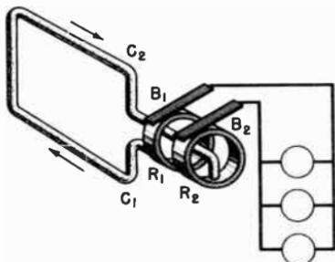
Fig. 12-14. Opening the loop and connecting the two ends of the conductor to slip rings make it possible to tap the current within the loop.
