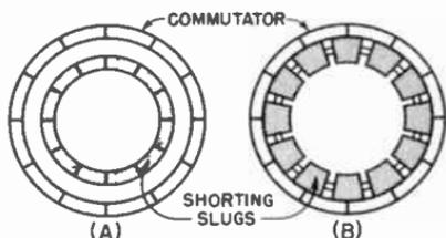
Fig. 13-29. The short circuiting "Necklace" which changes the armature of a repulsion induction motor into a squirrel cage rotor.
