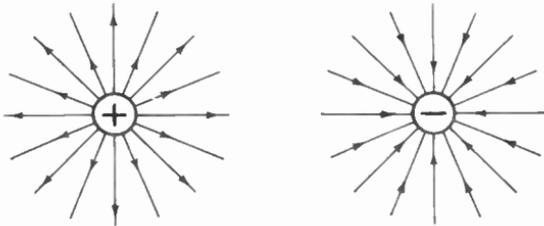
**Fig. 3-11.** The direction of electric fields about isolated positive and negative charges of static electricity.
