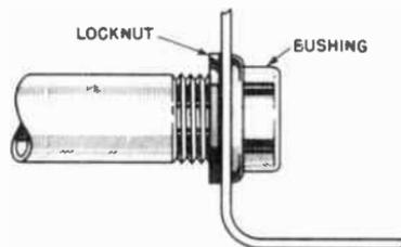
**Fig. 15-11.** How locknuts and bushings are used to fasten rigid conduit to a switch box or other metallic enclosure.
