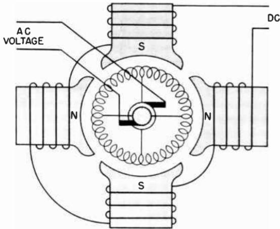
Fig. 13-3. A four-pole alternator with rotating armature.
