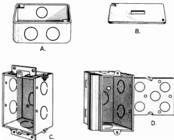
Fig. 15-33. "Switch boxes" used to enclose switches and convenience outlets.
