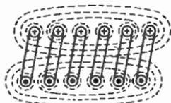
**Fig. 9-9.** How several parallel conductors are linked together with magnetic lines of force.
