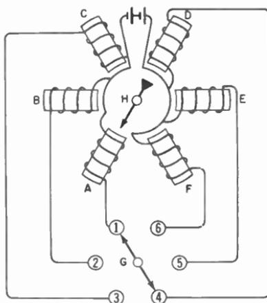
**Fig. 13-8.** This is a modified arrangement of Fig. 13-7 to show the principle of a rotating magnetic field.
