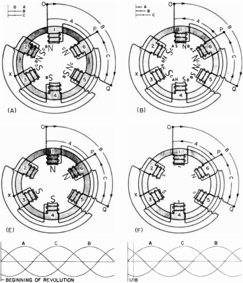
Fig. 13-17. Showing how the polarity of a three-phase
