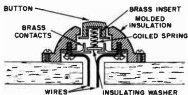
Fig. 14-4. Construction details of a push button.
