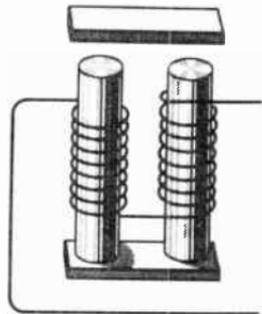
Fig. 14-16. Basic construction of an electromagnet.
