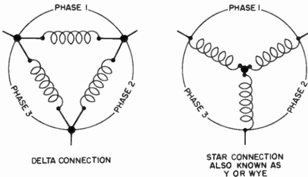
Fig. 13-15. Two methods of connecting a three-phase motor stator winding.
