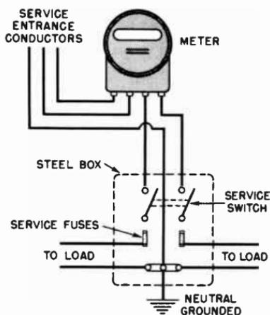
**Fig. 15-19.** Electrical connections to a meter, a switch, and a main fuse.
