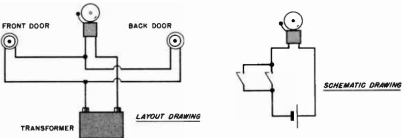
Fig. 14-24. A door bell controlled by two pushbuttons.
