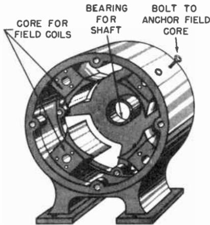
Fig. 12-21. The end bells and field cores are mounted on the frame. The bearings in the end bells receive the shaft on which the armature rotates.
