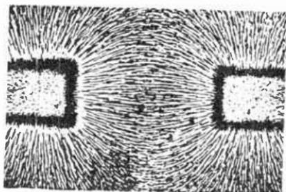
Fig. 8-9. The pattern assumed by the lines of force.
