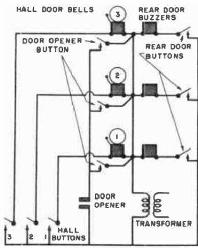
Fig. 14-27. A signal system commonly used in apartments.
