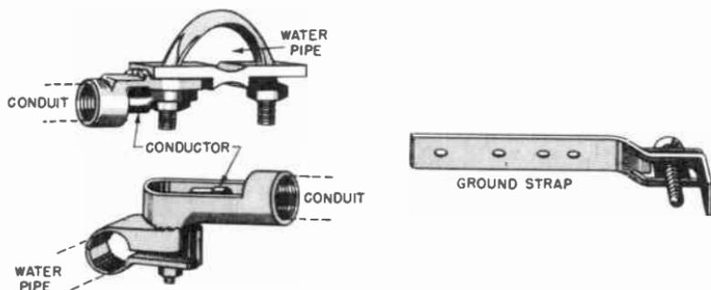
Fig. 15-22. Types of ground clamps and straps.
