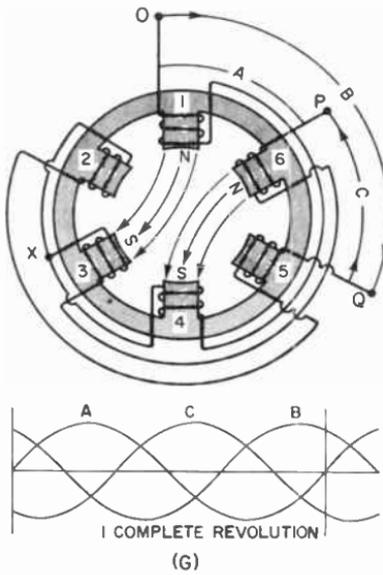
or rotates within the stator of a three phase motor.
