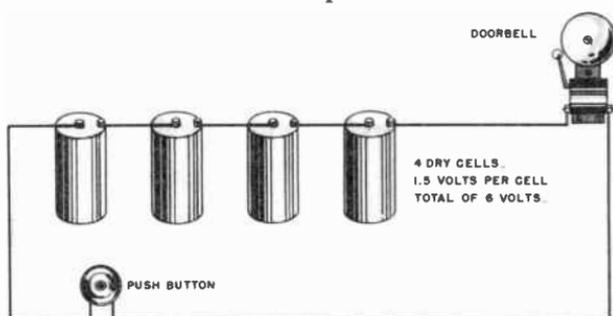
Fig. 14-1. A simple signal circuit powered from dry-cell battery.
