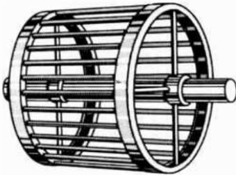
**Fig. 13-10. An elementary squirrel cage rotor.**
