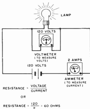
**Fig. 7-4.** Measuring the hot resistance of a lamp by using Ohm's law.
