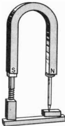
Fig. 8-19. A permanent magnet will induce magnetism in soft iron.
