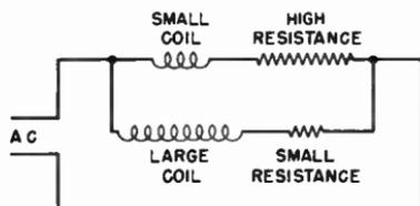
**Fig. 13-21.** Even though there is a resistance and a coil in each branch of the circuit there will be a splitting of the phase according to the amount of resistance and inductance in each branch.
