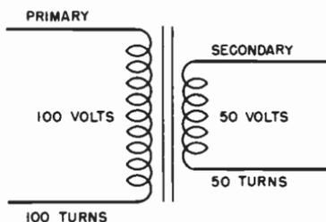
**Fig. 11-35.** If there are only one-half as many turns on the secondary as on the primary, there will be only one-half as much voltage.
