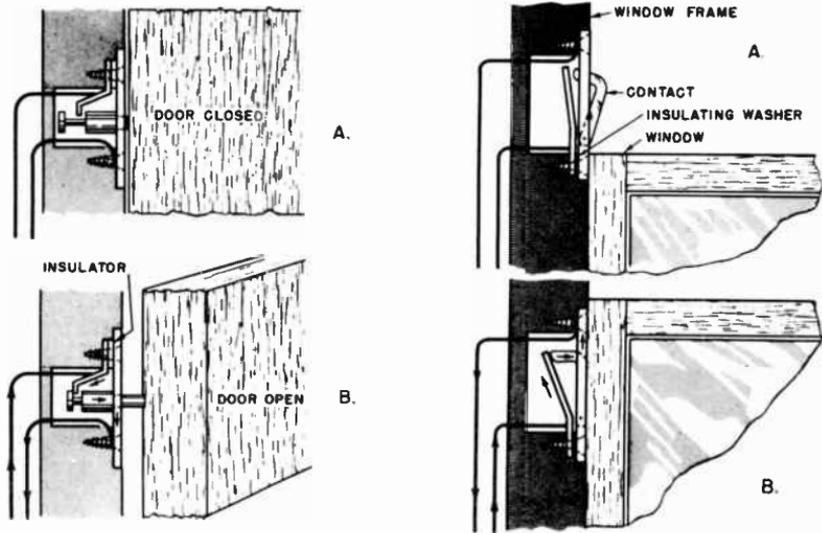
Fig. 14-12. A plunger-type door switch.
