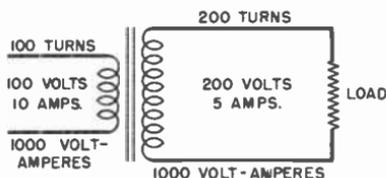
**Fig. 11-37.** As the transformer steps up the voltage, it automatically steps down the current.
