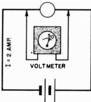
$$\begin{aligned} \text{POWER} &= 50 \times 2 \\ 50 \times 2 &= 100 \text{ WATT} \end{aligned}$$
