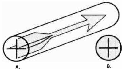
**Fig. 9-6. How an arrow is used to show the movement of current away from the observer.**
