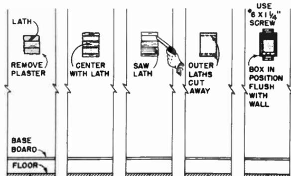
Fig. 15-37. Preparing a hole in the lath for a switch box.
