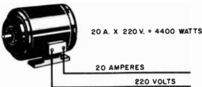
Fig. 10-12. The power delivered by an electrical source is equal to the product of the current and the voltage.
