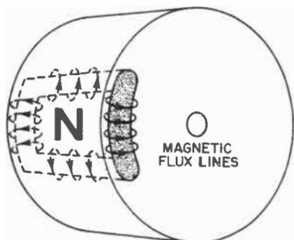
Fig. 13-13. How a current, induced in a short-circuited inductor of a squirrel cage rotor produces a magnetic field about itself.
