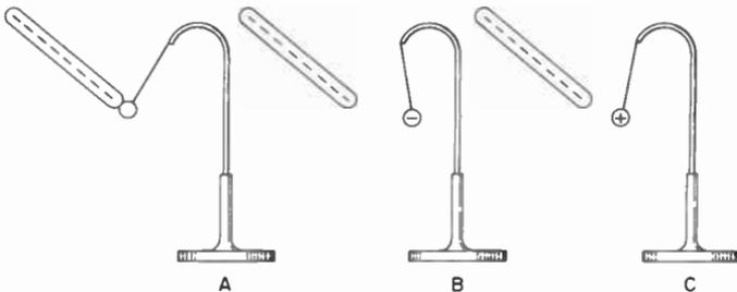
**Fig. 3-3. Placing a charge on a pith ball electroscope. Electric charges may be identified and their forces of attraction and repulsion observed.**
