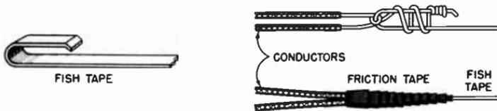
**Fig. 15-16. How conductors are fastened to fish tape for pulling.**
