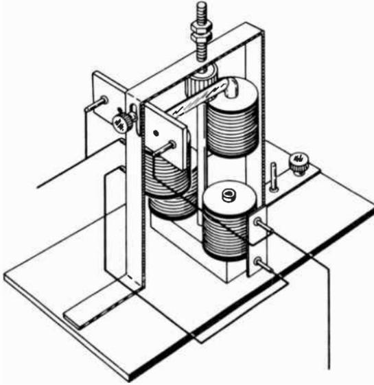
Fig. 12-3. The experimental direct-current generator assembled ready for operation.
