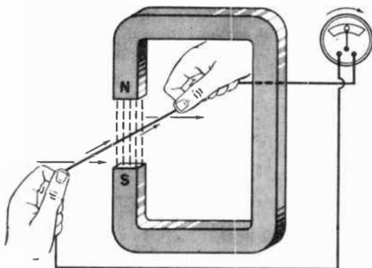
Fig. 11-25. Moving a conductor across magnetic lines of force at right angles to them induces a voltage in the conductor.
