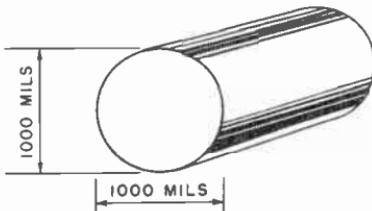
**Fig. 6-4.** The cross-sectional area of a conductor is one of the factors that determines the amount of current it will carry. The cross-sectional area is measured in circular mils.
