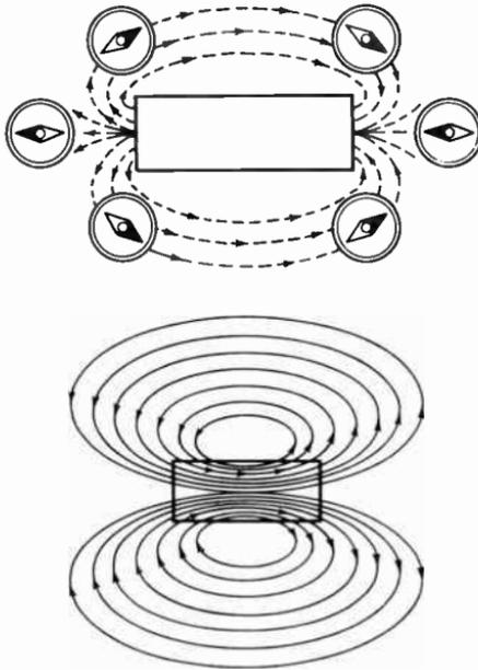
**Fig. 8-11. The lines of force assume direction in the manner shown.**
