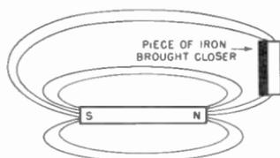
**Fig. 8-13.** When iron is moved closer, some of the lines of force enter it and try to draw it nearer the magnet.
