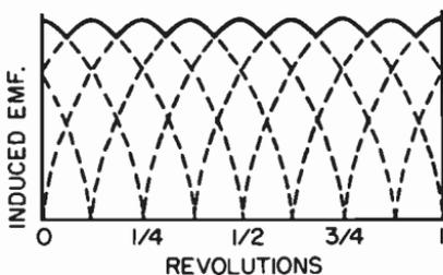
Fig. 12-18. An elementary four-coil armature and the fluctuating voltage waveform produced by it.
