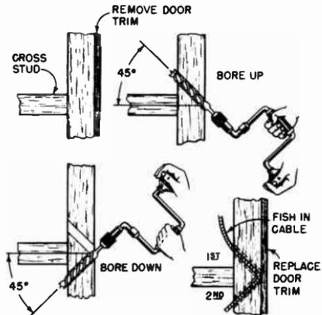
Fig. 15-31. Bypassing an obstruction without seriously marring the wall.
