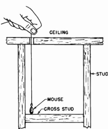
Fig. 15-30. How obstructions within a wall can be located.
