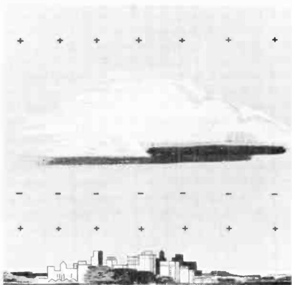
**Fig. 3-18.** During fair weather the earth's surface may be negatively charged, but it becomes positively charged by induction when a negative cloud passes over. (Courtesy of Westinghouse Mfg. Corp.)
