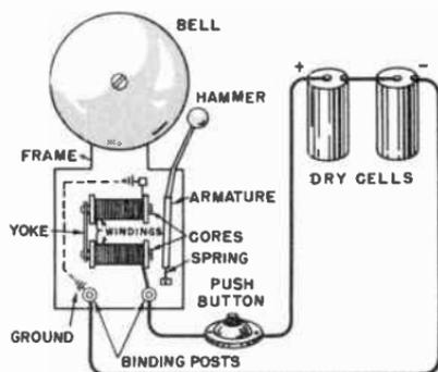
Fig. 14-18. Wiring details of a single-stroke bell.
