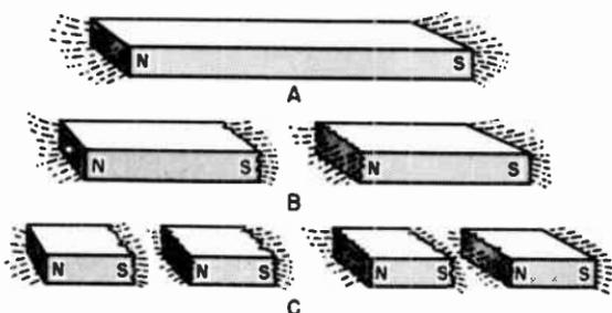
**Fig. 8-17.** Breaking a magnet results in the formation of new magnets which assume polarities as shown.
