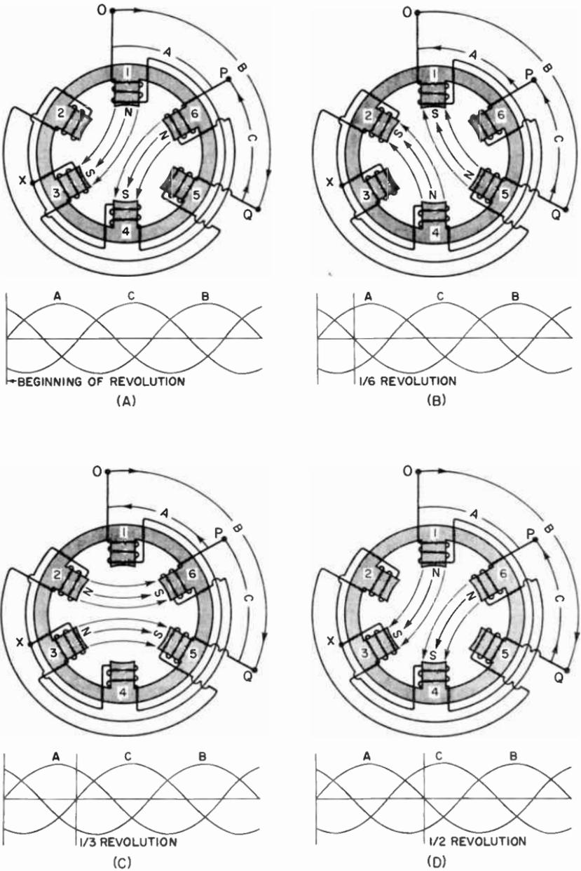
Fig. 13-16. How the rotating magnetic field shifts
