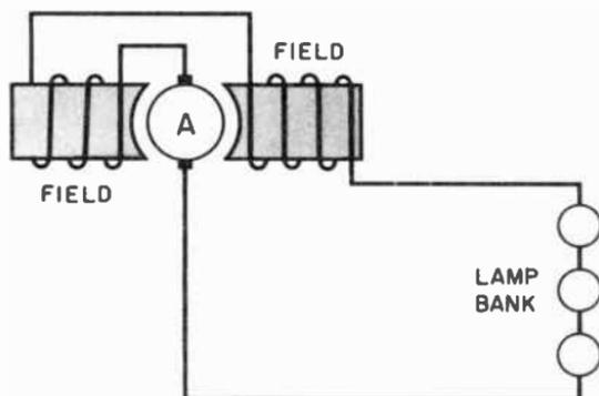
Fig. 12-25. Electrical circuit in a series generator. Note how the field coils obtain their exciting currents.
