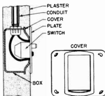
Fig. 15-35. How a "1900" box can be fitted with a cover and used as a switch box.
