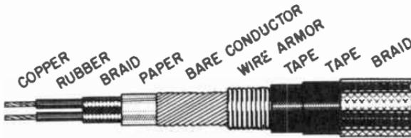
Fig. 15-17. Construction of service-entrance cable.
