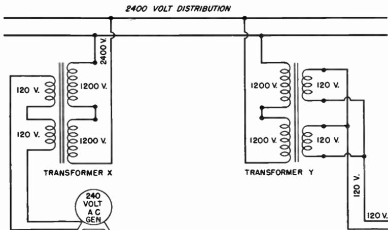
**Fig. 11-52.** Two transformers that are exactly alike can be used in two different and opposite manners.
