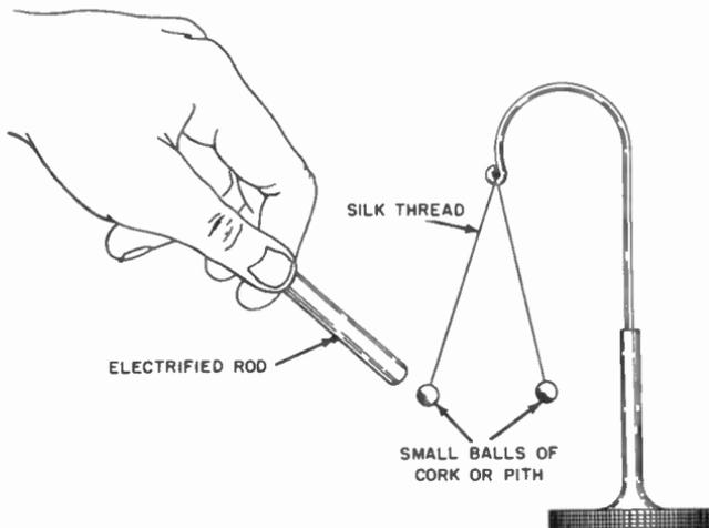
Fig. 3-5. A modified form of pith ball electro-scope.
