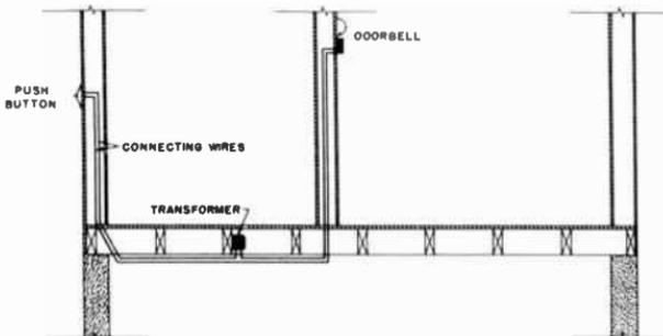
**Fig. 14-3.** How the wires are run to connect a door bell with its push-button control.
