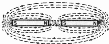
**Fig. 8-16.** How the lines of force act when the unlike poles of two magnets are brought near each other.
