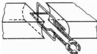
Fig. 12-16. Two loops, placed at right angles to each other and rotated at the same time make it possible to tap off a near continuous flow of current which does not drop to zero at each half-cycle.
