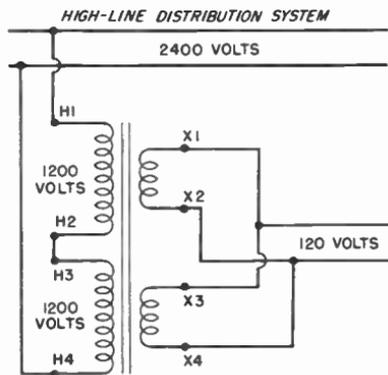
**Fig. 11-46.** The high-voltage windings are connected in series to serve as the primary for connection to 2400 volts. The low-voltage secondary windings are connected in parallel.
