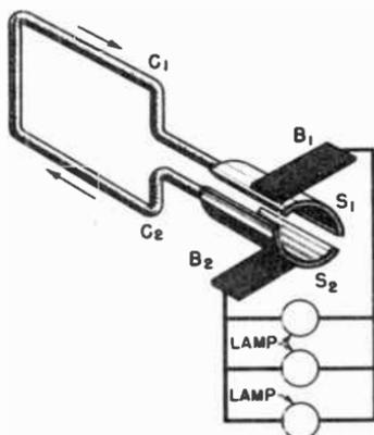
Fig. 12-15. A commutator, consisting of two or more segments, can be used to tap the current inside the rotating loop.
