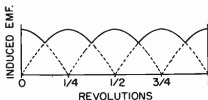
Fig. 12-17. An elementary two-coil armature and the fluctuating voltage waveform produced by it.
