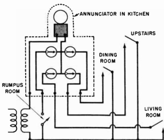
Fig. 14-32. A four-drop annunciator which would be suitable for use in a home.
