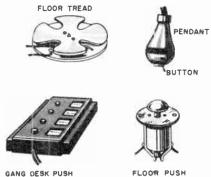
Fig. 14-9. Several types of low-voltage switches in common use.
