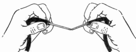
**Fig. 4-4. To make an electrical connection between two conductors it is necessary only to touch the two conductors together.**
