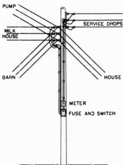
Fig. 15-5. The main fuse and main switch are often located on the meter pole.
