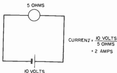
Fig. 7-1. A simple series circuit.
