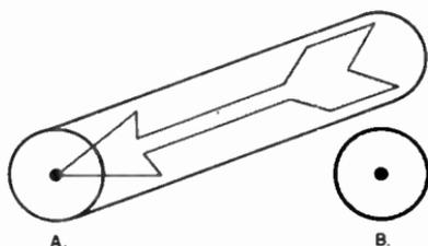
Fig. 9-4. How an arrow is used to show the direction of current flow.
