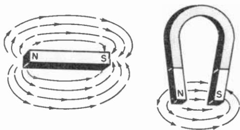
Fig. 8-10. The lines of force seem to travel in curved lines.
