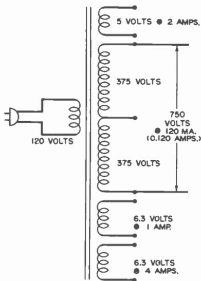
Fig. 11-53. Diagram of a typical radio power supply transformer showing primary and secondary windings.
