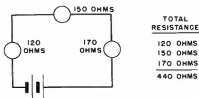
Fig. 6-10. Finding the total resistance of three resistances in series.
