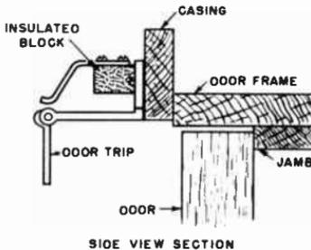
Fig. 14-10. Construction details of a door switch.
