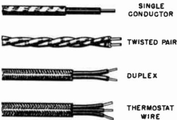
Fig. 14-21. Types of door-bell wire.
