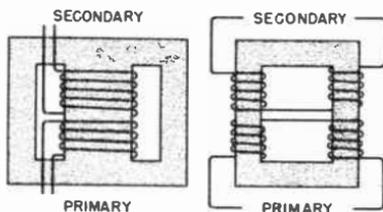
Fig. 11-18. Two common styles of transformer cores with windings.
