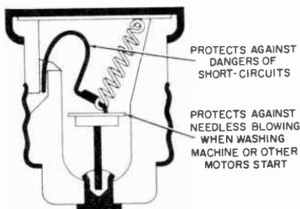
**Fig. 5-4.** Interior cross-section view of a Fusetron fuse. (Courtesy of Bussmann Mfg. Company.)
