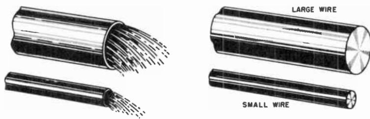
**Fig. 4-7. Just as more water can flow through a large pipe with less resistance than through a small pipe, electricity meets less resistance in a large conductor than in a small one.**
