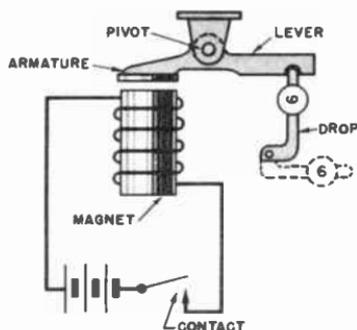
Fig. 14-31. Operating details of an annunciator drop.
