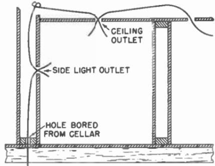
Fig. 15-28. Armored cable can be fished from outlet to outlet through the walls by using fish tapes and "snakes".
