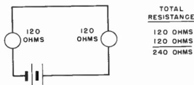
Fig. 6-9. How to determine the total resistance in a series circuit.
