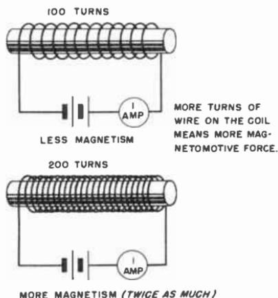
Fig. 9-16. The number of turns of wire in the coil affects the magnetic strength.
