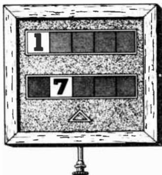
Fig. 14-29. The type of annunciator often used in rooming houses and small hotels.
