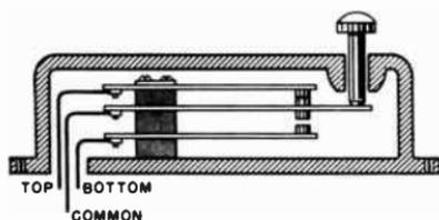
Fig. 14-6. A "leaf" or blade type two-contact switch.
