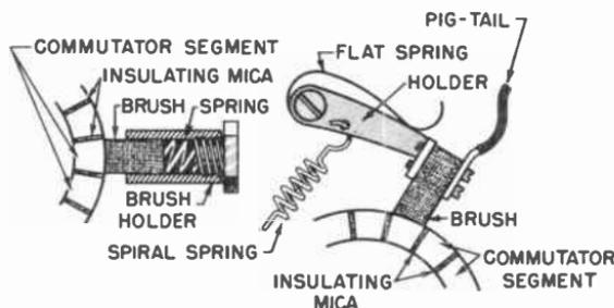
**Fig. 12-23.** How the brushes rest on the commutator. The brushes are held firmly against the commutator by spring tension. The individual segments of the commutator are separated from each other by insulating mica.
