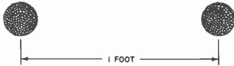
**Fig. 3-1.** Two globules of free electrons the size of small marbles placed one foot apart would repel each other with the tremendous force of 350 trillion tons.
