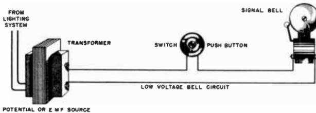
**Fig. 14-2.** A simple signal circuit powered from a transformer.
