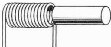
Fig. 9-12. A solenoid and a bar of iron.
