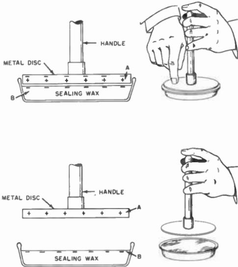
Fig. 3-14. The charges on an electrophorus.
