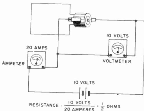
**Fig. 7-5. Measuring the resistance of a motor armature by applying Ohm's law to the measured current and voltage.**
