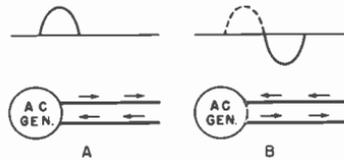
Fig. 11-48. A single-phase generator connected to a line.
