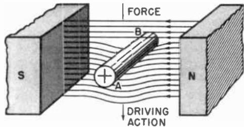
Fig. 12-10. A voltage is induced in a conductor when it is moved through a magnetic field.
