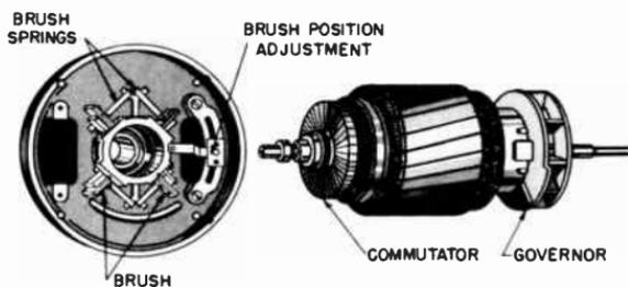
**Fig. 13-30.** The commutator of a repulsion-induction motor with the brushes and brush shifting mechanism.
