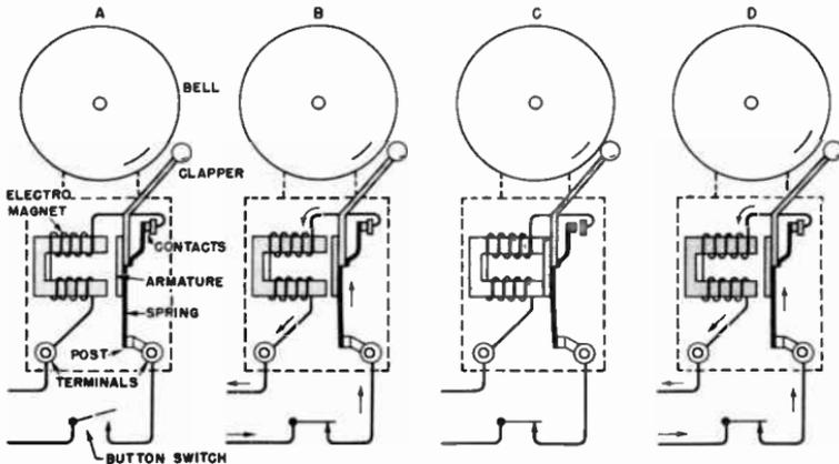
Fig. 14-17. How a vibrating bell works.
