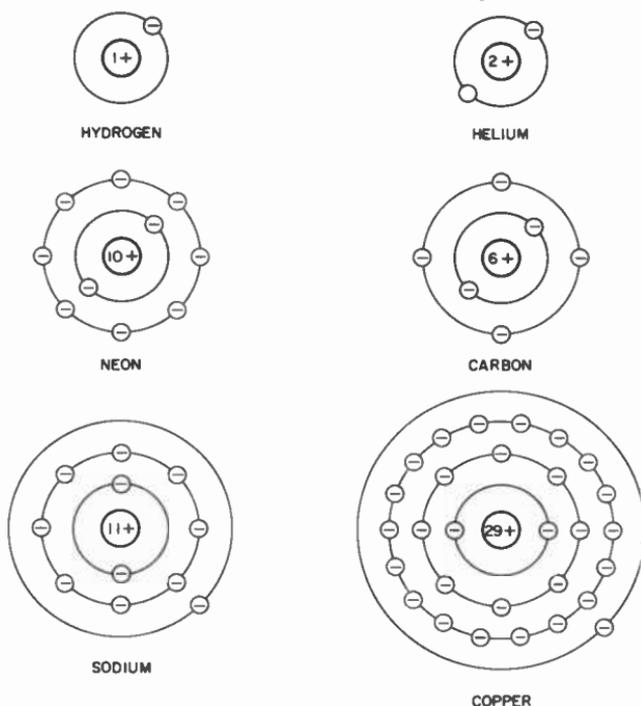
**Fig. 2-3. The dense nucleus (center) of the six elements shown contains the protons around which the electrons revolve.**
