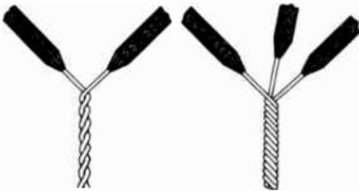
Fig. 15-40. How to make a rat-tail splice.
