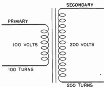
**Fig. 11-33.** If the secondary has twice as many turns as the primary, the secondary voltage will be twice as great as the primary voltage.
