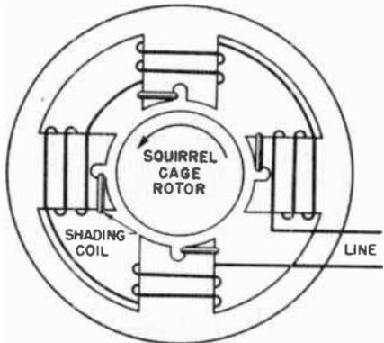
Fig. 13-31. A shaded-pole motor.
