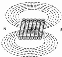
Fig. 9-11. The magnetic linkage is more complete when the turns are close together.
