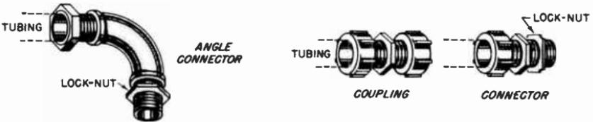
Fig. 15-14. Fittings used with thin-wall conduit.
