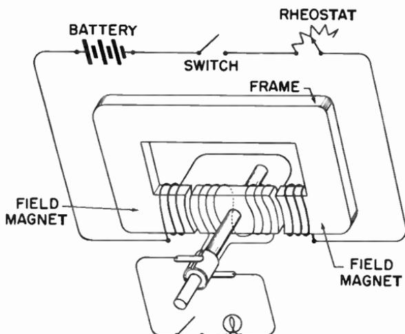
Fig. 12-6. Elementary separately-excited direct-current generator.
