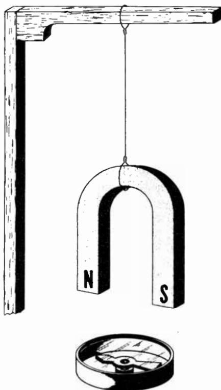
**Fig. 13-6.** An elementary demonstration to show the principle of a rotating magnetic field.
