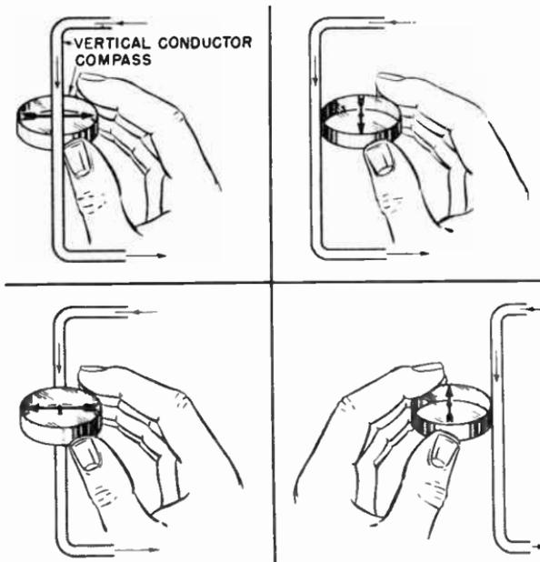
**Fig. 9-1.** The presence of a magnetic field around a conductor carrying an electric current can be detected by using a compass.
