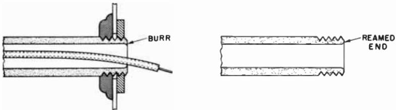
**Fig. 15-13.** End of conduit before and after reaming.
