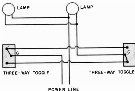
Fig. 14-36. How two three-way toggle switches can be used to control two lamps from two different positions.
