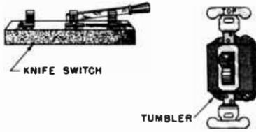
**Fig. 14-34.** A single-pole double-throw knife switch and a three-way tumbler or toggle switch.
