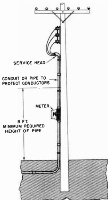
Fig. 15-3. A meter on a pole for an underground service.
