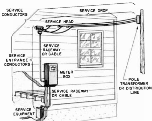
Fig. 15-2. The principal parts of an electrical service entrance.
