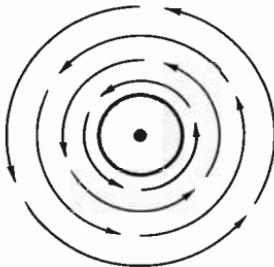
**Fig. 9-5. The magnetic lines of force form in a counterclockwise direction around a conductor when the current is moving toward the observer.**
