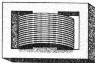
Fig. 11-20. How the coils are placed on the center leg of a shell-type transformer.
