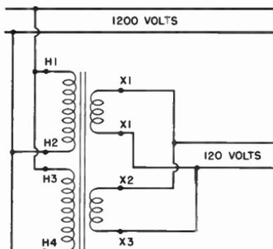
**Fig. 11-45.** Both primary windings and both secondary windings connected in parallel.
