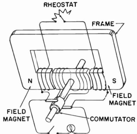
Fig. 12-7. Self-excited shunt-wound DC generator.
