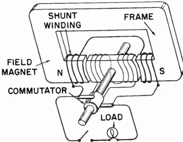
**Fig. 12-1. A simple type of elementary direct-current generator (dynamo).**
