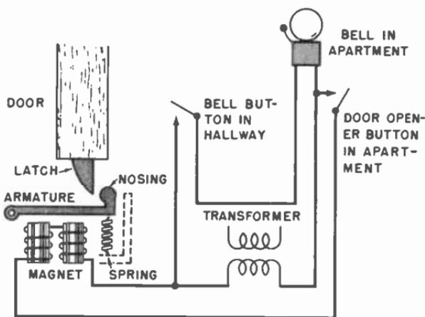
Fig. 14-28. Operating details of a door opener.
