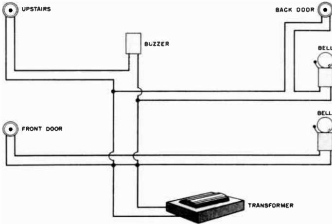
Fig. 14-23. A typical door bell signal system used in a better home.
