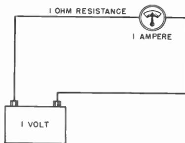
**Fig. 6-6.** One volt will force one ampere through one ohm of resistance.
