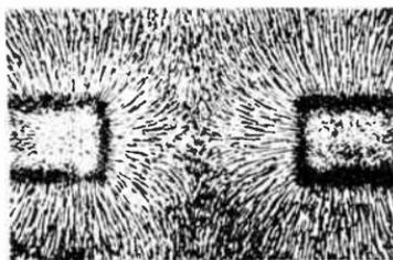
**Fig. 8-15.** Pattern formed by lines of force when two north poles are brought near each other.
