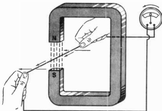
Fig. 11-26. Moving the conductor in the opposite direction induces a voltage with an opposite polarity.
