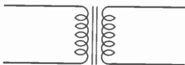
Fig. 11-19. Electrical symbol for a transformer.
