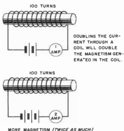
Fig. 9-17. The strength of the current through the coil affects the magnetic strength of the coil.
