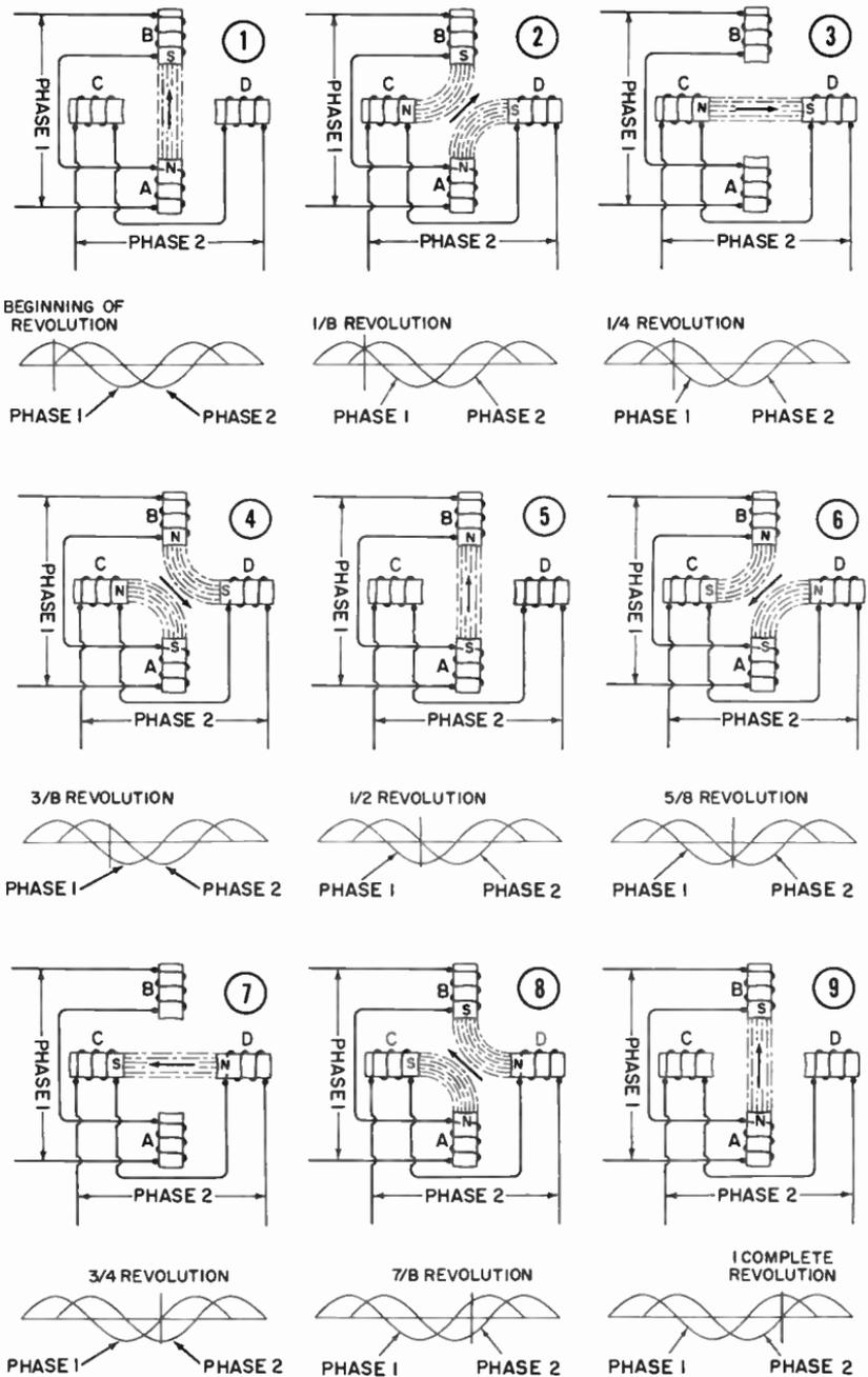
Fig. 13-9. Showing how a two phase current can produce a rotating magnetic field.
