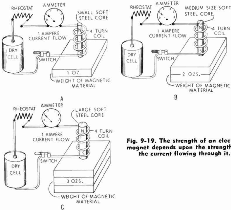
**Fig. 9-19.** The strength of an electromagnet depends upon the strength of the current flowing through it.
