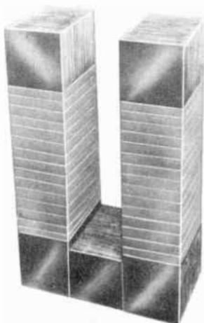
**Fig. 11-5. Laminated core for a core-type transformer. (Courtesy of Eisler Engineering Company.)**
