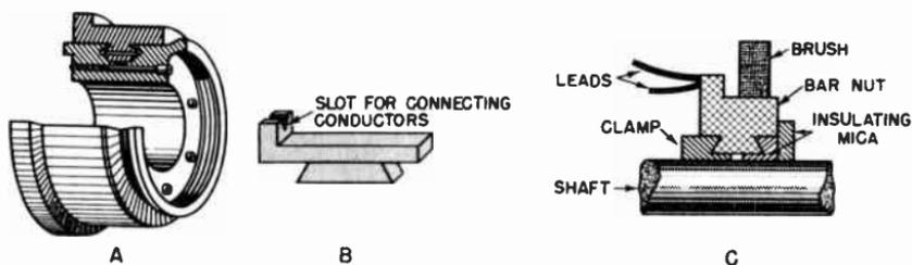
Fig. 12-22. The parts which go into the construction of a commutator.
