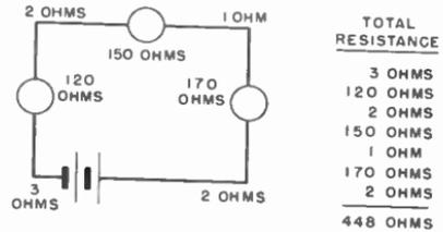
**Fig. 6-11.** Often it is necessary to take into consideration the resistance of the connecting conductors in determining the total resistance in a series circuit.
