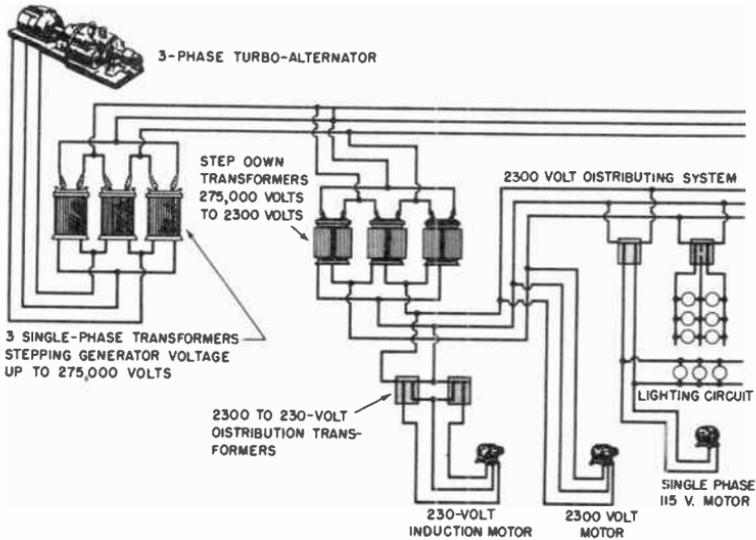
**Fig. 11-4. How transformers are used for many different purposes in a transmission and a distribution system.**
