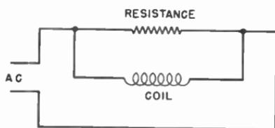
**Fig. 13-20.** Part of the current will flow through the resistance and part through the coil. That which flows through the coil will be retarded somewhat.
