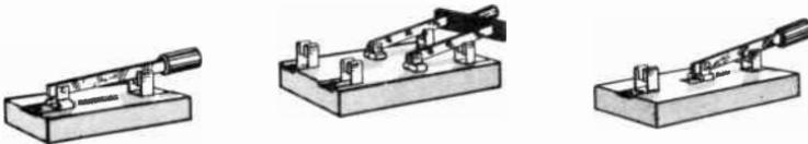
Fig. 4-6. Rigid insulation such as bakelite and porcelain is used as a base for switches.
