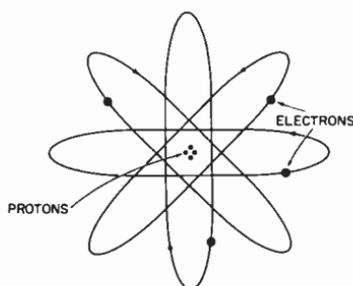
**Fig. 2-2.** Showing in a general way how the electrons revolve around the nucleus (protons) in a 4-electron, 4-proton atom.
