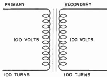
**Fig. 11-32.** If the secondary has the same number of turns as the primary, it will also have the same voltage.
