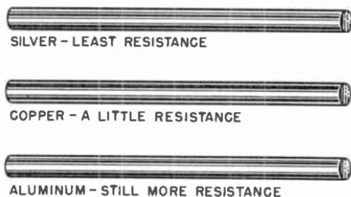
Fig. 4-9. The material from which a conductor is made affects its resistance to electrical current flow.
