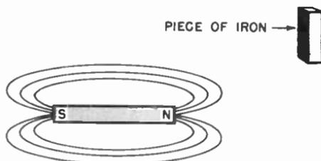
**Fig. 8-12.** The soft iron is not materially affected by the magnetic lines of force while at a distance.
