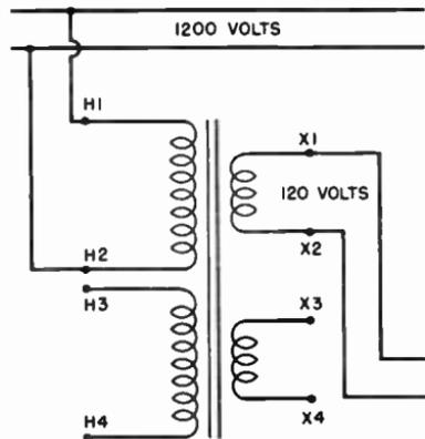
**Fig. 11-44.** How a transformer would be connected when only one high-voltage and one low-voltage winding is in use. This is not a normal method of using the transformer.
