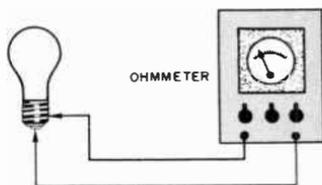
**Fig. 7-3.** The resistance of the filament in a lamp can be measured with an ohmmeter, but it is only the cold resistance which is measured.
