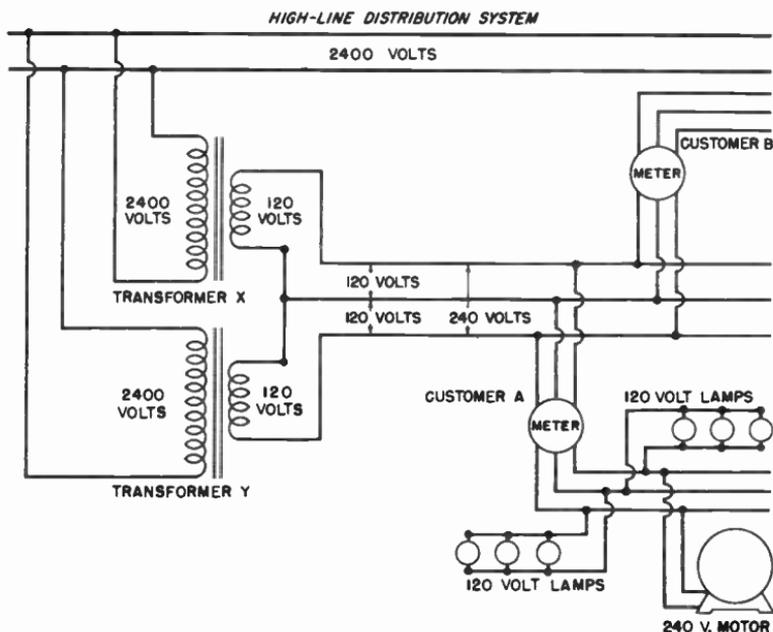
Fig. 11-42. How two transformers can be connected to a distribution system to supply power for a three-wire Edison system.
