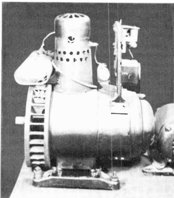
**Fig. 12-29.** A 32-volt electric generating plant intended for home use in remote areas where commercial power is not available.
