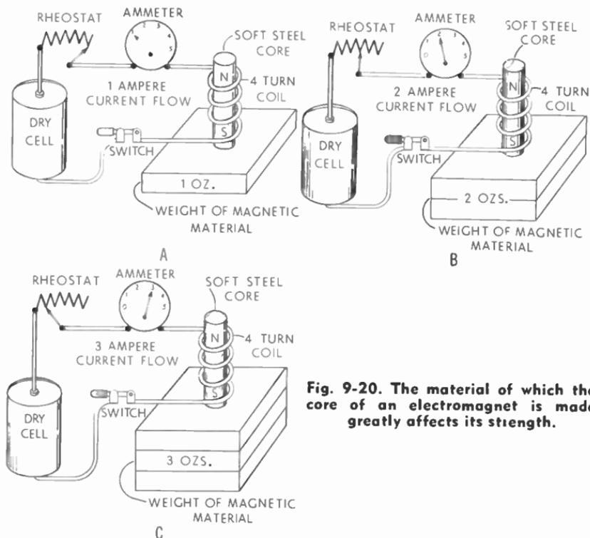
Fig. 9-20. The material of which the core of an electromagnet is made greatly affects its strength.
