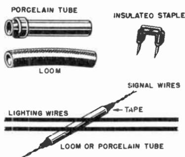
Fig. 14-22. An insulated staple, loom, and porcelain tube.
