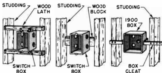
Fig. 15-36. Methods of mounting switch boxes.
