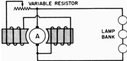
**Fig. 12-27.** The strength of the field magnetizing current in a shunt generator can easily be controlled by inserting a variable resistor in the field circuit.
