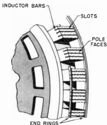
Fig. 13-19. How the squirrel-cage bars used to start the motor are imbedded in the faces of the poles on the rotor of a synchronous motor.
