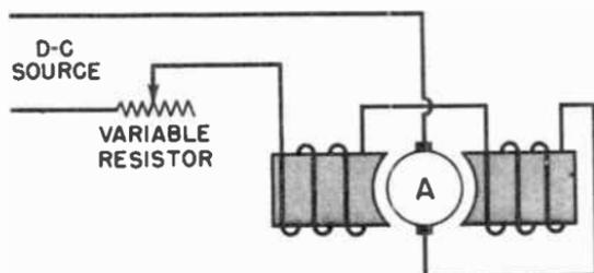
**Fig. 12-30.** A DC series motor can be controlled by inserting resistance in the circuits leading to the motor. The voltage drop across the resistance tends to reduce the voltage to the motor, thus slowing its speed.
