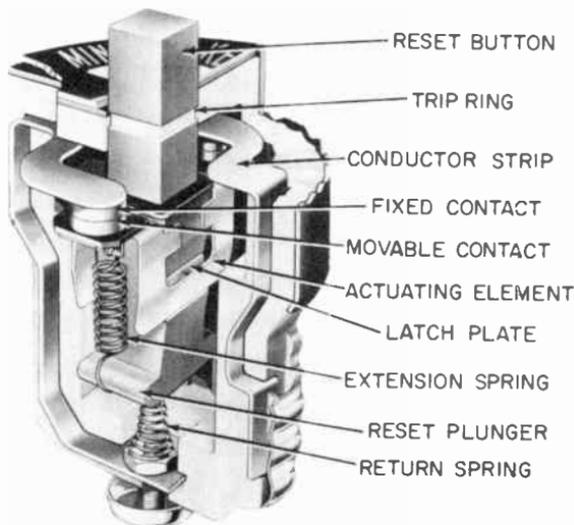
Fig. 5-17. A cross-sectional view of a mini-breaker showing its internal construction. (Courtesy of Mechanical Products Inc.)
