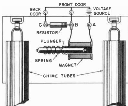
Fig. 14-20. How a door chime works.
