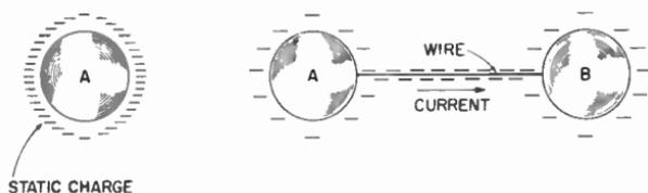
**Fig. 2-4.** By means of a small wire, a negative charge placed on metal ball (A) may be imparted to ball (B) to give it a charge.
