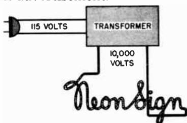
Fig. 11-3. The high voltage needed for the operation of a neon sign is provided by a transformer.
