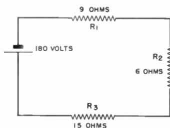
$$\begin{aligned} \text{TOTAL RESISTANCE} &= 9 + 6 + 15 = 30 \text{ OHMS} \\ \text{TOTAL CURRENT} &= \frac{180}{30} = 6 \text{ AMPERES} \\ \text{VOLTAGE DROP ACROSS } R_1 &= 6 \times 9 = 54 \text{ VOLTS} \\ \text{VOLTAGE DROP ACROSS } R_2 &= 6 \times 6 = 36 \text{ VOLTS} \\ \text{VOLTAGE DROP ACROSS } R_3 &= 6 \times 15 = 90 \text{ VOLTS} \\ \text{TOTAL VOLTAGE DROP} &= 54 + 36 + 90 = 180 \text{ VOLTS} \end{aligned}$$
