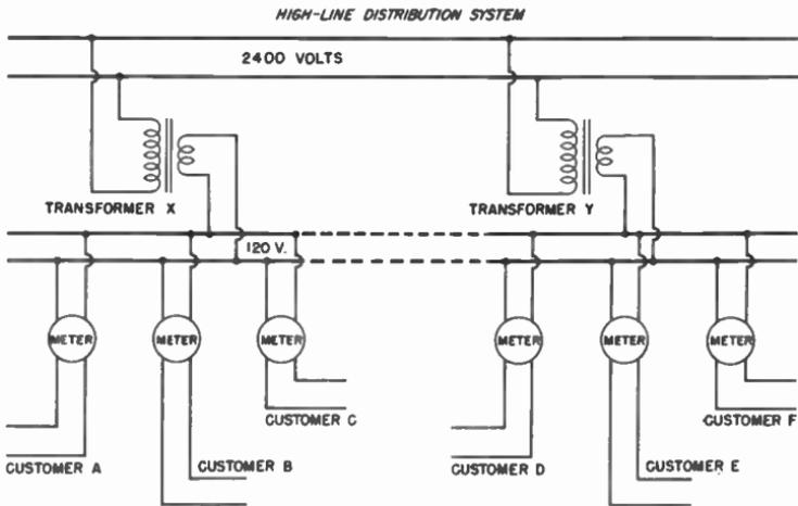
Fig. 11-41. How two transformers can be connected to supply power to a group of customers.
