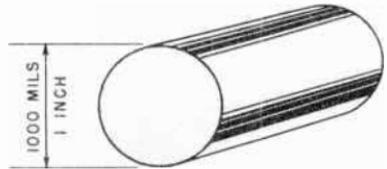
**Fig. 6-3.** The diameter of a conductor is measured in mils. One inch equals 1000 mils.
