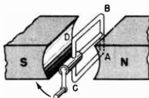
Fig. 12-13. When the conductors of a closed loop are moved so that they do not cut magnetic lines of force, no voltage will be induced within them.
