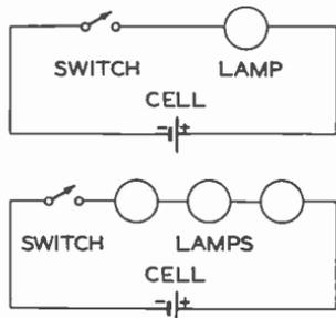
Fig. 4-15. Schematic diagrams of two series circuits.
