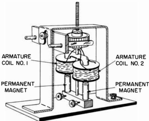
Fig. 12-4. A permanent-magnet type of experimental direct-current generator.
