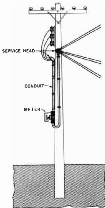
Fig. 15-4. A meter on a pole for an overhead service.
