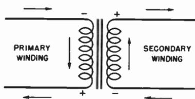
posite direction to that of the current in the primary. This is another fundamental principle of transformer operation. This action of the current is shown in Fig. 11-31.
