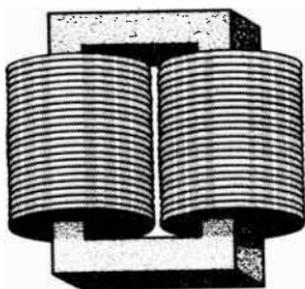
Fig. 11-21. How the coils are placed on a core-type transformer.
