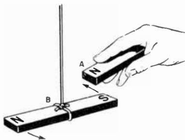
Fig. 8-4. The north pole of one magnet will attract the south pole of another magnet.
