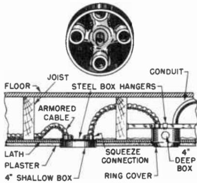
Fig. 15-27. Armored cable can be run from box to box. It can be easily fished through the hollow spaces within the walls and above the ceiling.
