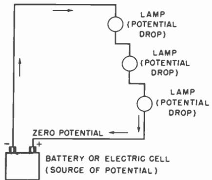
**Fig. 4-22.** As the current flows through the lamps under pressure of the voltage, there is a voltage drop across each of the lamps.
