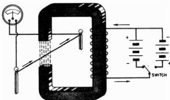
**Fig. 11-28.** During the instant a magnetic field is building up across the gap in the iron, the moving magnetic lines of force will induce a voltage in the conductor.
