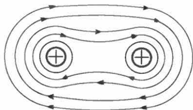
**Fig. 9-8. How the lines of force link together around two parallel conductors carrying current in the same direction.**
