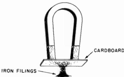
**Fig. 8-7.** The magnet will pick up the iron filings even though there is a piece of cardboard between.
