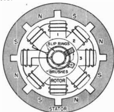
Fig. 13-18. The rotor and stator of a synchronous motor.
