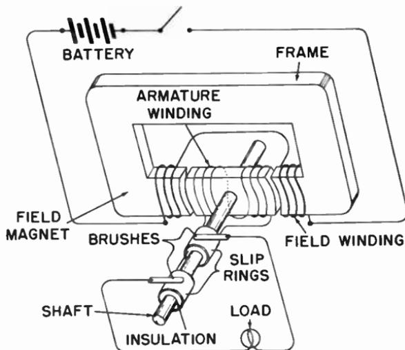
Fig. 12-5. Simple type of elementary (alternator) alternating-current generator.
