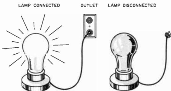
**Fig. 4-3. A complete metallic path must be provided for the passage of electricity.**
