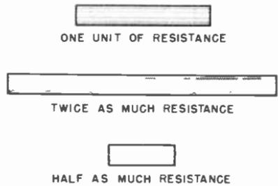
**Fig. 6-1.** The resistance is directly proportional to the length of the conductor.
