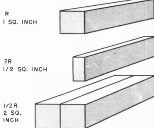
**Fig. 6-2.** The resistance is inversely proportional to the cross-section area of the conductor.
