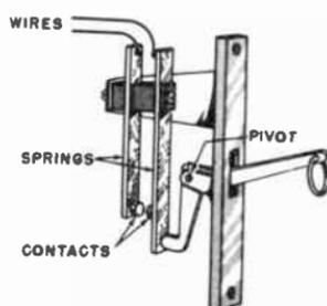
Fig. 14-5. A switch which could be used with a pull cord.
