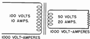
**Fig. 11-38.** As the transformer steps down the voltage, the current in the secondary increases.
