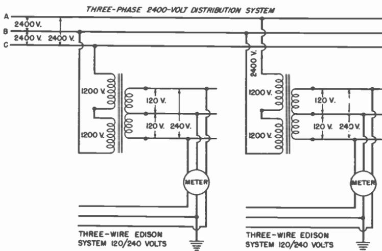
Fig. 11-51. How three-wire Edison-system power can be tapped off individual phases of the three-phase power distribution system. Power for use in the Edison system can be tapped off the distribution system between any two of the three wires.
