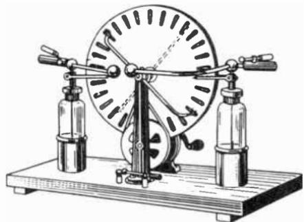
Fig. 3-15. A Wimshurst induction static machine.
