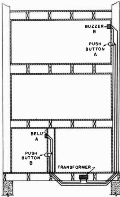
Fig. 14-26. The method of wiring a return-call system.
