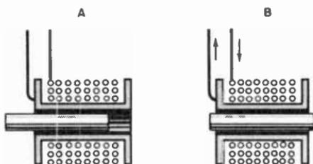
Fig. 14-19. Construction details of a plunger magnet.
