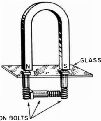
Fig. 8-20. There is no insulation for magnetism.
