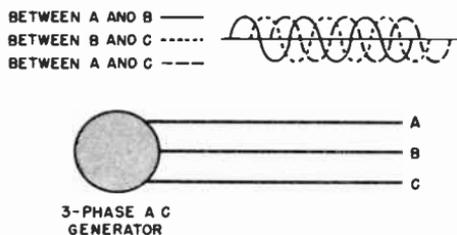
**Fig. 11-50.** A three-phase generator connected to three line wires. The voltage and current will rise and fall in the three line wires in time relation to each other as shown.
