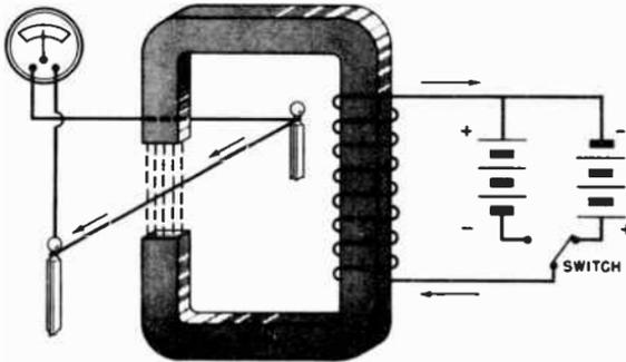
**Fig. 11-29.** If the current through the coil is reversed, the voltage induced in the wire in the gap will be reversed.
