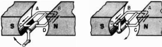
**Fig. 12-12.** When a closed loop is rotated within a magnetic field, an electrical current will flow within the conductors of the closed loop.
