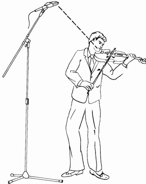
**Fig. 8-23.** Typical pickup placement of violin.
