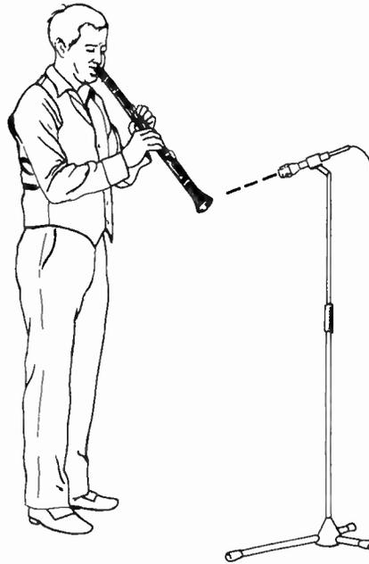
**Fig. 8-6.** Typical mike positioning for clarinet.
