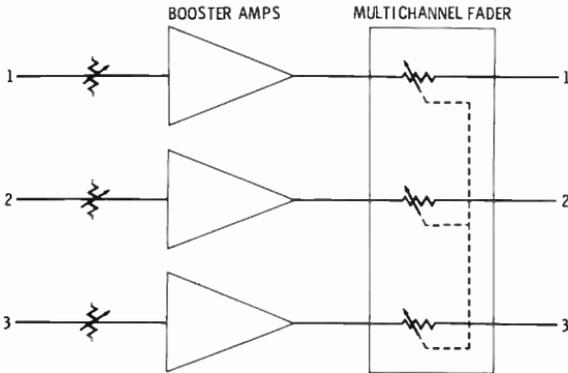
(B) Retaining separation by using a multichannel fader.
