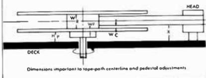
FIGURE 4. PEDESTAL HEIGHT & TAPE PATH DIMENSIONS (CONT.)
