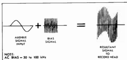
FIGURE 1. PRODUCTION OF RESULTANT SIGNAL
