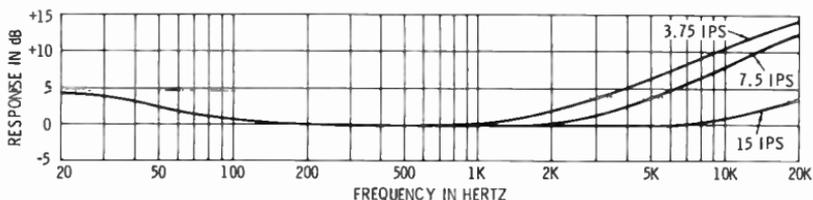
(A) Typical recording pre-equalization for 1/4-inch tape recorders using NAB characteristics.
