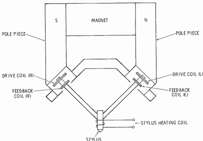
Fig. 12-10. Simplified drawing of a stereo cutter head.
