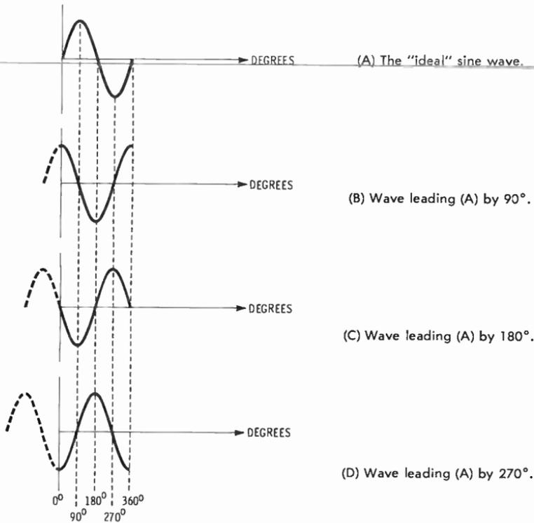
**Fig. 2-5. Demonstrating phase relationships of sine waves.**
