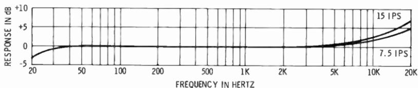
(C) Typical pre-equalization characteristics for 1/4-inch tape recorders running 7.5- and 15-ips, using CCIR (DIN) standard.
