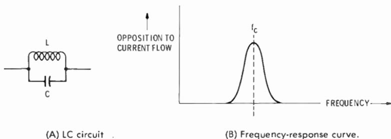
(A) LC circuit (B) Frequency-response curve.
