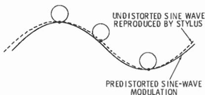
The tracing simulator can only optimize distortion for one tip radius at a time; it is usually adjusted for 0.6 mil which is the international standard for the radius of a conical stylus. The elliptical and Shibata styli with their narrow side radii would not completely cancel the second-harmonic distortion added to the signal by the
