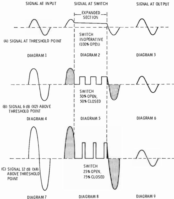
Fig. 5-42. Operation of the PDM system.
