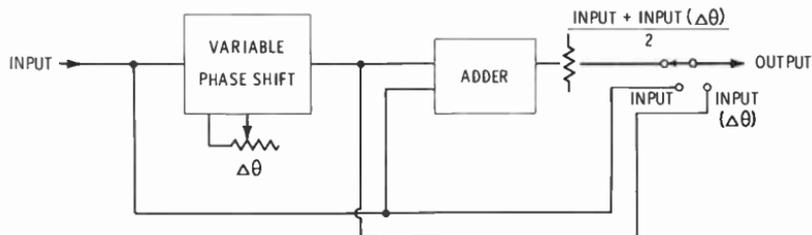
Fig. 5-72. Block diagram of the Countryman phase shifter.
