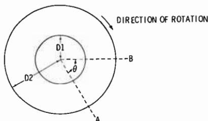
Fig. 12-12. Groove velocity decreases as groove diameter decreases.
