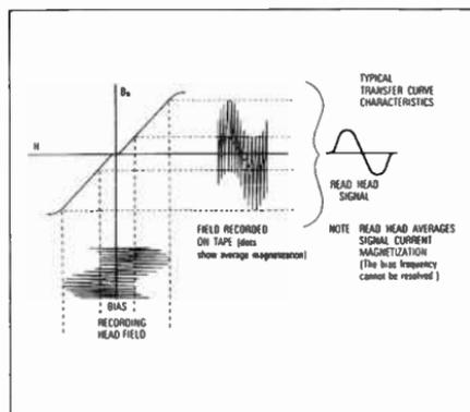
FIGURE 8. RECORDING TAPE TRANSFER CURVE
