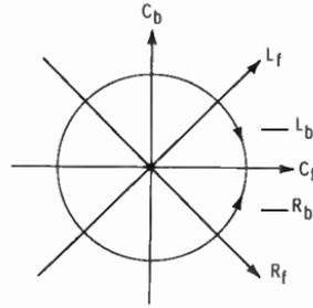
clockwise circle. The lengthwise motion of the groove under the stylus causes these two circular motions to form a double helix. Center-front information causes lateral stylus motion while center-back information causes vertical motion (Fig. 13-6).
