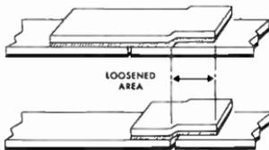
FIGURE 4. ENLARGED VIEW OF LOOSENED SPLICE
