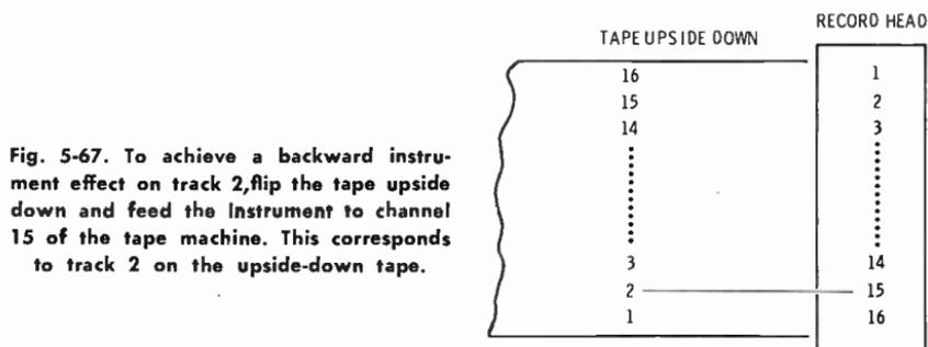
Fig. 5-67. To achieve a backward instrument effect on track 2, flip the tape upside down and feed the instrument to channel 15 of the tape machine. This corresponds to track 2 on the upside-down tape.
