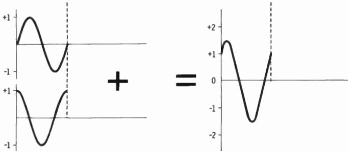
(C) The amplitudes of partially out-of-phase waves add in some places and subtract in others when mixed.
