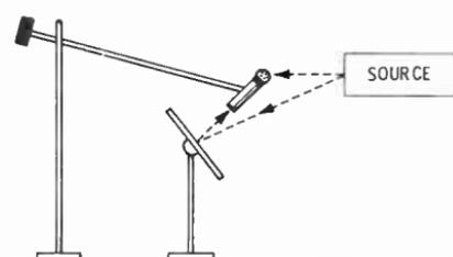
Fig. 9-4. Correct mike placement using a unidirectional mike.
