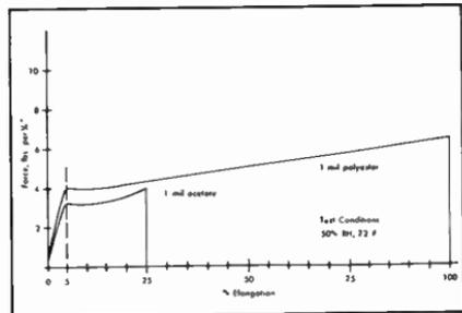
FIGURE 4. TENSILE PROPERTIES 1 MIL BACKING
