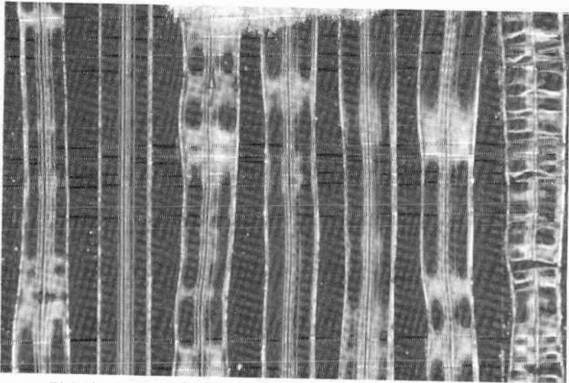
(B) A photomicrograph of grooves modulated with stereo program material.
