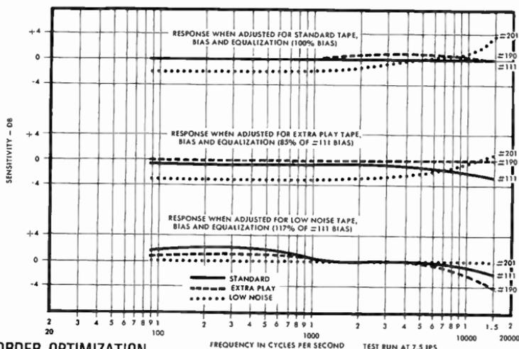
FIGURE 5. NORMALIZED TAPE RESPONSE CURVES
