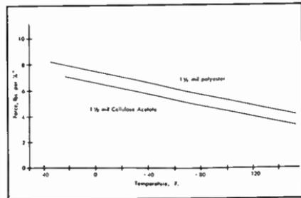
FIGURE 5. TEMPERATURE EFFECTS ON 5% ELONGATION POINT
