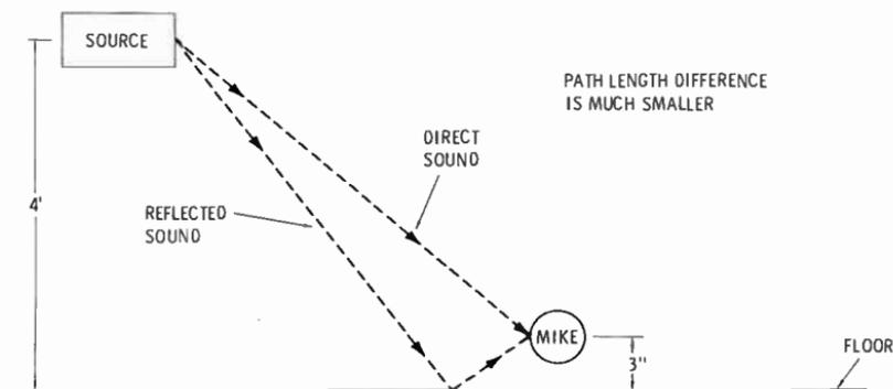
Fig. 3-26. Moving the distant mike toward the reflecting surface decreases the difference in path length and raises the lowest frequency of cancellation.
