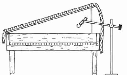
Fig. 9-2. Preventing leakage from getting into a piano mike.
