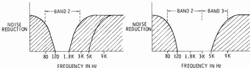
(A) Band 2 noise reduction is shut off by a high-level signal between 80 Hz and 3 kHz.
