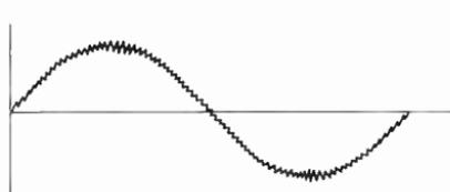
Fig. 7-2. Modulation noise on a sine wave.
