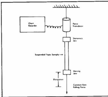
FIGURE 2. TENSILE STRENGTH TESTING APPARATUS DIAGRAM
