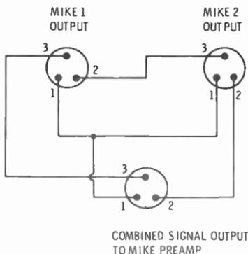
Fig. 3-28. Connecting two microphones in series. Pin 1 is ground, pin 2 is the high signal output, and pin 3 is the low signal output.
