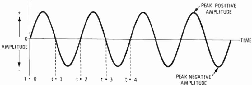
Fig. 2-1. Graph of waveform amplitude vs time.
