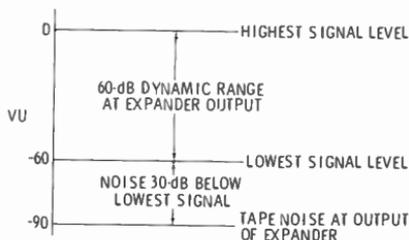
(C) Dynamic range is expanded on playback. Program signal is reduced from -30 to -60 dB, noise is reduced from -60 to -90 dB.
