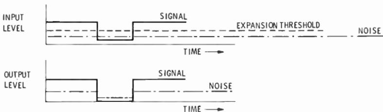
Fig. 5-34. When signal is above expansion threshold, gain is unity and both signal and noise appear at the output. When signal is below threshold, the gain decreases and reduces the level signal and the noise levels in the output.
