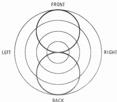
**Fig. 3-10. The normal pickup pattern of a ribbon microphone.**
