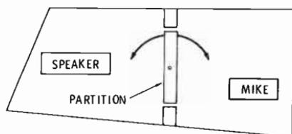
Fig. 5-56. An acoustic echo chamber. Decay time is a function of the partition position.
