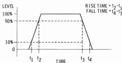
Each bit of data is represented by a current or voltage pulse. In order to insure accurate digital processing, these pulses must have rapid *rise* and *fall times*. Fig. 11-4 illustrates that the rise time of a pulse is the time needed for the level to increase from 10% to 90% of the maximum value and the fall time is the time needed to decrease from 90% to 10% of the maximum.
