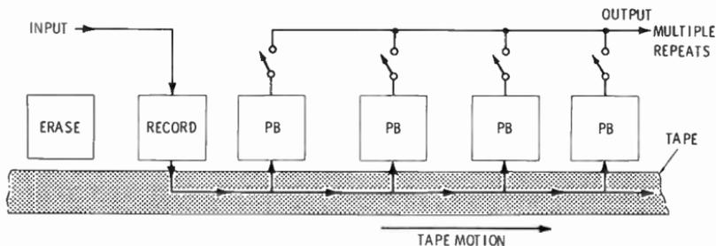
(A) By connecting different combination of playback heads.
