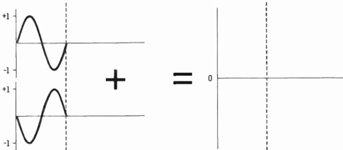
(B) Waves of equal amplitude cancel completely when mixed  $180^\circ$  out of phase.
