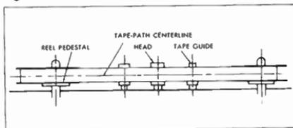
FIGURE 1. SIMPLIFIED TAPE PATH CENTERLINE
