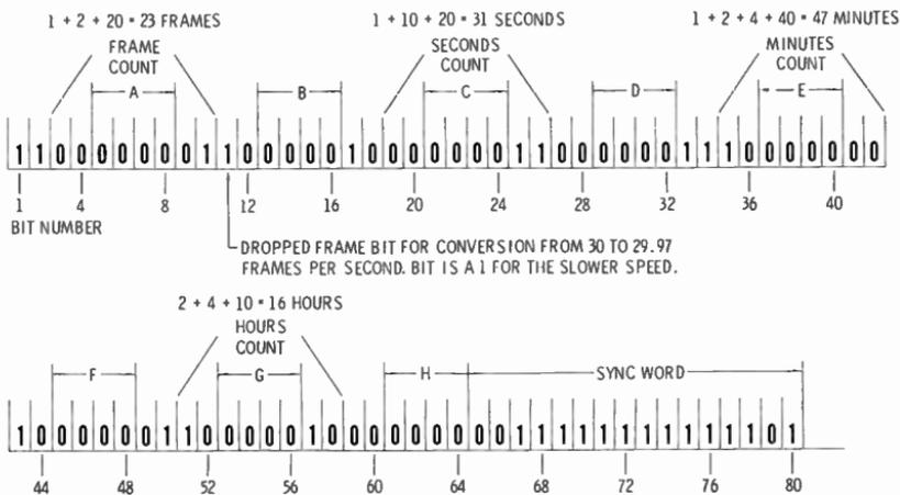
Fig. 10-7. The location of the 80 bits in the SMPTE digital word.
