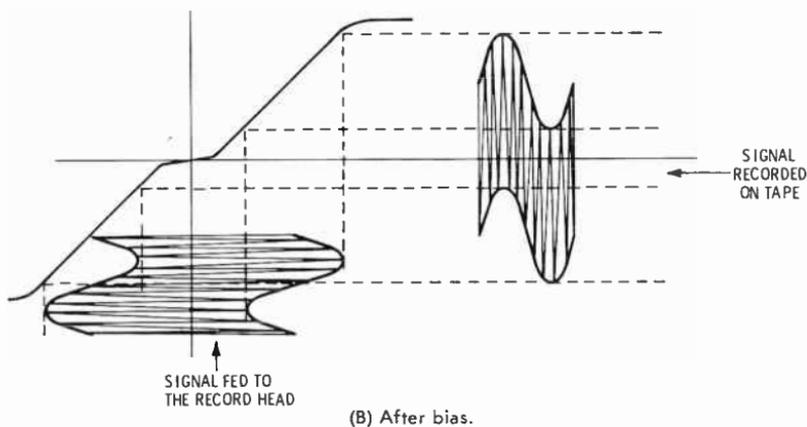
Fig. 4-14. Illustrating effect of biasing on recording linearity.
