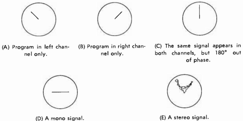
Fig. 12-24. Phase oscilloscope displays.
