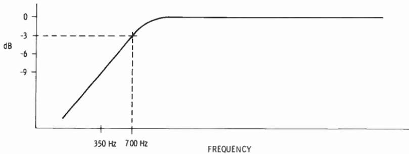
Fig. 5-19. A 700-Hz, high-pass filter with a slope of 6 dB per octave.
