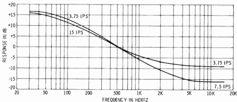
(B) Typical post-equalization for 1/4-inch tape recorders using NAB characteristics.
