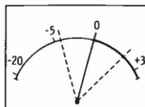
(C) Readings within the dotted lines are acceptable recording levels.
