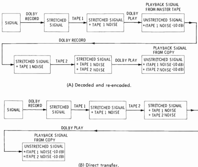
Fig. 7-15. The same amount of noise increase occurs in making tape copies of a stretched tape.
