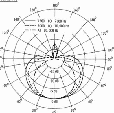
Fig. 3-34. The Shure SM57 dynamic cardioid microphone.
