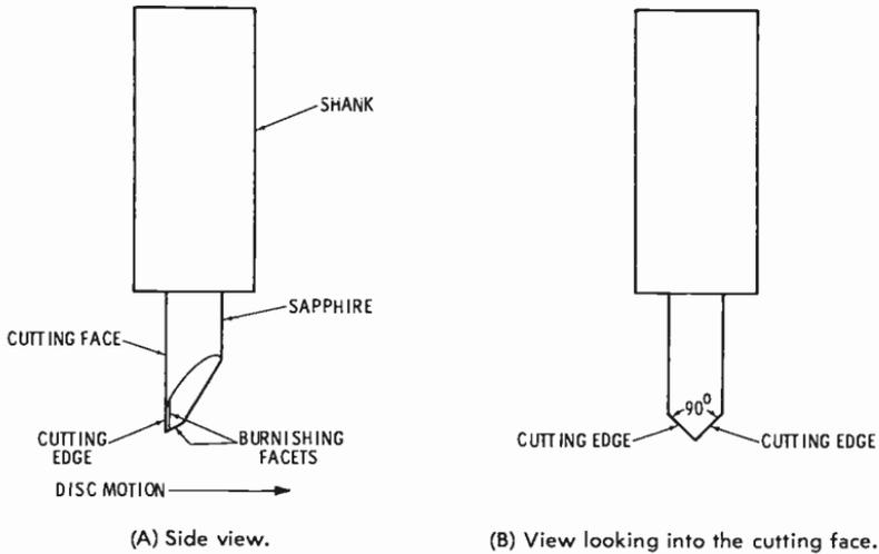
Fig. 12-11. A recording stylus.
