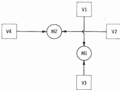
Fig. 3-27. Bidirectional mikes set at  $90^\circ$  angles to each other.
