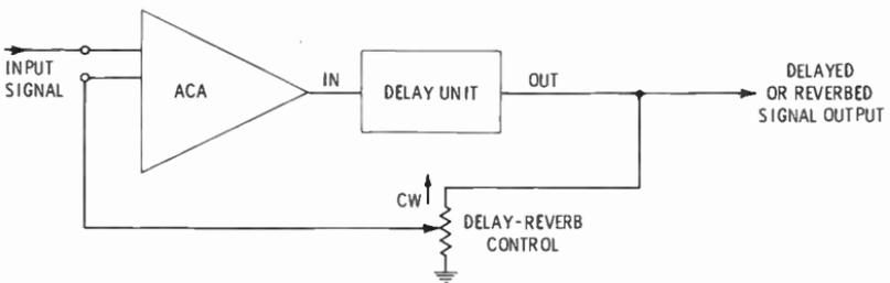
Fig. 6-17. Schematic diagram of a delay feedback system.
