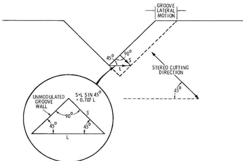
Fig. 12-23. Stereo groove motion with one channel modulated, producing the same amount of lateral motion as the mono groove in Fig. 12-22.
