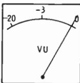
(A) The input signal to the compressor is below the threshold, and compressor gain is normal.
