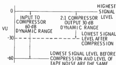
(A) A 60-dB dynamic range compressed to 30 dB before recording.
