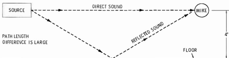
Fig. 3-25. A distant mike picks up both the direct sound from the source, and the reflected sound from nearby surfaces such as the floor.
