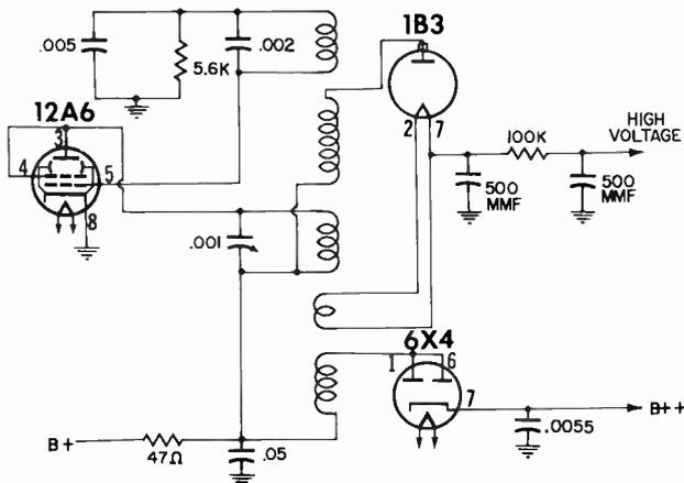
Fig. 4-3. RF oscillator and rectifier high-voltage supply system.
