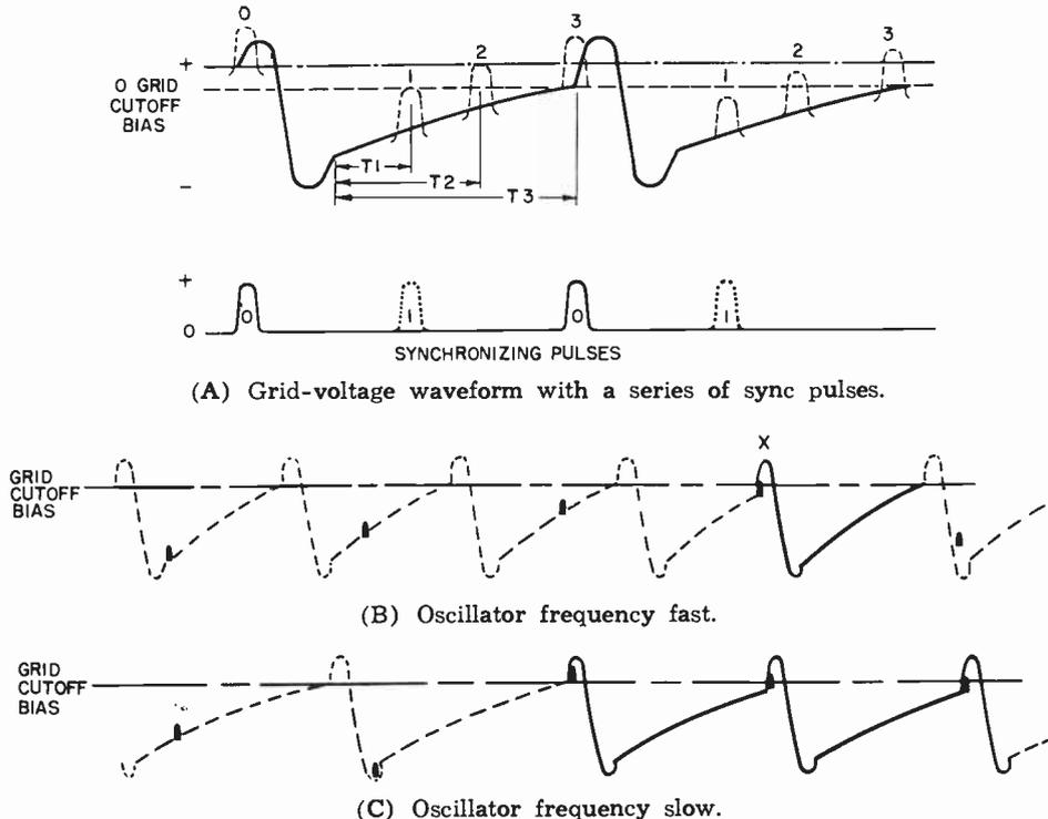
Fig. 7-4. Pulse control of a free-running blocking oscillator.
