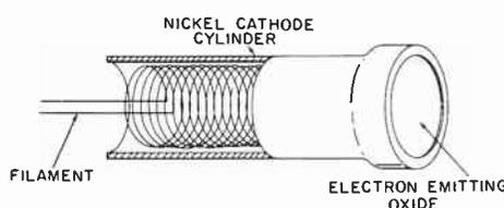
Fig. 1-2. Heater and cathode assembly.
