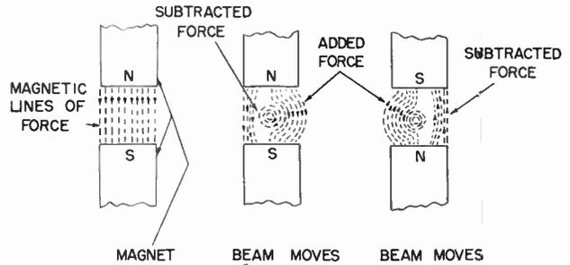
(A) Movement of electron beam in deflection field.
