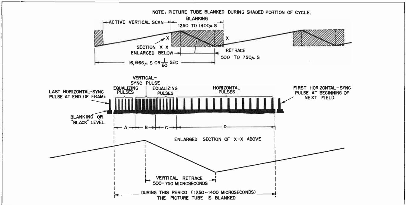
Fig. 7-2. Vertical-scanning wave and synchronizing signal.
