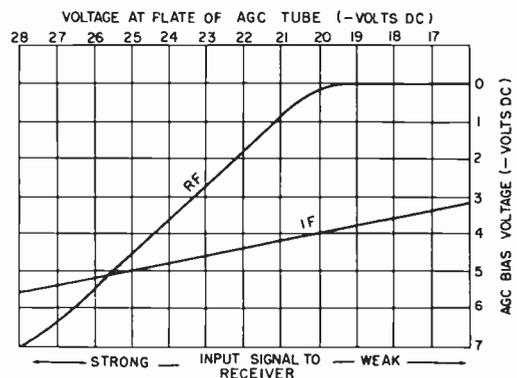
Fig. 16-6. Graph of the RF and IF bias voltages when an AGC delay circuit is employed.
