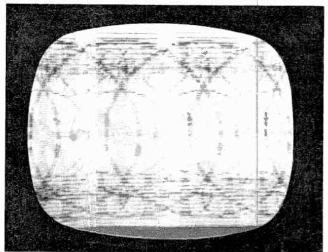
**Fig. 17-11. Horizontal-oscillator frequency misadjusted. (AFC system.)**
