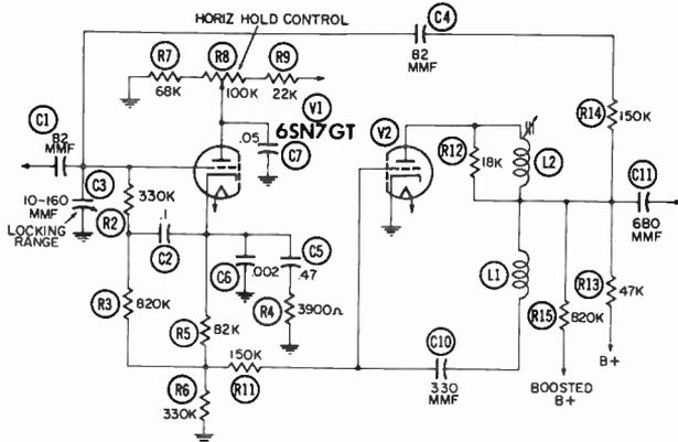
Fig. 8-18. A later version of the pulse-width circuit.
