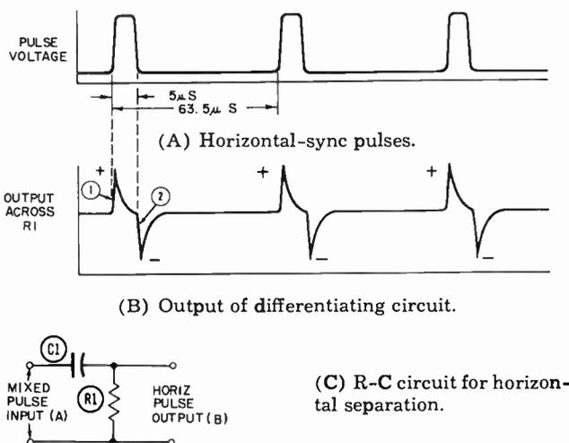
Fig. 10-10. Horizontal-pulse separation, or differentiation.
