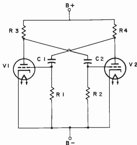
(B) Same circuit as (A), showing symmetry of circuit.
