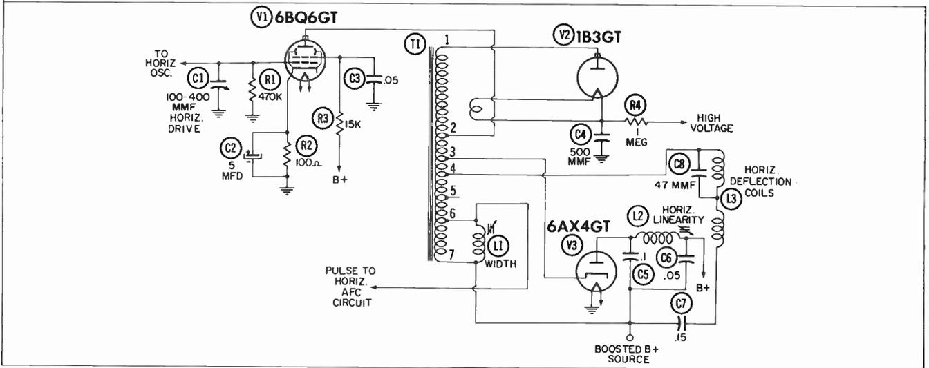
Fig. 8-5. A modern horizontal-deflection circuit.
