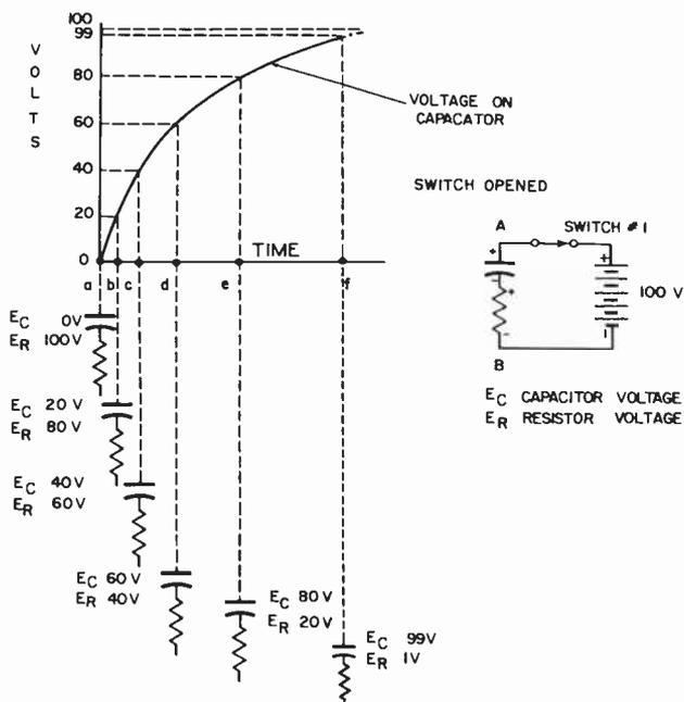
Fig. 5-1. Resistor-capacitor charging curve.
