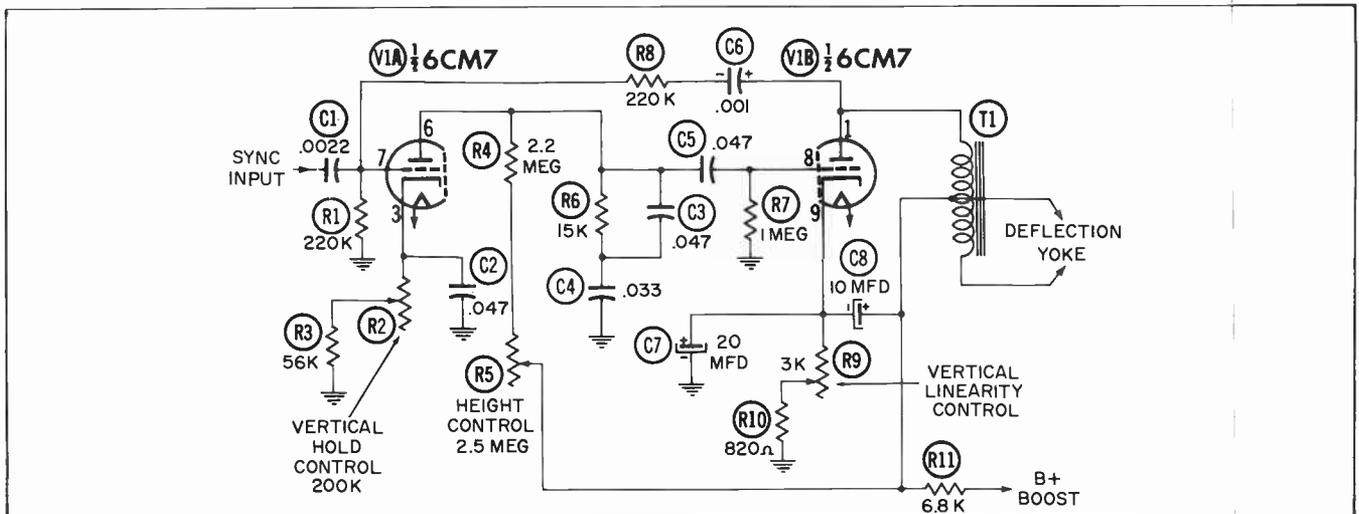
Fig. 8-12A. Vertical oscillator-output system employed in a modern TV receiver.
