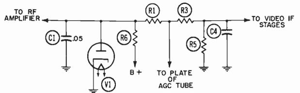
Fig. 16-5. AGC delay circuit.
