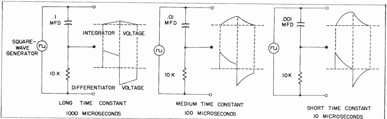
**Fig. 5-7.** Examples of time constants and their R-C waveforms.
