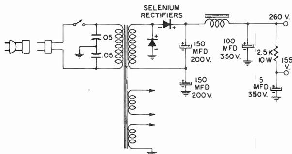
Fig. 4-1E. Schematic of power supply using a transformer and semiconductor rectifiers.
