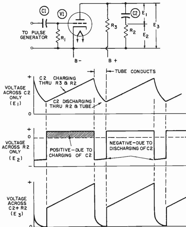
Fig. 7-8. Typical peaking circuit and associated waveforms.
