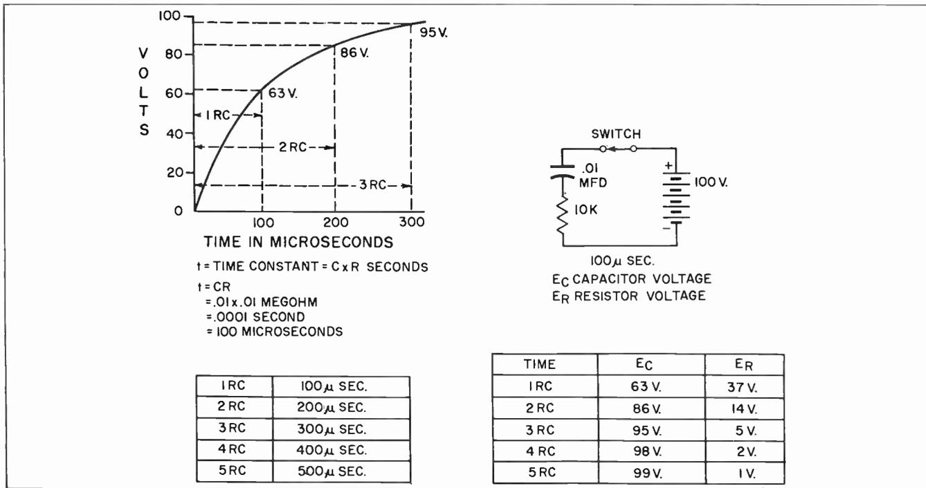
Fig. 5-3. Time constants of an R-C circuit.
