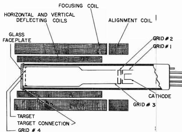
Fig. 3-4. Structural arrangement of the Vidicon.
