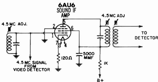
Fig. 14-3. A typical sound-IF amplifier circuit.
