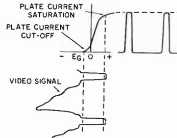
(B) Input and output waveforms.
