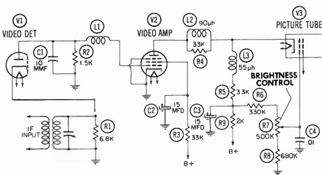
Fig. 13-17. A negative-output detector feeding the cathode of the picture tube through a single DC amplifier.
