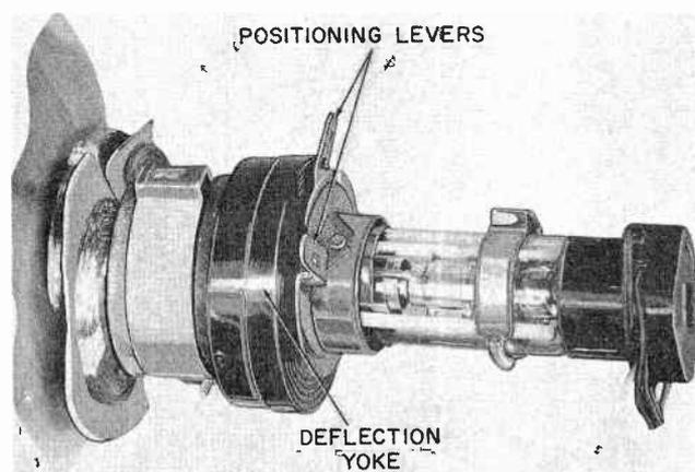
Fig. 1-13. Two magnetized rings used as centering device.
