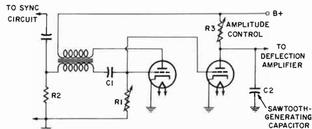
Fig. 6-13. Blocking oscillator and discharge tube as sawtooth generator.
