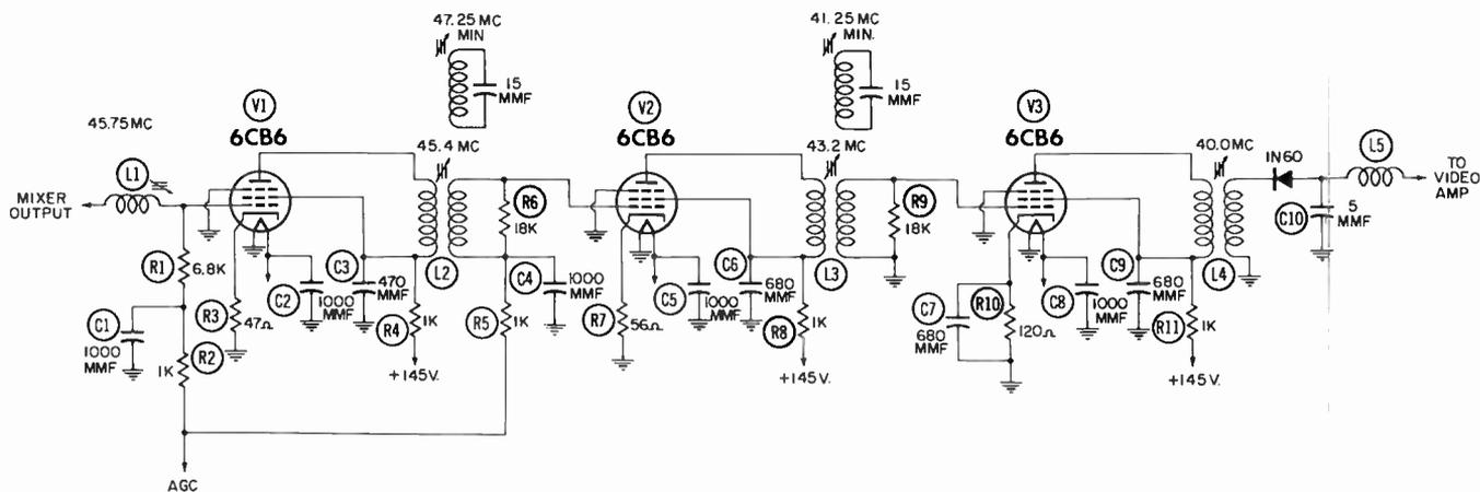
Fig. 13-6. Video IF amplifier employing overcoupled transformers.
