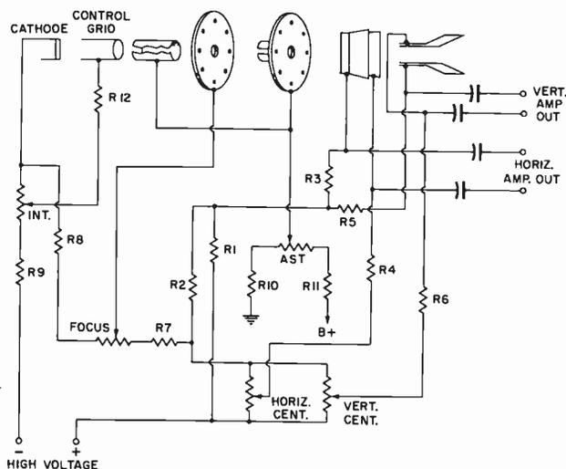
Fig. 1-11. Typical centering-control circuit.
