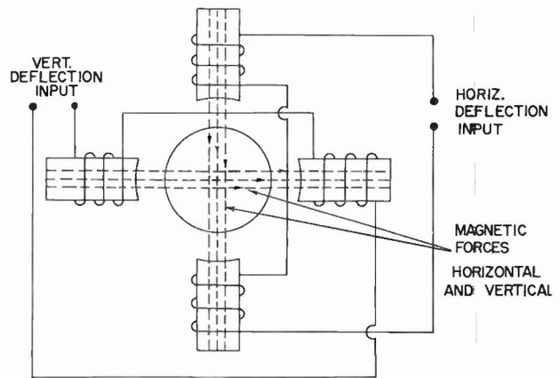
(B) Arrangement of magnetic coils in deflection yoke.
