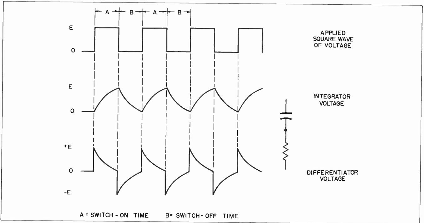
**Fig. 5-6.** Application of square wave of voltage to R-C circuits.
