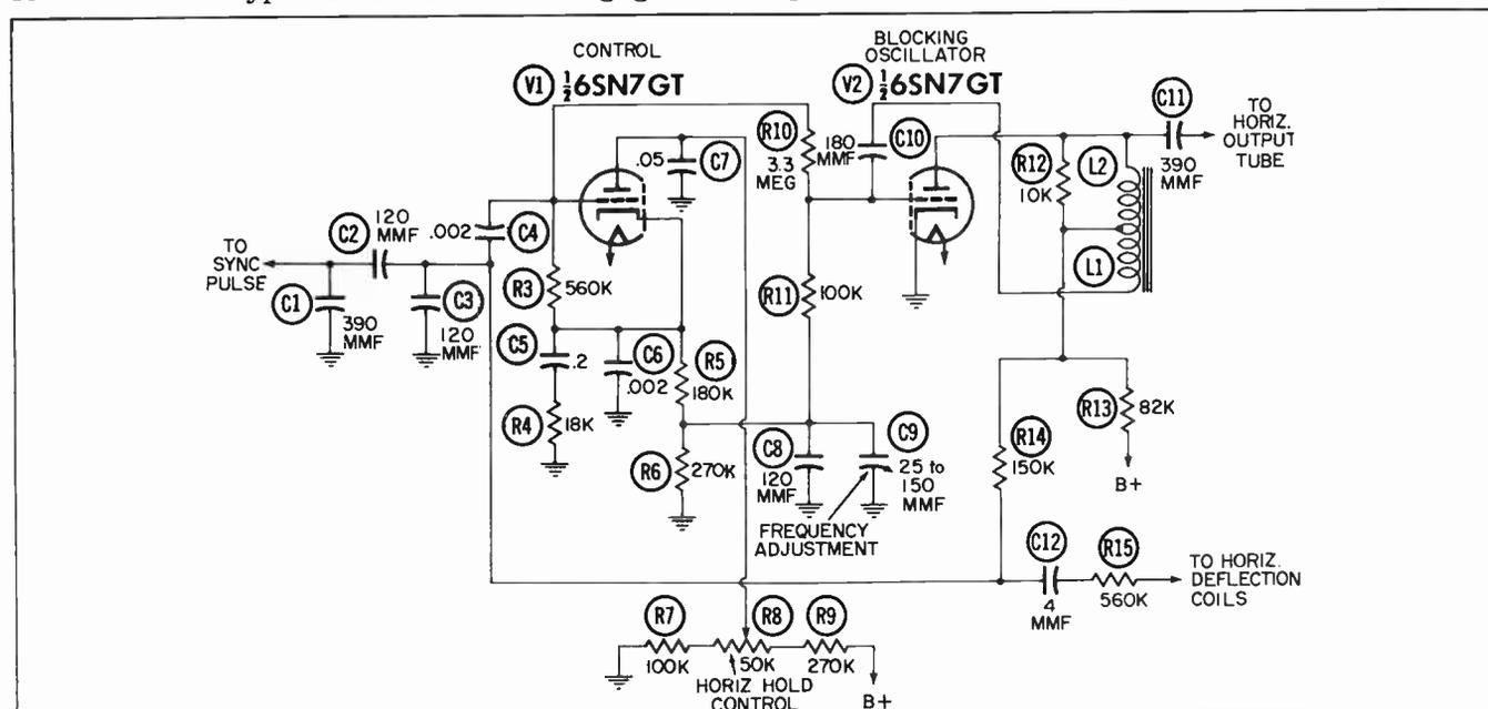
Fig. 8-17. Circuit using automatic pulse-width control of blocking oscillator.
