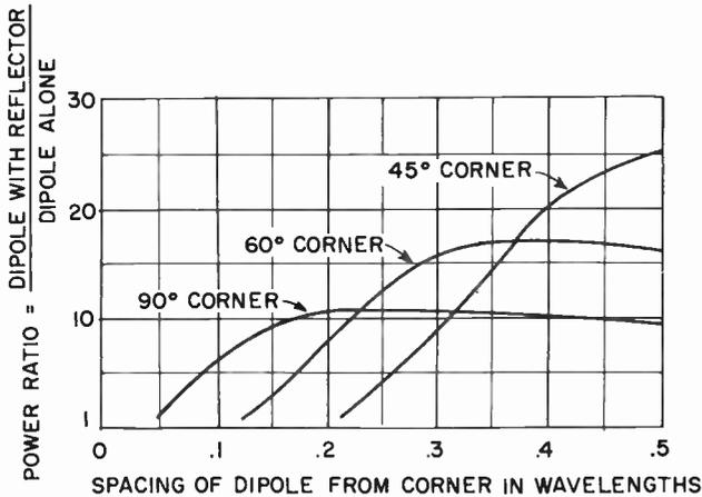
(B) Effect of corner angle and dipole position on gain of corner reflector.
