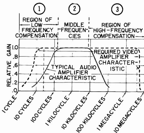
(B) Required video bandwidth compared with typical audio bandwidth.
