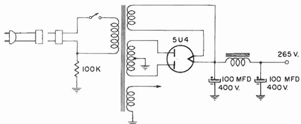
Fig. 4-1B. Schematic of typical low-voltage power supply used in present-day receivers.
