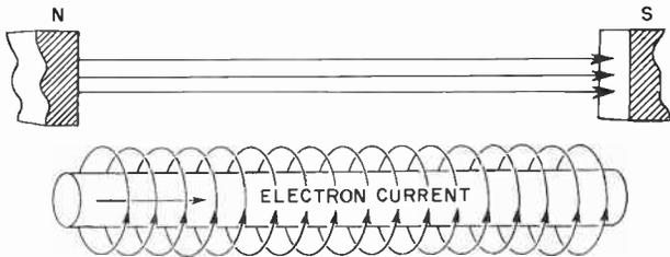
**Fig. 2-3. Conductor parallel to magnetic field.**
