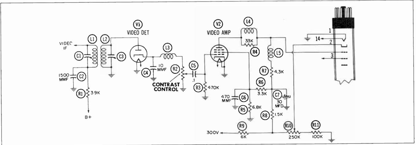
Fig. 13-16. Video detector of positive polarity feeding picture-tube grid through a single video-amplifier stage.
