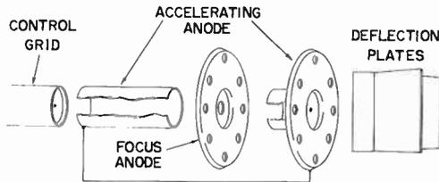
Fig. 1-6. Typical anode assembly.
