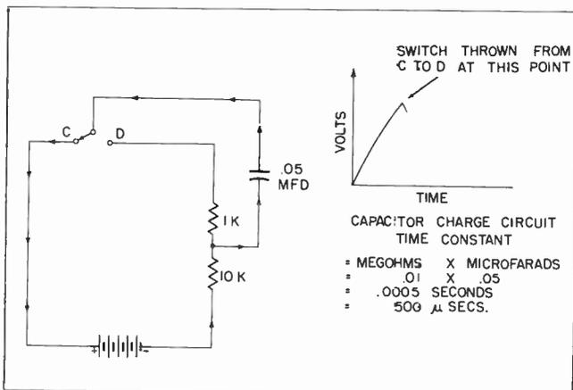
**Fig. 5-8.** Capacitor charge circuit for sawtooth waveform.
