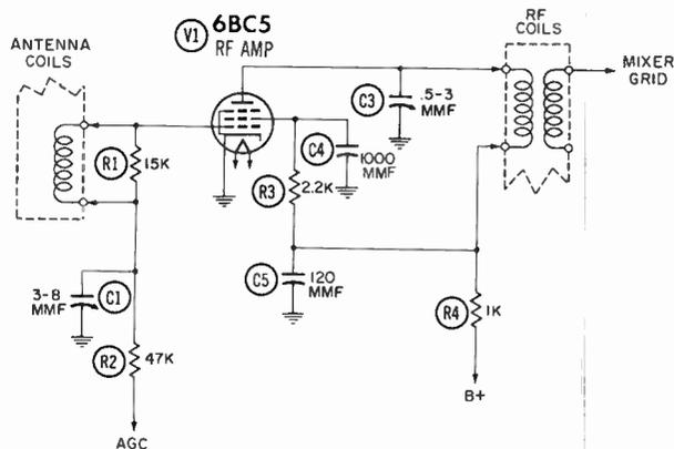
Fig. 12-1. Pentode RF amplifier circuit.
