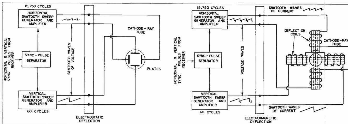
Fig. 7-7. Electrostatic and electromagnetic scanning systems.
