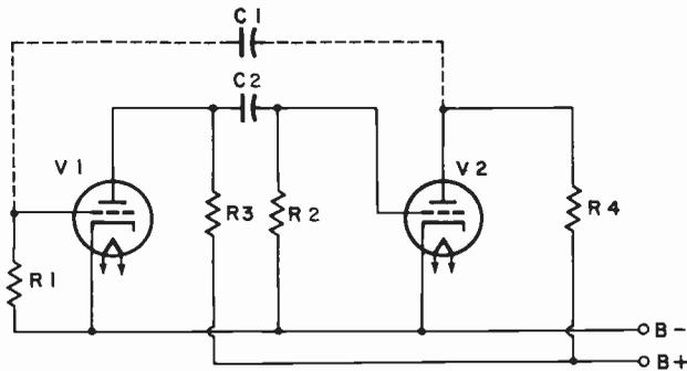
(A) A two-stage amplifier with capacitive feedback.
