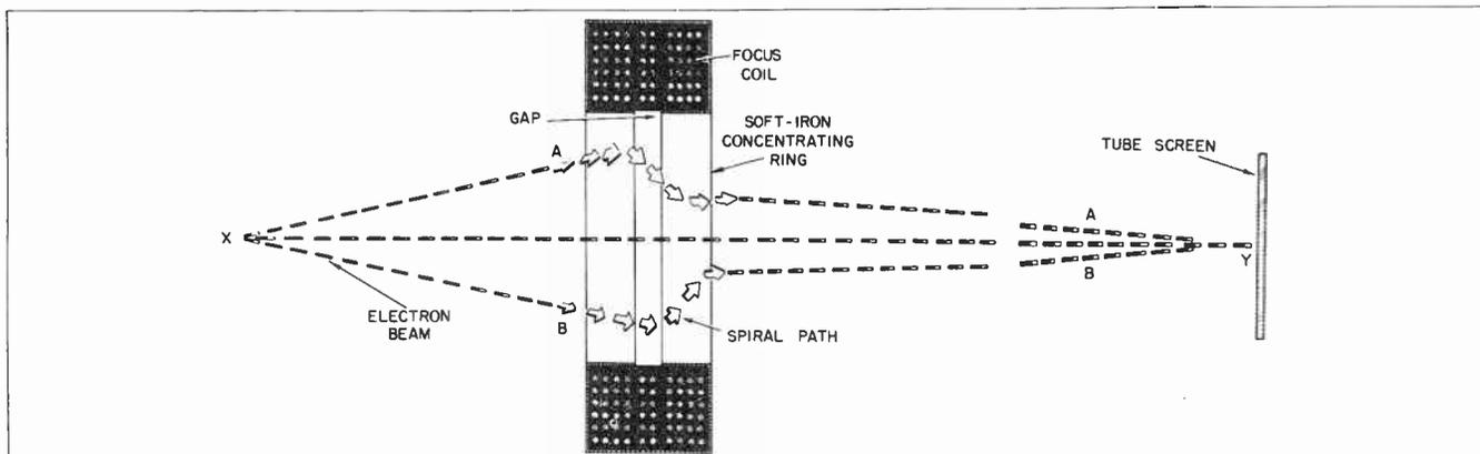
**Fig. 2-5. Action of focus coil on electron beam.**
