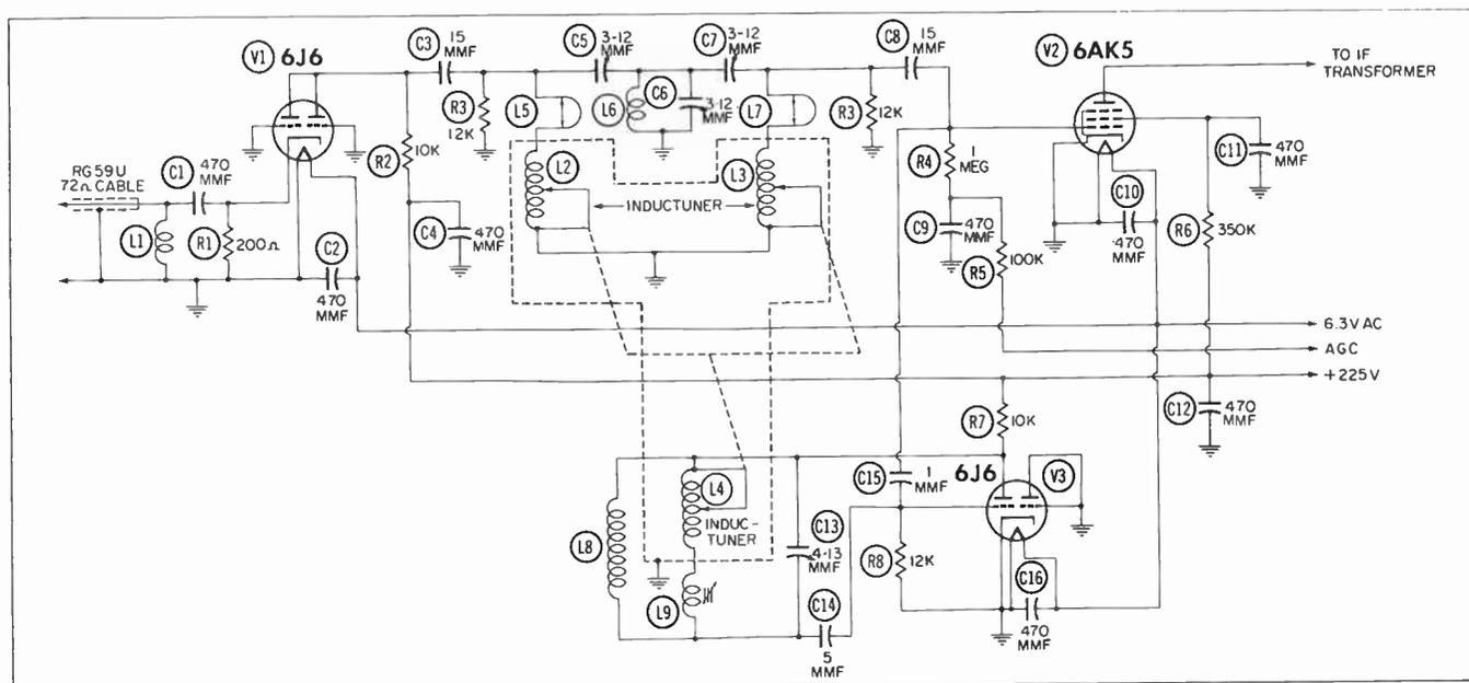
Fig. 12-7. Schematic of inductively-tuned input system illustrated in Fig. 12-6.
