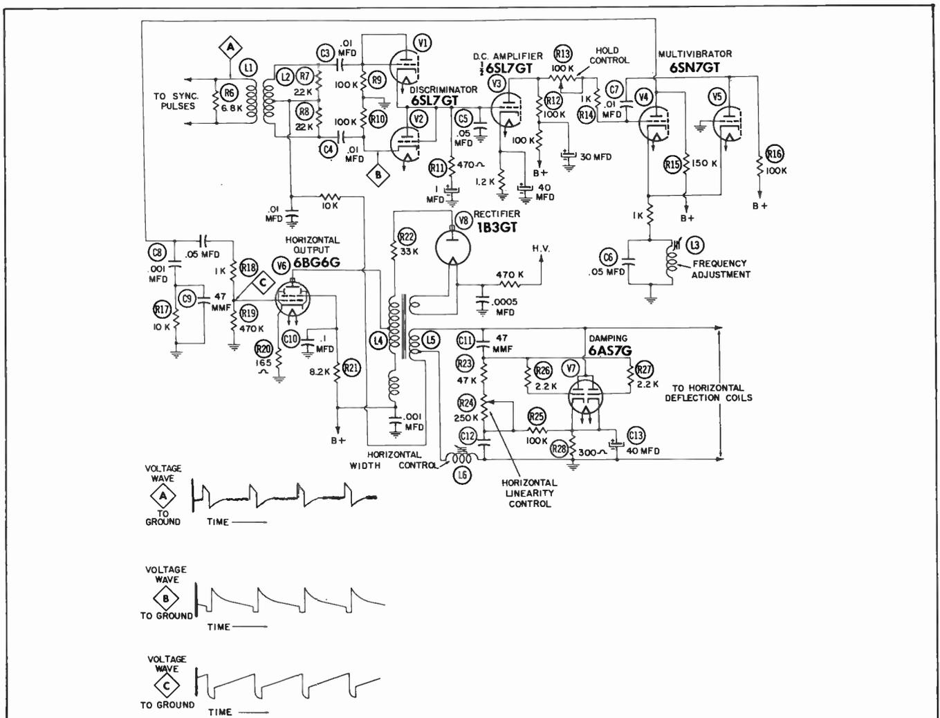
Fig. 8-14. Example of a multivibrator controlled by a discriminator.
