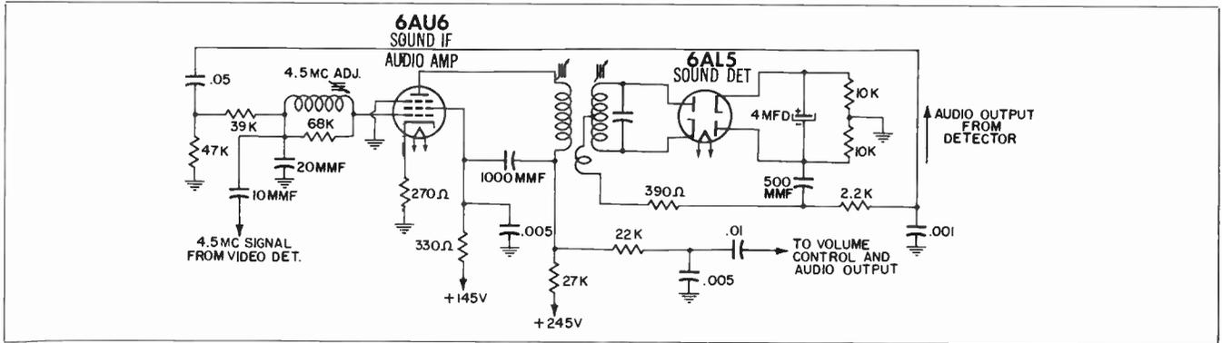
Fig. 14-5. A reflex amplifier which handles the sound IF and audio signals.
