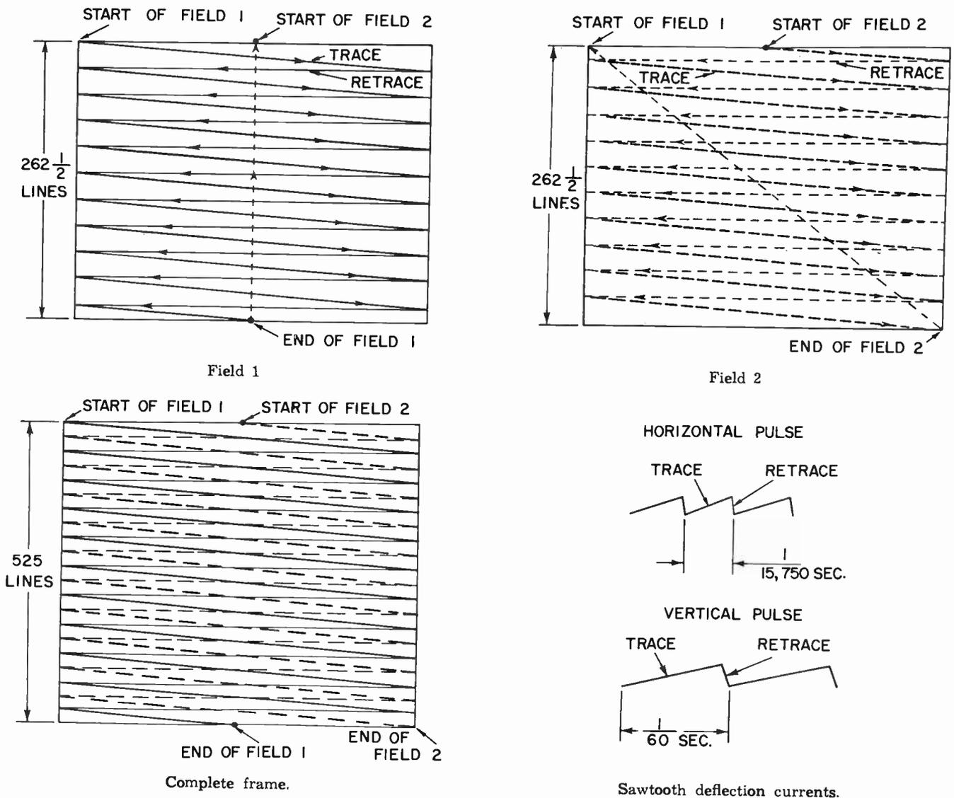
Fig. 3-5. The principles of interlaced scanning.
