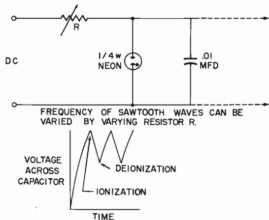
Fig. 6-1. Neon-tube relaxation oscillator.
