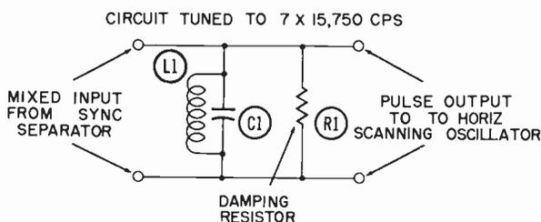
(C) Horizontal separation by tuned circuit action (one-half cycle of ringing employed).
