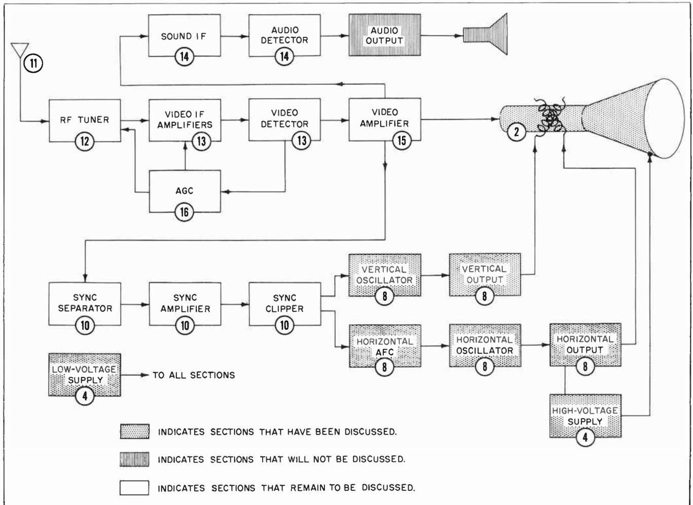
Fig. 9-1. Block diagram of a television receiver.
