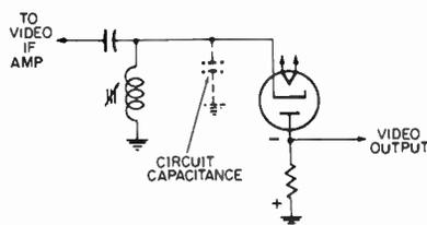
(A) Video output increases negatively with respect to ground as carrier increases.
