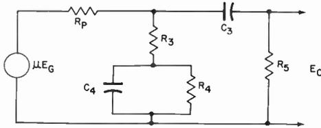
(B) Equivalent low-frequency circuit.
