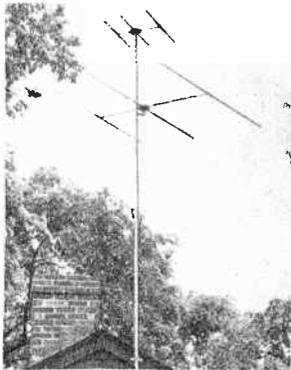
Fig. 11-10. Array with separate dipoles for high and low VHF bands.
