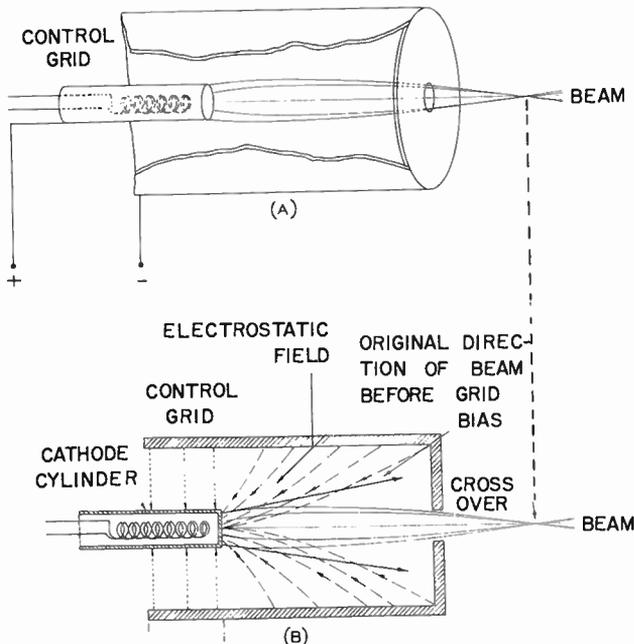
Fig. 1-3. Action of cathode and control-grid assembly.
