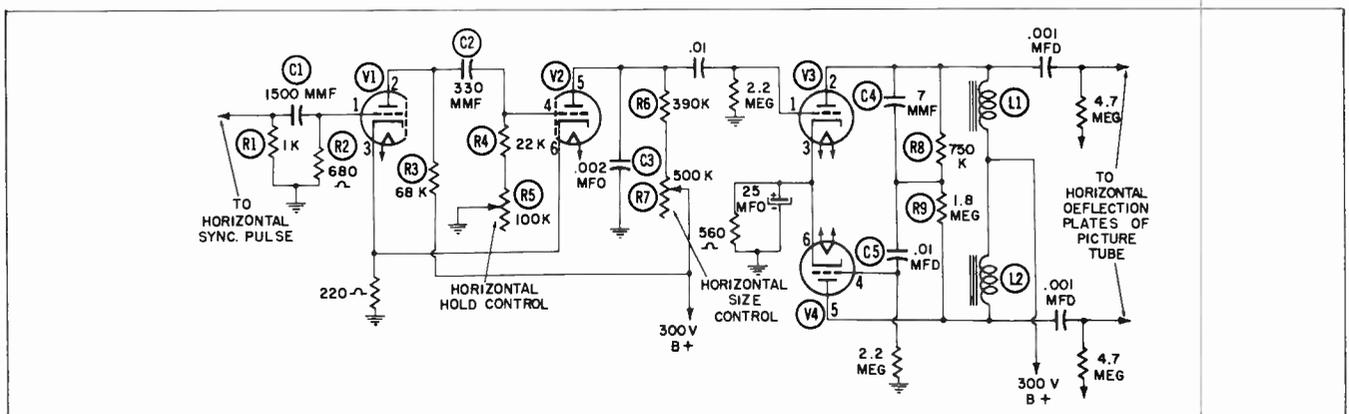
Fig. 8-7. Horizontal-deflection circuit for an electrostatic picture tube.
