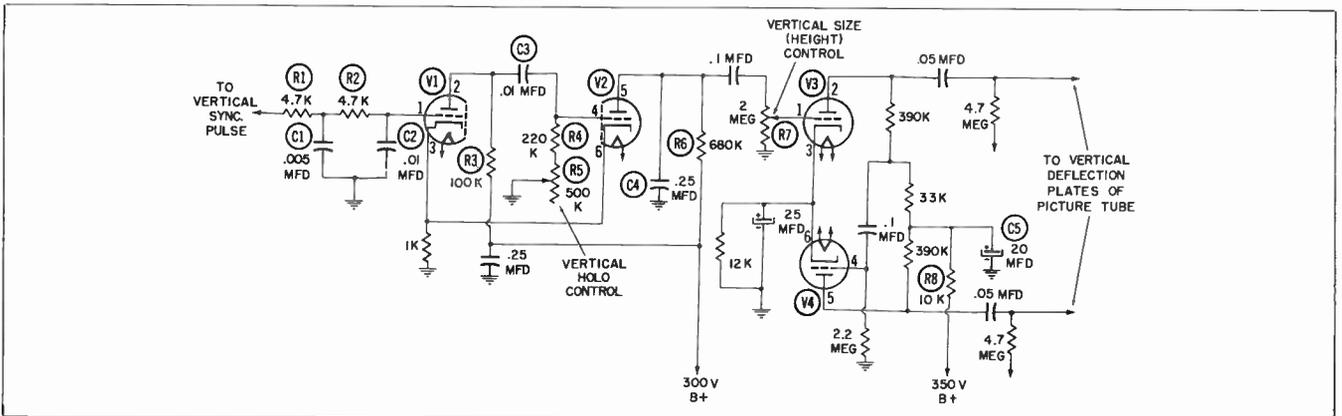
Fig. 8-6. Vertical-deflection circuit for an electrostatic picture tube.
