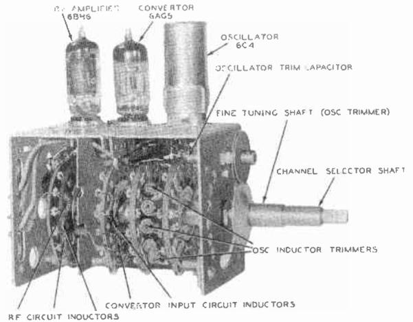
Fig. 12-16. Input tuning system employing rotary-switch inductors.
