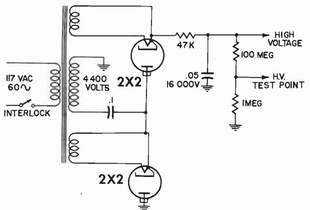
Fig. 4-2. "Brute Force" type high-voltage power supply employing doubler circuit.
