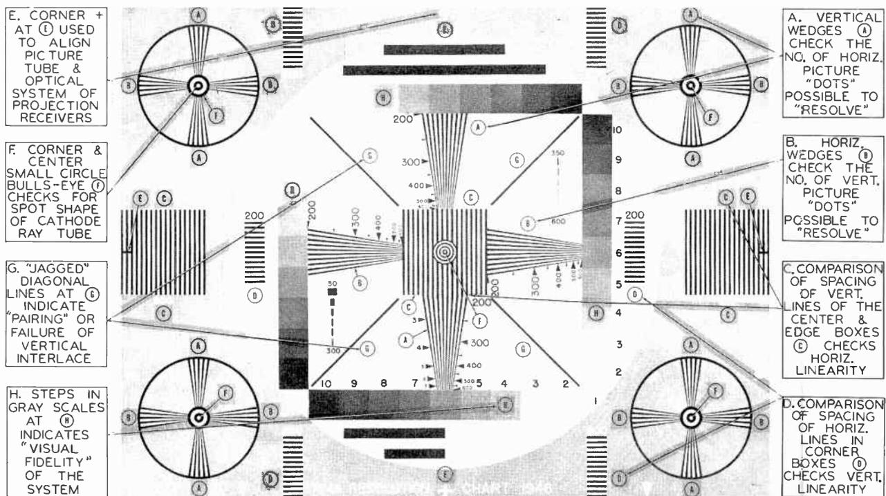
**Fig. 17-2. A transmitter test chart.**
