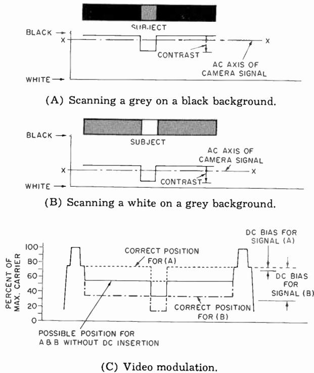
Fig. 9-9. Examples of why DC component of video signal is needed.
