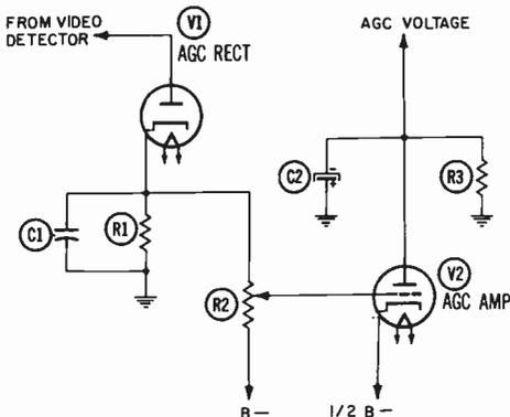
Fig. 16-2. Schematic of amplified-AGC circuit.
