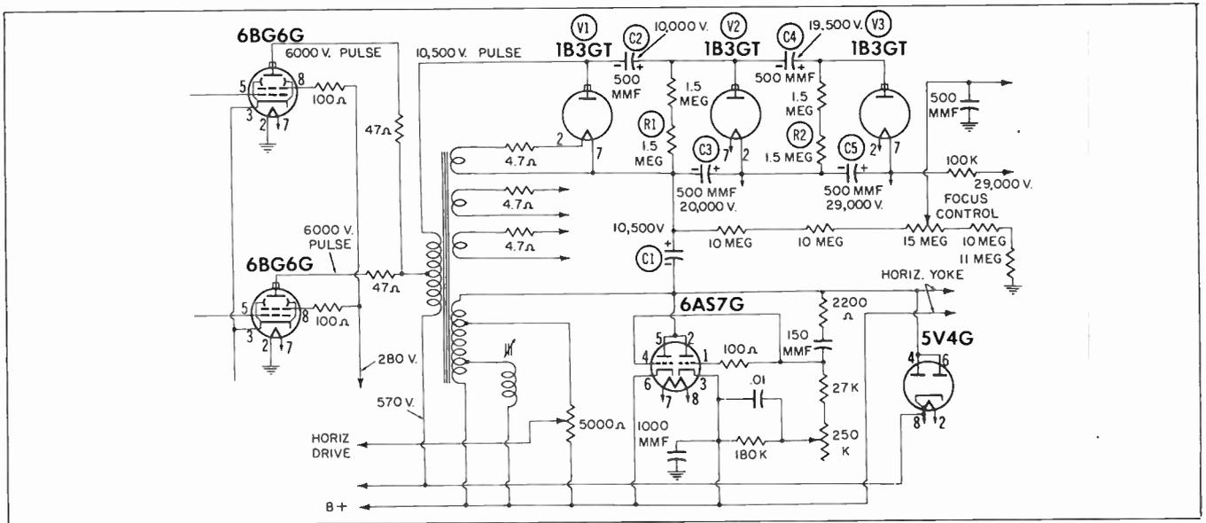
Fig. 4-8. Horizontal-flyback high-voltage tripler.
