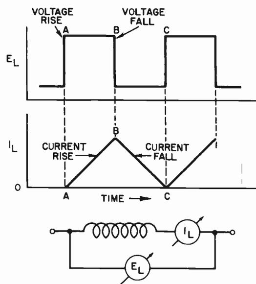
Fig. 7-5. Rise and fall of current through a pure inductance when a square voltage wave is applied.
