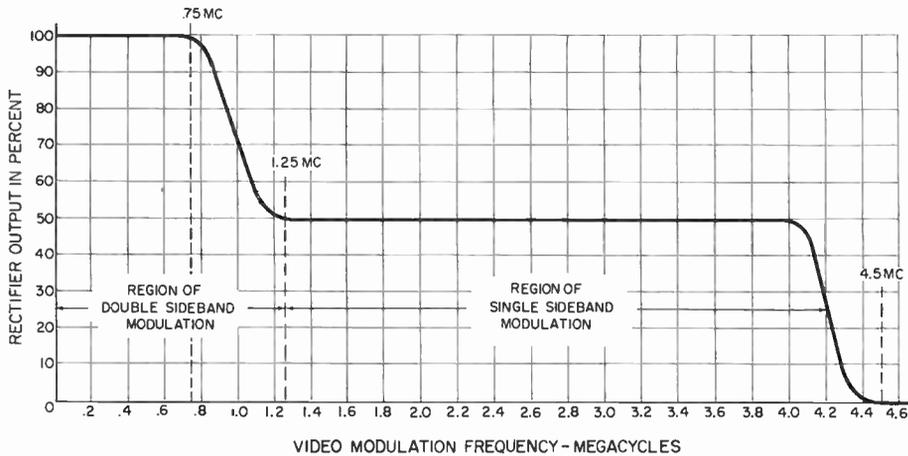
Fig. 13-3. Output of an ideal (linear) detector rectifying the vestigial-sideband modulated video carrier.
