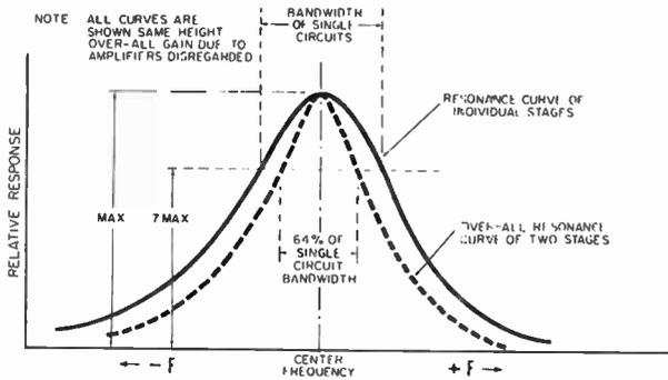
(B) Effect of cascading circuits on the same frequency.
