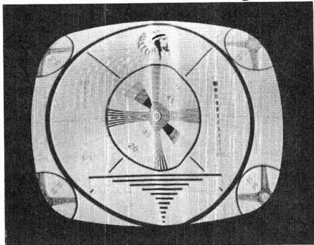
Fig. 17-18. Horizontal drive misadjusted.
