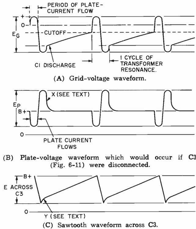
Fig. 6-12. Voltage waveforms in a blocking oscillator.
