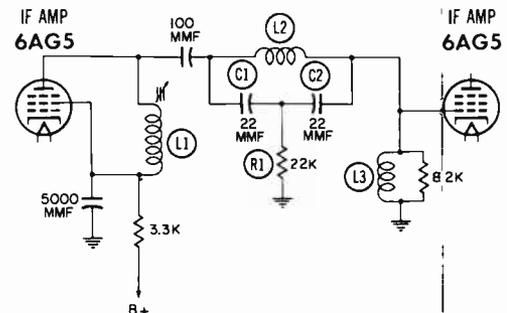
Fig. 13-10. The bridged-T network used as a trap.
