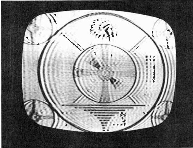
Fig. 15-12. A test pattern, showing the effect of transient oscillation.
