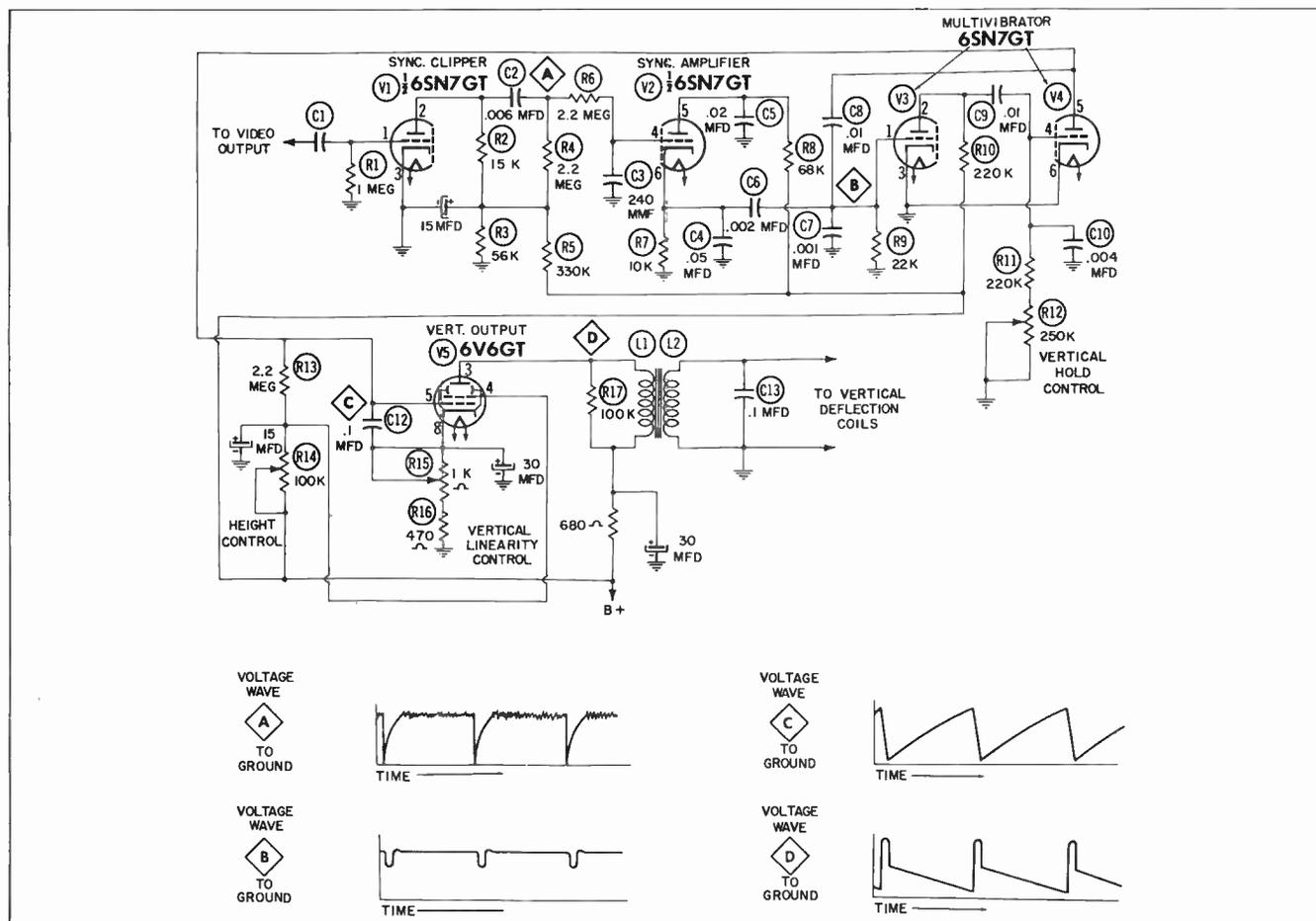
Fig. 8-11. Vertical-deflection circuit using multivibrator.
