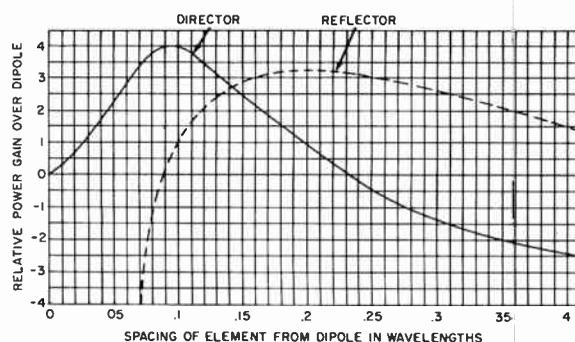
(B) Effect of director and reflector spacing on gain of parasitic array.
