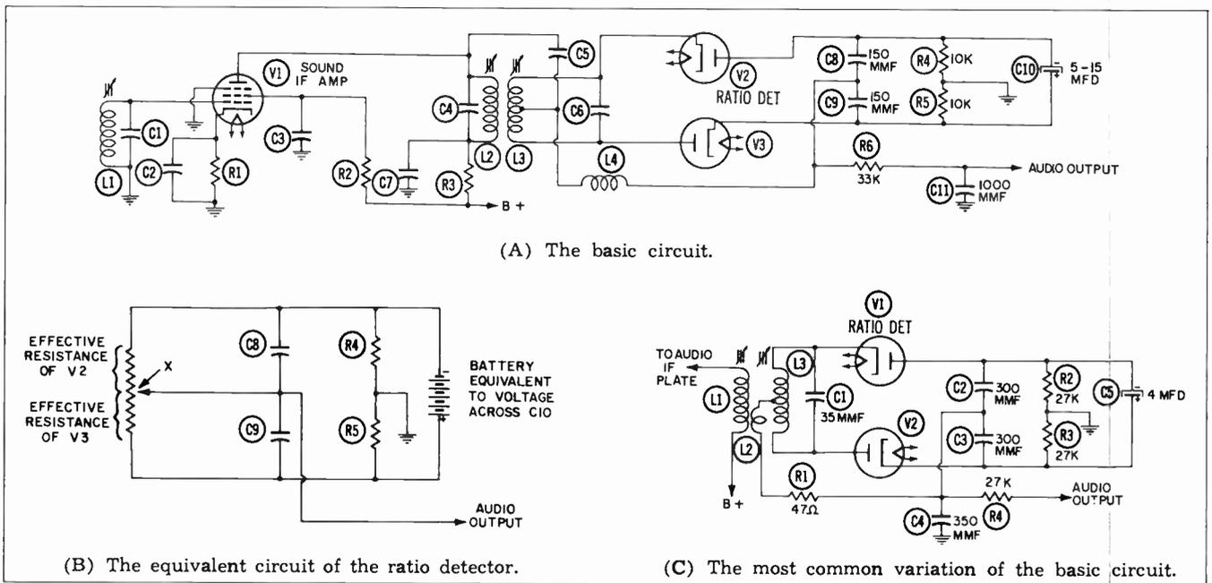
Fig. 14-7. Ratio-detector circuits.
