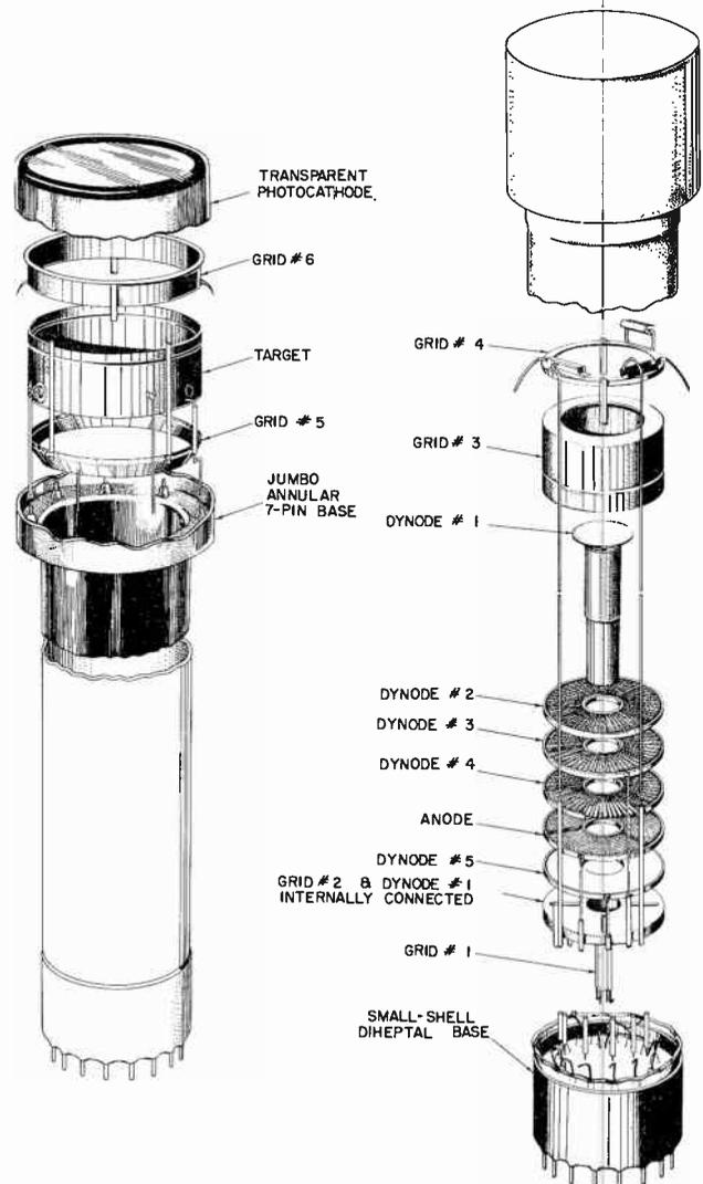
Fig. 3-2. RCA Type 2P23 Image Orthicon.
