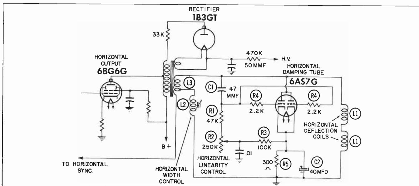
Fig. 8-4. Use of triode as horizontal-damping tube.
