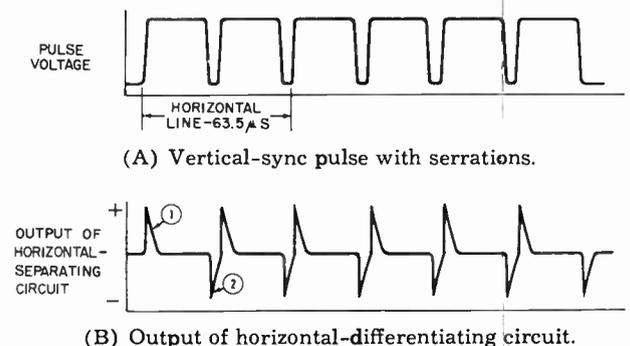
Fig. 10-11. Action of horizontal-differentiating circuit on vertical-sync signal.
