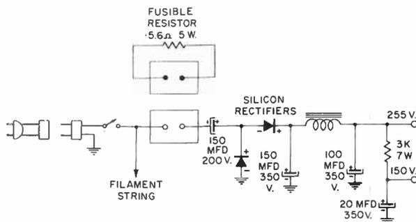
Fig. 4-1D. Schematic of typical low-voltage power supply used in portable television receivers.
