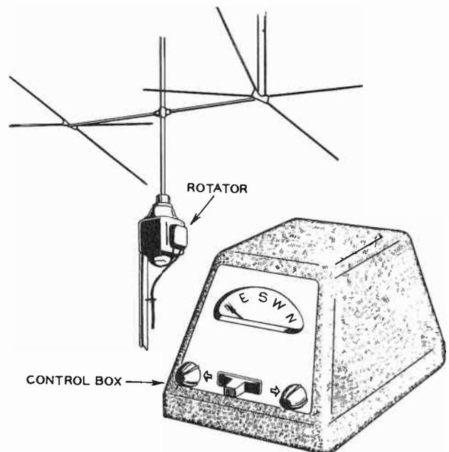
Fig. 11-17. Typical antenna rotator installation.
