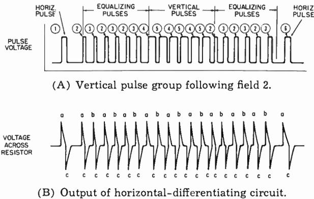
Fig. 10-15. Action of horizontal-differentiation circuits during vertical pulse period.
