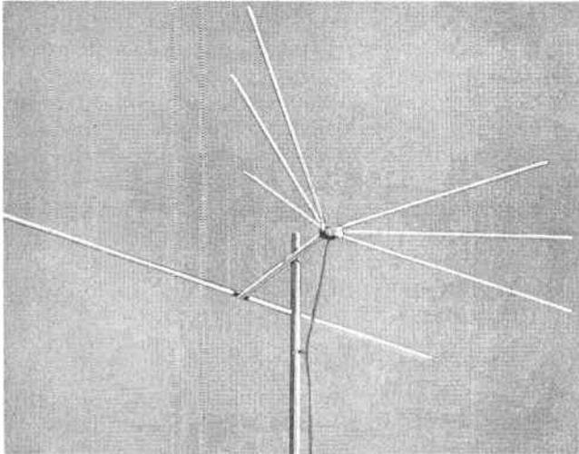
Fig. 11-13. A fan, or "conical," antenna having a broadband response.
