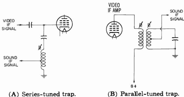
Fig. 13-11. Take-off points for sound-IF signal in nonintercarrier receivers.
