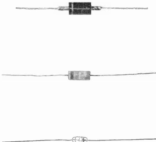
Fig. 13-18. Three types of fixed crystal detectors. (Shown actual size.)
