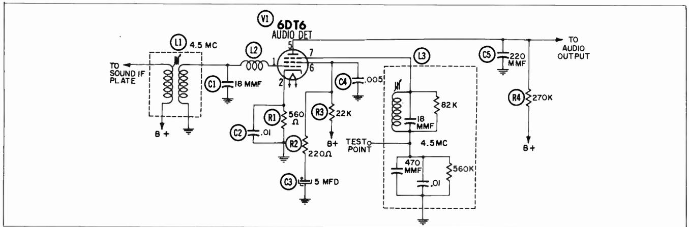
Fig. 14-10. The locked-oscillator 6DT6 detector.
