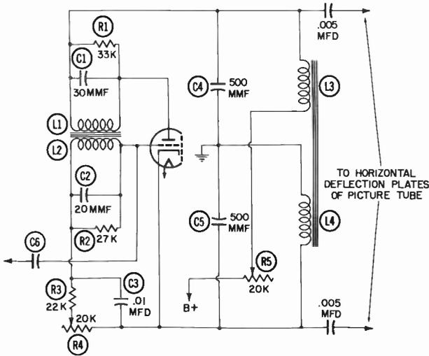
Fig. 8-9. Blocking oscillator—horizontal electrostatic-deflection circuit.
