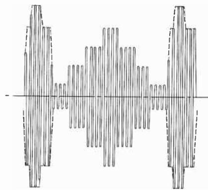
(D) Carrier envelope produced by modulation in C.
