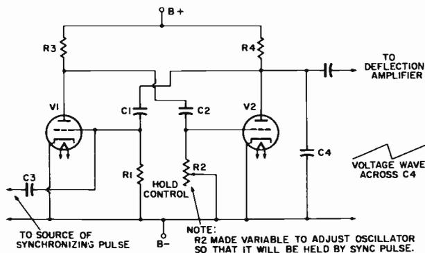
Fig. 6-8. Asymmetrical multivibrator, showing input coupling and sawtooth-forming capacitor.
