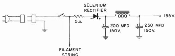
Fig. 4-1C. Schematic of typical low-voltage power supply using a selenium rectifier.
