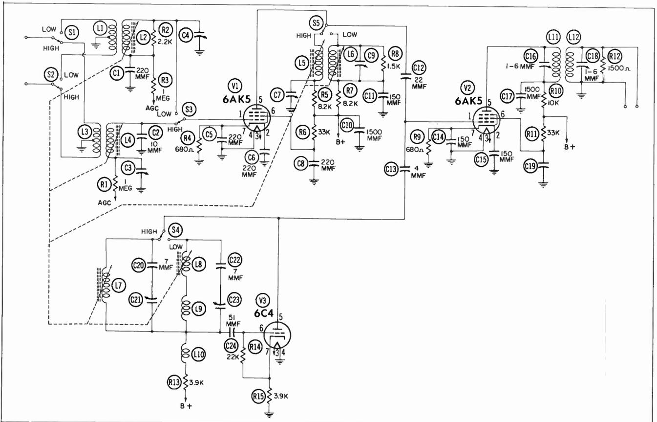
Fig. 12-9. Schematic of the iron-core tuning system illustrated in Fig. 12-8.
