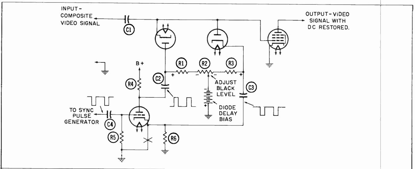
Fig. 9-10. Typical double-diode clamp circuit for reinserting DC at transmitter.
