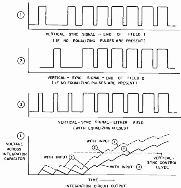
Fig. 10-14E. Action of vertical-integrating circuit for successive fields (with and without equalizing pulses).
