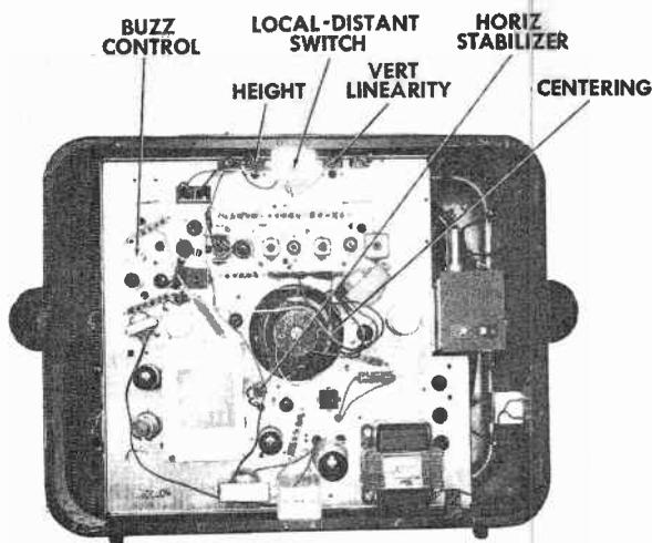
(B) Receiver employing vertical chassis. Back cover must be removed to adjust controls, except for two controls accessible from top of cabinet.
