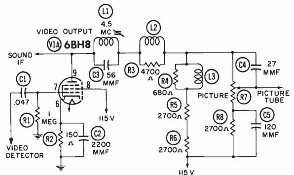
**Fig. 15-7. Video stage with both high- and low-frequency compensation.**
