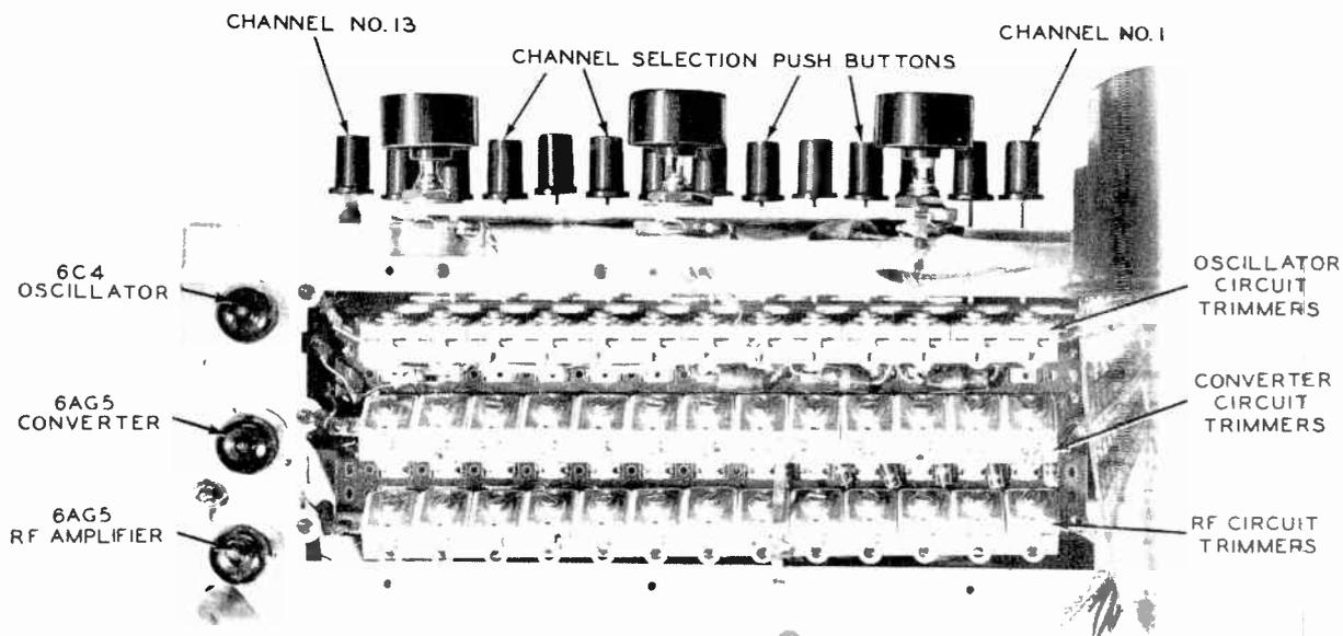
Fig. 12-12. Tuner employing push-button, trimmer-tuned circuits.
