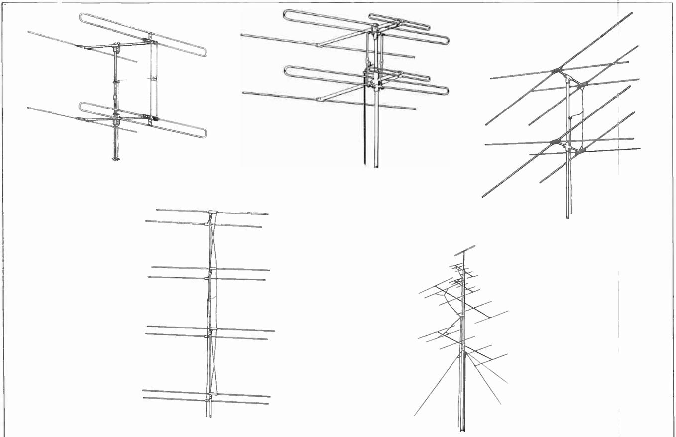
Fig. 11-15. Stacked arrays for higher gain and improved directional pattern.
