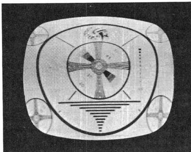
Fig. 17-19. Vertical-linearity control misadjusted.
