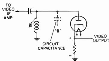
(B) Video output increases positively with respect to ground as carrier increases.
