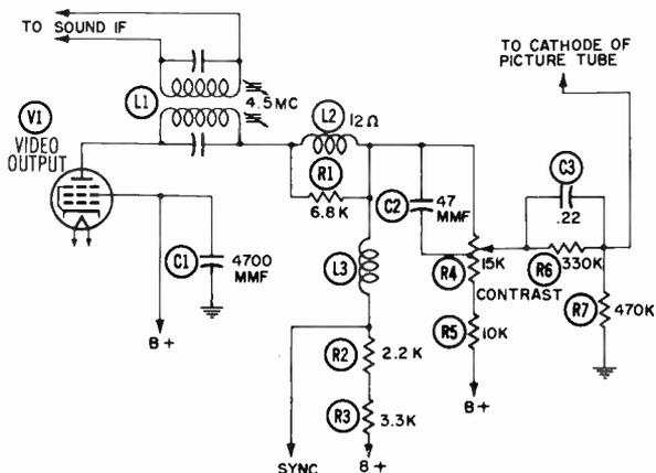
Fig. 15-16. Contrast-control circuit in coupling to picture tube.
