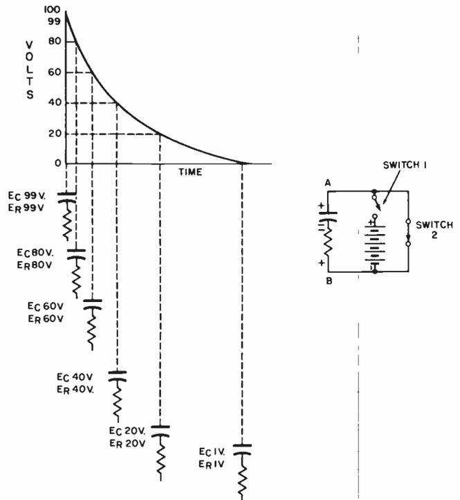
Fig. 5-2. Resistor-capacitor discharging curve.
