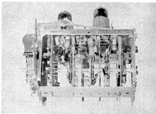
Fig. 12-18. A modern switch-type tuner.
