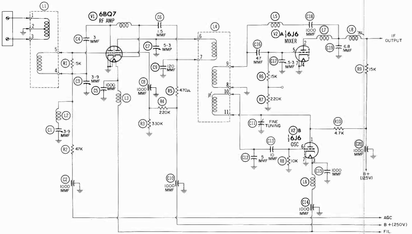
Fig. 12-21. Schematic diagram showing one version of the turret tuner.
