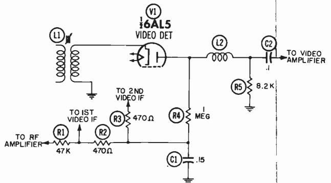
(A) AGC circuit composed of a simple filter network with a time constant of approximately 0.15 second.
