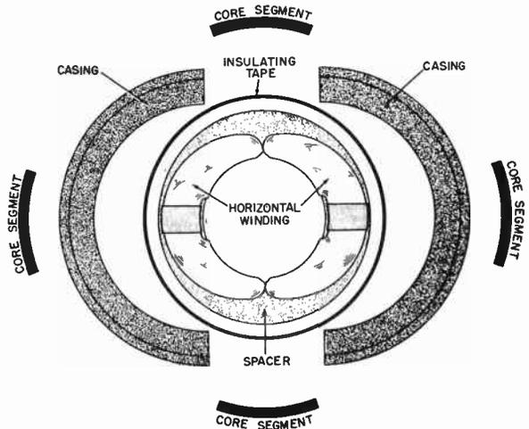
(C) Overhead view of windings and spacers arrangement.
