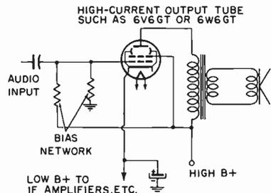
Fig. 4-1G. Schematic of power supply using audio output tube as voltage divider.
