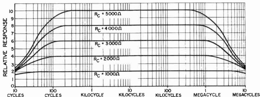
Fig. 15-3. Effect of plate-coupling resistor on gain and bandwidth.
