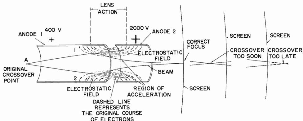
Fig. 1-4. Effect of an electrostatic field on an electron beam.
