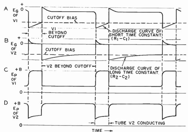
Fig. 6-7. Waveforms of an asymmetrical, or unbalanced, multivibrator.
