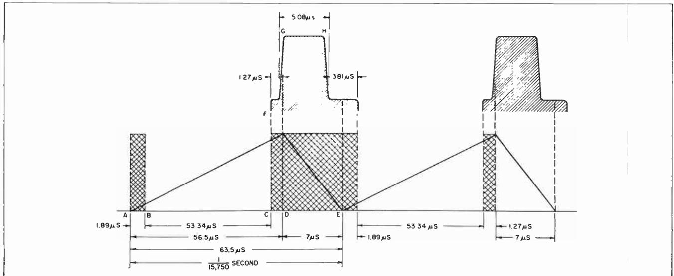
Fig. 7-1. Horizontal-scanning wave and synchronizing signal.
