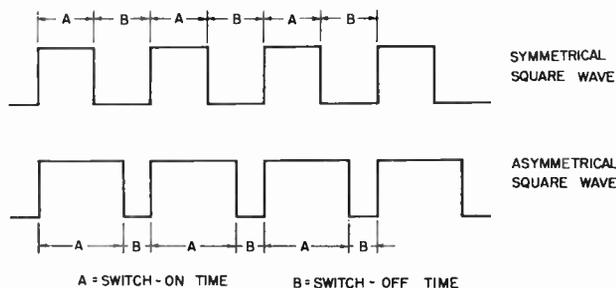
Fig. 5-5. Square waveforms.
