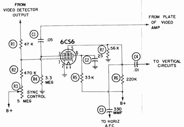
Fig. 10-8. Schematic of a gated-sync circuit.
