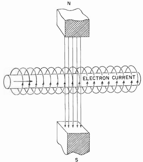
**Fig. 2-4. Conductor at right angles to magnetic field.**
