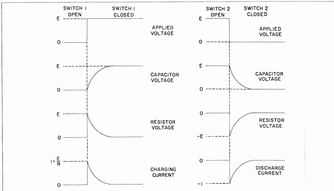
Fig. 5-4. R-C charge and discharge curves.
