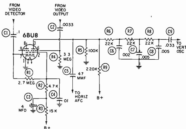
Fig. 10-9. The 6BU8 gated-separator circuit.
