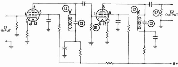
(A) Single-tuned coupling circuits between video IF stages.
