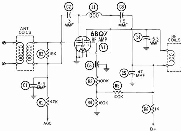
Fig. 12-5. The cascode RF amplifier circuit.
