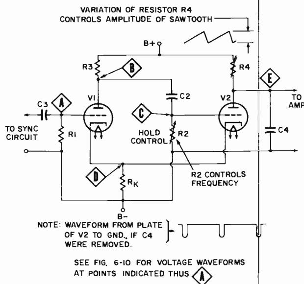
Fig. 6-9. A cathode-coupled multivibrator.
