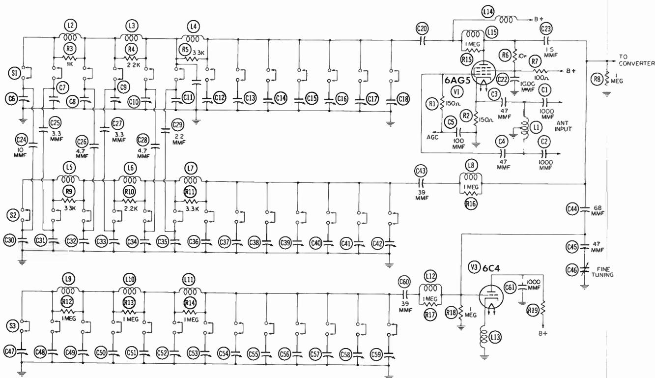
Fig. 12-13. Schematic of tuner shown in Fig. 12-12.
