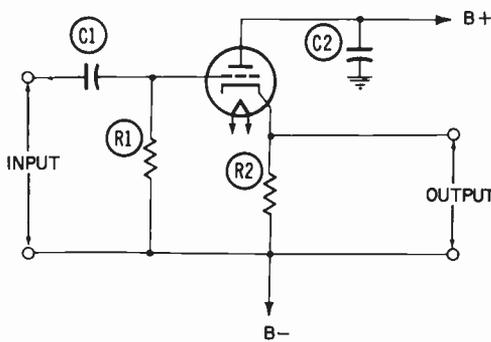
Fig. 10-2. The basic cathode-follower circuit.
