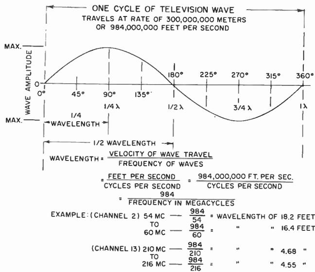
Fig. 11-4. Relation of carrier frequency to wavelength of television signal.
