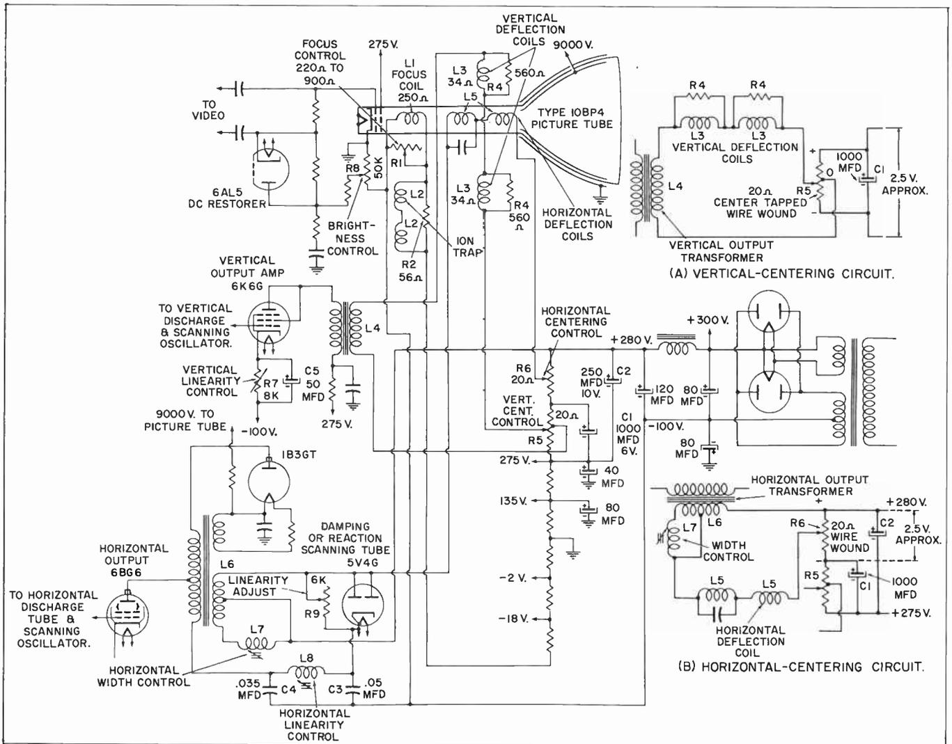
Fig. 8-1. An early type of electromagnetic-deflection system.
