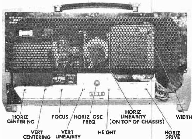
(D) Service controls at back of the chassis. Controls on top chassis and picture tube are accessible by removing protective screen.
