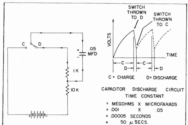
**Fig. 5-9.** Capacitor discharge circuit for sawtooth waveform.
