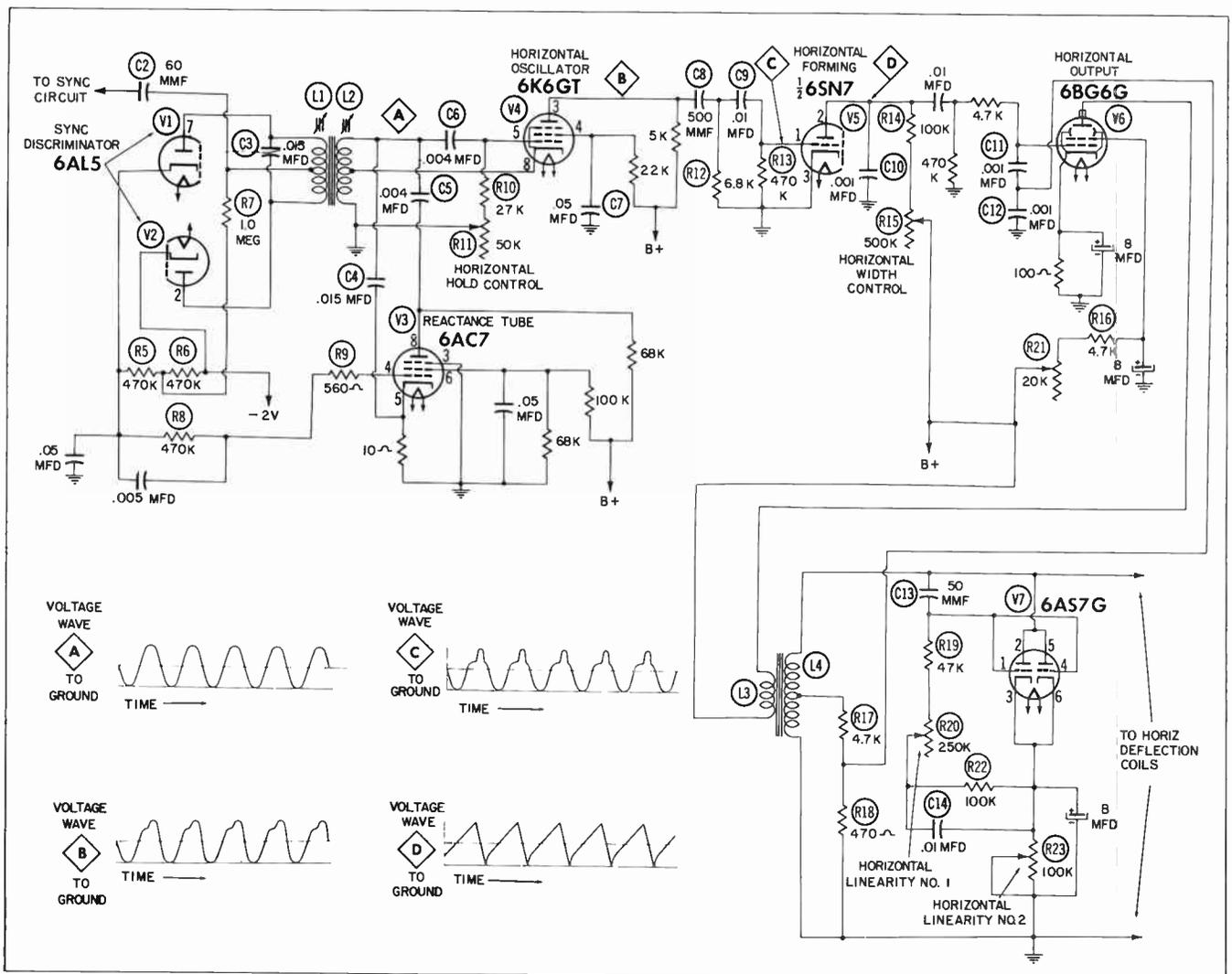
Fig. 8-13. Horizontal-deflection system using sine-wave oscillator and flywheel AFC.
