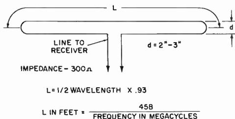
Fig. 11-8. Dimensions of a folded dipole.
