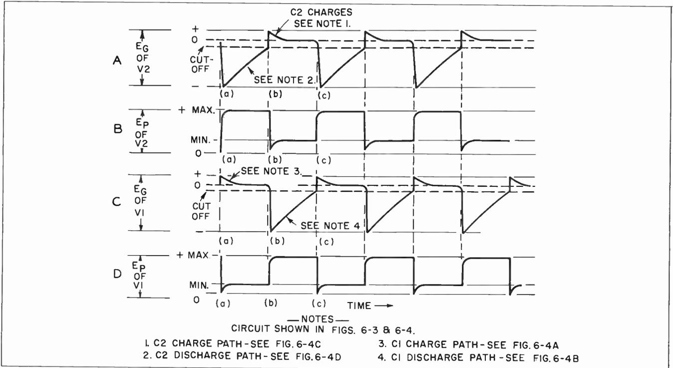
Fig. 6-6. Typical waveforms of a symmetrical multivibrator, showing square-wave switch action.
