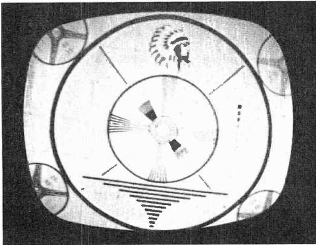
Fig. 17-6. Deflection yoke not properly adjusted.
