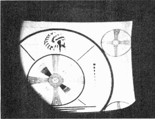
Fig. 17-5. Focus coil and ion trap misaligned.
