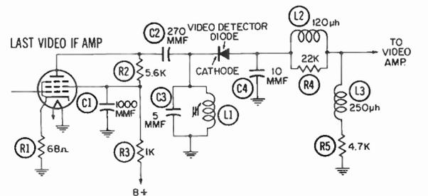
(A) Crystal diode with series load.
