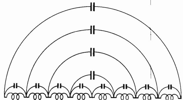
(B) Electrical circuit equivalent of the dipole.
