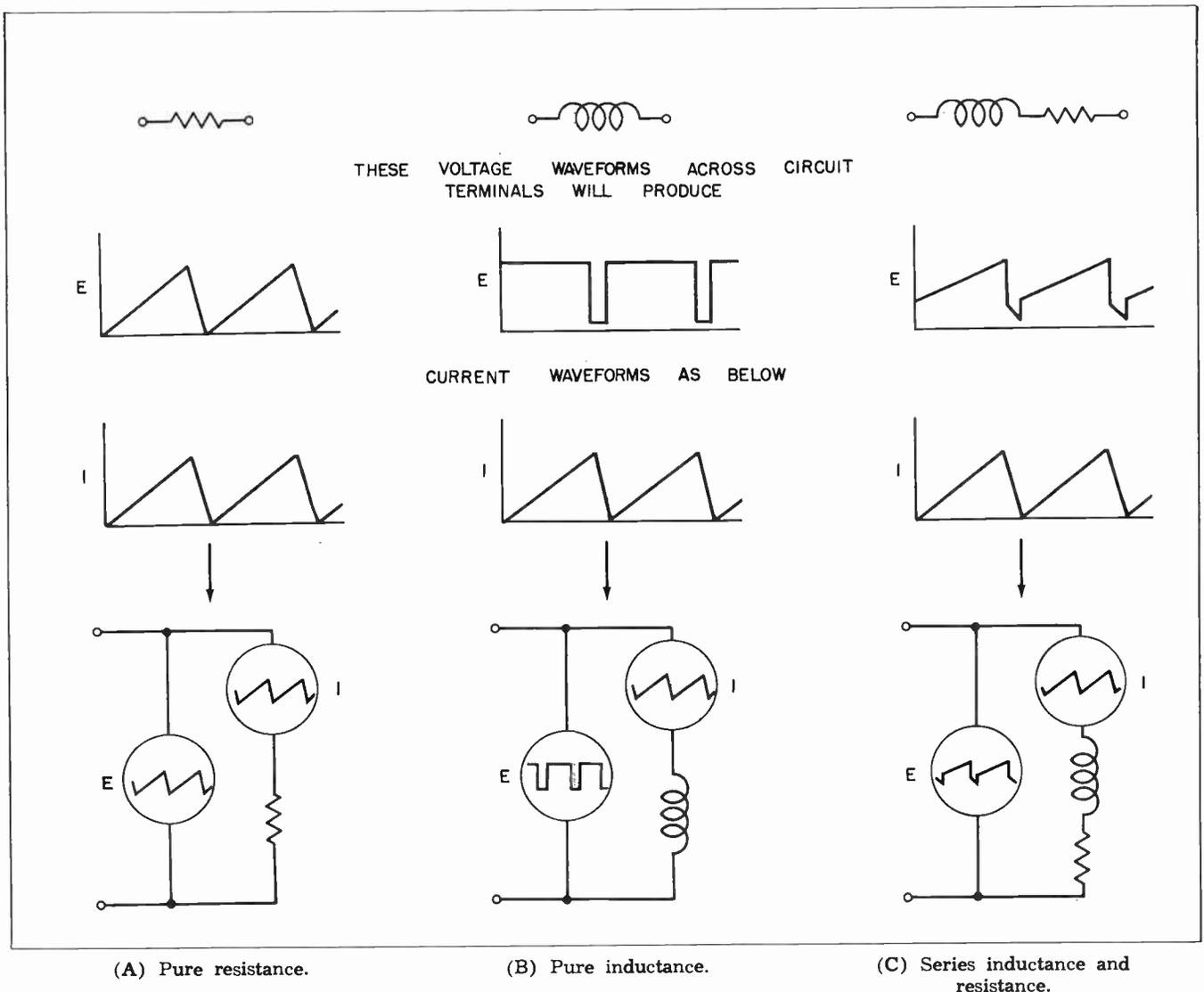
**Fig. 7-6. Voltage and current waveforms in inductance and resistance circuits.**
