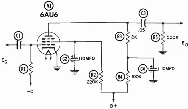
(A) Low-frequency compensation for effect of coupling network C3-R5.
