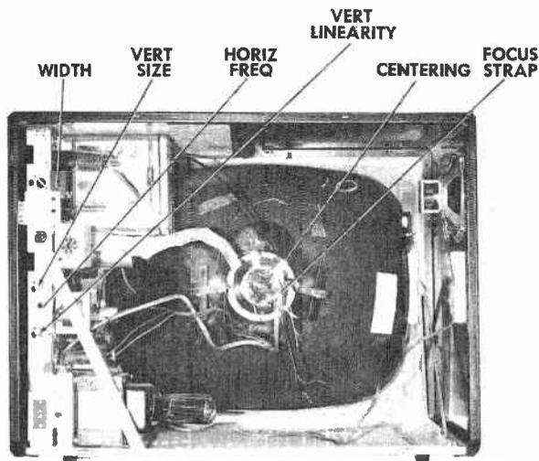
(A) Service controls located at back of chassis. Back cover is removable for servicing picture-tube controls.
