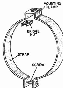
(D) Metal strap which holds core segments in place.
