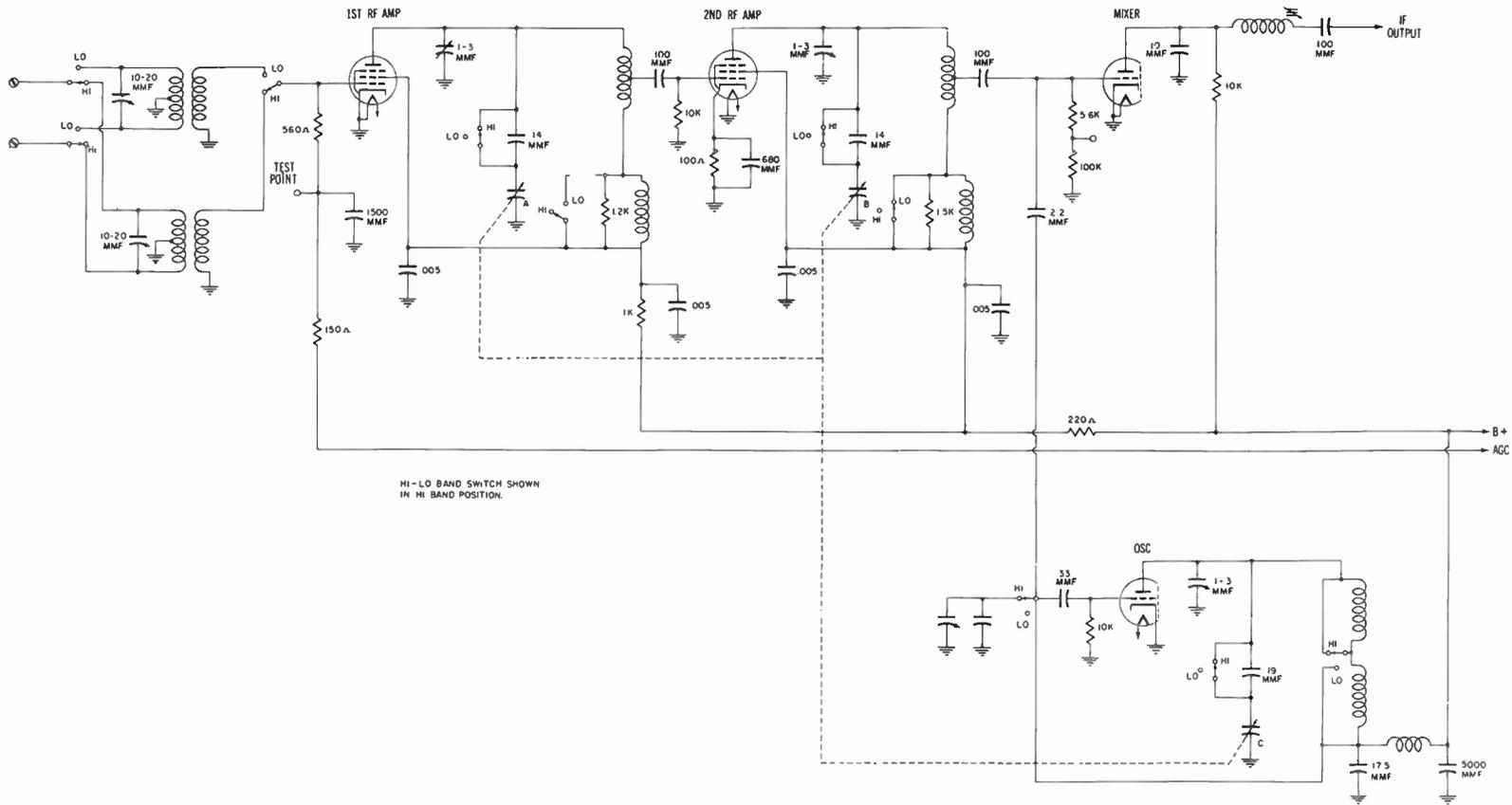
Fig. 12-11. Schematic of the tuner shown in Fig. 12-10.
