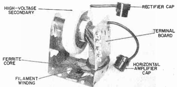
Fig. 4-7. Typical modern horizontal-flyback transformer.
