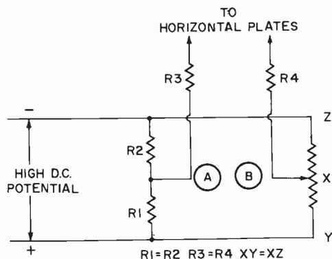
Fig. 1-12. Simplified horizontal-centering circuit.
