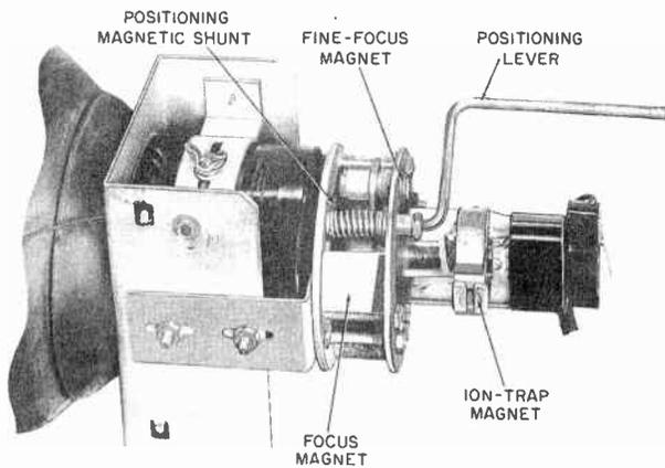
Fig. 2-6. Permanent-magnet focus device.
