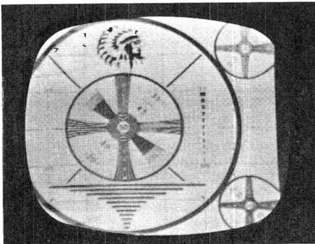
Fig. 17-13. Horizontal centering incorrect.
