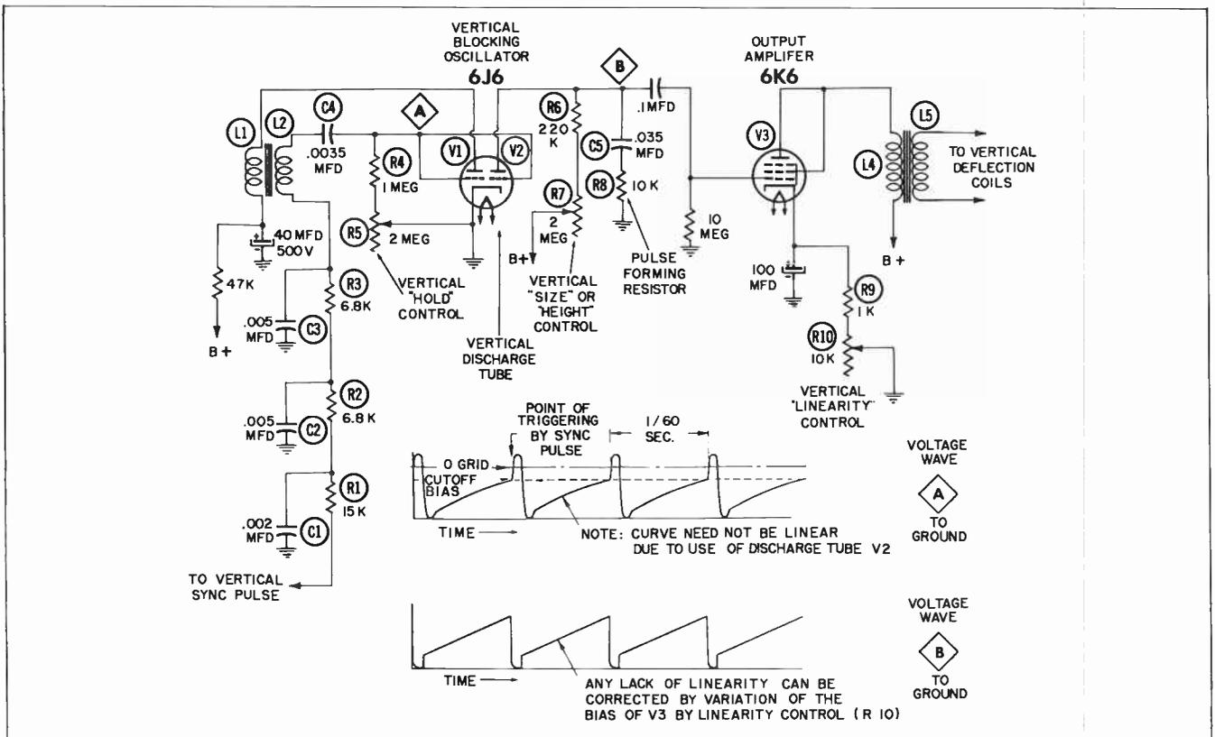
Fig. 8-10. Use of the blocking oscillator in a vertical-sweep circuit.
