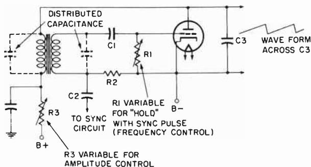
Fig. 6-11. Blocking oscillator.
