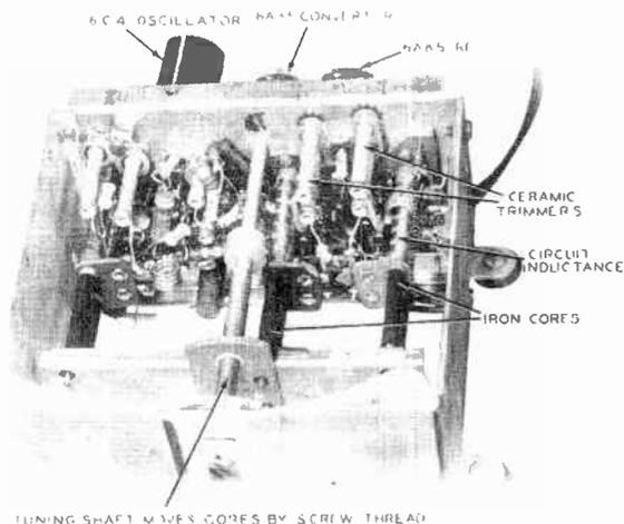
Fig. 12-8. A variable-inductance tuner employing movable powdered-iron cores.
