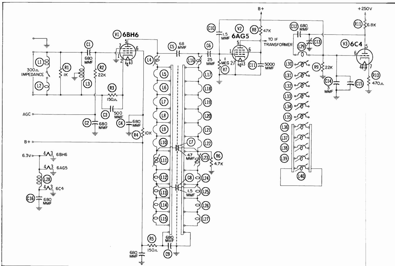
Fig. 12-17. Schematic diagram of tuner illustrated in Fig. 12-16.
