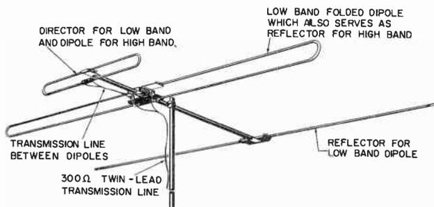
Fig. 11-11. "In-line" antenna array of folded dipoles for reception on both bands.
