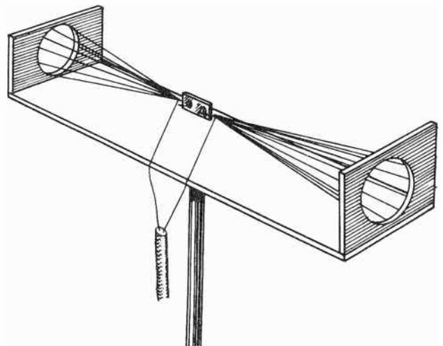
Fig. 11-12. The cage antenna—a variation of the dipole for wide-band reception.
