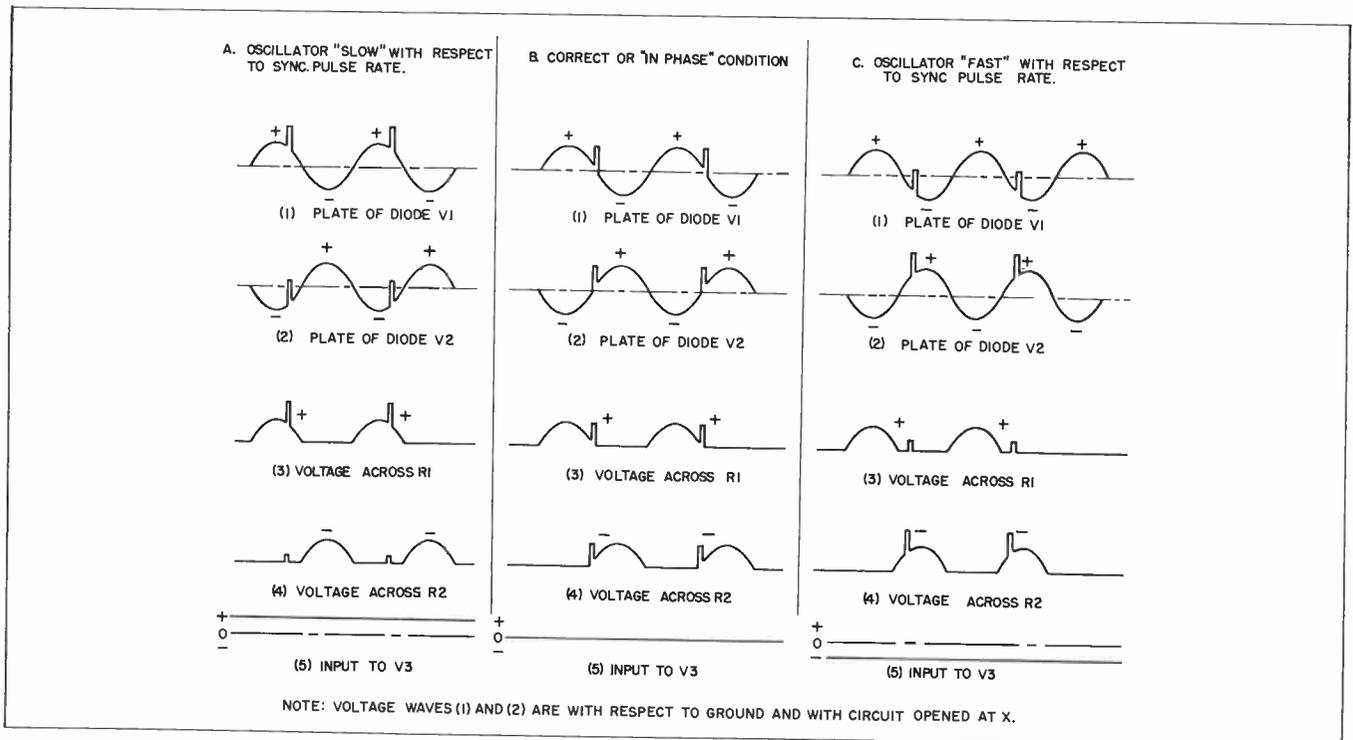
Fig. 8-21. Discriminator action in horizontal AFC sync control circuit of Fig. 8-20.
