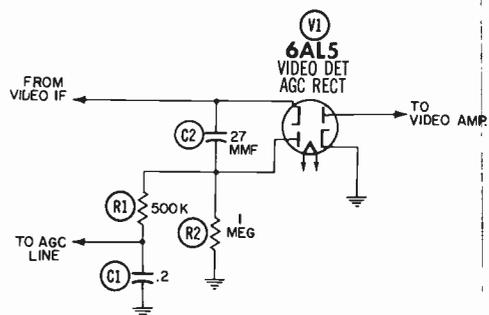
(B) AGC circuit with improved action obtained by a lengthened time constant in the discharge path.
