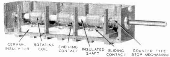
(A) Top view of tuning mechanism (shield removed).
