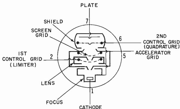
Fig. 14-9. Internal construction of the 6BN6 tube.
