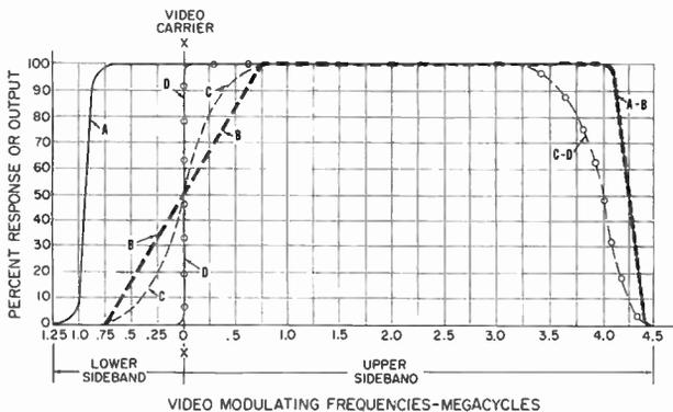
Fig. 13-4. Over-all receiver characteristic required to compensate for vestigial-sideband modulation.
