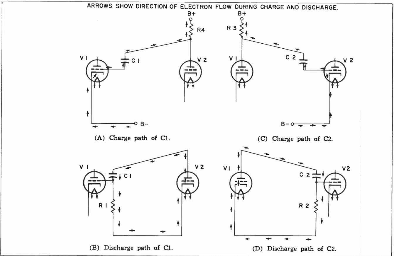
Fig. 6-4. Capacitor charge and discharge paths in a multivibrator.
