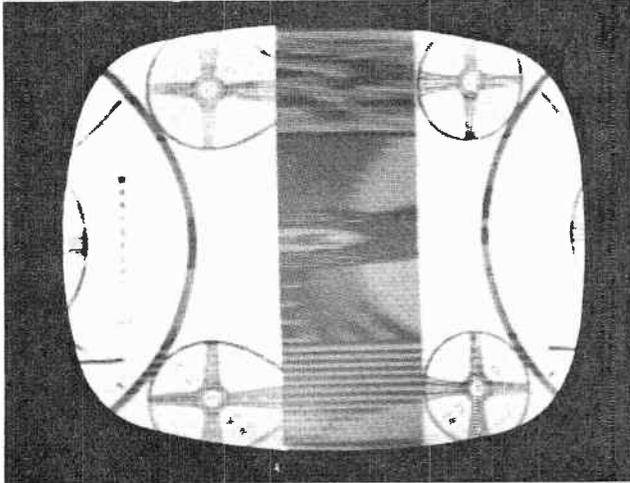
Fig. 17-12. Horizontal-discriminator phase misadjusted. (AFC system.)
