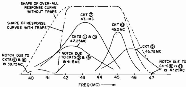
Fig. 13-9. The effect of cascading the staggered-tuned circuits of Fig. 13-8.
