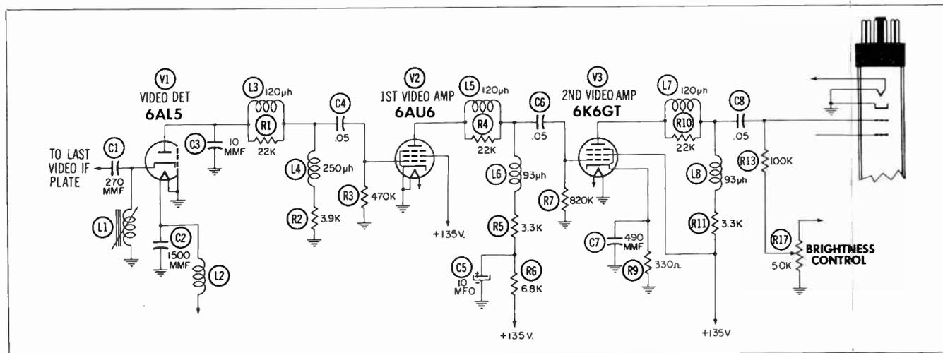
Fig. 13-15. Video detector of negative polarity feeding picture-tube grid through two video-amplifier stages.
