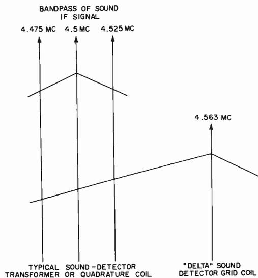
**Fig. 14-12. The frequency-response curve of the delta sound detector.**
