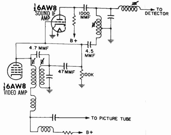
Fig. 14-4. A neutralized triode used as a sound IF amplifier.
