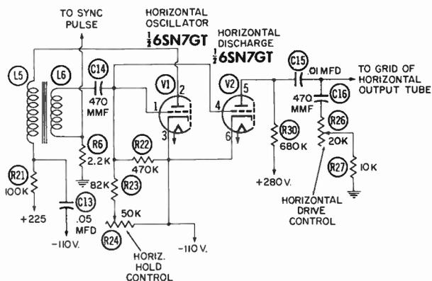
Fig. 8-16. Blocking-oscillator type of horizontal scanning generator.
