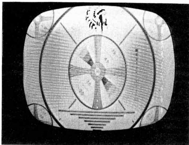
Fig. 17-16. Height control misadjusted.
