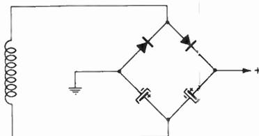
Fig. 4-1F. Schematic of Fig. 4-1E redrawn to show bridge configuration.
