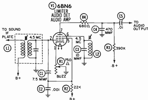
Fig. 14-8. The gated-beam 6BN6 detector.
