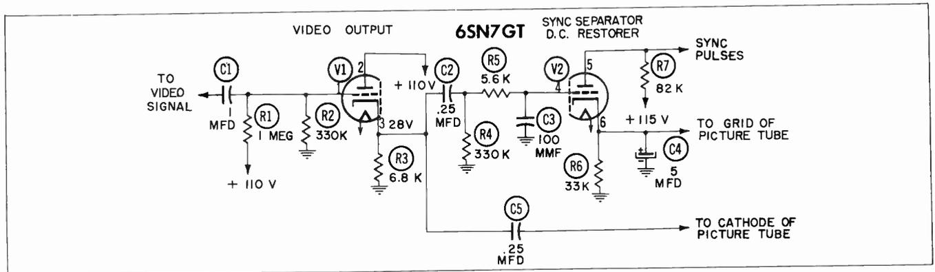
Fig. 10-7. Cathode-follower used with sync-separator.
