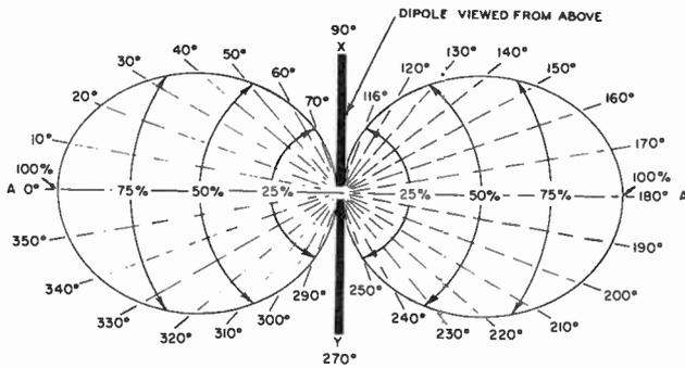
(A) Reception pattern of a half-wave dipole, showing relative response versus direction in a horizontal plane.
