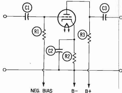
(A) Fixed bias in series with grid-return resistor.
