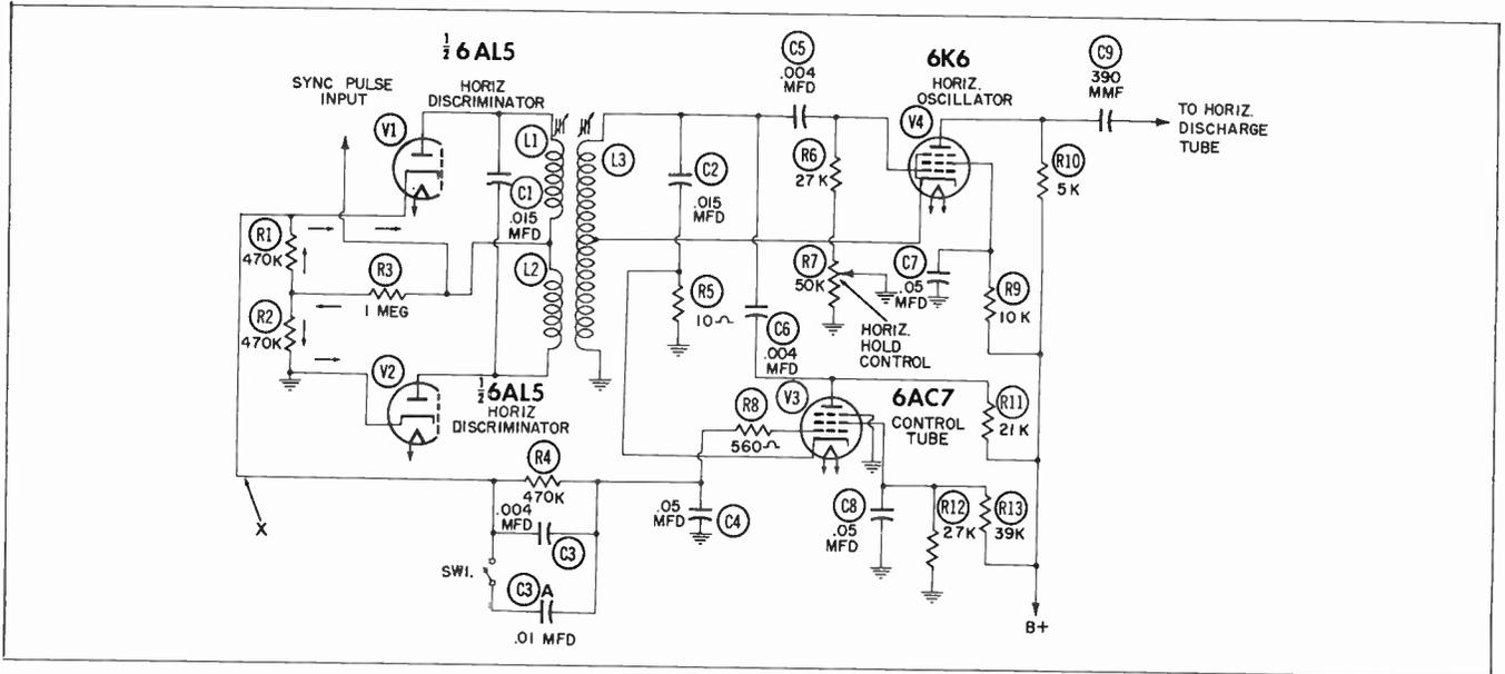
Fig. 8-20. Circuit using flywheel or AFC control of horizontal-scanning oscillator.
