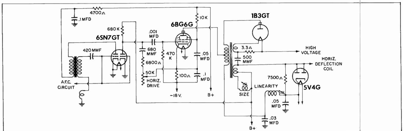
Fig. 4-4. Early type of horizontal-flyback, high-voltage system.
