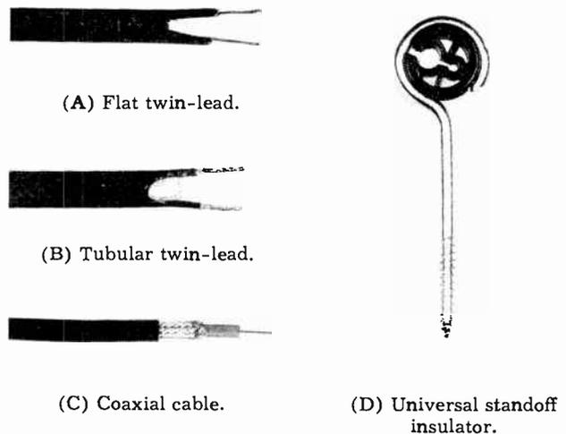
Fig. 11-18. Types of lead-ins and a standoff.
