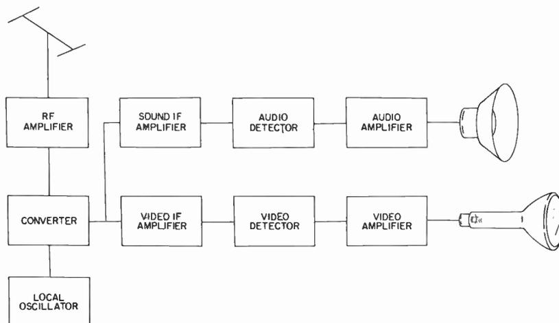
Fig. 13-1. Block diagram of a dual-IF channel television receiver.
