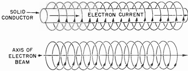
**Fig. 2-2. Similarity of solid conductor and electron beam.**
