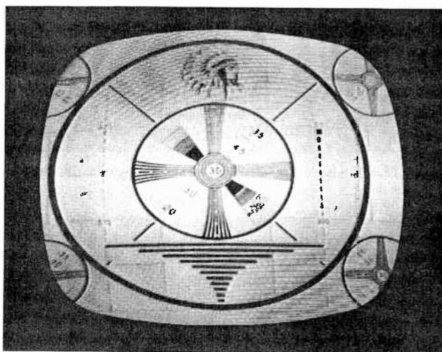
Fig. 17-17. Horizontal-linearity control misadjusted.
