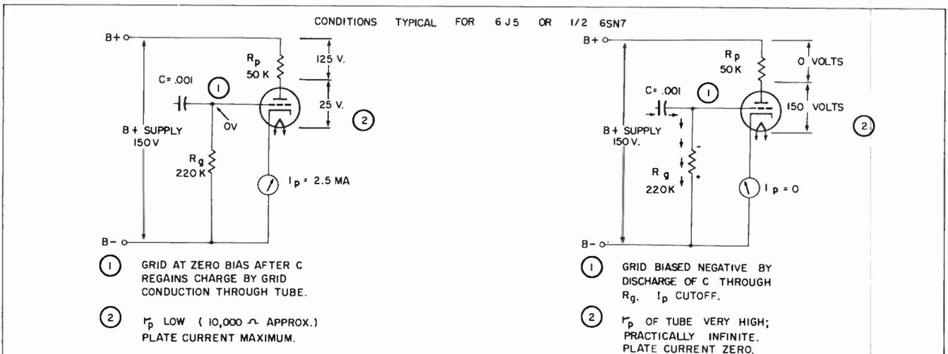
Fig. 6-5. Tube operating conditions in a multivibrator.
