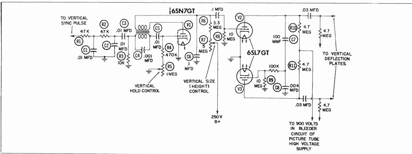
Fig. 8-8. Blocking oscillator—vertical electrostatic-deflection circuit.
