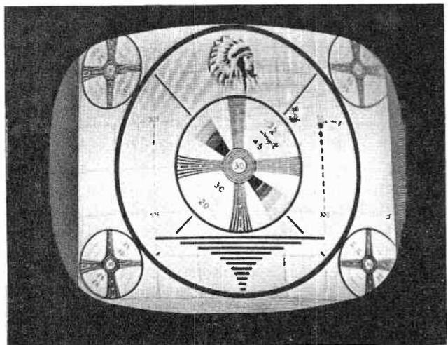
Fig. 17-15. Width control misadjusted.
