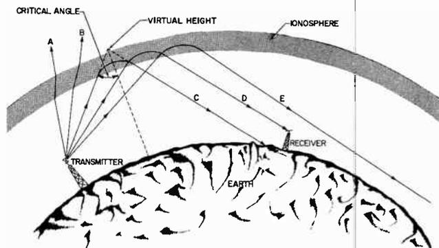
Fig. 11-2. The bending of radio waves back to the earth from the ionosphere. (Occurs at frequencies below 40 megacycles.)
