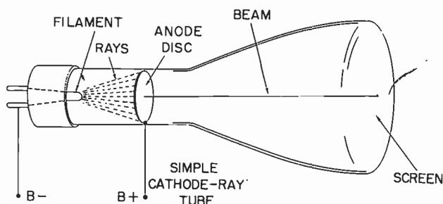
Fig. 1-1. Formation of a narrow beam of electrons. (Early experimental form.)
