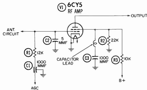
Fig. 12-4. The tetrode RF amplifier circuit.
