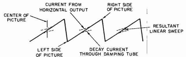
Fig. 8-3. Current waveforms in horizontal scanning.
