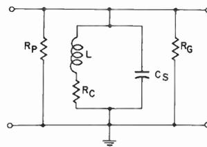
(B) High-frequency equivalent circuit.
