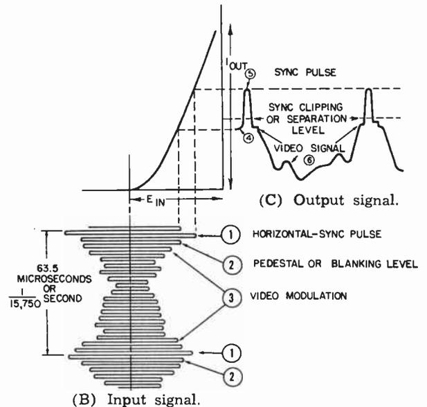
Fig. 10-3. Demodulation (detection) of the video (picture) carrier.
