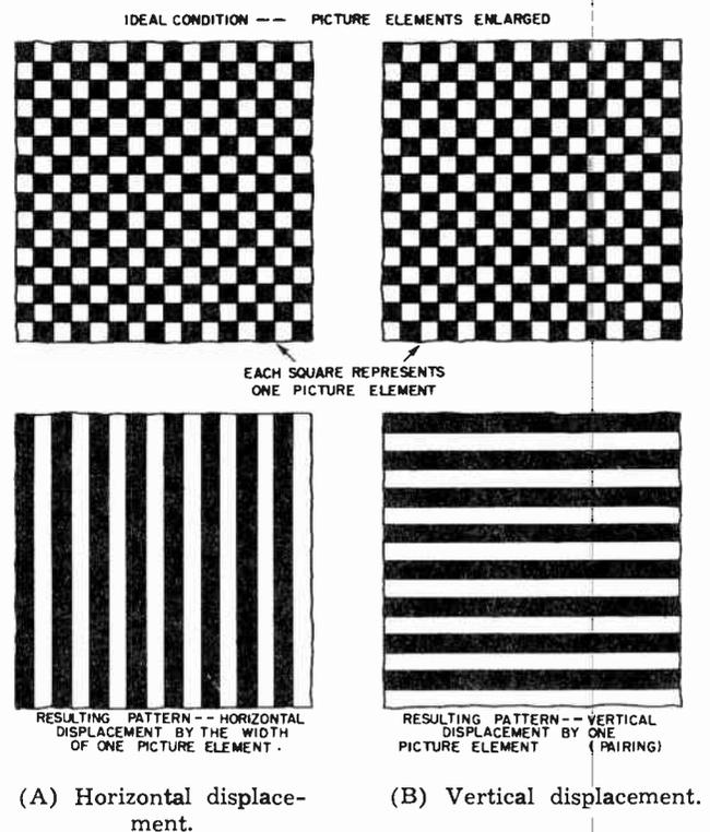
Fig. 7-3. Picture-element displacement which might result from scanning-oscillator instability.
