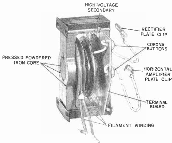
Fig. 4-5. Typical early horizontal-flyback transformer. (Photo from sample, courtesy of RCA.)
