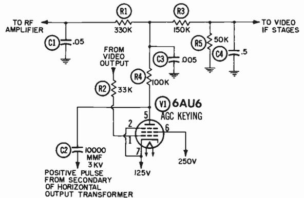
Fig. 16-3. Schematic of keyed-AGC circuit.
