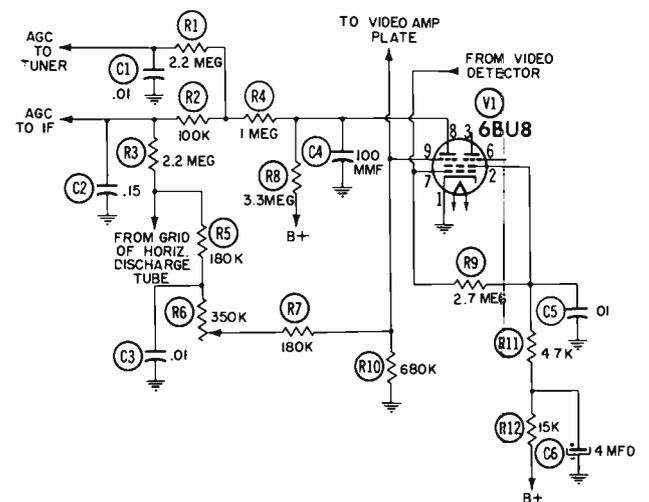
Fig. 16-4. Schematic of the 6BU8 AGC circuit.
