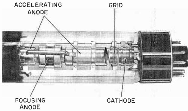
**Fig. 1-8. Electron gun of a low-electrostatic focus tube.**
