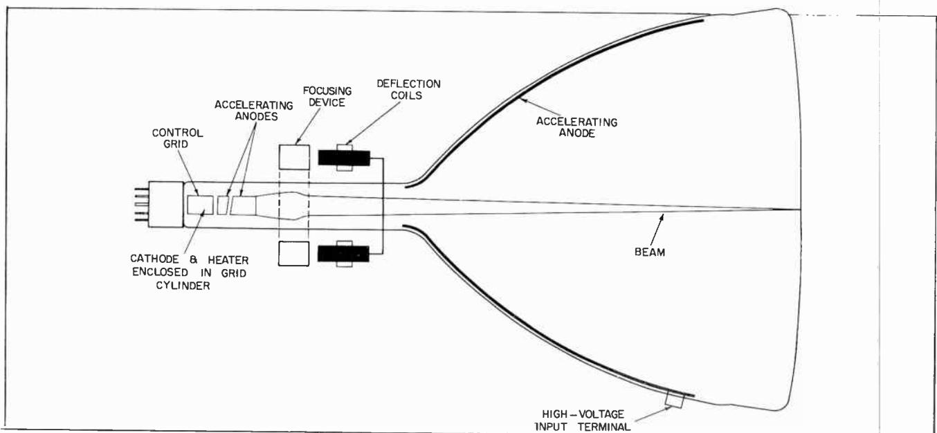
Fig. 2-1. Magnetically-controlled cathode-ray tube.
