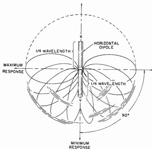
(B) Solid pattern in space of half-wave dipole.
