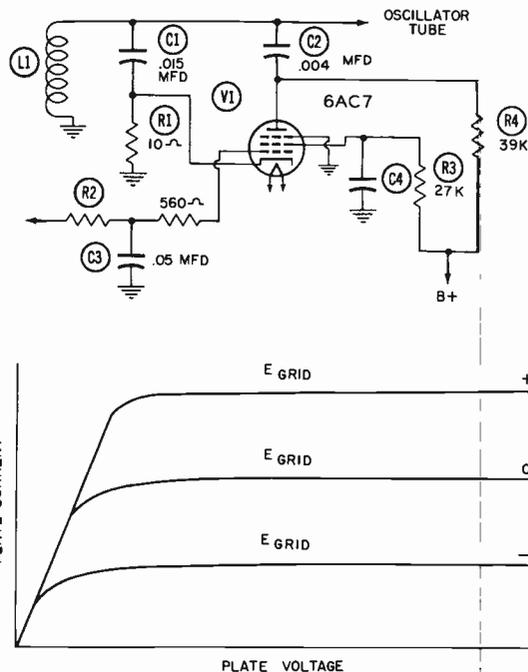
Fig. 8-22. Reactance-control operation.
