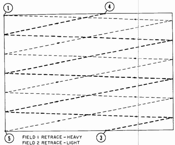
Fig. 10-14B. Inactive upward fields (vertical retrace).
