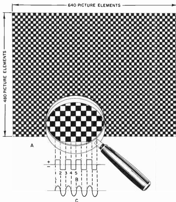
Fig. 9-3. Video modulation produced by scanning a checker board in which the picture elements are the limit of system resolution.
