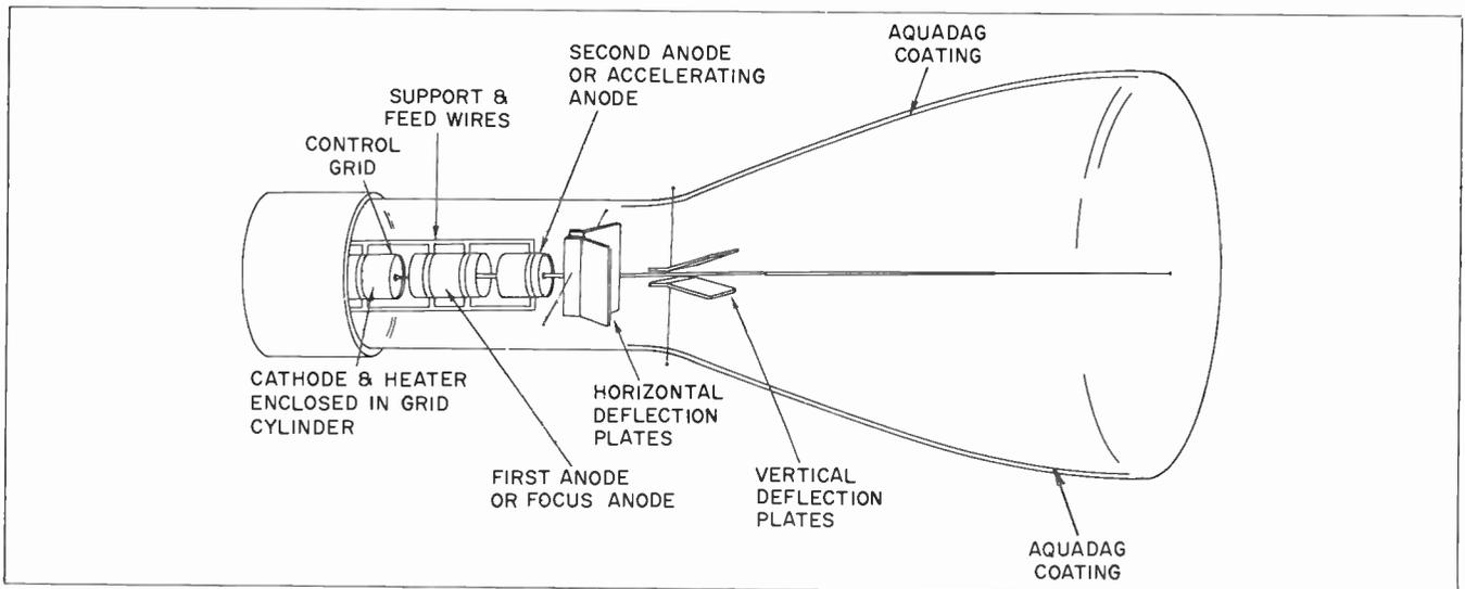
**Fig. 1-10. Electrostatic focus and deflection.**
