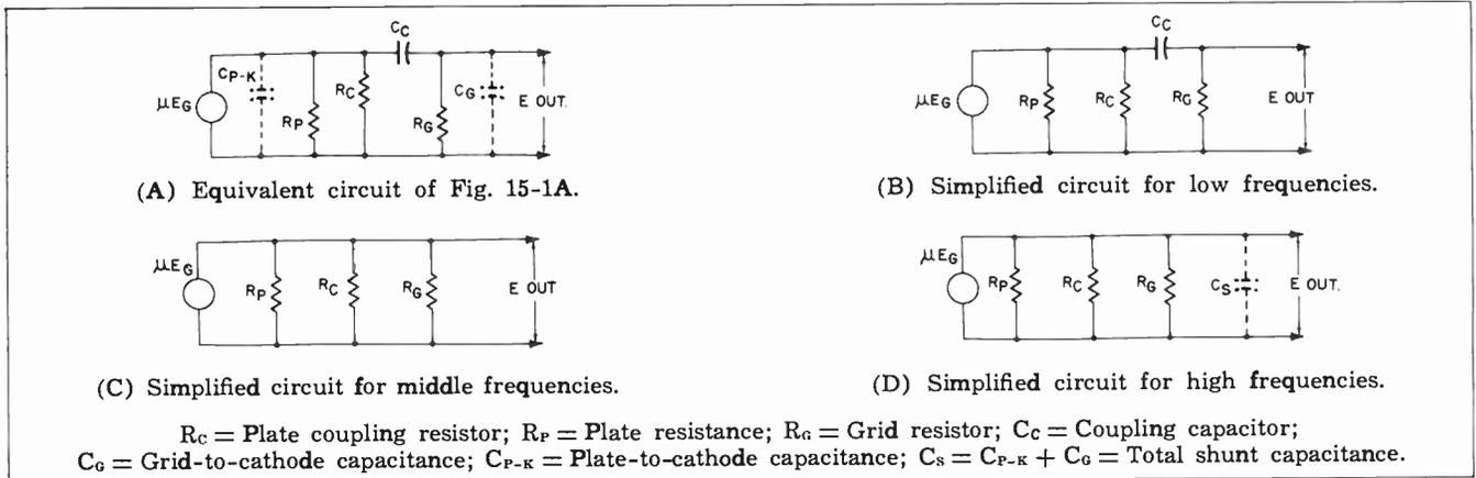
Fig. 15-2. Equivalent circuits of resistance-coupled stage at low, middle, and high frequencies.
