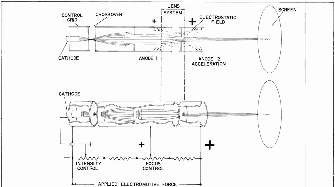
Fig. 1-7. Electron gun assembly.
