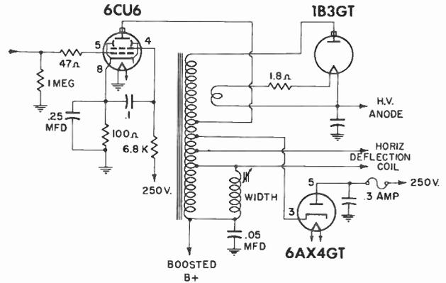
Fig. 4-6. Modern type of horizontal-flyback system.
