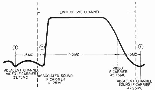
Fig. 13-5. Over-all video-IF response curve, showing location of IF trap frequencies.
