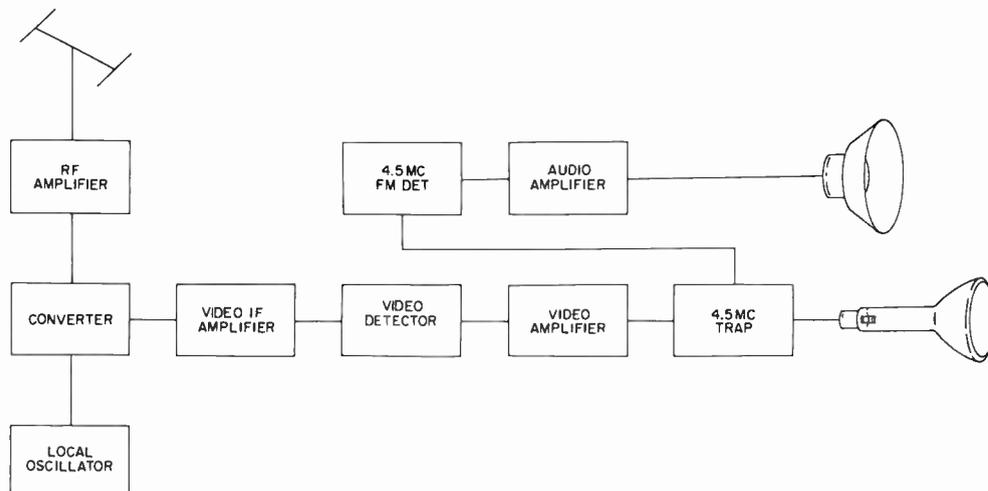
Fig. 13-2. Block diagram of an intercarrier-sound television receiver.
