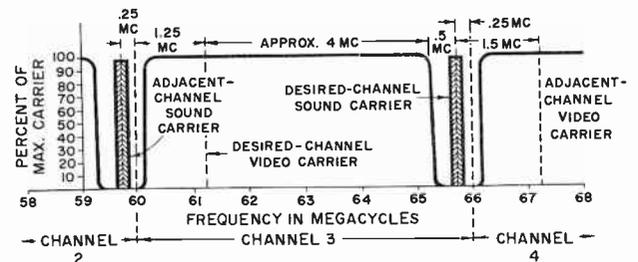
Fig. 9-6. Arrangement of consecutive channel spacing for Channels 2, 3, and 4.
