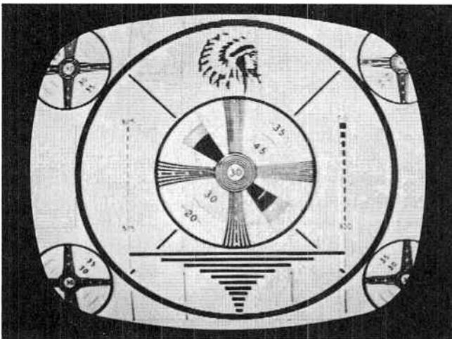
Fig. 17-1. Normal test pattern as it appears on a receiver that is operating normally.
