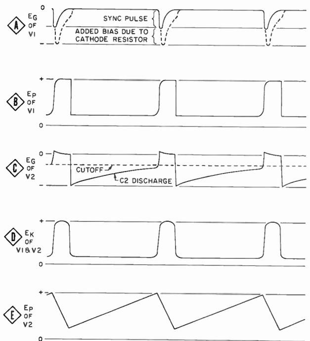
Fig. 6-10. Voltage waveforms in cathode-coupled multivibrator.
