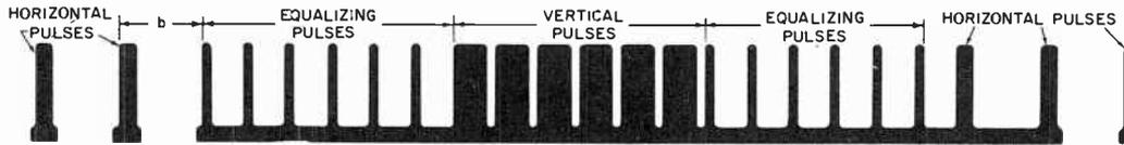
Fig. 10-14D. Vertical-sync signal for retrace after field 2.
