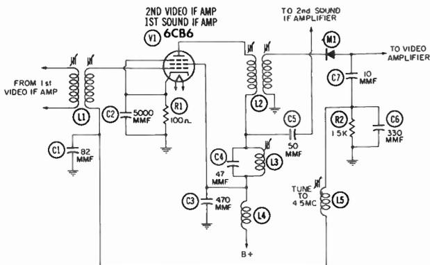
Fig. 13-12. Circuit of the reflex IF amplifier.
