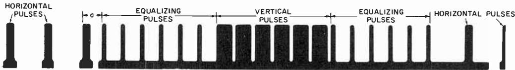
Fig. 10-14C. Vertical-sync signal for retrace after field 1.
