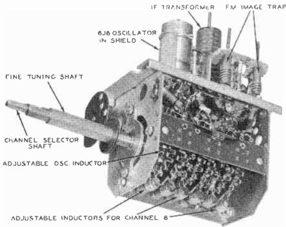
Fig. 12-14. Input tuning system employing lumped equivalents of quarter-wave transmission lines.
