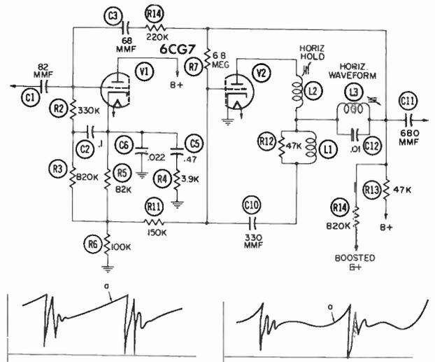
Waveform A — Grid of V2 without stabilizing coil.
