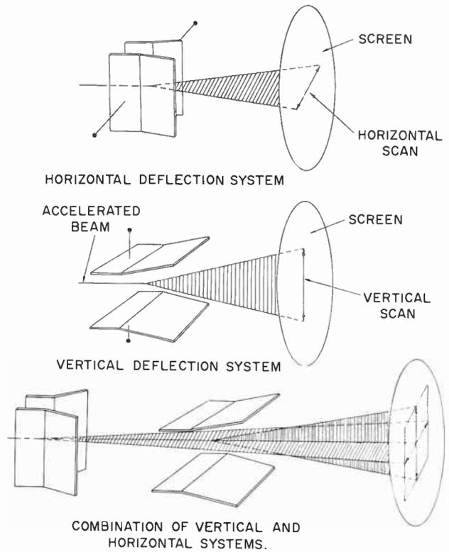
**Fig. 1-9. Electrostatic beam deflection systems.**
