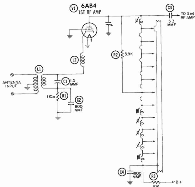
Fig. 12-2. RF amplifier using a grounded-grid triode.
