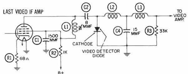
(B) Crystal diode with shunt load.
