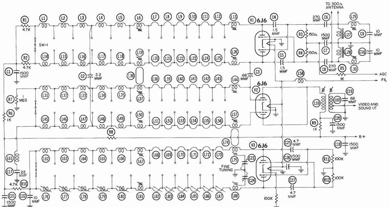
Fig. 12-15. Schematic diagram of tuning system illustrated in Fig. 12-14.
