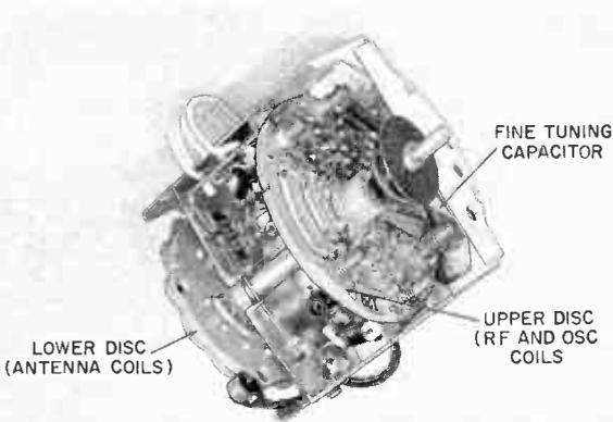
Fig. 12-22. A disc tuner.
