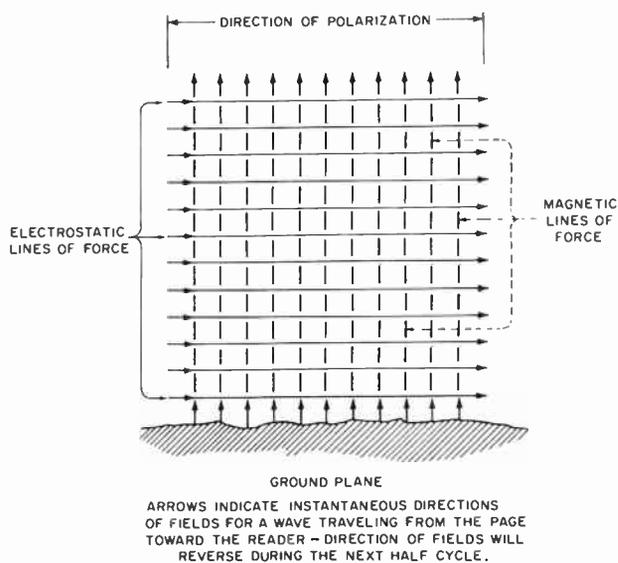
Fig. 11-1. Graphic representation of a horizontally-polarized electromagnetic wavefront.
