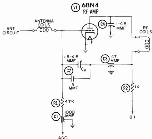
Fig. 12-3. The neutrode RF amplifier circuit.
