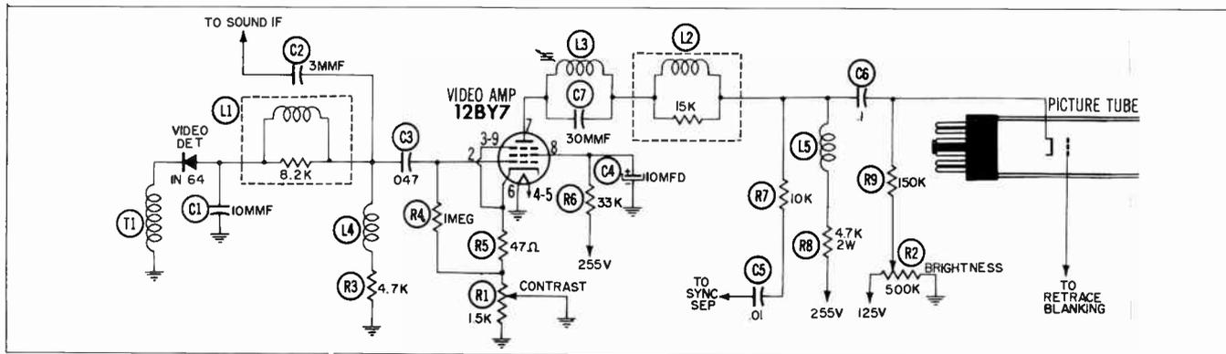
Fig. 15-15. Schematic of a typical single-stage video amplifier employing AC coupling.
