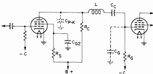
(A) Typical resistance-coupled audio-amplifier stage.
