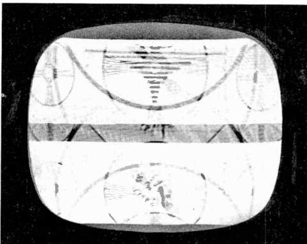
**Fig. 17-10. Vertical-hold control misadjusted.**
