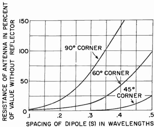
(C) Effect of corner angle and spacing on dipole resistance.
