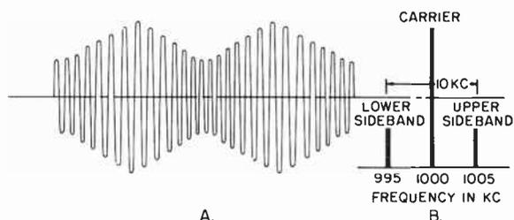
Fig. 9-2. Double-sideband modulated carrier wave; 50 per cent modulation, 5,000-cycle tone.
