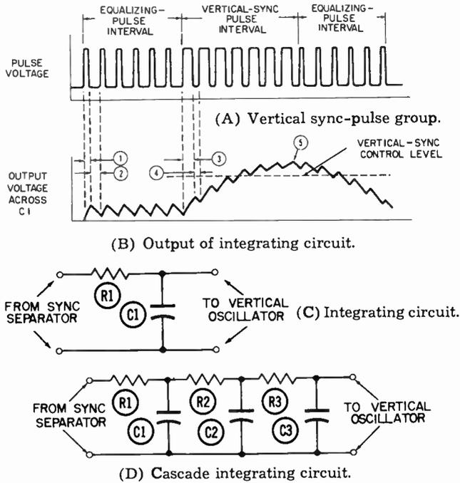
Fig. 10-13. Vertical-pulse separation by integration.
