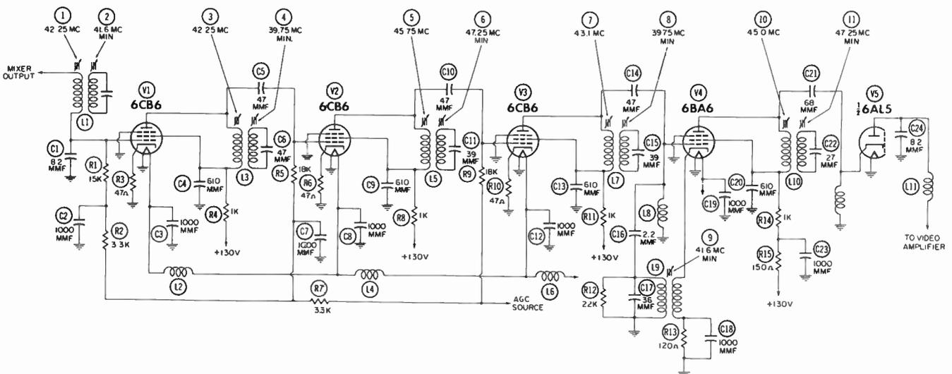
Fig. 13-8. An example of a staggered-tuned video-IF system.
