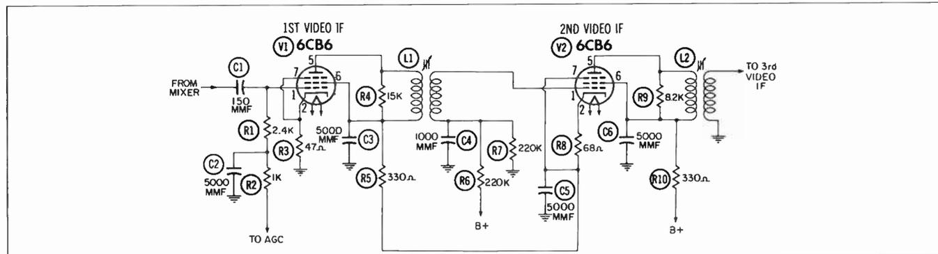
Fig. 13-13. Video-IF amplifier with two tubes in series.
