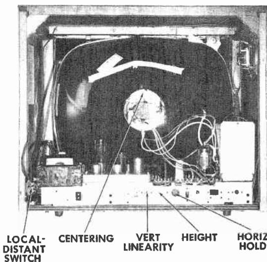
(C) Service controls accessible from rear of chassis. Back cover is removable for servicing picture-tube controls.
