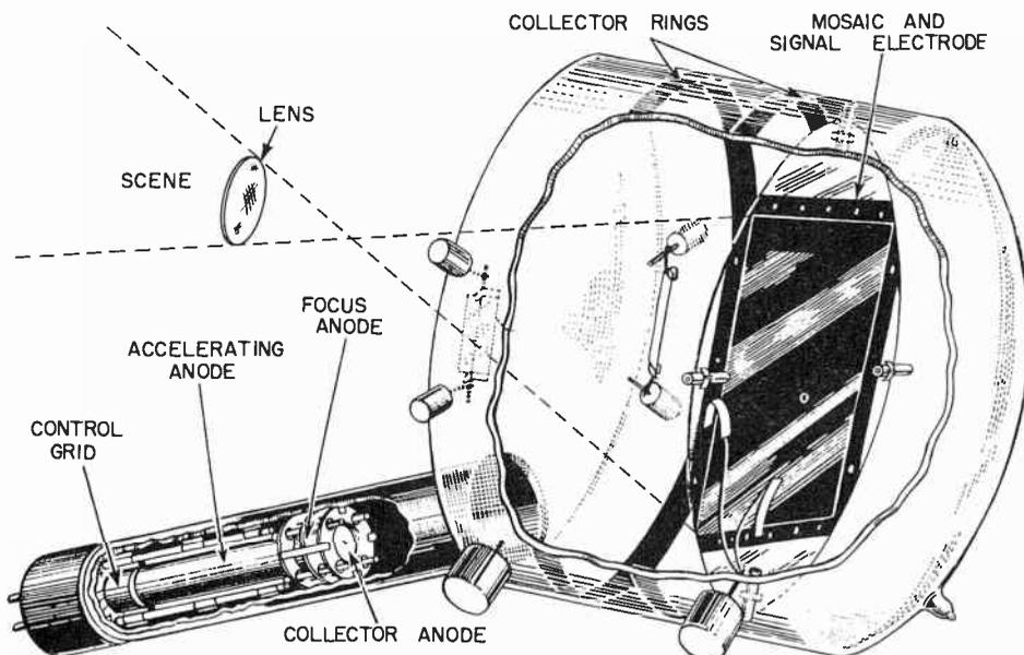
Fig. 3-1. RCA Type 1850-A Iconoscope.
