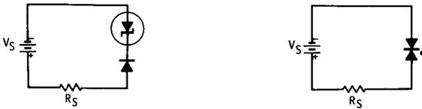
(A) Diodes as individual units. (B) Diodes combined into one package.
