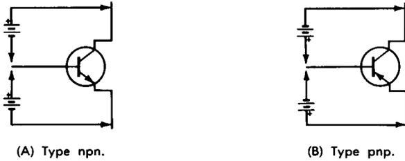
Fig. 2-2. Relative voltages as normally applied to transistors.
