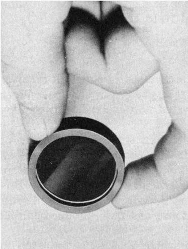
A silicon solar cell for the conversion of radiant energy into electrical energy.
