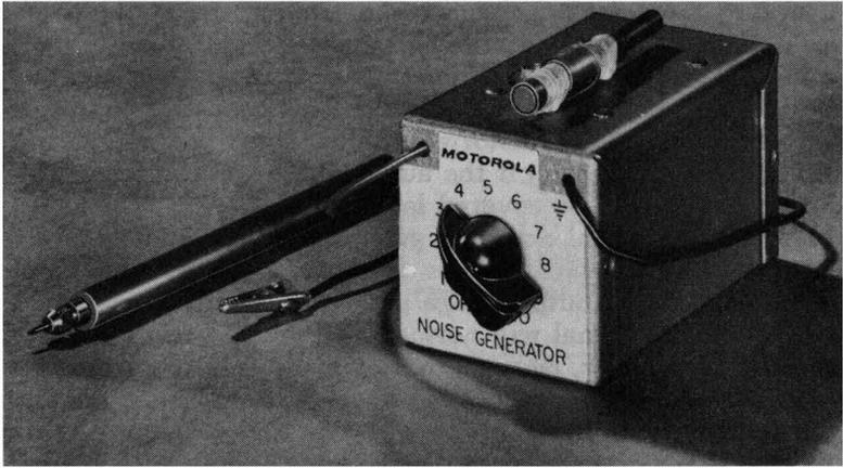
**Fig. 3-14.** A typical noise generator. (Courtesy of Motorola Communications and Electronics, Inc.)
