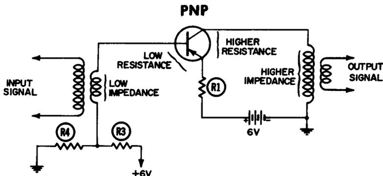
Fig. 2-15. Transformer method of coupling input signal to transistor stage.
