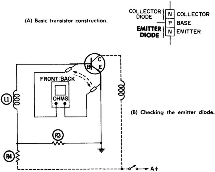
Fig. 7-2. An in-circuit test for an open emitter.
