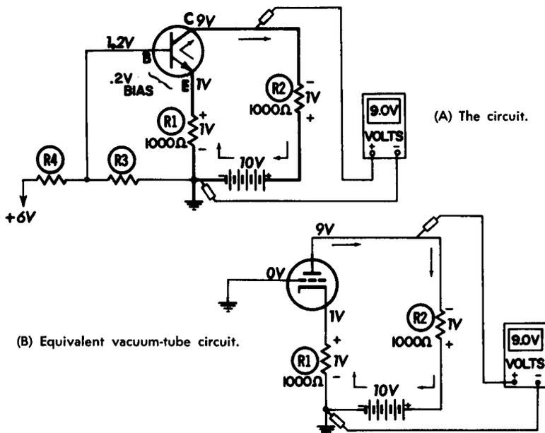
Fig. 5-5. Adding a collector resistor.
