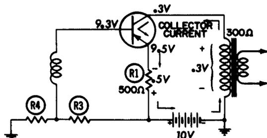
Fig. 5-12. A noticeable voltage drop occurs when there is an audio transformer in the collector circuit.
