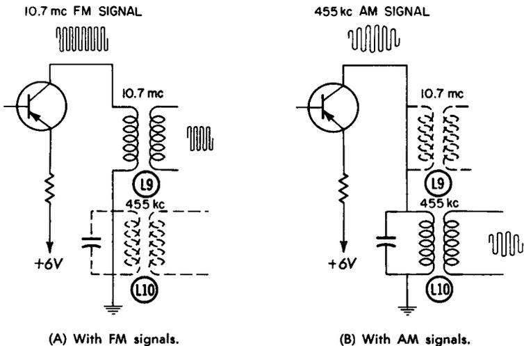
Fig. 4-4. How the IF tuned circuits look to incoming signals.
