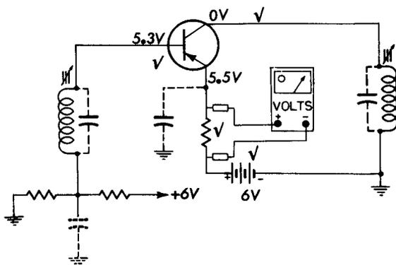
**Fig. 5-16. Normal voltages usually indicate that DC conducting components are OK.**
