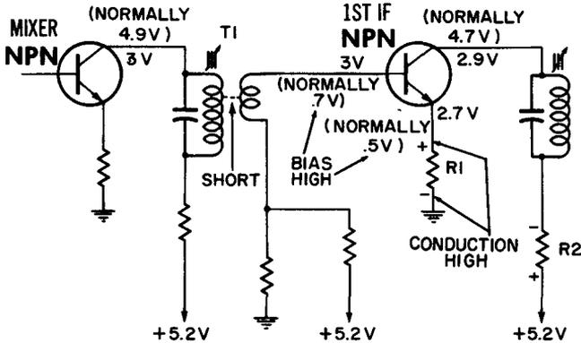
**Fig. 10-3.** Voltages caused by a short between the primary and secondary windings of the 1st IF transformer.
