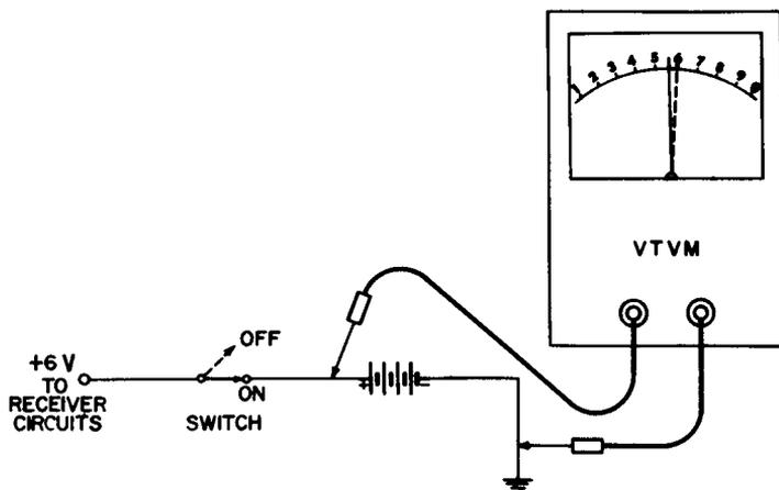
Fig. 3-3. Checking the battery voltage under load and no-load conditions.
