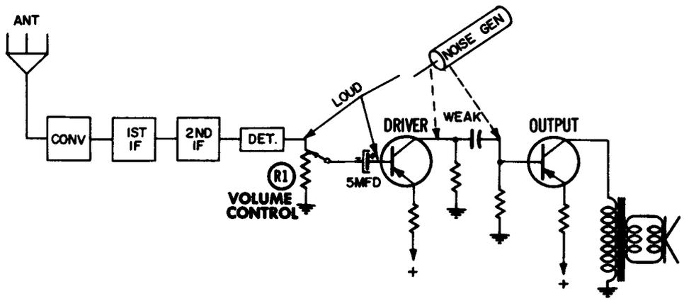
Fig. 3-16. Audio test points.
