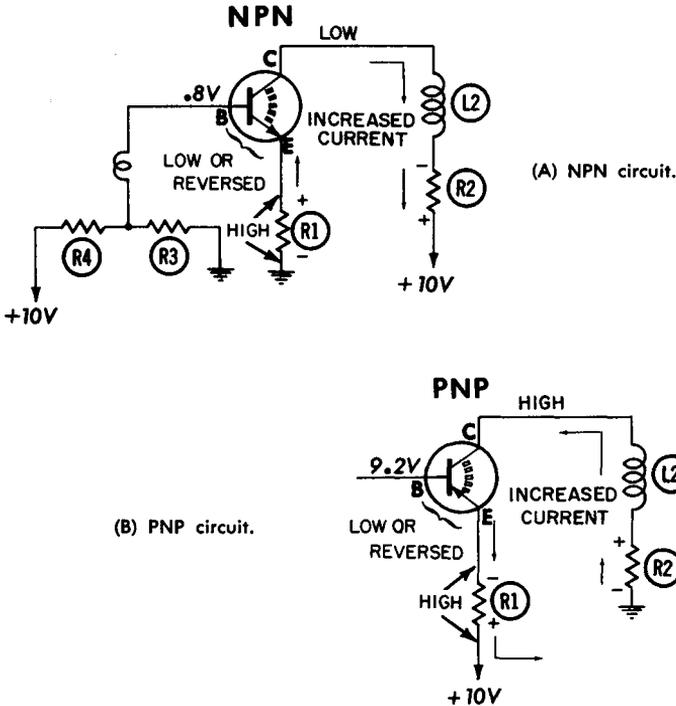
Fig. 6-7. Effect of a leaky transistor on the circuit.
