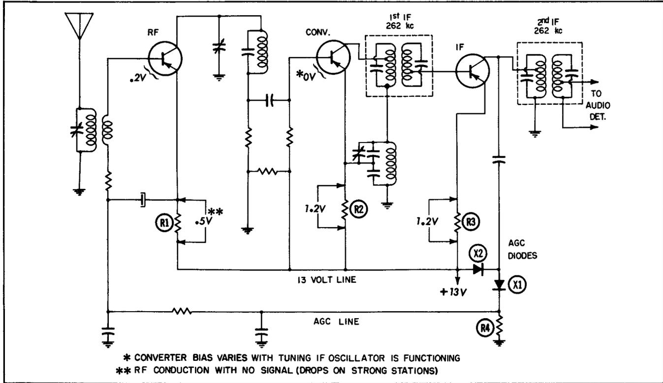
*Conclusion*—The RF transistor was leaky. A word of caution, however. Note that the base circuit of the RF stage is connected to the AGC (automatic gain control) system to control its gain. An open AGC diode can also cause high conduction of the RF transistor. In that case, however, conduction will be high, but bias will be normal or slightly high because AGC diodes X1 and X2 form one leg of the voltage divider for the RF base circuit (R4 completes the divider circuit).
