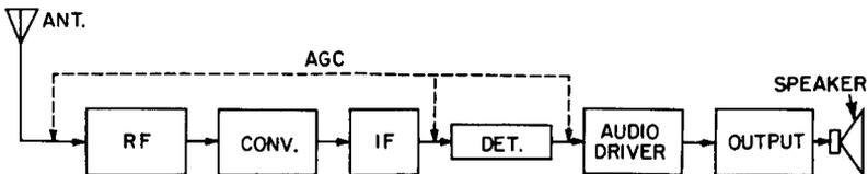
Fig. 8-2. Block diagram of the receiver in Fig. 8-1.
