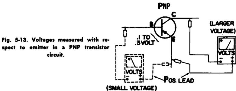
Fig. 5-13. Voltages measured with respect to emitter in a PNP transistor circuit.
