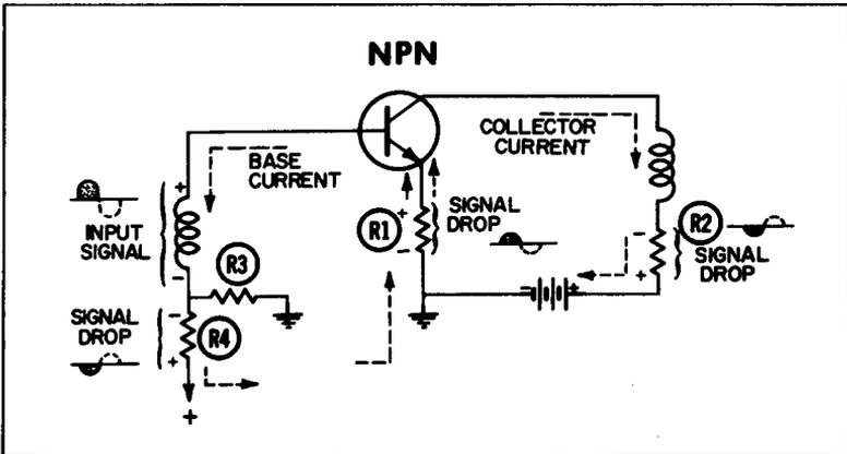
Fig. 2-16. Points where degeneration occur in the basic NPN transistor circuit.
