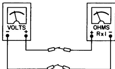
**Fig. 7-5. Checking the ohmmeter lead polarity.**
