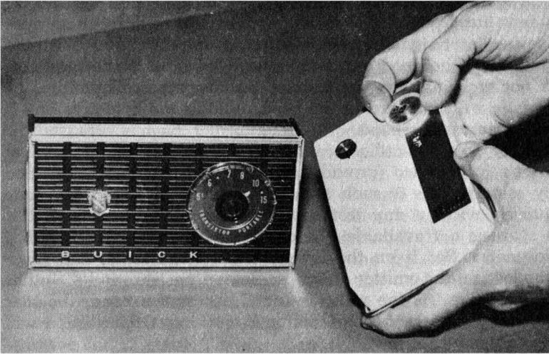
Fig. 3-18. A quick method of determining if the oscillator is operating.
