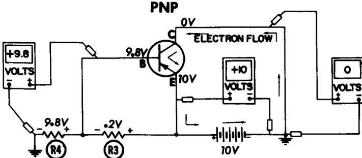
Fig. 5-10. The basic PNP transistor circuit.
