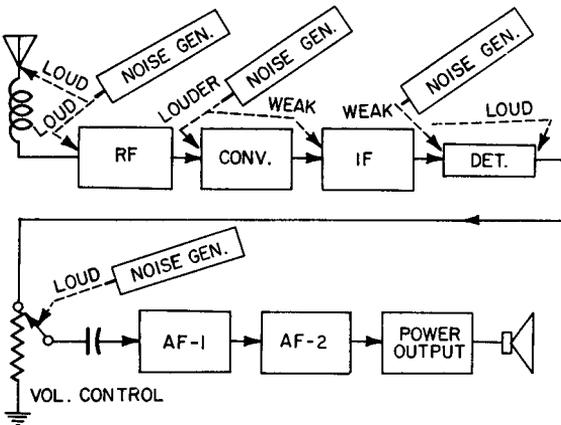
Fig. 8-13. Noise generator checks.
