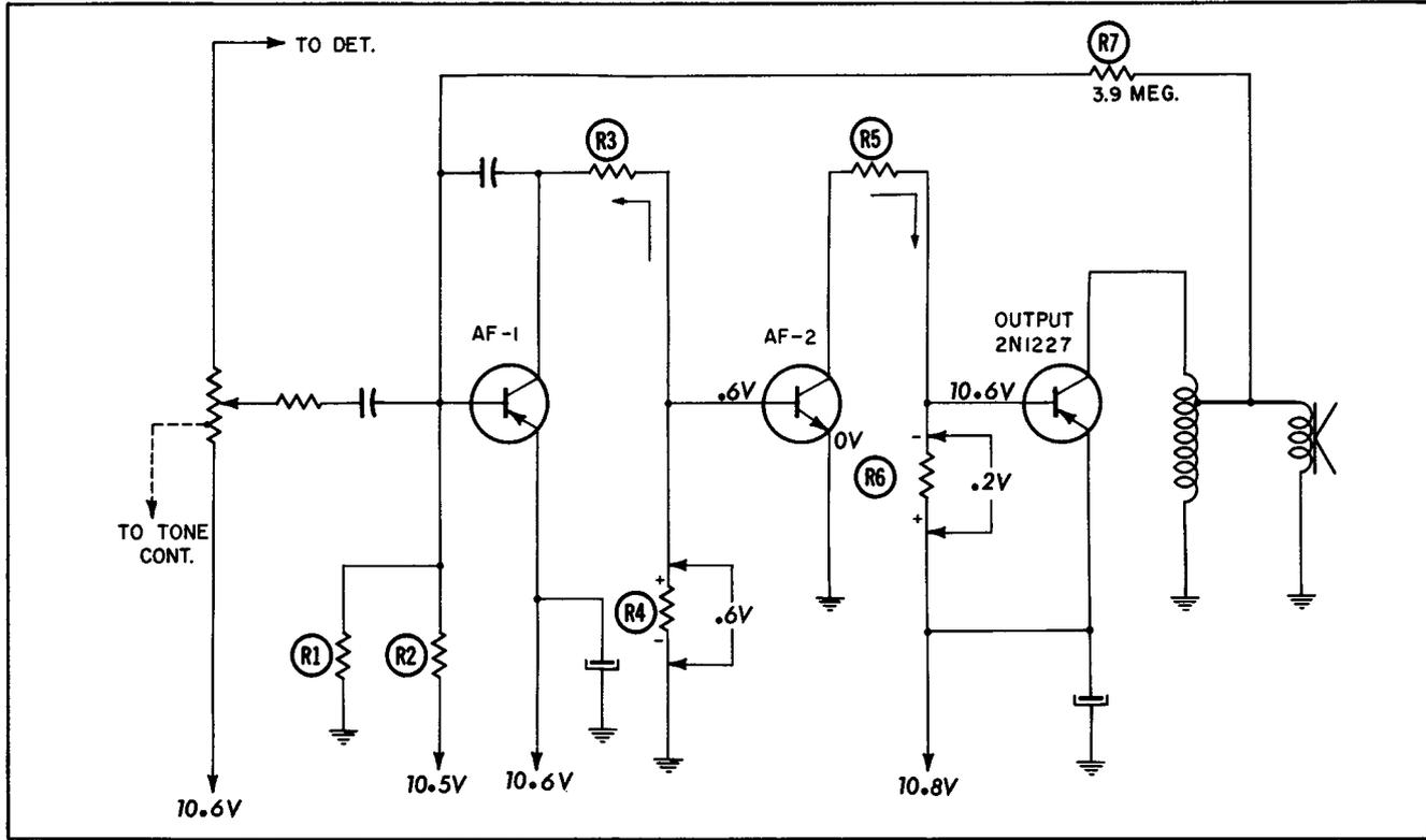
system and power supply with a good capacitor of the same value. If this doesn't locate the defective part and AF-1 is a PNP transistor, replace AF-2 (NPN unit).
