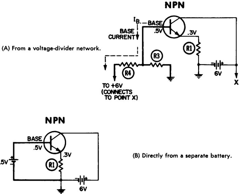
Fig. 2-11. Obtaining the bias voltage for an NPN transistor circuit.
