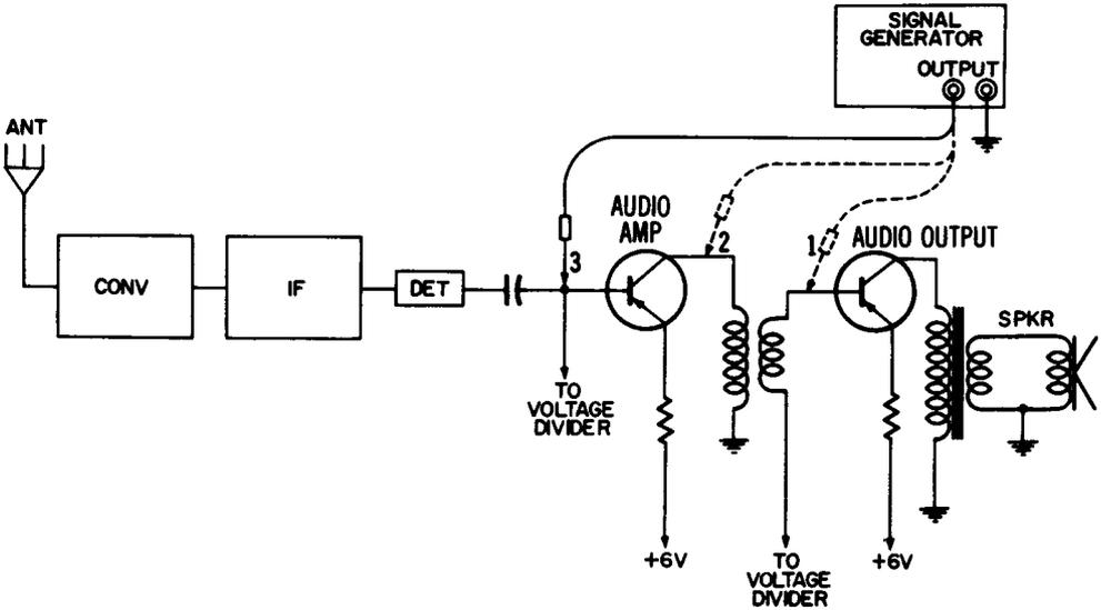
Fig. 3-7. Method of injecting a signal into the audio stages.
