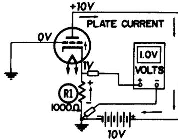
Fig. 5-4. Adding an emitter resistor.
