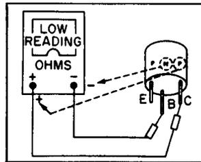
Fig. 7-8. Method of determining the transistor type.
