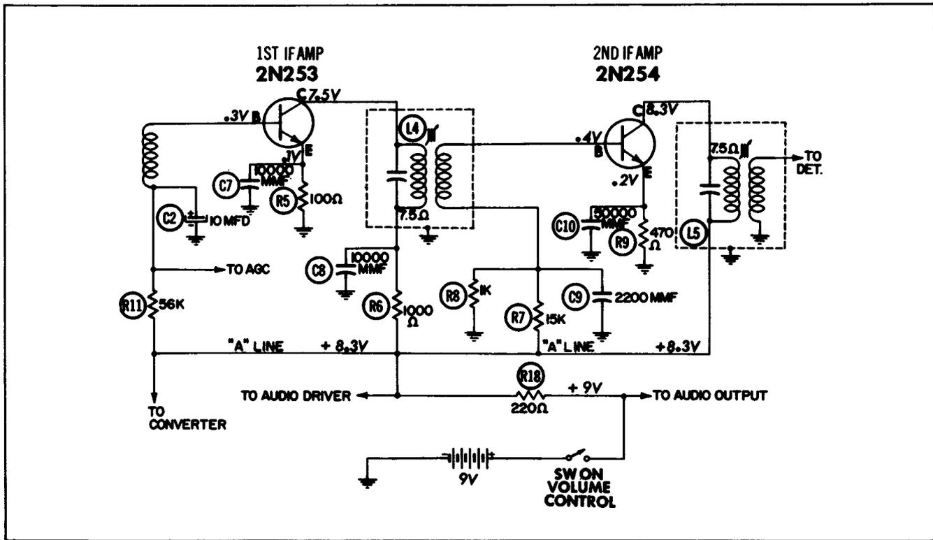
The 1st and 2nd IF stages of a typical transistor portable using NPN transistors is shown in Fig. 5-9. A 9-volt battery with negative ground is used. The full battery voltage is applied to the audio-output stage, but the voltage to the other stages is dropped to 8.3 volts by a 220-ohm resistor, R18 in the "A" line.
