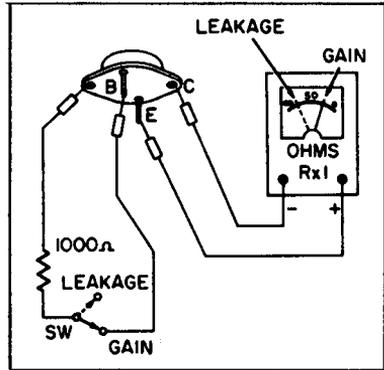
Fig. 7-7. Testing the gain of an audio transistor.
