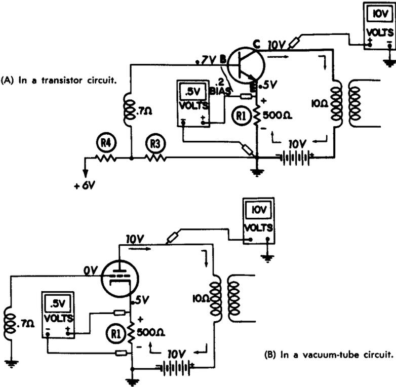
Fig. 5-6. Replacing R2 with a transformer.
