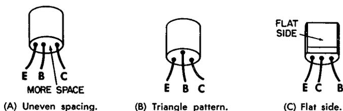
Fig. 3-11. Three methods of identifying transistor leads.
