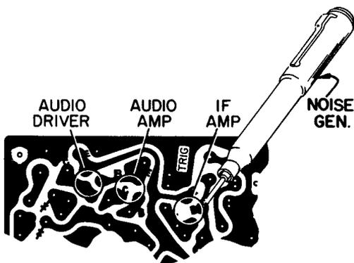
Fig. 8-14. Touching noise generator to printed board.
