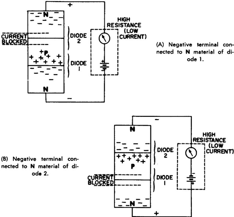
(A) Negative terminal connected to N material of diode 1.
