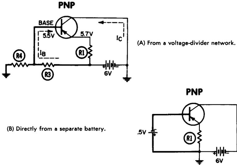
Fig. 2-13. Obtaining the bias voltage for a PNP transistor circuit.
