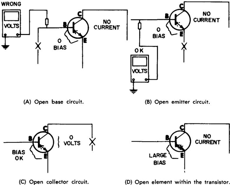
Fig. 6-6. Results of open conditions in a transistor circuit.
