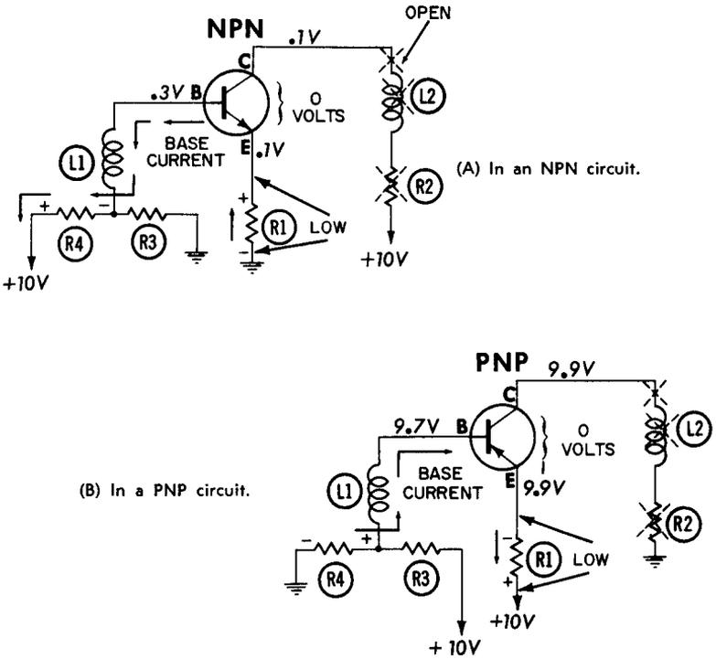
Fig. 6-4. Open collector circuit.
