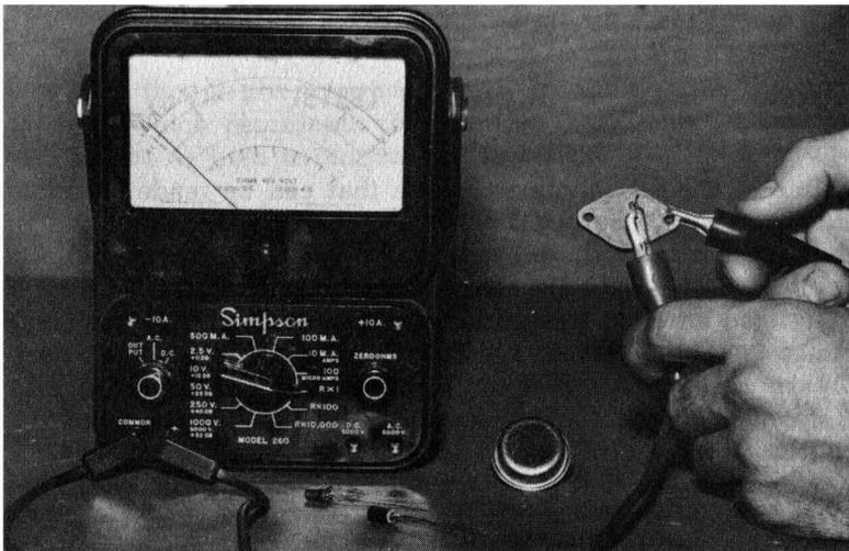
Fig. 7-1. Checking a transistor with an ohmmeter.
