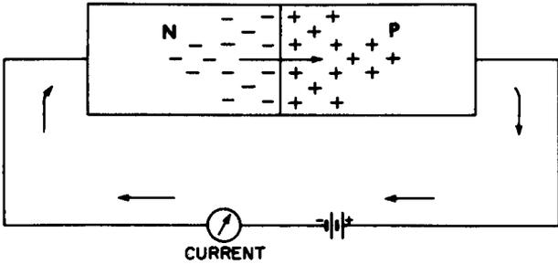
Fig. 1-3. Current will flow through the diode when a battery is connected in the proper direction.
