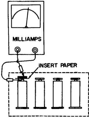
(C) With cells connected in series.
