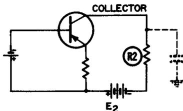
Fig. 2-7. A resistor in the collector lead will provide even better collector-current stability.
