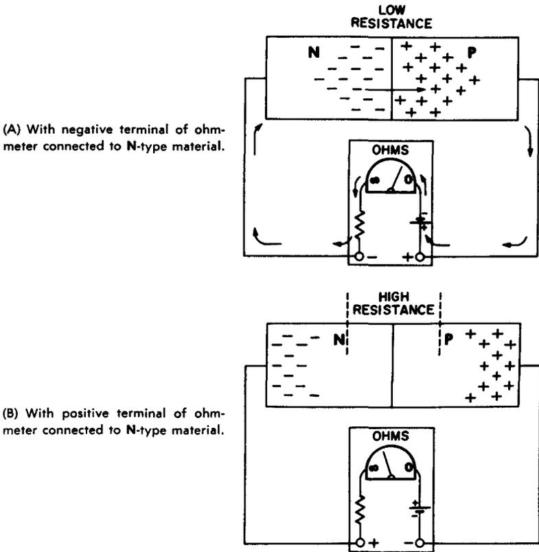
(A) With negative terminal of ohmmeter connected to N-type material.
