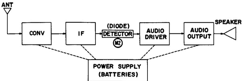
Fig. 3-2. Block diagram of the receiver in Fig. 3-1.
