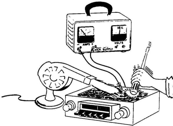
Fig. 8-7. Tapping the chassis, applying heat from hair dryer, and increasing input voltage to help locate intermittents.
