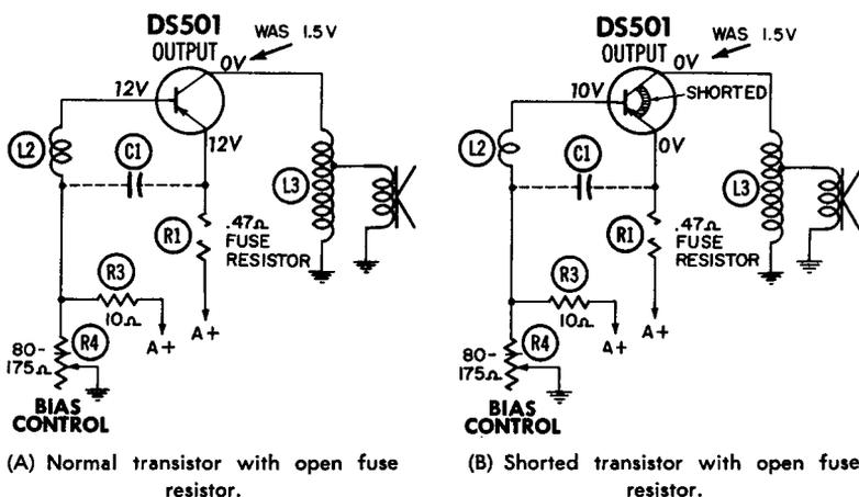
Fig. 8-9. The most frequent output stage troubles.
