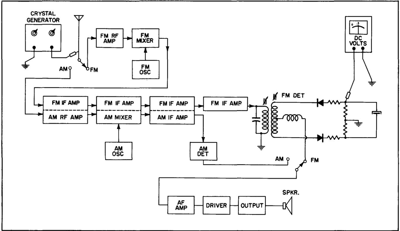
*Solution*—change one of the generator crystals to 9 mc. and use its harmonics (90 mc, 99 mc, 108 mc) for tuner alignment. A generator with two crystals (9 mc for tuner alignment and 10.7 mc for IF alignment) makes an excellent instrument.
