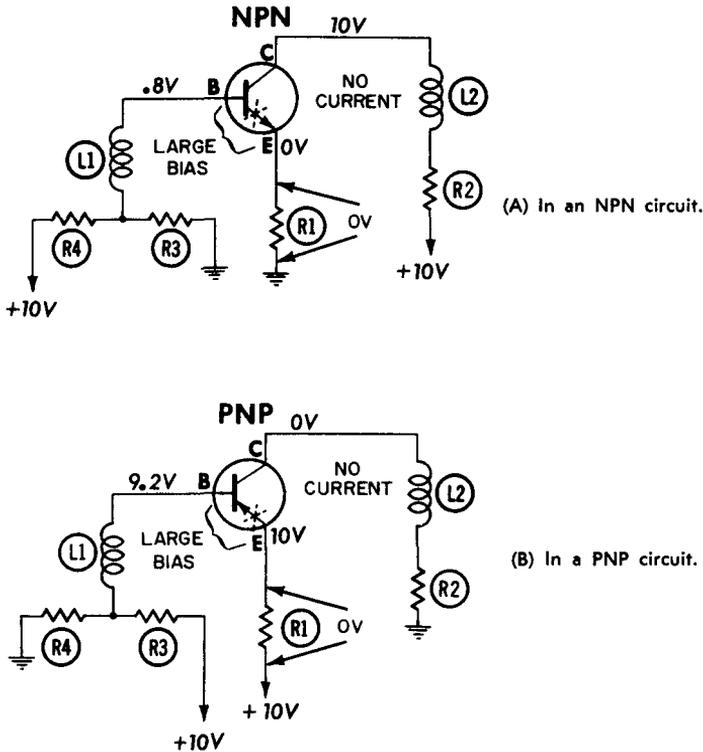
Fig. 6-5. Open emitter lead within the transistor.
