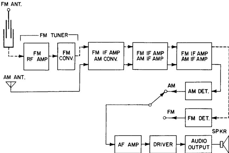
Fig. 4-2. Block diagram of the AM-FM receiver in Fig. 4-1.
