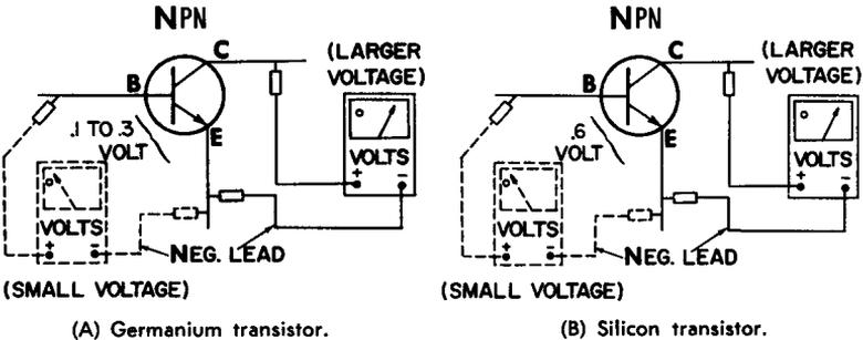
Fig. 5-7. Typical element-to-element voltage relationship in a basic transistor amplifier circuit.
