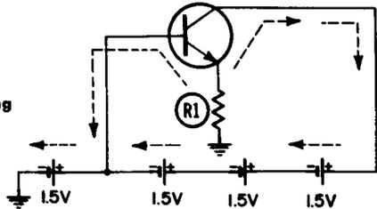
transistor will need exactly that voltage on the base. Besides, other transistors in the radio will also need some form of bias, each of a different voltage. But even if all base leads could be tied into that point, there is still a disadvantage: One battery would have more current passing through it than the others.
