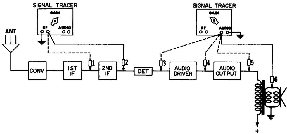
Fig. 3-22. Test-point sequence used in signal tracing.
