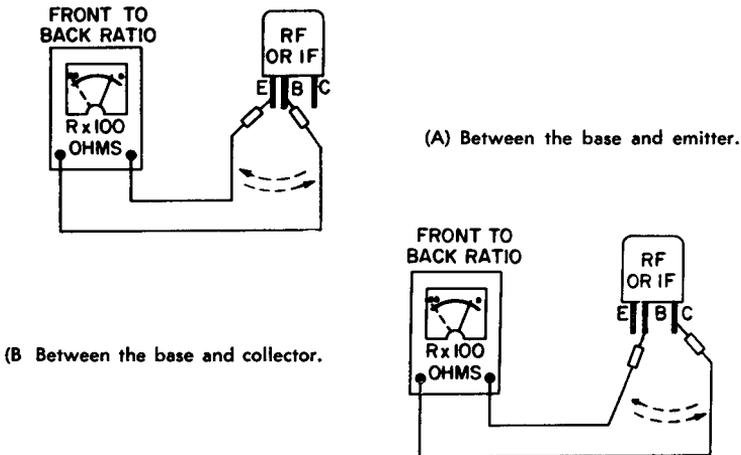
Fig. 7-4. Checking the front-to-back resistance ratio of a transistor.
