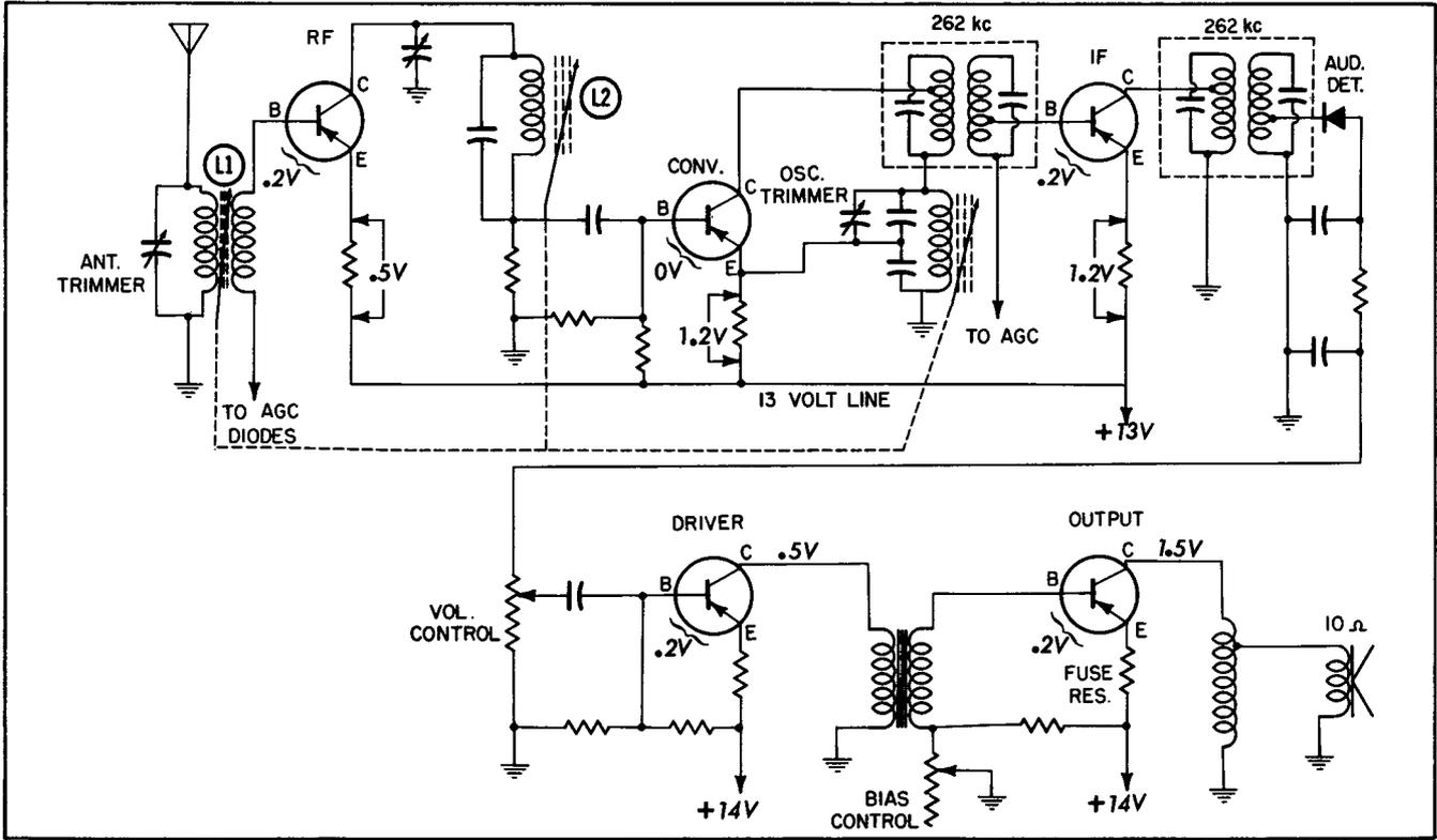
What do you notice about this schematic? First of all, it is *very* similar to the first transistor radio schematic studied (see Chapter 3). One additional stage—the RF stage—has been added, but otherwise, the auto radio contains the same number and type of stages.
