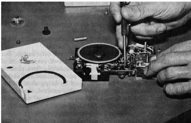
**Fig. 3-17.** Using the body resistance to protect the transistor when a "click test" is made.
