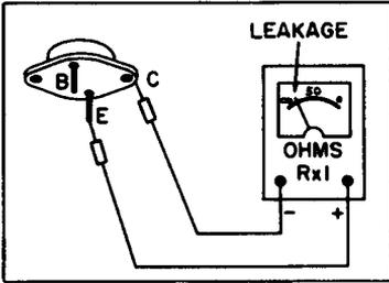
(A) The leakage test.
