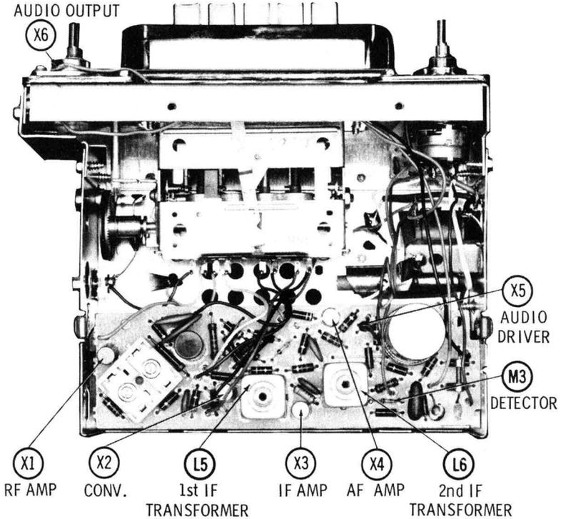
**Fig. 8-5. Top view of a typical auto radio.**
