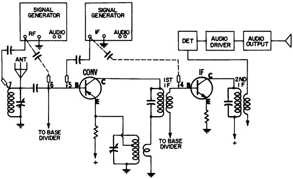
Fig. 3-8. Injecting a test signal into the RF and IF sections of a transistor receiver.
