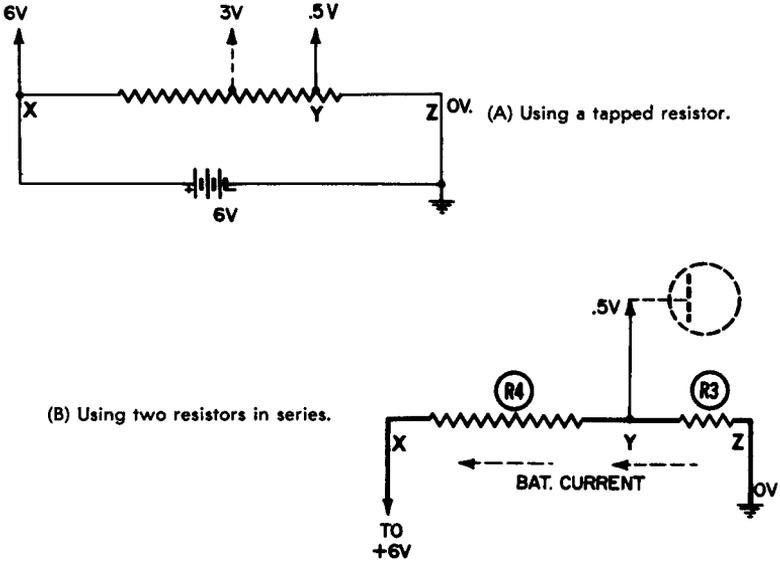
Fig. 2-10. Obtaining bias voltage from a divider network.
