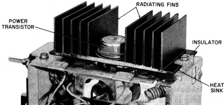
Fig. 2-8. Typical power transistor and heat sink used in an auto radio.
