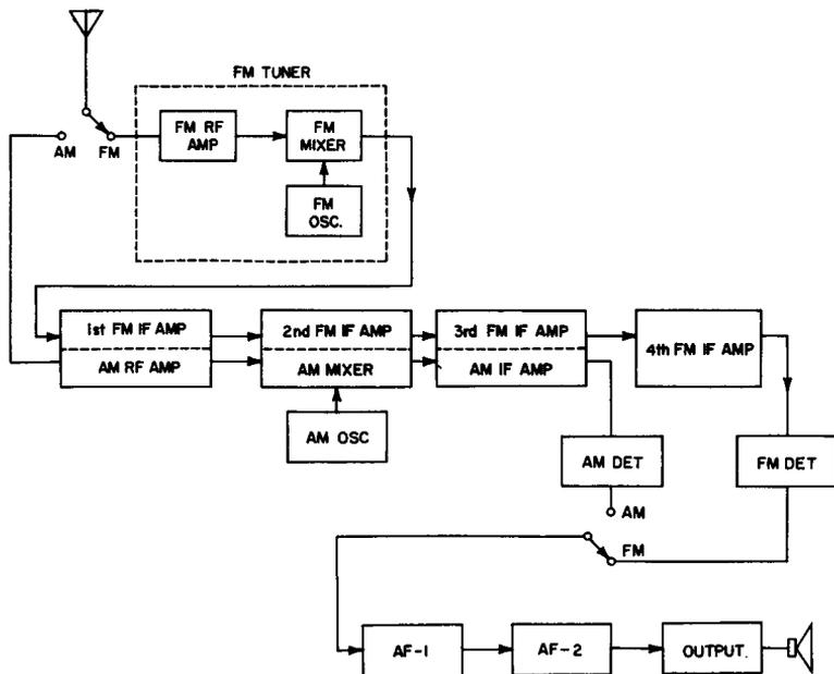
Fig. 9-4. Block diagram of a typical AM-FM auto radio.
