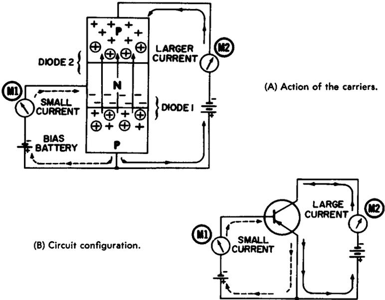
Fig. 1-10. Forward biasing the PNP transistor.
