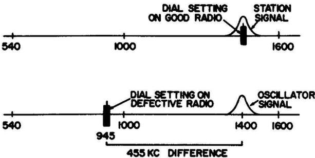
Fig. 3-19. Beat will occur at approximate position of dial pointers if the suspected oscillator is operating.
