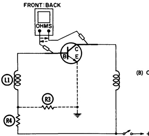
(B) Checking the collector diode.
