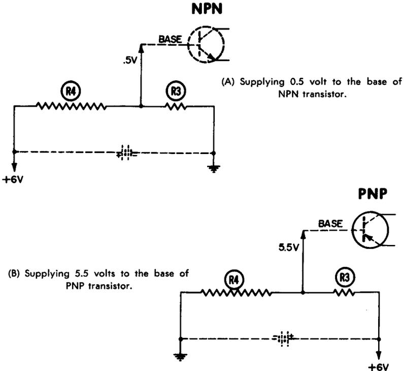
Fig. 2-12. Reportioning the voltage division across the divider network by reversing the battery connections.
