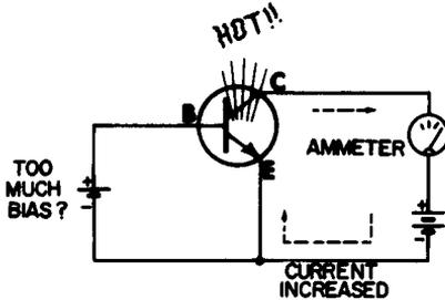
Fig. 2-2. Excessive collector current can ruin a transistor.
