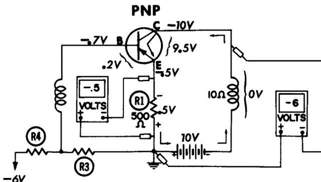
Fig. 5-14. A typical positive-ground PNP circuit.
