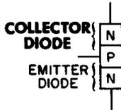
(A) Basic transistor construction.
