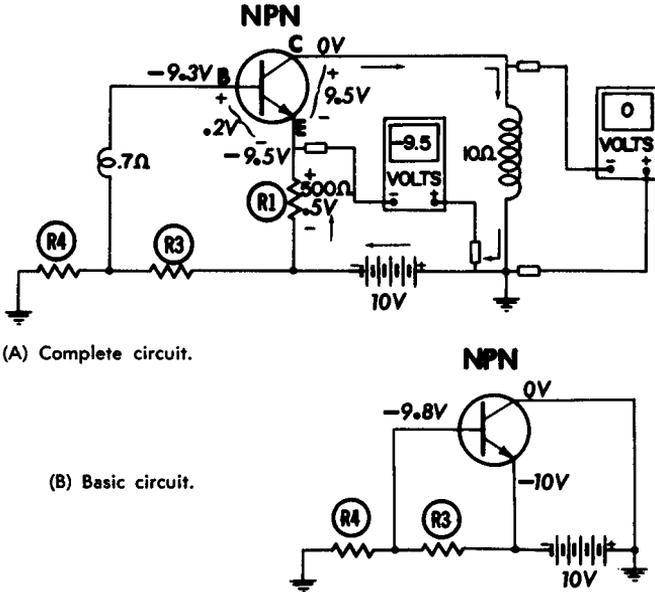
Fig. 5-8. A positive-ground NPN circuit.
