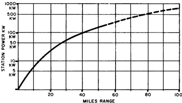
Fig. 9-1. Range versus FM station power for average condition in flat terrain.
