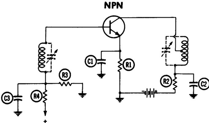
Fig. 2-17. Using bypass capacitors to prevent degeneration.
