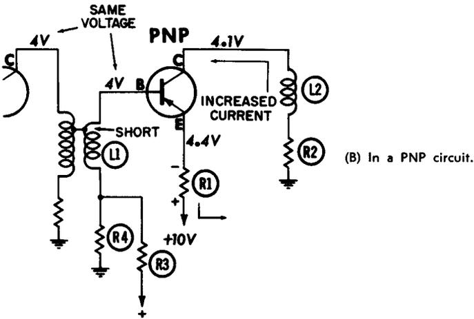
Fig. 6-8. Results of a short between the primary and secondary winding of a coupling transformer.
