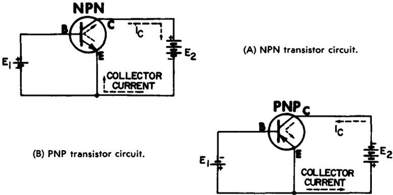
Fig. 2-1. The basic transistor circuits.
