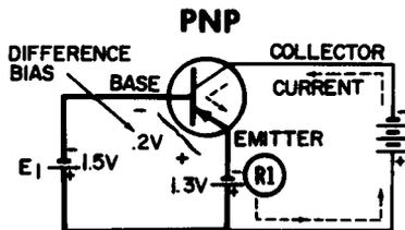
Fig. 2-6. Equivalent circuit of Fig. 2-5.
