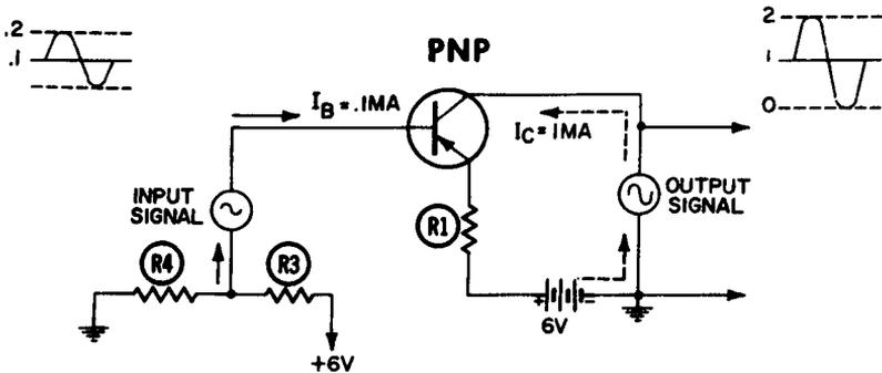
Fig. 2-14. How amplification is accomplished in a transistor circuit.
