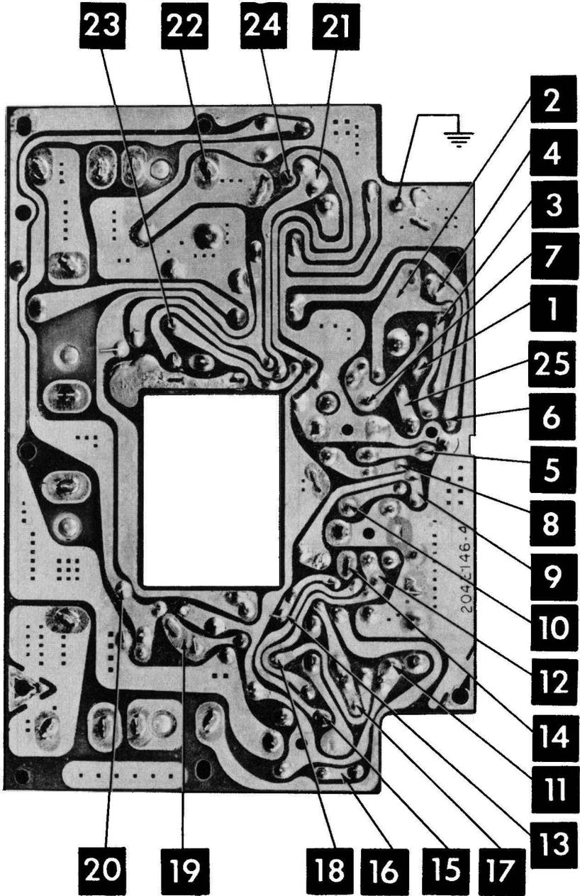
Fig. 3-13. Circuit board of receiver in Fig. 3-12, showing check points.
