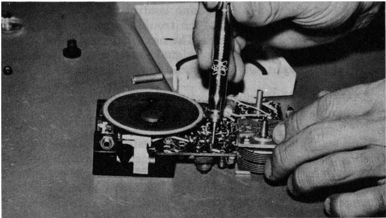
**Fig. 3-15.** The "Mosquito" noise generator in use.
