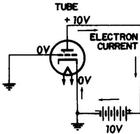
(B) Equivalent vacuum-tube circuit.
