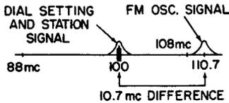
Fig. 4-3. The oscillator oscillates 10.7 mc above the incoming station frequency.
