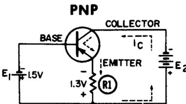
Fig. 2-5. Current flow through a basic PNP transistor circuit.
