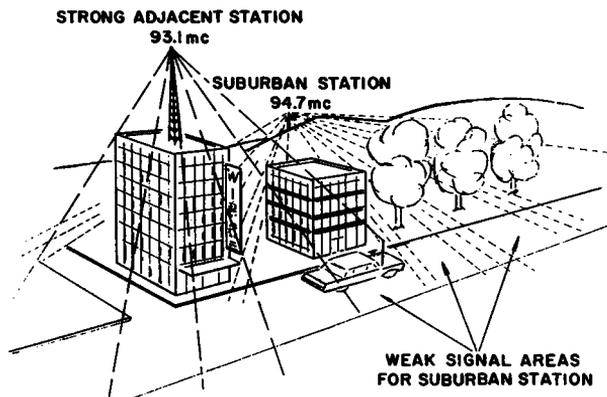
Fig. 9-2. How low antenna height, buildings, etc. limit FM range.
