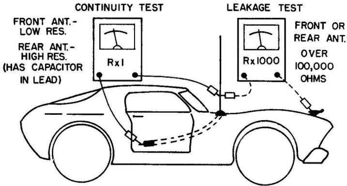
Fig. 8-3. Ohmmeter tests for an auto radio antenna.
