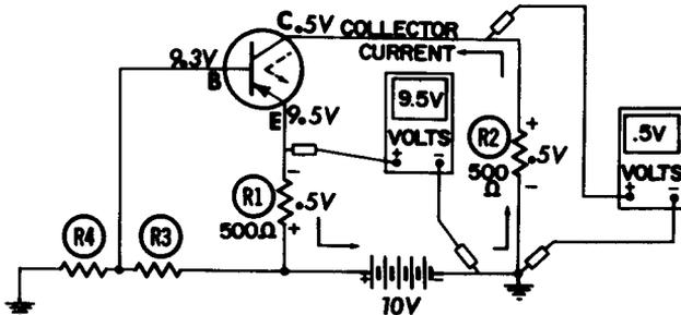
Fig. 5-11. Voltage distribution in the PNP transistor circuit.
