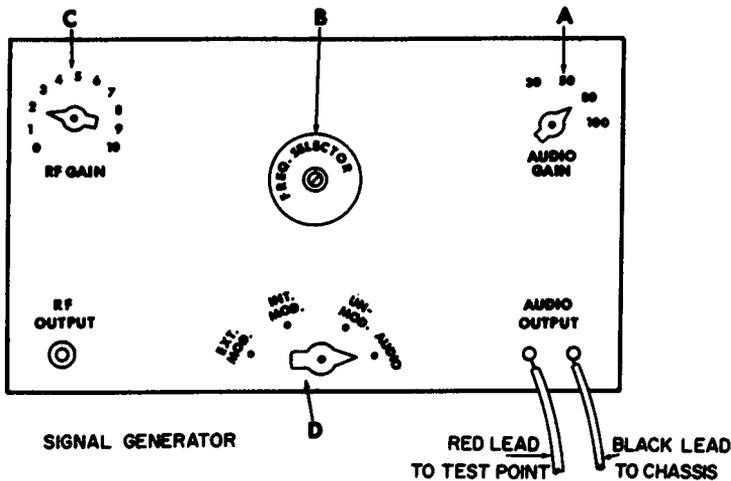
Fig. 3-9. Typical settings of the signal-generator control when the audio section is being tested.
