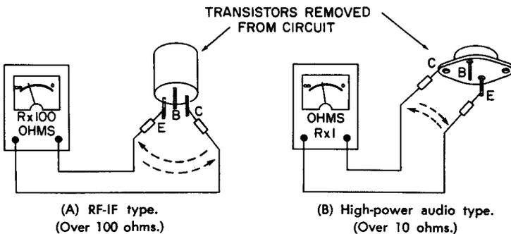
Fig. 7-6. Testing a transistor for leakage.
