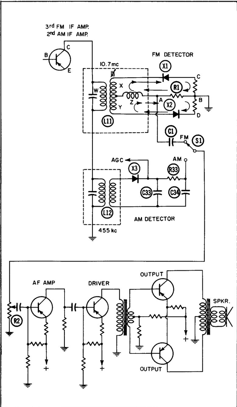
Fig. 4-5. Simplified schematic of detector and audio stages.
