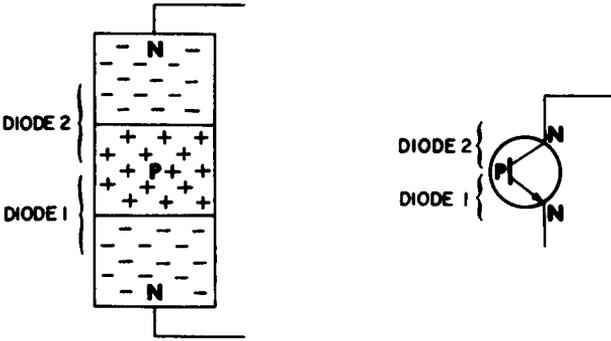
(A) Equivalent diode structure.
