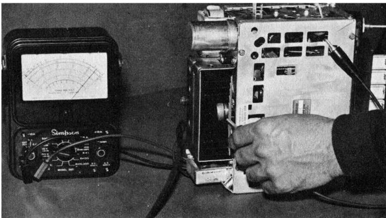
Fig. 8-8. Checking speaker and output transformer (and connections) by tapping ohmmeter ( $R \times 1$  range) on case of output transistor.
