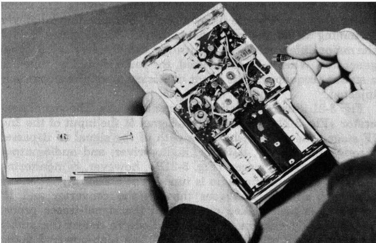
Fig. 3-20. Performing the click test by removing and replacing a transistor in its socket.
