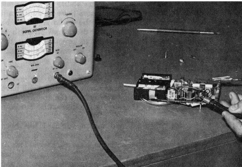
**Fig. 3-6.** Injecting a signal into the audio stages of a transistor radio.
