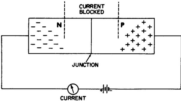
Fig. 1-4. Reversing the battery connections blocks the current through the diode.
