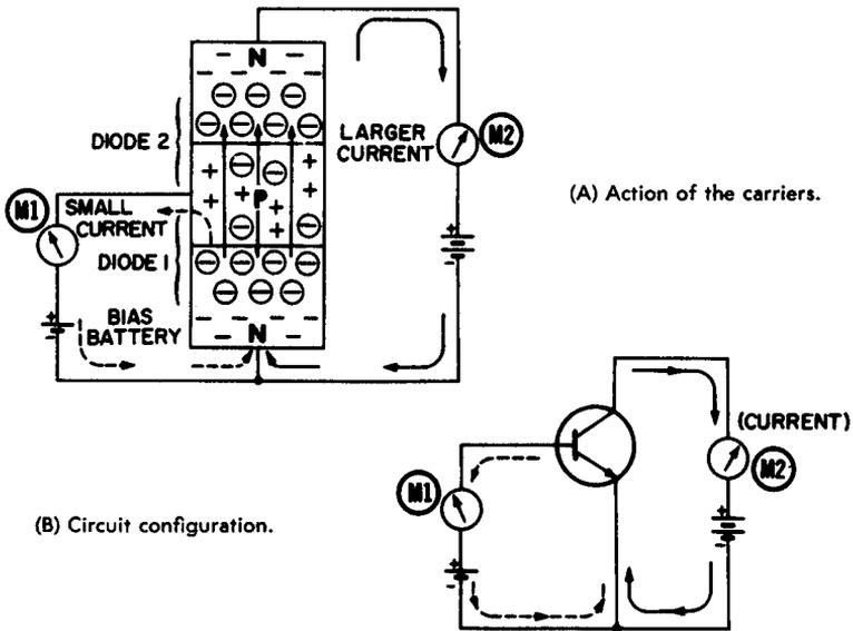
Fig. 1-8. Forward biasing the NPN transistor.
