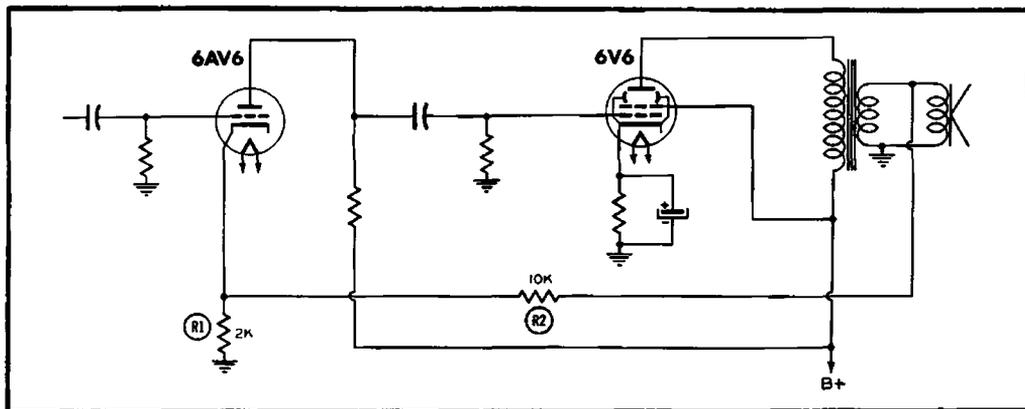
Fig. 8-3. Typical audio-output circuit employing negative feedback.
