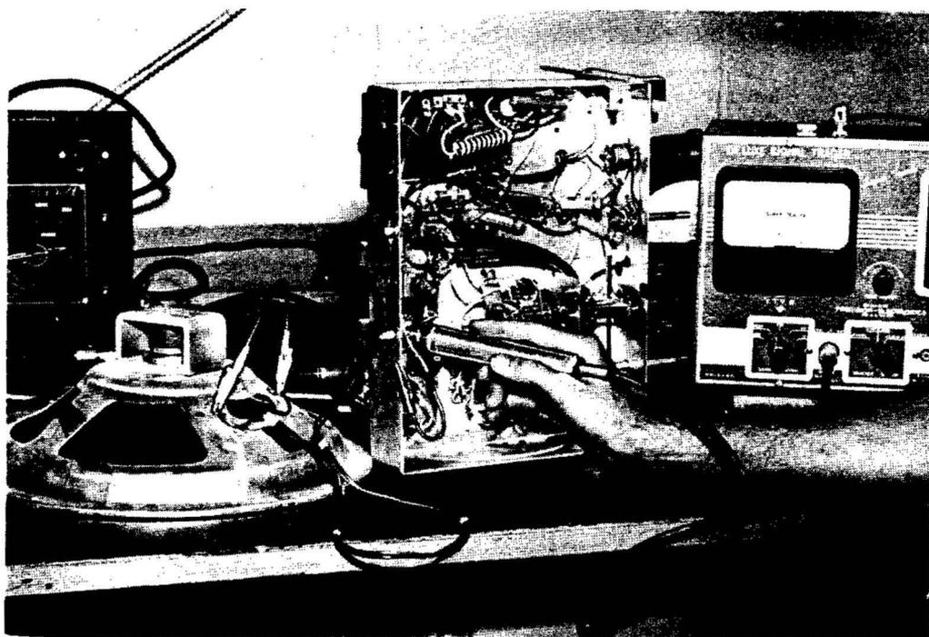
Fig. 6-3. Signal tracer in use.
