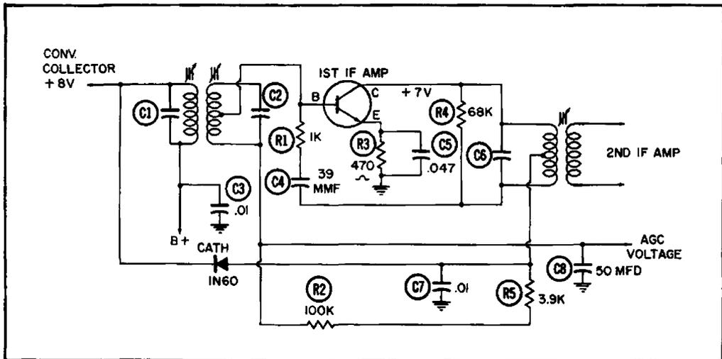
Fig. 14-6. AGC system using diode to improve action.
