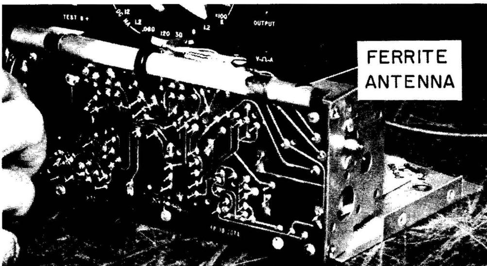
Fig. 7-7. Typical ferrite antenna.
