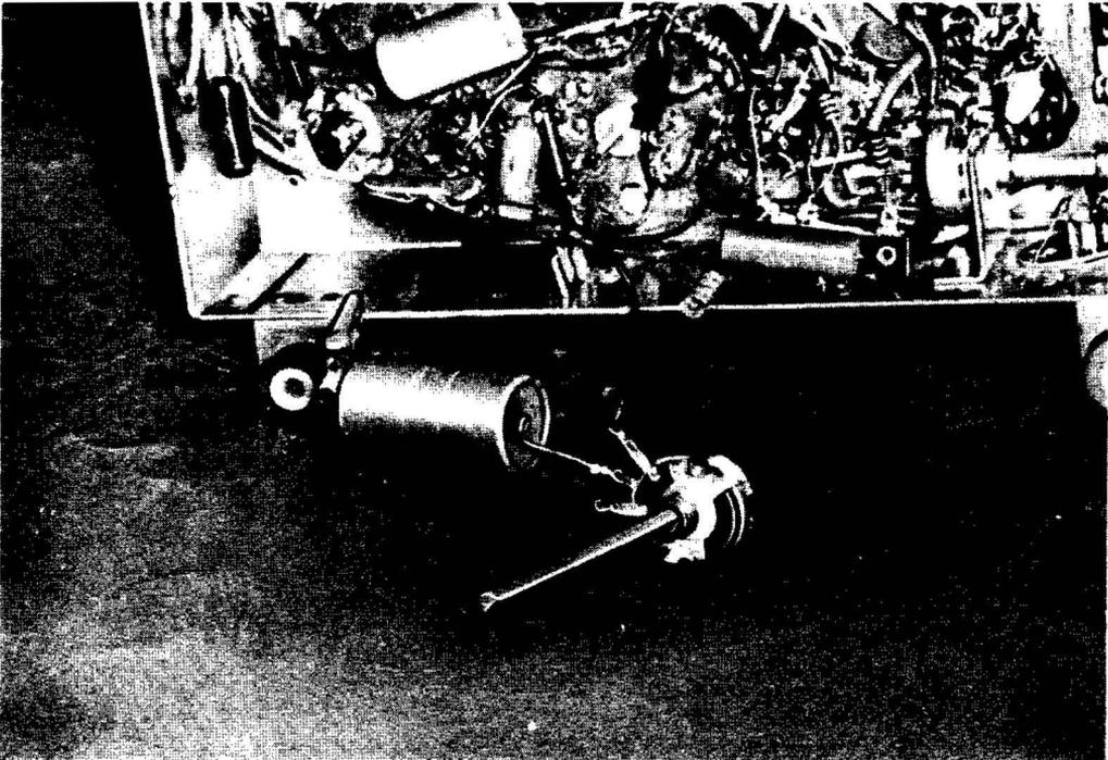
**Fig. 9-3. Variable resistor and capacitor to ease a bridging capacitor into a circuit.**
