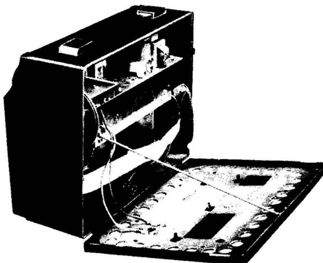
**Fig. 6-5. Portable receiver with loop antenna mounted in a hinged cover.**
