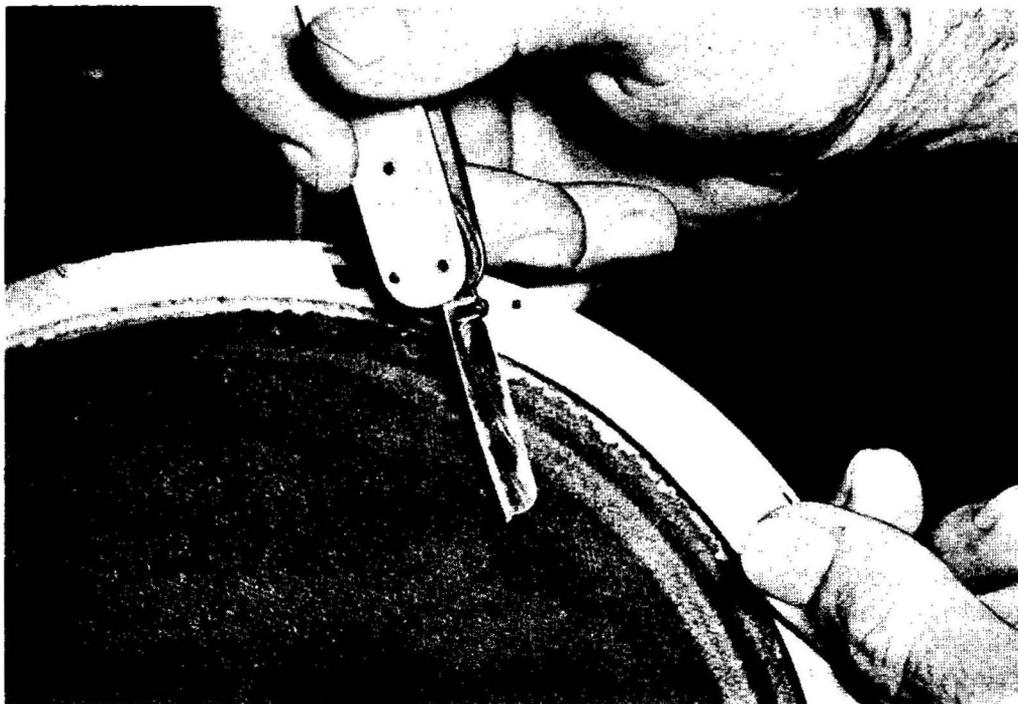
**Fig. 10-3. Repairing a break in the speaker cone.**
