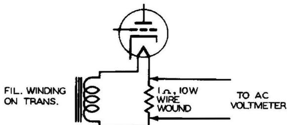
**Fig. 13-1. Measuring filament current by use of voltage drop.**
