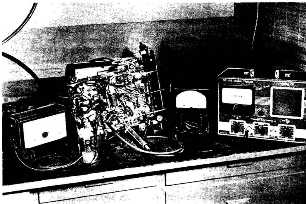
**Fig. 12-2. Test equipment connected to an intermittent chassis.**
