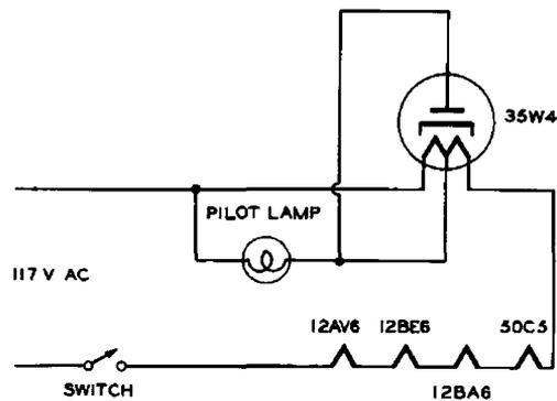
Fig. 1-3. Filament circuit of an AC-DC receiver.
