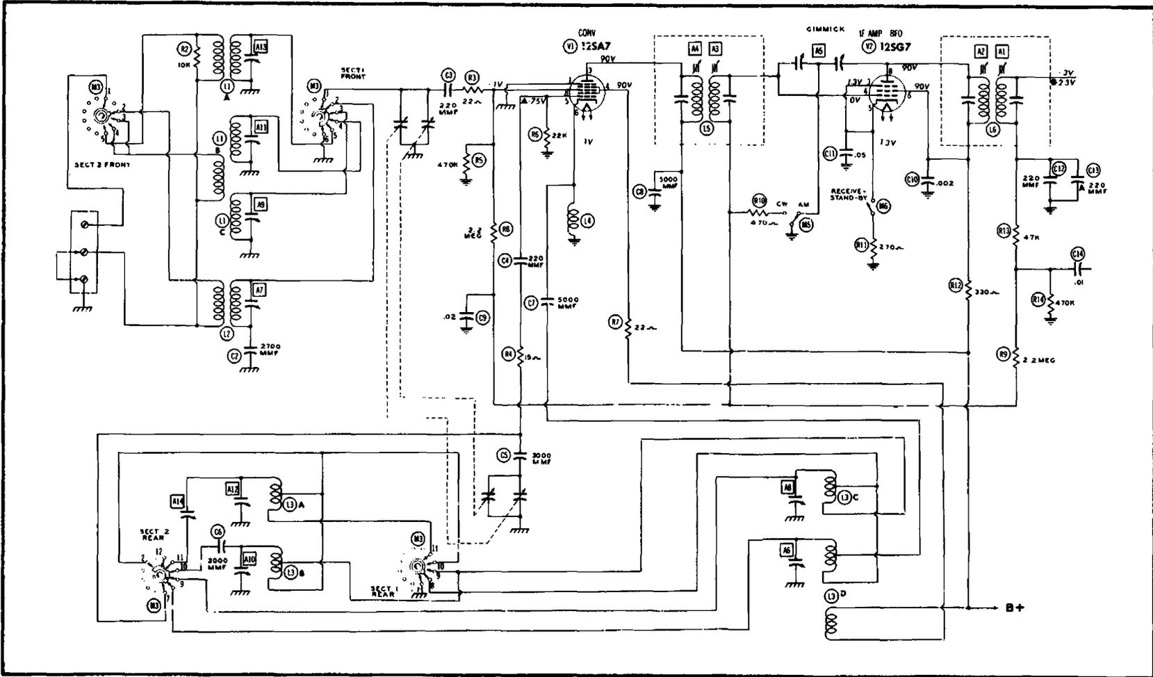
Fig. 16-3. Partial diagram of the RF and IF circuits of the receiver shown in Fig. 16-2.
