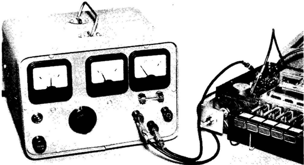
**Fig. 14-2. Using an auto-radio battery substitute that has the extra filtering required for hybrid and transistor receivers. (Courtesy of Electro Products Laboratories.)**
