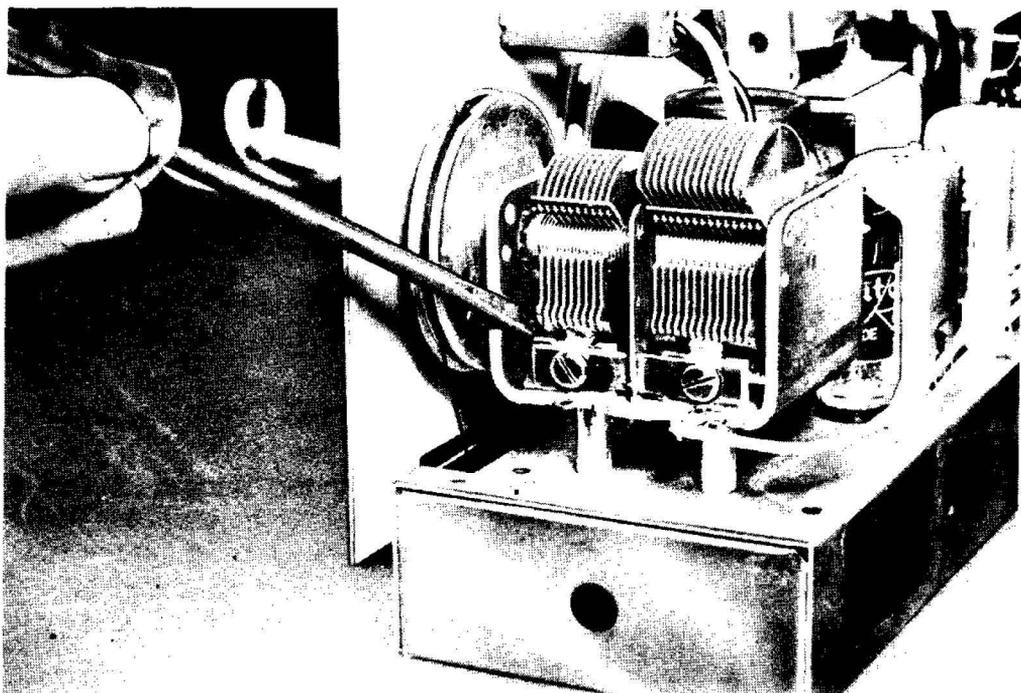
**Fig. 7-5. Stator section of tuning cap being pried into place.**
