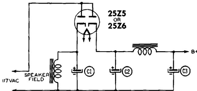
Fig. 11-5. Rectifier circuit formerly popular in AC-DC receivers.
