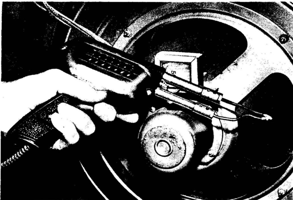
**Fig. 2-2. Using a solder gun to check the output transformer and speaker.**
