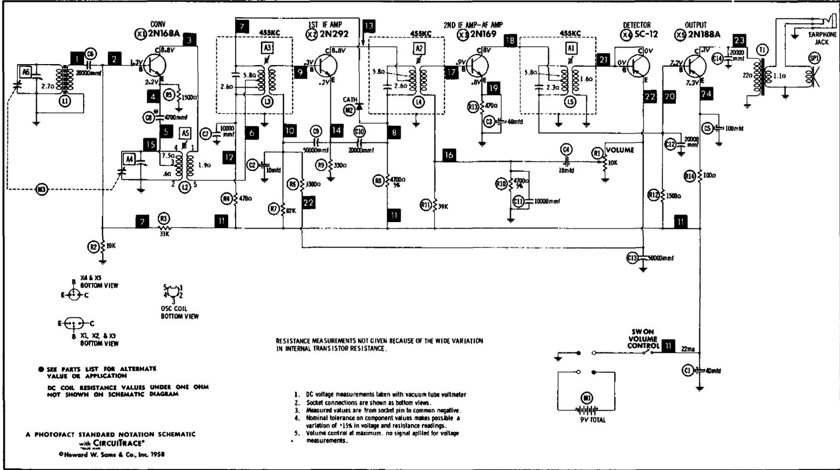
Fig. 14-7A. Schematic diagram of Trav-Ler Model TR-280 illustrating "CircuitTrace."
