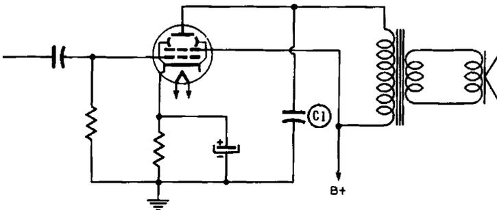
Fig. 3-5. Typical output circuit of AC-DC receiver.
