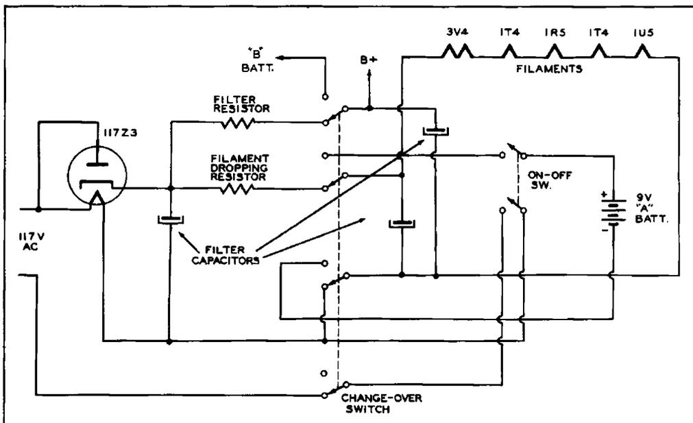
Fig. 1-6. Typical filament circuit of a three-way portable.
