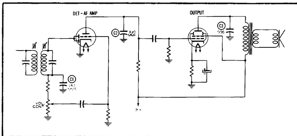
**Fig. 8-6. Partial schematic diagram of the detector and audio amplifier section of a typical receiver.**
