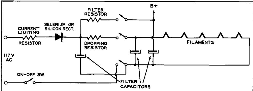
**Fig. 1-8. Filament circuit of a portable receiver employing a selenium or silicon rectifier.**
