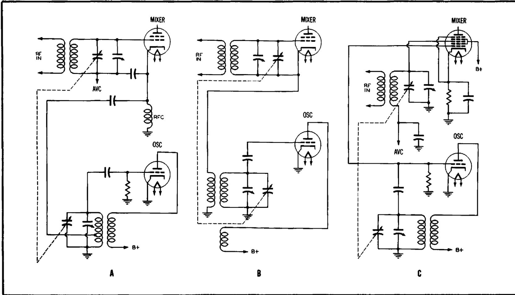
Fig. 4-2. Various methods of injecting the oscillator voltage into the mixer.
