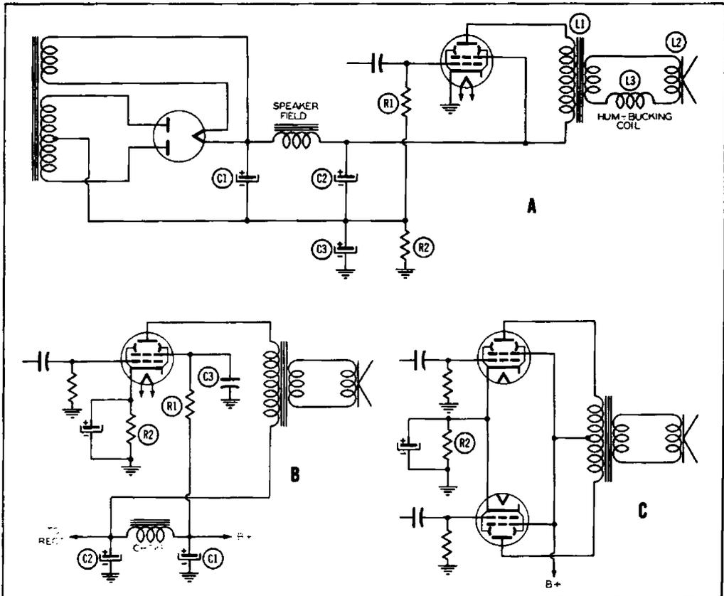
**Fig. 2-1. Basic output circuits commonly used.**
