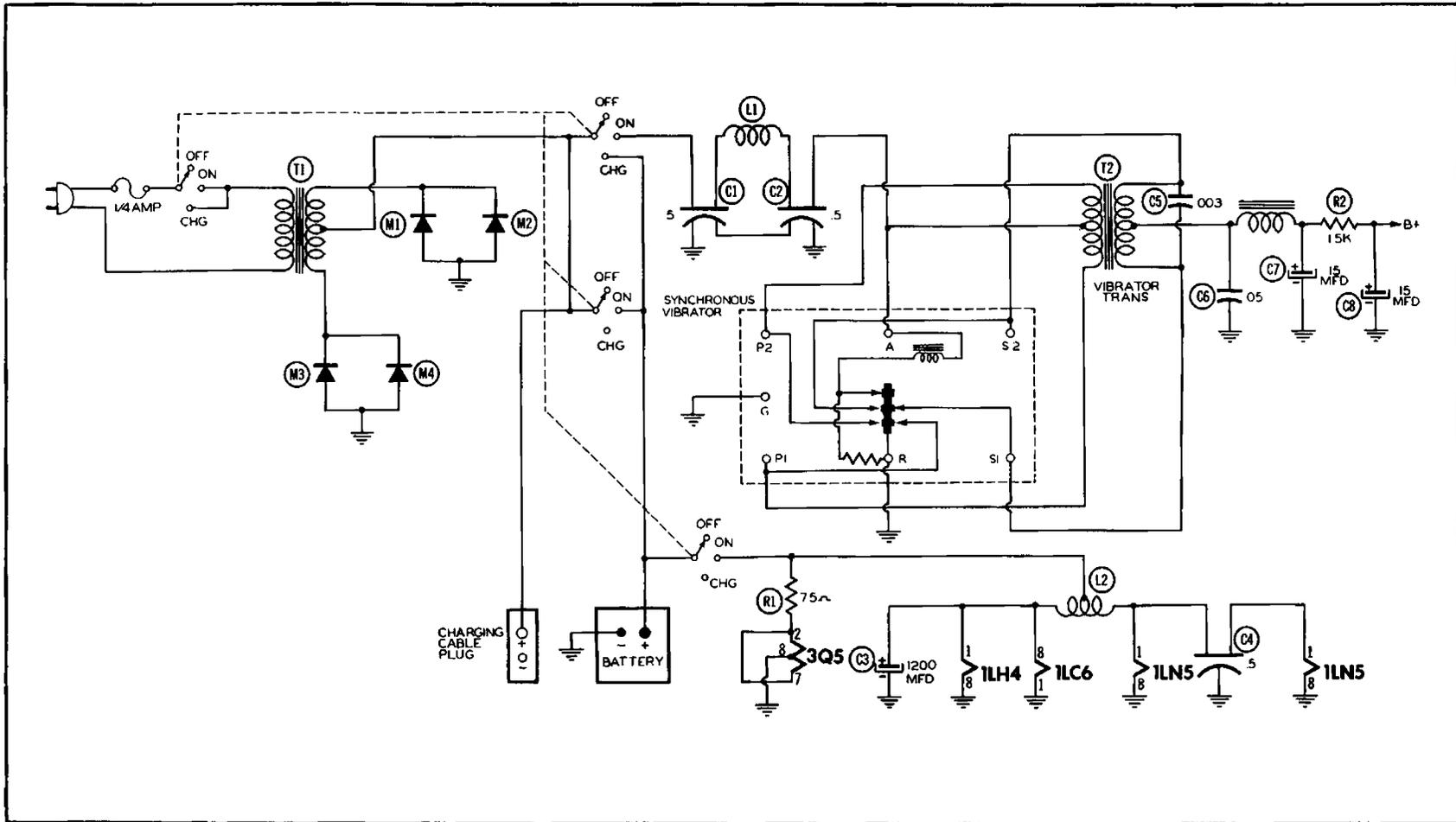
Fig. 15-6. Diagram of power supply used in the storage battery type of portable receiver.
