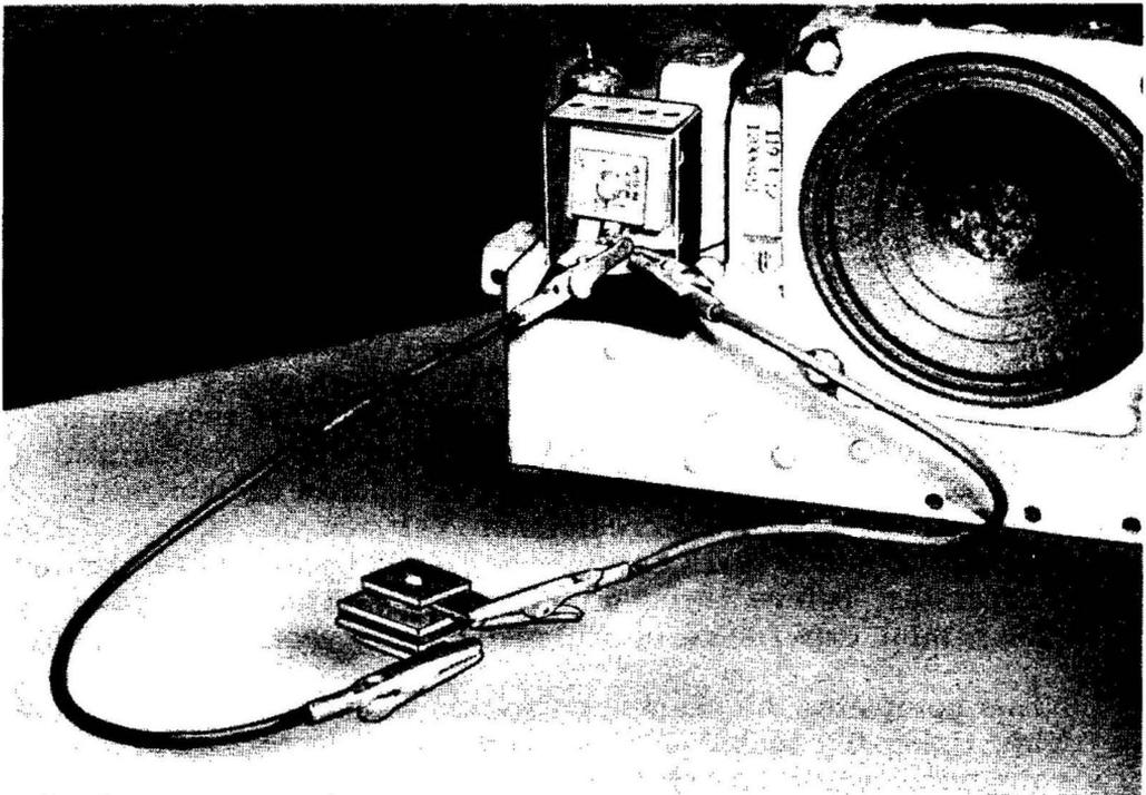
Fig. 1-9. Checking a selenium rectifier by substitution.
