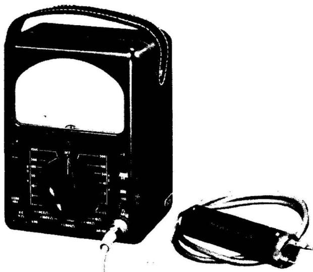
**Fig. 12-3. An RF probe for use with a VTVM.**
