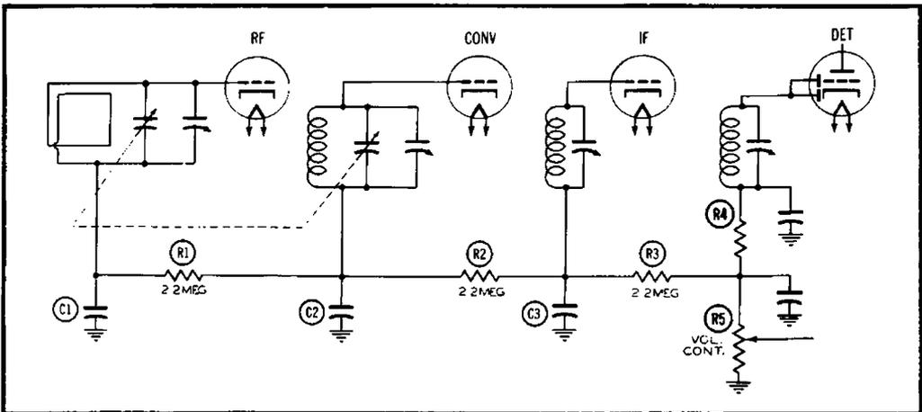
Fig. 8-4. Typical AVC circuit.
