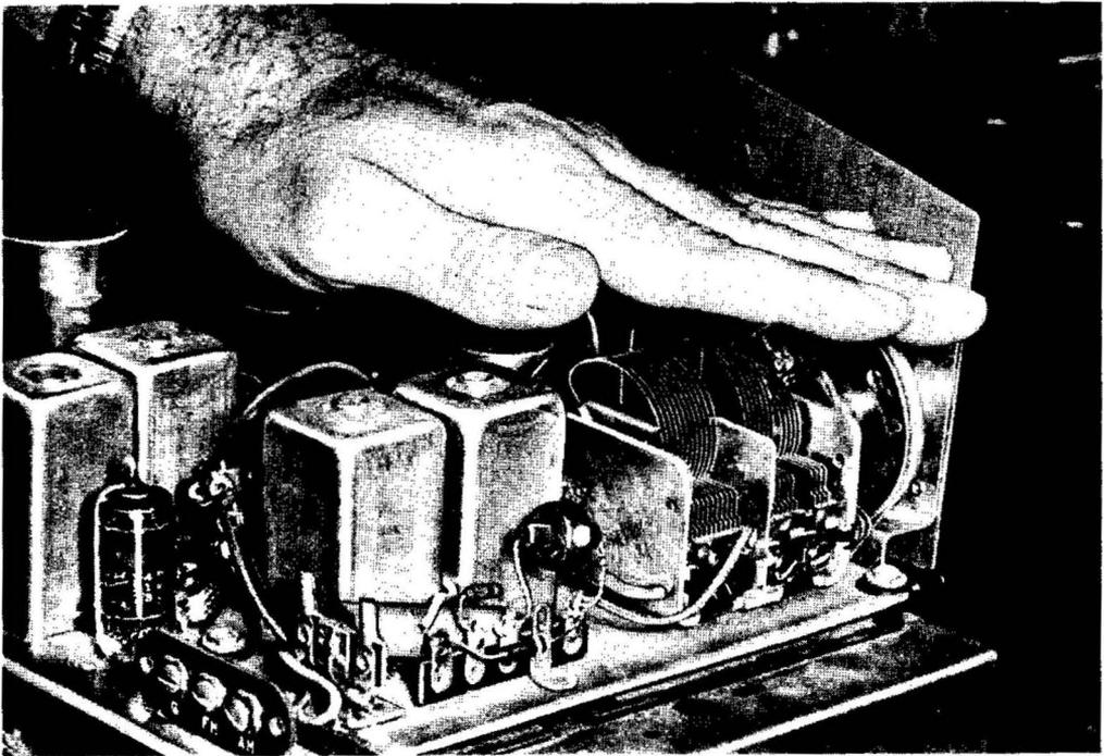
**Fig. 11-2. Checking for an open antenna coil.**
