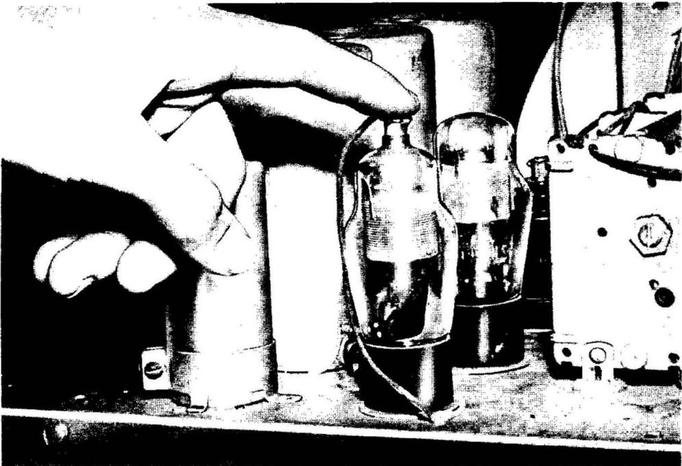
**Fig. 3-1. Method of injecting hum.**
