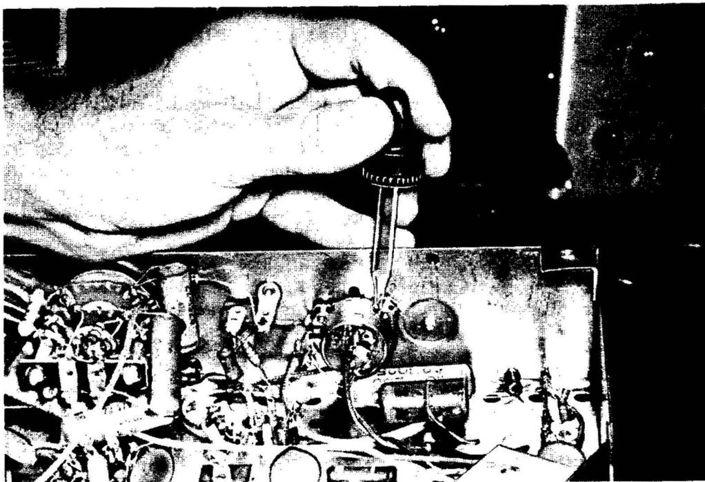
**Fig. 13-4. Contact cleaner being squirted into the volume control.**
