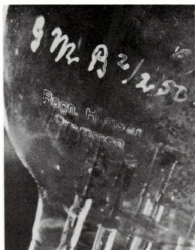
Fig. 22-2. Markings on Hansen Gmb 2/250 tube.
