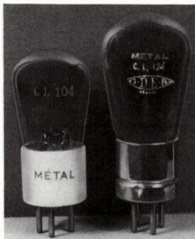
Fig. 19-8. Métal output tubes. Left: CL104. Right: CL124.
