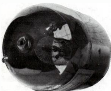
Fig. 11-12. Top view of the Round Type T valve, with tubulation removed, showing characteristic Round mesh-type grid.
