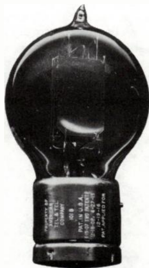
Fig. 6-14. A 101B repeater bulb with A.T.&T. Co. property markings.
