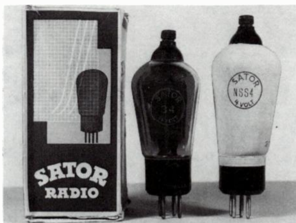
Fig. 19-24. Sator tubes. Left: S4. Right: NSS4.
