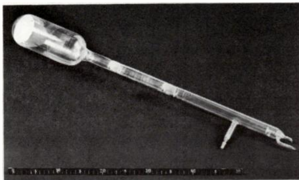
Fig. 2-10. The original Braun tube.
