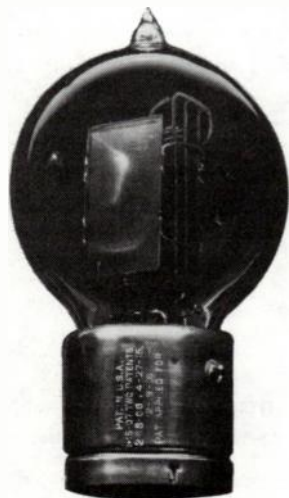
Fig. 6-13. An early-type of 101B repeater bulb with the patent markings steel-stamped on base shell. The code marking appears only in the wax on the bottom of the tube.
