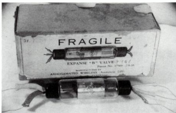
Fig. 13-5. The Expanse B valve made by Amalgamated Wireless (Australasia) Ltd. about 1920.
