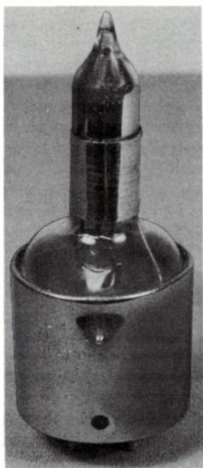
Fig. 17-6. A later Donle tube without the stabilizing enclosure and equipped with a UV base.
