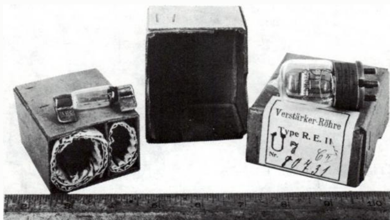
Fig. 12-29. The RE11 tube with ballast resistor.
