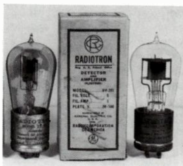
Fig. 16-1. The Radiotron UV201 amplifier tube. The tube at the left was made by Westinghouse Lamp Company and the one at the right by General Electric. The carton in the center is General Electric.
