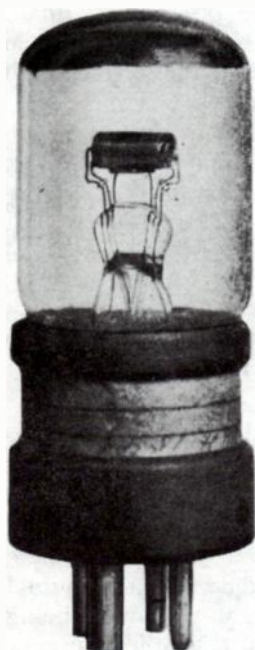
Fig. 12-30. The RE16 tube. The top is painted red. (Reproduced from E. Nesper, Der Radio-Amateur: Broadcasting , Berlin, 1923.)
