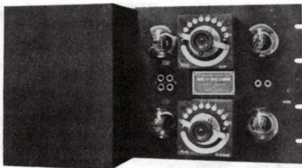
Fig. 18-3. Standard Telephones and Cables Type 4202F telephone repeater (four-wire type) using 4101D (V.T. No. 31) and 4102D (V.T. No. 32) valves. (Reproduced from P.O.E.E.J. , 1926.)
