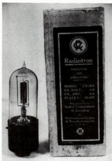
Fig. 16-3. Early Westinghouse Electric & Manufacturing Company version of Radiotron UV201, with shipping carton. Note the difference in filament rating from the tube shown in Fig. 16-1.
