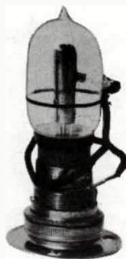
Fig. 3-9. Commercial form of Fleming valve, as used in Marconi-Fleming valve receiver.
