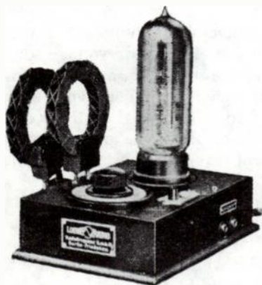
Fig. 21-27. Loewe Type OE333 radio receiver using 3NF tube. (Reproduced from Wireless Mag. , Dec. 1927.)
