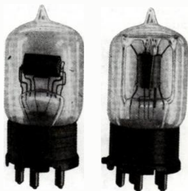
Fig. 12-33. Two RE20 tubes. Left: earliest construction. Right: improved version. (Reproduced from Telefunkenztg , 1920.)
