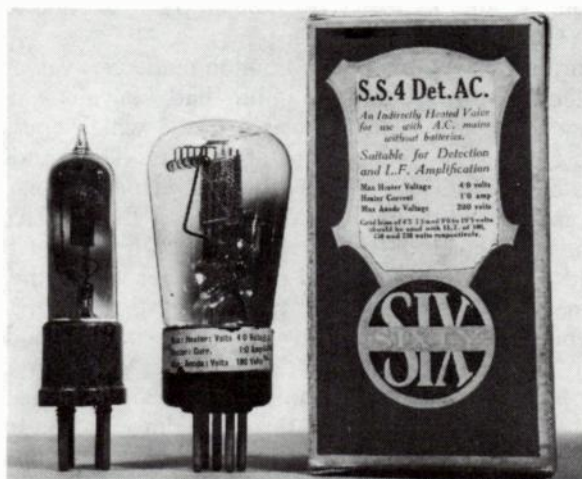
Fig. 18-31. Six-Sixty valves. Left: early design with no specific designation. Right: SS4 Det. A.C., made by Mullard.
