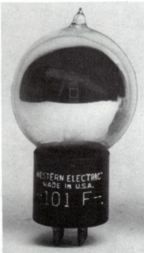
Fig. 14-7. A 101F with the code number stamped on molded base.
