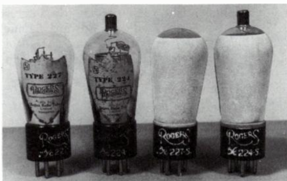
Fig. 17-22. Rogers Types 227 and 224 tubes. Left to right: Type 227 with paper label, Type 224 with paper label, Type 227S with spray shield and markings on base, and Type 224S with spray shield and markings on base.
