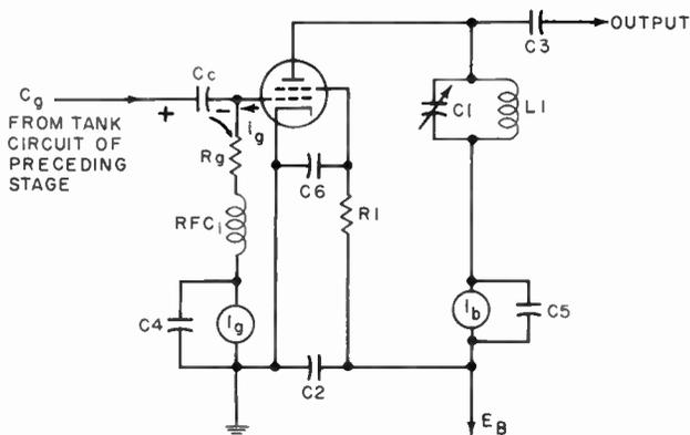
Fig. 2. Series-fed Class-C stage.
