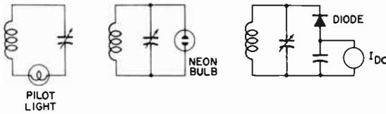
Fig. 2. Indicators for absorption wavemeters.
