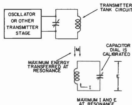
Fig. 1. Principle of the absorption wavemeter.
