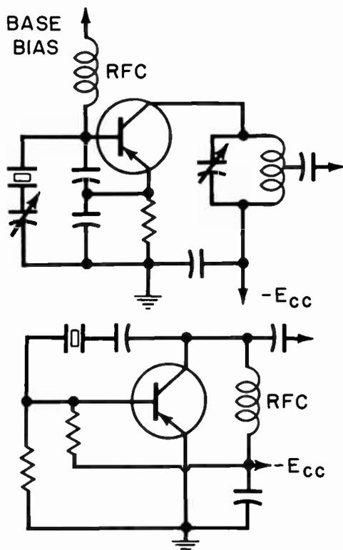
Fig. 11. Transistor crystal oscillators.
