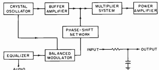
Fig. 4. Block diagram of a basic phase-modulation system.
