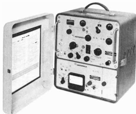
Fig. 18. Motorola Model T1099A frequency and deviation meter.
