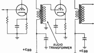
Fig. 13. Transformer-coupled audio stages.
