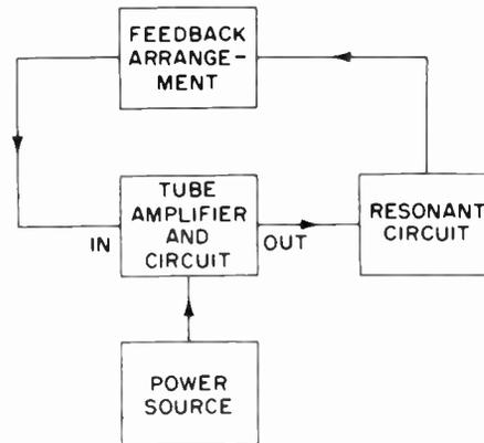
Fig. 13. Block diagram of a basic oscillator.
