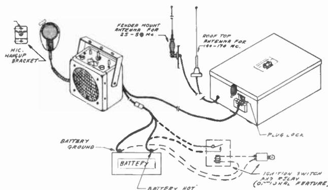
Fig. 2. Basic interconnections of mobile two-way radio components.
