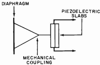
Fig. 3. Construction of a crystal or ceramic microphone.
