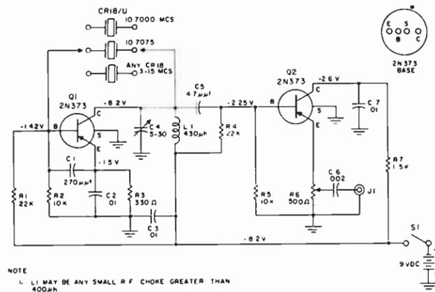
Fig. 3. Receiver alignment test oscillator.
