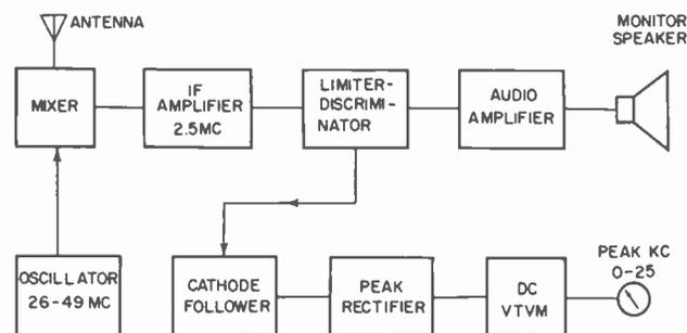
Fig. 17. Functional plan of Lampkin modulation meter.
