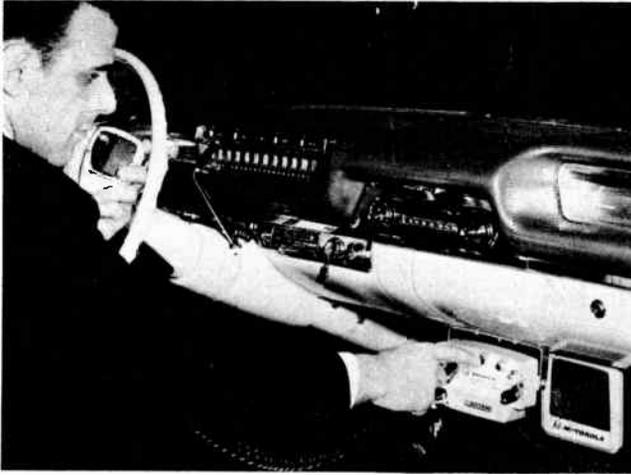
Fig. 2. Two-way radio control box and speaker.
