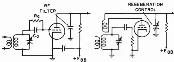
Fig. 2. Fundamental grid-leak and regenerative detector circuits.
