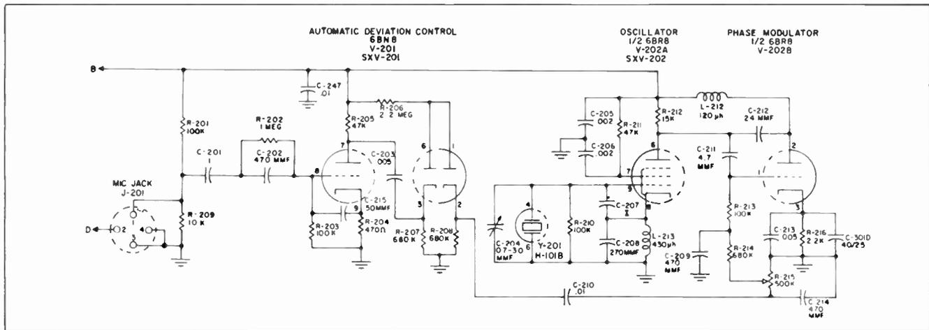
Fig. 10. NBFM phase modulation system of Aerotron transmitter.
