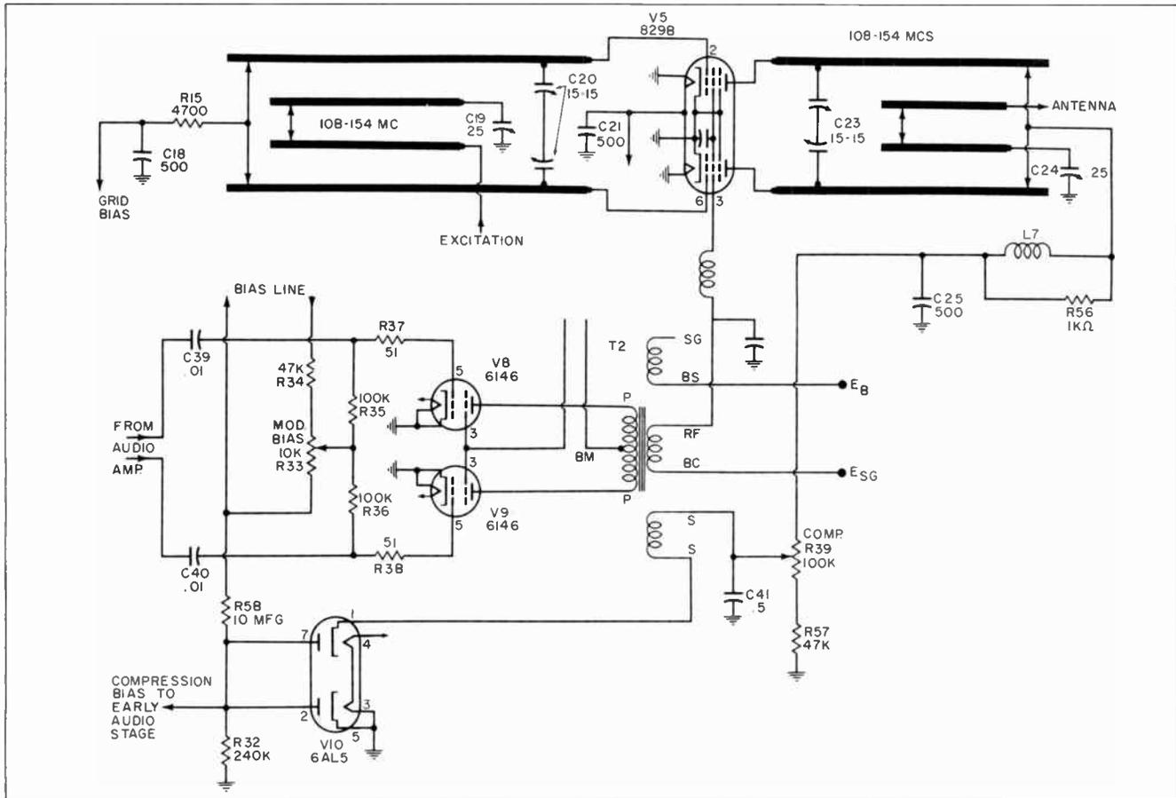
Fig. 4. Modulator and modulated amplifier of transmitter.
