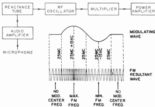
Fig. 1. Block diagram of a direct-FM system.
