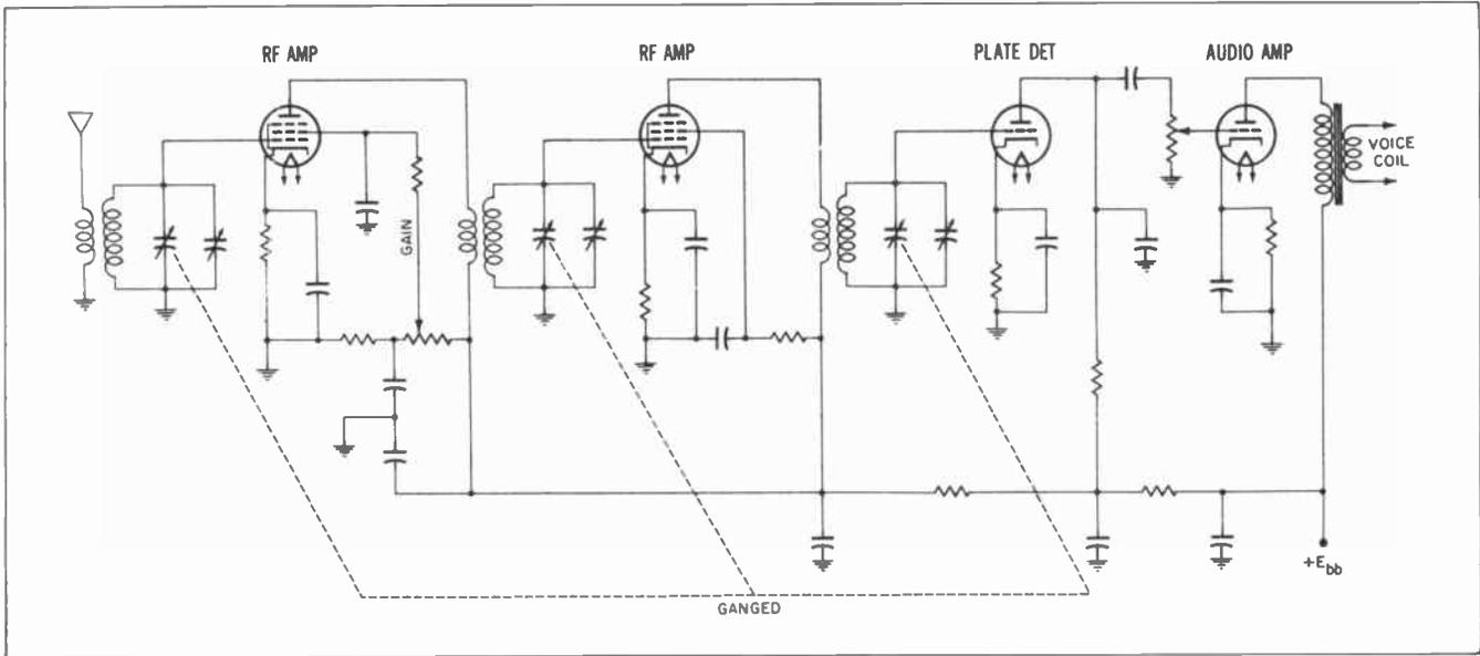
Fig. 6. Tuned RF receiver.
