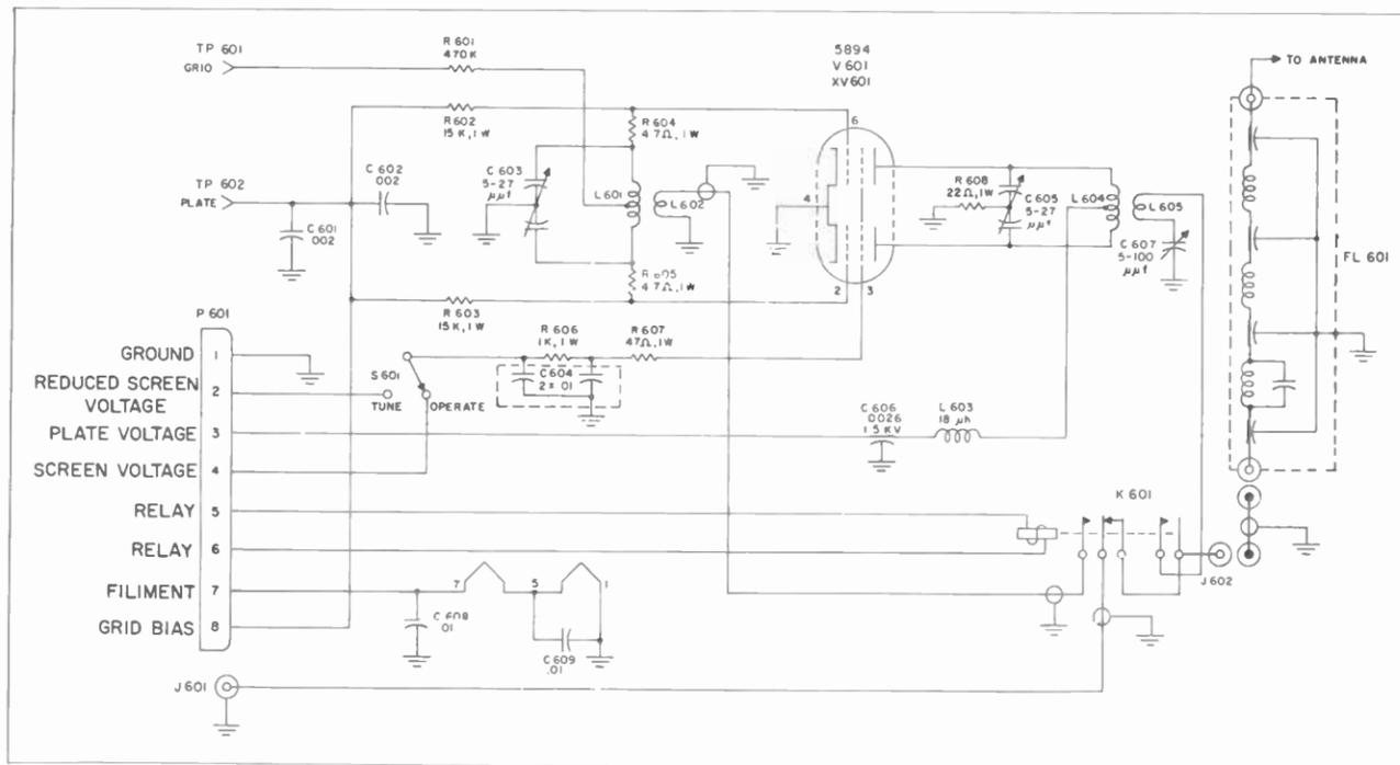
Fig. 7. Base station power amplifier.
