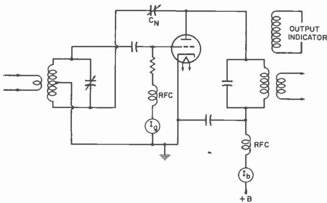
Fig. 3. Triode Class-C amplifiers must be neutralized.
