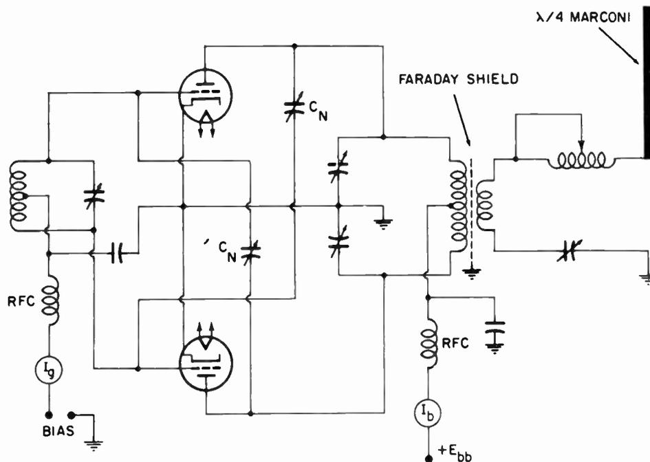
Fig. 11. Push-pull RF amplifier coupled to Marconi antenna.
