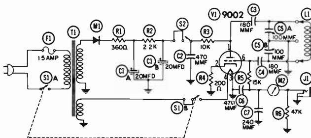
Fig. 6. Circuit of the Millen grid-dip oscillator.
