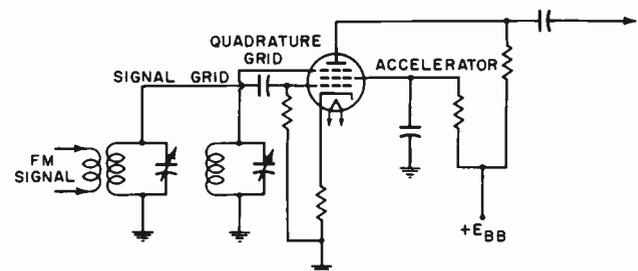
Fig. 10. Basic circuit for a gated-beam detector.
