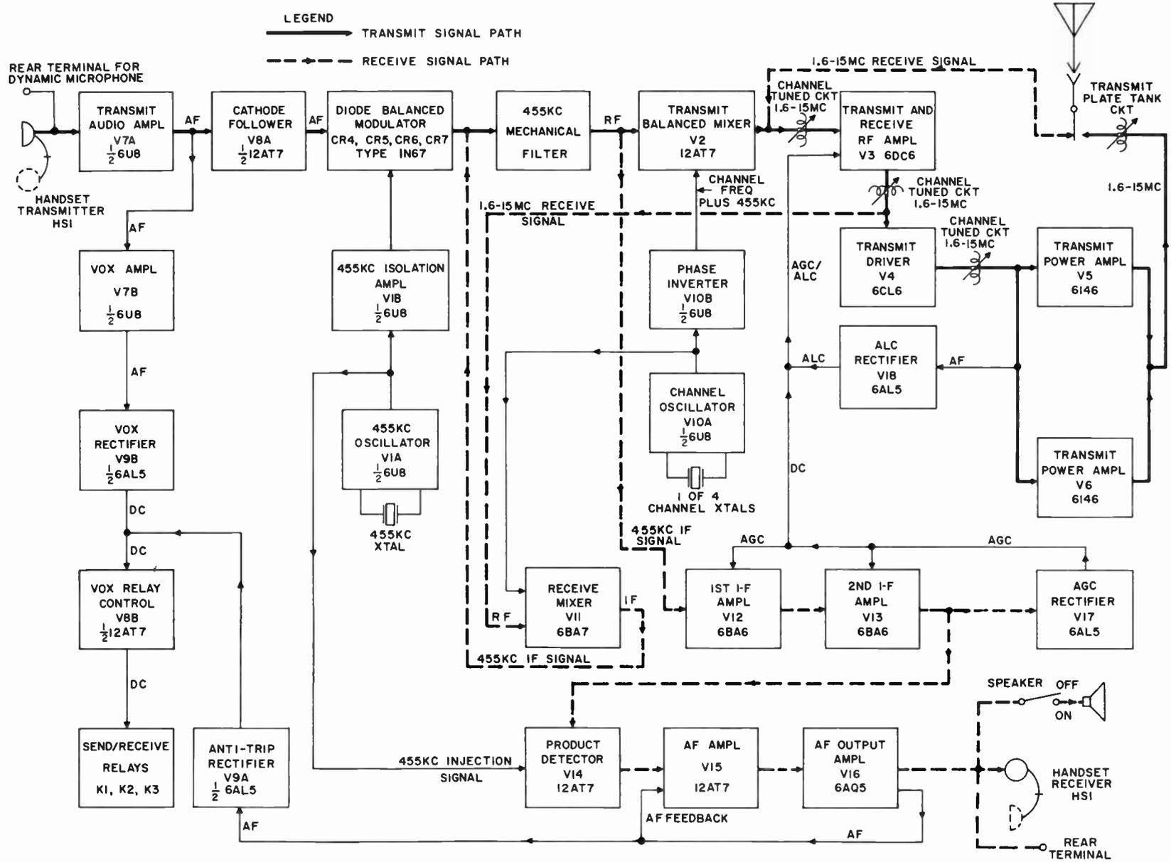
Fig. 4. Functional plan of Collins SSB system.
