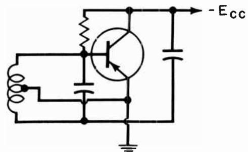
Fig. 10. Transistor Hartley oscillator.
