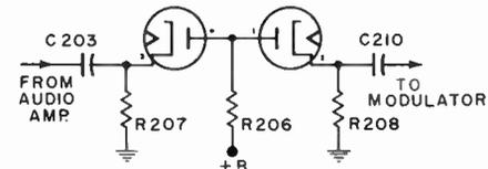
Fig. 12. Simplified schematic of an audio peak clipper.
