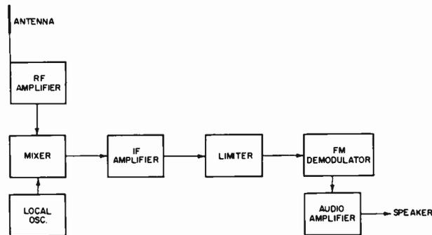
Fig. 8. Block diagram of an FM receiver.
