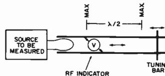
Fig. 12. Lecher-wire wavemeter.
