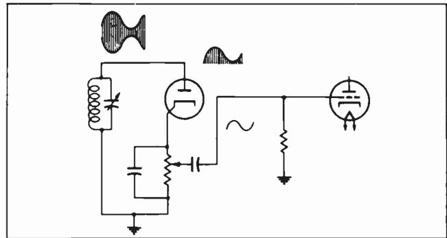
Fig. 11. Diode detector circuit, showing coupling to audio amplifier stage.
