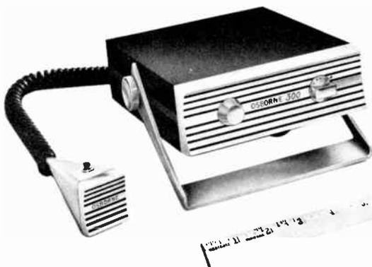
Fig. 3. Osborne all-transistor 5-watt CB unit.
