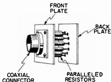
Fig. 10. Home-constructed dummy load.
