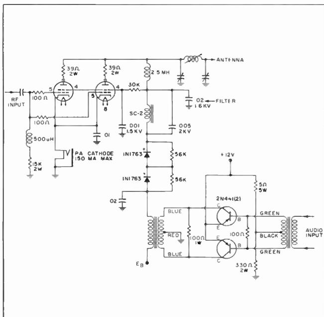
Fig. 6. Modulator and circuits for radiomarine transmitter.
