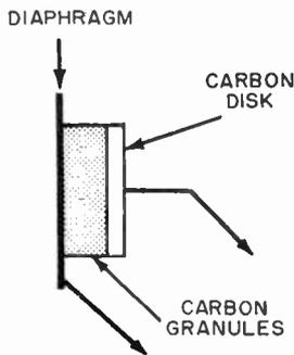
Fig. 1. Basic construction of a carbon microphone.
