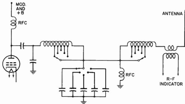
Fig. 9. Typical RF output system of a small-boat radio.
