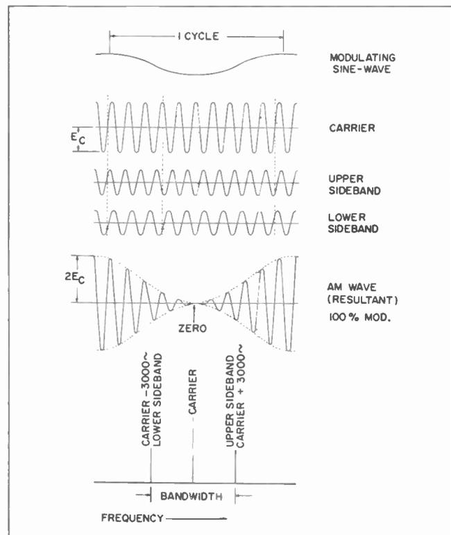
Fig. 1. The formation of an AM wave.
