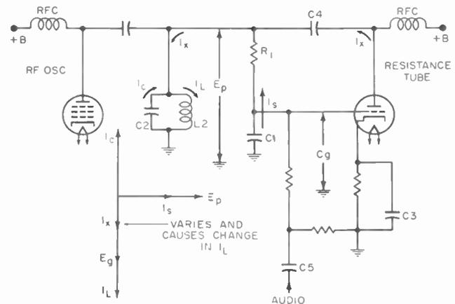
Fig. 2. Simplified schematic of a basic reactance-tube circuit.
