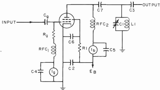
Fig. 3. Shunt-fed Class-C stage.
