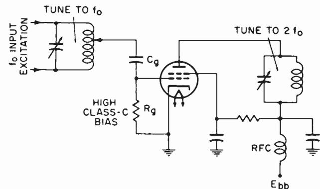
Fig. 10. Radio-frequency doubler.
