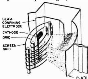
Fig. 10. Basic construction of a beam-power tube.
