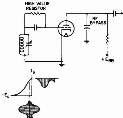
Fig. 12. Basic grid-leak detector circuit.
