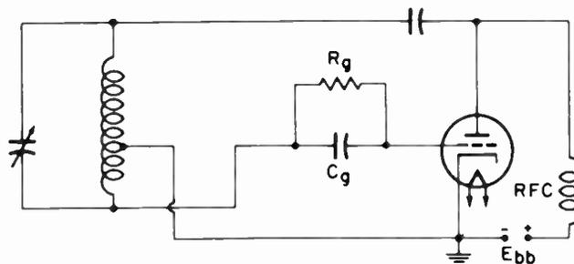
Fig. 12. Shunt-fed Hartley oscillator.
