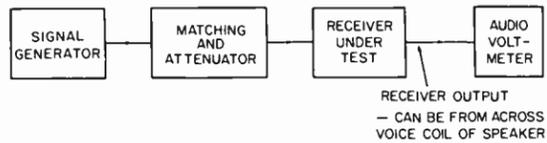
Fig. 2. Receiver sensitivity check.
