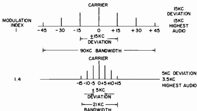
Fig. 3. FM sideband distribution as influenced by modulation index.
