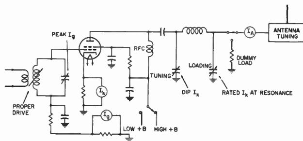
Fig. 5. Power amplifier tuning.
