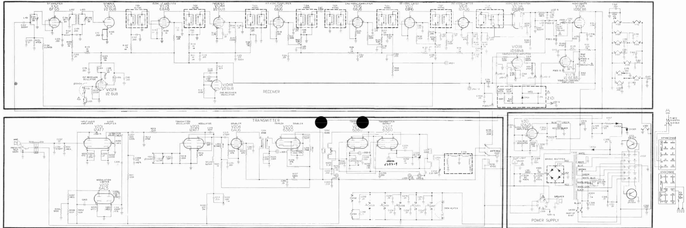
Fig. 1. Schematic diagram of Gonset FM communicator.
