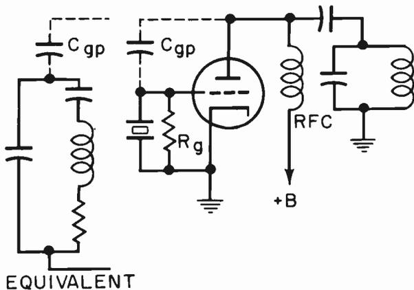
Fig. 6. Triode crystal oscillator and crystal equivalent.
