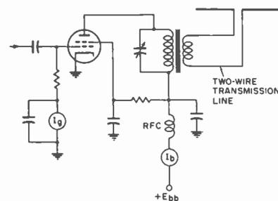
Fig. 10. Two-wire line feed to a Hertz antenna.
