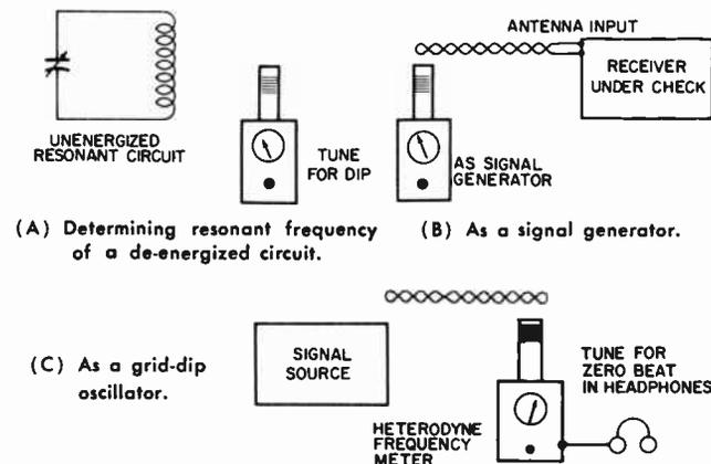
Fig. 7. Using the grid-dip meter.
