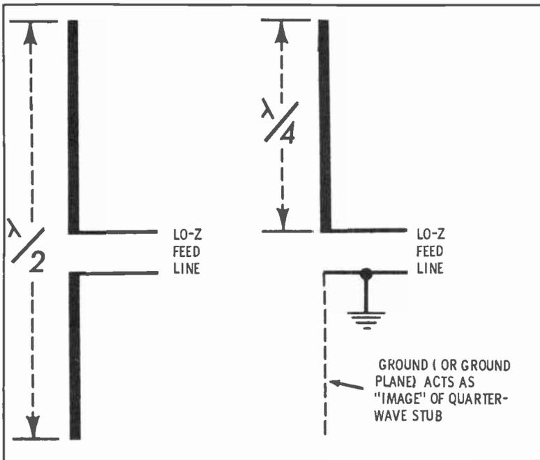
Fig. 1. Basic half-wave Hertz and quarter-wave Marconi antennas.
