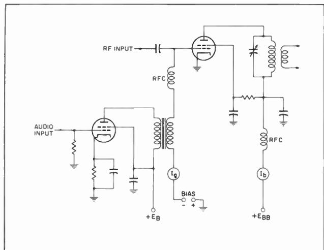
Fig. 9. Simplified grid-modulation system.
