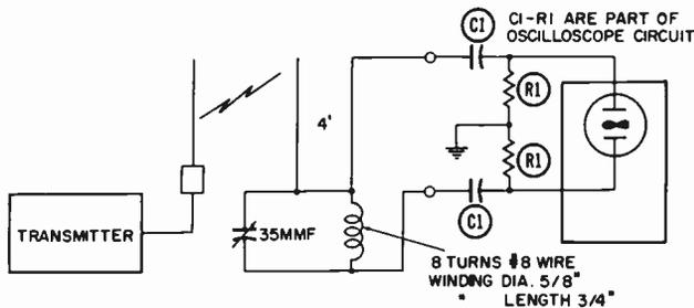
Fig. 19. Simple modulation-envelope check method.
