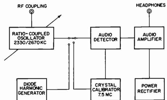
Fig. 15. Functional plan of Lampkin frequency meter.
