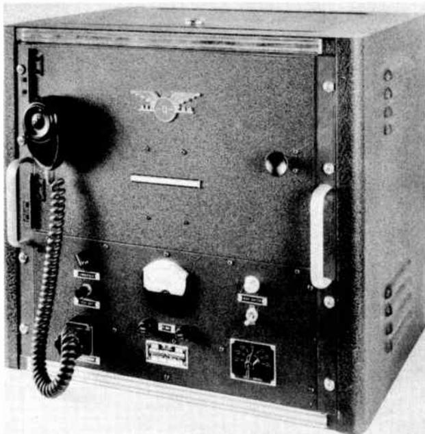
Fig. 5. Aerocom aeronautical base station transmitter.
