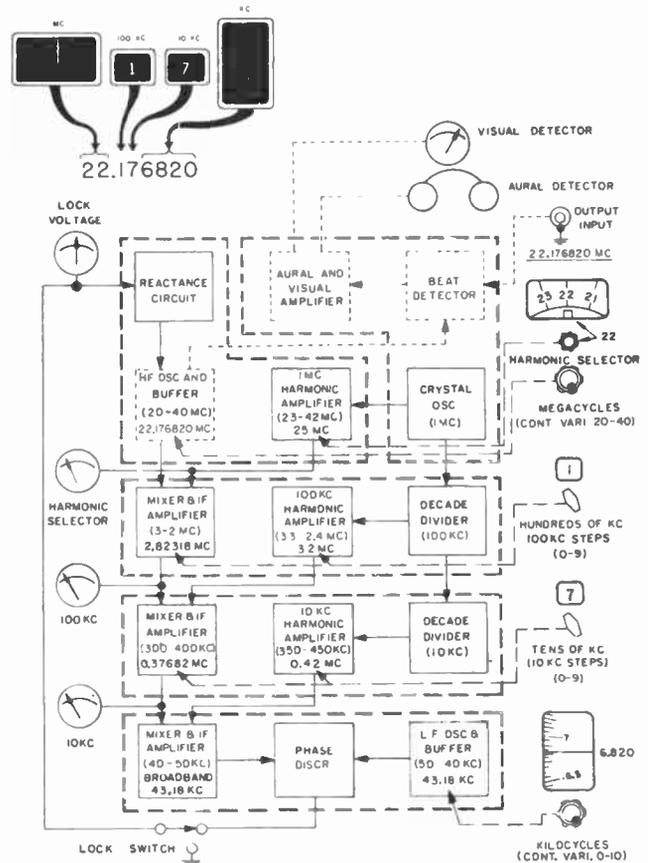
Fig. 13. Block diagram of Gertsch frequency meter.
