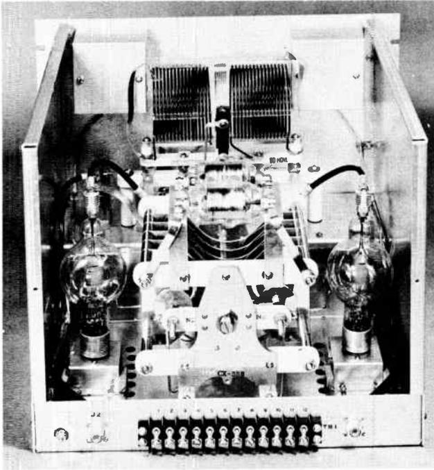
Fig. 8. Final power amplifier of Gates 500-watt transmitter.
