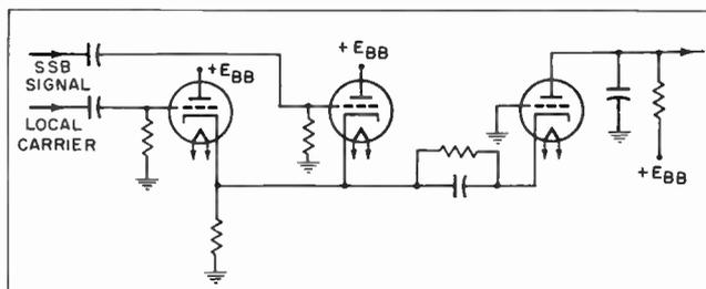
Fig. 7. Fundamental circuit of the Crosby product detector.
