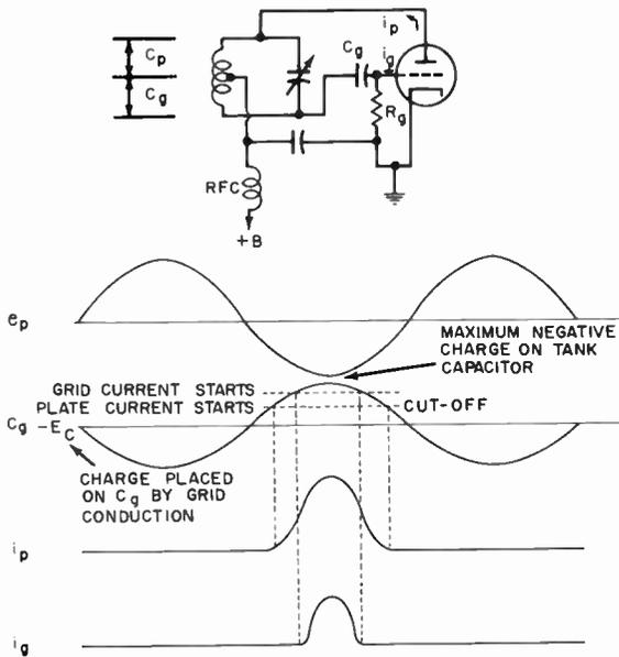
Fig. 2. Series-fed Hartley circuit and its associated waveforms.
