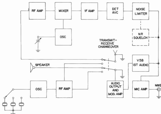
Fig. 1. Functional-block diagram of a Citizens band radio.
