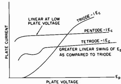
Fig. 9. Characteristics of triode, tetrode, and pentode tubes.
