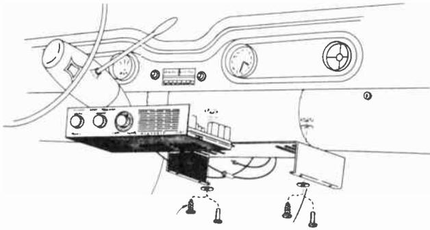
Fig. 8. Typical dashboard installation.
