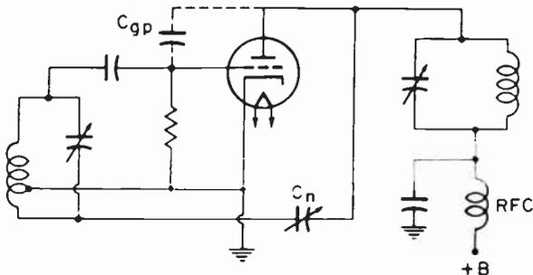
Fig. 9. Grid-neutralization triode RF stage.
