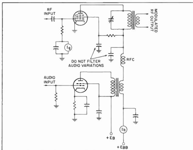
Fig. 8. Simplified plate-modulation circuit.
