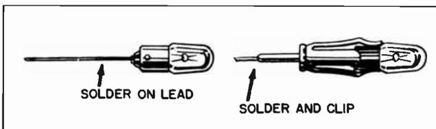
Fig. 12. A #47 bulb as a dummy load.
