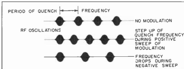
Fig. 4. The period between quench-frequency bursts varies with modulation.
