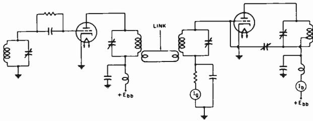
Fig. 11. TPTG oscillator link-coupled to a neutralized RF amplifier.
