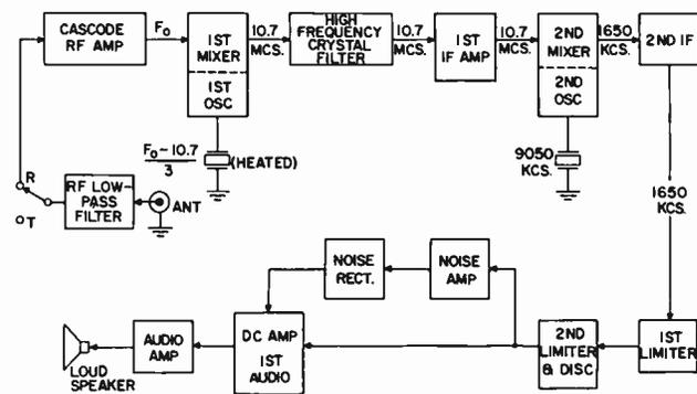
Fig. 2. Functional block diagram of an FM receiver.
