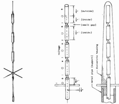
Fig. 5. Details of vertical collinear antenna structure.
