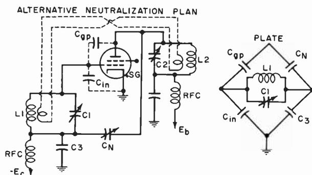
Fig. 8. Neutralization of a screen grid Class-C amplifier.
