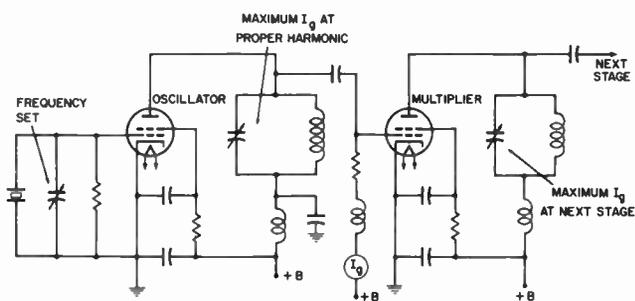
Fig. 4. Oscillator-multiplier adjustments.
