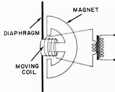
Fig. 4. Basic construction of a dynamic microphone.
