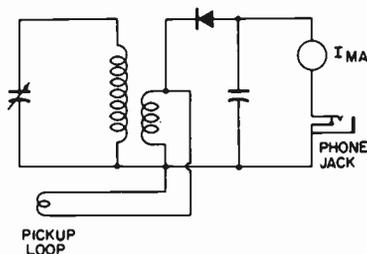
Fig. 3. Absorption wavemeter with pickup loop and phone jack.
