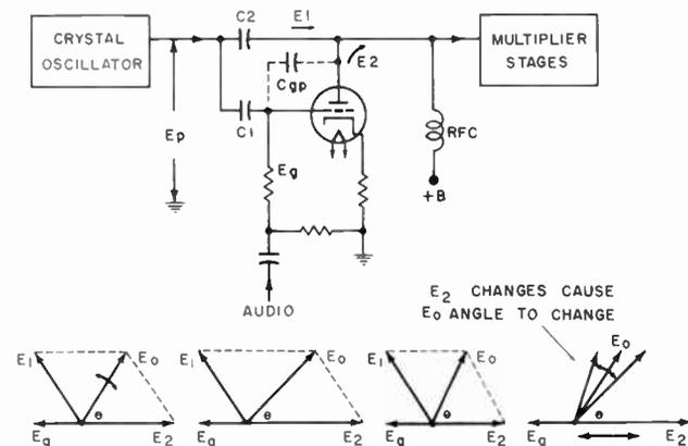
Fig. 6. Vector analysis of a narrow-band phase modulator.
