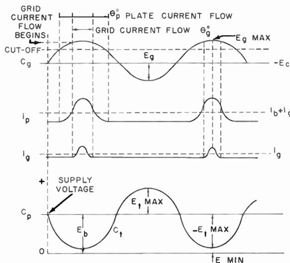
Fig. 4. Class-C waveforms.
