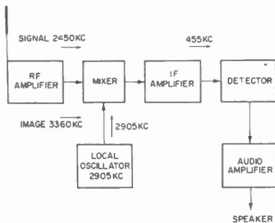
Fig. 7. Functional block diagram of a superheterodyne receiver.
