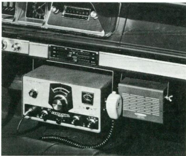
The Heathkit "Single Banders" are SSB transceivers giving individual coverage of 20, 40, and 80 meters. DC and AC power supplies make them suitable for either mobile or fixed operation.
