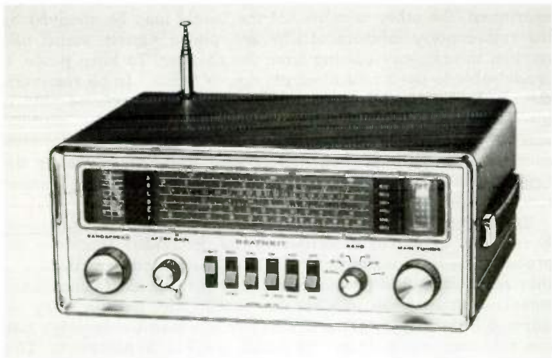
The Heathkit GR-78 is a six-band, solid-state, portable general-coverage receiver. It operates from a built-in nickel-cadmium battery, kept in condition by a self-contained AC charger. In addition to a full-tuning range from 550 kHz through 30 MHz, it also takes in the low-frequency band of 190-410 kHz. Never a dull moment with this set!
