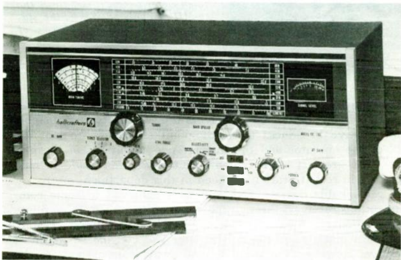
The Hallicrafters SX-133 is an AM broadcast and general-coverage short-wave receiver for monitoring applications on the international broadcast bands, the amateur bands, and the marine ship-to-shore frequencies. A large bandspread dial simplifies tuning.
