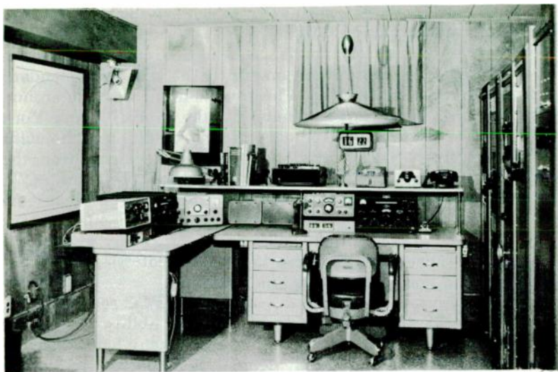
Two duplicate operating positions, five separate kilowatt amplifiers for the bands 10 through 80 meters, five separate antennas, and a generally elegant atmosphere are some of the features of station W2AB, assembled over a period of years by Lawrence LeKashman, Long Island, N.Y. A noted winner of operating contests, Larry can work on two bands at the same time by means of split headphones! Head of an electronic firm, he is one of many active hams who work professionally in electronics and enjoy radio as a hobby.
