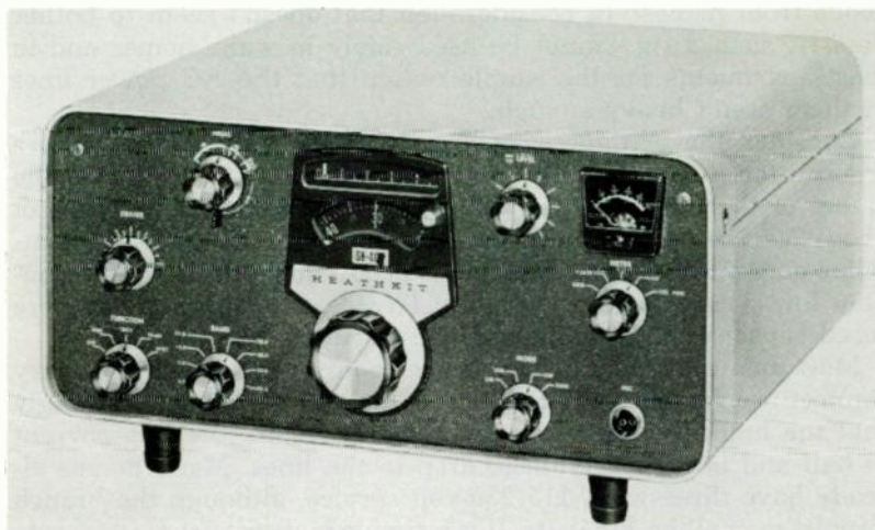
A companion for the SB-303 receiver, the Heathkit SB-401 transmitter offers full SSB and CW operation, and includes a built-in AC power supply. An interesting assembly project, but not for beginners.
