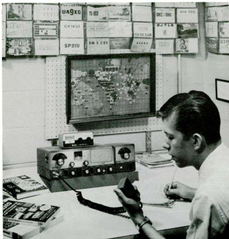
Here's a complete 6-meter station that occupies very little table space. Main unit is the Knight TR-106 transceiver, with V-107 VFO (variable frequency oscillator) and P-2 power meter. QSL cards on wall, which belong to Don Saxon, WA9FCD, Berwyn, Ill., represent 24 countries. Map shows local times in various countries having hams.
