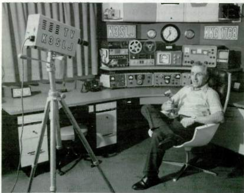
What's a TV camera doing in this beautiful ham shack of John A. Smetona, K3SLJ, of Pottsville, Pa.? Transmitting slow-scan pictures of John to other hams, that's what! Note monitor receiver under the clock. This television equipment, designed especially for amateur purposes, is made by Robot Research, Inc., San Diego, Cal.
