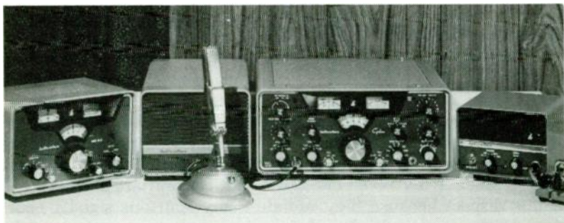
The Hallicrafters SR-400 "Cyclone" (center) is a high-grade transceiver shown here in a fixed installation. At left is optional variable-frequency oscillator, then combined AC power supply and speaker; at right, electric keyer.
