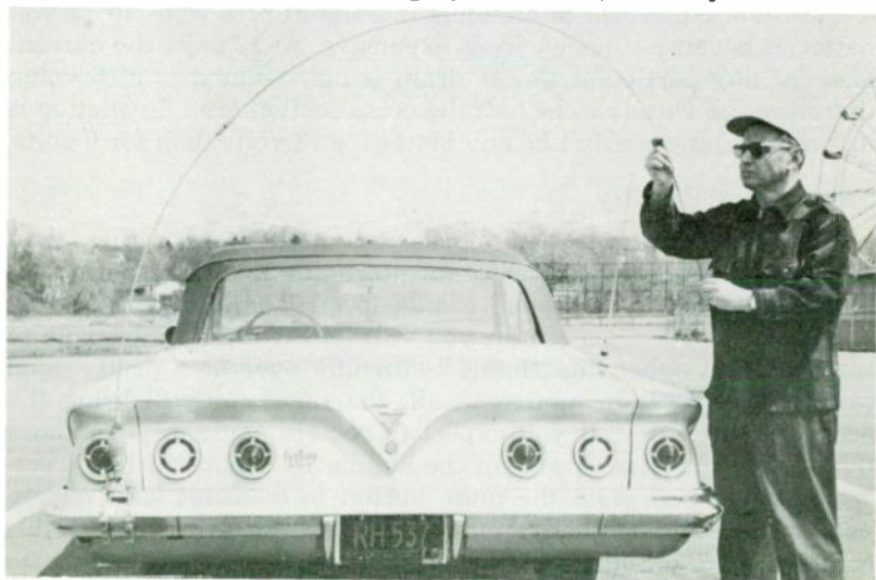
The simplest mobile antenna is a flexible 8-foot whip.
