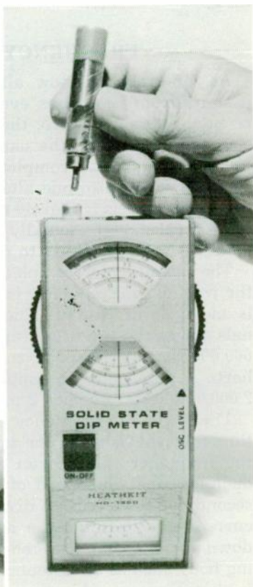
Above: Heathkit Model 1250 Dip Meter has plastic carrying case for outdoor use. Right: Coils for wide frequency spread plug into top edge of chassis. Dial is thumb operated. Below: Standard 9-volt transistor battery is self-contained.
