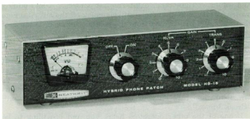
A phone patch puts telephone hook-ups on the air, a great stunt for letting service personnel overseas talk to their families stateside. This Heathkit unit Model HD-15 connects to the line without upsetting the characteristics of the ham equipment.
