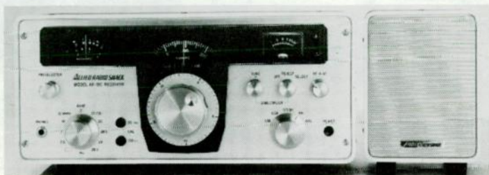
Allied Radio Shack, AX-190 is high-grade ham-band receiver, all solid state. Chassis is so crowded with circuit components that speaker is furnished as separate accessory, above.
