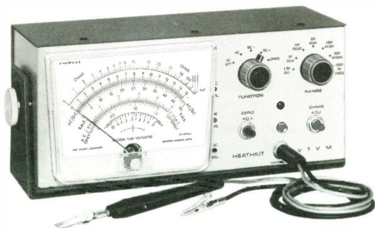
Horizontal-style vacuum-tube voltmeter, exemplified by Heathkit Model IM-28, is handy for bench use. Viewing angle is adjustable.
