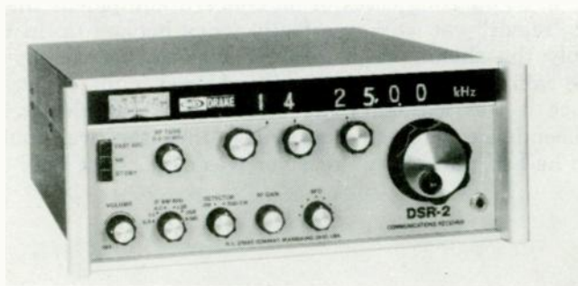
The Drake DSR-2 is a sophisticated general-coverage short-wave receiver, covering 10 kHz through 30 MHz. It has a digital readout of frequency accurate to 100 hertz, displayed along top edge of front panel.
