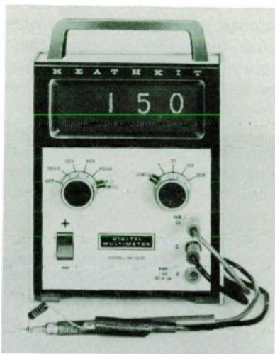
Representative electronic voltmeters popular with hams and technicians. Left: RCA Model WV-500B "VoltOhmyst" solid-state meter works on self-contained batteries. Right: Heathkit Model IM-1202 is an interesting multimeter with digital readout instead of a scale.
