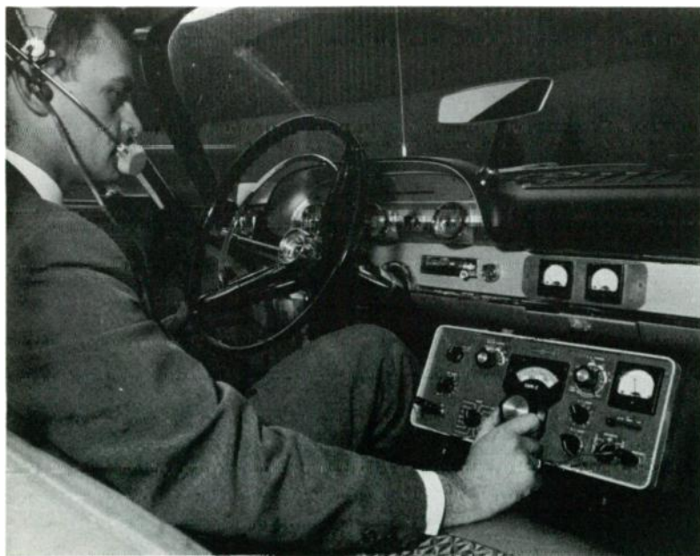
The Collins KWM-2 is a popular SSB transceiver for mobile use. Covers 10 through 80 meters; separate power pack. Note combined microphone and earphones. It leaves operator's hands free for driving and tuning.
