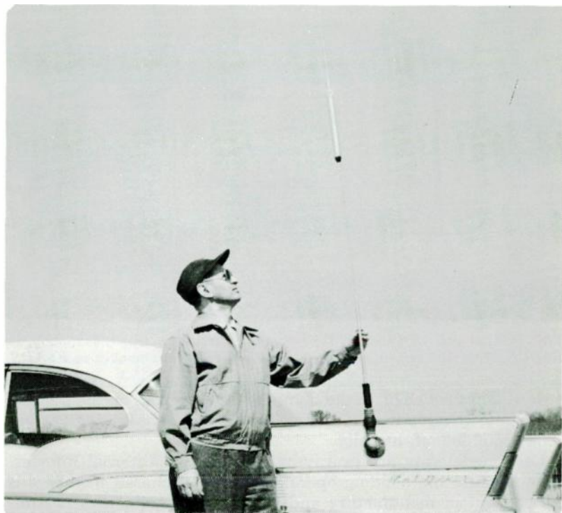
This Mosley MA-3 antenna works on 10, 15, and 20 meters without switches or adjustment—a great convenience in mobile operation. The owner of this car didn't mind making a hole in the body to put antenna in the clear. Result: He works world-wide DX with a 50-watt transceiver!
