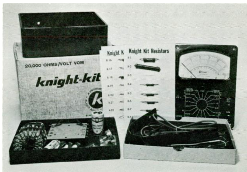
A typical VOM kit with its components spread out. Resistors are numbered individually for easy identification. The meter proper is part of the front panel. There are several similar kits on the market.
