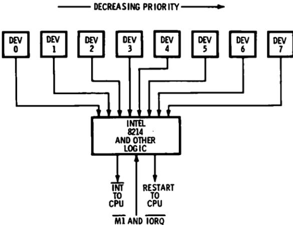
**Fig. 7-4. Priority encoding for interrupt mode 0.**
