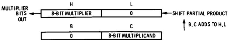
Fig. 12-10. An 8-bit multiply register arrangement.
