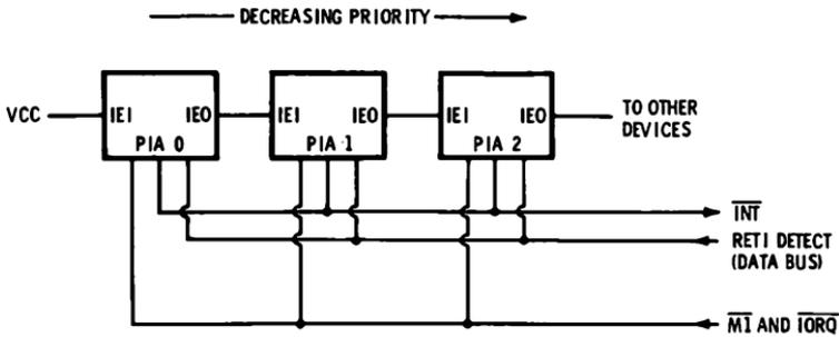
Fig. 7-7. Z-80 interrupt prioritizing interrupt mode 2.
