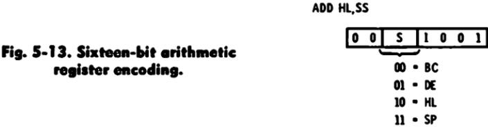
**Fig. 5-13. Sixteen-bit arithmetic register encoding.**
