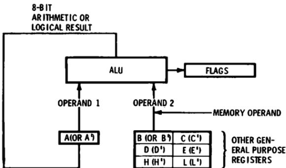
**Fig. 2-3. Arithmetic and logical operations.**
