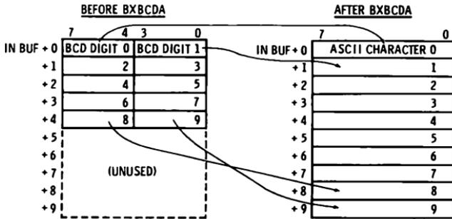
Fig. 12-6. Bcd to ASCII conversion.
