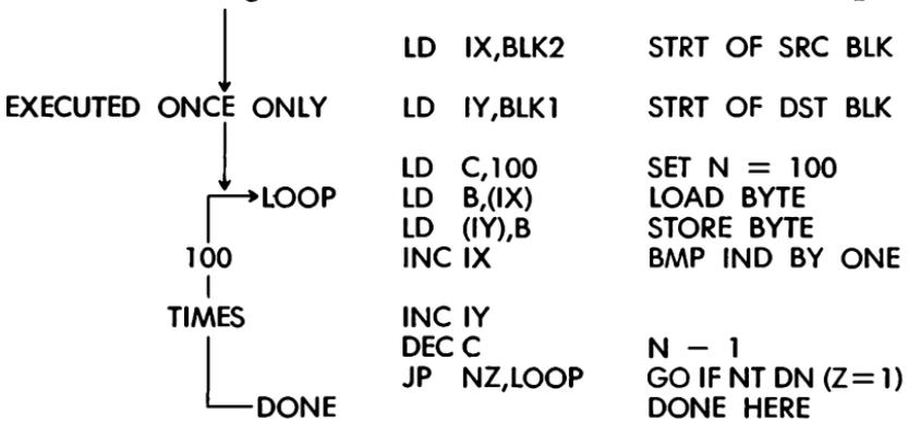
LOOP is executed 100 times as long as  $N = 100$  to 1, the Z flag is not set and the conditional branch JP NZ, LOOP is made. IX and IY are incremented by one each time through the loop to point to the next position in the blocks.
