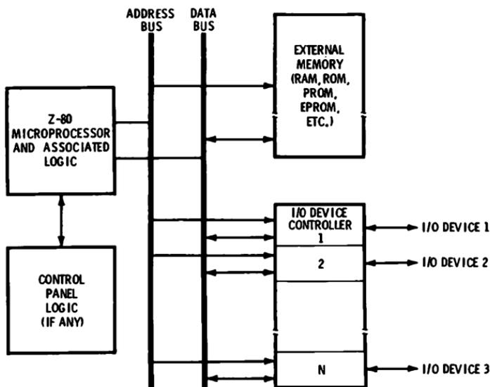
Fig. 2-10. Z-80 Microcomputer system component parts.
