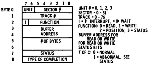
Fig. 15-2. Floppy-disc I/O driver-parameter block.
