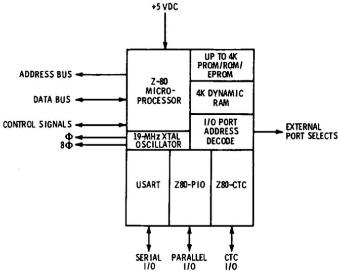
**Fig. 17-2. Z-80 MCB™ functional block diagram.**
