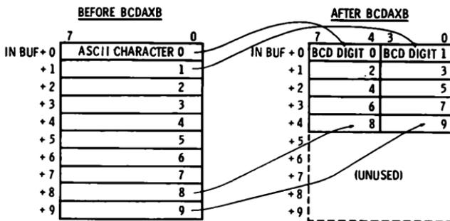
**Fig. 12-5. ASCII to bcd conversion.**
