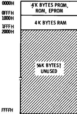
**Fig. 17-3. Z-80 MCB™ nominal memory mapping.**
