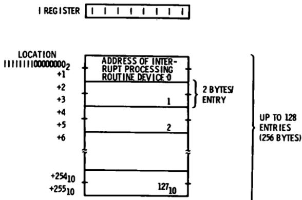
Fig. 7-5. Interrupt mode 2 interrupt vector table.
