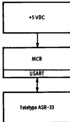
Fig. 17-4. Minimum MCB system.
