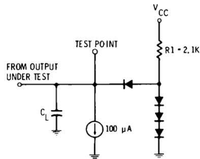
Fig. A-2. Load circuit for output.
