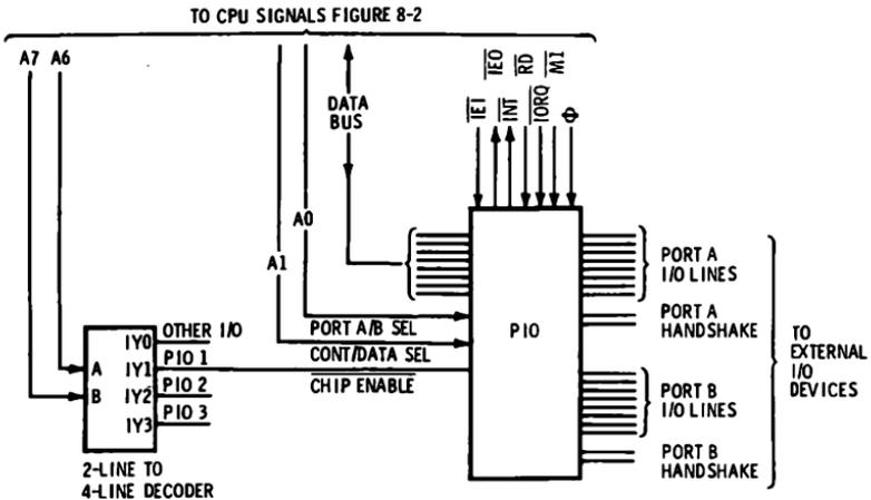
**Fig. 8-12. PIO use in minimum configuration system.**
