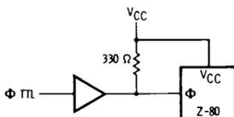
An external clock pull-up resistor of ( $330\ \Omega$ ) will meet both ac and dc clock requirements.
