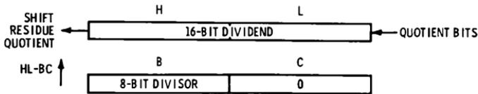
**Fig. 12-11. A 16-bit by 8-bit divide register arrangement.**
