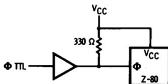
An external clock pull-up resistor of (330 $\Omega$ ) will meet both the ac and dc clock requirements.
