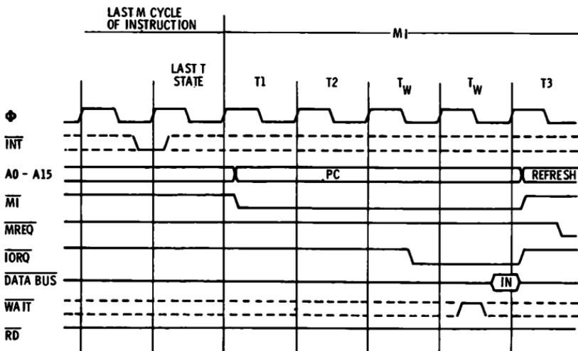
Fig. 3-9. Interrupt Request/Acknowledge cycle.
