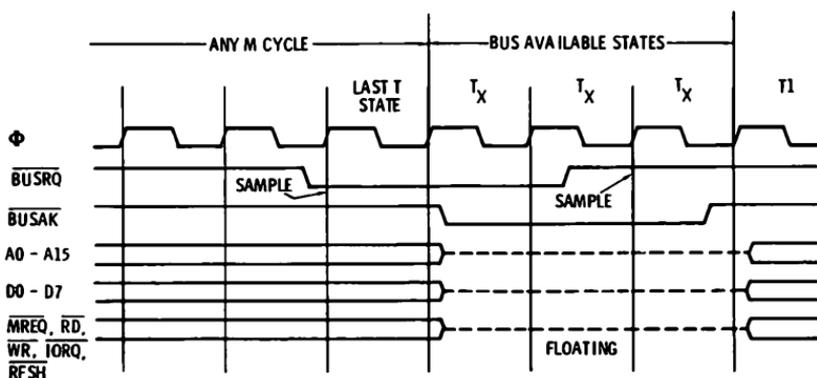
Fig. 3-8. Bus Request/Acknowledge cycle.
