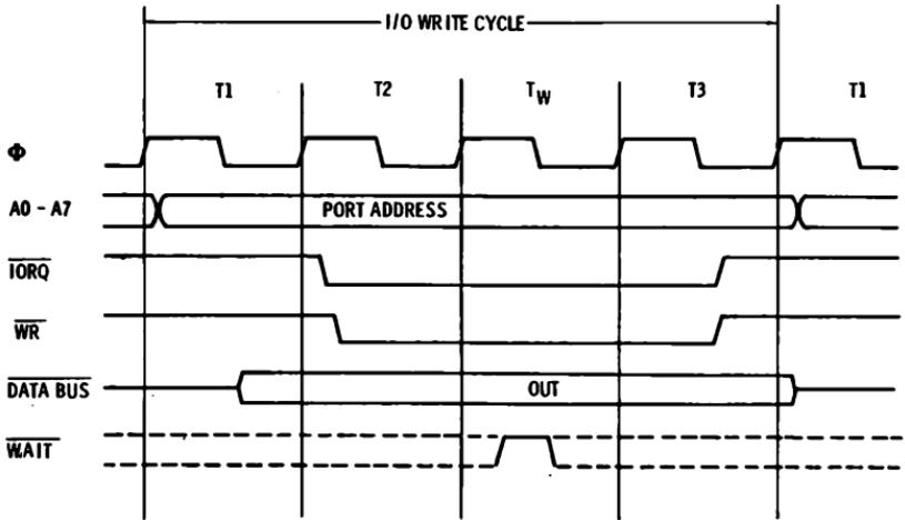
Fig. 3-7. I/O Write cycle.
