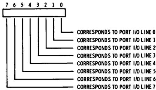
Fig. 8-9. PIO mode 3 input/output programming.
