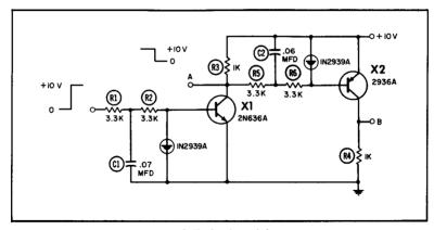
Tunnel-diode time delay.
