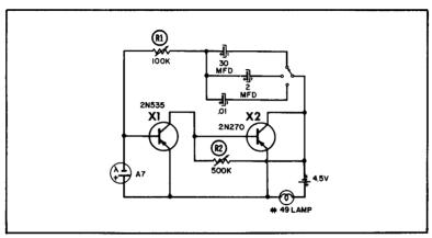
(B) Photocell stroboscope.
