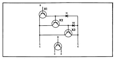
Fig. 5 — Composite transistor equivalent circuit.
