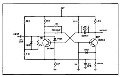
Output (at collectors) has 8 volt level change. Output pulse duration 2  $\mu$ sec to 1 sec, Maximum input frequency 250 kc. Maximum required input pulse is 5 volts. Duty cycle exceeds 60% Ambient temperature  $-56^{\circ}$  C to 71° C.
