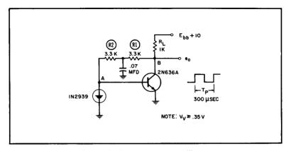
Tunnel-diode square-wave oscillator.
