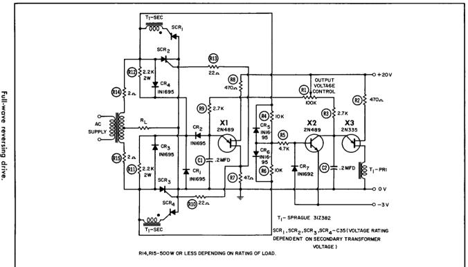
SCR-1 and SCR-4 have electrically isolated cathodes, the gate signal pulse generated by UJT X3 is coupled to the SCR gates by isolated secondary windings on transformer T1. Transistor clamp X2 synchronizes the firing of X3 to the anode voltages across SCR-1 and SCR-4.
