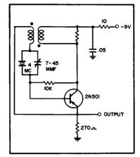
(C) 4-mc oscillator & waveform.
