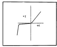
(B) Germanium diode operating curve.
