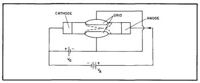
A) Physical construction of field effect transistor.
