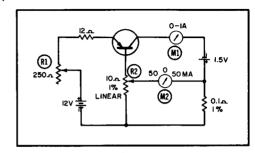
(B) Beta tester for power transistor.
