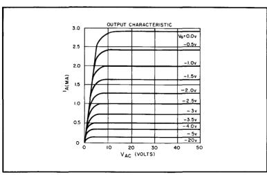
(B) Characteristic chart of field effect transistor.
