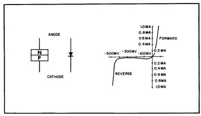
Fig. 17 — Backward diode and characteristics curve.
