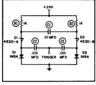
Four-layer diode RC oscillator.
