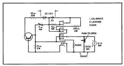
(A) Power transistor tester.
