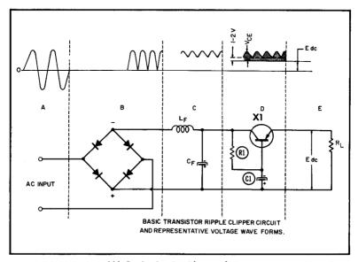
(A) Basic circuit with waveforms.
