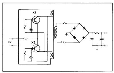
DC to DC converter (mobile radio supply).
