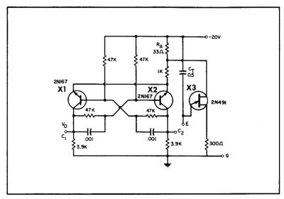
(D) NPN transistor timing circuit.
