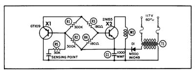
Transistor detection sensor.
