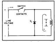
(C) Selenium rectifier shunts coil.
