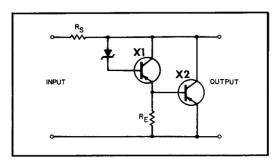
(B) Diode controlling base of X1.
