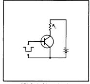
(B) High input impedance amplifier and converter.
