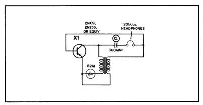
(B) Transistor oscillator.
