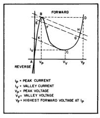
Fig. 16 — Tunnel diode characteristic curve.
