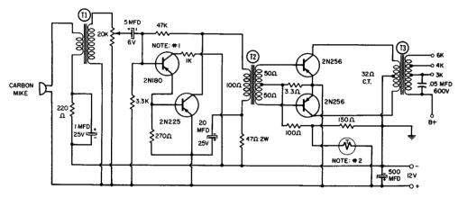
NOTE: #1 LOWER GAIN TRANSISTORS, SUCH AS THE 2NIO7, GT222, AND CK722, MAY BE SUBSTITUTED FOR THE 2NIBO UNITS.
