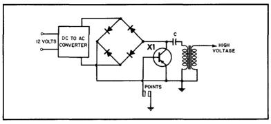
(B) Transistor switching.
