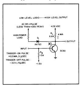
PNPN Trigistor as a static switch. tive AC peaks. During this period of high current flow, the *Trigistor* cannot be turned off, so the logic and high-level output functions must be accomplished on a time-sharing basis. During each negative excursion of the AC voltage, one or hundreds of logic operations can be performed.
