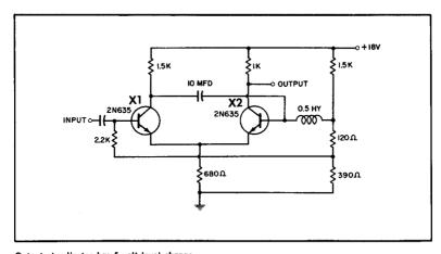
Output at collector has 5 volt level change. Output pulse duration approx. 600 µsec. Maximum input pulse required 3 volts. Ambient temperature —56° C to 71° C.
