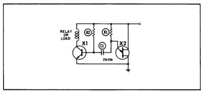
(B) UJT multivibrator driving an NPN transistor.
