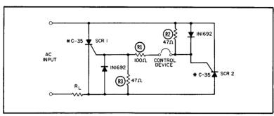
THE SCR AS AN AC STATIC SWITCH
