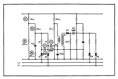
Tunnel-diode shift register.
