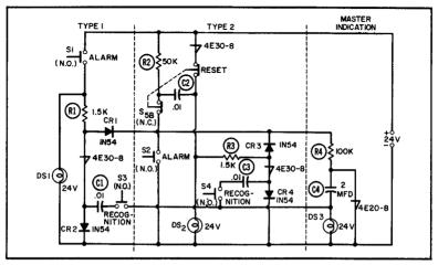
Alarm circuit with flashing master light.
