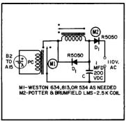
(D) Cascaded photoelectric relay.
