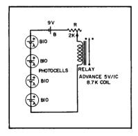
(C) Series photocell relay circuit.
