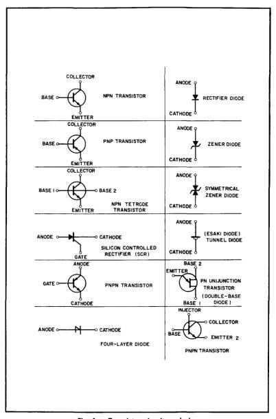
Fig. 1 — Transistor circuit symbols.
