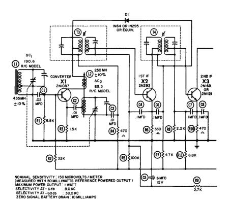
Six transistor, 12-volt superheterodyne.
