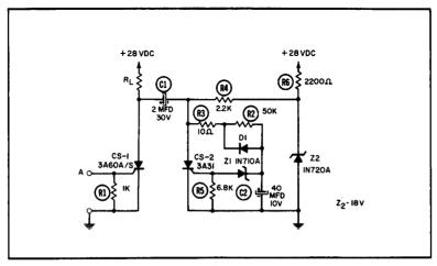
Interval timer with high-level output.
