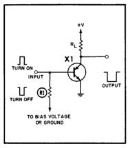
(A) Turn on-off at base; collector output.
