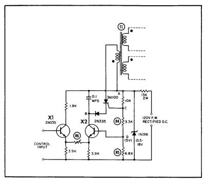
(C) Control circuit with balanced input amplifier.
