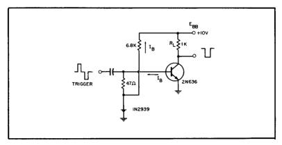
Tunnel-diode Bistable circuit.
