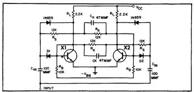
(A) Basic RC coupled flip-flop circuit.
