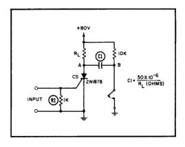
(B) Shunt capacitor turn off.
