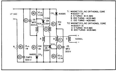
AC static switching circuit.
