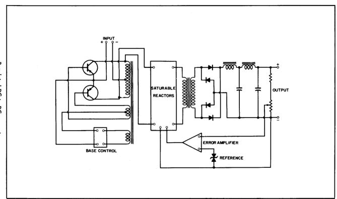
sistors (hence, the maximum base current of the oscillator pair) is determined by this bias voltage.
