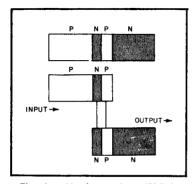
Fig. 6 — Hook transistor (PNN).
