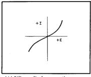
(A) Silicon diode operating curve.
