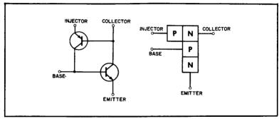
Fig. 12 - Binistor equivalent circuit.
