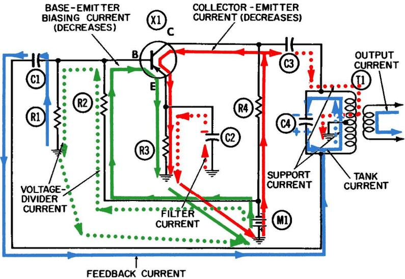
**Fig. 3-2. Operation of the Hartley oscillator—positive half-cycle.**
