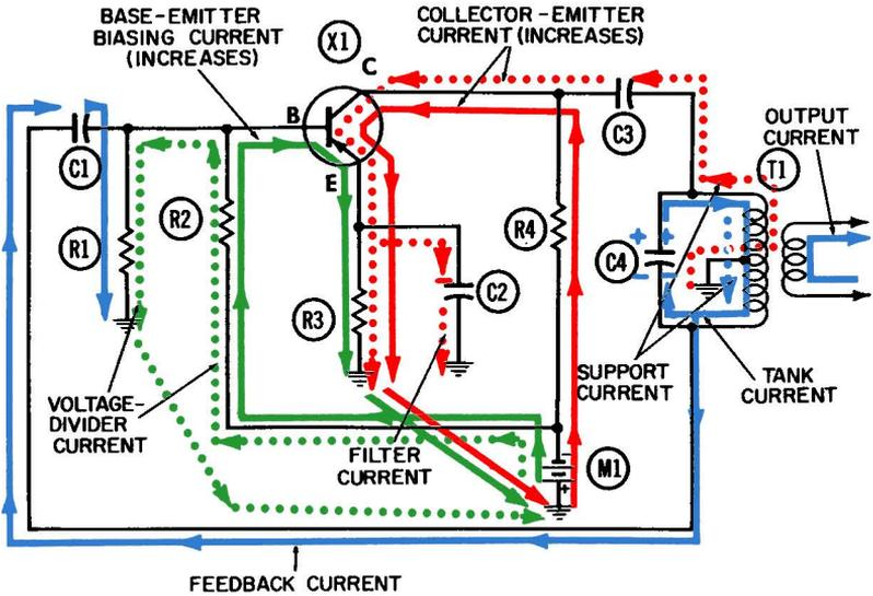
**Fig. 3-1. Operation of the Hartley oscillator—negative half-cycle.**
