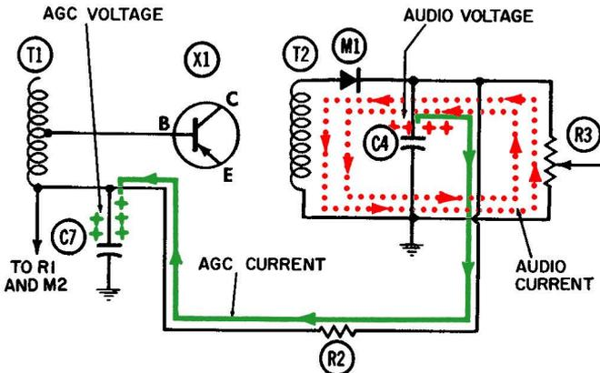
Fig. 5-8. AGC portion of the circuit in Figs. 5-4 and 5-5—modulating trough during a period of strong signal.
