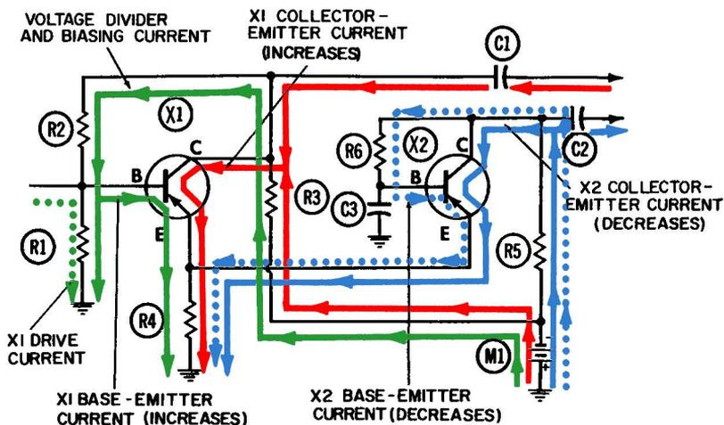
**Fig. 2-2.** Operation of a two-stage phase inverter using common-emitter and common-base configurations—negative half-cycle.
