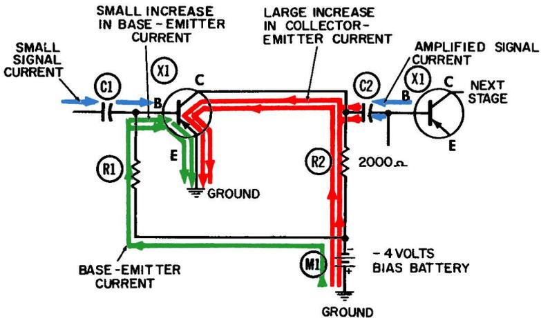
Fig. 1-12. A common-emitter PNP transistor circuit—negative half-cycle.
