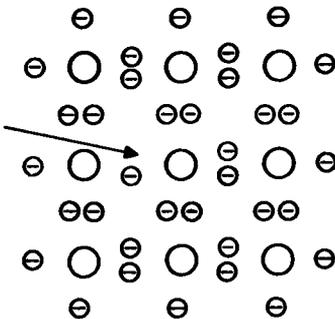
Fig. 1-2. A boron atom tied to four germanium atoms.
