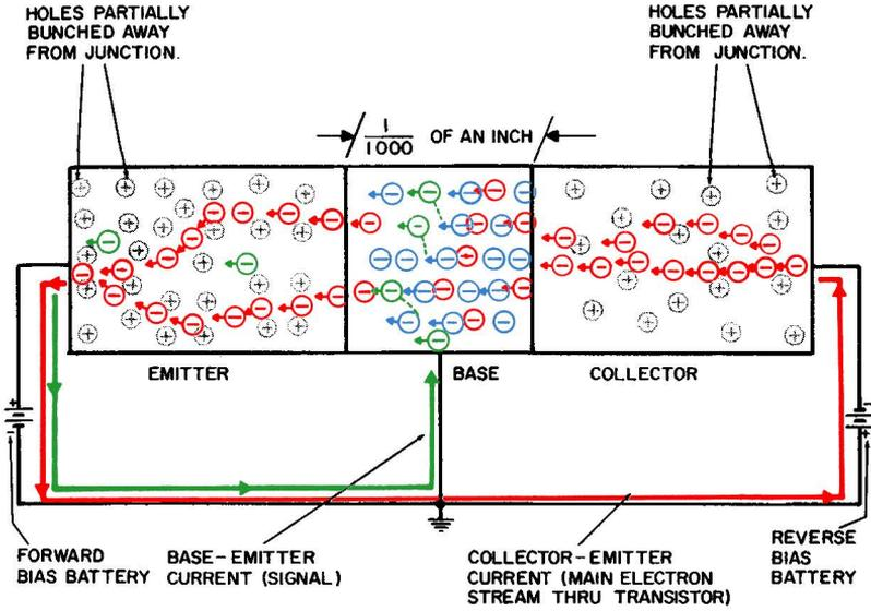
Fig. 1-8. The common-base PNP transistor circuit—no signal current.
