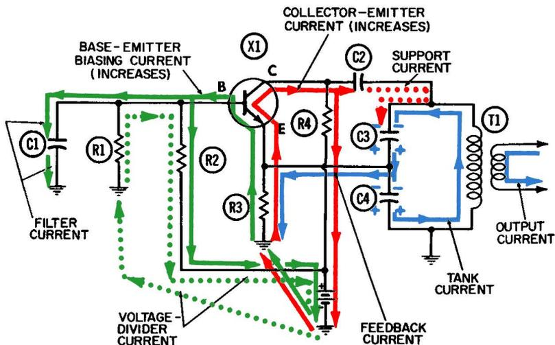
Fig. 3-3. Operation of the Colpitt's oscillator—negative half-cycle.
