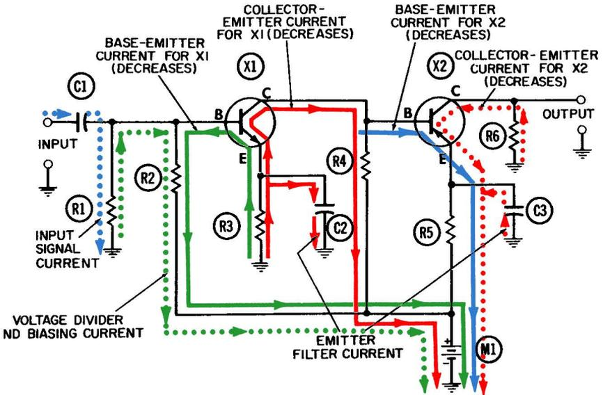
**Fig. 4-3. Operation of the direct-coupled amplifier—negative half-cycle.**
