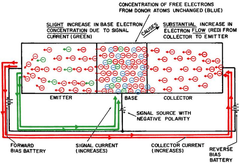
Fig. 1-9. The common-base PNP transistor circuit—negative half-cycle of operation.
