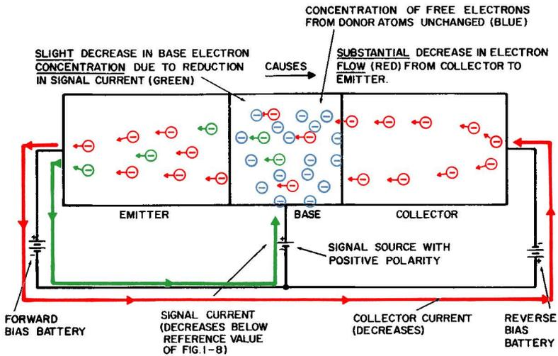
**Fig. 1-10. The common-base PNP transistor circuit—positive half-cycle of operation.**
