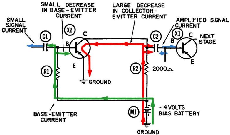
Fig. 1-13. A common-emitter PNP transistor circuit—positive half-cycle.
