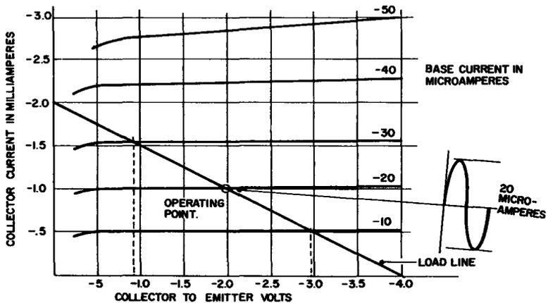
Fig. 1-11. Characteristic curve for a PNP transistor in a common-emitter configuration.
