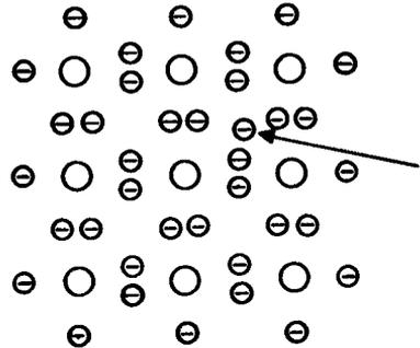
exist side by side in the same portion of the semiconductor without recombining. Although the total charge of this semiconductor will be zero (since the number of electrons released equals the number of positively charged donor atoms), the semiconductor becomes known as an N-type because of the availability of negative carriers (electrons). The positively charged donor atoms do not act as current carriers, and are not "holes."
