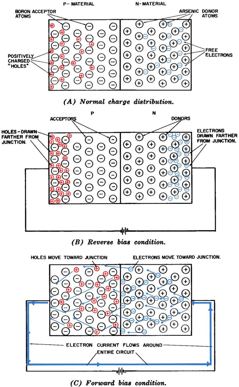
Fig. 1-4. The P-N junction under various bias conditions.
