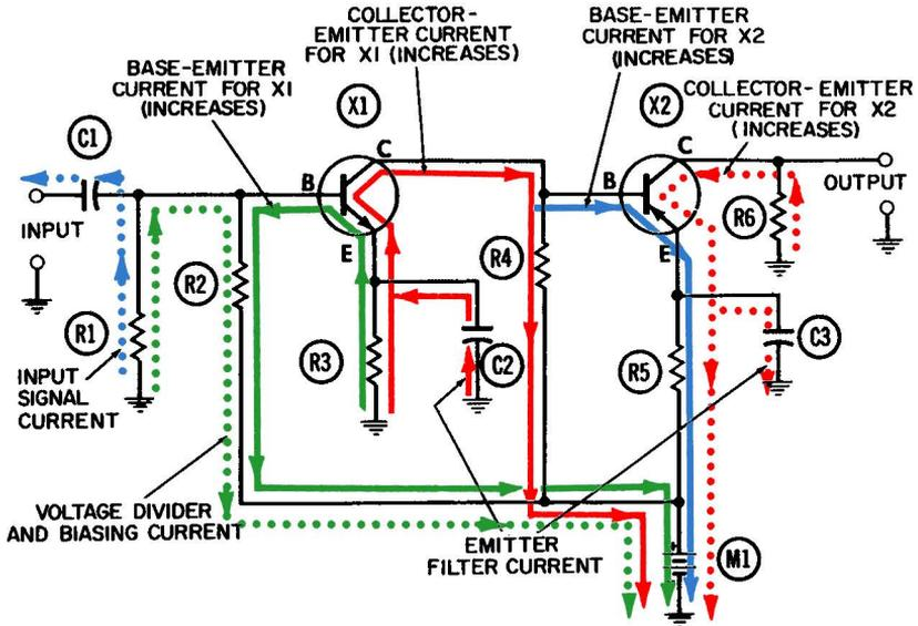
Fig. 4-4. Operation of the direct-coupled amplifier—positive half-cycle.
