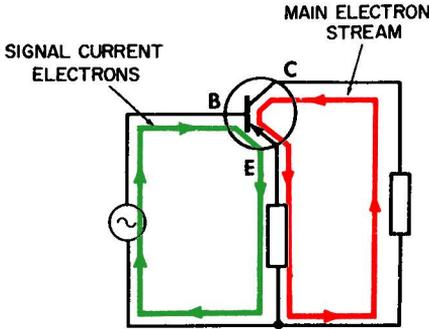
**Fig. 1-6. The PNP transistor, with external circuitry.**
