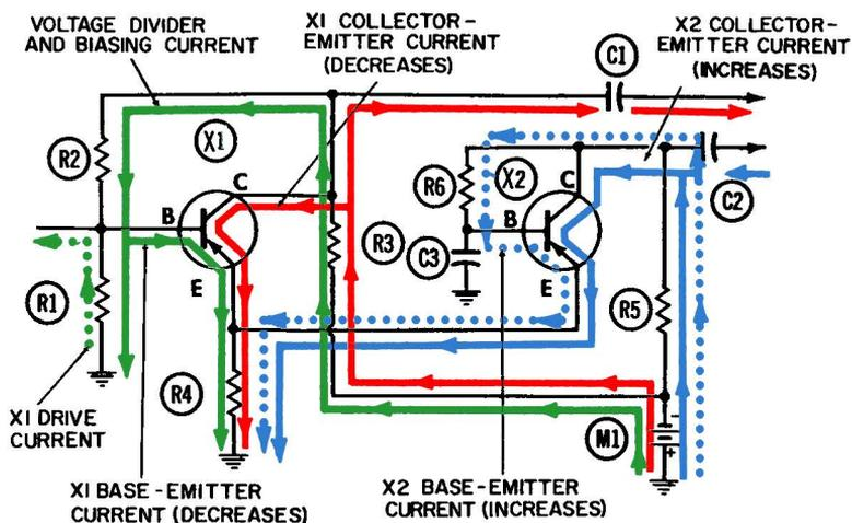
**Fig. 2-1.** Operation of a two-stage phase inverter using common-emitter and common-base configurations—positive half-cycle.
