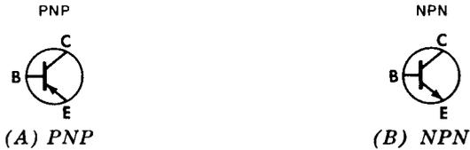
Fig. 1-5. Standard Schematic symbols.
