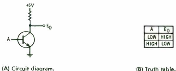
Fig. 1-6. Simple transistor inverter.
