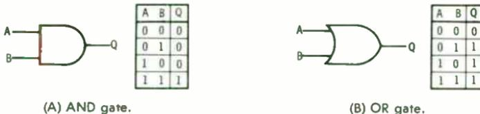
Fig. A-1. Basic logic gates and their truth tables.
