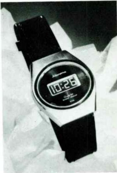
Fig. 8-6. A CMOS wristwatch.
