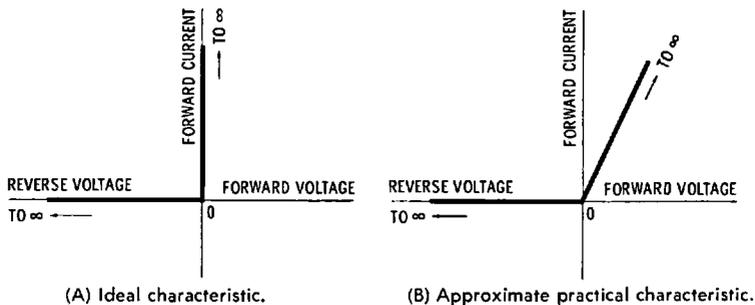
Fig. 9-8. Clamp characteristics.
