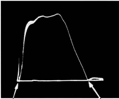
Fig. 5-14. Video-frequency response curve.
