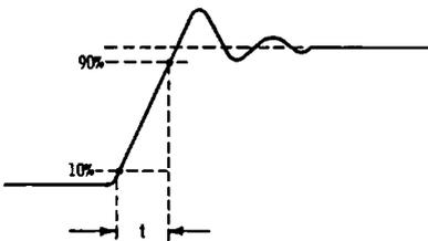
Fig. 3-11. Measurement of rise time  $t$ .
