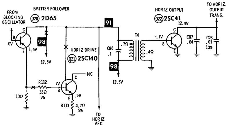
Fig. 6-14. Emitter follower used as an impedance-matching device.
