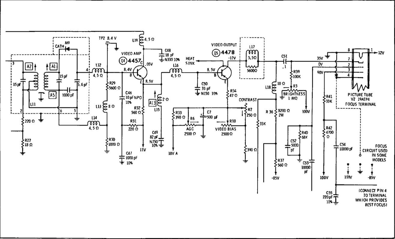
Fig. 7-8. Video-amplifier configuration.
