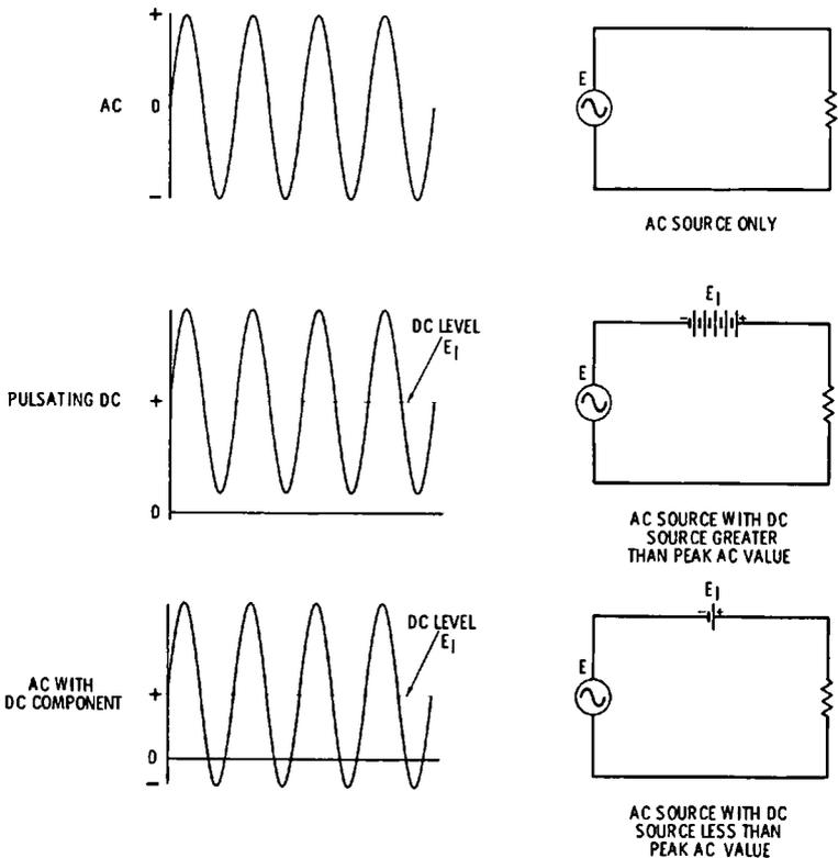
Fig. 1-13. Three basic combinations of ac and dc values.
