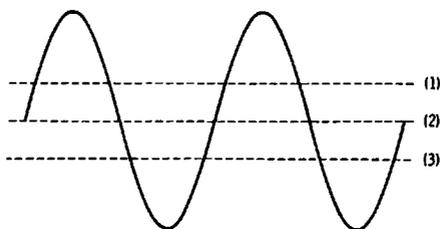
Fig. 6-4. Clipping of both positive and negative peaks.
