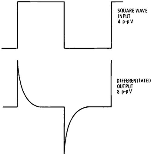
Fig. 3-4. Effect of differentiation on square wave.
