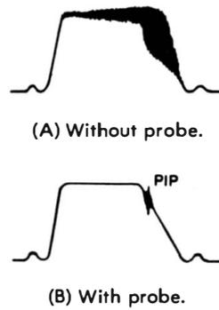
**Fig. 1-7. The effect of a resistive isolation probe on the sharpness of the marker pip.**
