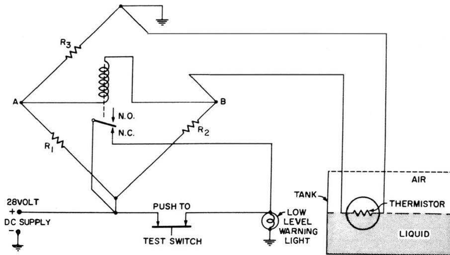
**Fig. 7-79. Simplified schematic of the instrument in Fig. 7-78.** (Courtesy of Simmonds Aerocessories, Inc.)
