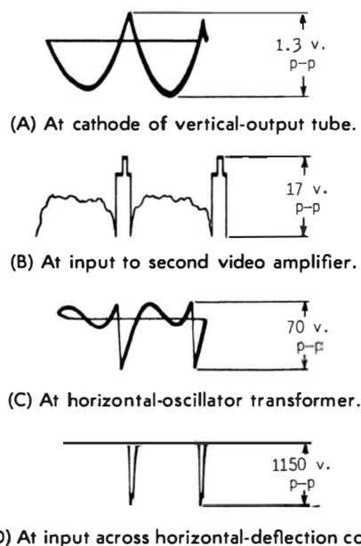
**Fig. 4-14. Typical nonsymmetrical nonsinusoidal voltages encountered in TV receivers.**
