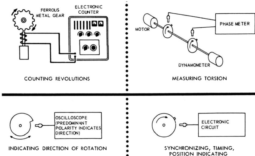
**Fig. 7-47. Possible applications for a magnetic proximity pickup probe.** (Courtesy of Electro Products Laboratories, Inc.)
