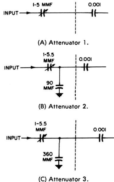
**Fig. 3-15. Attenuators used with the cathode-follower probe in Fig. 3-14.**
