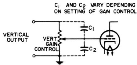
**Fig. 3-11. High-impedance uncompensated gain-control circuit used in some oscilloscopes.**
