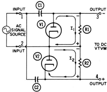
**Fig. 4-39. A symmetrical voltage-doubler circuit.**
