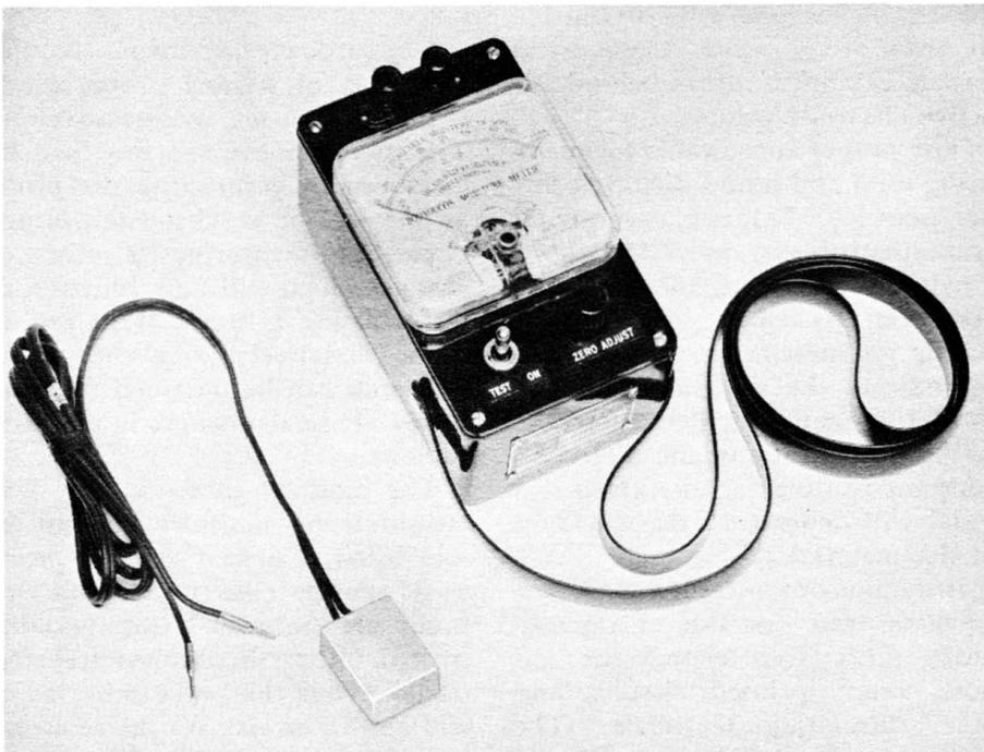
**Fig. 7-82. Instrument used for measuring moisture content of soil.**
