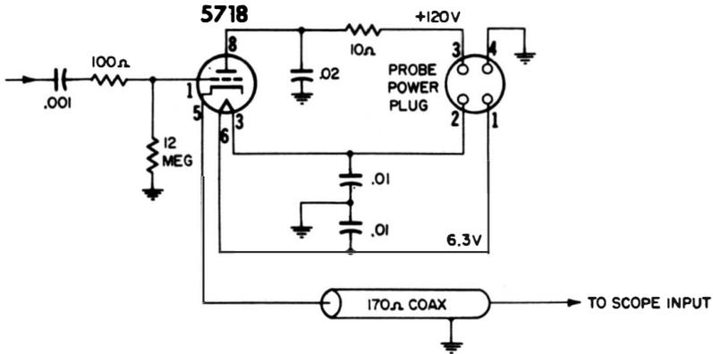
**Fig. 3-14. Schematic of the Tektronix P170-CF cathode-follower probe.**
