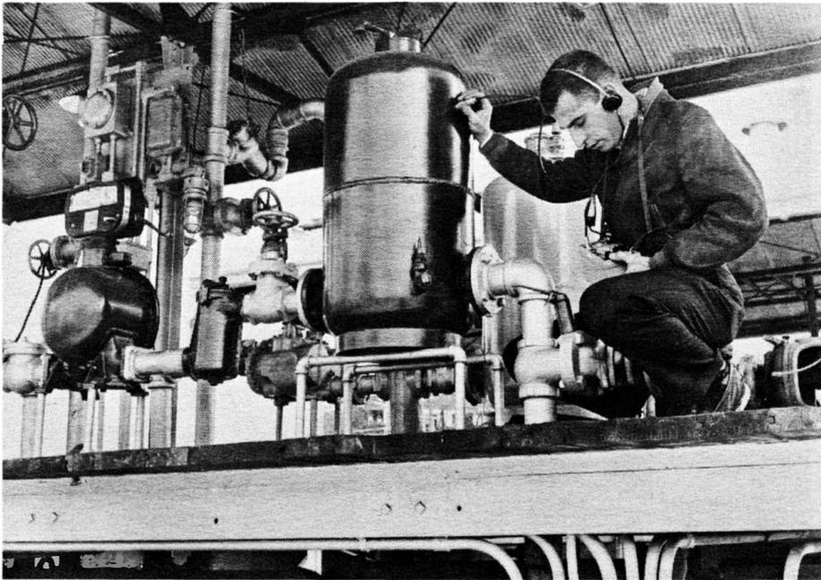
**Fig. 7-53. Ultrasonic thickness tester in use.** (Courtesy of Branson Instruments, Inc.)
