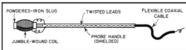
**Fig. 7-28. Hum field-tracing probe.**
