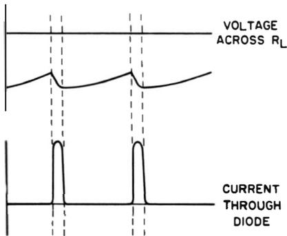
**Fig. 4-9.** Current pulses through diode after several cycles of input signal have passed.
