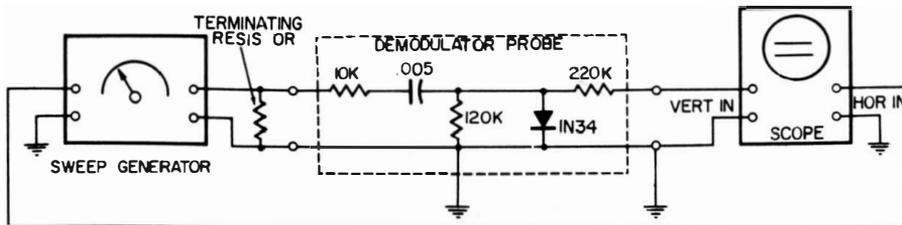
**Fig. 5-19. Equipment setup for testing flatness and linearity of sweep-generator output.**
