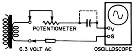
(B) Place potentiometer in series with scope vertical-input lead.
