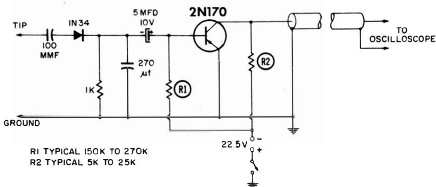
**Fig. 6-9. Single-transistor demodulator signal-tracer probe.**
