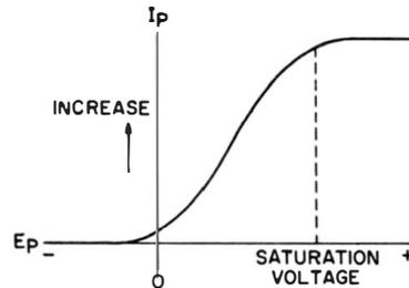
**Fig. 4-5. Typical plate-voltage and -current characteristics of a vacuum-tube diode.**
