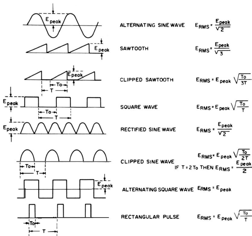
Fig. 4-37. Relationship between the peak and rms values of various waveforms.
