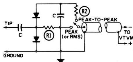
**Fig. 4-41. Circuit of a combination peak and peak-to-peak probe using semiconductor diodes.**
