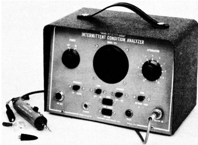
**Fig. 7-34. Intermittent-condition analyzer with intermittent probe.**
