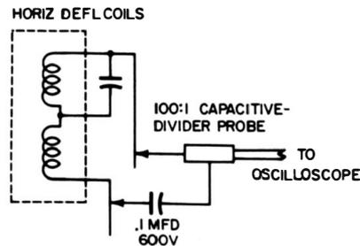
(C) Capacitor in series with ground lead of probe.
