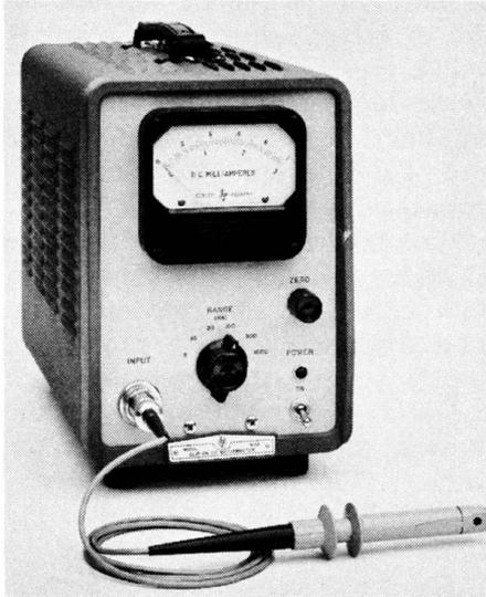
**Fig. 7-1. Clip-on probe used for direct-current measurements.** (Courtesy of Hewlett-Packard Co.)
