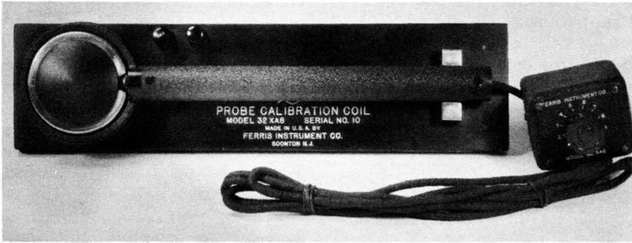
**Fig. 7-16. Loop exploring and calibration probe.** (Courtesy of Ferris Instrument Co.)
