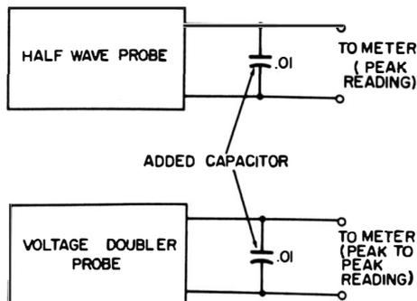
**Fig. 5-28. Converting demodulator probes for use with meters.**
