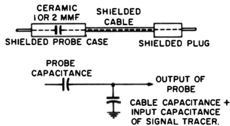
Fig. 6-12. Capacitance-type signal-tracer probe and equivalent circuit.
