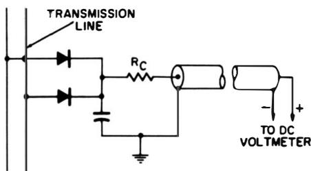
**Fig. 4-36. A probe suitable for measuring in a balanced circuit.**
