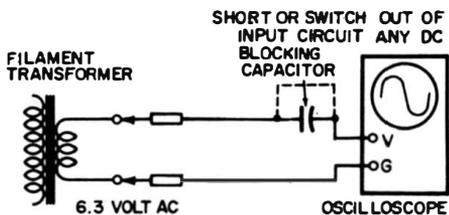
(A) Short DC blocking capacitor (if used) and connect signal source to scope.
