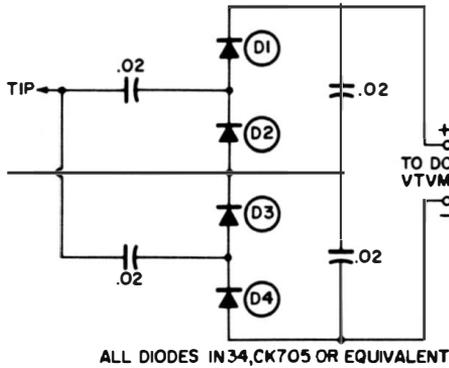
Fig. 4-44. A voltage-quadrupler circuit.
