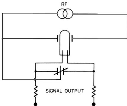
**Fig. 7-49. Basic circuit of capacity-sensitive probe. (Courtesy of The Decker Corp.)**
