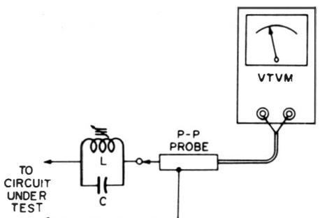
(A) Circuit for rejecting the horizontal-sync pulses.
