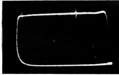
(A) Generator with flat output. Markers at 41.25 and 47.25 mc.
