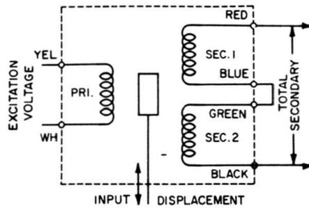
**Fig. 7-44. Schematic of the probe in Fig. 7-43.** (Courtesy of Sanborn Co.)
