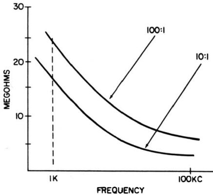
**Fig. 2-12.** Shunting impedance of a typical 100:1 capacitive-divider HV probe and a 10:1 low-capacitance probe.
