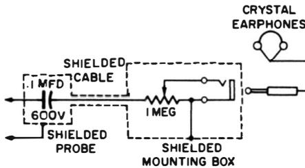
Fig. 6-11. AF signal-tracer probe with volume control.
