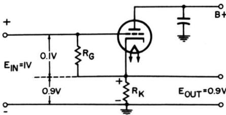
(B) Grid resistor connected to cathode.
