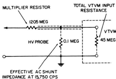
(B) Equivalent circuit of probe for 15,750-cps pulses.
