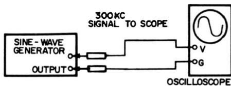
(A) Apply a 300-kc sine wave to vertical input of oscilloscope.
