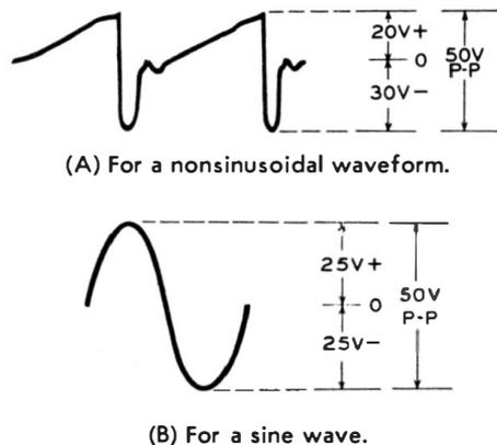
Fig. 4-45. The relationship between peak and peak-to-peak values of waveforms.
