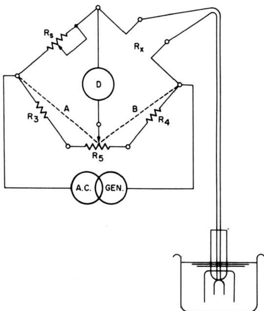
**Fig. 7-84. AC Wheatstone bridge used with conductivity probe.** (Courtesy of Industrial Instruments, Inc.)
