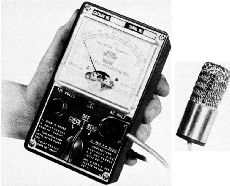
Fig. 7-83. Hygrometer and probe. (Courtesy of Labline, Inc.)
