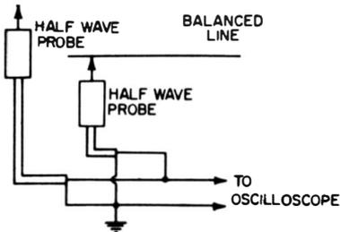
Fig. 5-11. Two identical half-wave probes used to make measurements on a balanced line.
