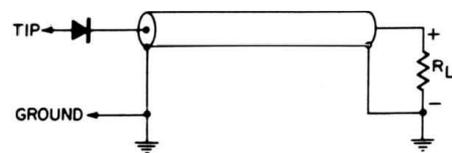
Fig. 4-32. Basic circuit of a peak-reading, series-type rectifier probe.
