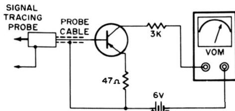
**Fig. 6-8. Transistor amplifier for signal-tracing probe.**
