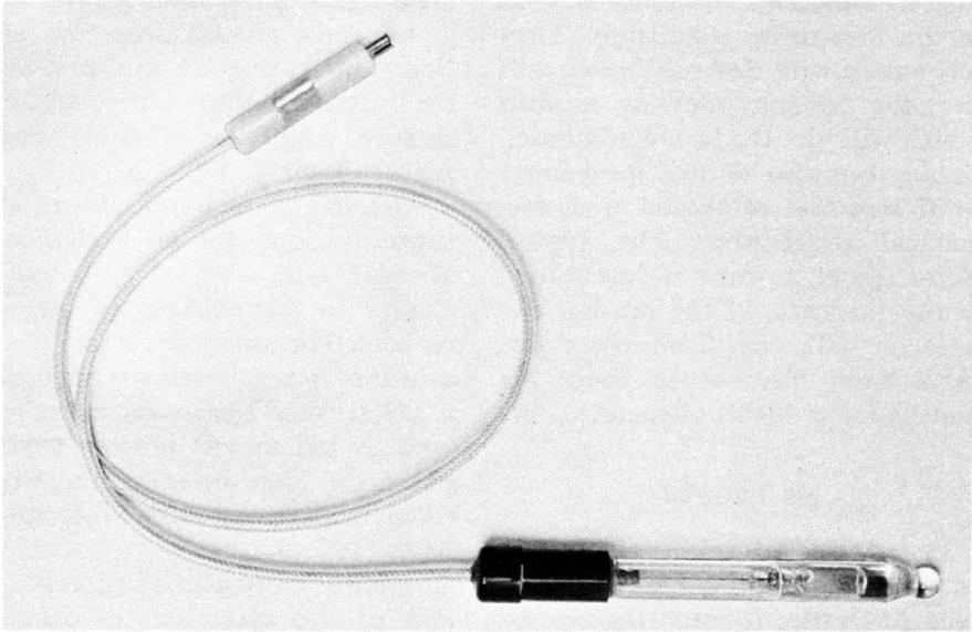
**Fig. 7-74. Typical probe used for pH measurements.** (Courtesy of Leeds and Northrup Co.)
