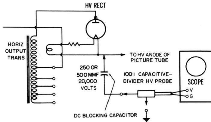
**Fig. 2-11. Connections for checking the waveform and peak-to-peak voltage in a TV high-voltage supply when a capacitive-divider HV probe is used.**
