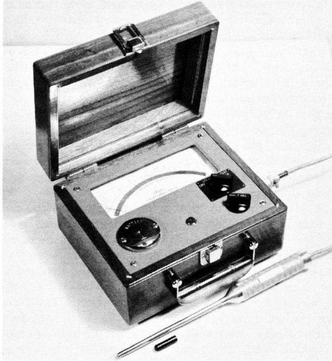
**Fig. 7-70. Thermoanemometer with thermocouple probe.** (Courtesy of Illinois Testing Laboratories, Inc.)
