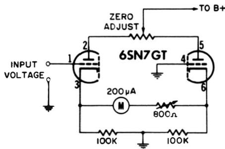
Fig. 4-1. Basic circuit of a vacuum-tube voltmeter.
