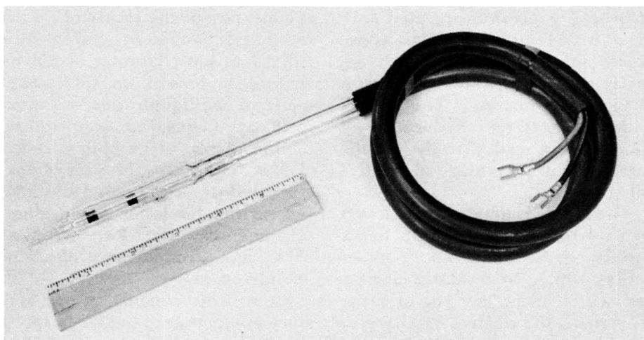
**Fig. 7-85. Conductivity probe.** (Courtesy of Industrial Instruments, Inc.)
