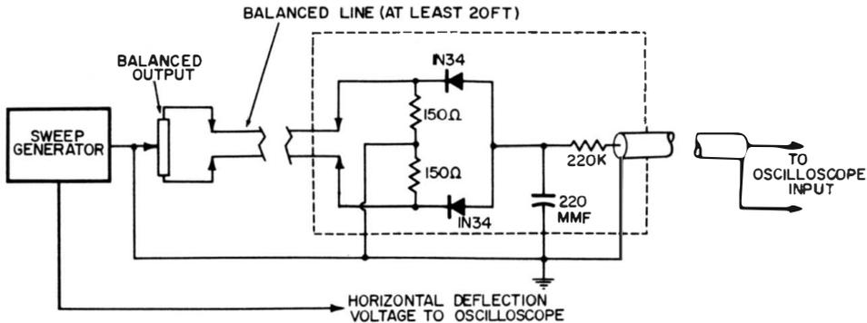
**Fig. 5-22. How to check the characteristic impedance of a balanced line.**
