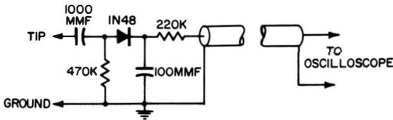
**Fig. 5-7. Series demodulator probe available in kit form (Eico Model PSD).**
