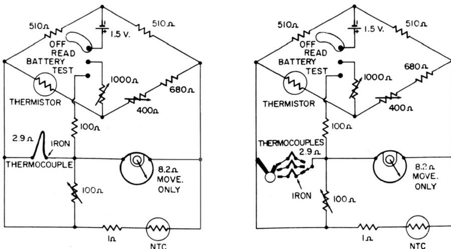
**Fig. 7-41. Schematic of probe and meter in Fig. 7-40.**
