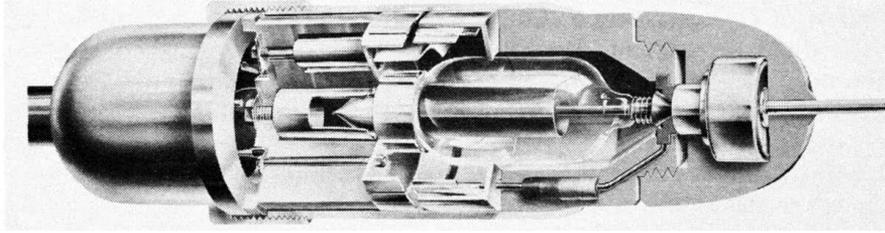
**Fig. 4-19. Internal view of the Hewlett-Packard high-frequency probe used with the Model 410-B VTVM. (Courtesy of Hewlett-Packard Co.)**
