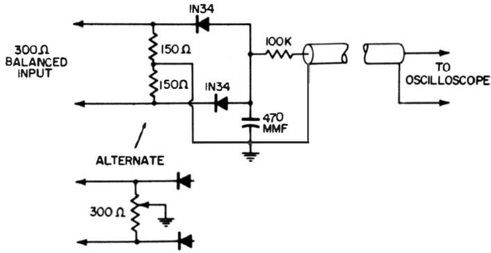
Fig. 5-10. Balanced demodulator probe having 300-ohm input.
