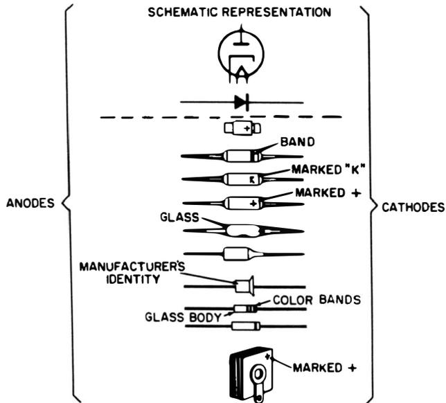
Fig. 4-6. Representations of vacuum-tube, germanium, silicon, and selenium diodes.
