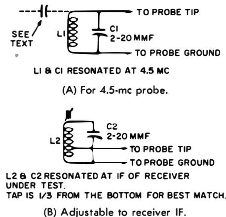
**Fig. 6-14. Tuned heads for signal-tracer probes.**
