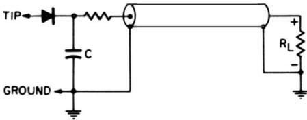
**Fig. 4-33.** Adding a charging capacitor and a resistor to the basic circuit will improve its performance.
