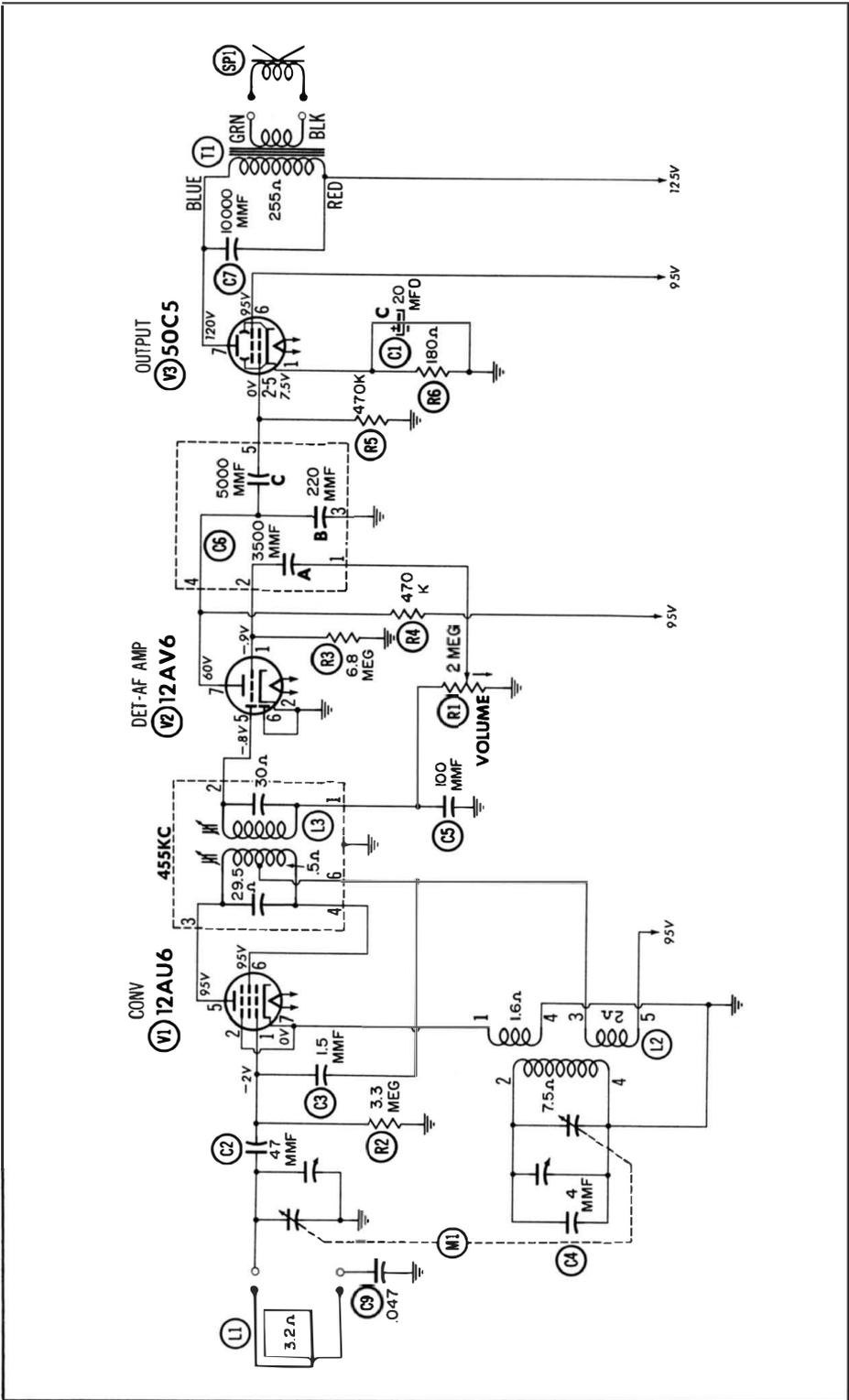
Fig. 6-1. Schematic of a typical superheterodyne receiver.
