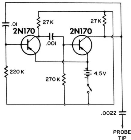
Fig. 6-18. Transistorized signal-injector probe.
