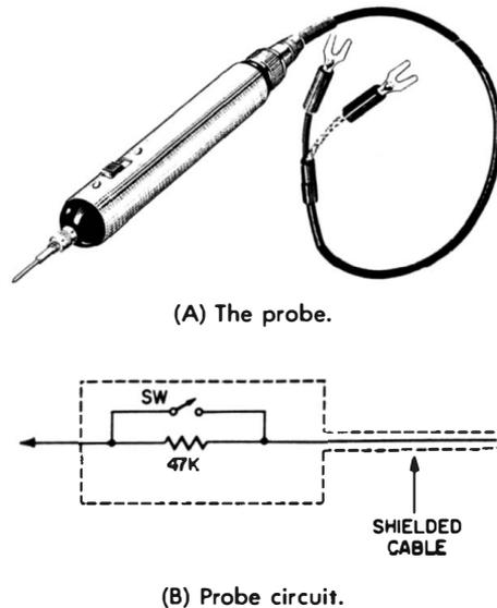
**Fig. 1-8. A combination direct-isolation probe for use with an oscilloscope. (Courtesy of Scala Radio Co.)**
