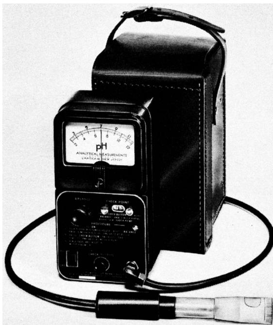
**Fig. 7-76. pH meter with combination probe.** (Courtesy of Analytical Measurements, Inc.)
