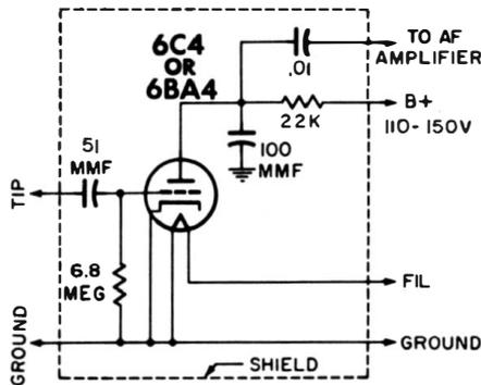
Fig. 6-15. Signal-tracing probe using grid-leak detection.
