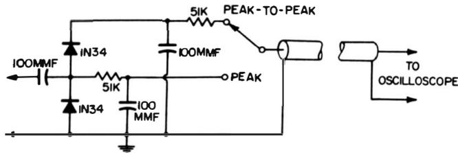
Fig. 5-15. Combination peak and peak-to-peak reading demodulator probe.
