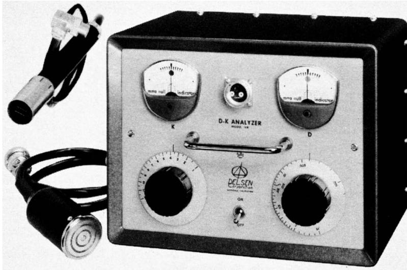
**Fig. 7-80. Dielectric constant and dissipation-factor analyzer with two probes.** (Courtesy of Delsen Corp.)
