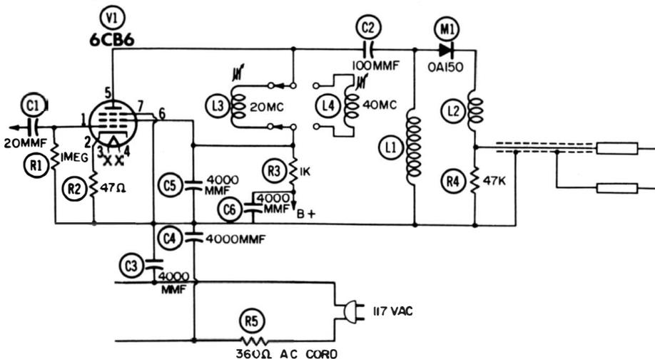
Fig. 5-16. Tuned high-gain RF demodulator probe (Doss D-200).
