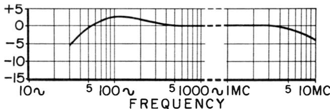
**Fig. 7-5. Frequency response of the clip-on probe and amplifier in Fig. 7-3.** (Courtesy of Hewlett-Packard Co.)
