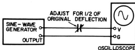
(B) Place an adjustable capacitor in series with scope vertical-input lead.
