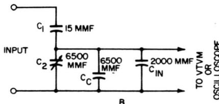
C<sub>1</sub> = INTERELECTRODE CAPACITY OF HV TUBE
