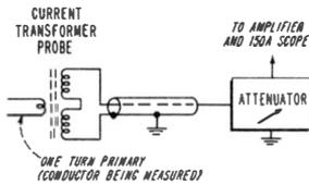
**Fig. 7-4. Basic schematic of the clip-on probe in Fig. 7-3.** (Courtesy of Hewlett-Packard Co.)
