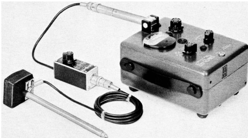
Fig. 7-60. Vibration pickup probe with control box and indicating meter. (Courtesy of General Radio Co.)
