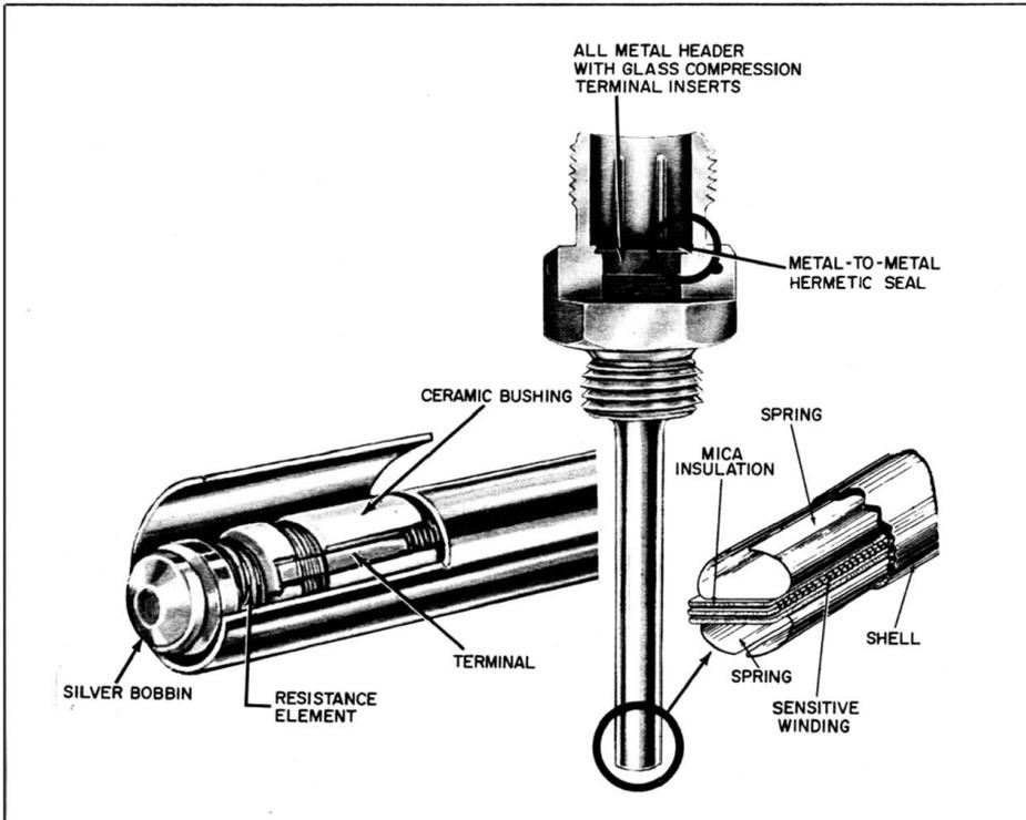
**Fig. 7-36. Temperature-sensing probes, showing tip-sensitive and stem-sensitive construction.** (Courtesy of Thomas A. Edison Industries.)
