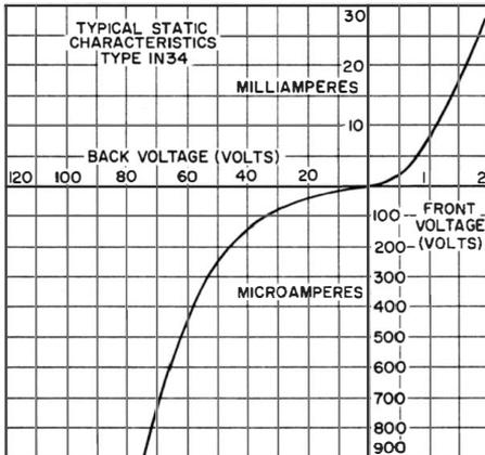
Fig. 4-7. Static characteristics of the 1N34 germanium diode. (Courtesy of Sylvania Electric Products, Inc.)
