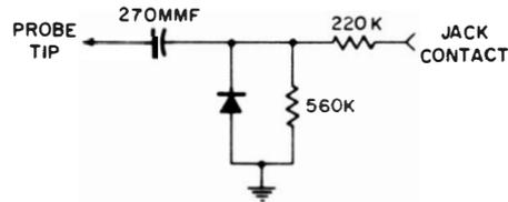
**Fig. 6-5. Schematic of RCA WG-302A signal-tracing probe.**
