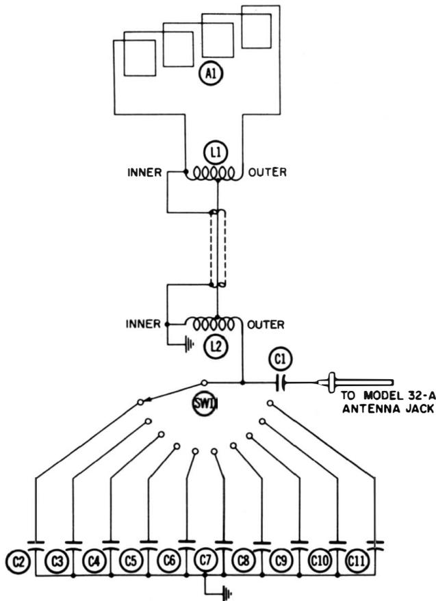
**Fig. 7-17 Schematic of the probe and coupling unit in Fig. 7-16.** (Courtesy of Ferris Instrument Co.)
