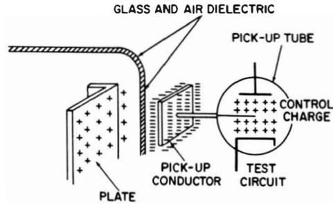
(A) Principle of electrostatic induction.
