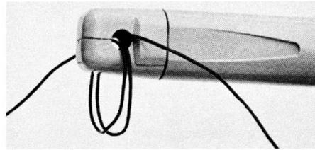
**Fig. 7-2. Clip-on probe showing method of increasing pickup sensitivity.** (Courtesy of Hewlett-Packard Co.)
