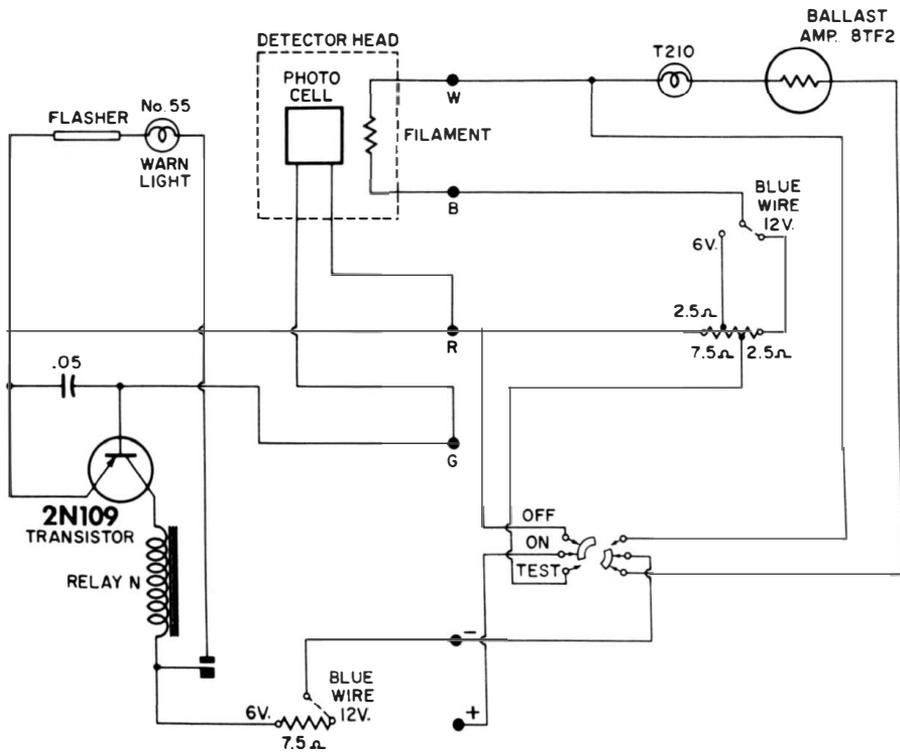
Fig. 7-63. Schematic of automatic gas detector.
