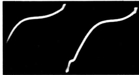
(A) Waveform without the probe.
