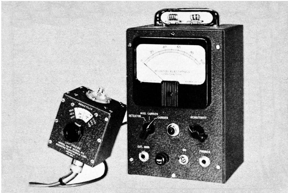
Fig. 7-24. Grid-dip meter with UHF probe in place. (Courtesy of Boonton Electronics Corp.)
