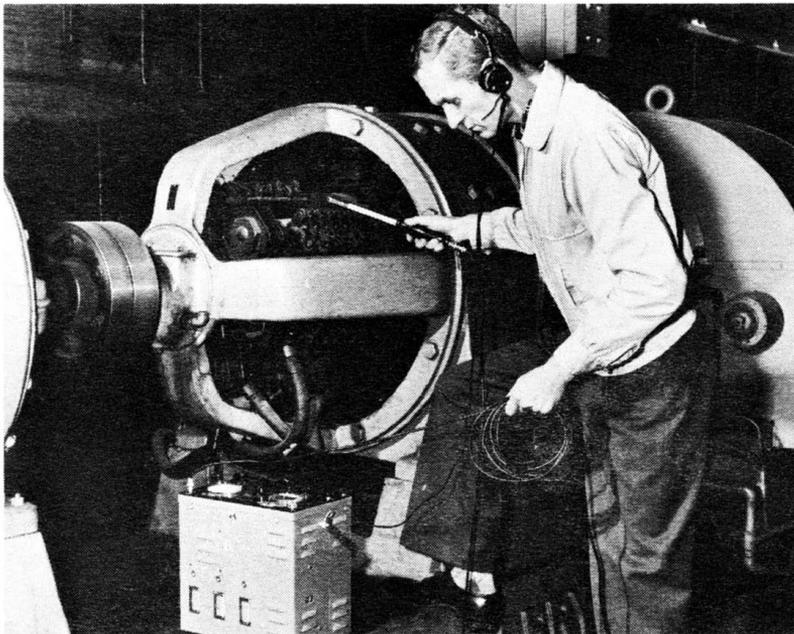
**Fig. 7-15.** Radio-interference locating probe in use. (Courtesy of Sprague Electric Co.)
