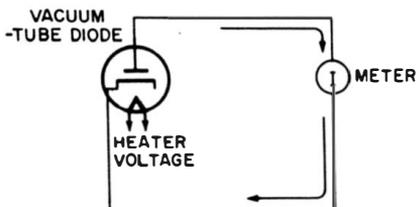
**Fig. 4-3. A small current will flow in a diode circuit with only heater voltage applied.**
