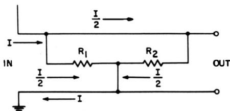
**Fig. 7-26. Current flow in the resistance element of the probe in Fig. 7-25.**
