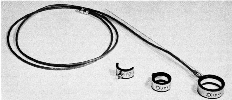
Fig. 7-11. Three forms of electrostatic pickup probes. (Courtesy of Kingston Electronics Corp.)
