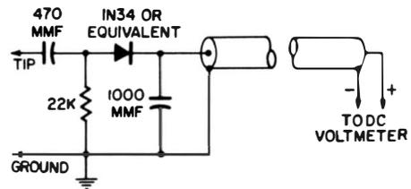
**Fig. 4-35.** A rectifier probe suitable for a VOM with a sensitivity of 5,000 ohms per volt or higher.
