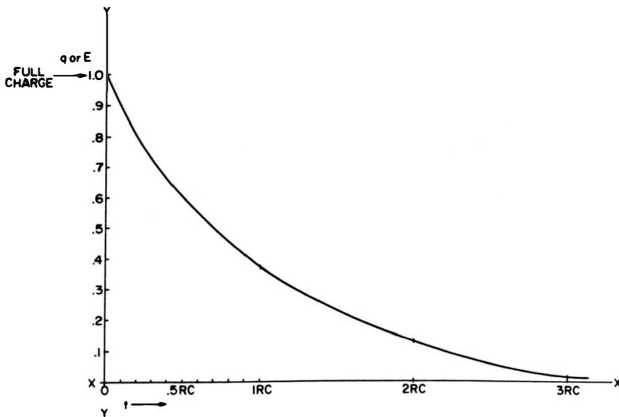
Fig. 4-11. Discharge curve for an RC circuit.
