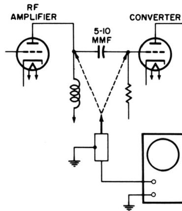
**Fig. 6-2. Signal tracing in an RF-converter stage.**
