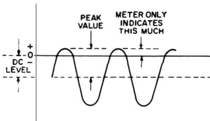
**Fig. 4-34.** Measuring error introduced when AC is measured in a circuit that also contains DC and no DC blocking capacitor is used.
