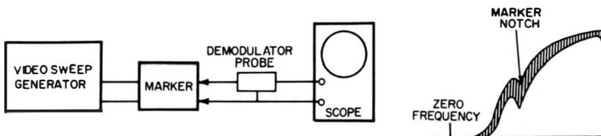
**Fig. 5-26. How to check the frequency-demodulation limit of a probe.**
