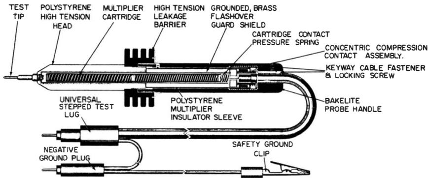
Fig. 2-1. Internal construction of a high-voltage probe.
