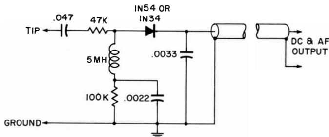
Fig. 6-6. AF-IF-RF signal-tracing probe.
