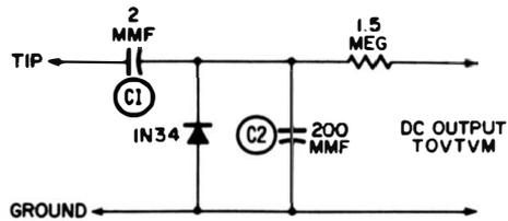
**Fig. 4-25.** Capacitive-divider method of increasing the voltage-handling capability of a probe.
