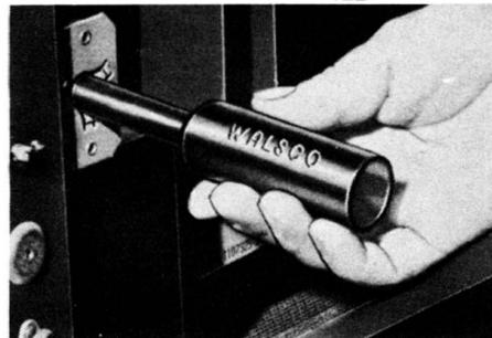
**Fig. 2-14. A color TV interlock "cheater" permits HV measurements with the back removed. (Courtesy of Walsco Electronics Manufacturing Co.)**
