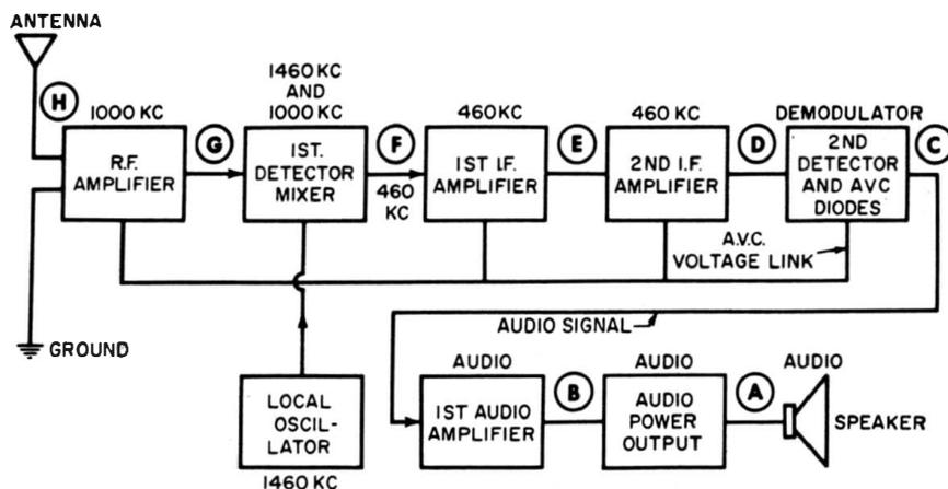
Fig. 6-16. Block diagram of a typical superheterodyne receiver.
