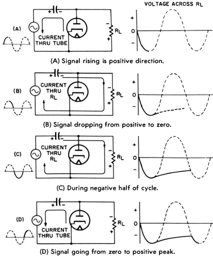
Fig. 4-8. Operation of a shunt-type rectifier.
