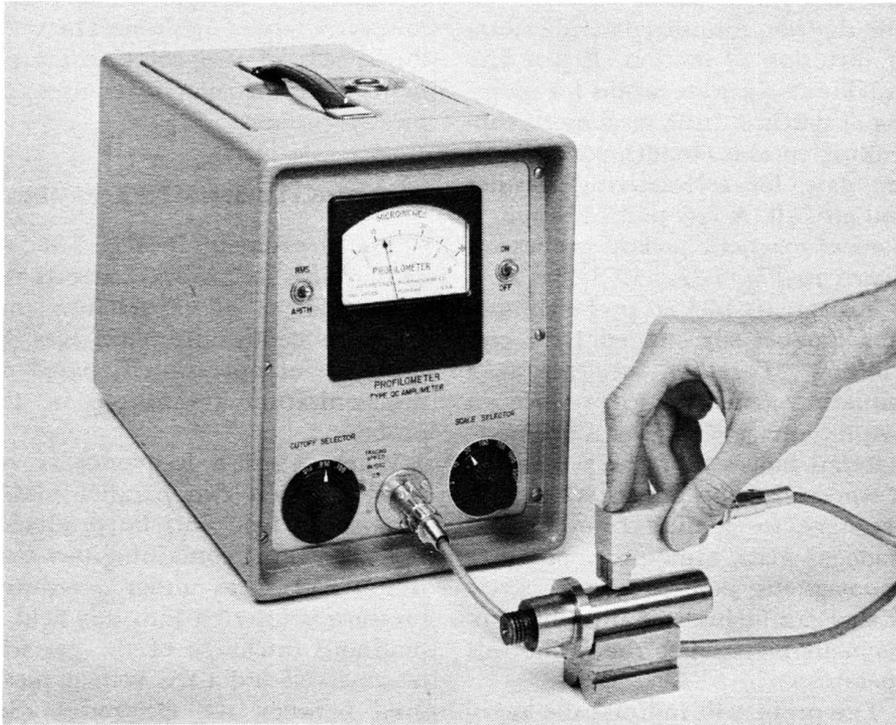
**Fig. 7-46.** Probe used for determining the "profile" of a smooth surface. (Courtesy of Micrometrical Manufacturing Co.)
