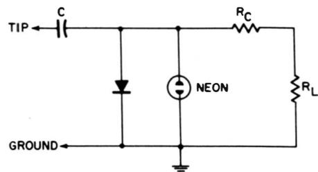
**Fig. 4-26.** Using a neon bulb to protect the diode against damage from voltage overloads.
