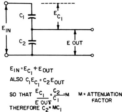
**Fig. 2-7. Basic capacitive-divider HV probe circuit, showing how voltage division is accomplished.**
