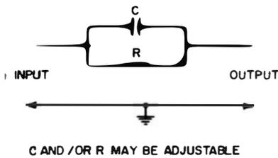
Fig. 3-2. Basic circuit of a low-capacitance probe.
