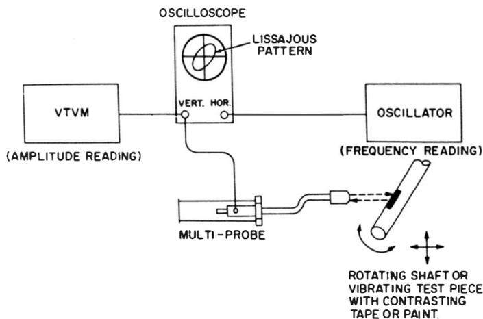
**Fig. 7-88. Application of optical tachometer probe.** (Courtesy of Optomechanism.)
