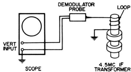
**Fig. 5-24.** How to check the 60-cycle sync-buzz voltage in a receiver.
