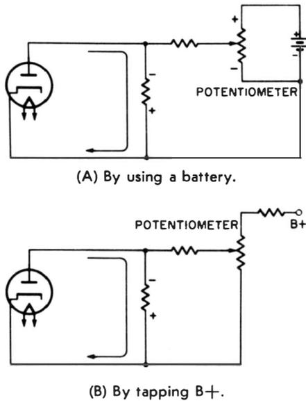
**Fig. 4-4. Two ways of obtaining a bucking potential.**
