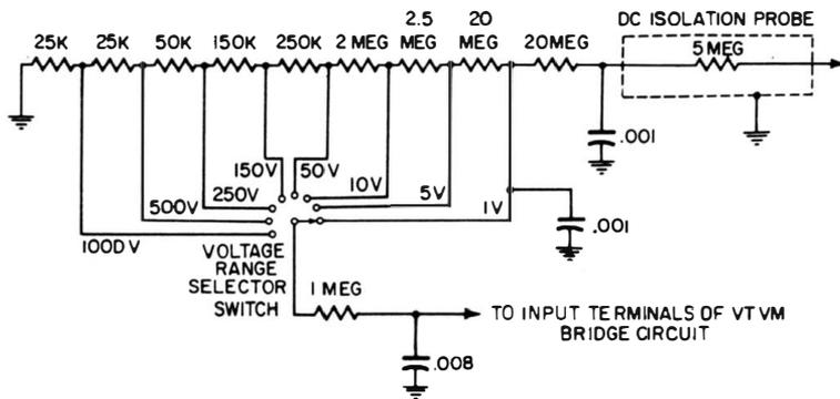
Fig. 2-3. Simplified input circuit of a typical VTVM.
