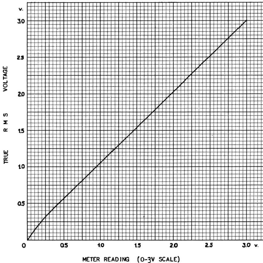
Fig. 4-30. Correction chart for the three-volt range of a VTVM when the probe in Fig. 4-29 is used. (Courtesy of Precision Apparatus Co.)
