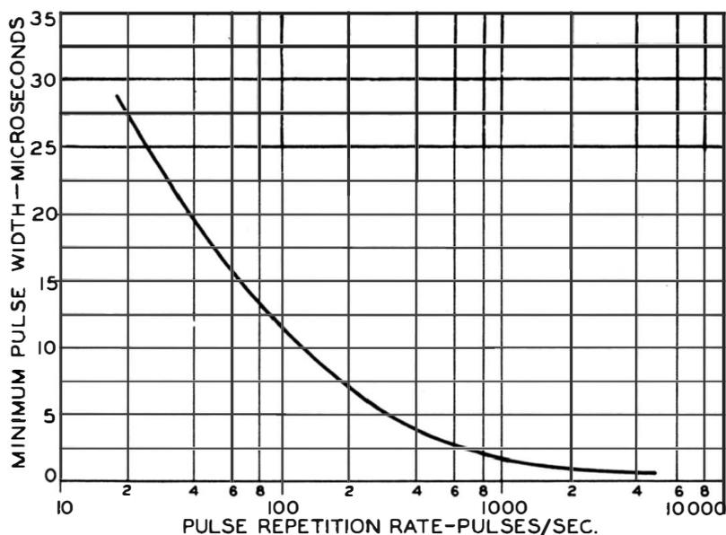
Fig. 4-15. Pulse-response capabilities of a typical VTVM. (Courtesy of Radio Corporation of America)
