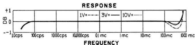
**Fig. 4-20. Frequency response of the probe in Fig. 4-19. (Courtesy of Hewlett-Packard Co.)**
