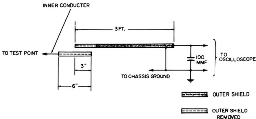
Fig. 2-10. A simple capacitive-divider HV probe can be made from two lengths of coaxial cable.
