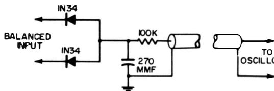
Fig. 5-12. Balanced high-impedance probe.
