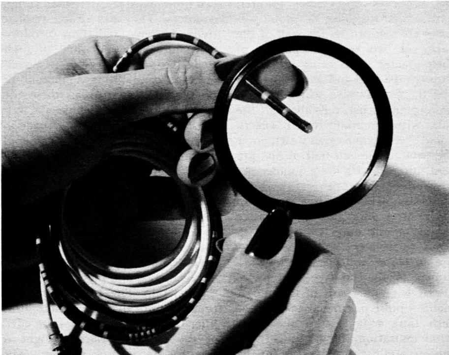
Fig. 7-91. Gastrointestinal probe. (Courtesy of Gulton Industries, Inc.)
