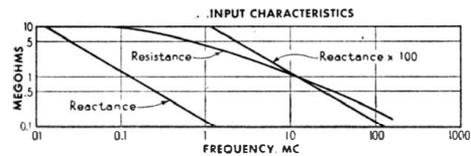
**Fig. 4-21. Input characteristics of the probe in Fig. 4-19. (Courtesy of Hewlett-Packard Company.)**
