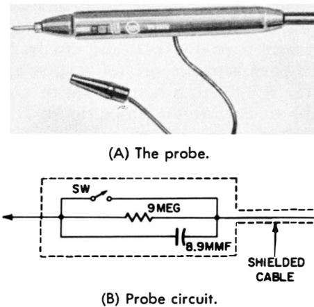
**Fig. 1-5. A combination direct-low-capacitance probe.** (Courtesy of Radio Corporation of America.)
