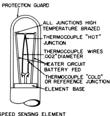
**Fig. 7-71. Construction of probe used with thermoanemometer.**
