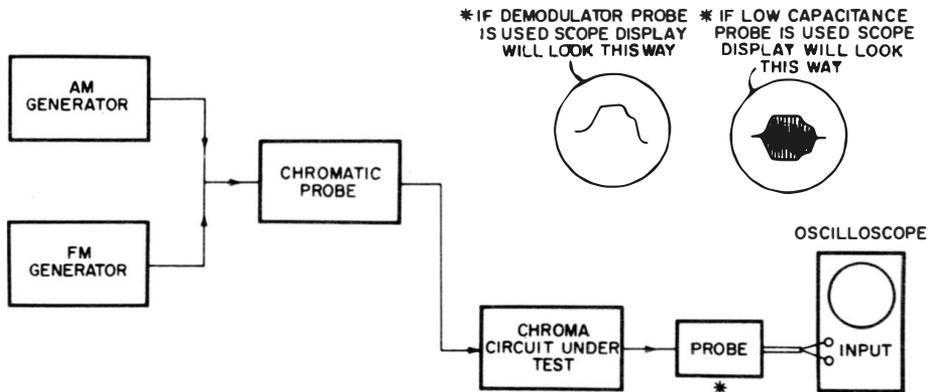
Fig. 7-30. Typical test setup for chromatic probe.
