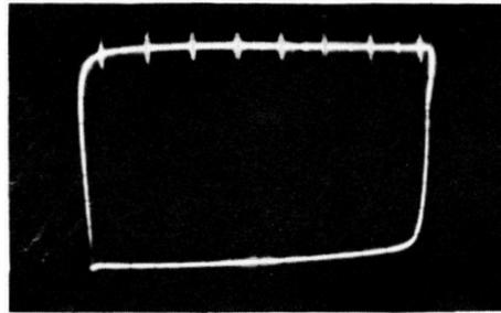
(C) Space between markers is 1.5 mc. Equal spacing indicates linear output from generator.
