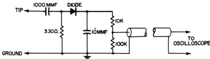
**Fig. 5-8. Probe recommended for TV receiver alignment.**
