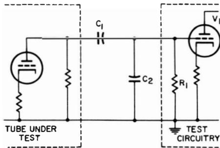
(C) Equivalent circuit for capacitive coupling with shield.
