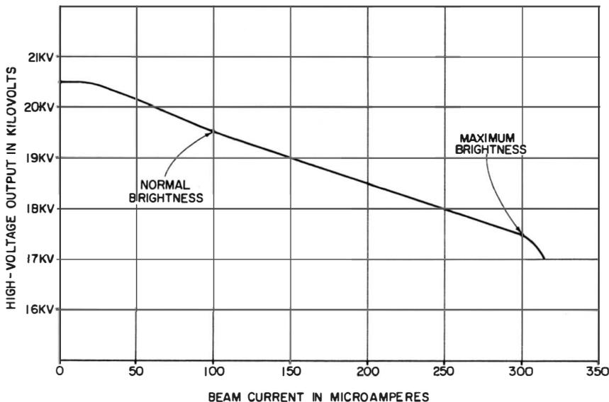
Fig. 2-4. Output voltage versus load current of a typical TV high-voltage supply.
