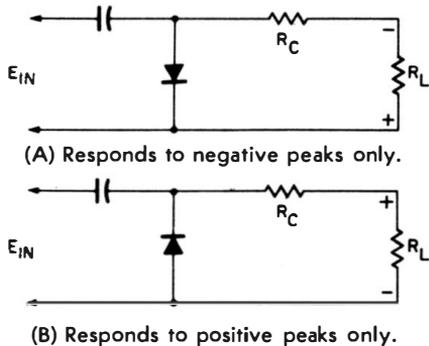
Fig. 4-22. Shunt-type peak-reading rectifier probes using germanium diodes.
