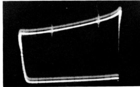
(B) Output from a second generator. Markers at 41.25 and 47.25 mc. Output is acceptable for all practical purposes.
