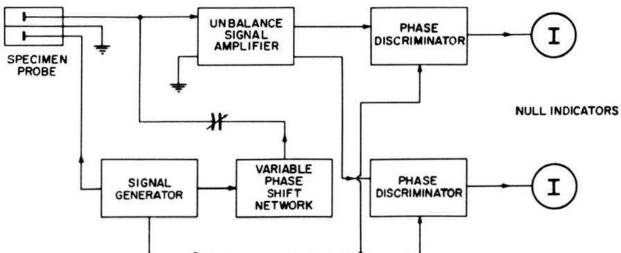
**Fig. 7-81. Functional block diagram of instrument in Fig. 7-80.**
