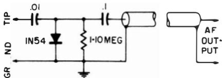
**Fig. 6-4. AF-RF signal-tracer probe for use with headphones or AF amplifier. RF signals must be modulated.**
