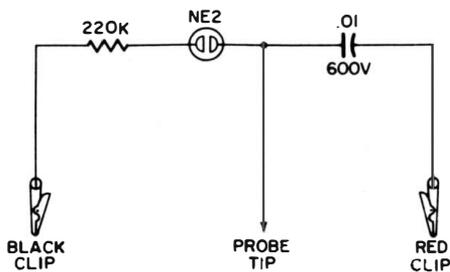
Fig. 7-33. Schematic of Probe-Master.
