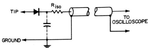
Fig. 5-4. Basic schematic of a series demodulator probe.
