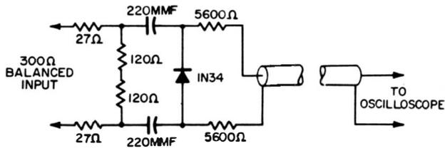
**Fig. 5-13. Balanced 300-ohm probe using only one semiconductor diode.**
