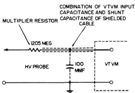
(A) Effective shunt capacitance for the DC measurement.
