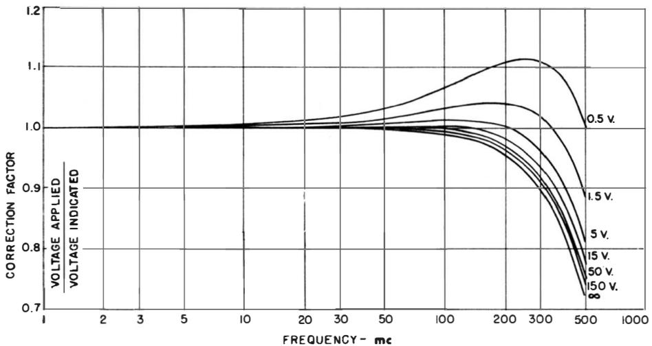
**Fig. 4-18. Frequency-correction curve for the probe in Fig. 4-17.** (Courtesy of General Radio Company.)
