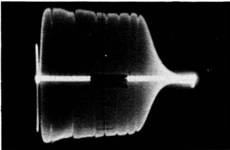
**Fig. 5-17. Video-amplifier output, showing response to a video-frequency sweep signal.**
