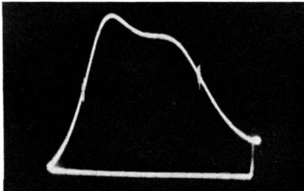
**Fig. 5-18. Typical response curve of a tuned circuit.**
