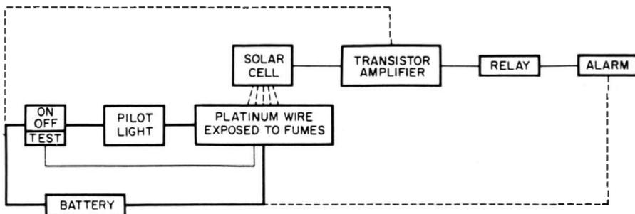
Fig. 7-64. Block diagram of the vapor detector in Fig. 7-62. (Courtesy of Raytheon Manufacturing Co.)
