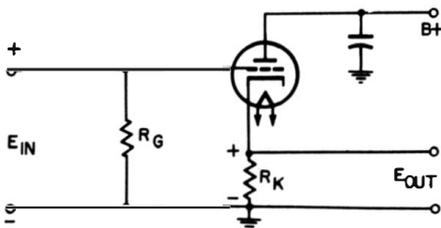
(A) Grid resistor connected to ground.
