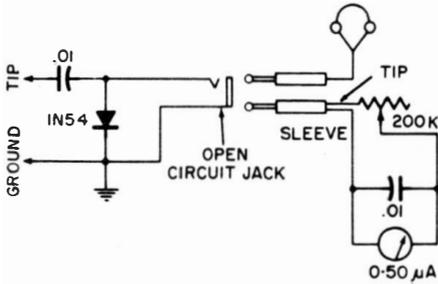
**Fig. 6-3. AF-RF signal-tracer probe giving both visual and aural indication.**
