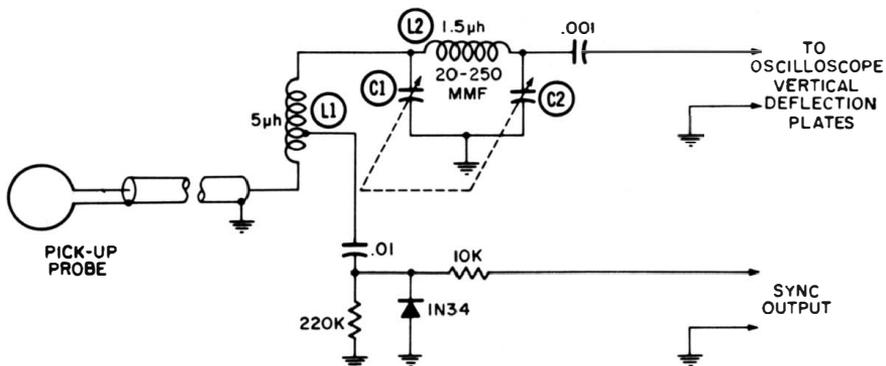
Fig. 7-19. Schematic of Q probe in Fig. 7-18.
