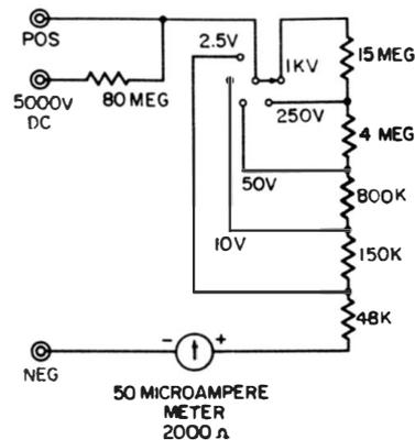
Fig. 2-2. Simplified DC input circuit of a typical VOM.
