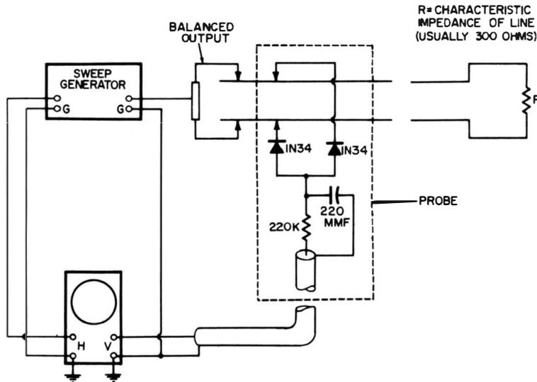
**Fig. 5-23.** Another way to check the characteristic impedance of a balanced line. (Generator and oscilloscope on the same side of line.)
