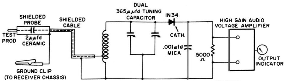
Fig. 6-13. Tuned signal tracer (Courtesy of Sylvania Electric Products, Inc.)
