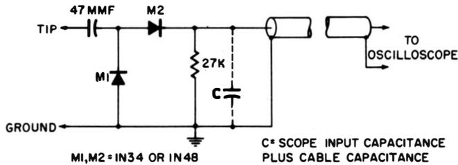
**Fig. 6-7. High-frequency signal-tracer probe — Voltage-doubler type.**
