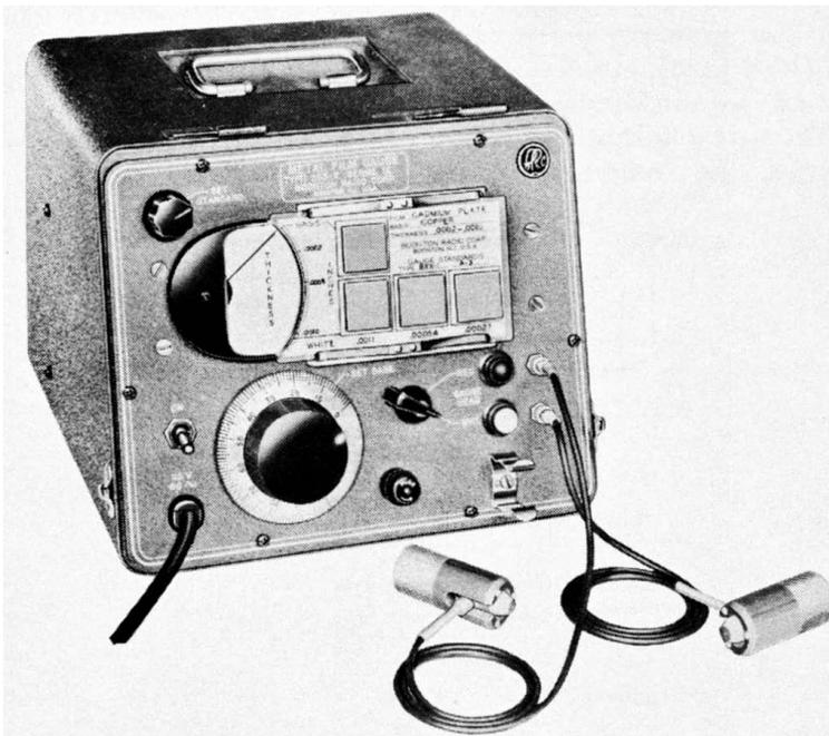
**Fig. 7-56. Metal film-thickness gauge with probes.** (Courtesy of Boonton Radio Corp.)
