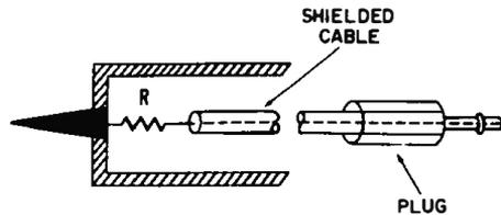
**Fig. 1-6. Internal construction of an isolation probe for a DC VTVM.**
