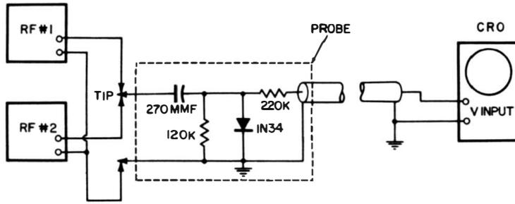
**Fig. 5-21. How to compare the frequency of one RF signal with another.**
