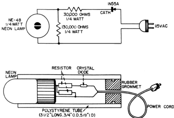
Fig. 7-89. Circuit diagram and construction details of a probe-type stroboscope. (Courtesy of Sylvania Electric Products, Inc.)
