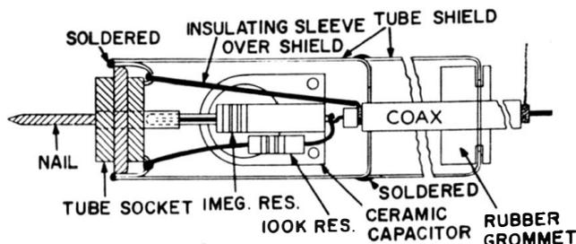
**Fig. 3-8. Constructing a low-capacitance probe.** (Courtesy of Philco Corp.)
