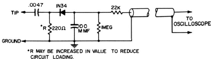
**Fig. 5-5. Series demodulator probe (low impedance).**
