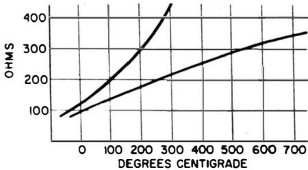
**Fig. 7-37. Variation of probe resistance with changing temperature for two different types of wire.**
