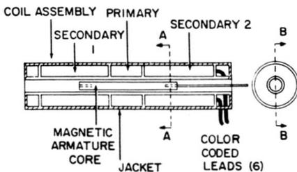
**Fig. 7-43. Cross-sectional view of a displacement-measuring probe.** (Courtesy of Sanborn Co.)
