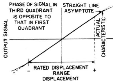
**Fig. 7-45. Characteristic curve of the output of the probe in Fig. 7-43.** (Courtesy of Sanborn Co.)
