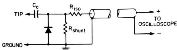
**Fig. 5-3. Basic schematic of shunt-type demodulator probe.**
