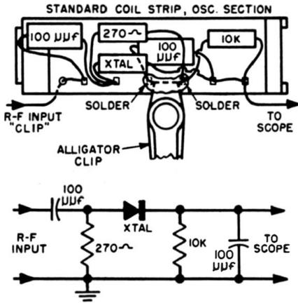
**Fig. 5-6. Series demodulator probe suitable for alignment of overcoupled video-IF stages.**
