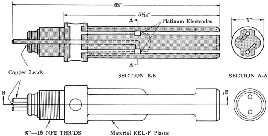
**Fig. 7-87. Electrolytic conductivity probe for insertion into a pipeline.** (Courtesy of Leeds and Northrup Co.)
