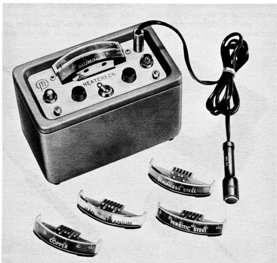
**Fig. 7-58. Eddy-current instrument for identifying alloys and properties in metals.**
