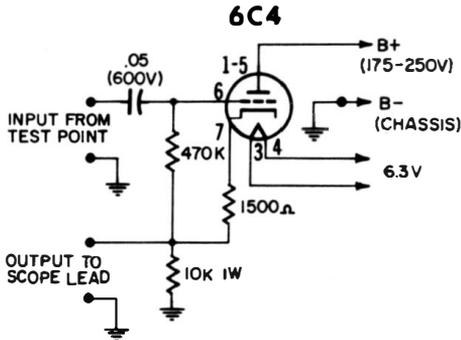
**Fig. 3-18. An easily constructed cathode-follower probe.**
