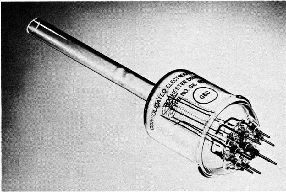
**Fig. 7-52. Ionization gauge for measurement of pressures in the ultra-high vacuum region.** (Courtesy of Consolidated Electrodynamics Corp.)
