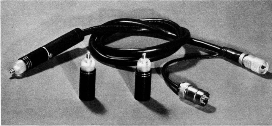
**Fig. 3-16. The P170-CF cathode-follower probe and the various attenuators.** (Courtesy of Tektronix, Inc.)
