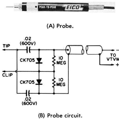
**Fig. 4-42. A typical symmetrical voltage-doubler, peak-to-peak probe using semiconductor diodes.** (Courtesy of Electronic Instrument Co., Inc.)
