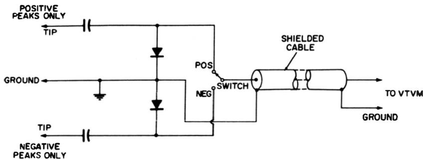
Fig. 4-23. A peak-indicating probe which will read either the positive or the negative peak, depending on the switch setting.
