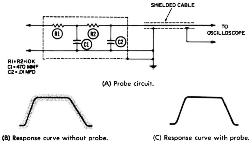
Fig. 1-9. Isolation-filter probe circuit and its effect on response-curve indications.
