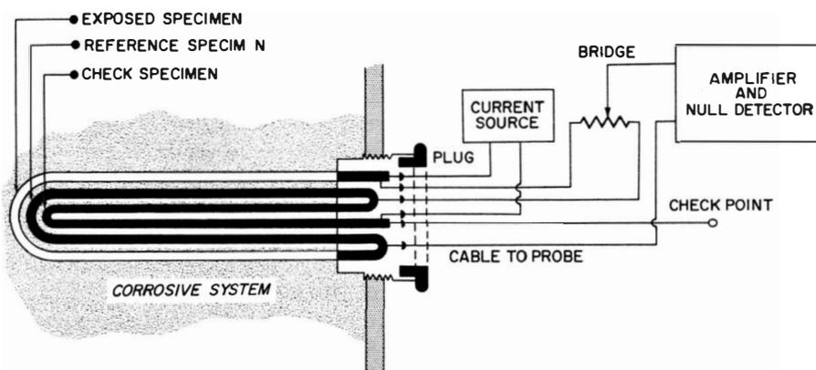
Fig. 7-73. Functional diagram of a corrosion-measuring instrument and probe.
