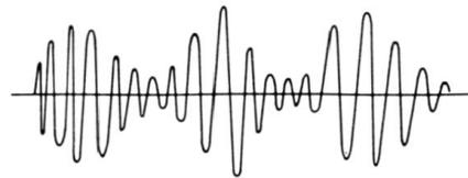
(A) Amplitude-modulated signal (input).
