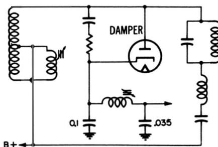
(A) Can be used at the damper cathode.
