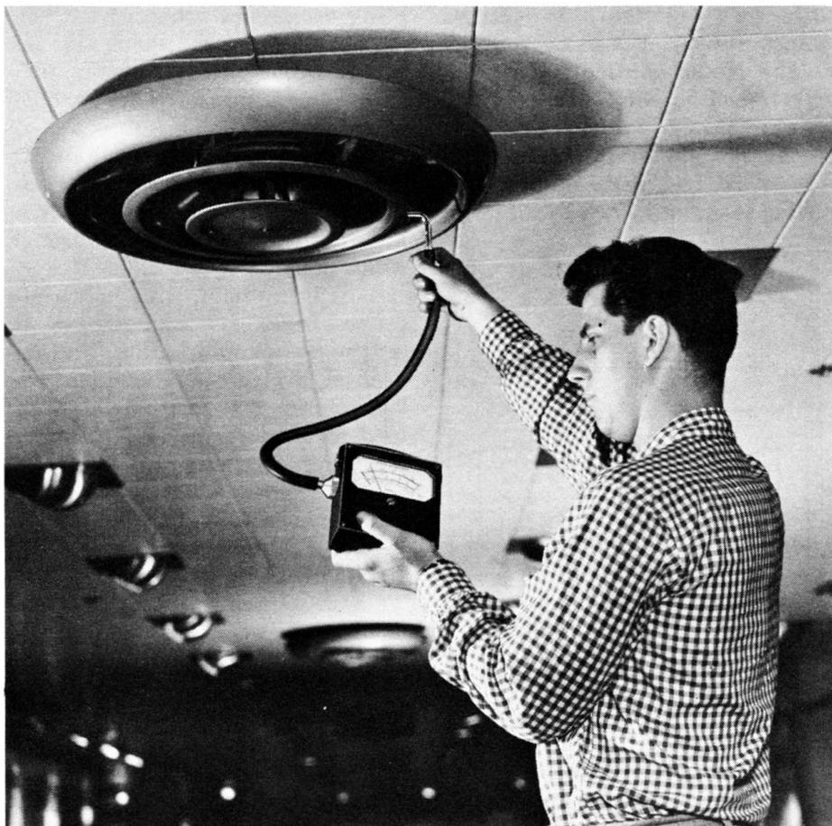
**Fig. 7-69. Air-velocity meter in use.** (Courtesy of Illinois Testing Laboratories, Inc.)
