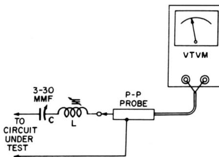
(B) Circuit for rejecting the vertical-sync pulses.
