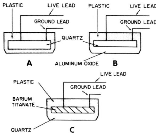
**Fig. 7-55. Basic construction of ultrasonic transducer probes.**
