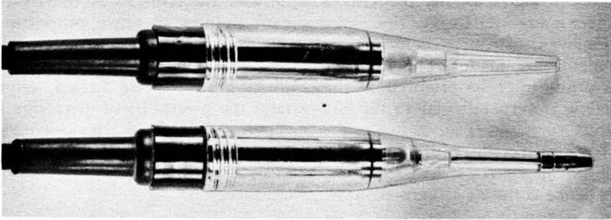
**Fig. 7-67. Probe used with gas-leak detector.** (Courtesy of General Electric Co.)
