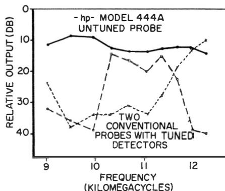
**Fig. 7-23. Typical response and efficiency characteristics of the untuned probe of Fig. 7-21 compared with the conventional probes having tuned detectors.** (Courtesy of Hewlett-Packard Co.)
