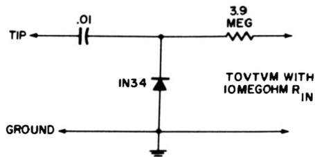
**Fig. 4-27.** A high-frequency peak-indicating probe for use with a VTVM having a 10-megohm input resistance.
