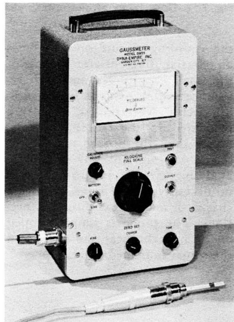
**Fig. 7-13. Transistorized gauss meter.**
