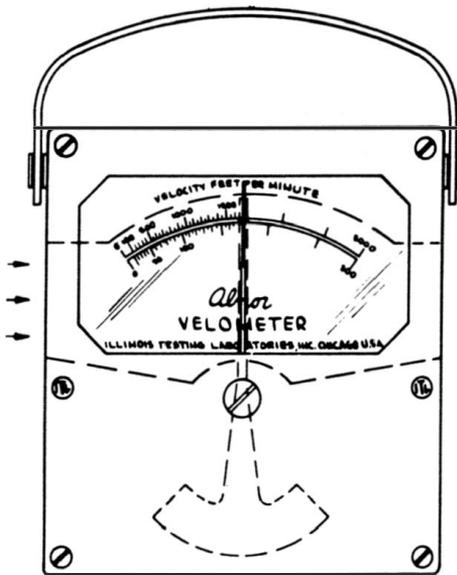
**Fig. 7-68. Phantom view of air-velocity meter.** (Courtesy of Illinois Testing Laboratories, Inc.)
