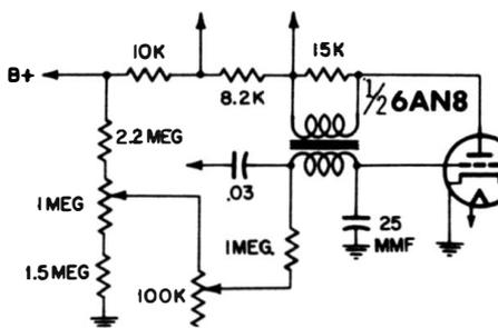
(B) Cannot be used at grid of vertical-blocking oscillator.
