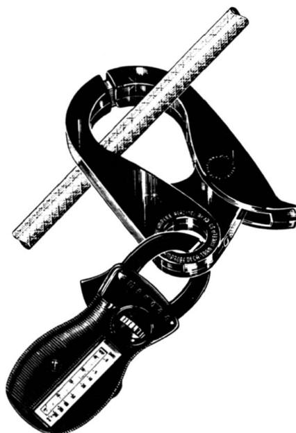
**Fig. 7-8. Adapter for extending current range of probe in Fig. 7-7.** (Courtesy of Pyramid Instrument Corp.)
