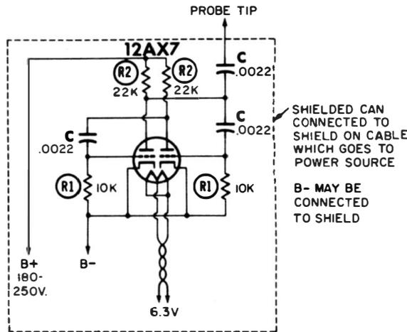
Fig. 6-17. Schematic of a signal-injector probe using a 12AX7 tube.
