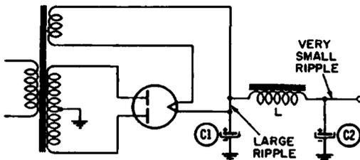
Fig. 3-4. A typical power-supply filter as used in radio and TV sets.
