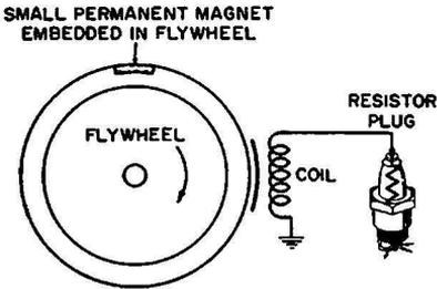
Fig. 6-13. A typical magneto ignition-system circuit.
