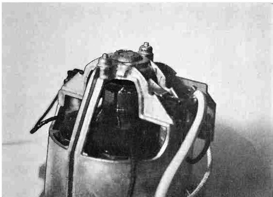
**Fig. 5-10.** A typical small motor, showing commutator and brush holders.
