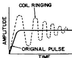
(B) The applied pulse and the ringing voltage.
