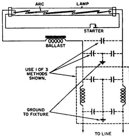
Fig. 6-15. Methods of eliminating noise from a fluorescent light.
