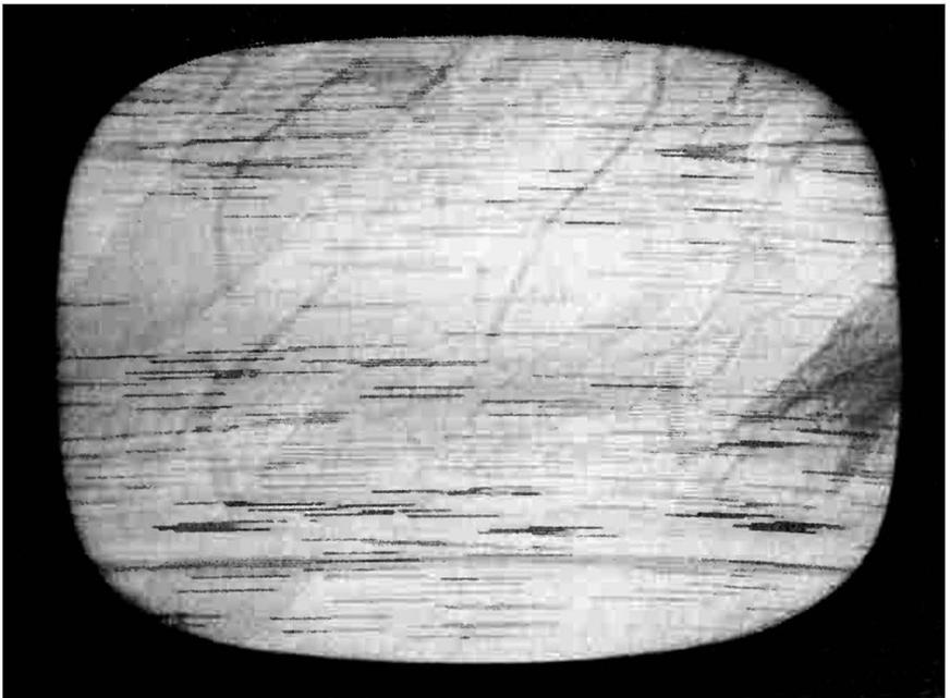
**Fig. 6-19. Severe neon-sign interference on a TV receiver.**
