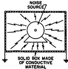
Fig. 2-10. Shielding a noise-producing device.
