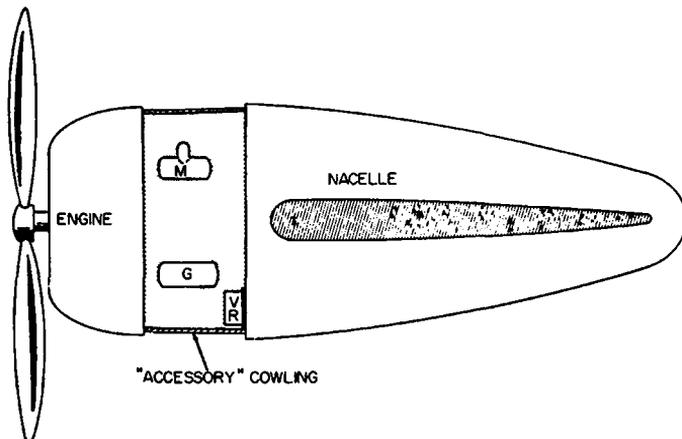
Fig. 9-1. Location of the generator, voltage regulator, and magneto on a typical aircraft engine.
