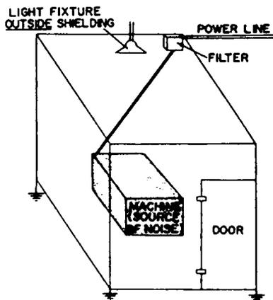
Fig. 11-10. Construction of a screen room.
