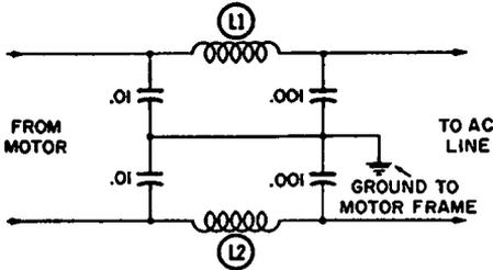
Fig. 6-9. Configuration of a line filter suitable for adding to an electric lawn mower.
