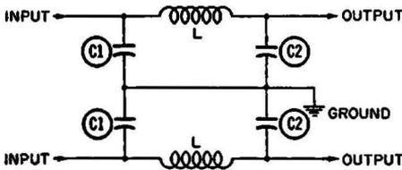
Fig. 3-20. Standard LC circuit used in series with the AC line.
