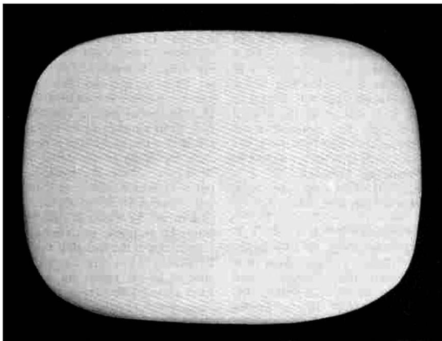
Fig. 6-46. RF beat interference in a TV receiver, caused by another transmitter.
