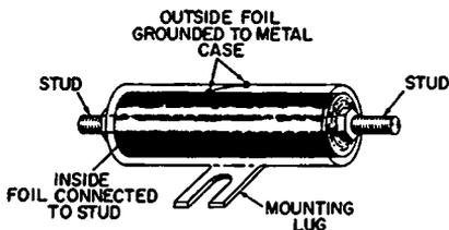
(B) Coaxial bypass capacitor.
