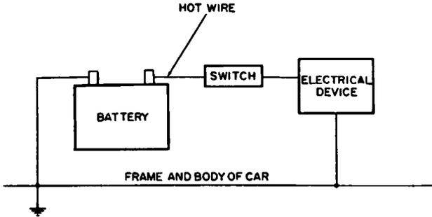
Fig. 7-2. Basic automotive electrical circuit.
