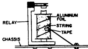
**Fig. 11-5. Shielding a relay coil with foil to eliminate interference.**
