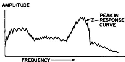
(B) Frequency versus amplitude curve.
