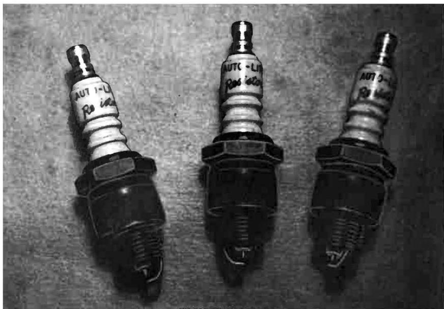
Fig. 7-9. Spark plugs with built-in suppressor resistors.
