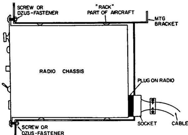
Fig. 9-2. Method of mounting aircraft radio equipment.
