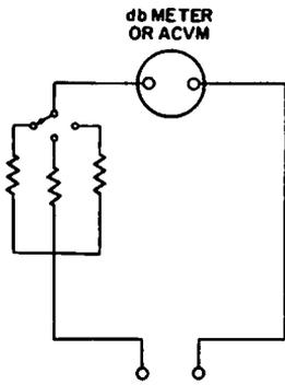
(A) Using series resistors.
