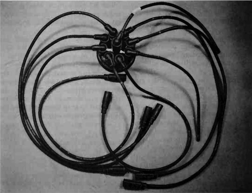
Fig. 8-7. A complete set of resistance-type ignition wiring.
