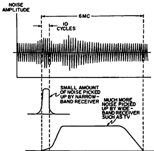
Fig. 1-5. Comparison of noise pickup by a receiver with 10-cycle bandwidth to that of a TV receiver.
