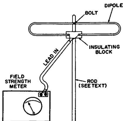
Fig. 4-13. A probe dipole and field-strength meter for locating TVI.
