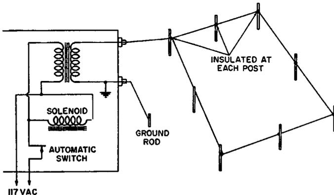
Fig. 6-28. A typical electric-fence circuit.
