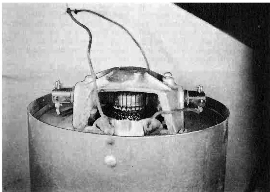
**Fig. 5-9.** Commutator and brushes of an AC motor, showing excessive wear.
