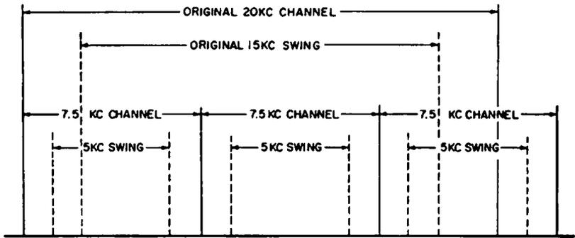
Fig. 8-1. Comparison of the original 20-kc channels with the narrow-band 7.5-kc channels.
