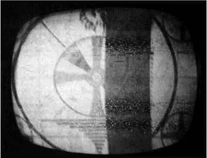
Fig. 6-44. A typical "cable bar" in a TV receiver.
