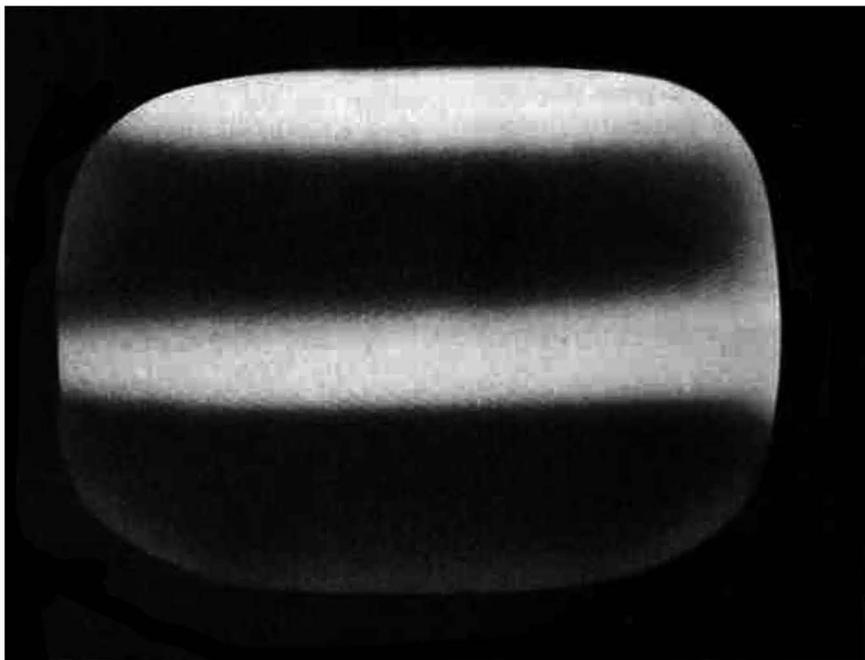
Fig. 6-39. Severe interference on Channel 4 due to strong second-harmonic radiation from a 36-mc transmitter.
