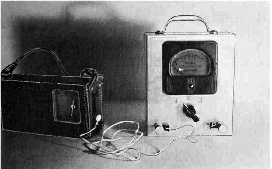
Fig. 4-1. A portable radio and meter for locating noise sources.
