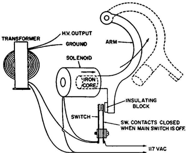
**Fig. 6-29.** The automatic keying device for an electric fence.
