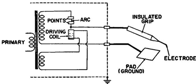
Fig. 11-9. Basic schematic of a "radio knife."
