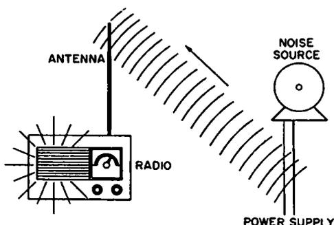
Fig. 2-3. "Broadcasting" of noise from the power lines.
