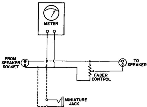
Fig. 4-10. Adapter-harness circuit.
