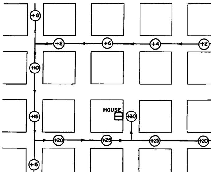
Fig. 4-11. Location of power lines, and readings found at various points along the lines.
