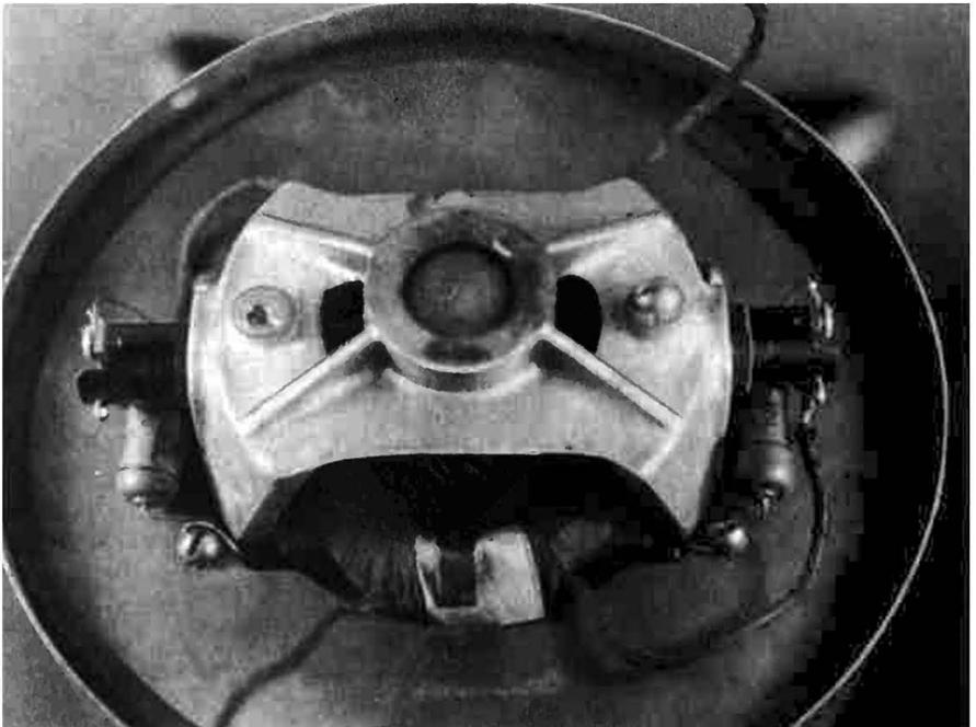
Fig. 6-12. Capacitors installed across the brushes of a vacuum cleaner.
