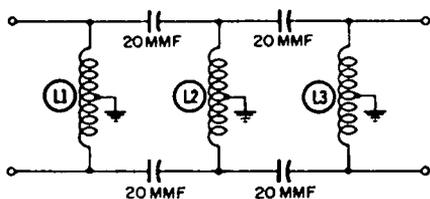
Fig. 6-56. A high-pass filter schematic.
