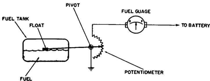
Fig. 7-16. Basic circuit of an electrically-operated fuel gauge.
