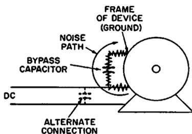
Fig. 2-4. Applying a bypass capacitor to the noise source.
