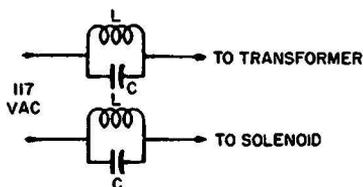
Fig. 6-31. LC filters added to the input of an electric fence.
