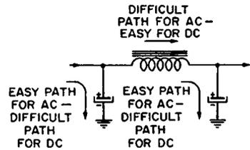
Fig. 3-5. Current paths for pi-section filter in Fig. 3-4.
