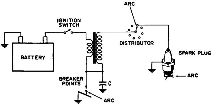
Fig. 7-3. Basic schematic of the automotive ignition system.
