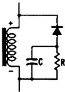
(D) Combination of diode and RC network across coil.
