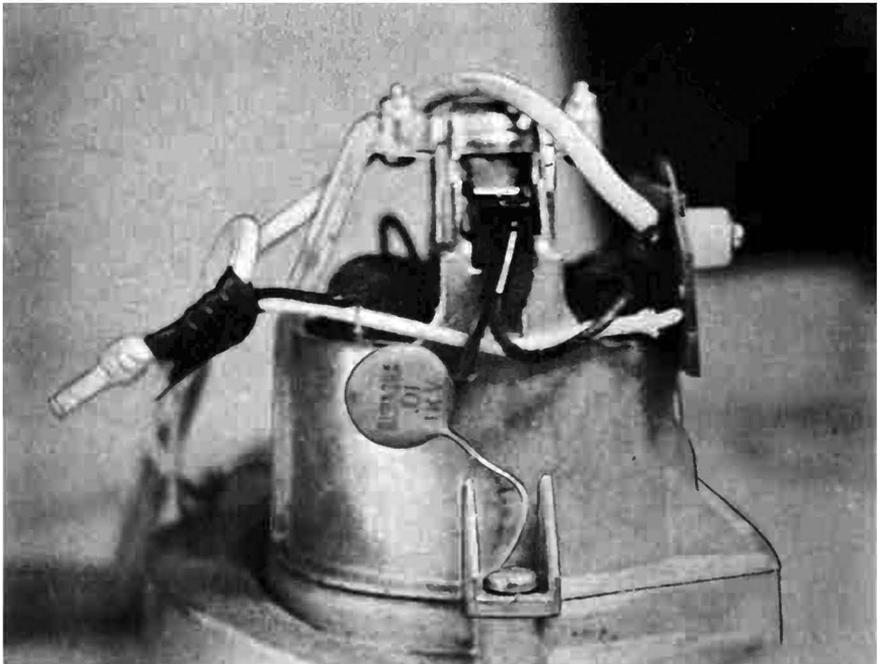
Fig. 6-3. Bypass capacitor added to a small brush-type AC motor.
