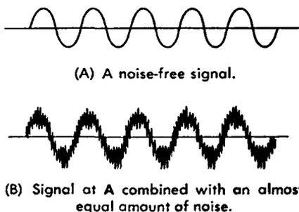
Fig. 1-2. Effect of noise on a signal.
