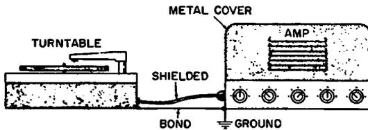
Fig. 6-35. Shielding an audio amplifier.
