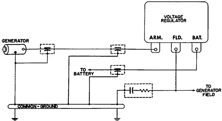
Fig. 8-8. Points where coaxial capacitors and the special field filter unit should be used for mobile-radio work.
