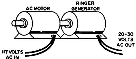
Fig. 6-33. Motor and "ringer" generator in a telephone office.
