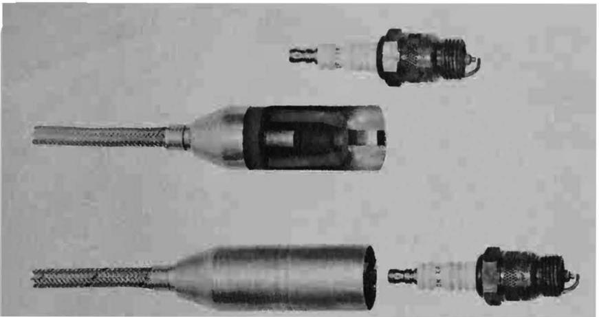
**Fig. 8-11. Special shielded terminals for spark plugs.**
