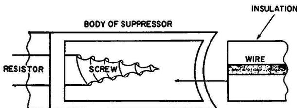
**Fig. 7-8. Detail of one end of a cable-type resistive suppressor.**
