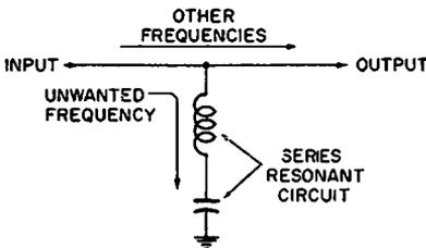
(A) Using series-resonant circuit.
