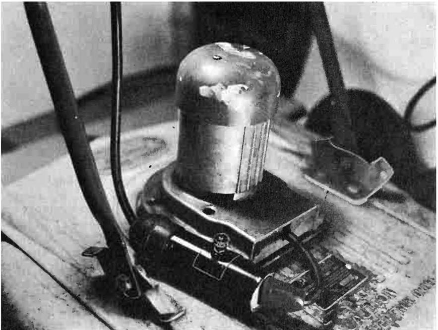
**Fig. 6-8. Line filter added to an electric lawn mower.**
