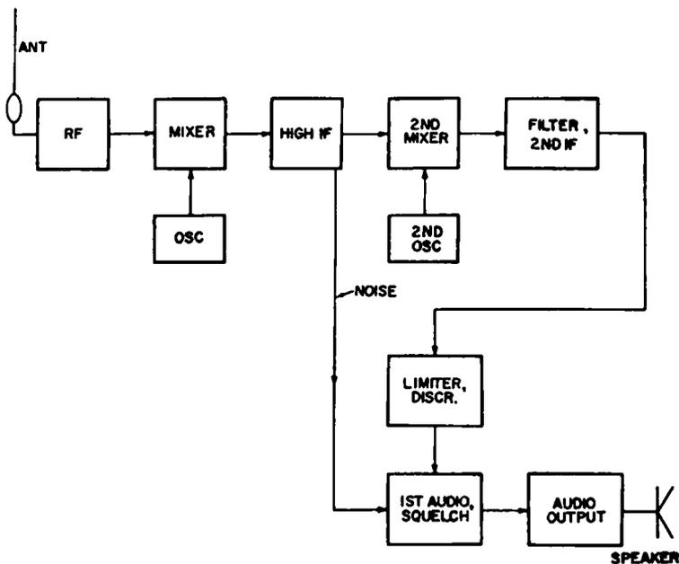
Fig. 8-3. Block diagram of a typical mobile FM receiver.
