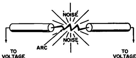
Fig. 2-1. Random noise created by an electric arc.
