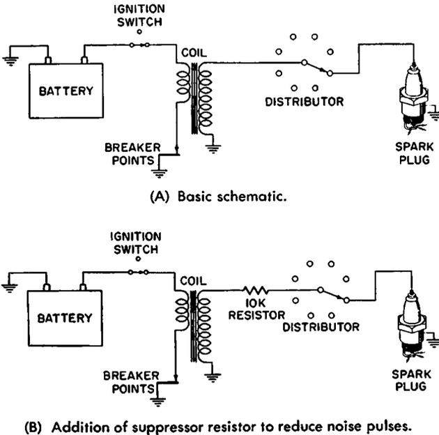
Fig. 2-8. Automobile electrical system.
