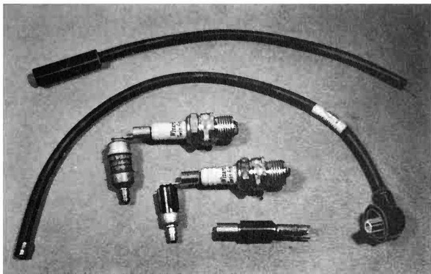
**Fig. 7-7. Different types of suppressors.**
