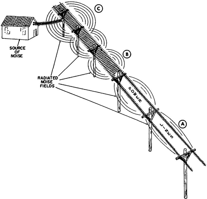
**Fig. 4-8. Relative amplitude of noise being conducted along power lines.**
