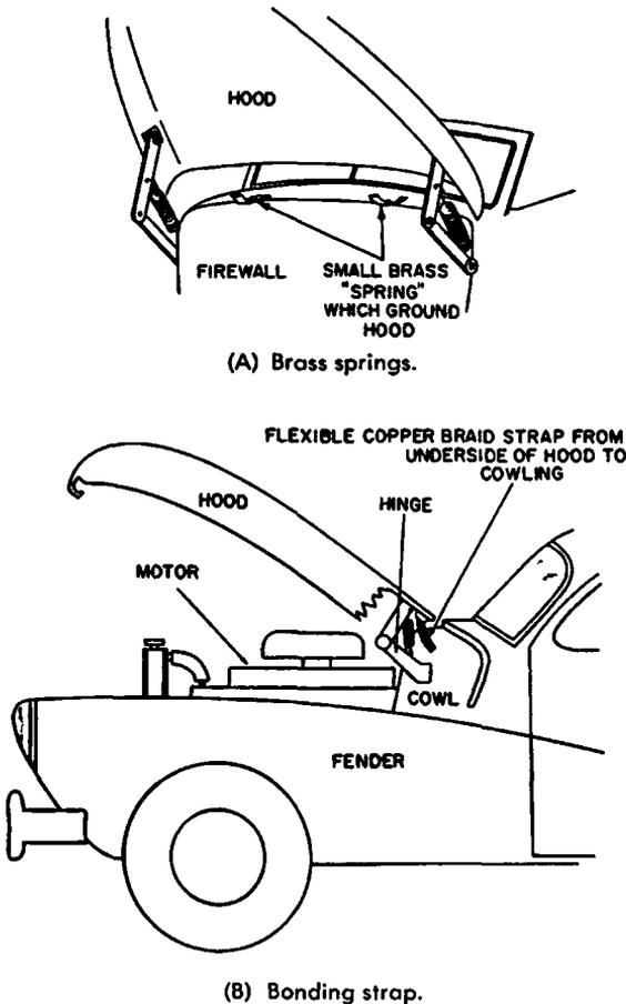
Fig. 7-17. Methods of grounding the hood of an automobile.
