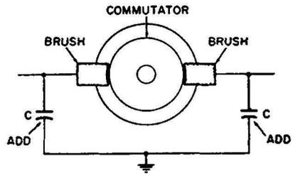
Fig. 6-2. Adding capacitors to brushes to eliminate noise.
