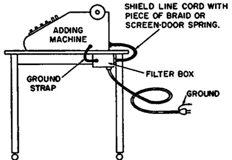
Fig. 6-10. Methods of eliminating noise in an adding machine.
