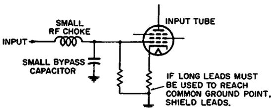
Fig. 6-36. Filter circuit added at input of audio amplifier.
