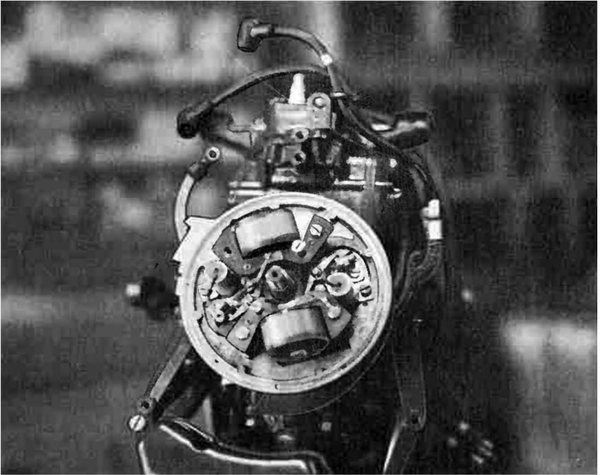
Fig. 10-1. Magneto and breaker points on a typical outboard motor.
