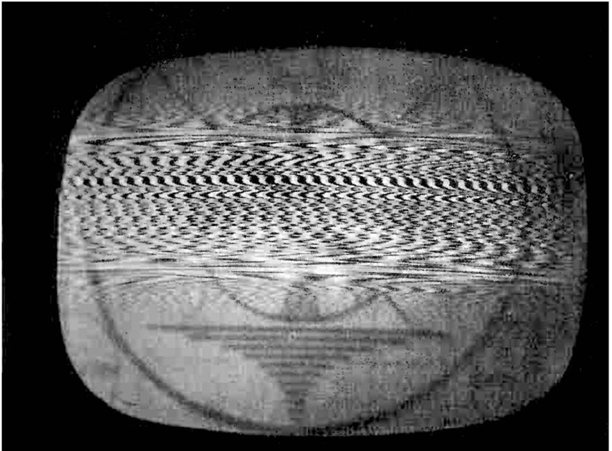
Fig. 6-40. FM receiver radiation in a TV receiver.
