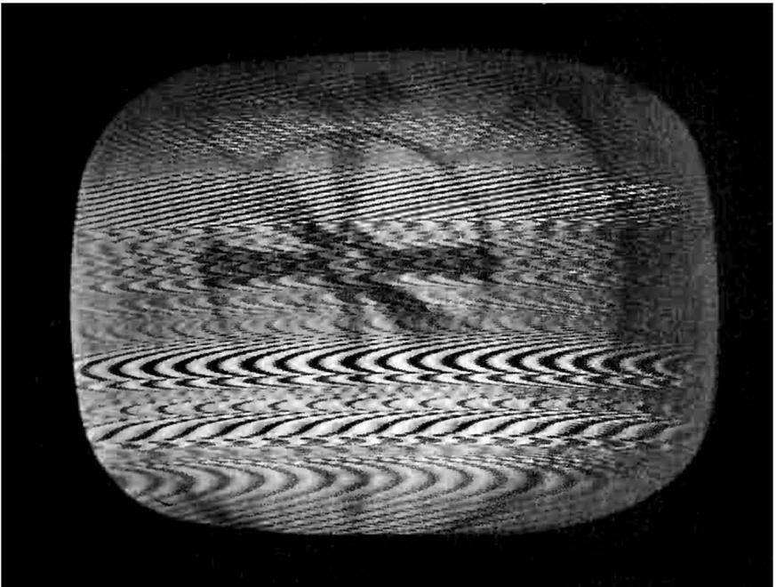
Fig. 6-38. Interference in a TV receiver, caused by a radio transmitter in a passing police car.
