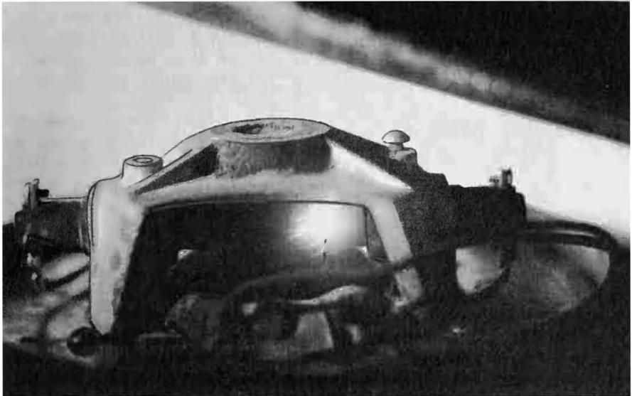
Fig. 5-7. Severe arcing at the brushes of a small motor.
