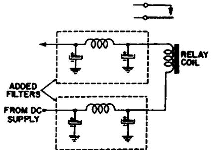
**Fig. 11-4. Adding LC filters on both sides of radiating coil to eliminate interference.**
