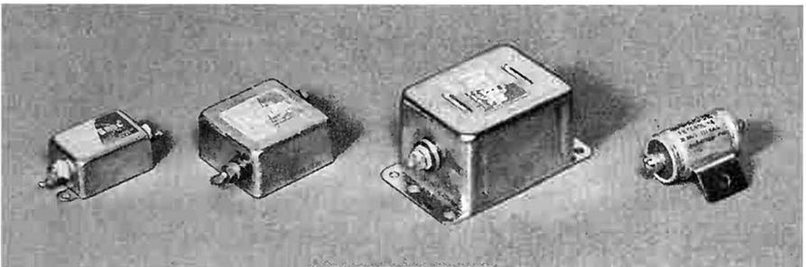
**Fig. 3-24. Commercial pi-network filters.**
