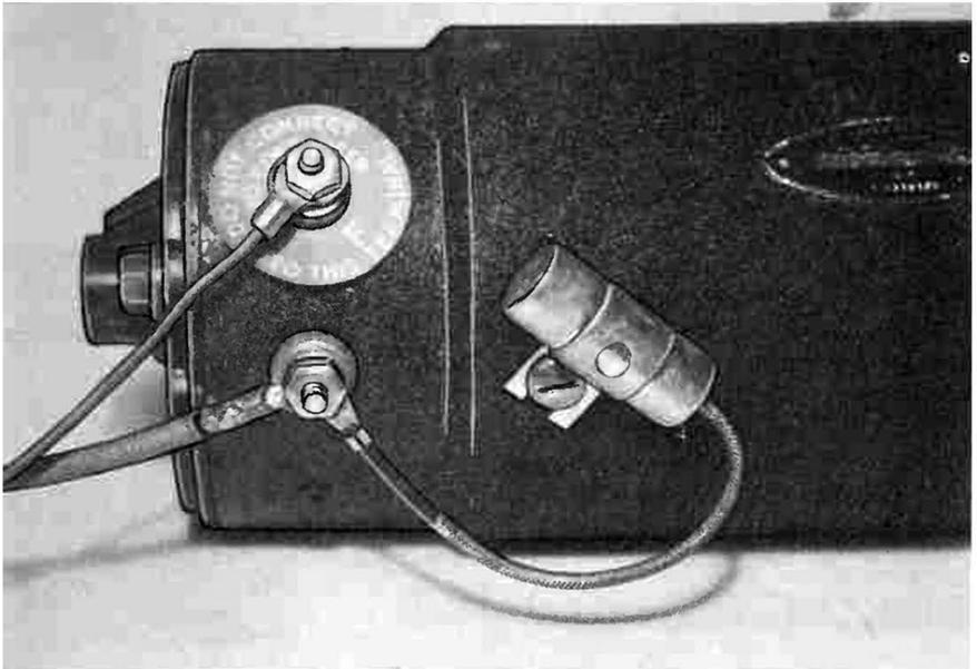
**Fig. 7-12. Generator capacitor mounted on generator housing.**
