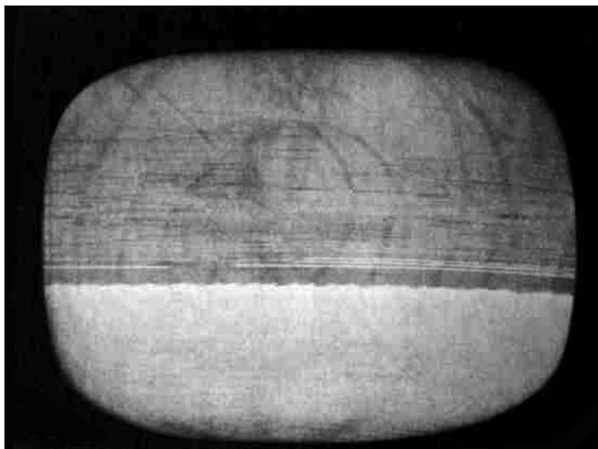
Fig. 6-24. Battery-charger interference in a TV receiver.
