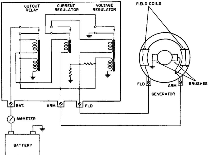
Fig. 7-13. A typical voltage-regulator circuit.
