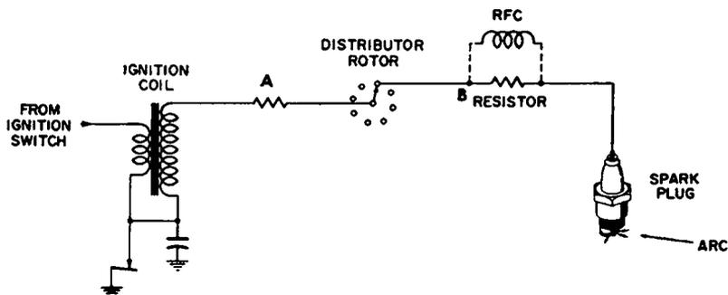
Fig. 7-6. Adding resistive suppression to damp pulses in the ignition system.
