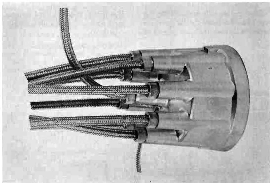
**Fig. 8-10. A special shielded distributor cap with shielded spark-plug wiring.**
