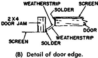
Fig. 11-11. Construction of a screen room door.
