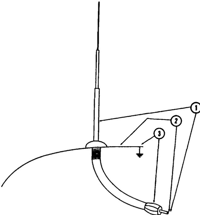
Fig. 7-18. The three tests for an automobile antenna.
