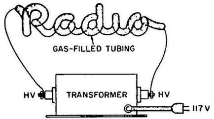
**Fig. 6-17. The basic neon-sign circuit.**
