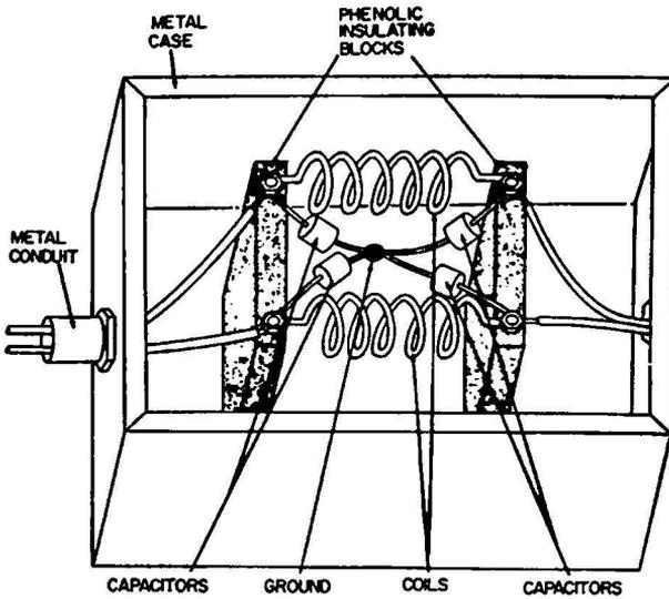
Fig. 6-43. Construction of an AC line filter for an industrial heater.
