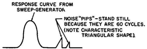
Fig. 6-22. Power-line interference in a sweep response curve.
