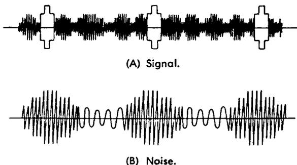
Fig. 1-1. Comparison of a signal and a noise voltage.
