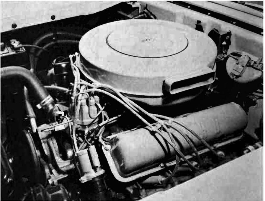
**Fig. 8-14.** Fully-shielded ignition system installed on a car.
