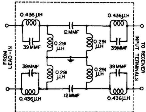
Fig. 6-52. Schematic of a typical high-pass filter.
