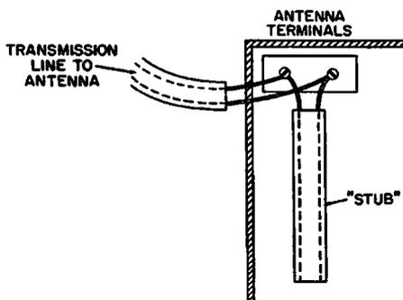
Fig. 6-49. A stub made of a length of transmission line connected across the antenna terminals of a TV receiver.
