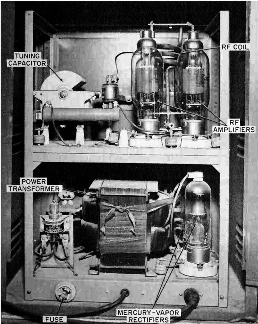
Fig. 6-42. Rear view of a typical RF induction heater.
