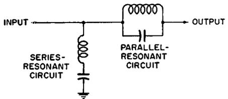
(B) Using both series- and parallel-resonant circuits.
