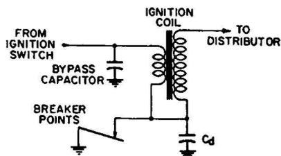
Fig. 7-10. Installing a bypass capacitor in ignition-coil circuit.
