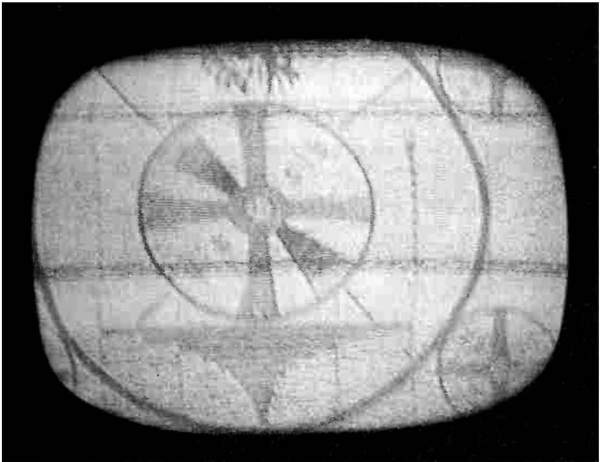
Fig. 6-14. Fluorescent-light interference on a TV screen.
