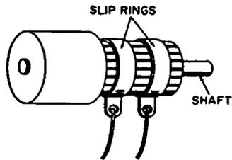
Fig. 6-34. Slip rings at the "ringer"-generator output.
