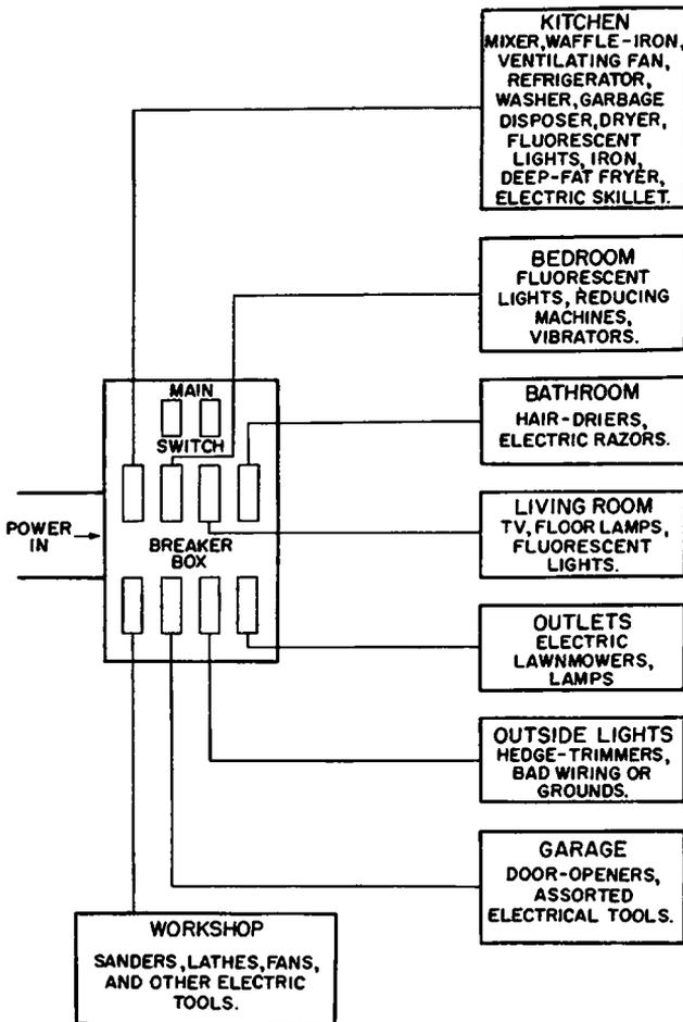
Fig. 4-6. Electrical circuits and potential noise sources in a modern home.
