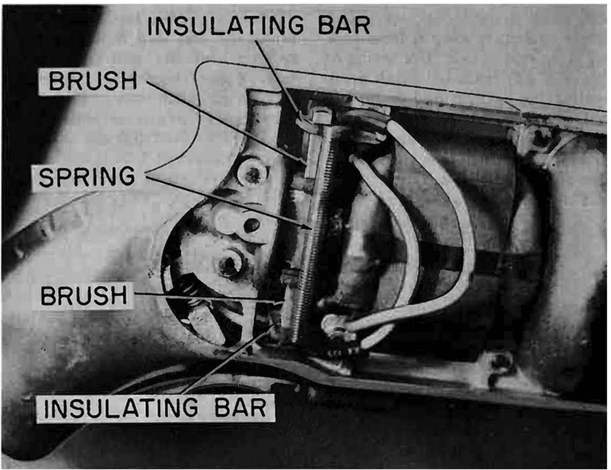
**Fig. 5-5. Brush holders and springs on an electric drill.**
