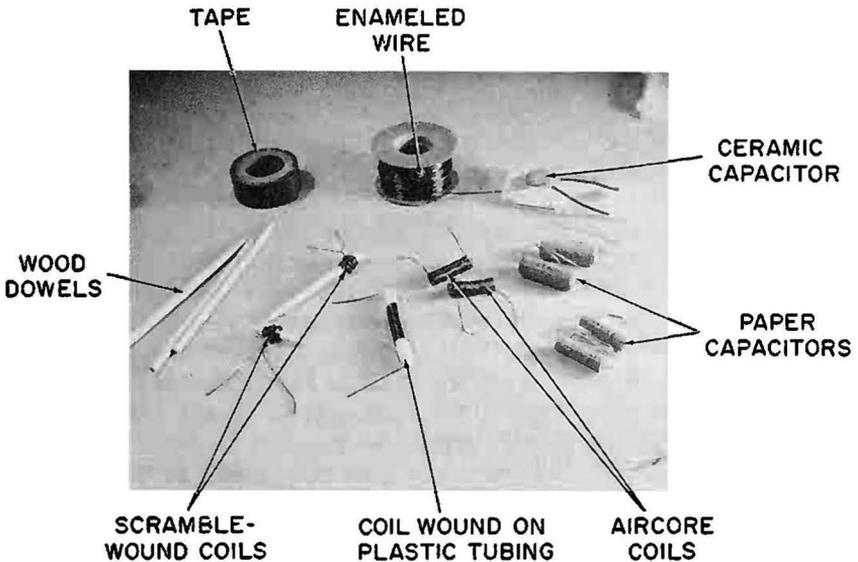
Fig. 3-21. Parts needed to build filters, and the completed filters.
