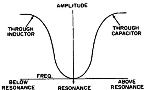
Fig. 3-14. Transmission characteristics of a parallel-resonant circuit.
