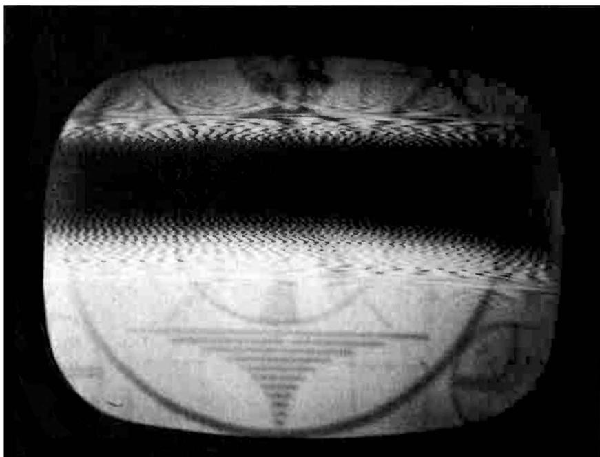
Fig. 6-41. Interference from an RF heater in a TV receiver.
