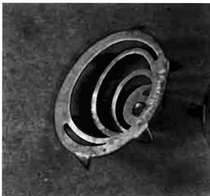
Fig. 7-15. A front-wheel grounding spring.
