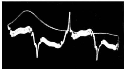
**Fig. 6-18. Voltage waveform at secondary of neon-sign transformer.**
