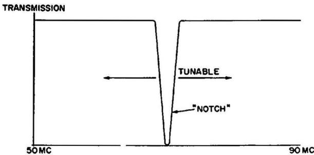
**Fig. 6-55. Transmission characteristics of the filter in Fig. 6-54.**
