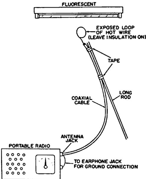
Fig. 4-2. A special probe for locating noise sources.
