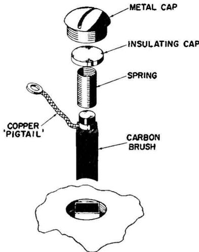
Fig. 5-4. Construction of a typical small motor.
