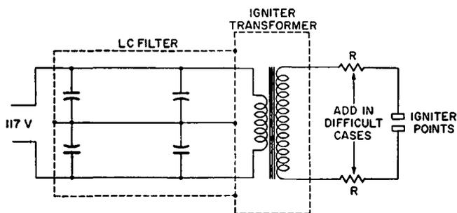
Fig. 6-25. Eliminating noise in an oil-burner igniter.
