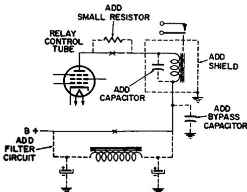
Fig. 11-6. Methods of reducing interference from a relay coil in the plate circuit of a vacuum tube.
