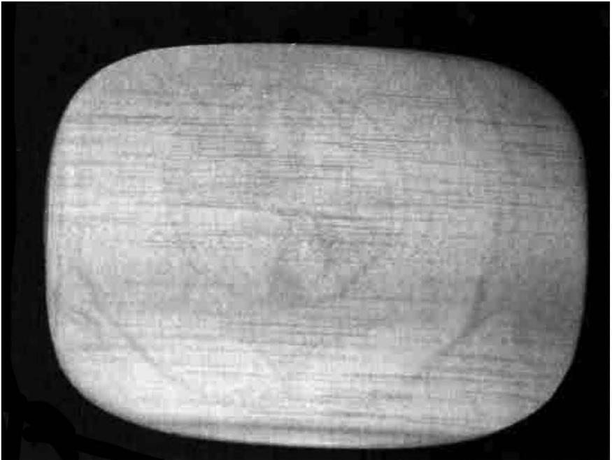
Fig. 6-27. Severe ignition noise in a TV receiver.
