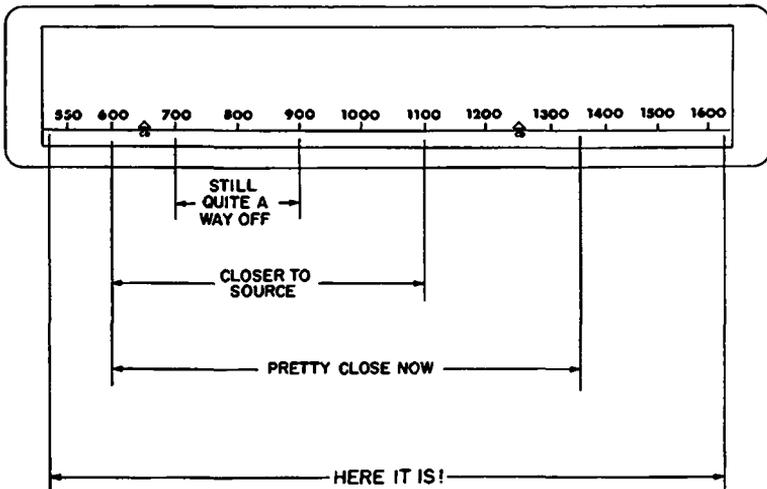
Fig. 4-4. Noise-distribution characteristics over the radio dial at various distances from the noise source.
