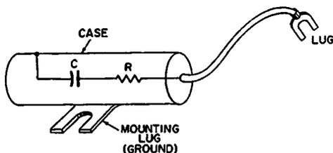
Fig. 8-5. A special RC filter for bypassing the voltage-regulator field connection.
