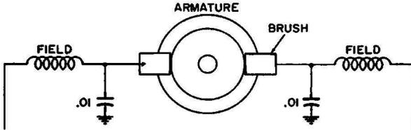
Fig. 6-4. Reconnecting small AC motors so the armature is between the field coils.
