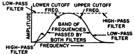
(C) Combining low-pass and high-pass filters.
