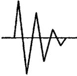
(B) Fluctuations when suppressor resistor is used.
