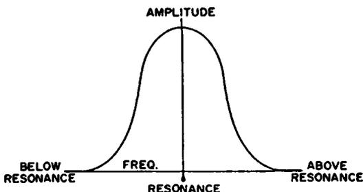
Fig. 3-16. Transmission characteristics of a series-resonant circuit.
