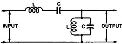
Fig. 3-9. A bandpass filter section.
