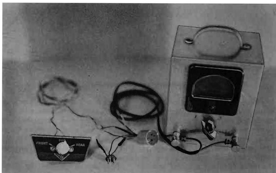
Fig. 4-9. Adapter harness for using portable meter with an auto radio.
