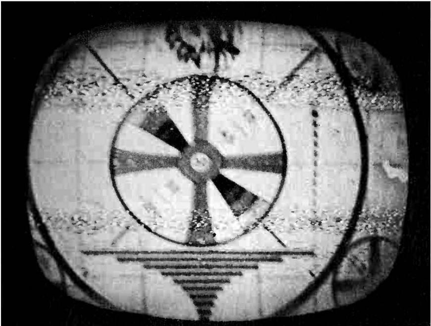
Fig. 6-21. Power-line interference in a TV receiver.
