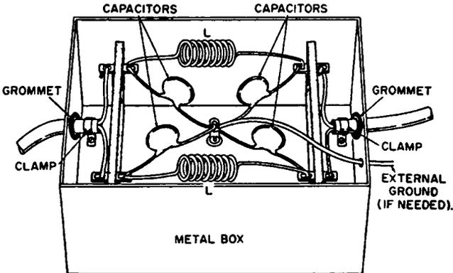
Fig. 3-22. Construction of a homemade filter.
