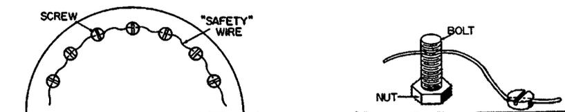
Fig. 9-3. Safety wiring of mounting bolts and screws.
