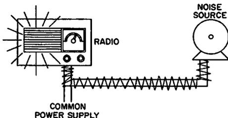
Fig. 2-2. Transmission of noise through the power lines.
