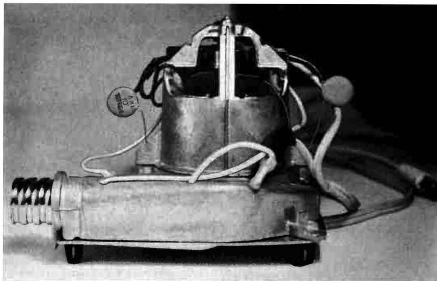
**Fig. 5-11. Adding bypass capacitors to the brushes of a small AC motor.**
