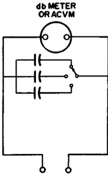
(B) Using shunt capacitors.
