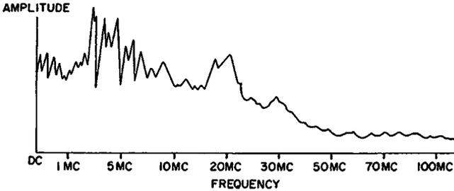
Fig. 1-3. Amplitude versus frequency spectrum of a typical arc noise.
