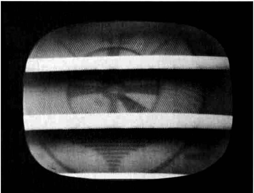
**Fig. 6-30.** Interference from an electric fence.
