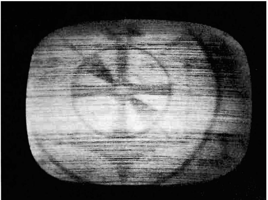
Fig. 6-1. Appearance of noise caused by an arcing motor.
