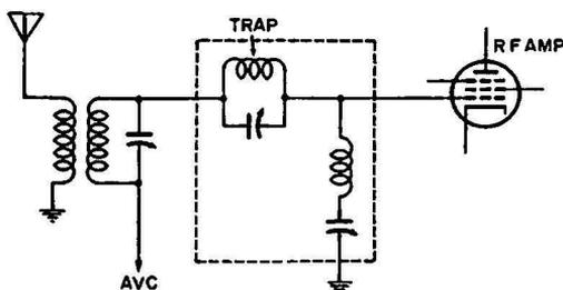
Fig. 6-47. Trap connected in an RF-amplifier grid circuit to reduce "false harmonics."
