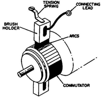
Fig. 5-3. Detail of brush holder and commutator on a small motor.
