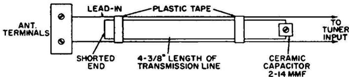
Fig. 6-50. The absorption trap attached to the transmission line.
