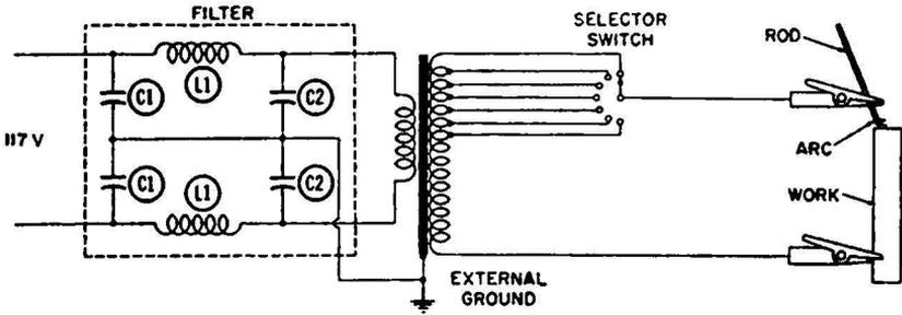
Fig. 6-26. Eliminating noise in an electric arc welder.
