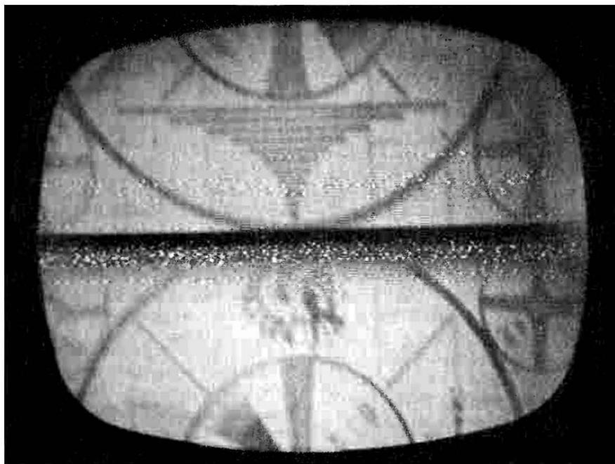
Fig. 6-32. Ragged noise pattern in a TV receiver, caused by intermittent arcing of an electric-range switch.
