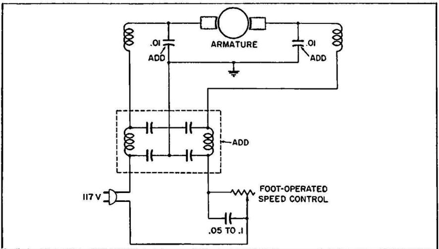
**Fig. 6-7. A typical old-type shunt sewing-machine motor.**
