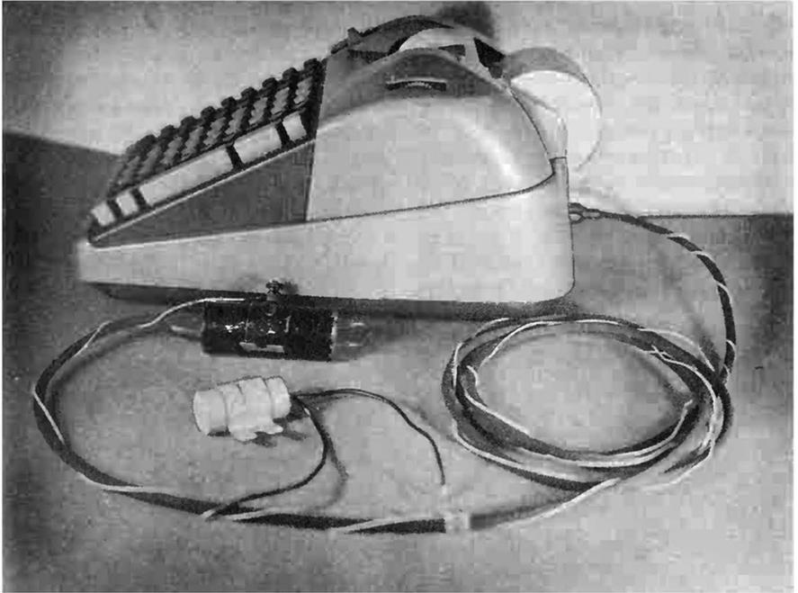
Fig. 6-11. Plug-in filter on a table-model adding machine.
