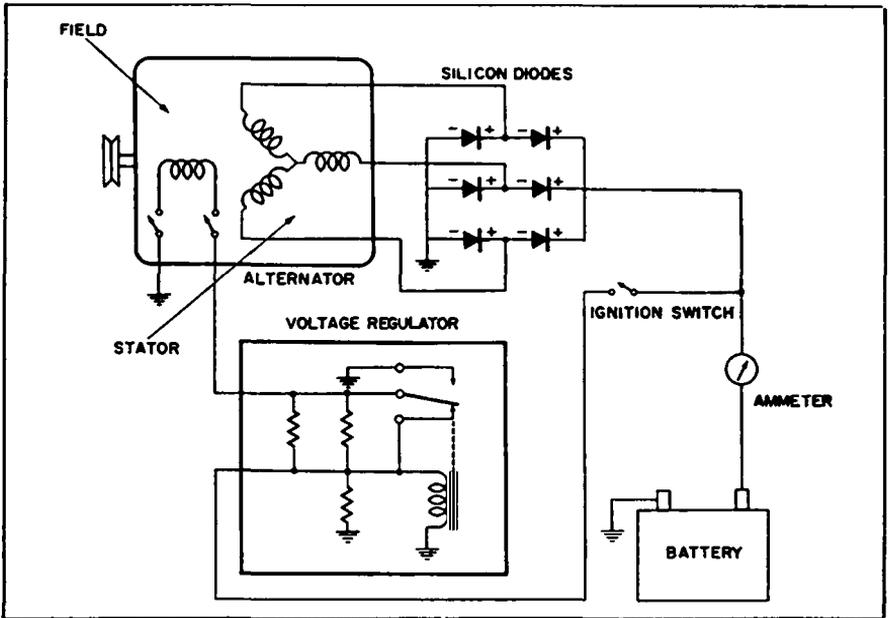
Fig. 7-19. Alternator-type automotive electrical system.
