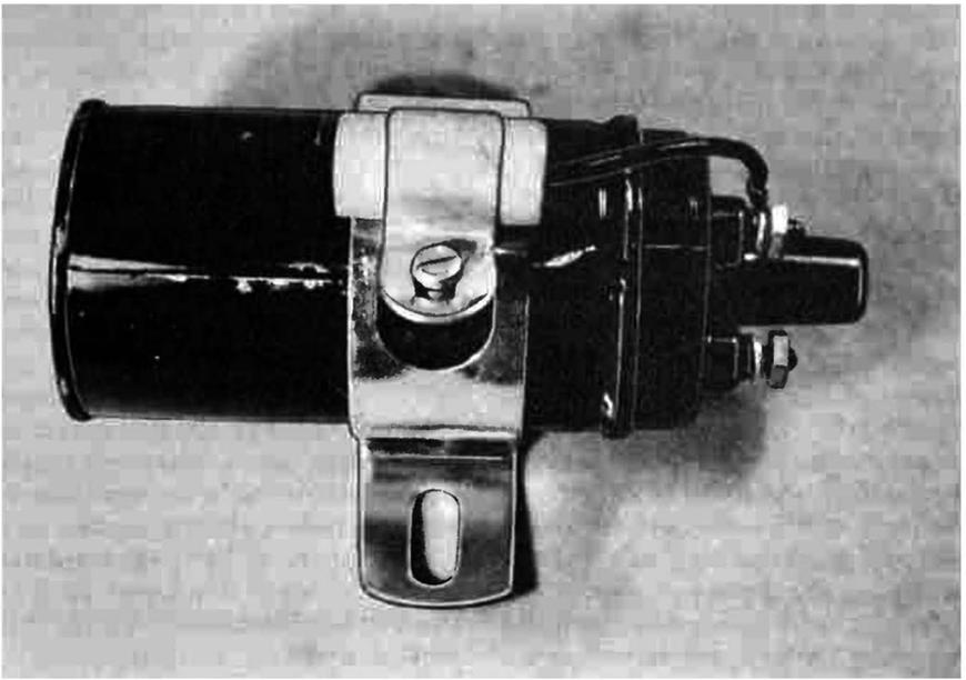
**Fig. 7-11. Bypass capacitor mounted on ignition-coil bracket.**
