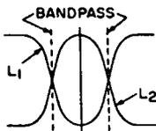
(D) Bandpass of circuit (curves B and C combined).
