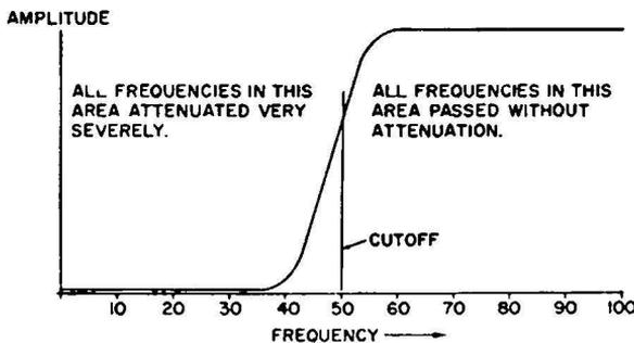
Fig. 6-53. Transmission characteristics of a 50-mc high-pass filter.
