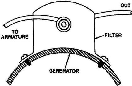
(B) Shown mounted on generator housing.
