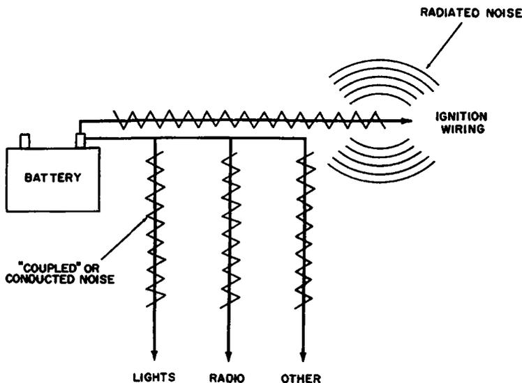
Fig. 7-4. Noise from the ignition system being radiated or conducted into other parts of the wiring.
