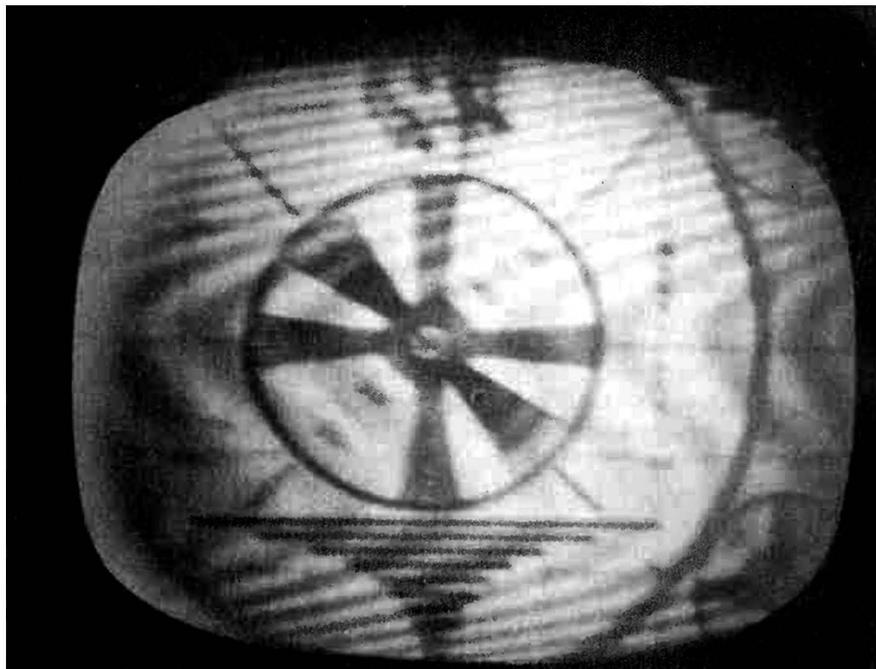
Fig. 6-45. RF beat interference in a TV receiver, caused by an oscillating booster.
