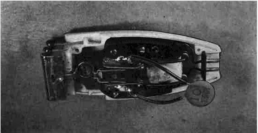
Fig. 6-6. A bypass capacitor added across the points of an electric shaver.
