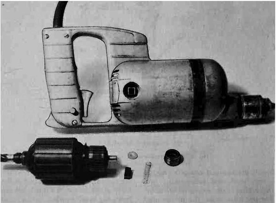
**Fig. 5-6. An electric drill with the brushes disassembled.**
