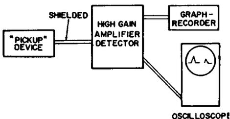
Fig. 11-7. Block diagram of a typical electromedical device.
