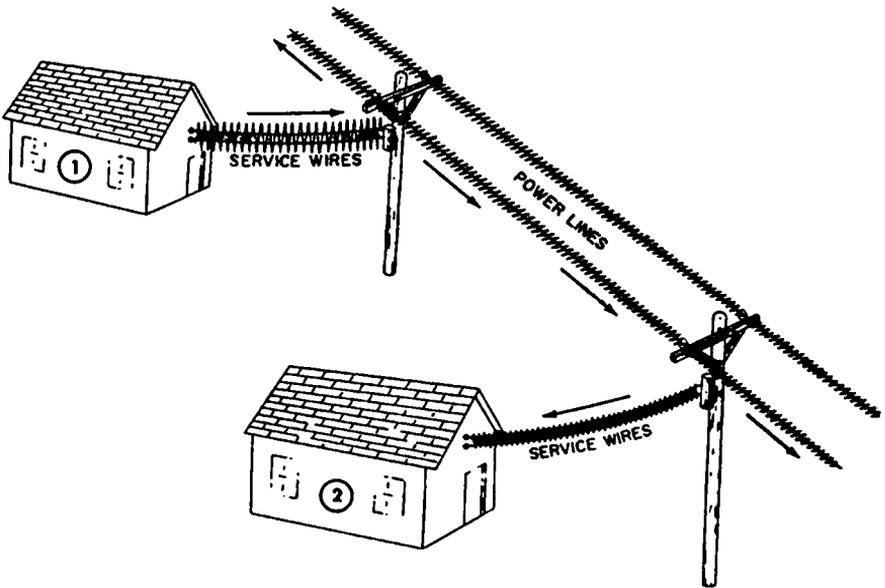
Fig. 4-7. Noise being conducted through the power lines from house No. 1 to house No. 2
