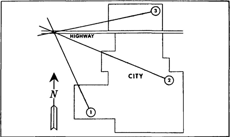
Fig. 4-12. Locating the noise source by shooting bearings on it with directional TV antennas and rotators.
