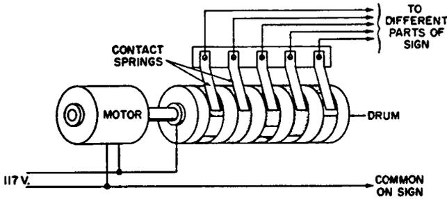
Fig. 6-20. Flasher system used on an electric sign.
