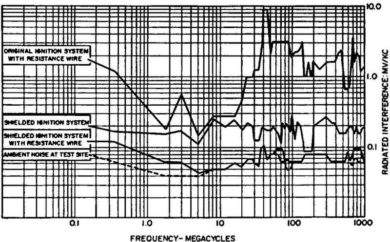
**Fig. 8-15.** Comparison of radiated noise from a shielded and an unshielded ignition system.
