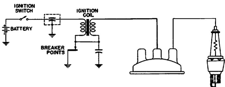
Fig. 8-9. A coaxial capacitor added in the primary side of the ignition coil.
