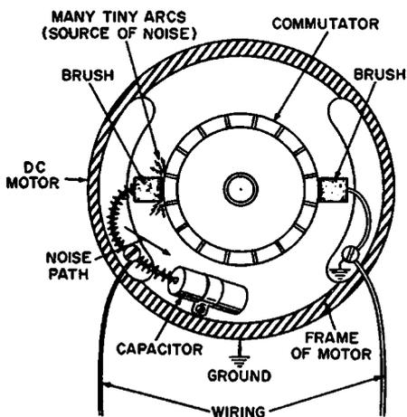
Fig. 2-5. Using a bypass capacitor to eliminate noise from a DC motor.
