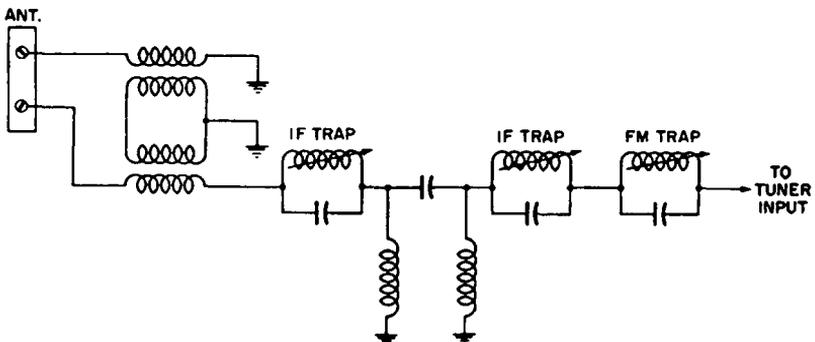
Fig. 6-48. A typical tuner input circuit in a TV receiver.
