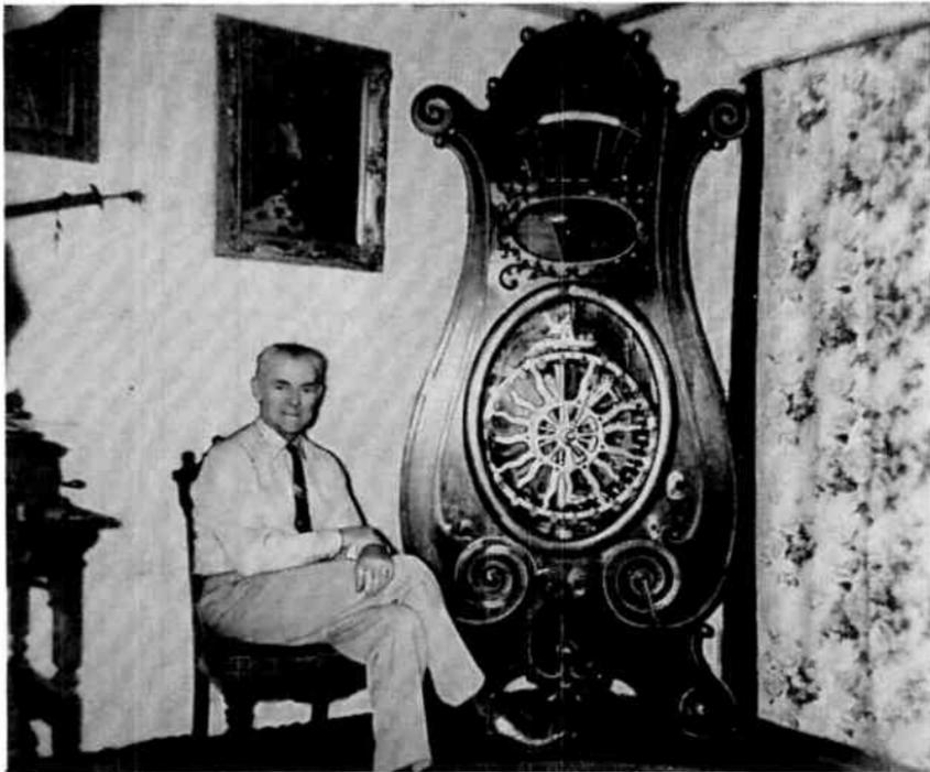
Fig. 9-2. The Multiphone was a monstrous coin-operated "jukebox" and contained 24 cylinders mounted on a large wheel. (Courtesy of C. Y. deKay.)
