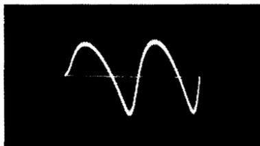
Fig. 9-7. Unsymmetrical waveform at input of the filter.
