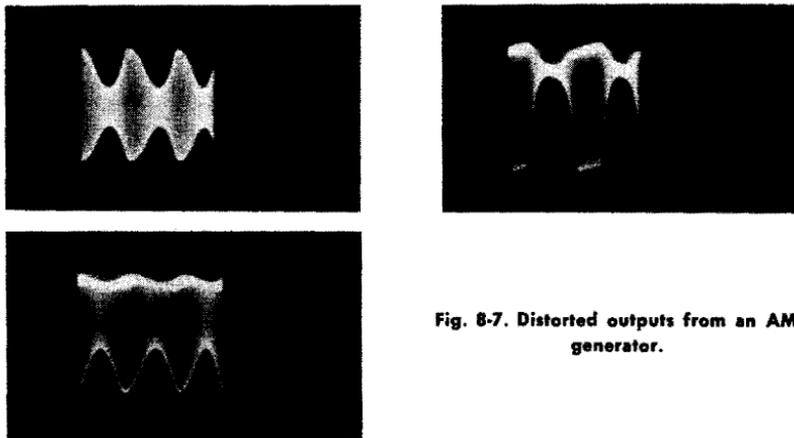
Fig. 8-7. Distorted outputs from an AM generator.
