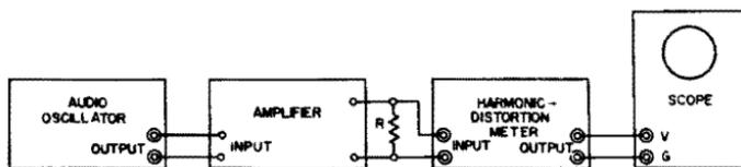
Fig. 11-7. Scope identifies the nature of distortion.
