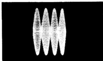
(A) Output waveform from AM generator.
