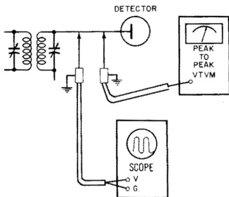
Fig. 10-2. Calibrating the probe and the scope.
