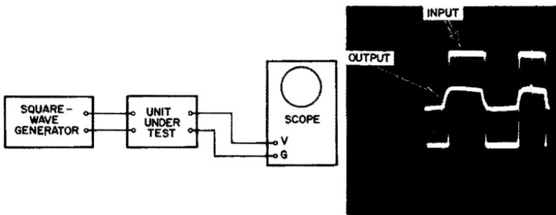
Fig. 1-46. Result of a typical square-wave test.
