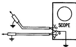
connected if the scope is well designed. The two vertical-input leads are used in exactly the same manner as the single vertical lead and ground lead of an ordinary scope. The chief advantage of this method is that the two vertical-input leads can be connected across any power-supply component without making the scope case hot. The case is always at ground potential.
