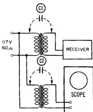
Fig. 2-20. Stray capacitances  $C_1$  and  $C_2$  form a high-impedance "connection" between the receiver chassis and scope case.
