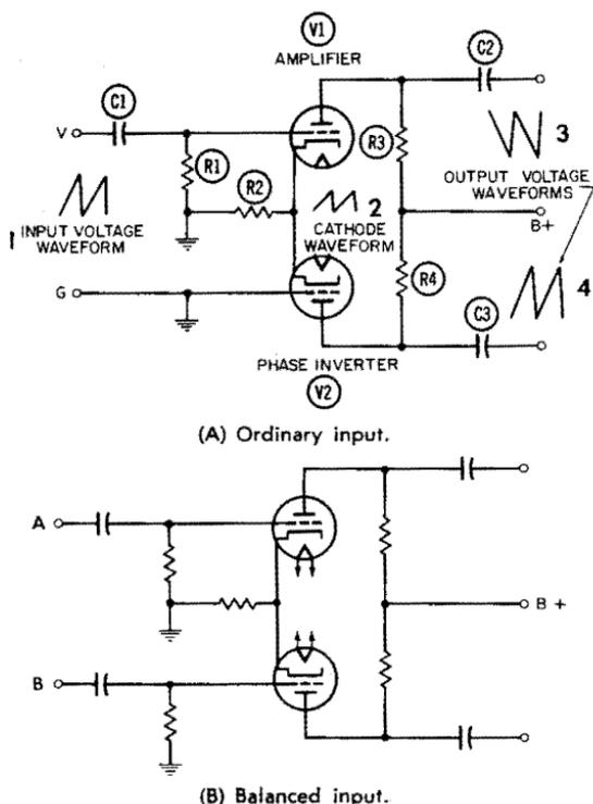
Fig. 9-12. Input circuits.
