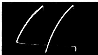
Fig. 5-4. Normal sawtooth waveform from horizontal-oscillator circuit.
