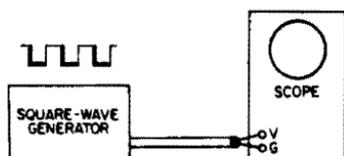
Fig. 11-10. Checking the transient response of the scope.
