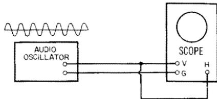
shown in Fig. 11-1. (The waveform of the audio oscillator is of no concern here.) Now set the audio oscillator frequency to approximately 400 cycles. A diagonal-line display appears on the scope screen.
