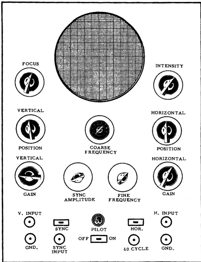
Fig. 1-1. Typical panel layout for a simple oscilloscope.
