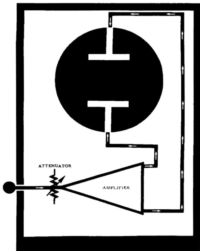
Fig. 1-17. Functional diagram of vertical-gain control.
