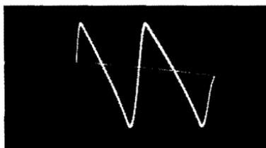
Fig. 5-18. Comparison sawtooth from the sweep circuit.
