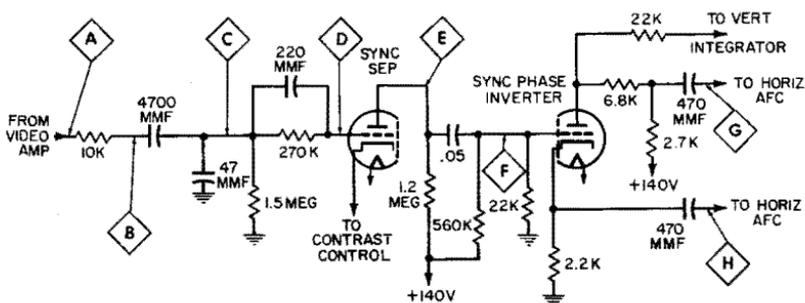
Fig. 4-12. Sync-separator and phase-inverter configuration.
