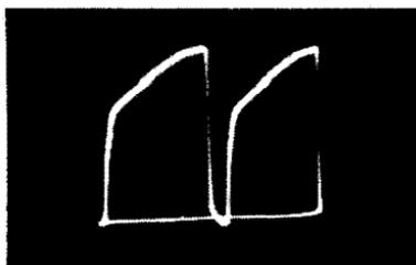
Fig. 5-12. Normal output waveform from horizontal oscillator.
