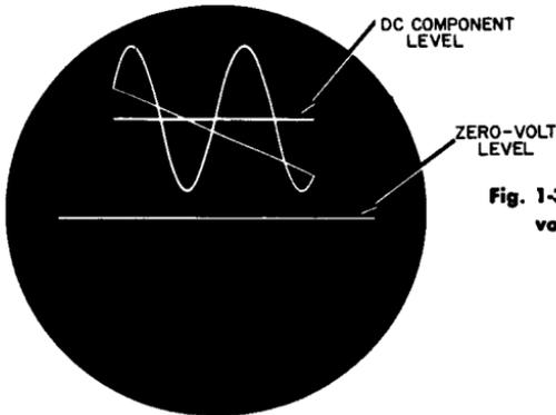
**Fig. 1-37. Response of DC scope to AC voltage with a DC component.**
