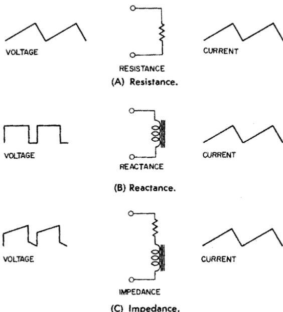
Fig. 6-3. Voltage waveforms needed for a sawtooth current.
