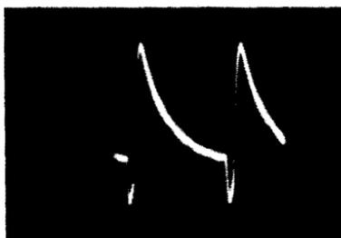
Fig. 5-8. Waveform at (B) when C3 is open.
