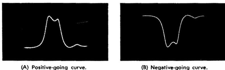
Fig. 2-12. Sweep-alignment curves.
