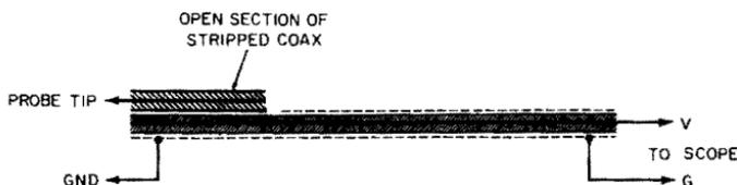
Fig. 6-10. Special high-voltage capacitance-divider probe.
