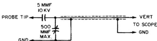
Fig. 2-8. Configuration of a typical high-voltage capacitance-divider probe.
