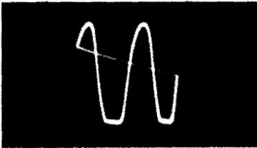
**Fig. 8-10. Negative peak clipping of the audio signal.**
