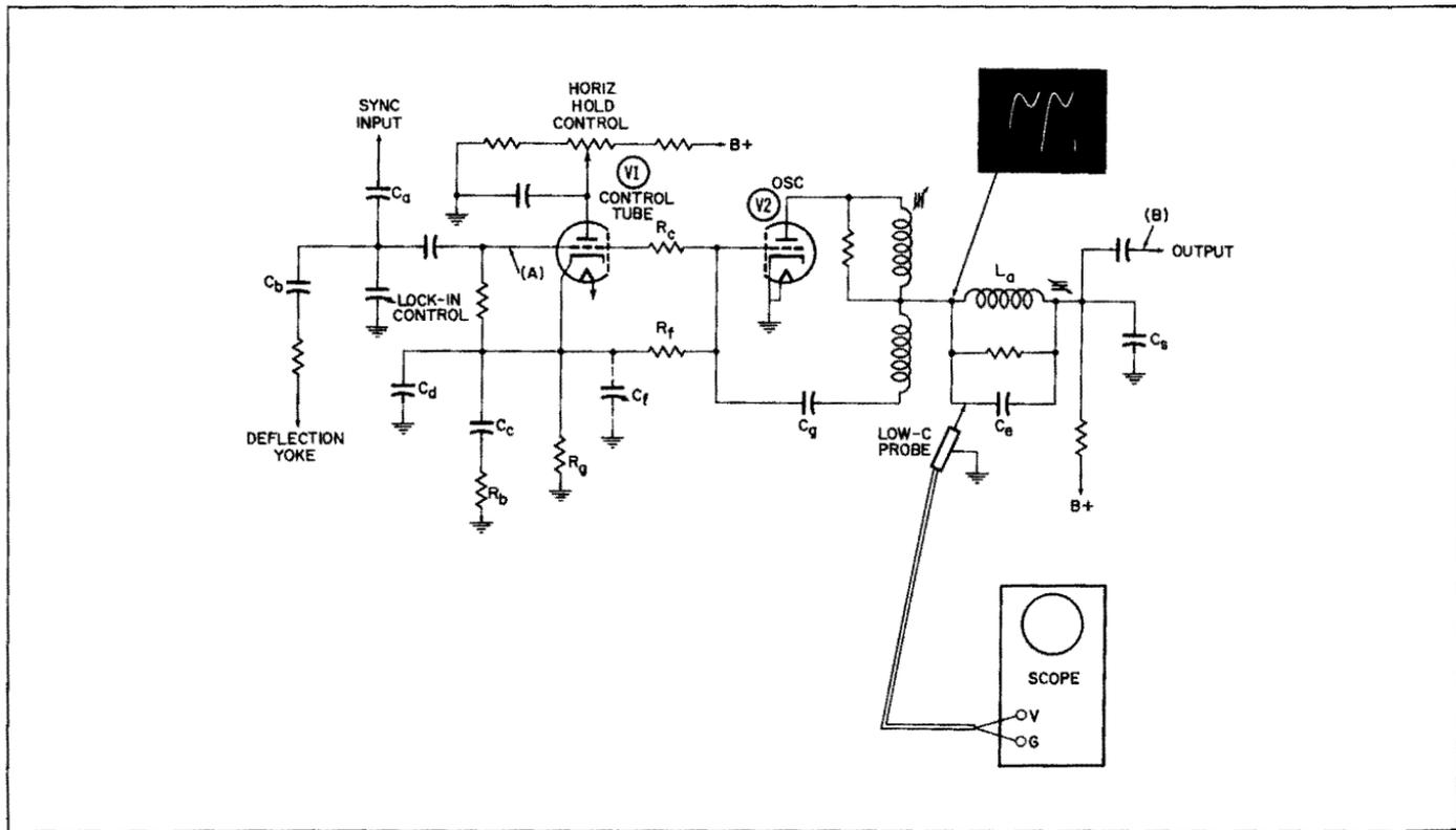
If the pulse moves slightly to the left on the sawtooth, more of the pulse appears on top thus making the conduction interval longer. In turn, more positive bias is generated and the oscillator speeds up. The sawtooth then pulls to the right, part of the pulse is lost, and, effectively, the pulse width decreases. Equilibrium occurs at the width which keeps the sawtooth frequency exactly in step with the sync pulse.
