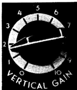
Fig. 1-15. Vertical-gain control incorrectly set.
