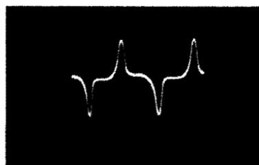
Fig. 9-6. Pulse-current flow without a sine-wave component.
