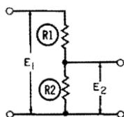
$$E_2 = E_1 \frac{R_2}{R_1 + R_2}$$
