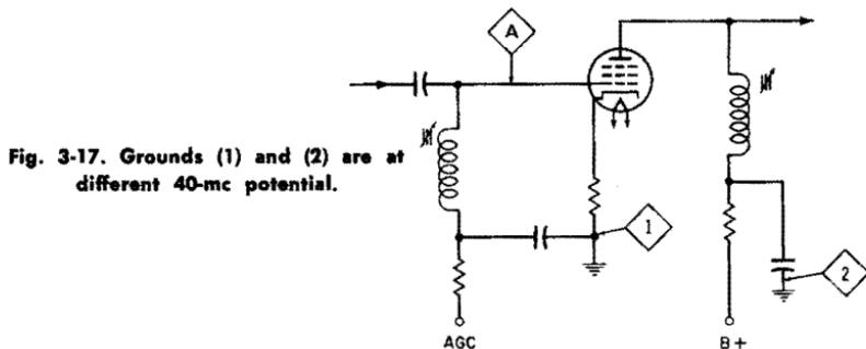
Fig. 3-17. Grounds (1) and (2) are at different 40-mc potential.
