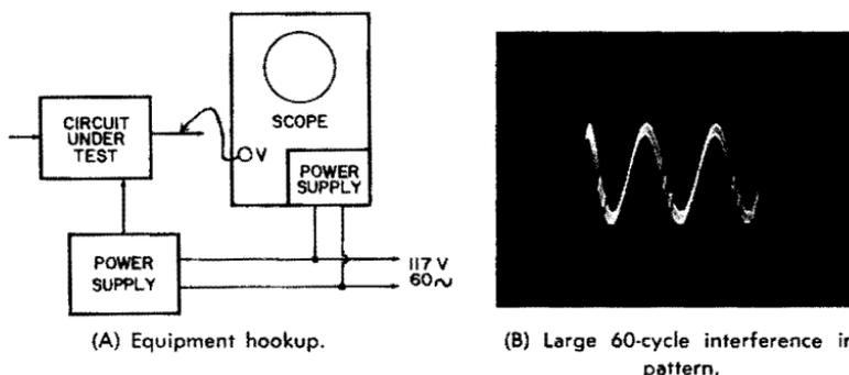
Fig. 2-17. Effect of ground-return lead to scope omitted.
