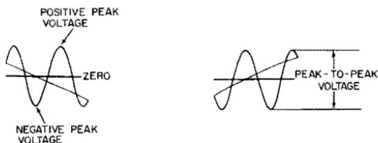
**Fig. 1-30. Meaning of positive-peak, negative-peak, and peak-to-peak voltages.**
