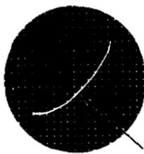
Fig. 1-28. Nonlinear amplification present.
