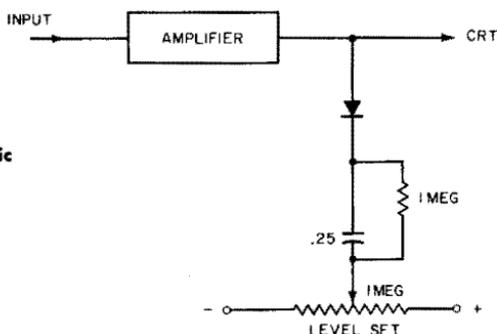
Fig. 4-10. Circuit for automatic centering.
