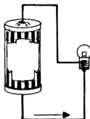
Fig. 2-18. If one of the leads is omitted, the lamp does not light.
