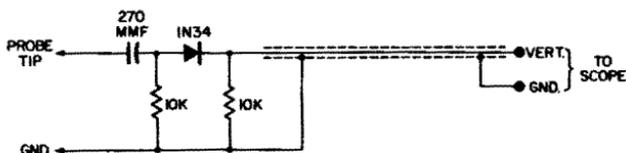
Fig. 2-5. A compromise type of demodulator probe.
