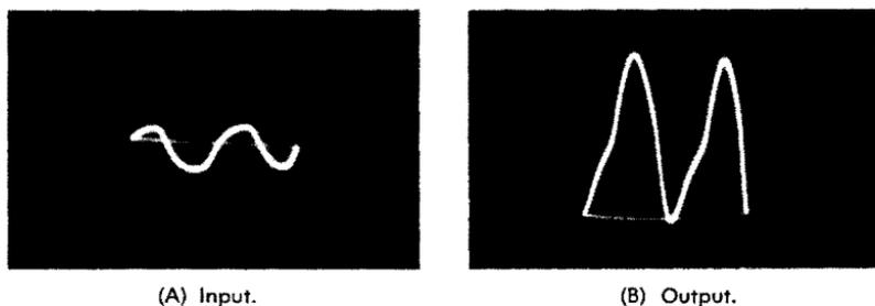
Fig. 10-8. Gain check of an audio-output stage.
