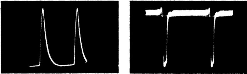
Fig. 4-15. Sync-separator outputs from two different receivers.
