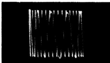
and tune the generator for the same number of peaks. The reading on the generator dial is then the same as the oscillator frequency. In normal operation, the oscillator frequency will differ from the RF input frequency by 455 kc. Even though the receiver dial may not be highly accurate, this procedure serves as a rough guide in evaluating oscillator operation.
