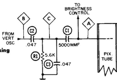
Fig. 7-14. Vertical-retrace blanking circuit.
