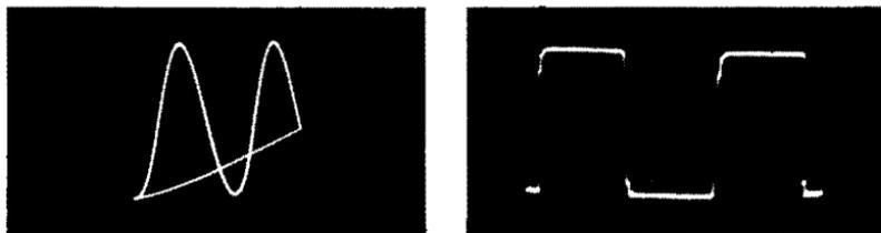
Fig. 1-34. These waveforms have the same peak-to-peak voltages, but their rms values are different.
