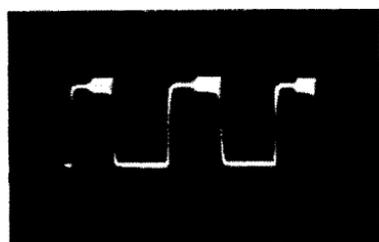
Fig. 11-16. Parasitic oscillation occurring in square-wave tests.
