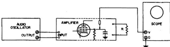
Fig. 11-6. Checking a screen-bypass capacitor.
