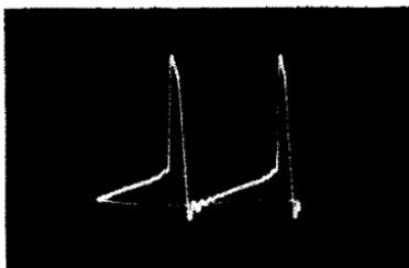
Fig. 6-9. Distorted waveform at point E resulting from increase in value of R5.
