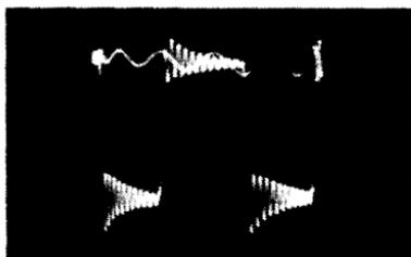
Fig. 11-15. Severe ringing occurring in square-wave pattern.
