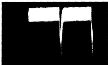
Fig. 4-16. Excessive residual video in the stripped-sync waveform.
