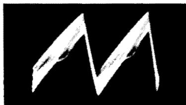
Fig. 5-5. Sawtooth waveform from horizontal-oscillator circuit, when coupling capacitor is leaky.
