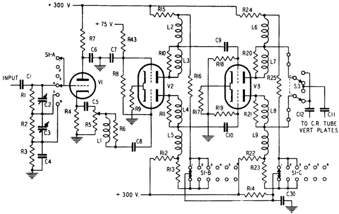
used to balance the high- and low-frequency response. These capacitors are maintenance adjustments, and are located inside the scope case.
