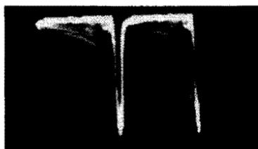
lock is lost completely, and the picture rolls. The vertical-sync pulse is completely unable to couple into the phase-inverter grid via stray capacitance, while a residue of horizontal sync does transfer.
