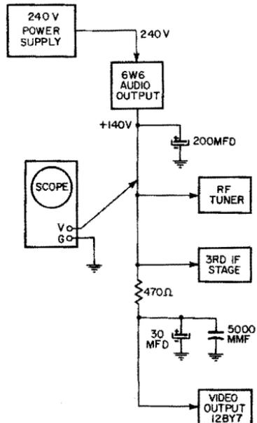
Fig. 9-1. Audio-output tube is also used as a B+ voltage divider.
