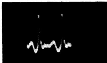
(B) Distorted wave, using demodulator probe.
