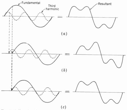
FIG. 11-13. How phase distortion changes the resultant signal wave shape. (a) Fundamental and third harmonic in phase. (b) Fundamental delayed by  $60^{\circ}$  and third harmonic with 120° delay. (c) Fundamental delayed by  $60^{\circ}$  and third harmonic with 180° delay.
