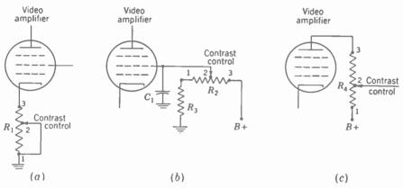
Fig. 11-7. Types of manual contrast control in a video amplifier. (a) Variable cathode bias. (b) Variable screen-grid voltage. (c) Potentiometer to tap off the desired amount of  $\mathbf{a}$ -c video signal voltage.
