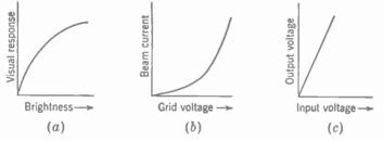
FIG. 5-14. Gamma characteristics. (a) Visual response of the eye. Gamma is less than one; (b) control-grid characteristic curve of picture tube (here gamma is more than one—equal to 2.2 in this case); (c) linear characteristic of amplifier: gamma equals one.
