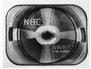
FIG. 21-4. Reproduced picture of test pattern, with ghost to the right caused by reflected signal. (From McGraw-Hill motion-picture series, Basic Television.)
