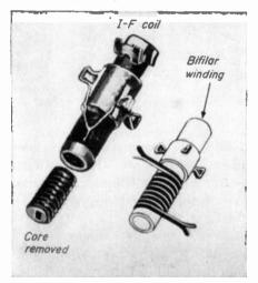
Fig. 19-11, Construction of a bifilar i-f coil. (*RCA*.)
