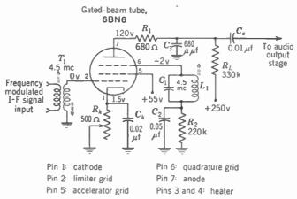
FIG. 22-13. Gated-beam tube circuit for limiting and FM detection. I-F center frequency is 4.5 Mc. Connections shown for 7-pin miniature glass tube 6BN6. (From Zenith K Series chassis.)
