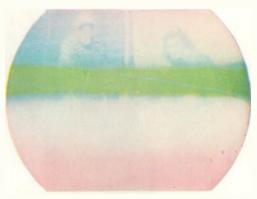
PLATE II. 60-eps hum voltage in the Q signal. (RCA.)
