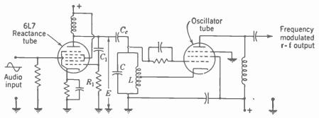
FIG. 7-4. Reactance-tube modulator for producing FM. The quadrature network  $R_1C_1$ , tuned circuit LC, and plate-to-cathode circuit of the reactance tube are effectively in parallel, with the voltage E across all three branches, since the coupling condenser  $C_c$  and cathode condenser bypass have no appreciable reactance at the operating frequency.
