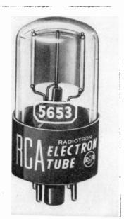
FIG. 2-3. A typical vacuum phototube. The average cathode current for such a tube is several microamperes with an anode voltage of 100-250 volts. (*RCA*.)
