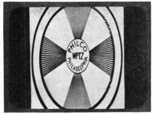
FIG. 17-22. Insufficient width. (Philco Corporation.)
