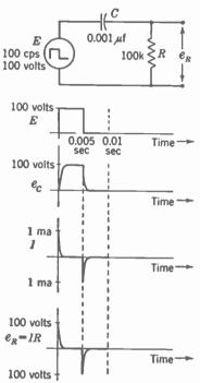
FIG. 16-9. Charge and discharge of an RC circuit with a short time constant.
