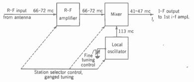
FIG. 20-1. Block diagram of r-f tuner. Oscillator frequency indicated for tuning in channel 4, in a receiver with picture i-f carrier of 45.75 Me.
