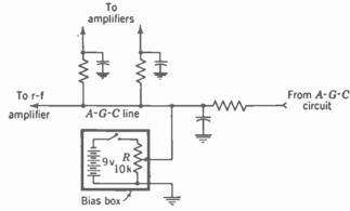
FIG. 15-10. Bias box connected to a-g-c line.
