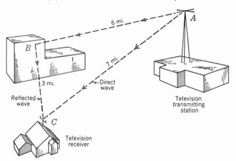
FIG. 21-5. Reception of multipath signals. The reflected wave distance ABC is 2 miles longer than the direct path AC.
