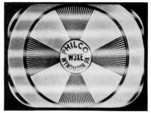
FIG. 19-13, Sound in the picture. The frequency of the audio signal interference at the kinescope grid is about 360 cps. (*Philco Corporation.*)
