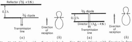
FIG. 21-13, Dipole with reflector in back of antenna. (a) Spacing of elements. (b) Directional pattern,
