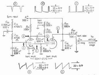
FIG. 17-17. Vertical deflection oscillator using the cathode-coupled multivibrator, with typical wave shapes. (*Belmont Radio Corporation.*)
