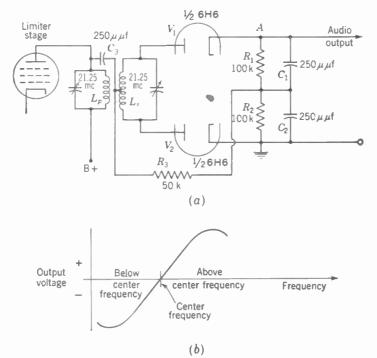
FIG. 22-4. Phase-shift discriminator for an i-f center frequency of 21.25 Mc. (a) Circuit, (b) Response curve.
