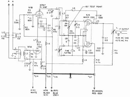
FIG. 20-18. Schematic diagram of v-h-f turret tuner with cascode r-f amplifier and twin-triode mixer-oscillator. Photo of tuner shown in Fig. 20-2. Resistance values in ohms and capacitance in  $\mu\mu f$ . (Standard Coil Products Co., Inc.)
