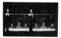
FIG. 11-20. Oscillogram of composite video signal. Oscilloscope internal sweep at 15,750/2 cps to show video signal for two horizontal scanning lines. Horizontal synchronizing pulses at top of waveform.
