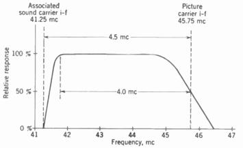
FIG. 19-2. Desired response curve of amplifier with picture i-f of 45.75 Me.
