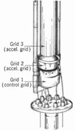
FIG. 3-3. Construction of an electron gun. (RCA.)
