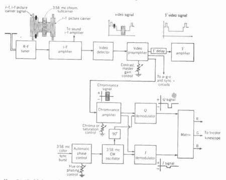
FIG. 24-15. Main sections of color television receiver. Signal wave shapes shown for vertical green bar on gray background.
