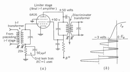
FIG. 22-8. Amplitude limiter for an FM receiver. Input and output circuits tuned to the i-f center frequency of the FM signal. (a) Circuit. (b) Constant plate-current characteristic for different grid-voltage amplitudes.
