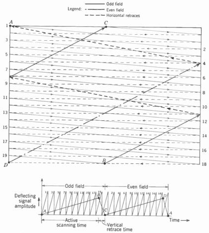
FIG. 4-4. A sample scanning pattern for 21 interlaced lines, with the required sawtooth deflecting signals. Beginning at point A the scanning motion is continuous through  $B_iC_iD_i$ , and back to A again.
