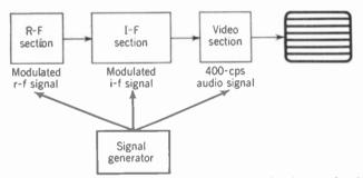
FIG. 23-14. Using generator to inject test signal in picture circuits.
