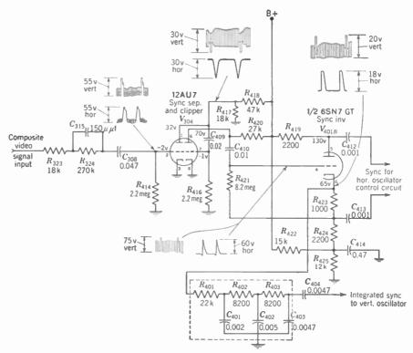
FIG. 16-20. Syne separation circuit with grid-leak bias separator, clipper, and phase inverter stages. Vertical wave shapes can be observed on oscilloscope with internal sweep frequency at 30 cps, horizontal at 15,750/2 cps. Wave-shape amplitudes are peak-to-peak voltage. Capacitance values less than 1 in  $\mu$ f, more than 1 in  $\mu\mu$ f. (Admiral Series 21 chassis.)
