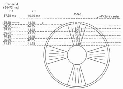
FIG. 19-3. A resolution chart to illustrate the continuity of r-f, i-f, and video signal frequencies for channel 4.
