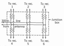
FIG. 21-33. Parallel distribution system for feeding signal from one antenna to multiple receivers from common junction box. All resistors are 750 ohms for six receivers with 300-ohm input impedance.
