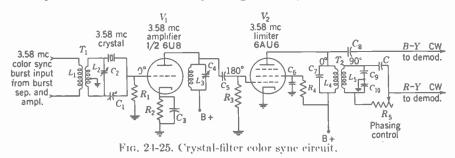
*control*, is usually available on the receiver's front panel to be adjusted for the correct hue of a known object. Proper flesh tones, as an example, provide a good guide in adjusting the phasing control for correct hues.
