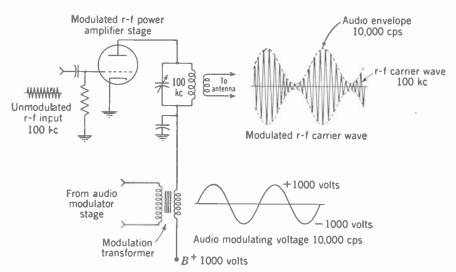
FIG. 6-2. A plate modulation arrangement for amplitude modulation of a 100-ke carrier wave by 1000-cps audio modulating voltage.
