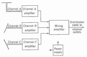
Fig. 21-34. Illustrating a master antenna distribution system using amplifiers.
