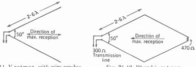
FIG. 21-11. V antenna, with wire conductors for the legs.
