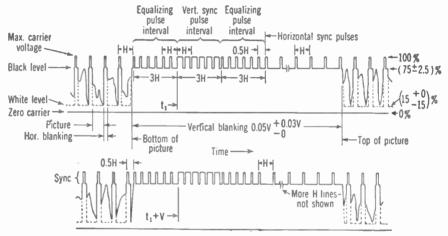
FIG. 5-5. Sync and blanking pulses for successive fields. V equals 160 sec.
