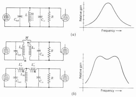
F16. 19-6. Basic picture i-f coupling circuits. (a) Single-tuned. (b) Double-tuned with inductive coupling.
