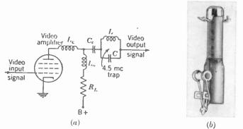
FIG. 23-9. 4.5-Mc parallel resonant trap circuit in the video amplifier. (a) Trap connected in series with output circuit. (b) Photo of typical trap. (RCA.)
