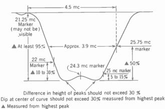
FIG. 23-16. I-F response curve for receiver in Fig. 23-15. (Admiral Corporation.)
