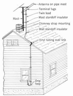
FIG. 21-31. An antenna installation.
