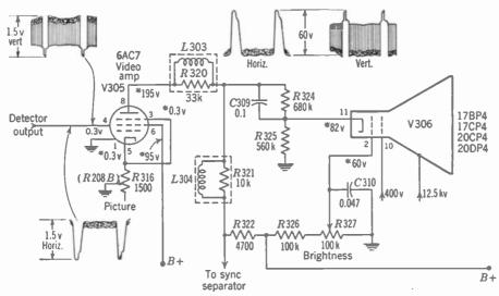
FIG. 11-21. Single-stage d-c video amplificr circuit. Capacitance values in microfarads and resistances in ohms, unless otherwise noted. Voltage values marked with asterisk vary widely with setting of controls. (Admiral Series 21 chassis.)
