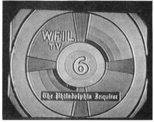
FIG. 11-29. Test pattern with outline distortion caused by ringing in the video amplifier. (RCA Pict-O-Guide.)
