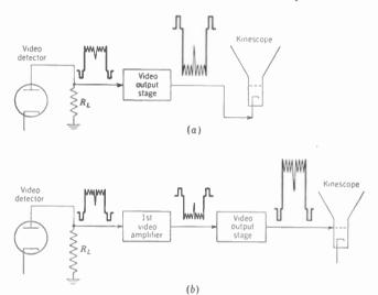
Fig. 11-4. Polarity of the video signal for the kinescope. (a) Negative picture phase at kinescope cathode. (b) Positive picture phase at kinescope grid.
