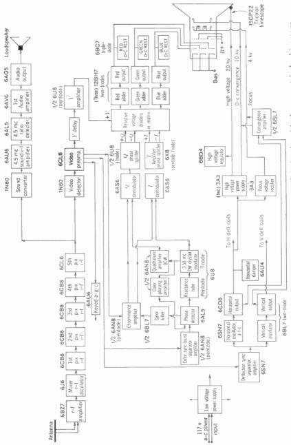
Fig. 24-33. Block diagram of typical color television receiver for I and Q signals, with three-gun tricolor kinescope.
