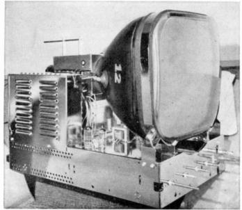
FIG. 1-7. A direct-view table-model television receiver. (Hallicrafters Co.)
