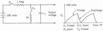
FIG. 16-10. RC circuit with a long time constant on charge and short time constant for discharge. The output across the condenser is a saw-tooth wave of voltage.
