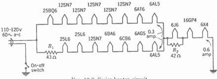
FIG. 10-8. Series heater circuit.
