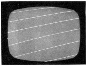
FIG. 11-24. No picture on kinescope screen. Raster is present, without snow.
