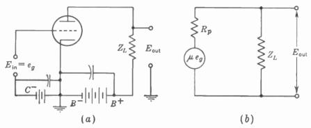
FIG. 12-1. A vacuum-tube amplifier circuit. (a) Typical operation. (b) Equivalent plate circuit.
