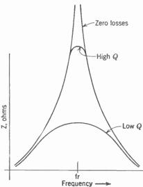
FIG. 19-7. Illustrating the increased bandwidth obtained with an increase in mutual coupling.
