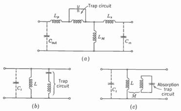
F10, 19-14. Three types of wave-trap circuits for rejecting an undesired signal frequency.
