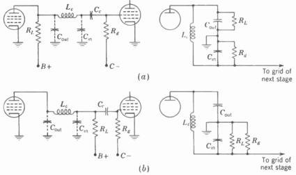
FIG. 12-8. Series peaking. (a) Series peaking circuit and equivalent plate load for  $C_{\rm in} = 2C_{\rm out}$ . (b) Series peaking circuit and equivalent plate load for  $C_{\rm in} = \frac{1}{2}C_{\rm out}$ .
