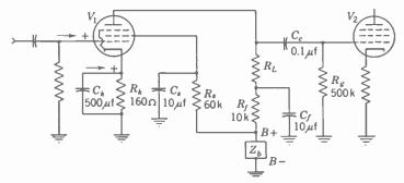
FIG. 12-11. Sources of low-frequency distortion in the conventional resistance-coupled amplifier are cathode bypass condenser  $C_k$ , screen bypass  $C_k$ , power-supply impedance  $Z_{b_1}$  and coupling circuit  $R_gC_c$ .
