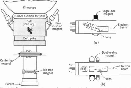
FIG. 9-5. Centering magnet mounted on kinescope.
