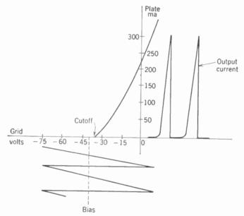
FIG. 18-14. Operation of horizontal output tube as class C amplifier. Saw-tooth plate current flows for only part of the input voltage cycle.
