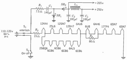
FIG. 10-12. Transformerless low-voltage power supply.
