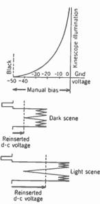
FIG. 13-8. Video signals on the kinescope grid with the pedestals in line at cutoff because of the d-c reinsertion. Manual brightness control set at cutoff.
