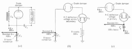
FIG. 18-19. Producing the boosted B + voltage. (a) Diode damper in secondary circuit of horizontal output transformer. Component part numbers are the same as in Fig. 18-12. (b) Equivalent circuit of a, with diode damper in secondary circuit. (c) Diode damper in primary circuit, where a-e deflection voltage has opposite polarity, and B + boost condenser returns to B + instead of ground.
