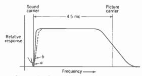
FIG. 19-4. Response for associated sound i-f carrier frequency in pieture i-f amplifier. (a) Practically zero response for receivers with separate sound i-f amplifier. (b) 2 to 5 per cent response in common i-f amplifier of intercarrier-sound receivers.
