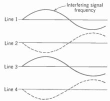
FIG. 24-11. Chrominance interlace for a frequency exactly an odd multiple of one-half the horizontal line-scanning frequency. Solid lines represent first and odd vertical scanning fields; dotted lines second and even fields. Missing part of sine wave corresponds to horizontal flyback time.
