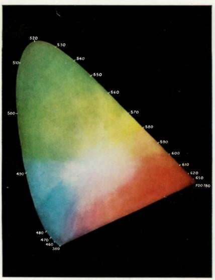
PLATE VIII. Hue and saturation values for red, green, blue, and their color mixtures. In terms of the rectangular coordinates in the chromaticity diagram in Fig. 24-38, the lowest point on the horseshoe curve at darkest blue has the approximate coordinates x = 1.7, y = 0.1; the highest point of green is x = 0.8, y = 8.4; the darkest red at the right is x = 7.3, y = 2.7. (RCA.)
