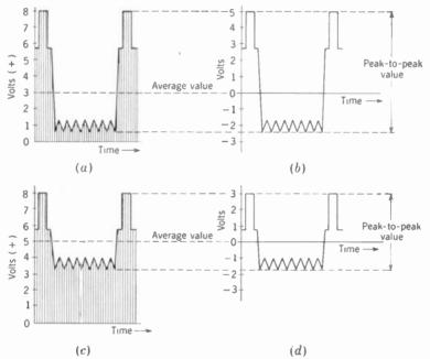
FIG. 11-3. Peak-to-peak value of the video signal. (a) D-c form for a white video signal. (b) A-c form for the same white video signal. (c) D-c form for a gray video signal. (d) A-c form for the same gray video signal.
