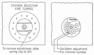
FIG. 20-15. R-F oscillator adjustments. (a) Removing escutcheon plate. (b) Location of coil slugs. Channel 13 adjustment on top of tuner. (*RCA KRK-11 R-f unit.*)
