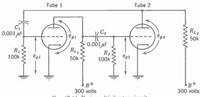
FIG. 17-14, Basic multivibrator circuit.
