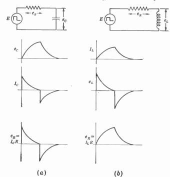
FIG. 16-11. Comparison of wave shapes in RC and RL circuits. The current in the RL circuit cannot change instantaneously but must build up or decay exponentially in the same manner as the condenser voltage in the RC circuit. (a) RC circuit. (b) RL circuit.
