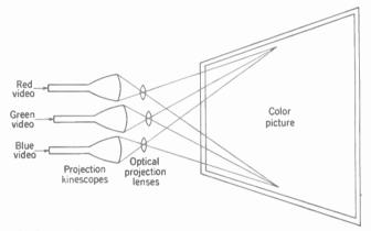
FIG. 24-26. Optical projection arrangement for three color kinescopes.
