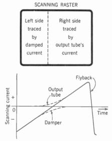
FIG. 18-18. Illustrating how the damped current and output current combine to produce horizontal scanning in the raster.
