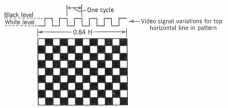
FIG. 5-7. Checkerboard pattern and corresponding camera signal variations.
