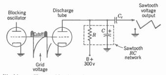
FIG. 17-5. Blocking oscillator grid voltage driving discharge tube to produce saw-tooth voltage output across saw-tooth condenser C in plate of discharge tube. Shaded area in grid-voltage waveform indicates when the discharge tube conducts.
