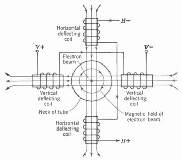
FIG. 3-10. Two pairs of coils around the neck of the cathode-ray tube for horizontal and vertical electromagnetic deflection. The electron beam will be deflected upward and to the left for the directions of current shown.
