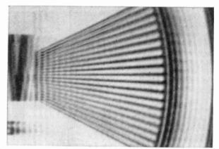
F1G, 19-22, Multiple outlines in picture caused by regeneration in the i-f amplifier,  $(RCA_{+})$
