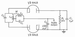
FIG. 22-12. Single-ended ratio detector circuit.
