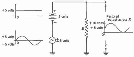
FIG. 13-7. Illustrating positive d-c insertion.
