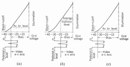
FIG. 13-1. The d-e bias on the kinescope grid determines the average brightness or background of the reproduced picture. (a) Correct bias. (b) Too little negative bias. (c) Too much negative bias.
