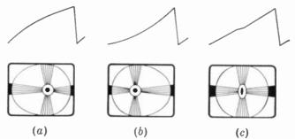
FIG. 18-26. Effects of nonlinear horizontal scanning, with corresponding distorted saw-tooth current wave shape. (a) Stretching at the left side and crowding at the right. (b) Crowding at the left side and stretching at the right. (c) Crowding at the center.
