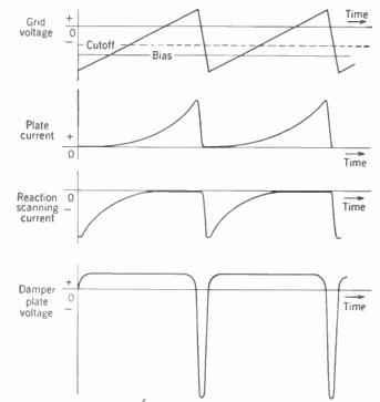
FIG. 18-17. Comparison of waveforms in the horizontal output stage, for two scanning lines.
