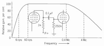
Fig. 11-16, Typical response curve for the RC-coupled amplifier,
