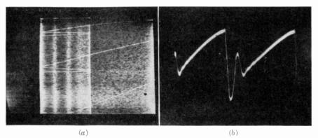
FIG. 18-9. Effect of insufficient damping in horizontal output circuit. (a) Wide white vertical bar at left side of raster caused by oscillation. (b) Oscillogram of current in horizontal deflection coils with oscillations. Oscilloscope internal sweep at 15,750/2 cps. (*RCA Institutes, Inc.*)
