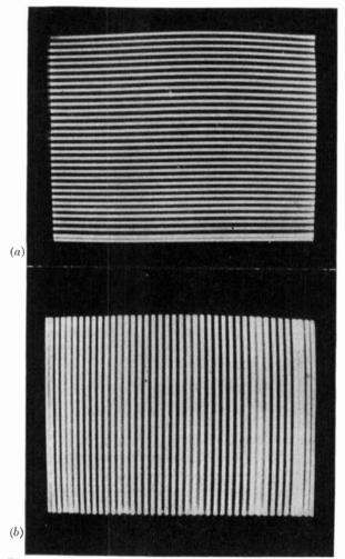
FIG. 18-34. Bar patterns on kinescope screen obtained with signal generator. (a) Horizontal bars to check vertical scanning linearity. (b) Vertical bars to check horizontal scanning linearity. (From Donald G. Fink, Television Engineering, McGraw-Hill Book Company, Inc.)
