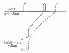
FIG. 17-25. Effect of injecting positive d-c grid voltage to increase the frequency of blocking oscillator, or multivibrator, Dotted wave is lower frequency without the added d-c voltage.
