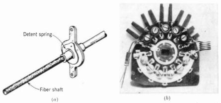
FIG. 20-22. Detent for rotary-switch-type tuner and one switch-wafer section. (a) Detent. (b) Switch wafer for oscillator section. Screws are oscillator frequency adjustments for individual channels. (From RCA KRK-2 R-f unit.)
