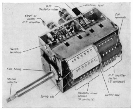
Fig. 20-2. Typical turret-type r-f tuner, with individual coil strips for each channel. Bottom shield cover and tube shields removed to show components. Schematic diagram shown in Fig. 20-18. (*Standard Coil Products Co., Inc.*)
