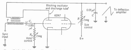
FIG. 17-12. Blocking oscillator and discharge tube circuit combined in one stage. Component values given are for vertical deflection oscillator, but same circuit can be used with different components for horizontal deflection oscillator.
