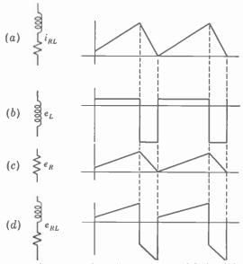
FIG. 17-19. For saw-tooth current, the voltage across an RL circuit has the trapezoidal wave shape shown in d. (a) Saw-tooth current through RL circuit. (b) Rectangular voltage across inductance. (c) Saw-tooth voltage across resistance. (d) Combined voltage across R and L in series.
