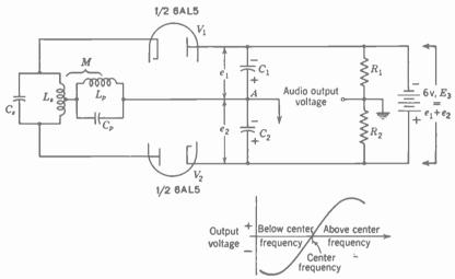
FIG. 22-9. Basic ratio detector circuit and its response curve. Just as in the phase-shift discriminator, the primary and secondary of the coupling transformer are tuned to the i-f center frequency of the FM signal.
