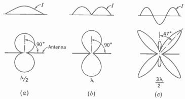
Fig. 21-7. Directional characteristics of dipole antenna connected to transmission line at center, with distribution of current I on antenna. (a) Figure-eight pattern at half-wave resonance. (b) Broadened response at twice the resonant frequency. (c) Lobes split because of operation as harmonic antenna at three times the resonant frequency.
