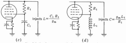
FIG. 7-5. Quadrature networks for a reactance tube.
