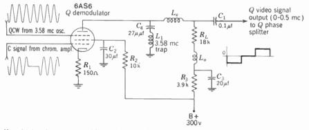
F16, 24-19, Suppressor-grid synchronous detector circuit for I or Q demodulator stage. Wave shapes illustrated for yellow, white, and blue information.
