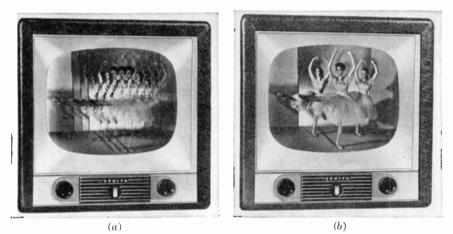
FIG. 8-9. Picture reproduction in Phonevision system. (a) Without coding signal at receiver. (b) With coding signal. (Zenith Radio Corp.)
