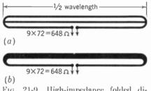
FIG. 21-9. High-impedance folded dipole antennas. (a) With additional closed conductor section. (b) With wider-diameter closed conductor section.
