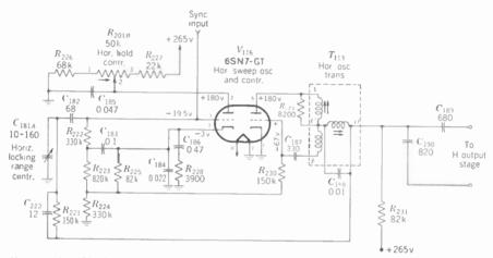
FIG. 17-29. Horizontal blocking oscillator circuit with stabilized Synchro-Guide. Capacitance values more than one in  $\mu\mu$ f and less than one in  $\mu$ f; resistance values in ohms unless otherwise noted. Direction of arrows at controls indicates clockwise rotation, (*RCA KUS66 chassis.*)
