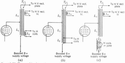
FIG. 18-27. Types of horizontal output transformer circuits. (a) Separate secondary winding. (b) Autotransformer. (c) Direct-drive, with horizontal deflection coils in primary plate circuit.
