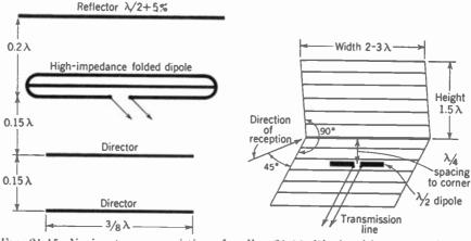
FIG. 21-15. Yagi antenna, consisting of dipole with one reflector and two directors.
