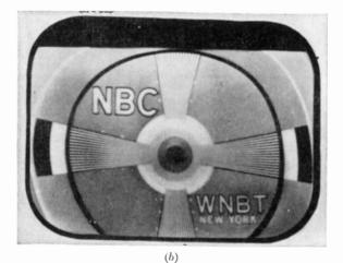
FIG. 23-4. Raster off center, (a) horizontally and (b) vertically. (RCA.)
