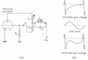
FIG. 17-28. Sine-wave stabilizing tuned circuit in blocking oscillator. (a) Circuit arrangement. (b) Grid waveforms. Dotted-line axis is cutoff voltage.
