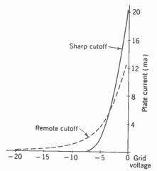
FIG. 15-2. Comparison of the grid-plate transfer characteristic curves of the 6CB6 sharp cutoff pentode and the 6BA6 remote cutoff pentode.
