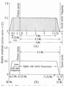
FIG. 6-5. The standard television channel. (a) The generalized structure for any channel; (b) channel 4, 66 to 72 Me.
