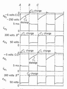
FIG. 17-15. Plate- and grid-voltage waveforms for the multivibrator in Fig. 17-14.
