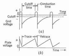
FIG. 17-6. The positive pulse of grid voltage produces flyback in the saw-tooth wave; cutoff corresponds to the linear rise on the saw-tooth wave for the trace. (a) Grid voltage of blocking oscillator and discharge tube. (b) Plate voltage of discharge tube.
