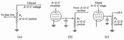
FIG. 15-7. Circuit arrangements for a-g-e level control. (a) Adjusting the bias voltage. (b) Adjusting the input voltage to the a-g-e amplifier. (c) Adjusting the screen-grid voltage of the keyed a-g-e tube.
