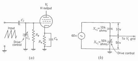
FIG. 18-21. The horizontal drive control varies the amount of saw-tooth voltage input to the grid of the deflection amplifier. (a) Circuit diagram, with component part numbers the same as in Fig. 18-12. (b) Equivalent a-c voltage divider.
