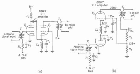
F1G. 20-9. Driven grounded grid, or cascode, r-f amplifier circuits. (a) A-C coupling between the two triode sections. (b) Direct-coupled.
