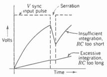
FIG. 16-14. Difference in integrated output between even and odd fields with no equalizing pulses. The dotted waveform in the upper figure is the lower waveform superimposed. The horizontal dashed lines in both figures represent the level to which the condenser voltage must rise to trigger the vertical scanning generator.
