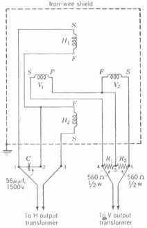
FIG. 18-30. Deflection-yoke wiring connections, with damping network connected across output terminals in yoke. S is start and F finish of winding.
