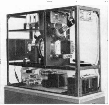
FIG. 2-9. Inside view of an iconoscope camera for film. Note back-light housing at left; rim light not shown. (Allen B. Du Mont Laboratories, Inc.)
