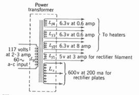
FIG. 10-6. Filament windings on low-voltage power-supply transformer.
