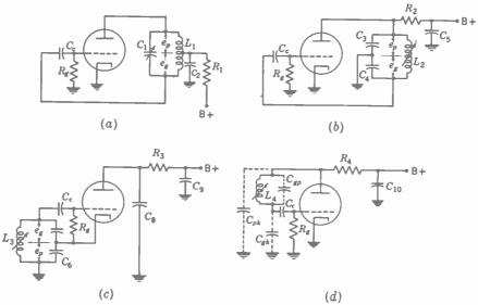
FIG. 20-11, Four typical oscillator circuits. (a) Hartley oscillator with grounded cathode. (b) Colpitts oscillator with grounded cathode. (c) Colpitts oscillator with grounded plate. (d) Ultraudion oscillator.
