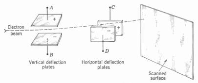
FIG. 3-8. Electrostatic deflection.
