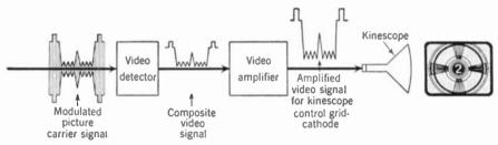
FIG, 11-1. The video signal coupled to the kinescope control-grid cathode circuit produces the picture on the raster.
