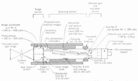
FIG. 2-11. Construction of the image orthicon. All potentials are with respect to zero volts at the cathode of the electron gun.
