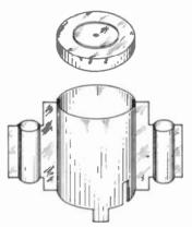
FIG. 3-2. Control-grid cylinder with aperture disk. (Sylvania Electric Products, Inc.)
