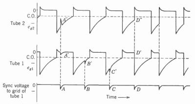
FIG. 17-18. Waveforms of grid voltage in multivibrator synchronized by negative pulses. The oscillator is pulled in to the synchronizing frequency at time D,
