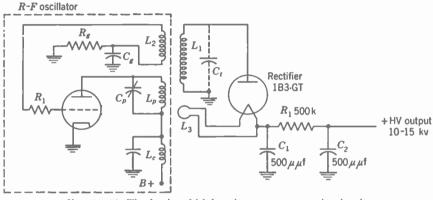
FIG. 10-13. The basic r-f high-voltage power-supply circuit.
