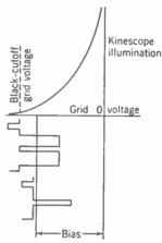
FIG. 13-6. Pedestals out of line on the kineseope grid, for the two lines of video signal in b and c of Fig. 13-5. A single value of bias cannot be correct for both signals.
