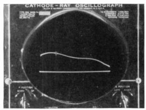
FIG. 20-16. R-F response curve for channel 12, with marker at picture r-f carrier frequency of 205.25 Mc. (From McGraw-Hill motion-picture series, Basic Television.)
