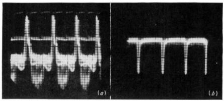
FIG. 16-3. Oscillograms of the composite video signal and separated sync. Only horizontal sync is evident with the oscilloscope internal sweep frequency at 15,750/4 cps, but vertical sync and equalizing pulses are also in the signal. (a) Video signal with positive sync polarity. (b) Separated sync with negative polarity. (RCA.)
