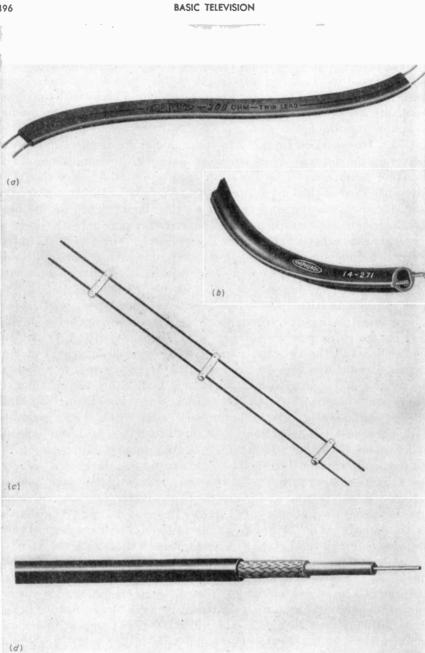
FIG. 21-24. Common types of transmission line. (a) 300-ohm flat, or ribbon, twin lead. (b) 300-ohm tubular twin lead. (American Phenolic Corporation.) (c) 450-ohm open-wire line. (Gonset Company.) (d) 72-ohm coaxial line. (American Phenolic Corporation.)
