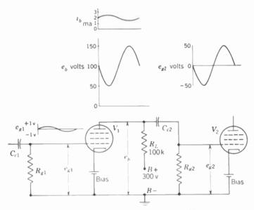
Fig. 11-5. Phase inversion in an amplifier.
