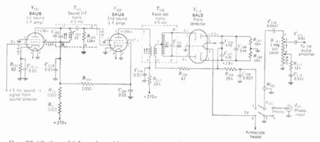
FIG. 22-18. Sound i-f section of intercarrier-sound receiver with ratio detector. Resistance value in ohms, capacitance values less than one in  $\mu$ f and above one in  $\mu\mu$ f, unless otherwise noted. (*RCA KCS 78H chassis.*)
