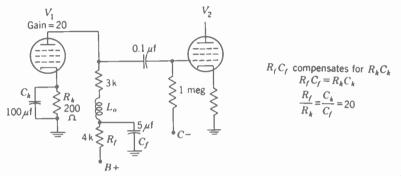
FIG. 12-14, Low-frequency compensating filter with values to correct for the  ${\it cathode}$  impedance.
