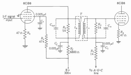
FIG. 19-5. Picture i-f amplifier stage with double-tuned transformer.
