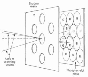
FIG. 24-28. Relationship of shadow mask to phosphor-dot trios. (RCA.)
