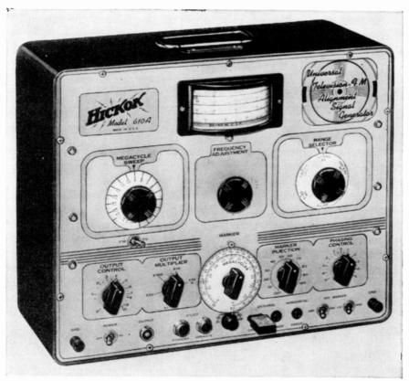
FIG. 19-16. TV sweep generator for alignment. R-F range 30 to 230 Mc;output up to 0.5 volt; 4.5 Mc crystal for intercarrier-sound i-f alignment; sweep width 15 Mc or 1.5 Mc; sweep rate 60 cps; marker absorption dip or oscillating pip frequency range 19 to 48 Me. (*Hickok Electrical Instrument Company.*)
