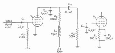
Fig. 11-17, Video amplifier with shunt peaking. Suppressor and screen-grid connections are omitted,
