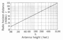
FIG. 6-6. The horizon distance r depends on the antenna height h.
