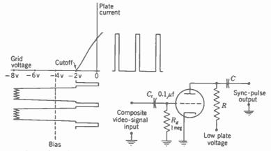
FIG. 16-4. Operation of sync separator using a grid-leak bias clipper amplifier. A pentode can be used instead of the triode.
