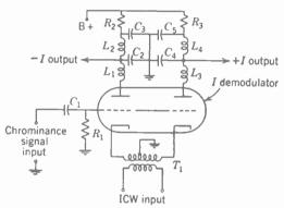
FIG. 24-20. Pulsed-envelope synchronous detector circuit for I or Q demodulator stage.
