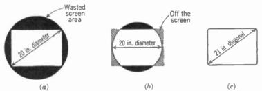
FIG. 9-9. Size of raster on round and rectangular screens. (a) Rectangular raster on round screen. (b) Full-width raster on round screen. (c) Rectangular raster filling rectangular screen.
