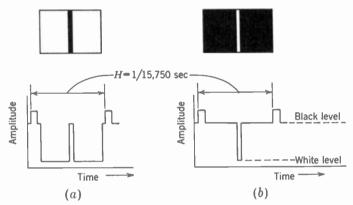
FIG. 5-6. Composite video signal obtained in scanning one line of a pattern containing a vertical line down the center of the frame. (a) Black line on white background; (b) white line on black background.
