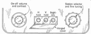
Fig. 8-5. Receiver operating controls. The hinged lid on the front panel normally covers the three controls at the center.
