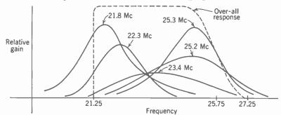
FIG. 19-19. Stagger-tuned response for i-f circuit with picture carrier frequency of 25.75 Mc. The sharp cutoff at 21.25 Mc is produced by the associated sound traps. Effect of traps on individual response curves not shown.
