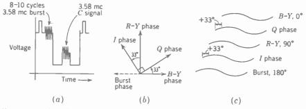
FIG. 24-22. The color sync burst and hue values in terms of its reference phase angle. (a) Burst consisting of 8 to 10 cycles of 3.58-Mc subcarrier; (b) phase angles of vectors for chrominance signals and burst phase; (c) phase angles of one sine wave for chrominance signals and burst phase.
