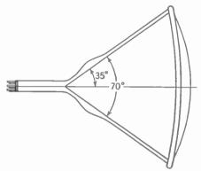
FIG. 9-12. Metal-cone kinescope. (*RCA*.) FIG. 9-13. Kinescope with deflection angle of 70°.
