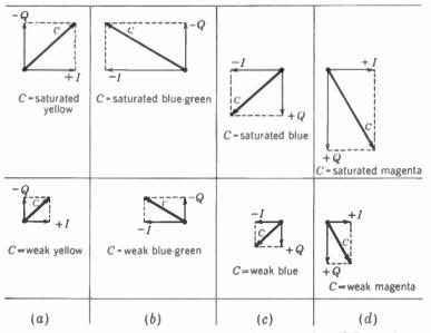
FIG. 24-6. Vector addition of I and Q signal voltages for four different hues. The phase angle of the resultant signal C indicates the hue while its length corresponds to saturation. (a) Yellow; (b) blue-green; (c) blue; (d) red-purple.
