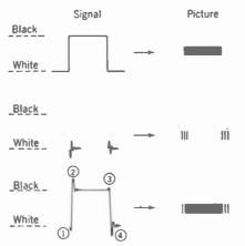
FIG. 11-30. How excessive response for the high video frequencies causes outline distortion.
