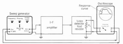
FIG. 19-15. Test equipment and connections for obtaining the visual i-f response curve.
