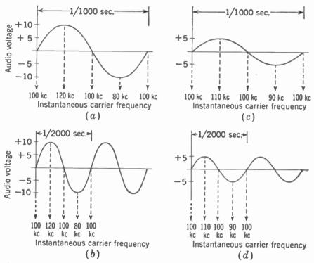
FIG. 7-3. The effect of the audio modulating voltage on the instantaneous frequency of the FM signal.
