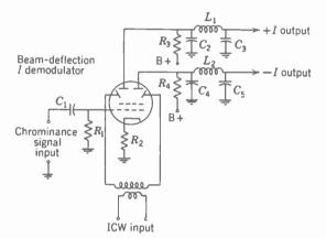
FIG, 24-21, Synchronous detector circuit using beam-deflection tube for I or Q demodulator stage.
