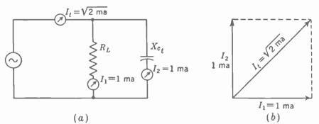
FIG. 12-5. When  $R_L$  equals  $X_{co}$  the total impedance of the high-frequency equivalent plate load circuit is equal to  $(1/\sqrt{2}) \times R_L$ . (a) Plate load connected across an a-c generator. (b) Vector addition of the two branch currents.
