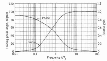
FIG. 12-13. Gain-frequency and phase-angle-frequency response of the uncompensated RC amplifier, as determined by the coupling condenser and grid resistor. At  $F_1$  the response is down 3 db and the leading phase angle is 45°. The leading phase angle at 10  $F_1$  is 6°.
