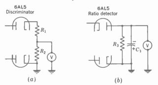
FIG. 22-19. Meter connections to check d-c voltage output of FM detector. (a) Discriminator. (b) Ratio detector.
