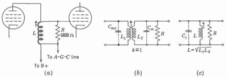
FIG. 19-10. Single-tuned i-f amplifier stage with bifilar i-f coil. (a) Amplifier circuit. (b) Circuit of bifilar coil.  $C_{out}$  is shunt capacitance of amplifier plate circuit, and  $C_{in}$  is grid input capacitance of next stage. (c) Equivalent circuit of bifilar coil.  $C_t$  is total shunt capacitance.
