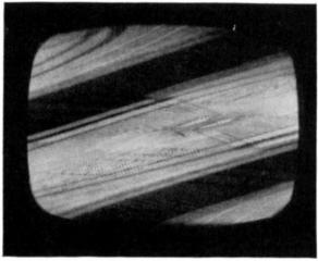
FIG. 16-2. Horizontal scanning not synchronized, resulting in no horizontal hold.
