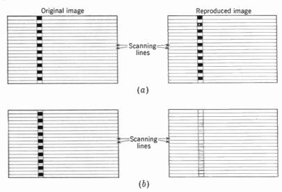
FIG. 5-8. The vertical detail depends on how the scanning lines cover the picture elements. (a) Each scanning line covers an individual vertical detail; (b) the scanning lines straddle the vertical details.
