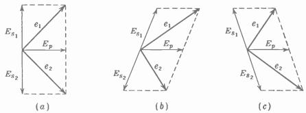
FIG. 22-5. Vector magrams for the phase-shift discriminator as the FM signal varies above and below the i-f center frequency. (a) At center frequency; resonance; 90° phase angle between  $E_p$  and  $E_{s1}$ ;  $e_1 = e_2$ . (b) Above center frequency; above resonance; 70° angle between  $E_p$  and  $E_{s1}$ ;  $e_1 > e_2$ . (c) Below center frequency; below resonance; 110° angle between  $E_p$  and  $E_{s1}$ ;  $e_1 > e_2$ .
