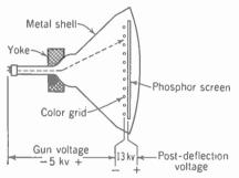
FIG. 24-30. Single-gun, line-screen color kinescope. The chromatron is this type.
