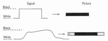
FIG. 11-27. How excessive low-frequency response with phase distortion causes severe smear.
