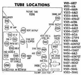
FIG. 23-17. Top view of chassis with tube locations for receiver in Fig. 23-15. (Admiral Corporation.)
