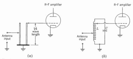
FIG. 20-14. R-F amplifier input circuit using a quarter-wave line as the tuned circuit. (a) Schematic diagram. (b) Equivalent tuned circuit.
