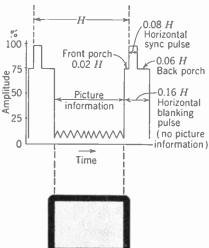
FIG. 5-4. Details of the horizontal blanking and sync pulses. H equals 1/15,750 sec.
