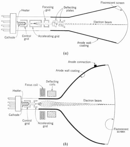
FIG. 3-7. Cathode-ray tubes. Although not shown, electrostatic focus can be used with magnetic deflection or vice versa. (a) Electrostatic cathode-ray tube; (b) electromagnetic cathode-ray tube.
