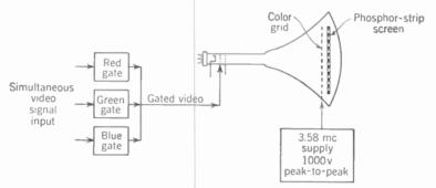
FIG. 24-32. Requirements of gated video signal for control grid and switching voltage for color grid of single-gun, line-screen kinescope.
