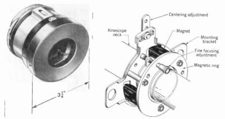
FIG. 9-3. Kinescope deflection yoke. (*RCA*.)
