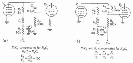
F1G. 12-15. Low-frequency compensation to correct for the reactance of the coupling condenser  $C_c$ . (a)  $R_f C_f$  filter. (b)  $R_f C_f$  and  $R_c$  across  $C_c$ .
