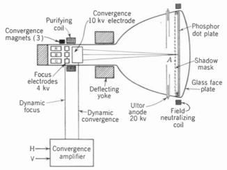
FIG. 24-27, Construction and operating requirements of tricolor kinescope.  $(RCA_{\cdot})$
