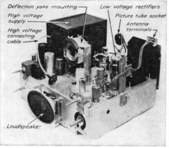
FIG. 8-1. Television receiver chassis. (RCA.)
