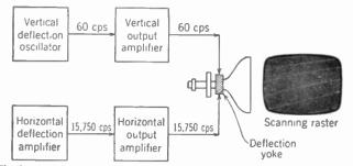
F10. 18-1. The horizontal and vertical deflection circuits produce the scanning raster on the kinescope screen.
