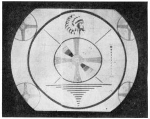
FIG. 18-23. White vertical bar near the center of raster, eaused by excessive horizontal drive.  $(Admiral \ Corporation.)$
