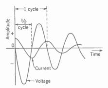
FIG. 18-11. Current and voltage waveforms in the oscillating *LC* circuit.
