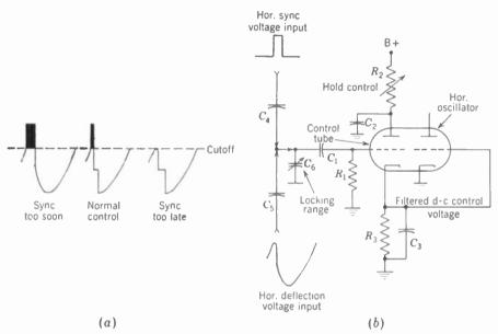
FIG. 17-26. D-C control tube for automatic control of horizontal oscillator frequency, (a) Wave shapes at grid of control tube. The shaded area is effective in producing plate current and control voltage. (b) Circuit arrangement.
