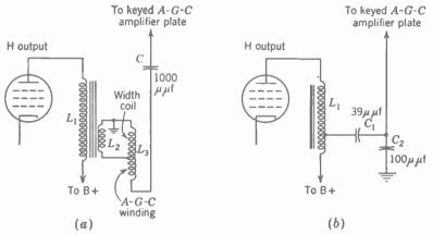
FIG. 18-33. Circuit arrangements for obtaining horizontal flyback pulses for keyed a-g-c amplifier from horizontal output circuit. (a) From a-g-c winding in secondary. (b) With capacitive voltage divider in primary.
