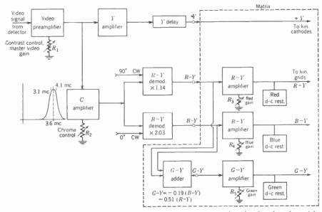
FIG. 24-17, Chrominance circuit for receiver having narrow-band color decoder with matrix for R - Y and B - Y color voltages.
