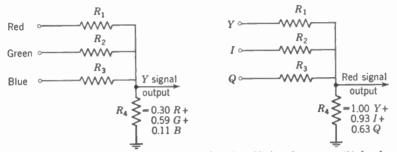
FIG. 24-8. Resistive matrix circuits: (a) for forming Y signal output; (b) for forming red signal output.
