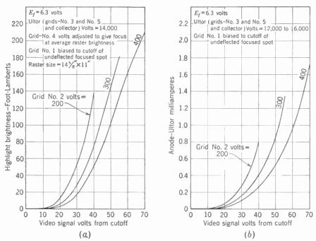
FIG. 9-15. Average grid-drive characteristics of 17TP4 kinescope. (a) Highlight brightness vs. grid drive. (b) Anode-Ultor current vs. grid drive. (RCA.)
