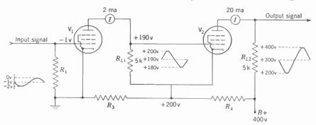
FIG. 11-15. A direct-coupled amplifier. A sine-wave signal is illustrated instead of video signal, and screen-grid voltages are omitted.
