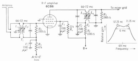
F1G. 20-4. R-F amplifier circuit with r-f response curve showing gain from antenna input to mixer grid, illustrated for channel 4. The resonant circuits are tuned to provide the same r-f response for each channel.
