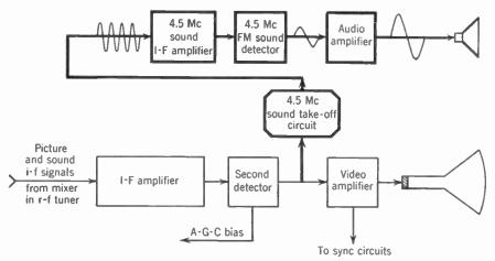
FIG. 8-3. Signal circuits in an intercarrier-sound receiver, showing sound take-off in the second detector output.
