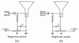
FIG. 13-2. Manual brightness-control circuits. (a) In the control-grid circuit of the kinescope. (b) In the cathode circuit of the kinescope.
