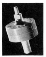
FIG. 10-14. 500  $\mu\mu$ f high-voltage filter condenser. Voltage breakdown rating may be 10 kv or 20 kv. Diameter approximately 1 in. (*Centralab.*)
