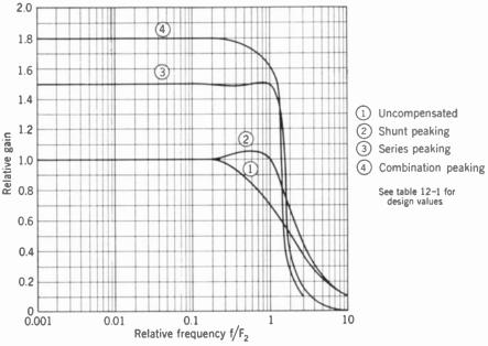
FIG. 12-10. Universal response curves for the video amplifier.
