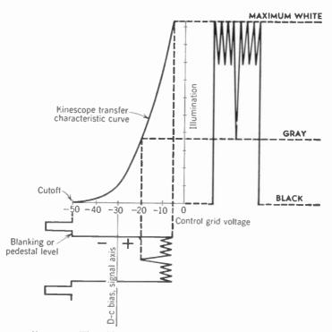
FIG. 11-2. The video signal voltage on the kinescope grid.
