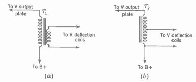
FIG. 18-7. Vertical output transformer connections. (a) Transformer with isolated secondary winding. (b) Autotransformer.
