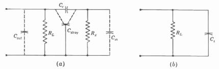
FIG. 12-4. Plate load impedance of the uncompensated video amplifier. (a) Actual circuit. (b) Equivalent circuit.
