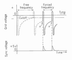
FIG. 17-13. Synchronizing the blocking oscillator.
