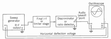
FIG. 22-17. Test equipment and connections to obtain visual response curve of discriminator or ratio detector.
