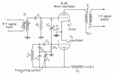
FIG. 20-10. Mixer-qseillator circuit illustrated for a single channel. The r-f transformer  $T_1$  and oscillator coil  $L_0$  are tuned for each selected channel.
