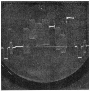
FIG. 24-14*i*. Oscillogram of colorplexed total composite video signal S. From left to right: horizontal sync pulse; 3.58-Mc color sync burst; black, red, yellow, green, eyan, gray, magenta, blue, and white bars. (*Philco Corporation.*)
