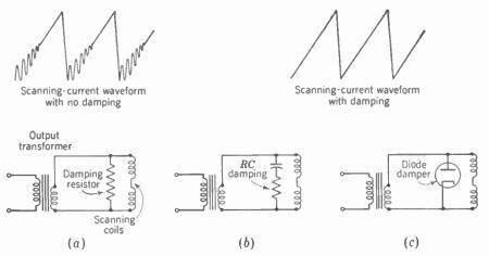
FIG. 18-8. Sine-wave oscillations in saw-tooth deflection current waveform, and methods of damping. (a) Resistor damping. (b) RC damping. (c) Diode damper tube,
