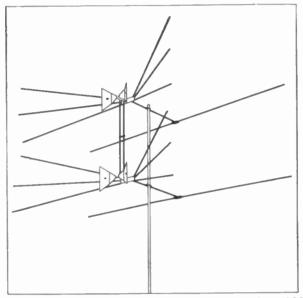
FIG. 21-21. V-H-F fan antenna with u-h-f triangular dipole. (Channel Master Corporation.)
