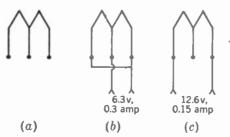
FIG. 10-9. Connections for heater with two sections. (a) Three-pin connections. (b) Parallel connection. (c) Series connection.
