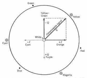
FIG. 24-7. Color wheel showing approximate chrominance values for different combinations of I and Q signal voltage. The -Q voltage is shown upward to conform to color positions on the standard chromaticity diagram in Fig. 24-38, which gives exact chrominance values.
