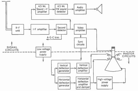
Fig. 8-13. Signal circuits and raster circuits in a typical television receiver.
