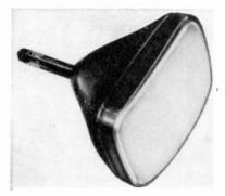
FIG. 1-6. A typical picture tube. The electron-gun structure in the narrow part of the tube produces a beam of electrons that is accelerated to the screen. (Sylvania Electric Products, Inc.)
