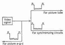
FIG. 14-7. Three functions of the composite video signal.
