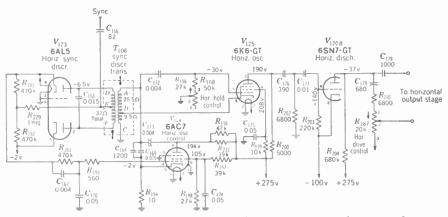
FIG. 17-31. Hartley oscillator with reactance tube. Capacitance values more than one in  $\mu\mu$ f and less than one in  $\mu$ f; resistance values in ohms unless otherwise indicated. Direction of arrows at controls indicates clockwise rotation. (*RCA* 630*TS* and 8*TS*30 chassis.)
