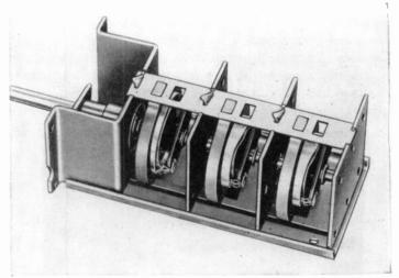
FIG. 20-3. U-H-F inductuner with three ganged spiral-inductance sections. Continuous tuning range covered in  $\frac{3}{4}$  turn of shaft. Height of unit 1.755 in. (*P. R. Mallory and Co.*)
