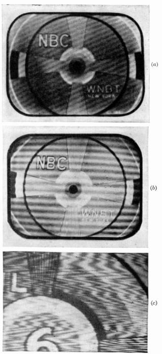
FIG. 23-5. R-F interference effects in the picture. (a) Uniform diagonal bars caused by unmodulated r-f interference. (b) Horizontal bars caused by amplitude modulation. (c) Herringbone-weave effect caused by frequency modulation. (RCA.)
