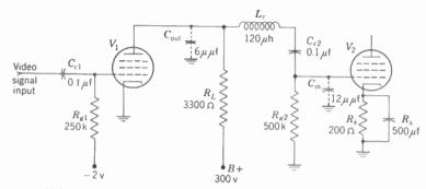
FIG. 11-18. Video amplifier with series peaking. Suppressor and screen-grid connections are omitted.
