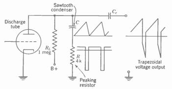
FIG. 17-20. Discharge tube with saw-tooth condenser and peaking resistor to generate trapezoidal voltage wave shape required for saw-tooth current in an RL circuit.
