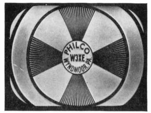
FIG. 4-9. Faulty interlacing. Note how the line divisions in the horizontal wedges appear to be interwoven, in a moire effect. (*Philco Corporation.*)
