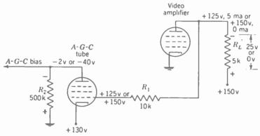
FIG. 15-9. Illustrating how the control-grid voltage of the a-g-c tube depends upon plate current in the video amplifier. Voltages above line are normal; voltages below line are with zero plate current in video amplifier.
