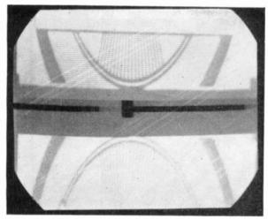
FIG. 16-24. The hammerhead pattern with vertical sync and equalizing pulses on the kinescope screen within the vertical blanking bar. (RCA.)
