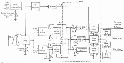
FIG. 24-16. Chrominance circuits for receiver having wide-band color decoder with matrix for I and Q color voltages.
