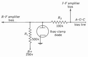
FIG. 15-4. A bias-clamp circuit.
