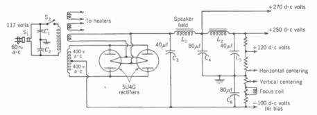
FIG. 10-2. Low-voltage power supply with two full-wave rectifiers in parallel,
