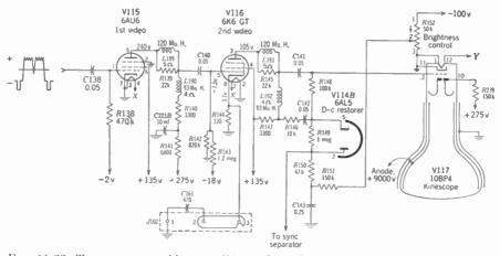
FIG. 11-22. Two-stage a-c video amplifier. Capacitance values in microfarads and resistances in ohms, unless otherwise noted. (*RCA 8TS30 chassis.*)
