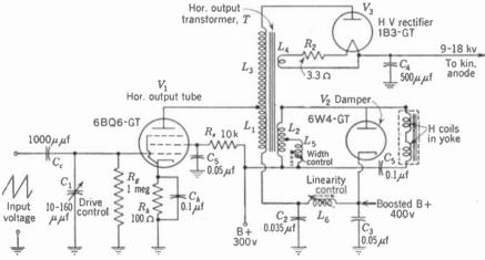
Fig. 18-12. Horizontal deflection amplifier and output circuit.
