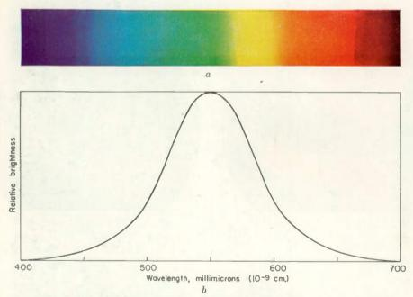
PLATE VI. Relative brightness response of the eye for different hues, with corresponding camera signal voltage. (a) Colors of different wavelengths; (From Weber, White & Manning, ('ollege Physics, McGraw-Hill Book Company, Inc., 1952.) (b) Brightness, or signal voltage response.
