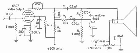
FIG. 13-9. Manual and automatic brightness-control circuit using a positive diode restorer in the kinescope grid circuit. (RCA 630TS and 8TS30 chassis.)
