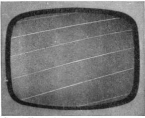
FIG. 4-5. The scanning raster on the kinescope screen.
