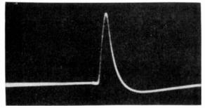
FIG. 16-17. Oscillogram of the integrated vertical synchronizing signal. Vertical deflection oscillator must be disabled to see this pulse without oscillator grid voltage. Oscilloscope internal sweep frequency at 60 cps.  $(RCA_{\cdot})$
