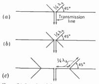
FIG. 21-20. Dual-frequency dipoles.  $\lambda_h$  is high-frequency wavelength. (a) Straight dipole elements added at center for third harmonic. (b) Double-dipole elements added at center for third harmonic. (c) Double-dipole elements added quarter wavelength from center for fourth harmonic.
