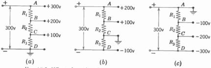
FIG. 10-5. Effect of moving the ground point on a voltage divider.
