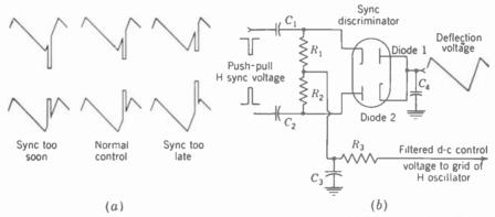
FIG. 17-27. Sync discriminator circuit for automatic control of horizontal oscillator frequency. (a) Wave shapes of the two diode voltages. (b) Circuit arrangement.
