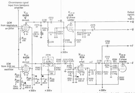
FIG. 24-35. I and Q video signal circuits in receiver illustrated in Fig. 24-33. (RCA.)
