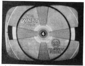
FIG. 23-7. Short, horizontal black streaks caused by auto-ignition interference. (From McGraw-Hill Motion-picture Series, Basic Television.)
