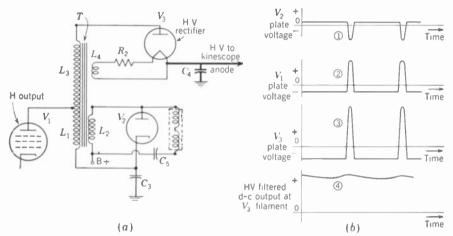
**FIG. 18-20.** Producing the flyback high voltage. (a) Typical circuit. Component part numbers the same as in Fig. 18-12, (b) Voltage wave shapes, with numbers corresponding to the steps described in text.
