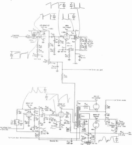
FIG. 18-31. Deflection circuits with autotransformer-coupled vertical output and transformer-coupled horizontal output. Resistance values in ohms, capacitance less than one in  $\mu$ f and more than one in  $\mu\mu f$ . Wave shapes are approximate. (Admiral Series 21 chassis.)
