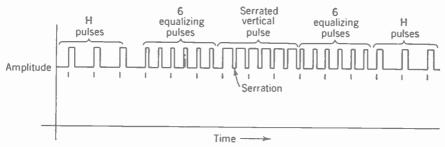
FIG. 4-10. The synchronizing pulses.
