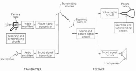
FIG. 1-5. Block diagram of the television system.
