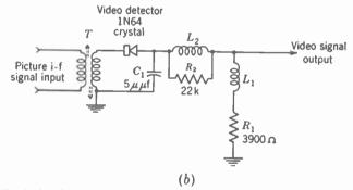
FIG. 14-6. Typical video detectors. (a) Circuit using one diode section of 6AL5 tube. (b) Circuit using crystal diode.
