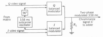
FIG. 24-9. Two-phase modulation of the suppressed color subcarrier by the I and Q video voltages produces the modulated chrominance signal.
