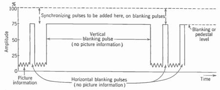
FIG. 5-3. Horizontal blanking pulses and vertical blanking pulse in the video signal. Sync pulses not shown.
