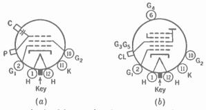
FIG. 9-10. Common duodecal base and socket connections for magnetic-deflection kinescopes, bottom view. (a) 20CP4A, 5-pin. Typical for tubes with magnetic focus or self-focus. (b) 17TP4, 6-pin. Typical for tubes with low-voltage electrostatic focus. The nomenclature is as follows:
