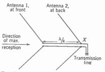
FIG. 21-22. Two vertically stacked antenna bays connected to common transmission line.
