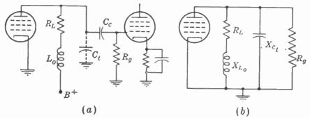
FIG. 12-7. Shunt peaking.  $R_L$  and  $L_a$  can be reversed in the circuit, but the connection shown reduces the stray capacitance. (a) Shunt-peaked stage. (b) Equivalent plate load circuit.
