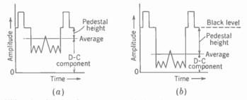
FIG. 5-9. Video signals with the same a-c variations but different average brightness values. (a) Dark scene with average value close to black level; (b) light scene with average value further from black level.
