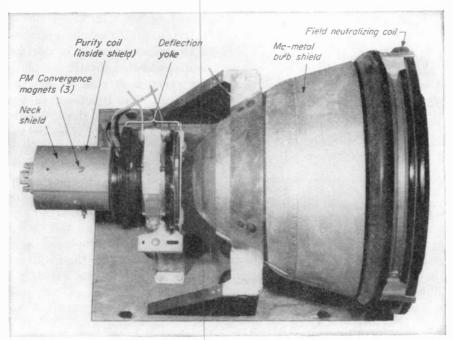
$F_{1G.}$  24-29. Color kinescope mounted with auxiliary operating units. (CBS-Columbia.)
