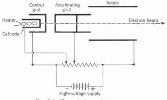
FIG. 3-1. Elements in an electron gun,
