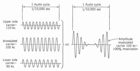
FIG. 6-3 Equivalence of the amplitude-modulated carrier to the modulated carrier plus the two side carriers produced by modulation.
