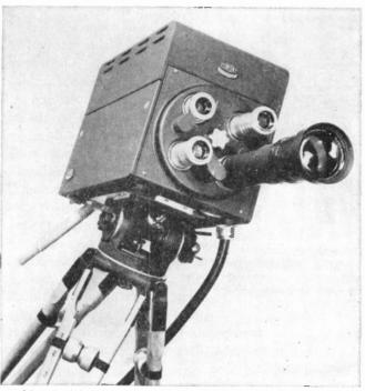
FIG. 2-2. Portable television camera, with four lenses of different focal lengths mounted on a revolving turret. The long barrel has a telephoto lens for close-ups. An image orthicon camera tube is used in this camera head. (Allen B. Du Mont Laboratories, Inc.)
