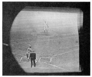
FIG. 16-26. Bend just at the top of the picture, with straight edge on raster. (RCA.)
