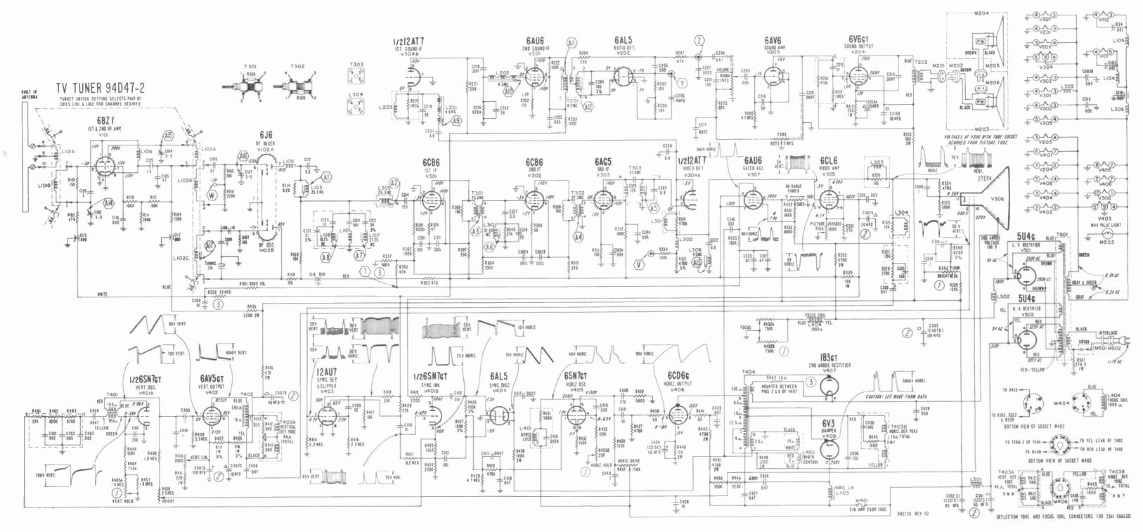
FIG. 23-15. Complete television receiver schematic diagram. Alignment adjustments indicated by letter A. Letters V, W, Y, Z and T indicate alignment connections and test points. Numerical symbols in parts of circuit indicate production changes. Voltages marked with asterisk vary widely with setting of controls. Resistance in ohms, capacitance values less than 1 in  $\mu$ f and more than 1  $\mu\mu$ fd, unless otherwise noted. (Admiral Series 23 chassis.)
