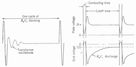
FIG. 17-9. Output of blocking oscillator. Each cycle consists of a high-amplitude pulse at the blocking rate followed by several low-amplitude oscillations.
