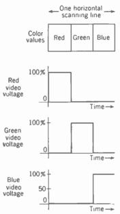
FIG. 24-2. Red, green, and blue color video signal voltages corresponding to color-bar pattern.
