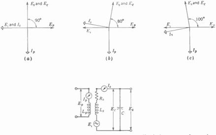
FIG. 22-7. Equivalent circuit and phase relations for the discriminator transformer in a phase-shift discriminator. (a) At center frequency  $I_s$  is in phase with  $E_s$  and  $E_s$  leads  $E_p$  by 90°. (b) Above center frequency  $I_s$  lags  $E_i$  by 10° and  $E_s$  leads  $E_p$  by 80°. (c) Below center frequency  $I_s$  leads  $E_s$  by 10° and  $E_s$  leads  $E_p$  by 10°.
