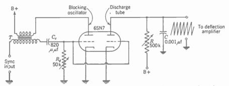
FIG. 17-11. Blocking oscillator and discharge tube circuit. Component values given are for horizontal deflection oscillator, but the same circuit can be used with different components for vertical deflection oscillator.
