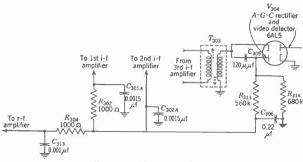
FIG. 15-3. A picture a-g-c circuit.
