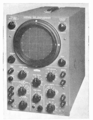
FIG. 23-10. Typical 5-in, oscilloscope. Frequency response of vertical amplifiers is from d-c to 100 kc within 1 db. Internal-sweep frequency range 2 to 30,000 cps. (Allen B. DuMont Laboratories, Inc.)
