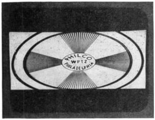
FIG. 17-21. Insufficient height. (Philco Corporation.)
