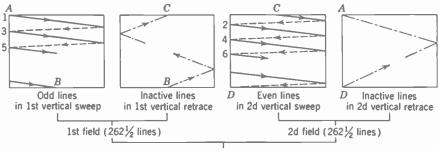
Frame (525 lines) Fig. 4-3. The odd-line interlaced scanning procedure.
