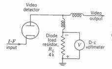
FIG. 14-8. Measuring the rectified output across the detector load resistor with a d-c voltmeter.
