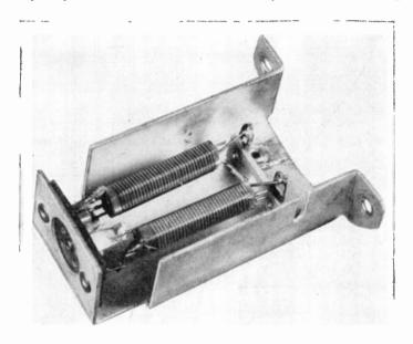
Fig. 21-28. Elevator transformer to match between 72-ohm unbalanced impedance and 300-ohm balanced impedance.  $(RCA_{\cdot})$
