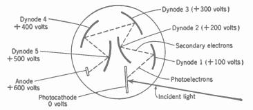
Fig. 2-5. Illustrating an electron-multiplier structure for a phototube.
