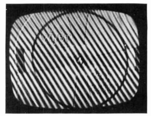
FIG. 20-12. R-F interference pattern produced by local oscillator radiation from a nearby receiver. (From McGraw-Hill motion-picture series, Basic Television.)
