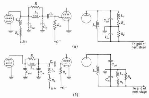
FIG. 12-9. Combination peaking, combining the shunt and series peaking methods. (a) Circuit and equivalent plate load for  $C_{\rm in} = 2C_{\rm out}$ . (b) Circuit and equivalent plate load for  $C_{\rm in} = \frac{1}{2}C_{\rm out}$
