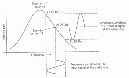
FIG. 22-2. Conversion of frequency variations to amplitude variations by slope detection of an FM signal. Both the input and output are r-f signals, although only the audio variations are illustrated.
