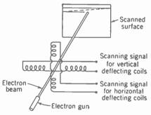
FIG. 3-12. Action of the deflection coils on the electron scanning beam.
