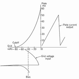
FIG. 18-4. Effect of vertical output tube's grid-plate transfer characteristic on linearity of the saw-tooth output current.
