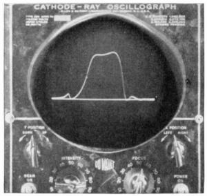
FIG. 19-17. Over-all picture i-f response curve. Marker at picture i-f carrier frequency. (From McGraw-Hill motion-picture series, Basic Television).
