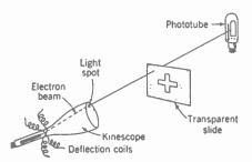
FIG. 2-6. Flying-spot scanning arrangement.
