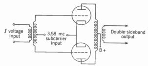
Fig. 24-10. Balanced modulator circuit for suppressed carrier modulation of the 3.58-Mc color subcarrier by the l video signal.
