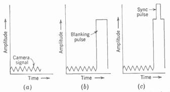
FIG. 5-1. Components of the composite video signal. (a) Camera signal; (b) camera signal plus horizontal blanking pulse; (c) composite video signal with camera signal, blanking pulse, and sync pulse.
