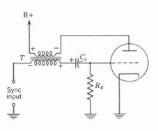
FIG. 17-7. Blocking oscillator circuit diagram.
