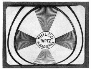
FIG. 18-5. Incorrect adjustment of vertical linearity. (Philco Corporation.)
