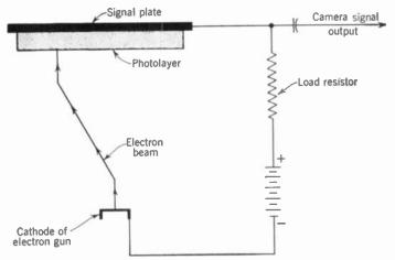
FIG. 2-15. Signal circuit for camera signal output from the vidicon.
