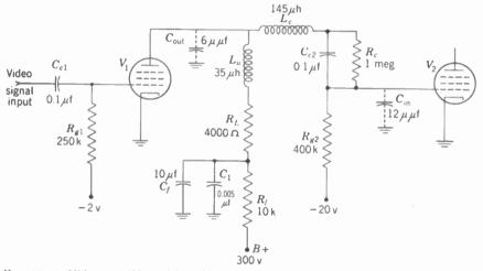
FIG. 11-19. Video amplifier with series-shunt combination peaking for high-frequency compensation, and  $R_f C_f$  and  $C_c R_c$  filters for low-frequency compensation.
