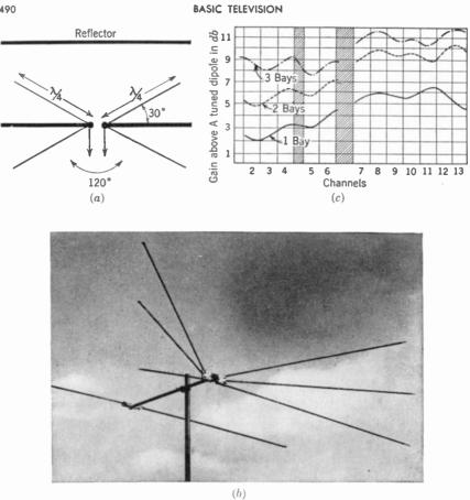
FIG. 21-17. Conical dipole with reflector. (a) Spacing of elements. (b) Typical antenna, single bay. (c) Gain-frequency response curves for channels 2 to 13. (Channel Master ('orporation.)
