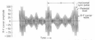
Fig. 6-1. The transmitted picture carrier wave, amplitude-modulated by the composite video signal.
