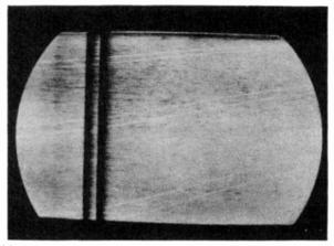
FIG. 18-40. Thin, dark lines at left side caused by Barkhausen oscillations. (RCA.)
