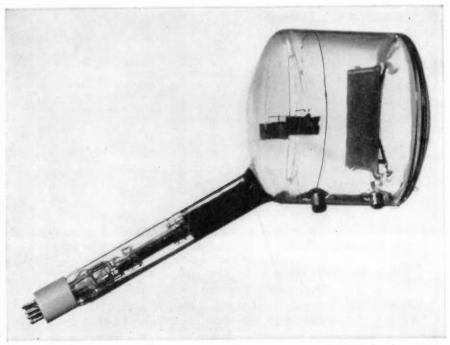
FIG. 1-3. The iconoscope camera tube. The electron-gun structure in the narrow part of the tube produces a beam of electrons aimed at the mosaic image plate. (RCA.)
