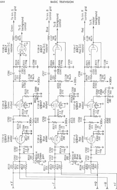
(RCA.)Fig. 24-36. Matrix section in receiver illustrated in Fig. 24-33.
