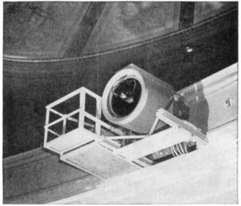
Fig. 8-8. Large-screen television projector mounted on front of balcony in the ater,  $(RCA_{\ast})$
