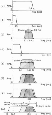
FIG. 24-5. Bandwidth requirements of luminance and chrominance signal frequencies. (a) Y video signal; (b) Q video signal; (c) Q chrominance signal as side bands of 3.58-Mc suppressed subcarrier; (d) I video signal; (e) I chrominance signal; (f) total chrominance signal—crosshatch indicates where I and Q frequencies overlap; (g) colorplexed video signal S with Y, I, and Q; (h) side-band frequencies of colorplexed signal transmitted as amplitude modulation of channel 4 picture carrier.
