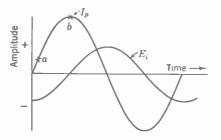
FIG. 22-6. The induced voltage  $E_{e}$  varies in magnitude with the change in primary current and therefore is 90° out of phase with  $I_{p}$ .
