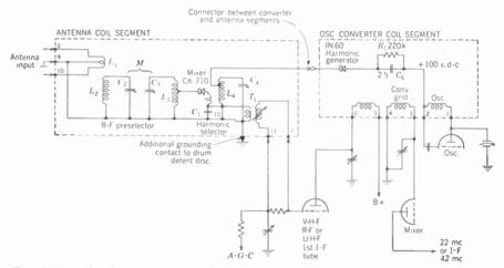
FIG. 20-20. Circuit arrangement of u-h-f conversion strips for v-h-f turret tuner in Fig. 20-18. (Standard Coil Products, Inc.)
