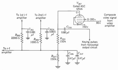
FIG. 15-6. Keyed a-g-c circuit. Voltages indicated are positive d-c volts. A-g-c voltage at plate is zero with no signal input. (Admiral Series 23 chassis.)
