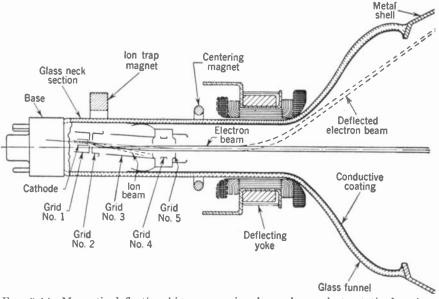
FIG. 9-14. Magnetic-deflection kinescope using low-voltage electrostatic focusing. Note the internal connection of grids 3 and 5 to the anode, and the position of the centering magnet. (RCA.)
