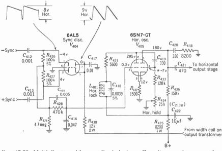
FIG. 17-30. Multivibrator with sync discriminator. Capacitance values more than one in  $\mu\mu$  and less than one in  $\mu$ ; resistance values in ohms unless otherwise noted. Voltage at pin 4 of 6SN7-GT varies widely with setting of hold control. (Admiral Series 21 chassis.)
