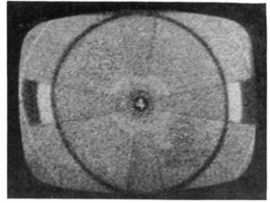
FIG. 20-5. White speckled background of snow, produced by receiver noise voltages. with weak r-f signal. (From McGraw-Hill motion-picture series Basic Television.)
