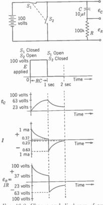
FIG. 16-8. Charge and discharge of an RC circuit in RC time.
