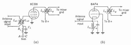
FIG. 20-7. Signal input and output for two basic types of r-f amplifiers. (a) Conventional pentode grounded cathode amplifier. (b) Triode grounded grid amplifier.
