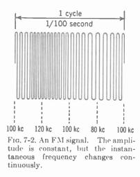
taken as  $\frac{1}{100}$  sec, the r-f output of the oscillator will appear as in Fig. 7-2. The amplitude remains the same at all times but the frequency is changing continuously, with the instantaneous frequency being *wobbled* around the center carrier frequency. Starting from rest position when the trimmer condenser is half in mesh, the output frequency is at its
