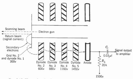
FIG. 2-12. Illustrating the electron-multiplier section of the image orthicon.
