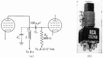
FIG. 19-9. (a) Single-tuned i-f amplifier stage with RC grid coupling circuit. (b) Single-tuned 22-Mc i-f coil with wave trap. Inductance 3.1 to 5.2 microhenrys.
