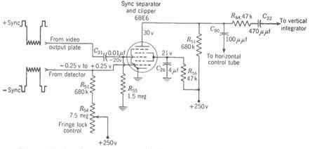
FIG. 16-23. Gated sync separator and clipper stage. (Zenith chassis 22L20.)
