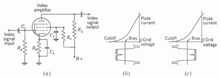
FIG. 11-6. Video amplifier circuit and its operating characteristics. (a) Basic RCcoupled amplifier. (b) Video signal voltage of negative picture phase on control grid. (c) Video signal voltage of positive picture on control grid.
