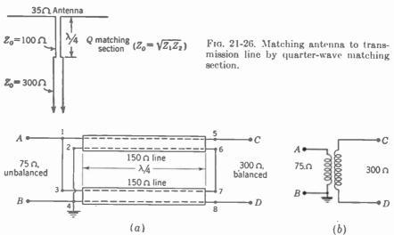
FIG. 21-27. Balancing unit to match between 75-ohm unbalanced impedance and 300-ohm balanced impedance. (a) With two 150-ohm line sections. (b) Equivalent circuit.
