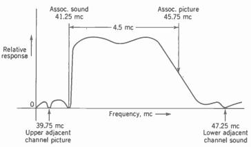
FIG. 19-12. Location of carrier frequencies for the associated sound and picture, lower adjacent channel sound, and upper adjacent channel picture, in the picture i-f response.
