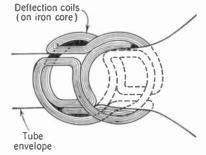
FIG. 3-13. Construction of a deflection yoke.
