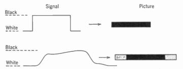
FIG. 11-27. How excessive low-frequency response with phase distortion causes severe smear.
