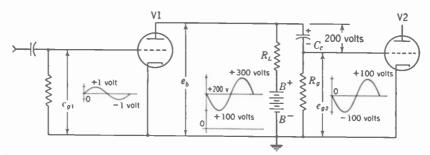
FIG. 13-4. Capacitive coupling. For simplicity, a sine-wave signal is illustrated instead of the video signal. Grid bias is omitted.
