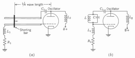
FIG. 20-13. Ultraudion oscillator circuit using a quarter-wave line as the tuned circuit.(a) Schematic diagram. (b) Equivalent tuned circuit.
