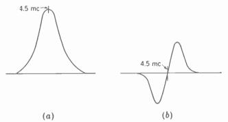
FIG. 22-15. Response curves for sound i-f section with center frequency of 4.5 Me. (a) Single-peaked response of sound i-f stages. (b) S curve of discriminator or ratio detector.
