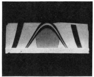
FIG. 18-38. Fold-over at bottom edge of raster and picture caused by leaky coupling condenser in grid of vertical output tube. (RCA.)
