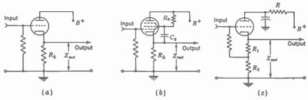
FIG. 12-18. The eathode-coupled stage. The load is in the cathode instead of the plate circuit. (a) Triode cathode follower. (b) Pentode cathode follower. (c) Triode cathode follower, with plate-dropping resistor R and grid returned to tap on cathode resistance.
