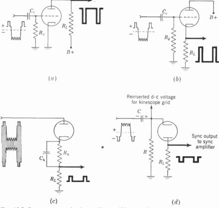
FIG. 16-5. Sync separator circuits. All use self-bias to allow plate-current flow only for the synchronizing pulses. Pentodes can be used in place of the triodes. (a) Grid-leak bias separator with negative sync output across plate load resistor. (b) Grid-leak bias separator with positive sync output across eathode load resistor. (c) Diode separator with modulated i-f signal input. (d) Inverted diode operating as combined d-c restorer and sync separator.
