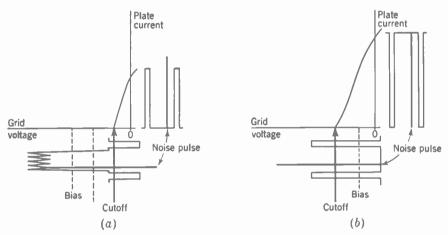
FIG. 16-18. Noise pulse and signal in sync stages. (a) Composite video with positive sync and noise pulse at grid of sync separator. (b) Separated sync of negative polarity with noise pulse at grid of succeeding sync clipper.
