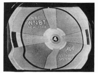
Fig. 16-28, 60-cycle hum bend in the picture, but not in the raster, without hum bars. See text for explanation of these symptoms that indicate heater-to-cathode leakage in a horizontal sync tube.  $(RCA_{\cdot})$
