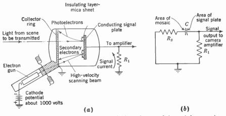
FIG. 2-8. The iconoscope camera tube.  $R_s$  is the resistance of the path for secondary electrons from the mosaic to the collector anode, which is about 5 megohms. A typical value of the load resistor  $R_1$  is 10,000 ohms. The capacitance of C is about 100  $\mu\mu$ f per sq cm. (a) Tube construction; (b) signal circuit.
