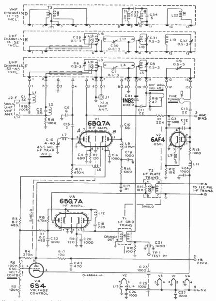
FIG. 20-21. Schematic diagram of r-f tuner for u-h-f and v-h-f channels. (RCA KRK-12 r-f unit.)
