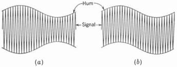
FIG. 10-19. Waveforms of hum combining with higher frequency signal. (a) Modulation hum. (b) Additive hum.
