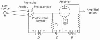
FIG. 2-4. Phototube amplifier circuit. The A battery supplies filament power, the B supply provides plate voltage and the C battery furnishes grid bias for the amplifier. The D supply makes the phototube anode positive with respect to its cathode.
