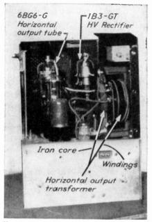
FIG. 18-13. Components of horizontal output circuit in high-voltage compartment on receiver chassis. (*RCA Institutes, Inc.*)
