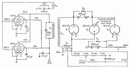
FIG. 10-15. Schematic diagram of 30 ky r-f power supply. (Essex Electronics.)
