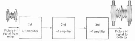
Fig. 19-1. The picture i-f stages amplify the picture signal from the mixer to supply enough signal to the video detector,
