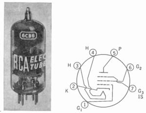
FIG. 8-10. Miniature glass tube with 7-pin base.  $(RCA_{\cdot})$
