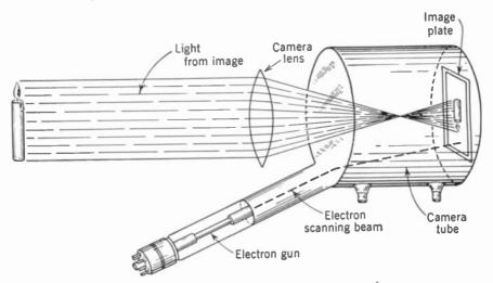
FIG. 2-1. Televising an image with a camera tube.
