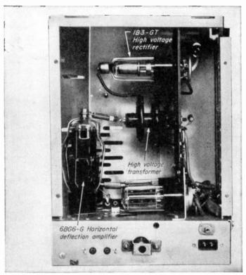
FIG. 10-17. Flyback power supply in high-voltage cage on receiver chassis. (RCA.)
