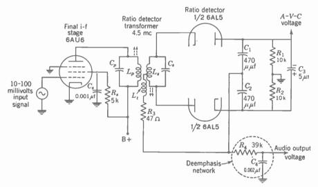
FIG. 22-10. Schematic diagram of ratio detector for i-f center frequency of 4.5 Me, with balanced output circuit.
