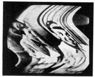
FIG. 17-35. Horizontal pulling in picture caused by heater-cathode leakage in horizontal control tube. (RCA.)
