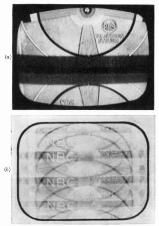
FIG. 16-1. Vertical scanning not synchronized, resulting in no vertical hold. (a) Picture slowly slips frames vertically. (b) Picture rolts fast vertically.
