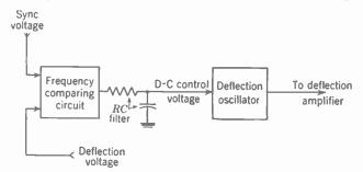
FIG. 17-24. Block diagram of a-f-e circuit for horizontal deflection oscillator.
