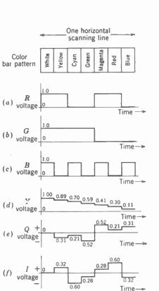
FIG. 24-4. Video voltage waveforms of Y, Q, and I signals formed from primary color video voltages, corresponding to color-bar pattern. (a) Red video signal; (b) green video signal; (c) blue video signal; (d) luminance signal Y; (e) Q color video signal; (f) I color video signal.
