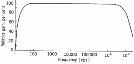
FIG. 11-9. Desired video amplifier response curve.
