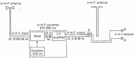
FIG. 20-19. Operation of u-h-f converter, illustrated for u-h-f channel 19 converted to v-h-f channel 6 frequencies.
