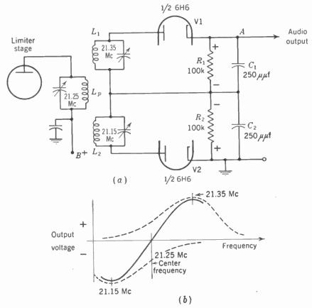
FIG. 22-3. Triple-tuned discriminator for an i-f center frequency of 21.25 Mc. (a) Circuit. (b) Response curve.
