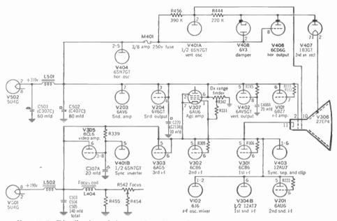
FIG. 10-3. Distribution of d-c supply voltages from two separate low-voltage power supplies. (Admiral Series 23 chassis.)
