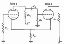
FIG. 17-16. Cathode-coupled multivibrator, using direct coupling between the cathodes. The circuit can also be arranged with separate cathode resistors and capacitive coupling between the two cathodes.
