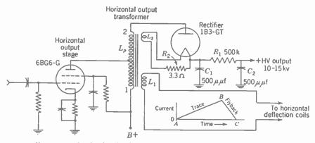
FIG. 10-16. Basic circuit of the flyback type of high-voltage supply.
