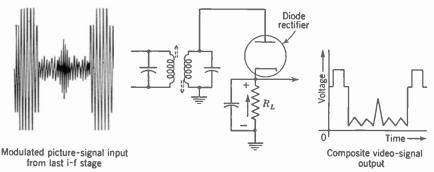
FIG. 14-1. Function of the video detector. The modulated picture signal is rectified and filtered to provide the composite video signal in the output.
