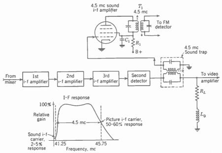
FIG. 22-14. The intercarrier-sound system, showing the common picture and sound i-f amplifier with its response curve, 4.5-Me sound take-off circuit in output of second detector, and 4.5-Me sound i-f amplifier driving the FM detector.
