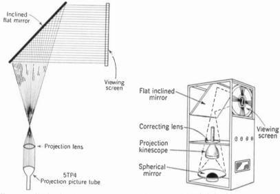
FIG. 8-6. Projection-lens system for television receivers.
