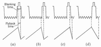
FIG. 17-34. Phasing of flyback and blanking time for horizontal scanning. (a) Flyback within blanking time. (b) Flyback starts too soon. (c) Flyback starts too late. (d) Flyback time too long.
