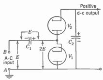
FIG. 10-10, <sup>7</sup> Full-wave voltage doubler circuit.
