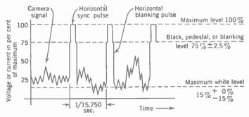
Fig. 5-2. Composite video signal for three consecutive horizontal lines.
