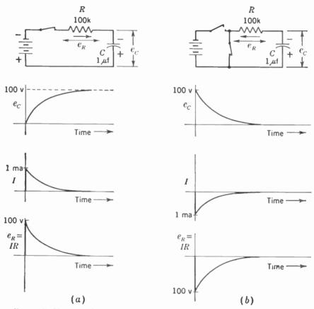
FIG. 16-7. Charge and discharge of an RC circuit. (a) Charge. (b) Discharge.
