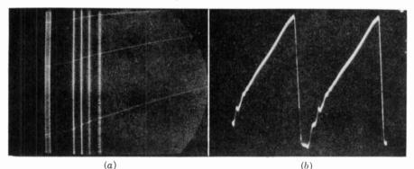
FIG. 18-36. Excess ve horizontal drive. (a) Thin, bright bars at left side of raster caused by ripples in horizontal scanning current in (b). (*RCA Institutes, Inc.*)
