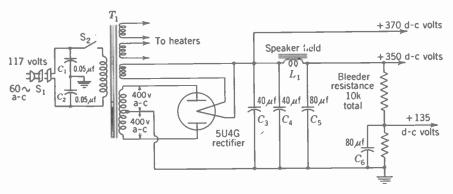
Fig. 10-1, Low-voltage power supply for a television receiver,
