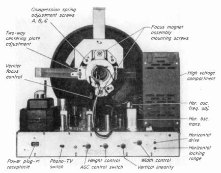
Fig. 23-1, Set-up adjustments at back of receiver chassis. (RCA KCS 47 chassis.)
