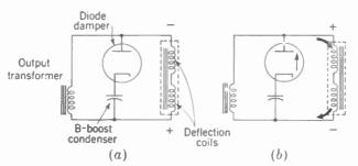
Fig. 18-15. A-c equivalent circuit of the damper tube in the horizontal output circuit. (a) Damper plate negative and nonconducting for the retrace. (b) Damper plate positive and conducting for the trace.
