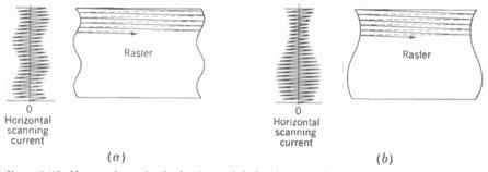
FIG. 18-35. Hum voltage in the horizontal deflection circuits. (a) Addition of 120 cps hum and horizontal scanning signal. (b) Modulation of horizontal scanning signal by 60 cps hum.
