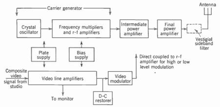
FIG. 6-11. Block diagram of television transmitter for picture signal.
