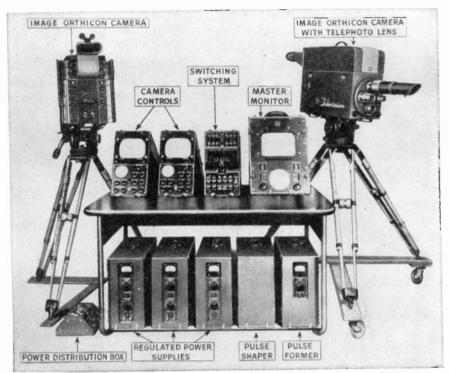
Fig. 6-9. Portable field equipment for two camera chains. (RCA.)
