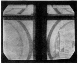
FIG. 16-25. Horizontal sync and blanking bars on the kinescope screen. (RCA.)
