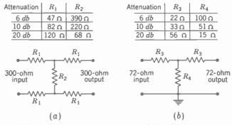
FIG. 21-29. Resistance pads with values for 6 db, 10 db, or 20 db attenuation. (a) Balanced II pad. (b) Unbalanced T pad.
