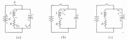
FIG. 18-10. Shock-exciting a tuned circuit into oscillation. (a) Switch is closed, and the battery supplies current and voltage for the LC circuit. (b) Switch is opened, and the self-induced voltage across L acts as the generator. (c) Reversed polarities one-half cycle later, with the voltage across C as the generator.
