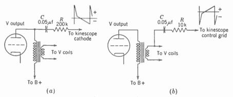
FIG. 18-32. Circuit arrangements for using vertical flyback pulses to provide internal vertical blanking. (a) From plate of vertical output tube. (b) From secondary of vertical output transformer.
