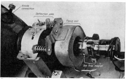
FIG. 9-2. Control units mounted on neck of picture tube using magnetic deflection and magnetic focus. (RCA.)
