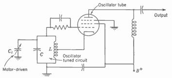
FIG. 7-1. The wobbulated oscillator. The shaft of the variable air condenser  $C_t$  is mechanically coupled to a motor to make the condenser rotate in and out of mesh to change the frequency of the oscillator.
