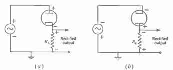
FIG. 14-2. Rectifier polarity. (a) The diode load resistance in the cathode circuit provides output voltage of positive polarity. (b) The diode load resistance in the plate circuit provides negative output voltage.
