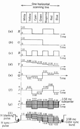
FIG. 24-14*a*-*h*. Construction of colorplexed composite video signal from Y, I, and Q voltages. (a) Red video; (b) green video; (c) blue video; (d) luminance video; (e) Q video; (f) I video; (g) 3.58-Me subcarrier chrominance signal C modulated by I and Q in quadrature; (h) colorplexed total video signal S, including Y, I, and Q with standard blanking, deflection sync, and color sync burst.
