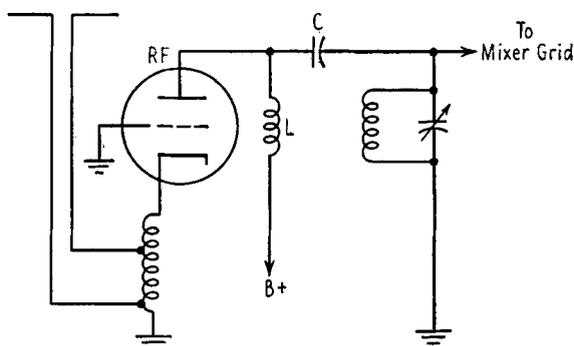
FIG. 24-7. RF stage in an F-M receiver, using a grounded-grid triode.
