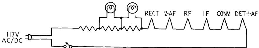
With minor modifications, the typical circuit of Fig. 18-1 is capable of a large number of possible combinations. Figure 18-3 shows a variation of the same circuit to supply an RF tube and an extra pilot light.
