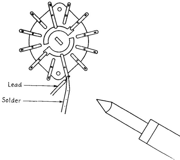
FIG. 12-22. Method of supplying solder when speed-soldering wafer-type switch connections.
