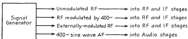
FIG. 5-9. Output voltages and currents from a signal generator.
