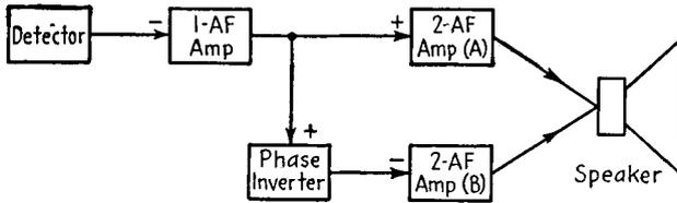
FIG. 22-9. Block diagram of a phase-inverter type of push-pull amplifier.
