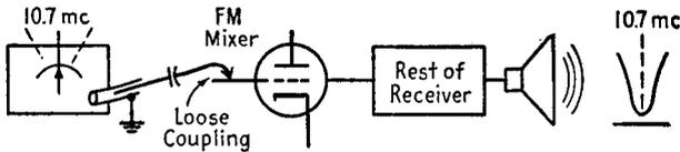
Couple signal generator output loosely to F-M mixer grid.
