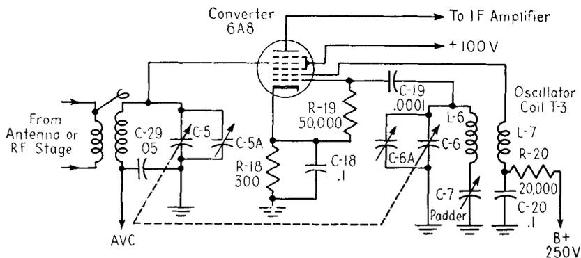
FIG. 14-28. The oscillator circuit in a 6A8 pentagrid converter.
