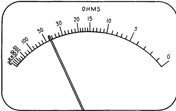
FIG. 4-14. Typical ohmmeter scale.
