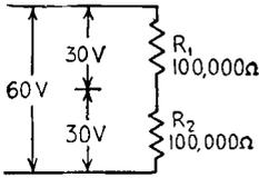
FIG. 4-6. Voltage distribution across two equal resistors.
