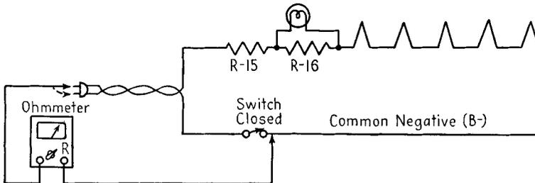
FIG. 18-12. Checking the line cord and switch in an AC/DC heater circuit.
