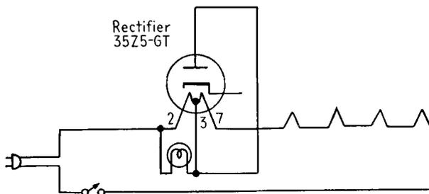
FIG. 18-21. Pilot-lamp circuit for a 0.15-amp heater line.
