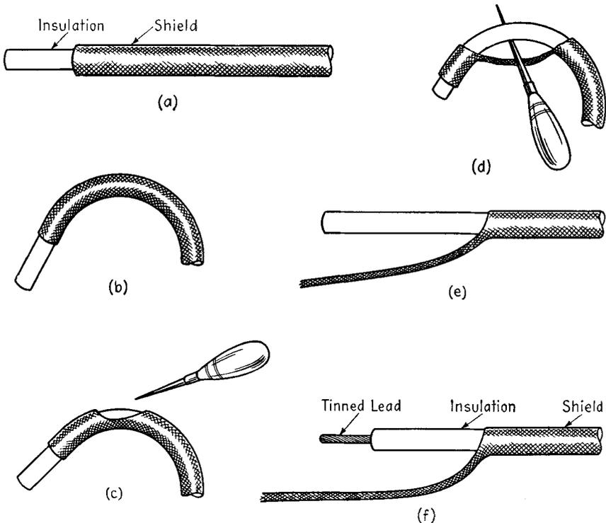
FIG. 11-18. How to prepare shielded wire for use: (a) push back the shielding to loosen the weave; (b) bend a loop in the lead; (c) work the weave back and forth with a pointed instrument until the hole is large enough to pull the wire through; (d) pull the end of the wire through the hole; (e) pull out the empty piece of sleeving; (f) strip and tin the ends of the lead.
