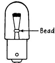
FIG. 18-16. A pilot lamp showing position of bead.
