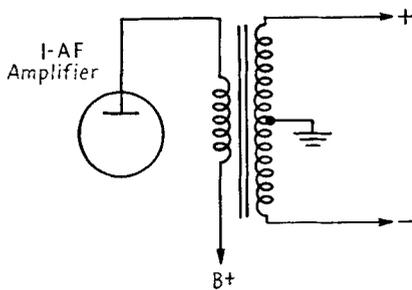
FIG. 22-2. The center-tapped transformer for obtaining input voltages for a push-pull stage.
