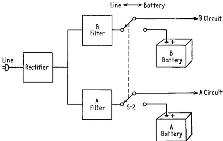
FIG. 19-8. Block diagram of the power supply in a three-way portable receiver.
