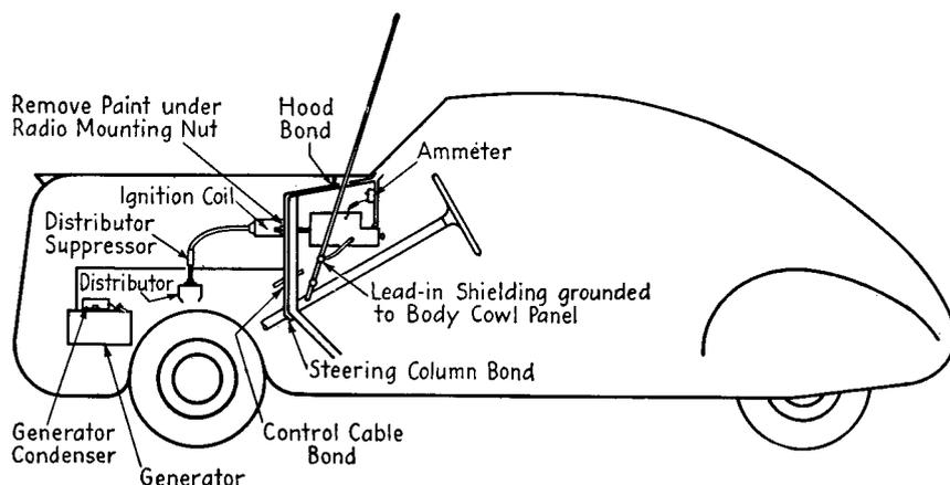
FIG. 20-11. Standard automobile radio installation for side-cowl antennas.
