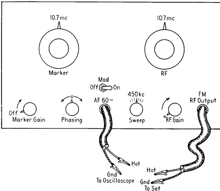
FIG. 26-15. Controls of a basic sweep-frequency signal generator.
