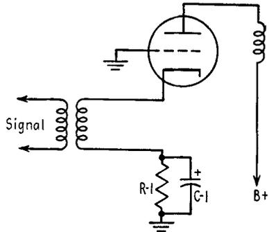
FIG. 25-17. Simplified grounded-grid triode amplifier.
