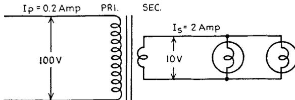
FIG. 10-8. Transformer lighting two lamps.
