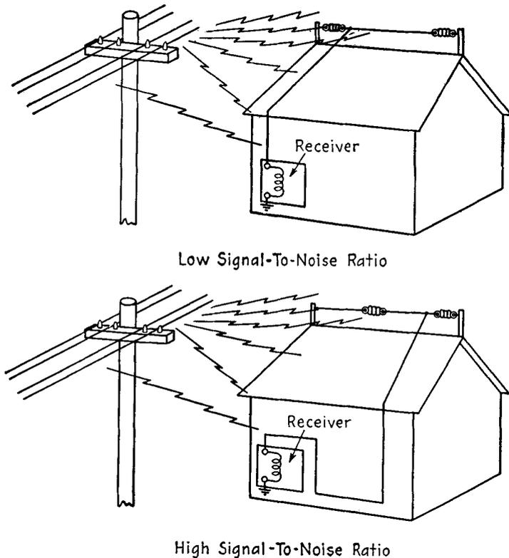
FIG. 17-3. Low and high signal-to-noise ratios.
