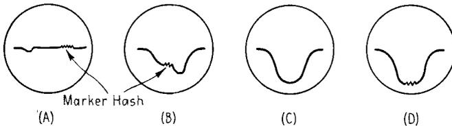
FIG. 26-20. Oscilloscope traces in alignment of the third IF transformer.
