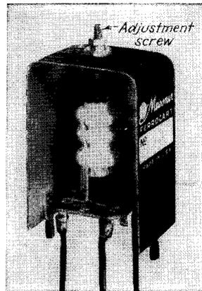
properly in the circuit in which it is being placed. The adjustable feature of these coils is permeability tuning with a screw adjustment similar to that used in IF transformers, so that the inductance of the coil may be varied to suit the receiver. An adjustable replacement coil of this type is shown in Fig. 14-13.
