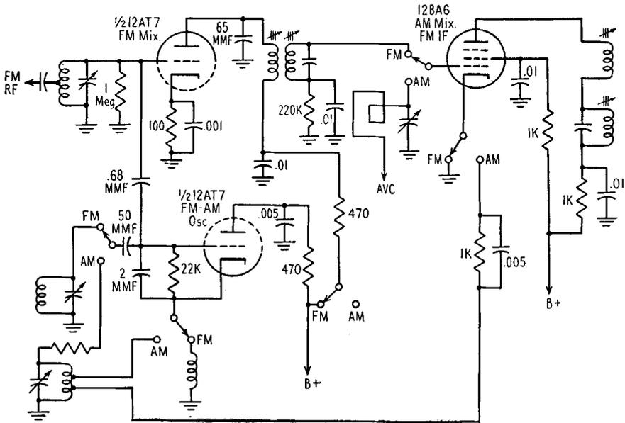
FIG. 25-14. A-M/F-M converter with a combination A-M mixer and F-M IF amplifier tube.
