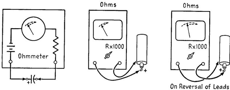
FIG. 8-11. Checking an electrolytic condenser with an ohmmeter.
