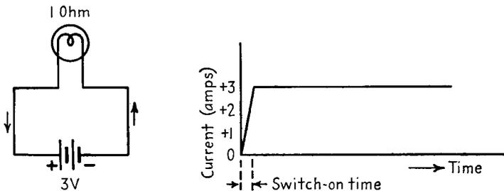
FIG. 5-1. Circuit and wave form for a pure direct current (DC).
