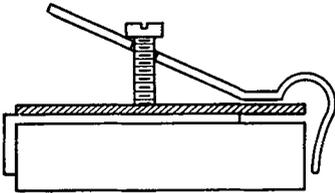
FIG. 23-9. A trimmer condenser at its low-capacity setting.
