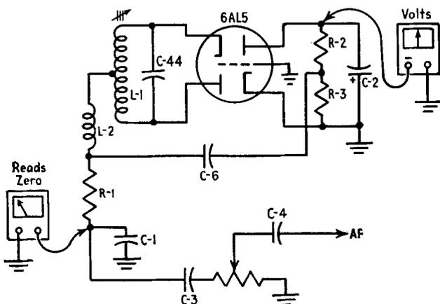
FIG. 25-8. Checking operation of the ratio detector.
