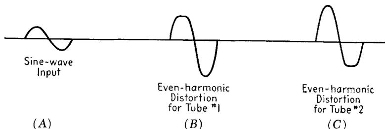
FIG. 22-6. The wave form of even-harmonic distortion developed in single-tube amplifiers.
