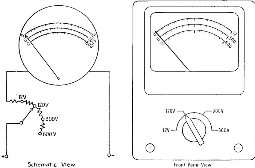
FIG. 4-5. Multirange voltmeter showing range switch.
