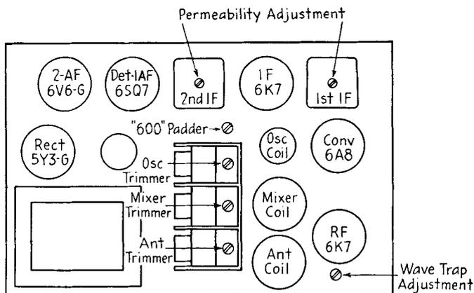
FIG. 23-6. Layout diagram of a six-tube superheterodyne receiver.
