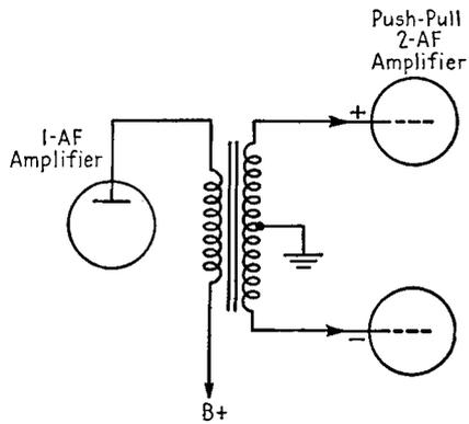
FIG. 22-3. Applying the signal-input voltages to the push-pull grids.
