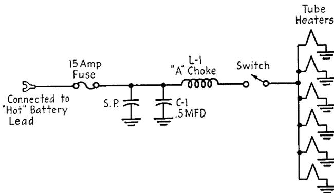
FIG. 21-1. Typical automobile radio heater circuit.
