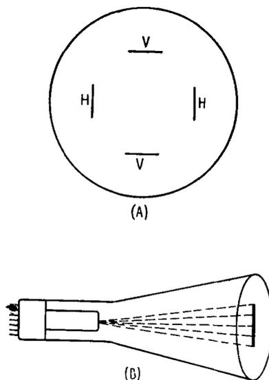
FIG. 26-17. Deflecting plates and their action in a cathode-ray tube.
