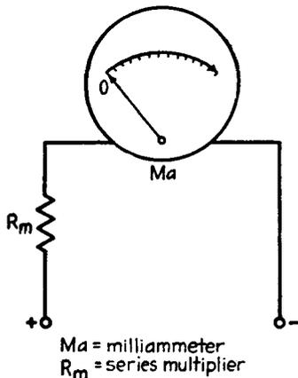
FIG. 4-2. A basic voltmeter.
