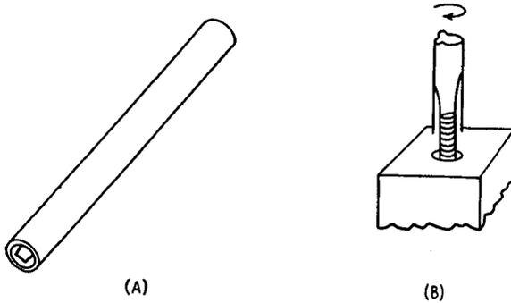
FIG. 26-3. Recessed nib alignment tool.
