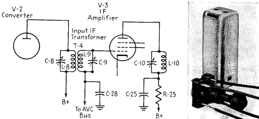
FIG. 13-12. The input IF transformer and its position in the circuit.
