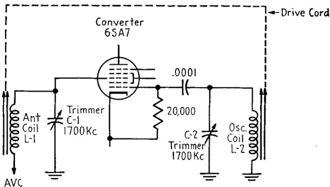
FIG. 15-7. Skeleton diagram of drive-cord type of permeability tuner.
