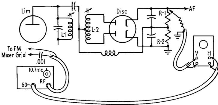
FIG. 26-24. Aligning the Foster-Seeley discriminator.
