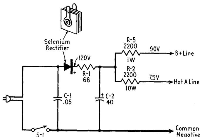
FIG. 19-17. The selenium rectifier and normal voltage measurements at test points in the power supply of three-way portable receivers.
