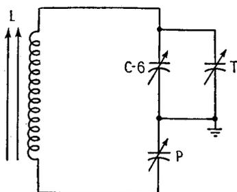
FIG. 14-23. Oscillator tuning-circuit adjustments.
