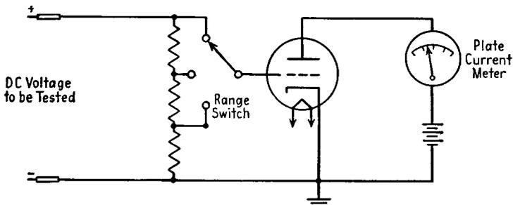
FIG. 4-17. Basic DC electronic voltmeter.
