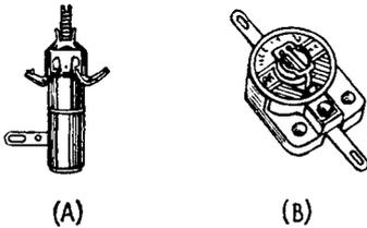
FIG. 26-1. High-frequency trimmers used in A-M/F-M receivers.
