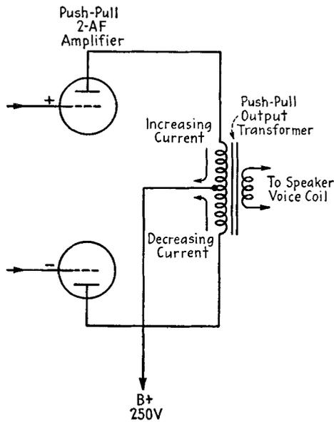
FIG. 22-5. The output circuit of a push-pull amplifier.
