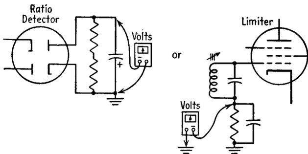
FIG. 25-21. Meter connections for checking oscillation.
