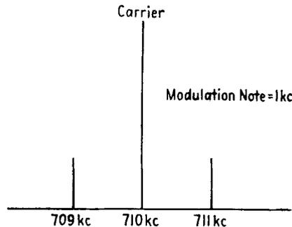
FIG. 24-3. Sidebands in an A-M signal.
