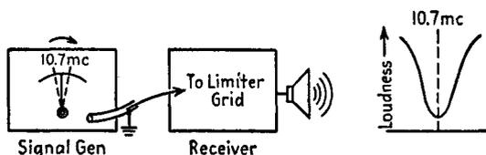
FIG. 25-4. Characteristic dip in volume on signal check in F-M receivers.
