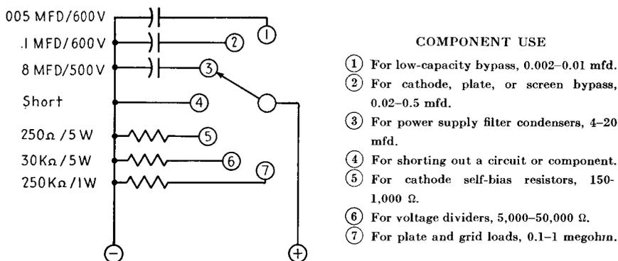
FIG. 28-11. Schematic diagram of resistor and condenser substitution box.
