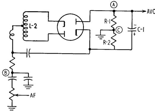
FIG. 26-12. Alignment test points for a ratio-detector variation.
