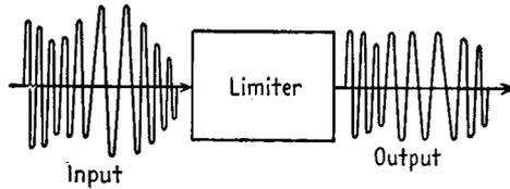
FIG. 24-11. Limiter action when the input signal is too low.
