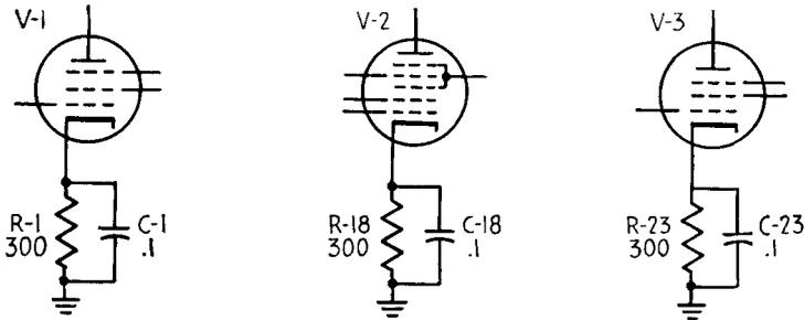
FIG. 13-7. Cathode circuits with individual self-bias resistors to avoid inter-stage coupling.
