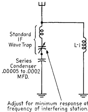
FIG. 16-8. Using a standard IF wave trap to reduce image-frequency interference.
