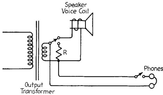
FIG. 9-17. Circuit for connecting headphones to a receiver.
