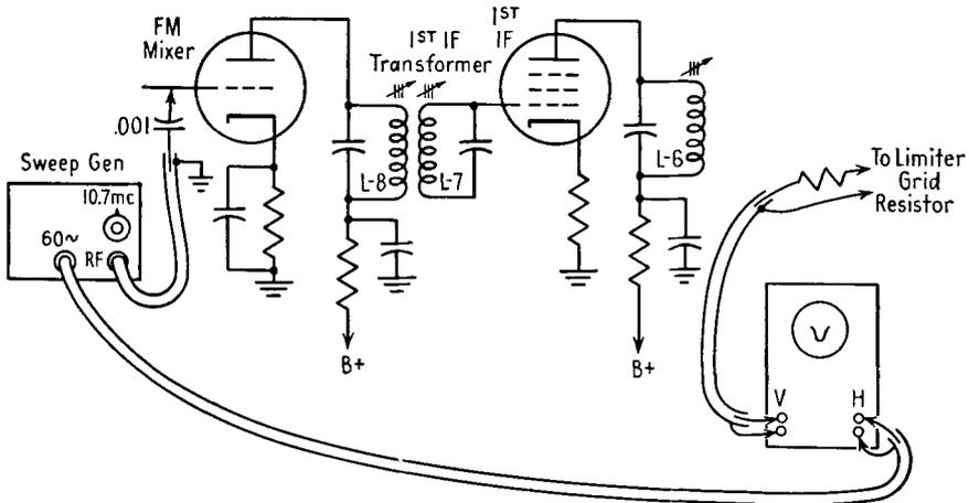
FIG. 26-23. Aligning the first IF transformer.
