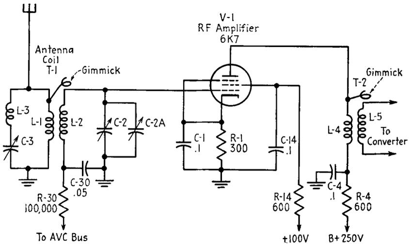
**Normal voltage data for the RF stage**
