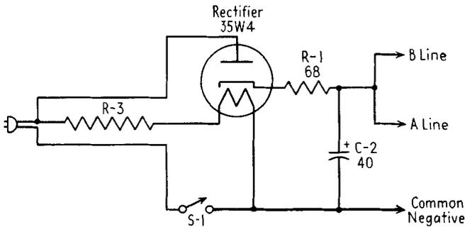
FIG. 19-14. The 35W4 tube used as the rectifier in a three-way portable receiver.
