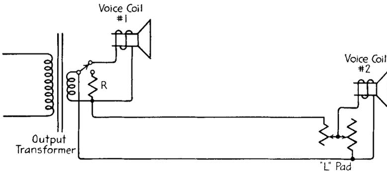
FIG. 9-16. Volume control for an auxiliary speaker.
