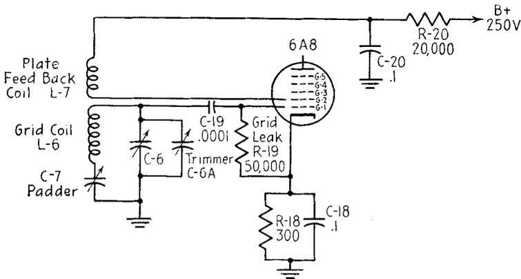
FIG. 14-2. Oscillator circuit in the 6A8 pentagrid converter.
