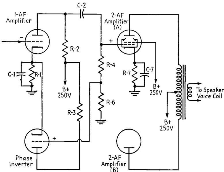
FIG. 22-11. Applying a portion of the positive output signal of the first AF amplifier to the phase-inverter grid.
