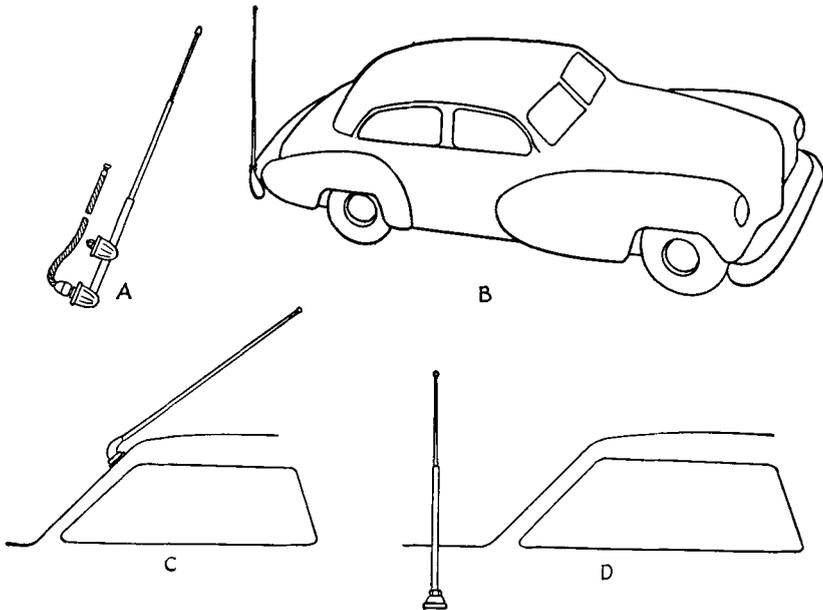
FIG. 20-2. Common automobile radio antennas. (A) Side cowl; (B) rear-bumper mount; (C) topper; (D) disappearing cowl.
