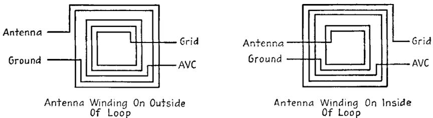
FIG. 14-15. Identifying loop antenna leads.
