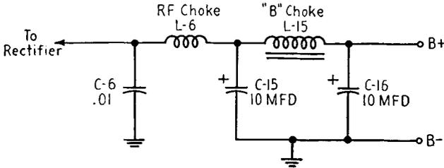
FIG. 21-17. The automobile radio *B* filter circuit.
