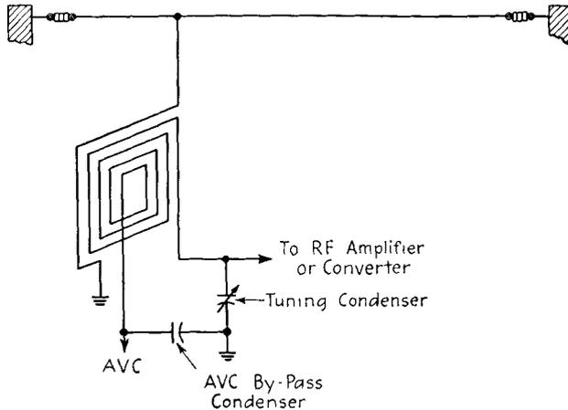
FIG. 17-20. A loop with an antenna winding.
