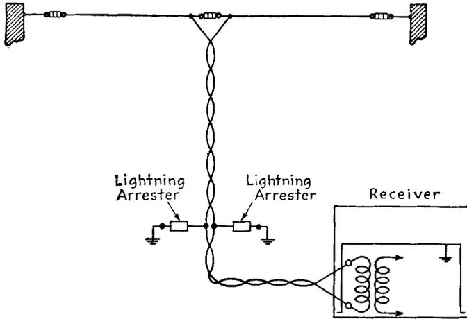
FIG. 17-24. Connected lightning arresters to a twisted-pair leadin.
