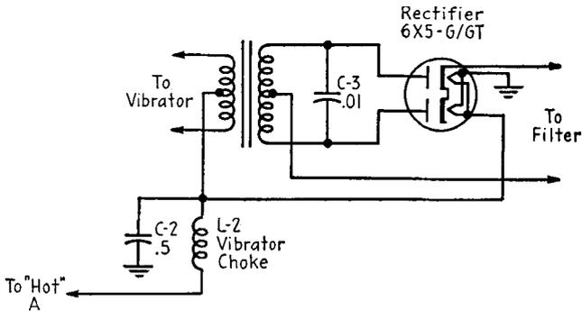
FIG. 21-9. Full-wave rectifier in the vibrator-type power supply.
