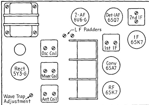
FIG. 23-7. Layout diagram of a six-tube, two-band receiver.
