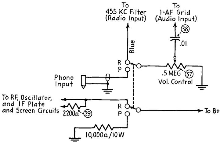
FIG. 12-26. Adding a radio-phonograph switching circuit to the receiver shown in Fig. 12-14.
