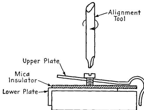
FIG. 23-8. Adjusting a trimmer condenser.
