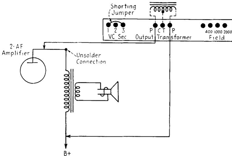
FIG. 28-6. Checking a receiver output transformer by substituting the bench test speaker.
