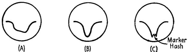
FIG. 26-22. Traces in the alignment of the second IF transformer.
