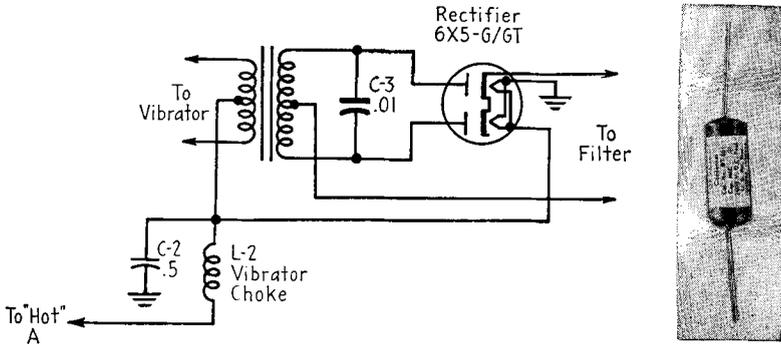
FIG. 21-15. A typical buffer condenser and its position in the circuit.
