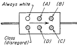
First dot is always white. This indicates a molded mica condenser. Direction for reading indicated by arrow or equivalent marking.
