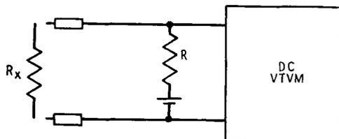
FIG. 4-20. Basic electronic ohmmeter.
