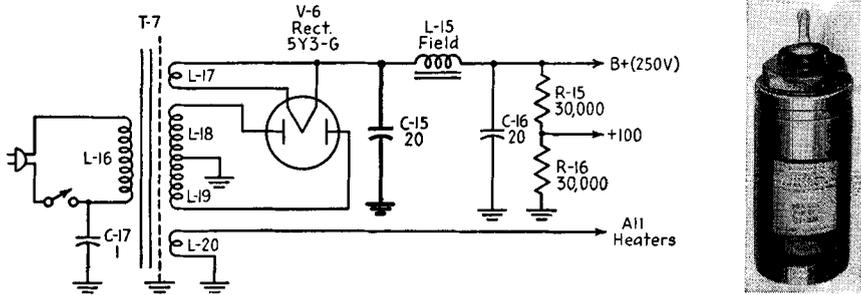
FIG. 8-10. A typical input filter condenser and its position in the power-supply circuit.
