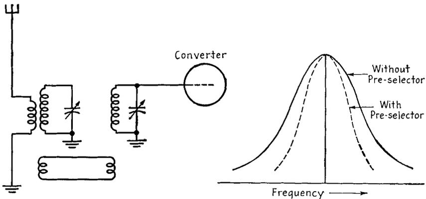
FIG. 16-1. A preselector circuit and its effect on selectivity before the converter signal grid.
