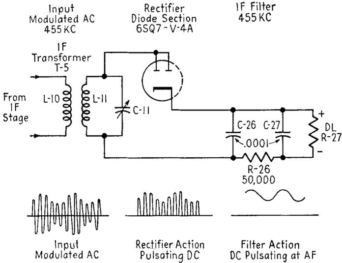
FIG. 12-3. Diode detector operation—developing the audio output signal from the modulated IF input signal.
