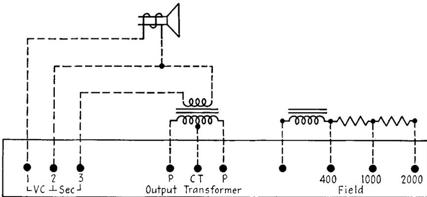
Note: When using Test Speaker Output Transformer, place a Shorting Jumper from 1 to 3. When using Receiver Output Transformer, use Terminals 1 and 2
