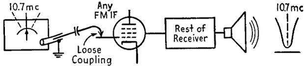
Couple signal generator output loosely to any IF grid to be checked.
