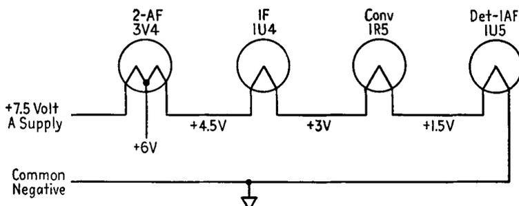
FIG. 19-9. Series arrangement of tube filaments in three-way portable receivers.
