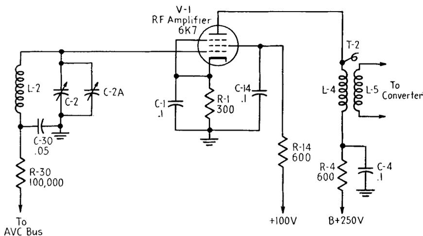
FIG. 16-6. Decoupling filters in the RF stage.
