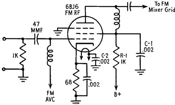
FIG. 25-18. RF amplifier using a pentode tube.
