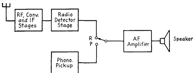
FIG. 12-15. Block diagram of radio-phonograph operation.
