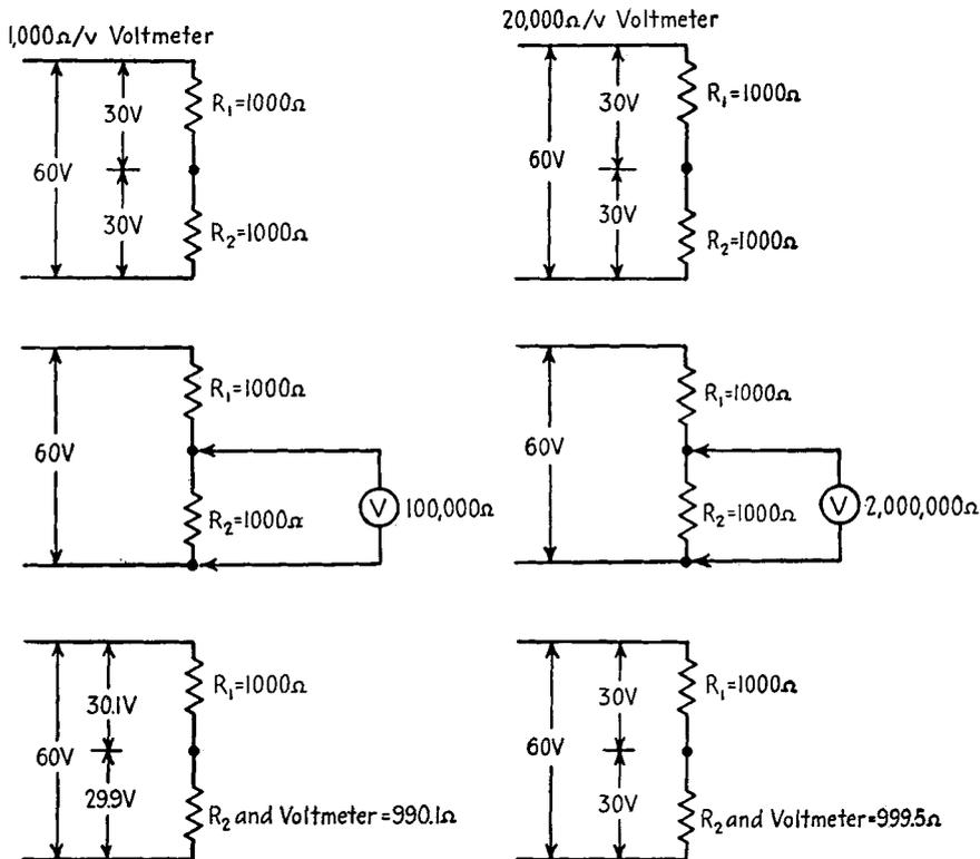
FIG. 4-11. Comparison between a 1,000-ohms-per-volt meter and a 20,000-ohms-per-volt meter in a low-resistance circuit.
