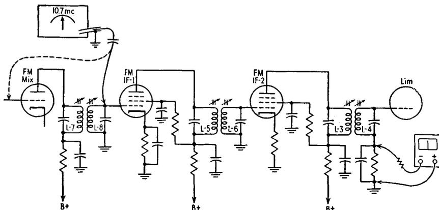
FIG. 26-9. Aligning the second and first IF transformers.
