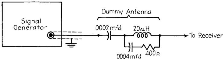
FIG. 7-1. The I.R.E. standard dummy antenna, connected to signal generator and receiver.
