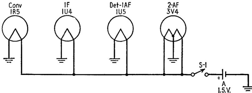
FIG. 19-2. Filament circuit commonly used in battery portables.
