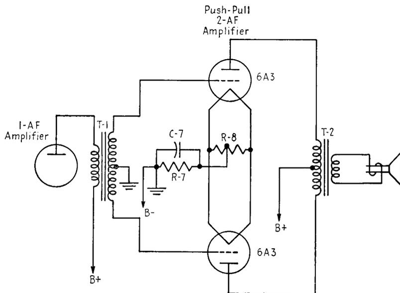
FIG. 22-8. Schematic diagram of a transformer-coupled push-pull stage.
