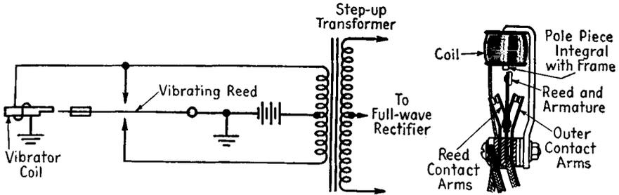
FIG. 21-6. A typical vibrator used in automobile radio power supplies and a basic vibrator circuit.
