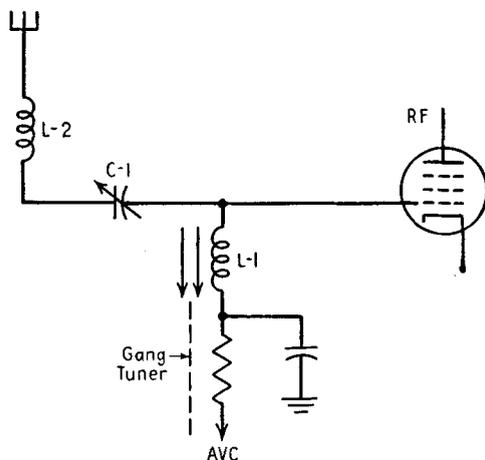
FIG. 20-3. Typical automobile radio antenna coupling circuit.
