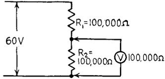
FIG. 4-7. Measuring voltage with a 1,000-ohms-per-volt meter.
