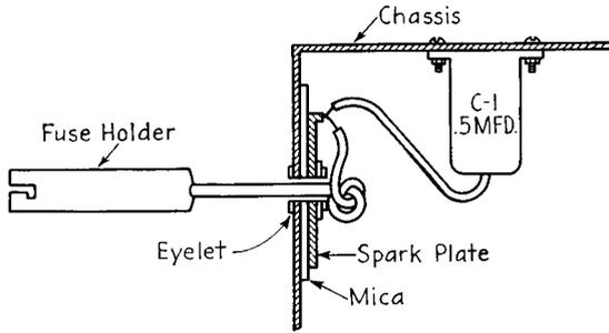
FIG. 21-2. Spark-plate filter connected to the "hot" battery lead at the point of entry to the receiver.
