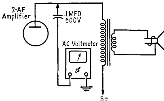
FIG. 23-4. Connecting an output indicator for alignment.
