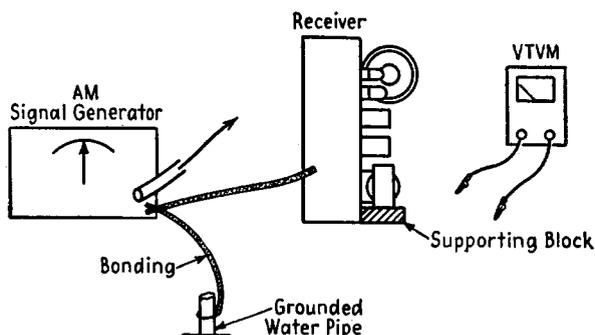
FIG. 26-4. Setting up equipment for meter alignment.
