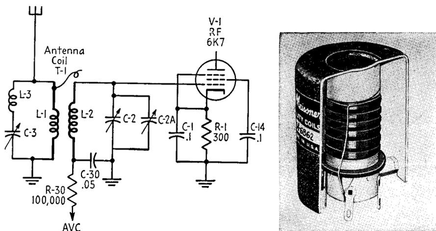
FIG. 16-5. An antenna coil and its position in the RF circuit.
