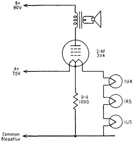
FIG. 19-11. Resistor compensating for the B current of the 3V4 tube.
