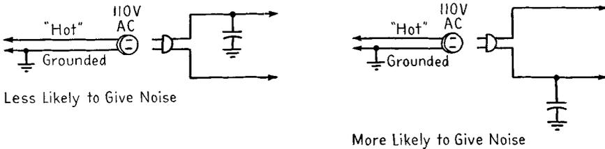
FIG. 17-15. Noise reduction by reversing the receiver line plug.
