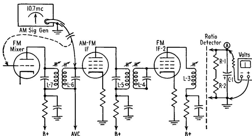
FIG. 26-14. Alignment of the IF stages of a ratio-detector type of receiver.
