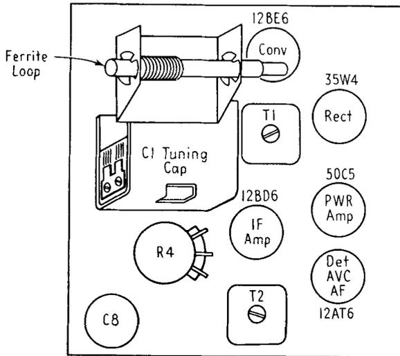
FIG. 17-22. The ferrite antenna mounted in position in a receiver.
