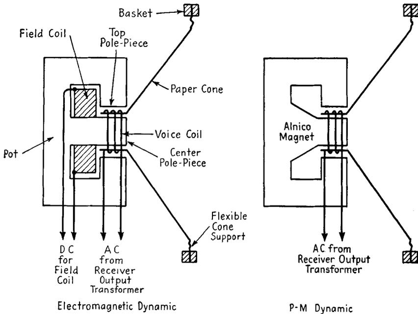
FIG. 9-1. Typical moving-coil dynamic speakers.
