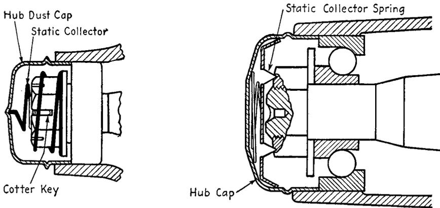
FIG. 20-10. Front-wheel static-collector-spring installation.
