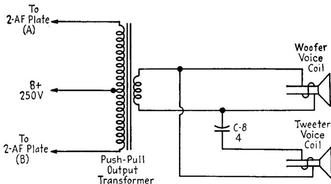
FIG. 22-18. A high-fidelity loudspeaker system.
