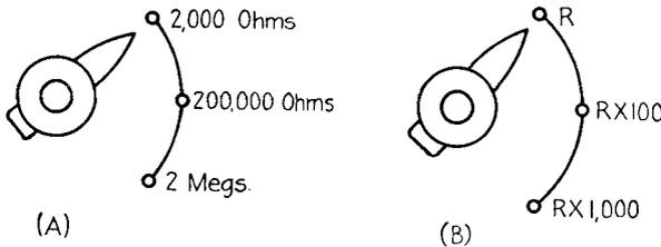
FIG. 4-15. Typical ohmmeter range switches.
