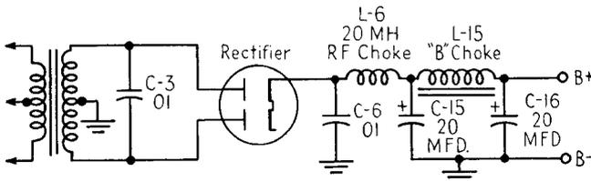
FIG. 21-12. An RF filter in the *B* plus circuit for hash suppression.
