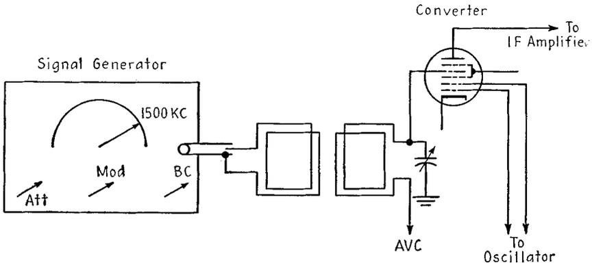
FIG. 14-5. Method of connecting a signal generator to a loop-operated receiver.
