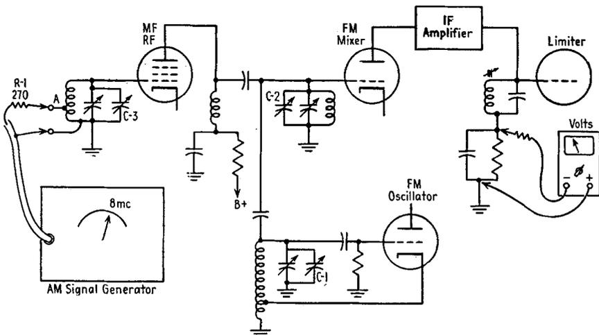
FIG. 26-10. Aligning the RF end of the receiver.
