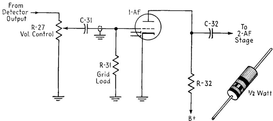
FIG. 11-19. The first AF grid-load resistor and its position in the circuit.
