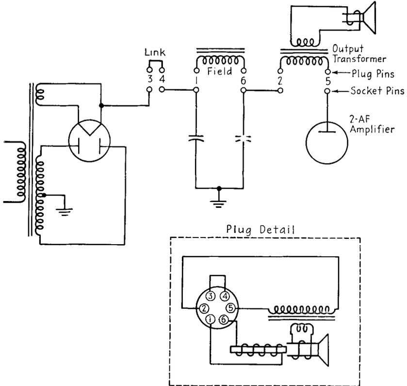
FIG. 28-9. Speaker-plug arrangement which opens the *B* circuit when the plug is removed.
