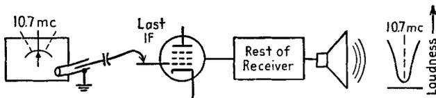
Connect signal generator to last IF grid.
