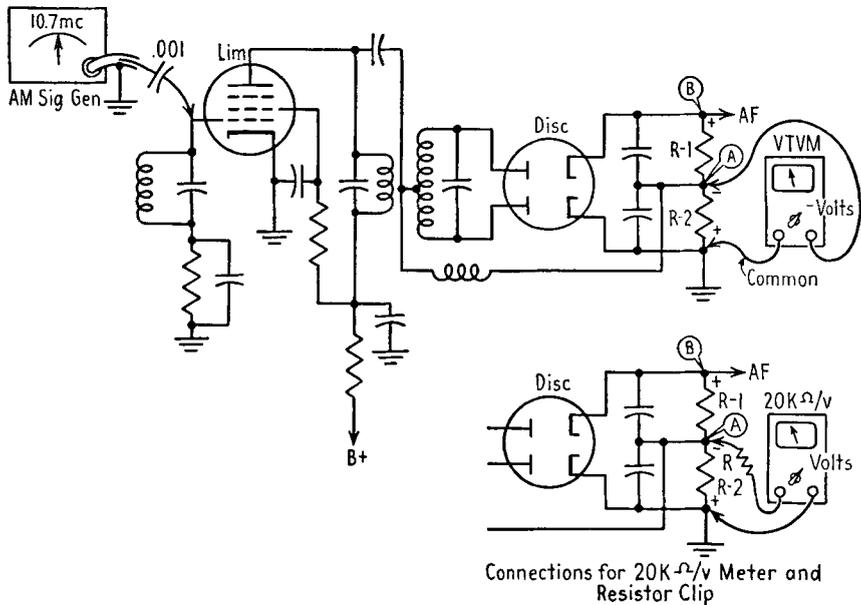
FIG. 26-6. Alignment of a Foster-Seeley discriminator.
