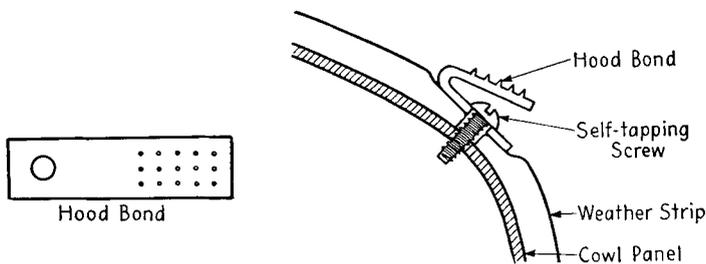
FIG. 20-6. Hood-bond installation.
