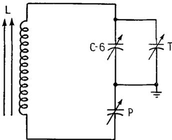
FIG. 14-24. Oscillator tuning-circuit for adjustments.
