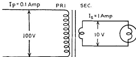
FIG. 10-7. Transformer lighting one lamp.
