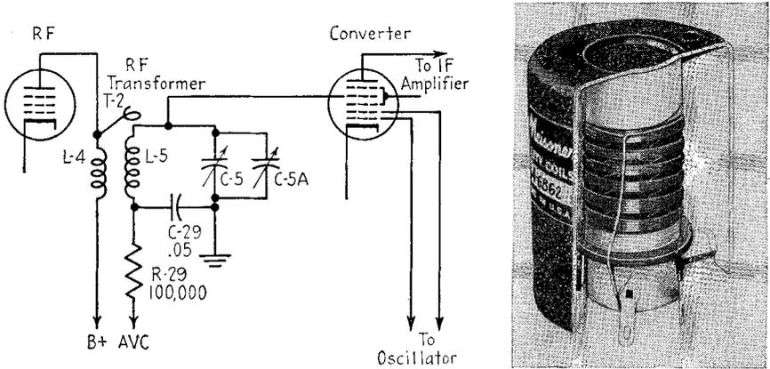
FIG. 14-9. A typical interstage RF transformer and its position in the circuit.
