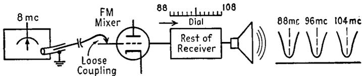
Connect signal generator output loosely to F-M mixer grid.
