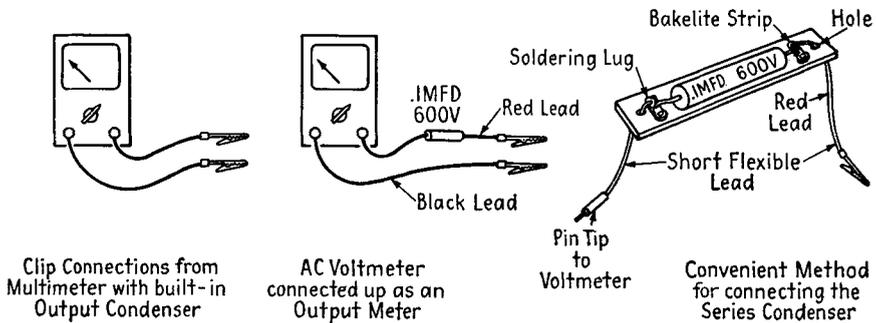
FIG. 11-7. Test leads for the output meter.
