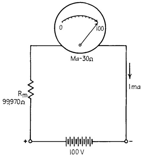
FIG. 4-3. Voltmeter with 0- to 1-volt range at full-scale deflection.
