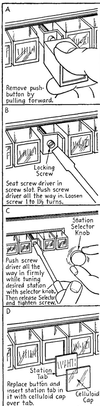
FIG. 15-15. Adjustment of push button for mechanical automatic tuners.
