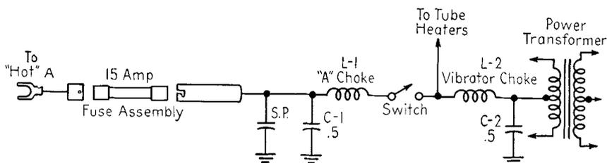
FIG. 21-19. Partial automobile radio A circuit.
