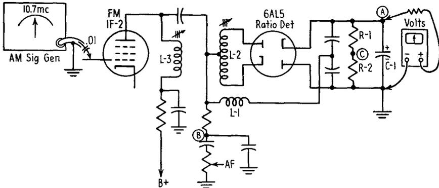
FIG. 26-11. Alignment of the ratio detector, with test points indicated.
