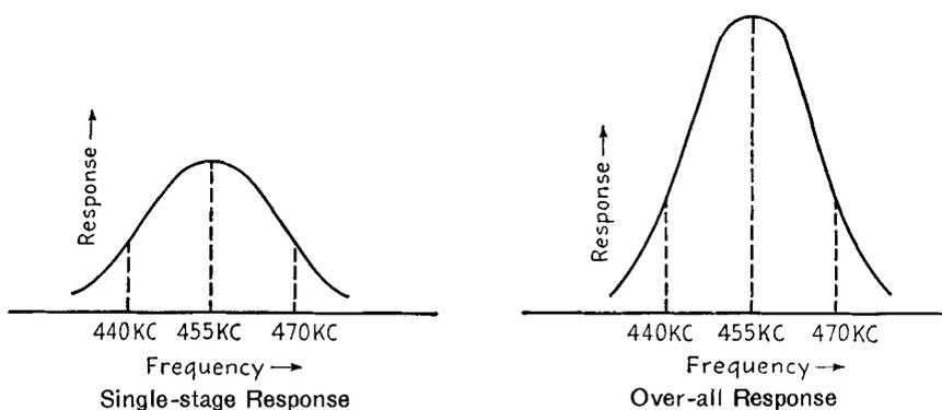
FIG. 13-18. Frequency-response curve of a high-fidelity IF amplifier.
