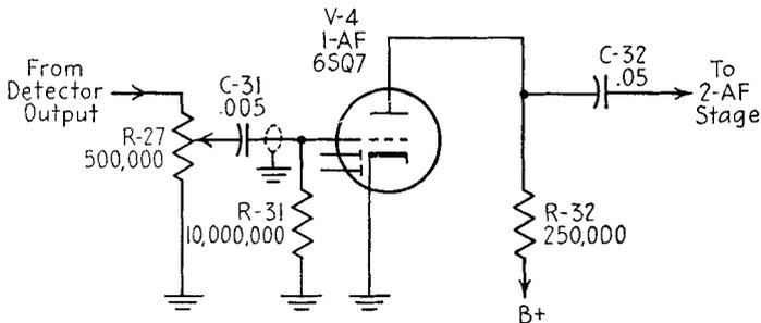
FIG. 11-1. Typical first audio-frequency amplifier stage.
