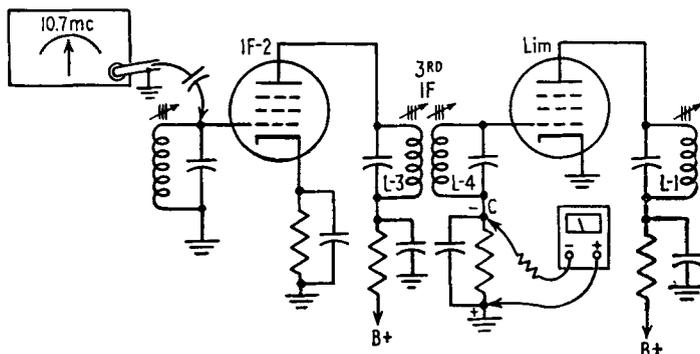
FIG. 26-8. Aligning the third IF transformer.
