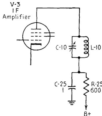
FIG. 13-10. Plate-circuit decoupling filter in the IF amplifier stage.
