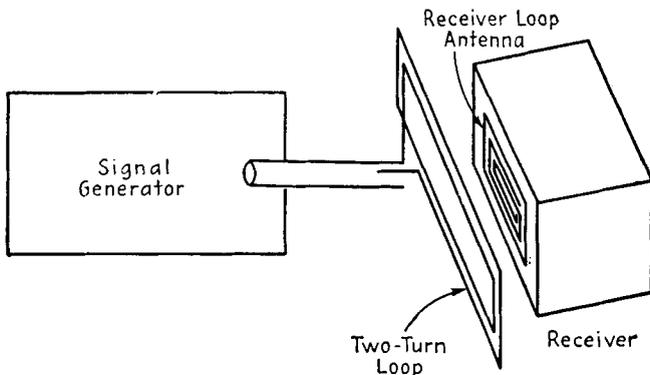
FIG. 23-2. Coupling the signal generator to a loop-operated receiver.
