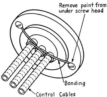
FIG. 20-8. Control-cable bonding installation.
