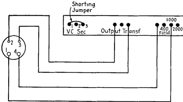
FIG. 28-8. Connecting the bench test speaker to a receiver using a standard four-prong speaker-plug arrangement.
