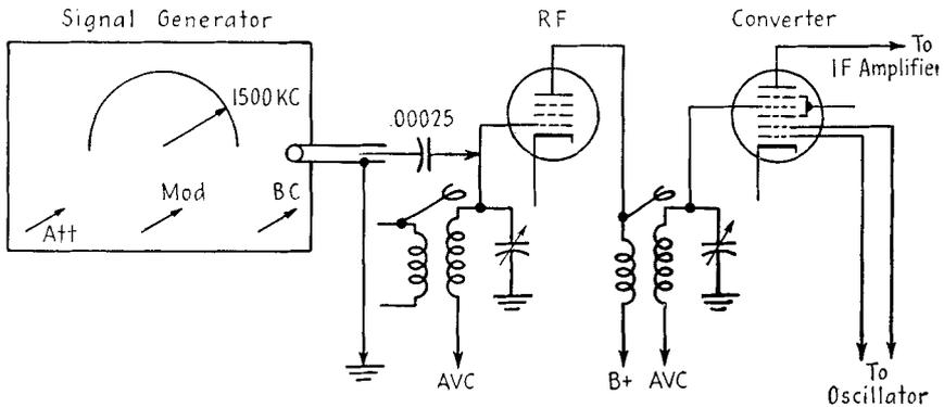
FIG. 14-7. Signal-generator connections for sensitivity measurements of the converter when the receiver incorporates an RF stage.
