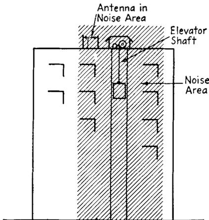
FIG. 17-9. An antenna installed in a noise area.
