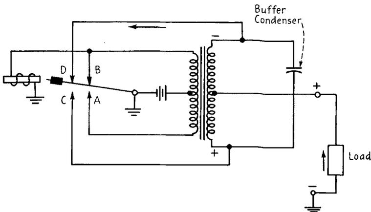
FIG. 21-21. The synchronous vibrator: operation position 2.
