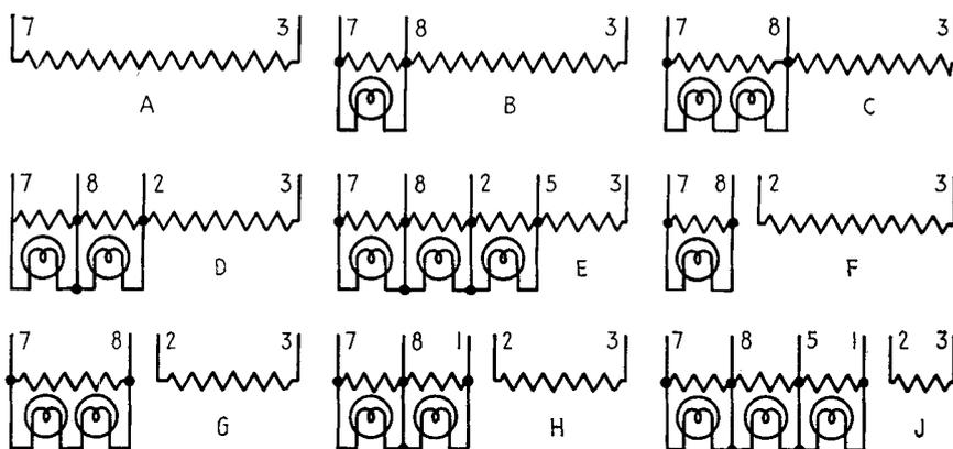
FIG. 18-18. Standard base wiring for ballast tubes.
