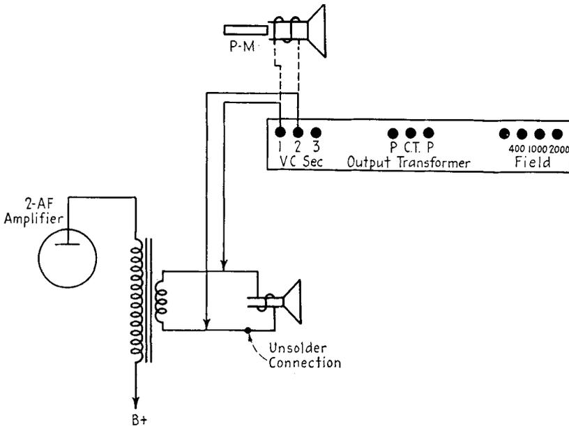
FIG. 28-5. Checking a speaker voice coil by substituting the bench test speaker.
