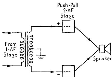
FIG. 22-1. Block diagram of a push-pull amplifier.
