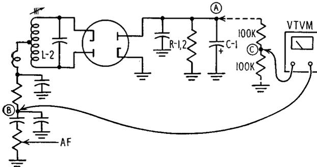
FIG. 26-13. Making up a test point for a ratio-detector variation.
