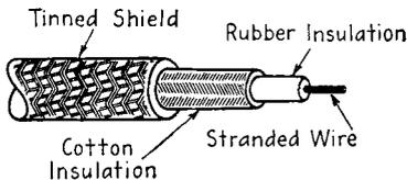
FIG. 17-11. Structure of shielded lead-in wire.
