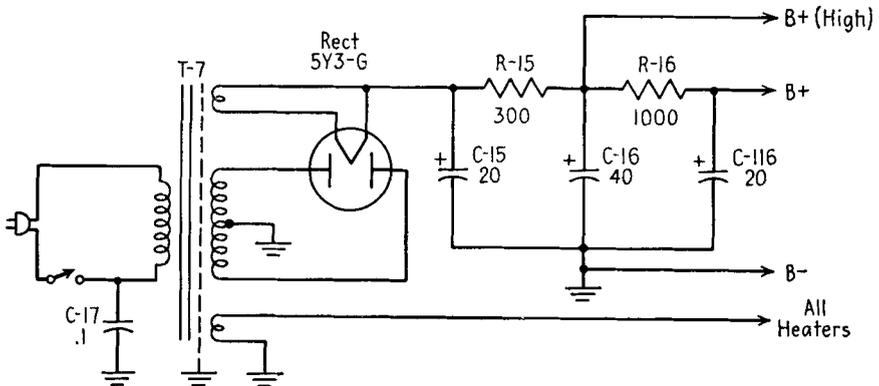
FIG. 8-22. Power supply with R-C filter.
