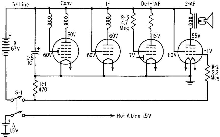
FIG. 19-22. Basic A and B circuits of a battery portable receiver.
