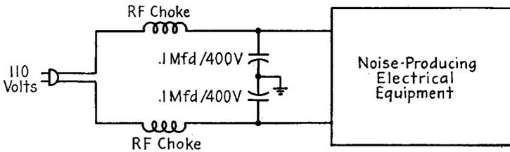
FIG. 17-16. Filtering line noise at the source.
