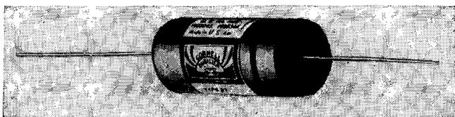
FIG. 8-17. Paper tubular condenser.
