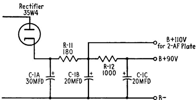
FIG. 18-27. Two-section R-C filter used in the receiver shown in Fig. 18-26.
