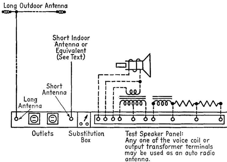
FIG. 28-10. Panel on test bench showing antenna leads.
