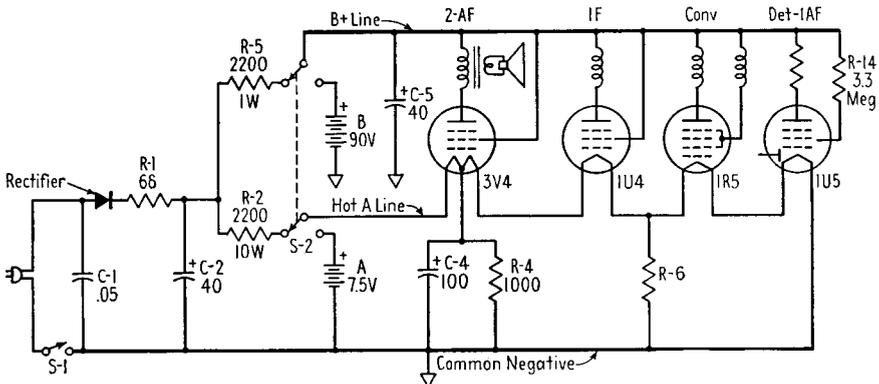
FIG. 19-23. Basic A and B circuits of a three-way portable receiver.
