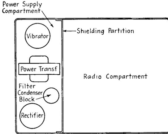
FIG. 21-8. Top view of an automobile radio, showing separate shielded compartments for the receiver and power supply.
