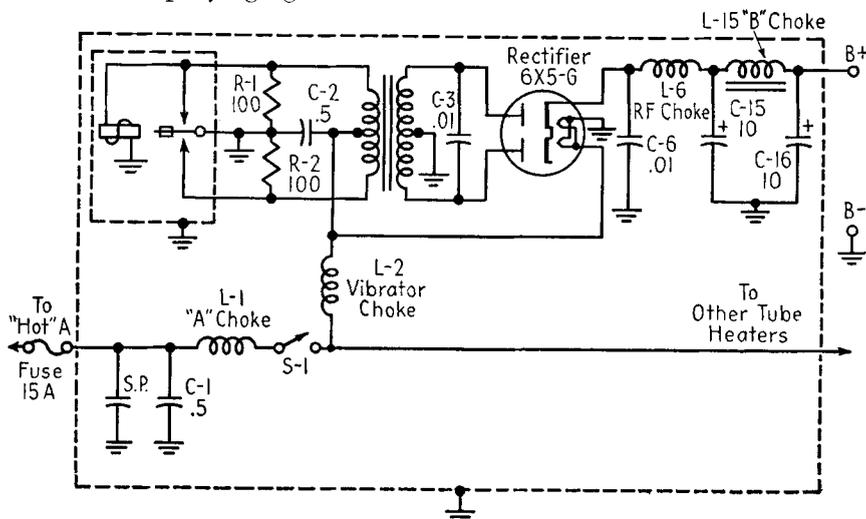
**Normal voltage data for the auto radio power supply**
