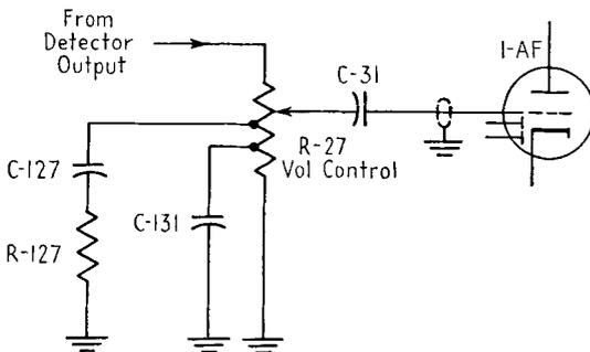
FIG. 11-23. Bass compensation at two points in the volume range.
