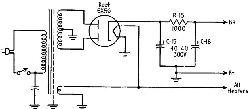
FIG. 8-24. Power supply in small AC receivers.
