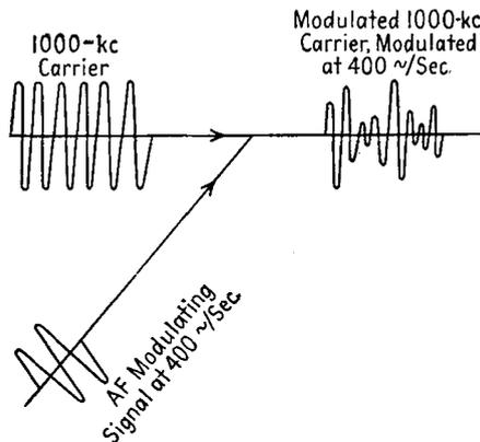
FIG. 24-1. The A-M signal.
