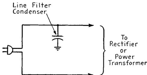
FIG. 17-14. Line filter condenser in a receiver.
