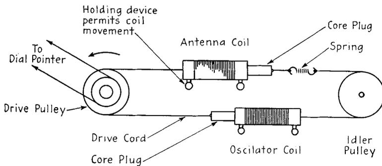
FIG. 15-6. Drive-cord type of permeability tuner.
