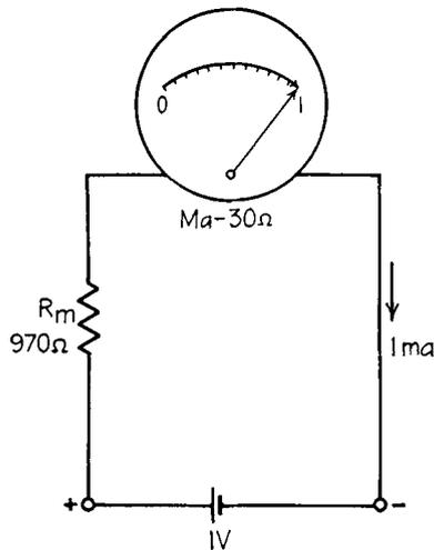
FIG. 4-4. Voltmeter with 0- to 100-volt range at full-scale deflection.
