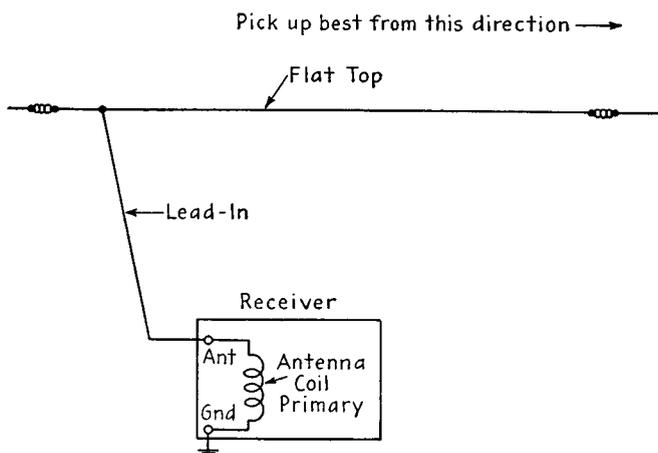
FIG. 17-1. Simple inverted-L antenna.
