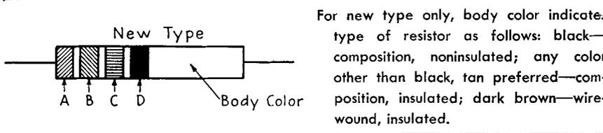
For new type only, body color indicates type of resistor as follows: black—composition, noninsulated; any color other than black, tan preferred—composition, insulated; dark brown—wire-wound, insulated.
