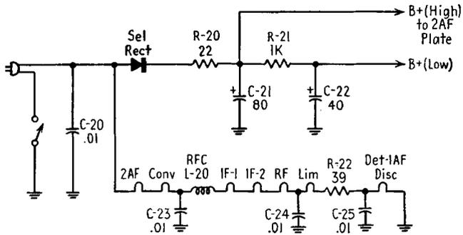
FIG. 25-6. Typical AC/DC power supply for an A-M/F-M receiver.
