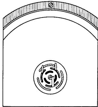
FIG. 9-8. Centering a voice coil with three shims.
