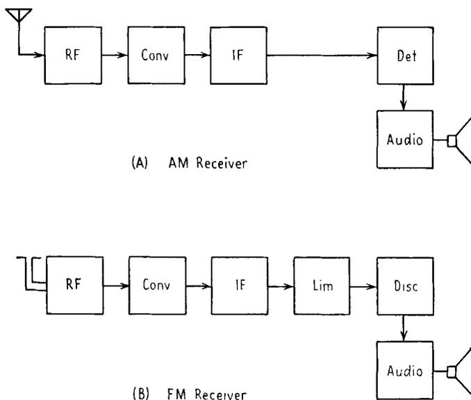
FIG. 24-6. Comparison of A-M and F-M receivers.
