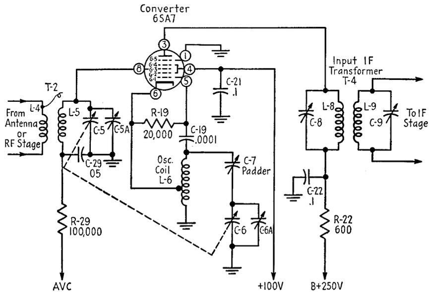
FIG. 15-1. Schematic diagram of a 6SA7-type pentagrid converter.
