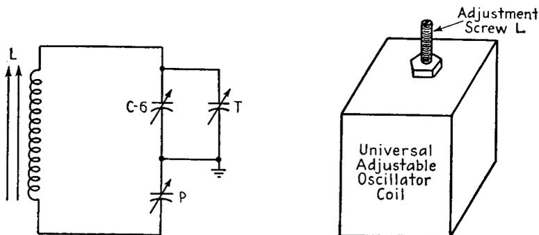
FIG. 14-22. Oscillator tuning-circuit adjustments when a universal adjustment replacement oscillator coil is used: *T*, high-frequency trimmer; *P*, series 600 padder; *C-6*, main tuning condenser.
