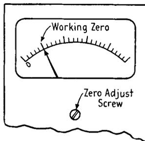
FIG. 26-7. Adjusting a meter to get an off-zero, no-voltage point.
