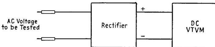
FIG. 4-18. Basic electronic AC voltmeter.
