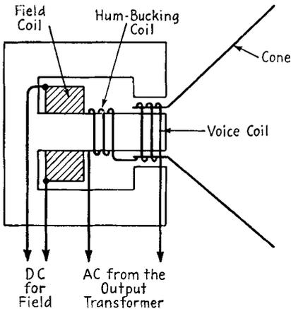
FIG. 9-5. Electrodynamic speaker with a hum-bucking coil.
