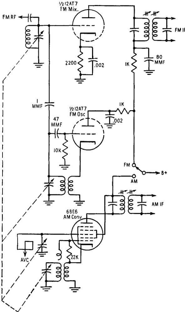
FIG. 25-13. A-M/F-M converter with separate oscillator tube.
