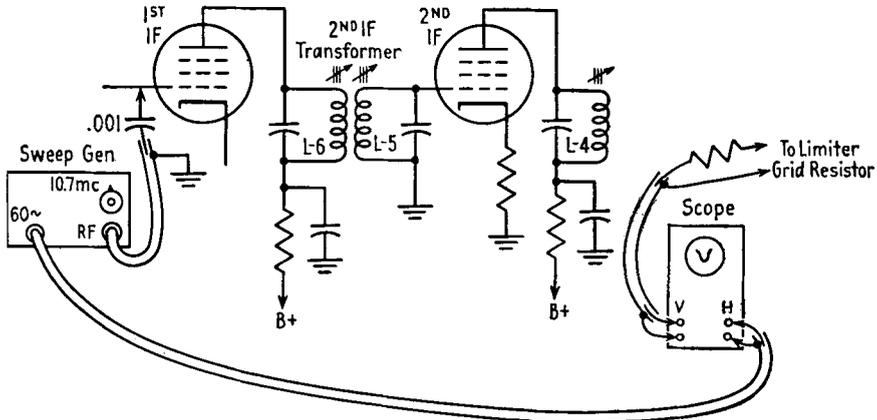
FIG. 26-21. Alignment of the second IF transformer.
