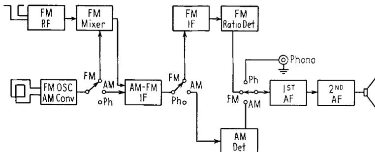
FIG. 25-1. Block diagram of a typical A-M/F-M receiver.
