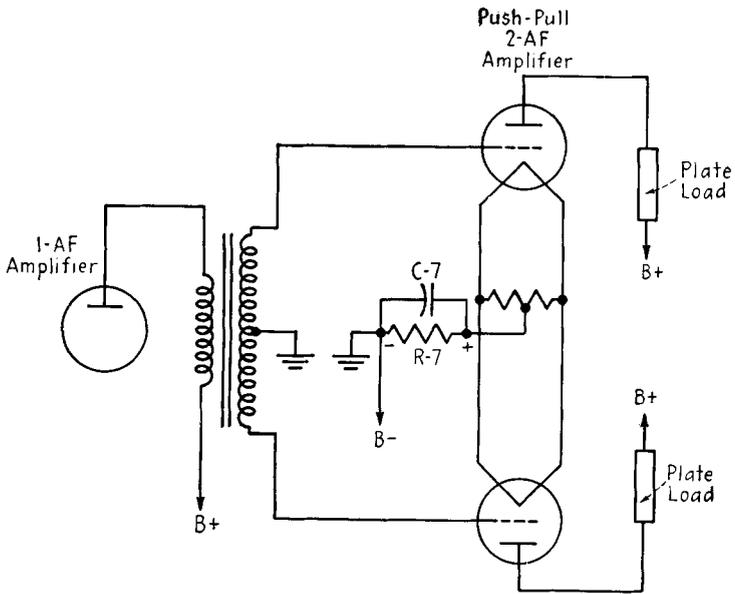
FIG. 22-4. A method of obtaining bias voltage for a push-pull stage.
