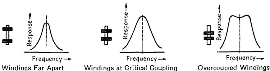
FIG. 13-19. Effect of coupling on the frequency-response curve of an IF transformer.
