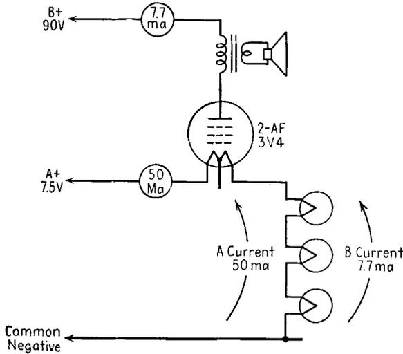
FIG. 19-10. Plate and filament currents of the 3V4 second AF tube.
