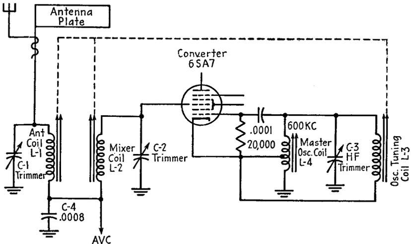
FIG. 15-9. Three-coil permeability tuner with a preselector circuit.
