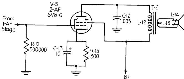
FIG. 10-6. The AF by-pass condenser and its position in the second AF circuit.
