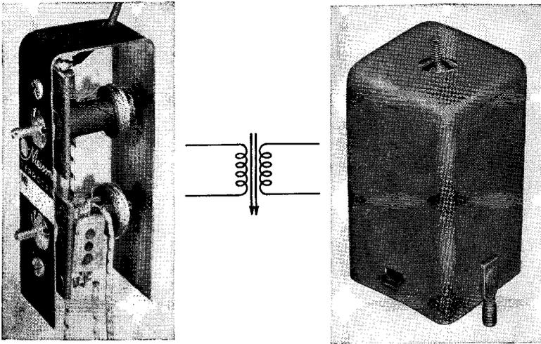
FIG. 12-9. Permeability-tuned IF transformers.
