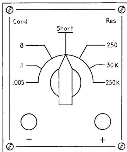
FIG. 28-12. Front panel of resistor and condenser substitution box.
