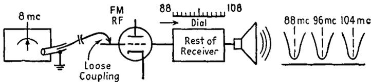
Connect signal-generator output loosely to F-M RF grid.
