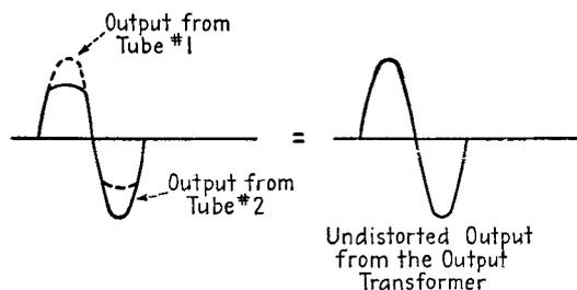
FIG. 22-7. Wave form showing cancellation of even-harmonic distortion in the output circuit of a push-pull amplifier.
