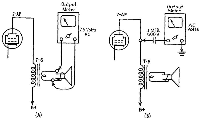
FIG. 11-6. Connection of an AC voltmeter as an output meter.
