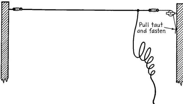
FIG. 17-6. Attaching the second end of the antenna.
