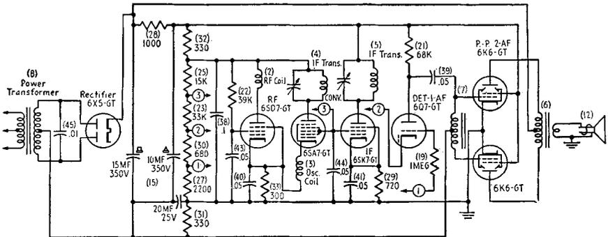
FIG. 21-18. Skeleton *B* circuit of the automobile radio receiver in Fig. 21-13.
