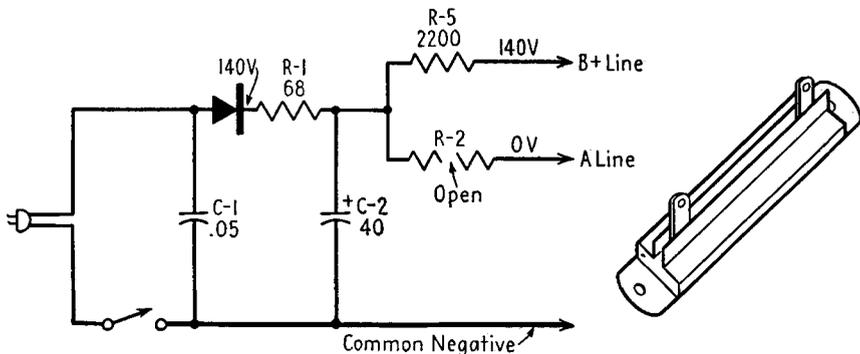
FIG. 19-18. A typical A filter resistor and the effect when it is open.
