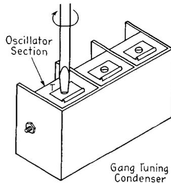
FIG. 14-27. Adjusting the high-frequency trimmer *T*.
