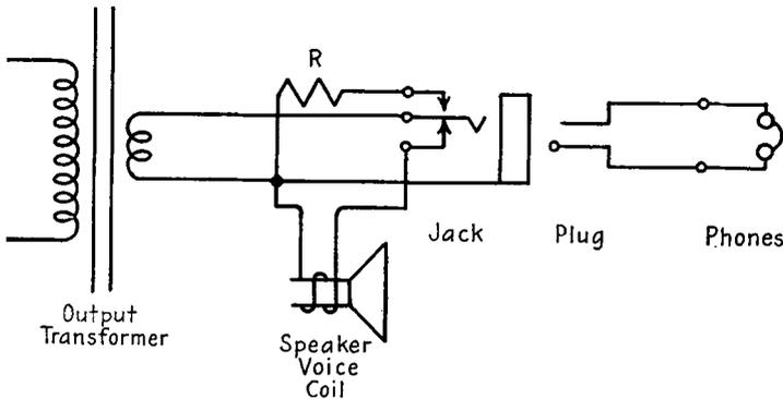
FIG. 9-18. Circuit for adding headphones to a receiver—using jack and plug.
