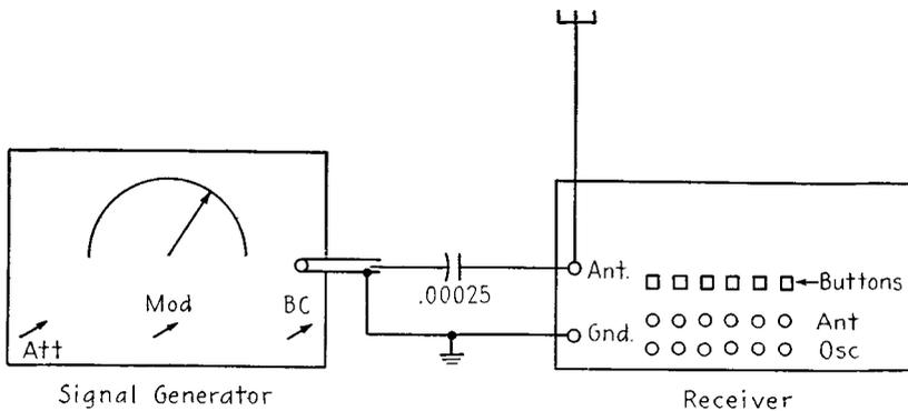
FIG. 15-13. Using a signal generator as an aid in quickly presetting push buttons.
