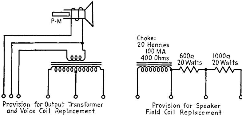
FIG. 28-3. Bench test speaker.
