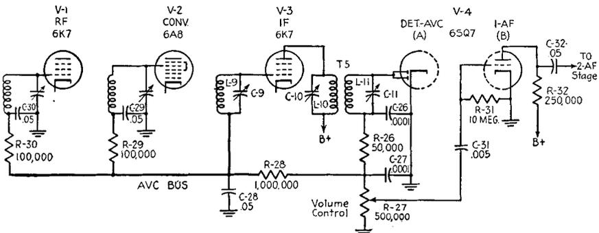
FIG. 12-5. Typical detector and AVC circuit.
