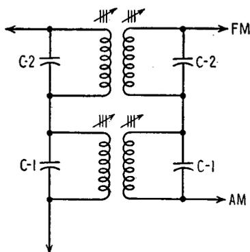
FIG. 24-17. IF transformer assembly for an A-M/F-M receiver.
