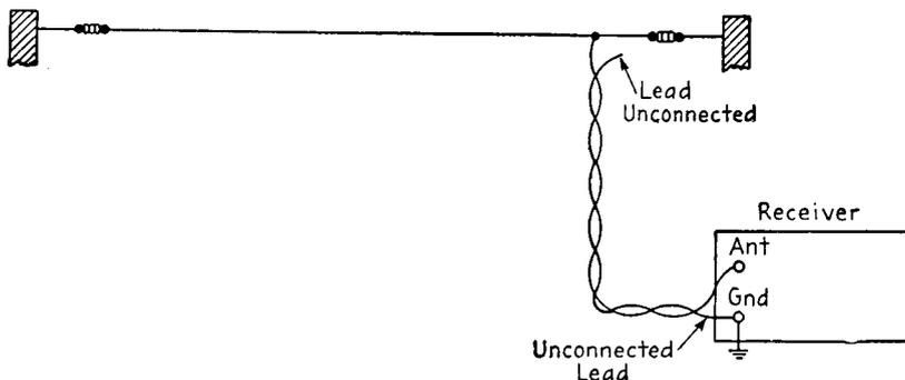
FIG. 17-13. Noise reduction by means of a twisted-pair lead-in.
