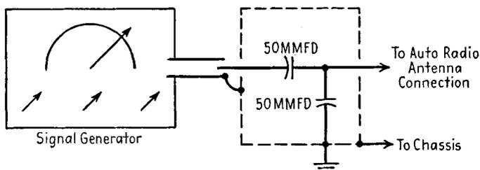
FIG. 23-1. Automobile radio coupling device.
