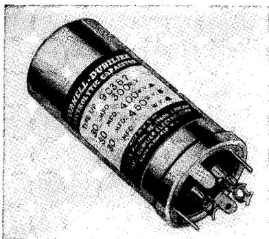
NOTE: The triangle, square, and half-circle on the label are to identify the individual condensers in the block. They are repeated on the insulating strip near the proper soldering lugs.
