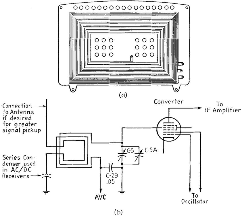
FIG. 14-14. (a) A loop antenna and (b) the schematic diagram of a loop antenna providing signal input to the converter tube.
