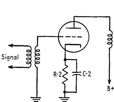
FIG. 25-16. Conventional triode amplifier.
