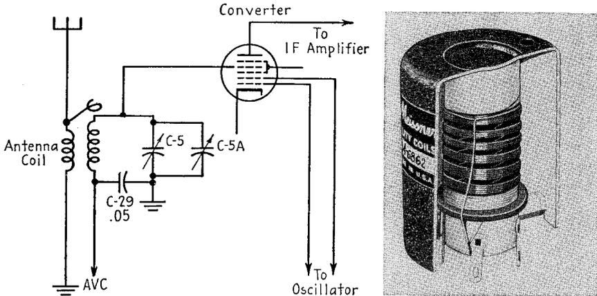
FIG. 14-11. A typical antenna coil and a circuit showing antenna input to the converter tube.
