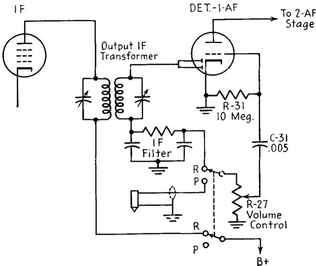
FIG. 12-16. Typical radio-phonograph switching circuit.
