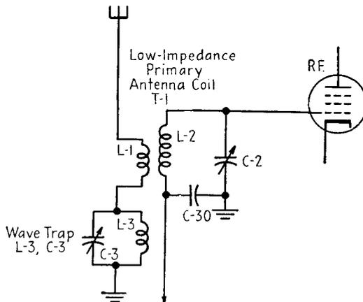
FIG. 16-3. Wave trap in series with antenna circuit.
