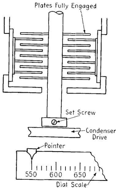
FIG. 14-16. Position of condenser drive, setscrew, and dial pointer.
