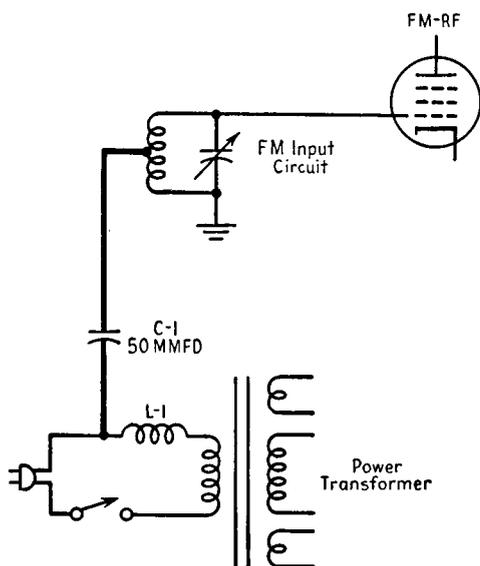
FIG. 17-27. Line-cord antenna for F-M reception.
