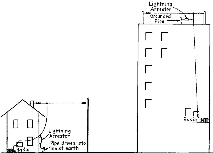
FIG. 17-8. The installation of lightning arresters.
