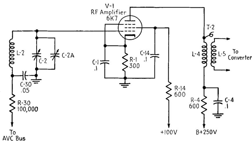
FIG. 16-4. Decoupling filters in the RF stage.
