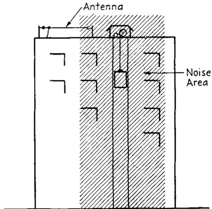
FIG. 17-10. Moving antenna out of the noise area.
