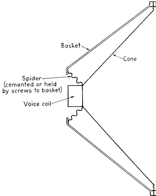
FIG. 9-9. Inside spider connected to speaker basket.
