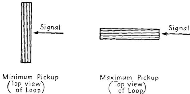
FIG. 17-21. Directional characteristic of a loop antenna.
