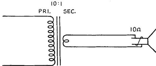
FIG. 10-9. Transformer feeding a 10-ohm voice coil.
