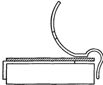
FIG. 23-10. Provision to avoid microphonics when the trimmer condenser peaks at the low-capacity setting.
