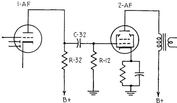
FIG. 11-4. Resistance coupling between the first AF and second AF stages.
