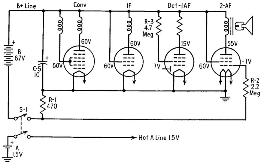
FIG. 19-7. A and B circuit of a battery portable receiver.
