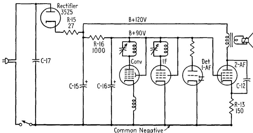
FIG. 18-24. Skeleton *B* circuit of a typical AC/DC receiver.
