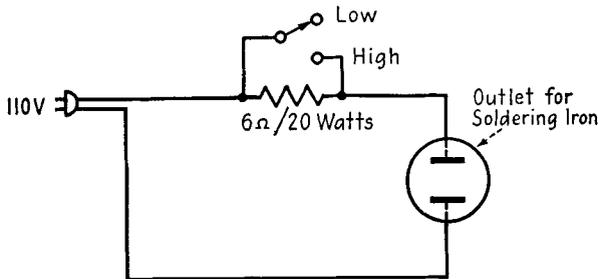
FIG. 28-13. Schematic diagram of a "high-low" soldering-iron outlet.
