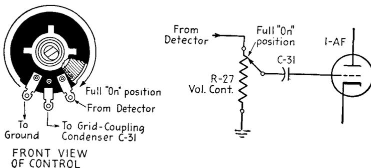
FIG. 11-16. Volume-control connections.
