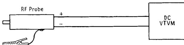
FIG. 4-19. Basic electronic RF voltmeter.
