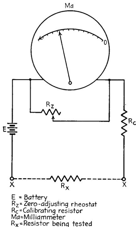
FIG. 4-13. Basic ohmmeter circuit.
