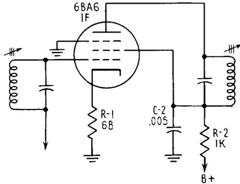
FIG. 24-9. A typical F-M IF amplifier stage.
