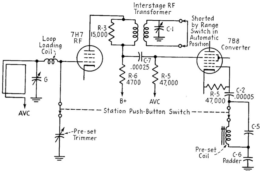
FIG. 15-12. Simplified diagram of the tuning circuit of the Zenith receiver shown in Fig. 15-11.
