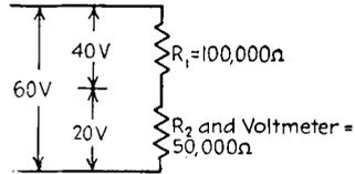
Which voltmeter was correct in its reading? If interpreted properly, both gave correct results. The serviceman may use either of the two voltmeters of different sensitivities, but at all times he must interpret his results. Generally, it is true that, when the voltage across a high-resistance circuit is measured, the voltmeter of the higher ohms-per-
