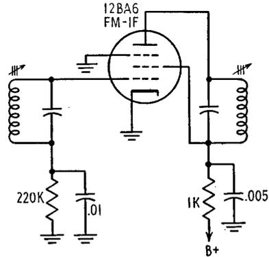
FIG. 25-10. A variation of the IF amplifier in an A-M/F-M receiver.
