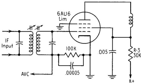
FIG. 24-12. A typical F-M limiter stage.
