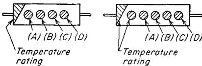
Tubular condensers read from the end color to the right. End color identifies inside lead. Leads may be axial or radial.
