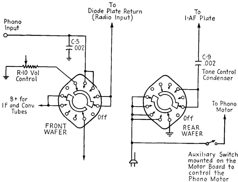
FIG. 12-23. Alternate radio-phonograph switching circuit for the receiver shown in Fig. 12-17.
