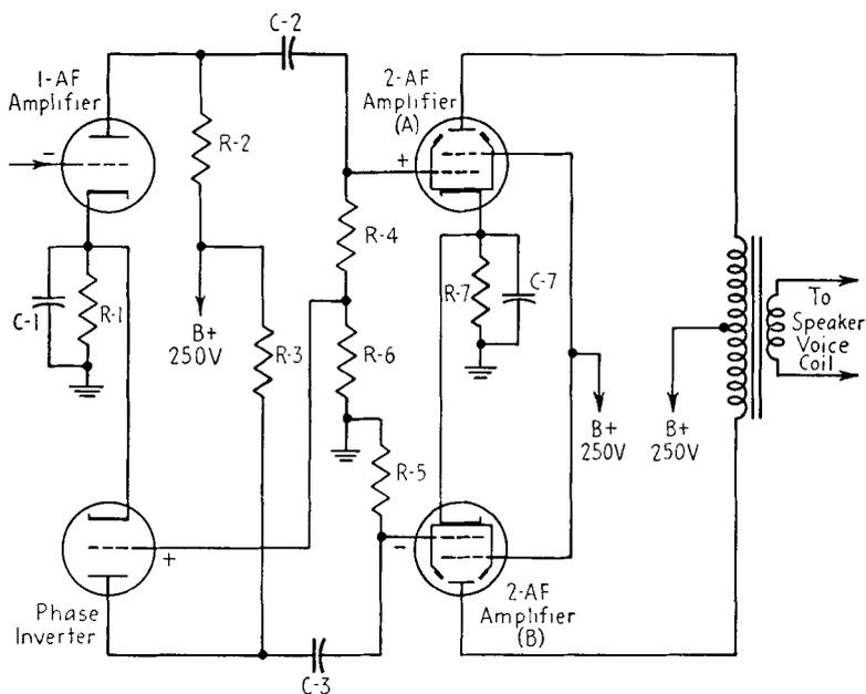
FIG. 22-12. Obtaining a negative signal on the other push-pull tube grid from the output of the phase-inverter tube.
