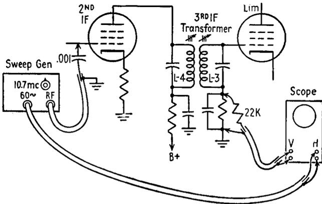
FIG. 26-19. Visual alignment of the third IF transformer.
