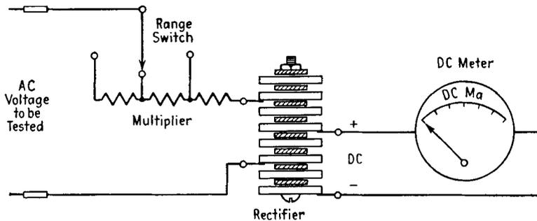
FIG. 4-12. Typical multirange AC voltmeter.
