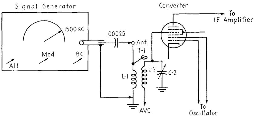
FIG. 14-8. Signal-generator connections for measurements of converter gain when the receiver does not include an RF stage.
