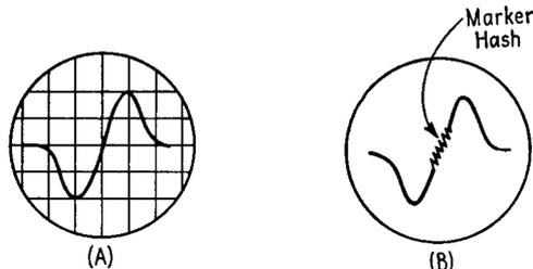
FIG. 26-25. Trace in alignment of the secondary of the discriminator transformer.
