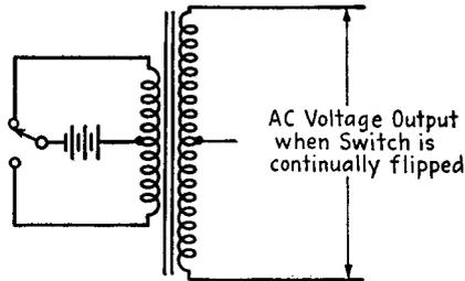
FIG. 21-5. Reversing direct current through a transformer primary.
