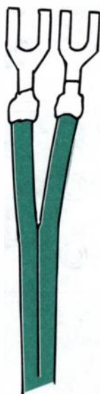
2-wire audio cable with spade lugs
