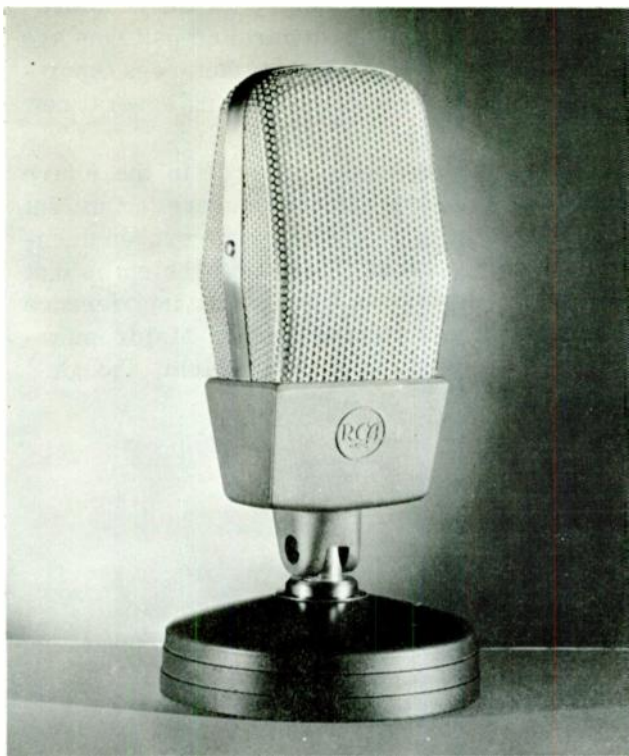
Fig. 12-7. A typical velocity microphone.
