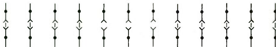
Fig. 6-5. Typical jack panel terminations for "Plan 1 or 2" broadcast stations.
