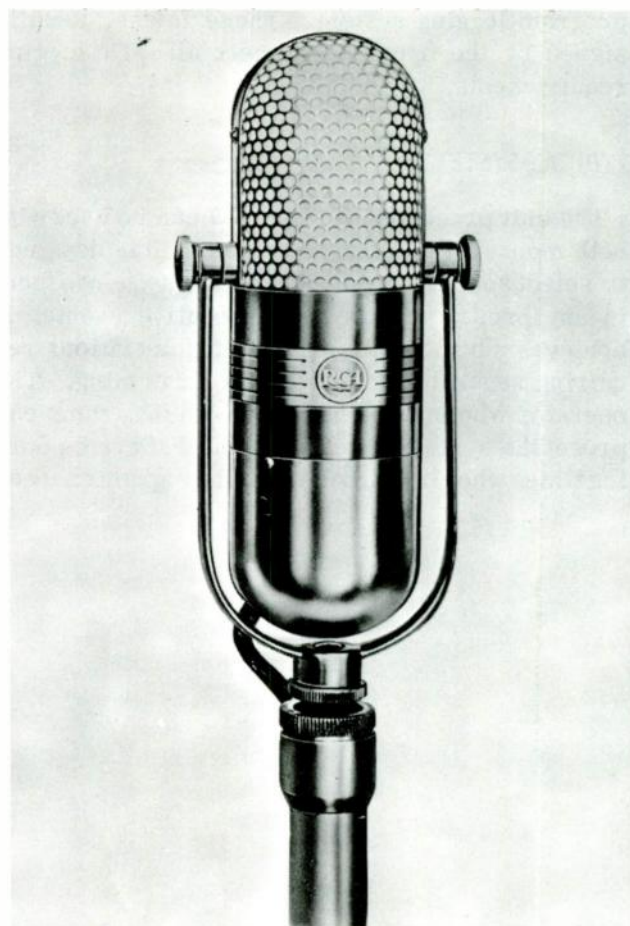
Fig. 12-2. A polydirectional microphone.
