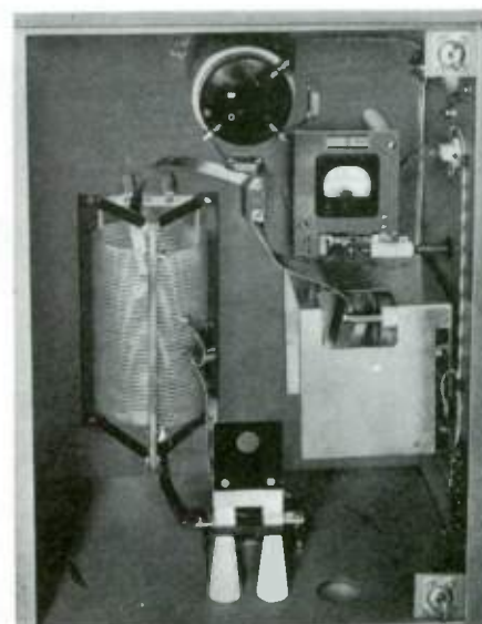
Fig. 7-5. A typical antenna tuning unit. The lighting choke is at the top of the cabinet.
