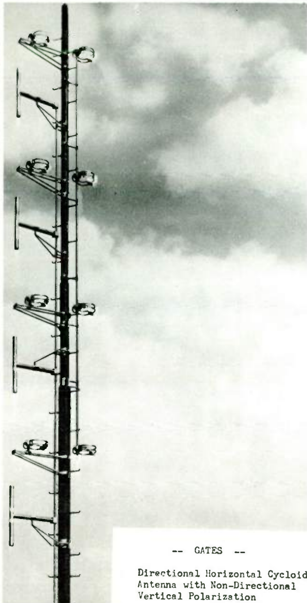
Fig. 8-14. Directional horizontal antenna with non-directional vertical antenna.
