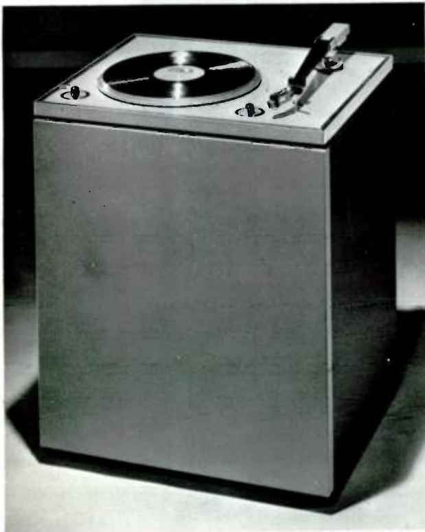
Fig. 10-10. A dual-speed transcription turntable.
