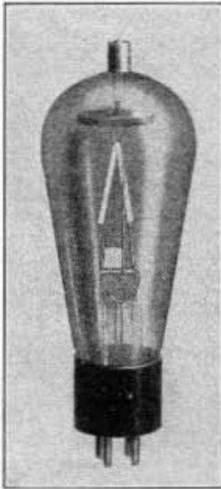
A TYPICAL HOT-CATHODE MERCURY-VAPOR RECTIFIER TUBE
