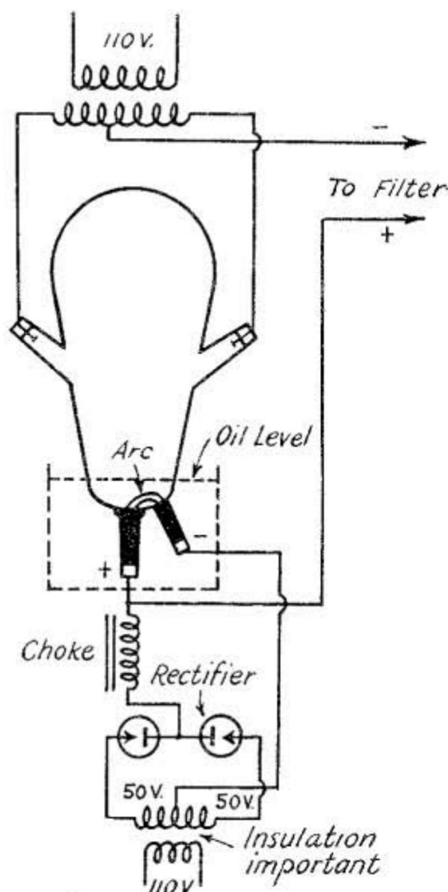
CIRCUIT FOR MERCURY-ARC RECTIFIER
