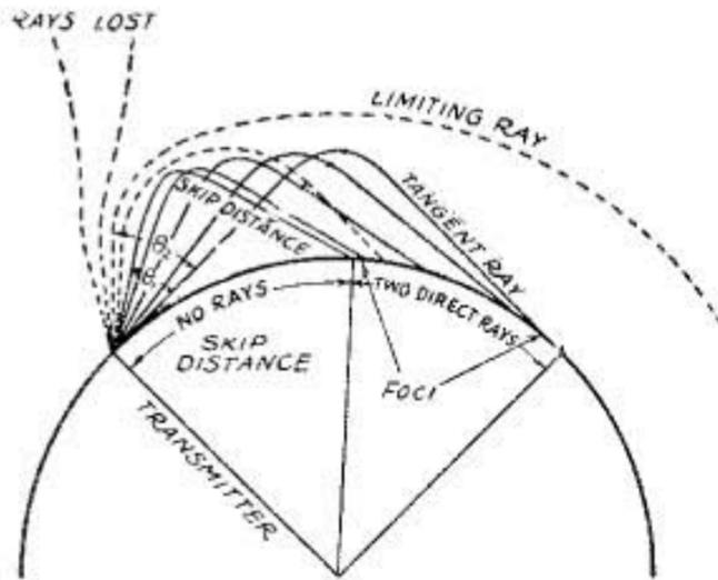
$\theta_1$  ANGLE AT TRANSMITTER CORRESPONDING TO THE FIRST CRITICAL ANGLE
