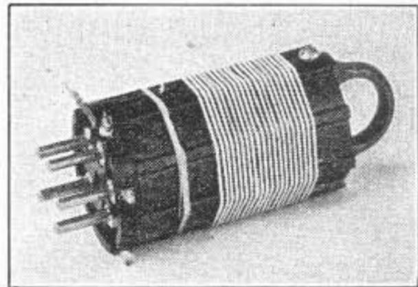
TYPICAL COIL CONSTRUCTION WITH MANUFACTURED FORMS
