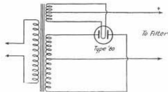
**CONNECTIONS USED WITH A TYPE '80 TUBE**
