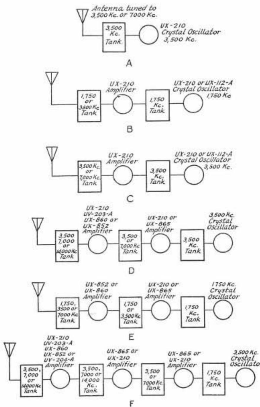
ADDITIONAL SUGGESTIONS FOR TUBE COMBINATIONS IN CRYSTAL-CONTROLLED TRANSMITTERS
