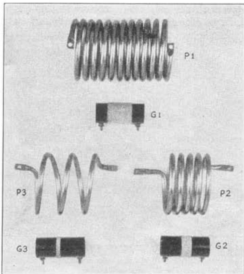
THE PLATE AND GRID COILS
