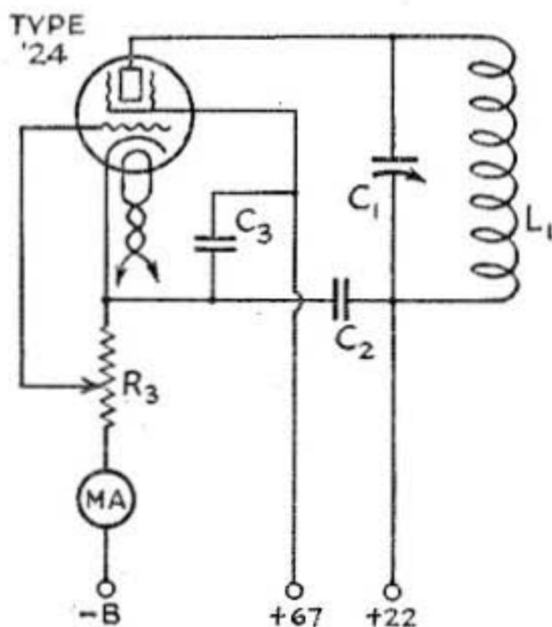
WIRING OF THE A.C. DYNATRON FREQUENCY METER
