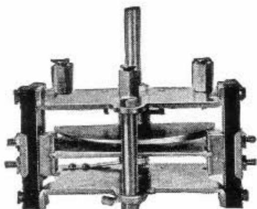
Among the special purpose condensers is the 201-E, a Taper Plate condenser, in which the stator plate is adjustable, affording maximum capacities from 50 mmfds. to 10 mmfds. with a constant minimum of 7 mmfds.
