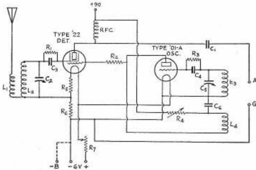
THESE CONNECTIONS ARE USED WITH D.C. TUBES
