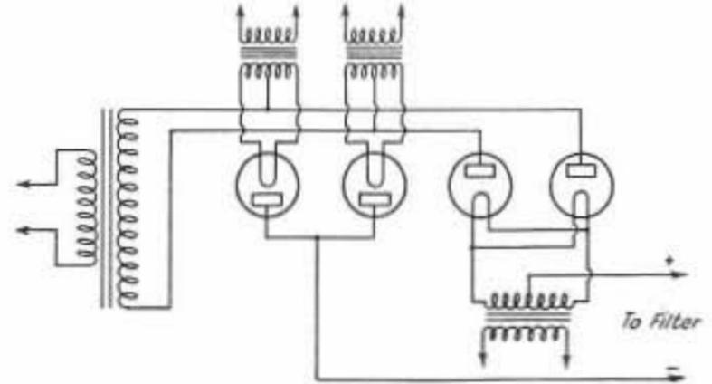
A BRIDGE RECTIFIER WITH MERCURY-VAPOR TUBES
