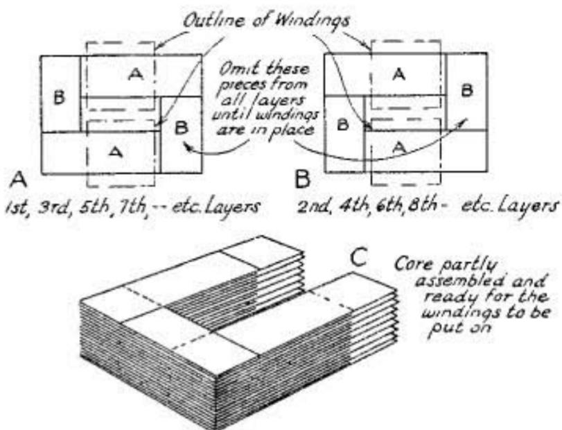
HOW TO PUT A TRANSFORMER CORE TOGETHER
