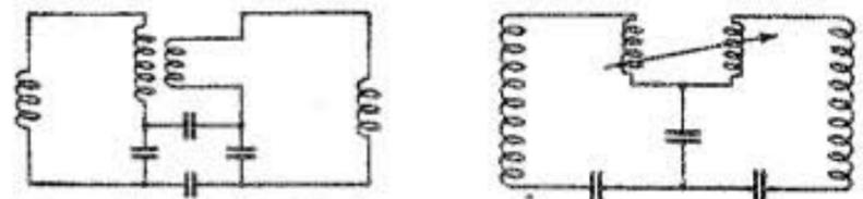
Magnetic and indirect Capacitive Coupling
