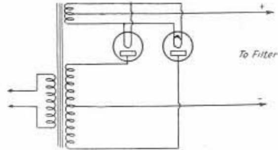
**FULL-WAVE RECTIFICATION WITH THERMIONIC OR MERCURY-VAPOR TUBES**
