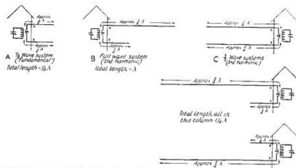
NOTE — Losses tend to be high at points X unless they are near voltage node
