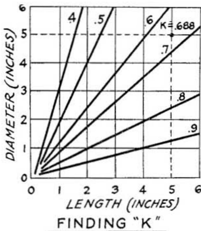
diameter is 5" and the length 5" go to the right from "5" on the diameter scale. At the same time go "up" from "5" on the length scale. Notice where the two lines meet. They meet at "X" between the lines "6" and "7." We estimate the value of *K* at .688 and proceed.
