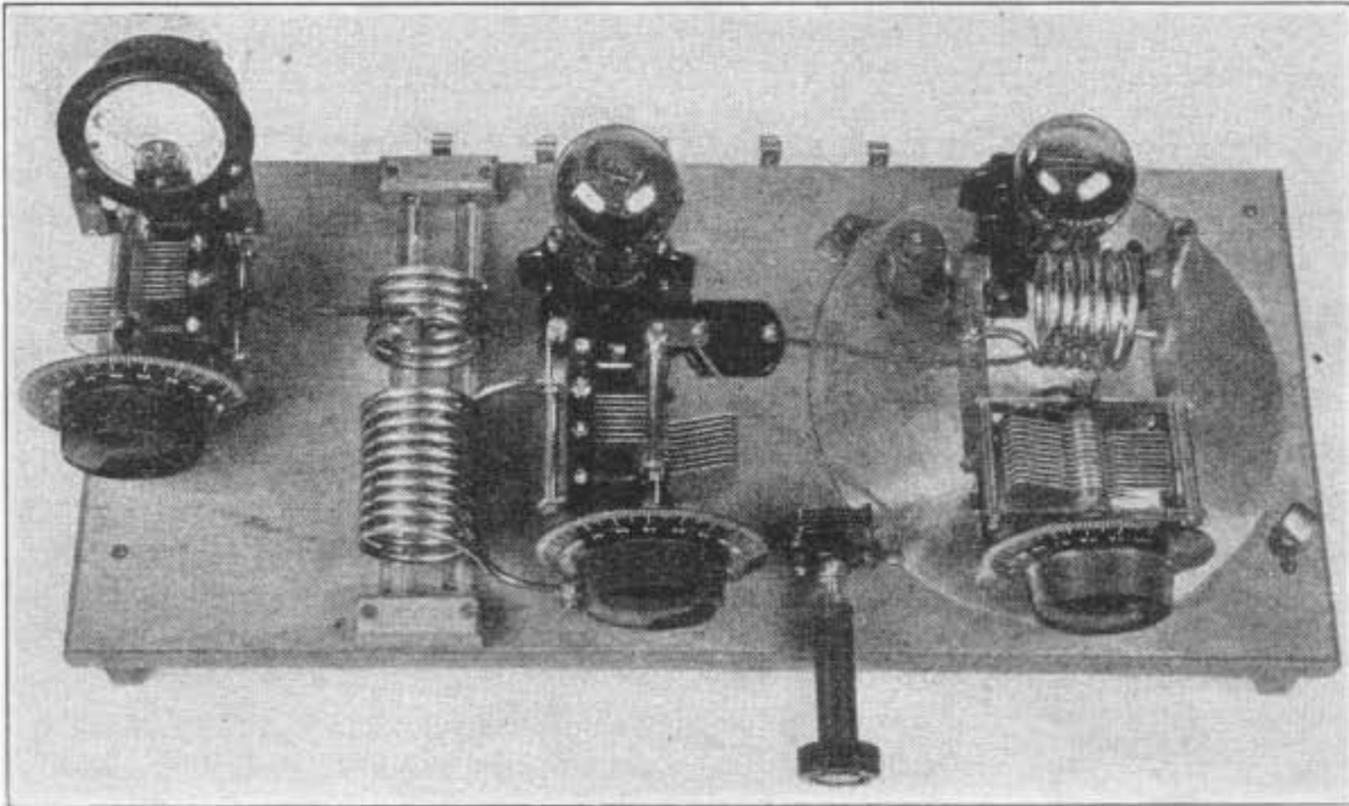
*THE TRANSMITTER WITH THE OSCILLATOR SHIELD REMOVED*
