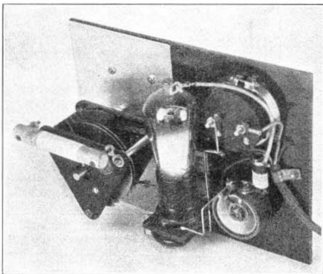
REAR VIEW OF THE DYNATRON FREQUENCY METER
