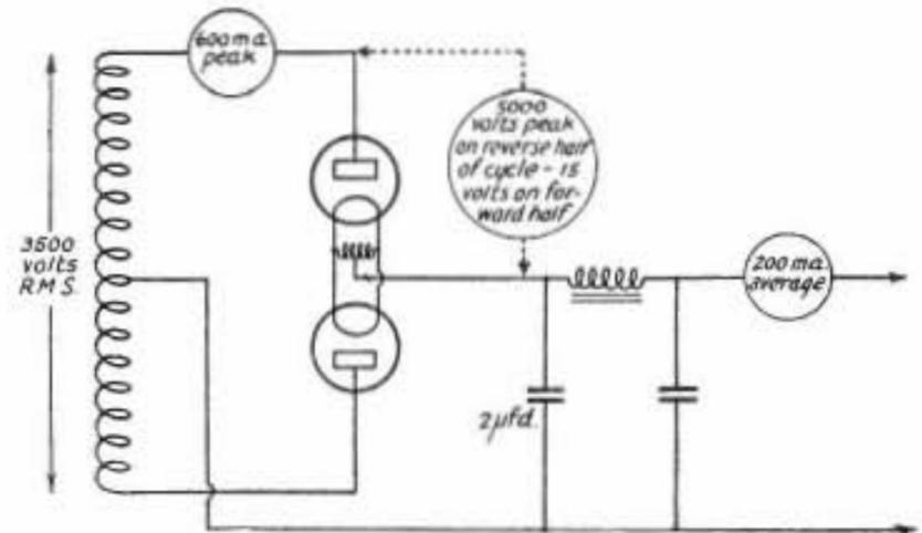
TWO MERCURY-VAPOR TUBES IN A FULL-WAVE CIRCUIT
