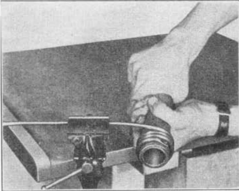
WINDING A COPPER-TUBING INDUCTANCE
