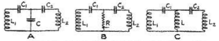
Direct coupling with condenser, resistor, or coil.
