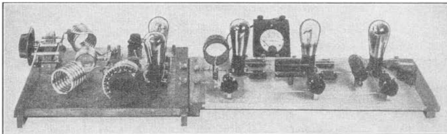
A CRYSTAL-CONTROLLED TRANSMITTER WITH TWO FREQUENCY DOUBLERS
