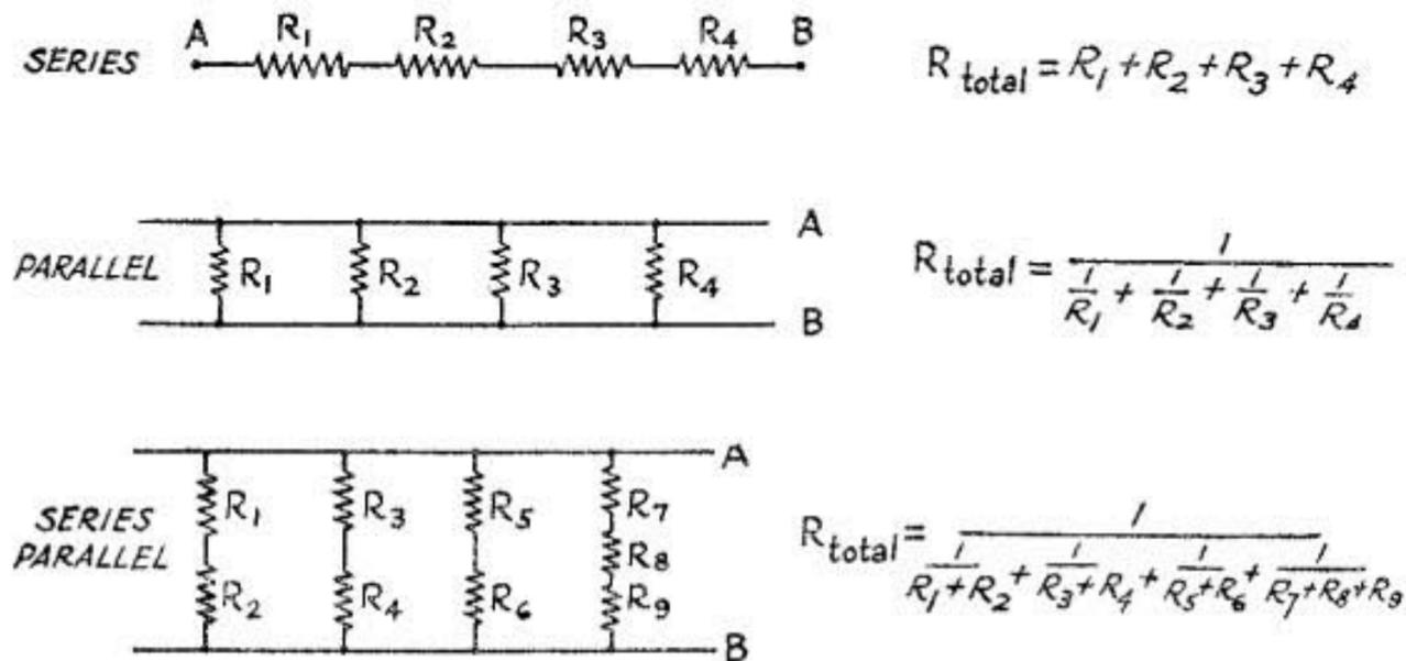
RESISTANCES CONNECTED IN SERIES, PARALLEL, AND SERIES-PARALLEL
