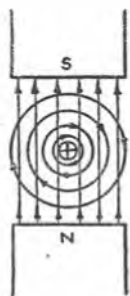
Illustrating Reaction between Current-carrying Conductor and Magnetic Field.
