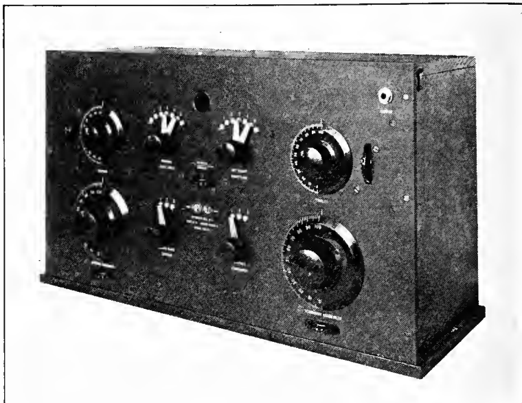
FIG. 113.—Front view of a Grebe receiving set with a range of wave lengths from 500 meters to 24,000 meters.
