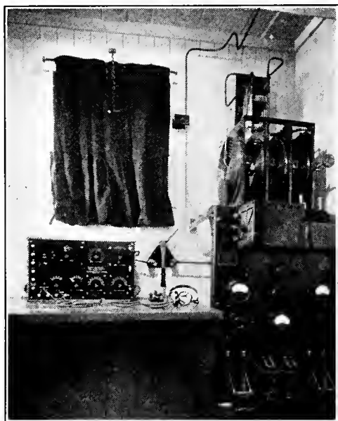
FIG. 170.—A typical spark transmitting ship station, this particular station being on one of the Luckenbach steamers.
