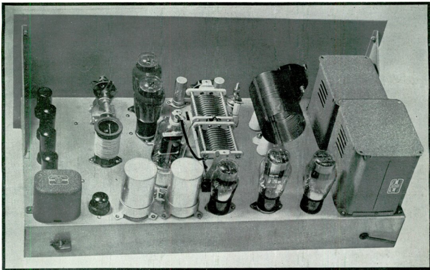
■ Top view of complete transmitter, showing placement of r.f., audio and power supply components. The plate transformers
