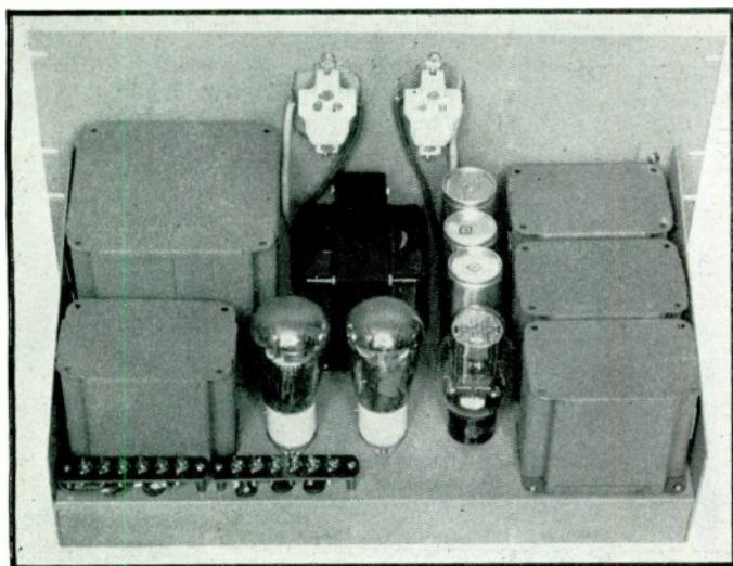
■ Power supply components for buffer-doubler and TZ20 modulator. 866-Jr. rectifier tubes are used. Chassis is 10x17x2 in.
