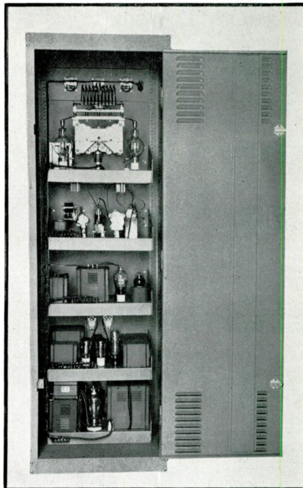
■ Rear view, showing compactness and small size of components for a high power cathode-modulated transmitter.
