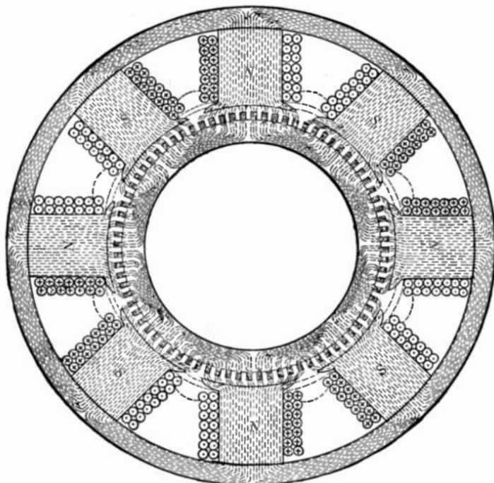
FIG. 182.—Magnetic circuits of a multipolar generator.
