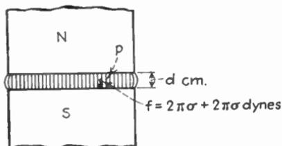
FIG. 146.—Force of attraction between parallel magnetized surfaces.
