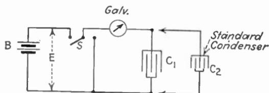
FIG. 243.—Ballistic method of measuring capacitance.
