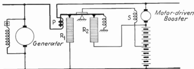
FIG. 435.—Regulating storage-battery discharge with booster set.
