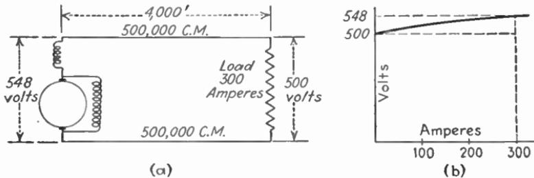
FIG. 337.—Overcompounded generator maintaining constant voltage at the end of feeder.
