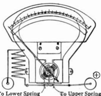
Fig. 93.—A typical Weston direct-current millivoltmeter.
