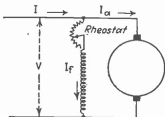
FIG. 399.—Determination of stray power in a dynamo.
