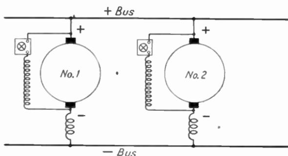
FIG. 408.—Compound generators in parallel.
