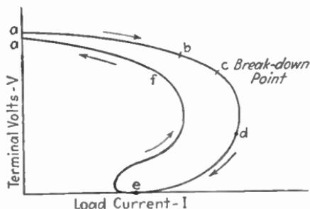
FIG. 327.—Shunt-generator characteristic.
