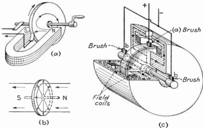
FIG. 349.—Unipolar generator.
