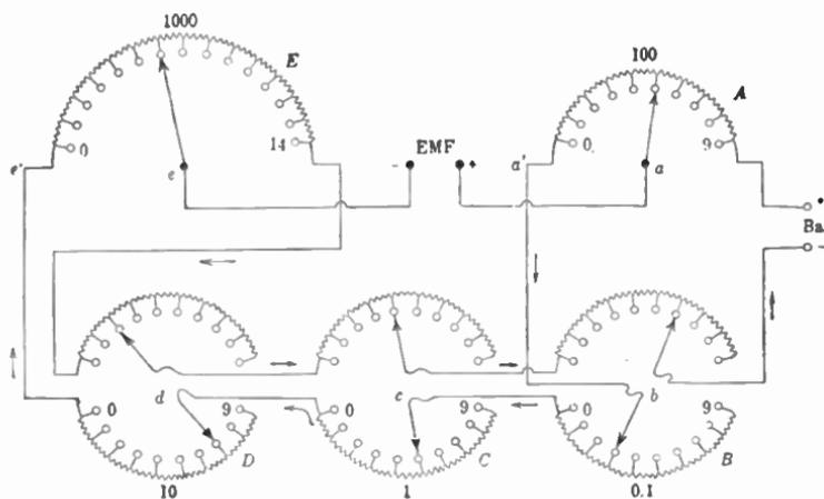
FIG. 121.—Principle of the Wolff potentiometer.
