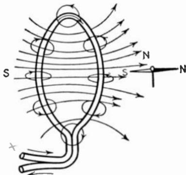
FIG. 166.—Magnetic field produced by a single turn.
