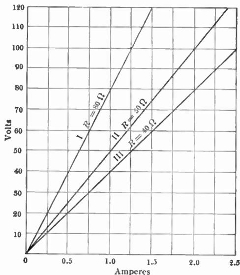
FIG. 295.—Field-resistance lines.
