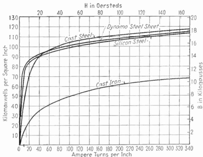
FIG. 190.—Typical magnetization curves for iron and steel.
