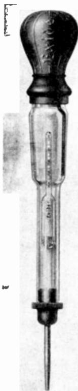
FIG. 70.—Syringe hydrometer.
