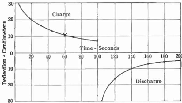
FIG. 115.—Charge and discharge curves of a cable.
