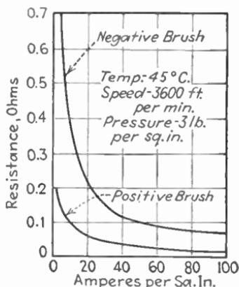
FIG. 318.—Contact-resistance characteristics of carbon brushes.
