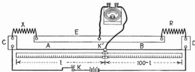
FIG. 109.—Slide-wire bridge.
