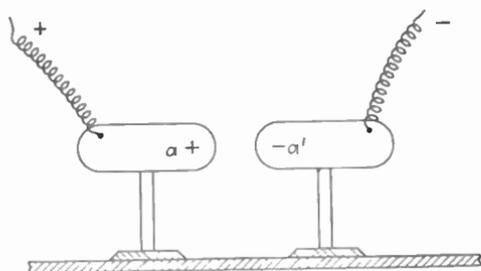
FIG. 221.—Electrostatic charges on insulated conducting bodies.
