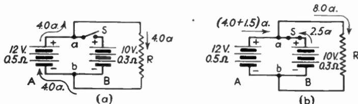
FIG. 38.—Unequal batteries in parallel—floating-battery method.
