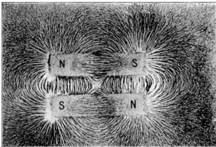
FIG. 141.—Magnetic figure, unlike poles adjacent.
