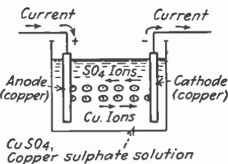
FIG. 82.—Electrolysis of copper in copper-sulphate solution.
