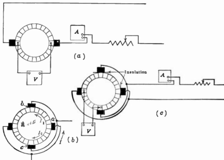
FIG. 405.—Measurement of armature resistance for temperature test.
