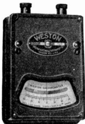
FIG. 94.—Weston portable galvanometer and microammeter.
