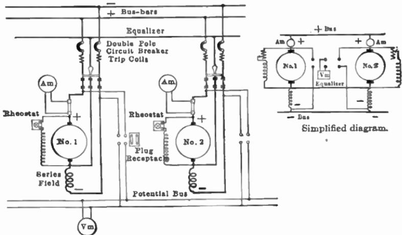
FIG. 410.—Typical connections for two compound generators operating in parallel.
