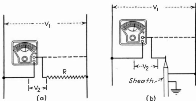
FIG. 103.—Measurement of resistance by the voltmeter method.
