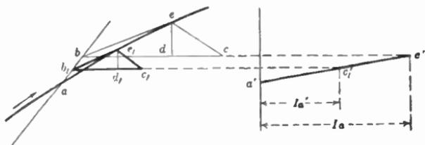
FIG. 341.—Compound characteristic and saturation curve.
