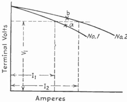
FIG. 406.—Characteristics of shunt generators in parallel.
