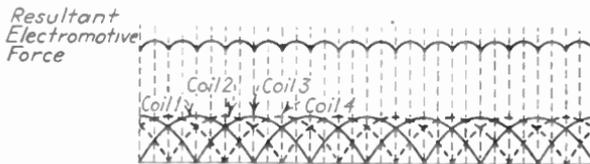
FIG. 254.—Resultant electromotive force due to four series-connected coils between brushes.
