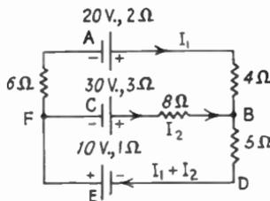
FIG. 44.—Procedure in network solution.
