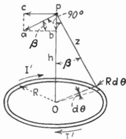
FIG. 167.—Field intensity due to a single turn.
