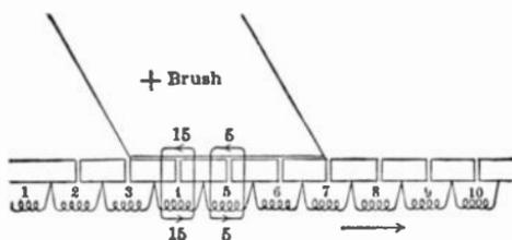
FIG. 312.—Short-circuit currents through brush.
