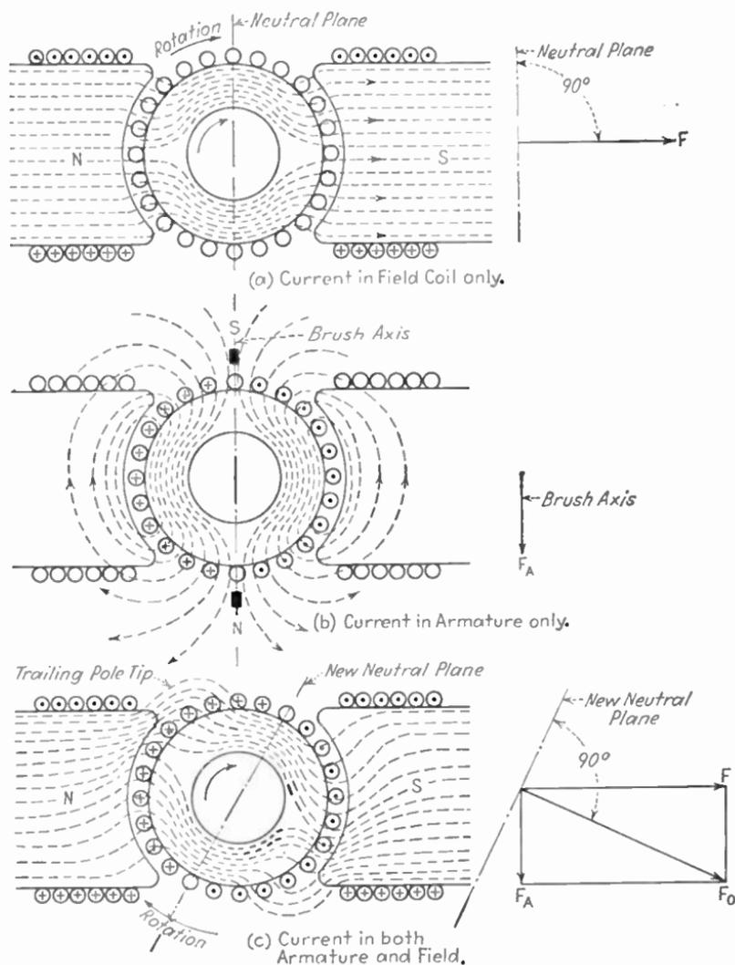
FIG. 299.—Effect of armature reaction on field of generator.
