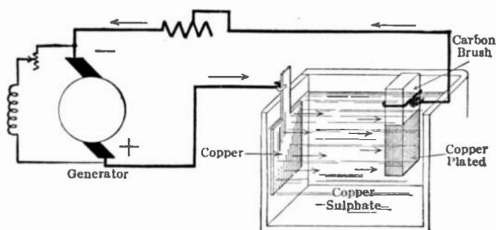
FIG. 83.—Copper-plating bath.
