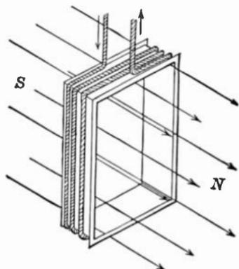
FIG. 85.—Magnetic field produced by an instrument coil.
