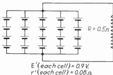
FIG. 36.—Series-parallel grouping of where  $r'$  is the resistance of one cell.
