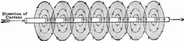
FIG. 157.—Magnetic field about a straight conductor.
