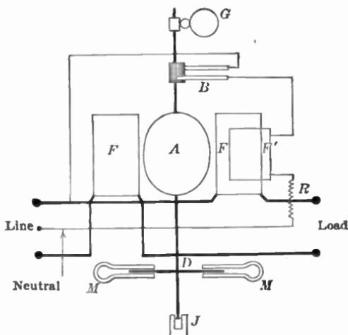
FIG. 130.—Diagram of a 3-wire watthour meter.
