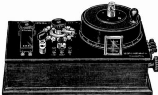
FIG. 119.—Leeds and Northrup potentiometer without accessories.
