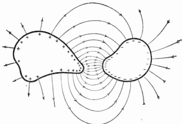
FIG. 224.—Electrostatic field between charged electrodes.
