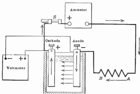
FIG. 52.—Current flow in a single cell.
