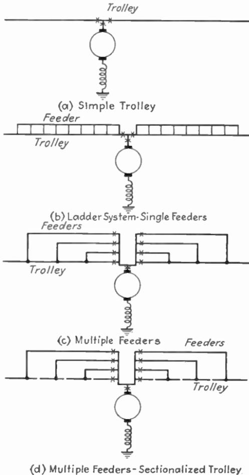
FIG. 430.—Methods of feeding a trolley system.
