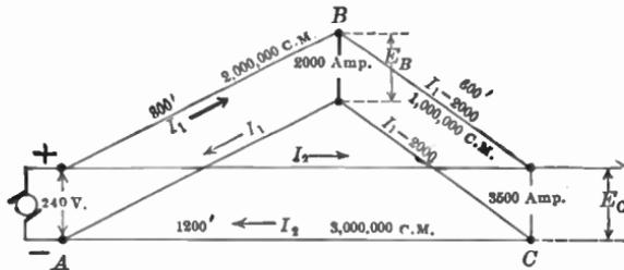
FIG. 48.—Ring-feeder system.
