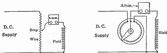
FIG. 294.—Drop-wire connections for obtaining field current.
