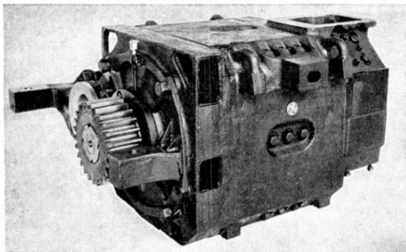
FIG. 371.—Railway motor, three-quarter view commutator end, axle side. (General Electric Company.)
