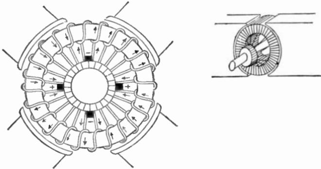
FIG. 253.—Gramme-ring winding.
