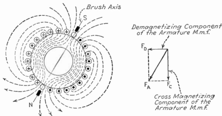
FIG. 300.—Relation of armature field to brush axis.
