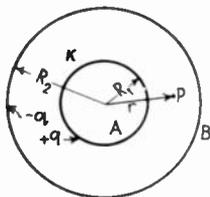
FIG. 237.—Concentric spherical condenser.
