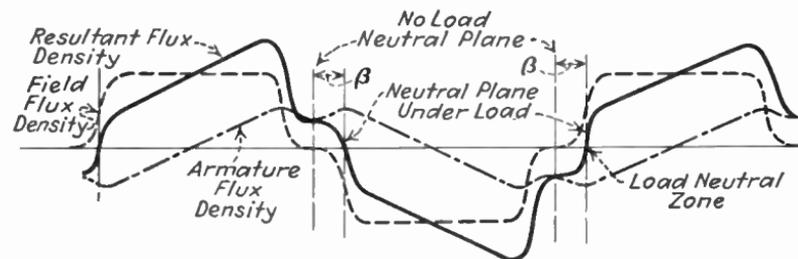
FIG. 305.—Resultant flux density found by combining field flux density (Fig. 303) and armature flux density (Fig. 304).
