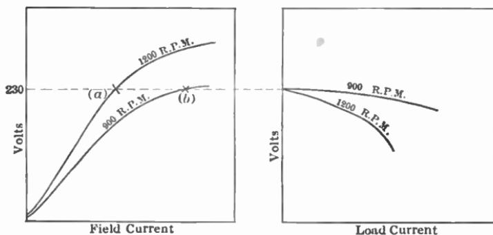
FIG. 330.—Relation of shunt characteristics to speed.
