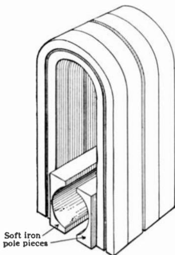
FIG. 153.—Compound horseshoe magnet used in magnetos.
