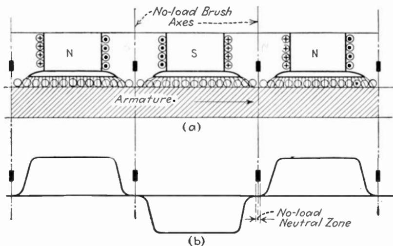
FIG. 303.—Field flux density in a multipolar generator.
