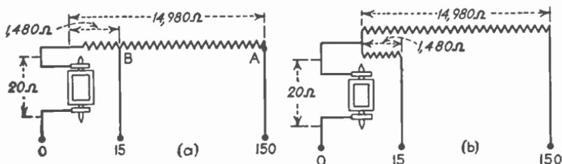
FIG. 98.—Methods of connecting a voltmeter resistance.
