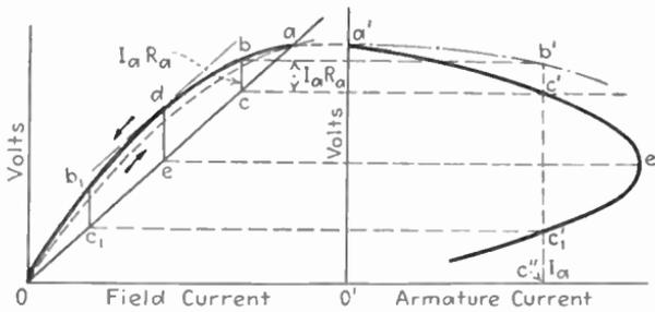
FIG. 332.—Relation of shunt characteristic to saturation curve—no armature reaction.
