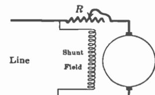
FIG. 373.—Resistance used for starting purposes.
