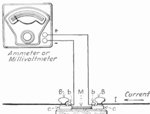
FIG. 95.—Ammeter with an external shunt.
