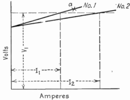
FIG. 409.—Characteristics of compound generators in parallel.
