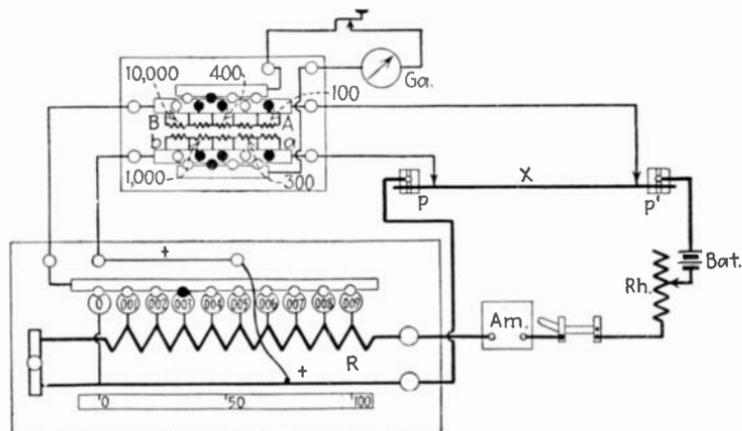
FIG. 111.—Actual connection of Kelvin bridge. (Leeds and Northrup type.)
