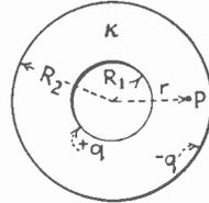
FIG. 236.—Concentric cylindrical condenser.
