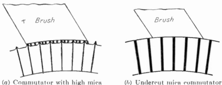
(a) Commutator with high mica (b) Undercut mica commutator
