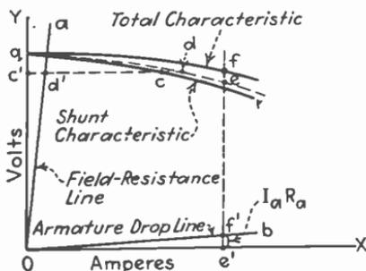
FIG. 331.—Total characteristic of shunt generator.
