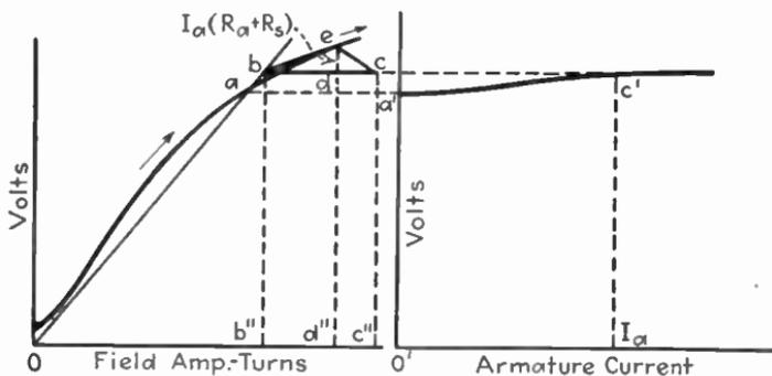
FIG. 340.—Relation of compound characteristic to saturation curve.
