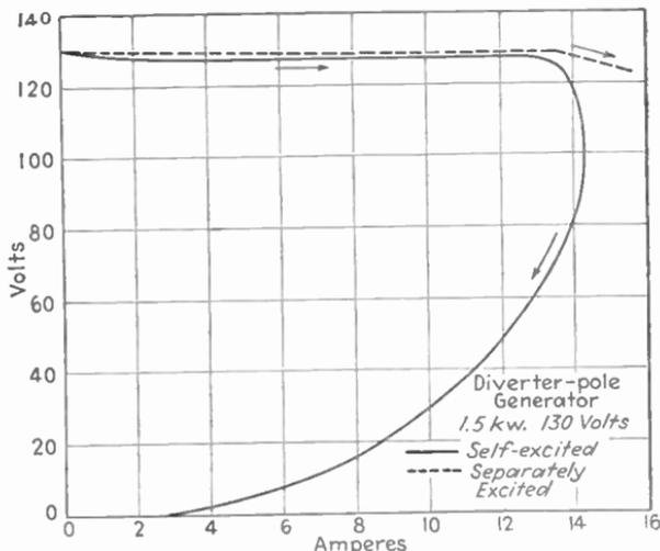
FIG. 352.—Load characteristic of diverter-pole generator.
