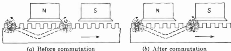
FIG. 316.—Change of flux through coil undergoing commutation.
