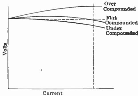
FIG. 336.—Compound-generator characteristics.
