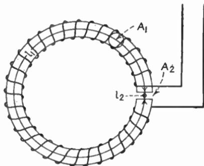
$$\begin{aligned} l_1 &= 18 \text{ in.} = 45.7 \text{ cm.} \\ A_1 &= A_2 = 0.2 \text{ sq. in.} = 1.29 \text{ sq. cm.} \\ l_2 &= \frac{3}{16} \text{ in.} = 0.476 \text{ cm.} \end{aligned}$$
