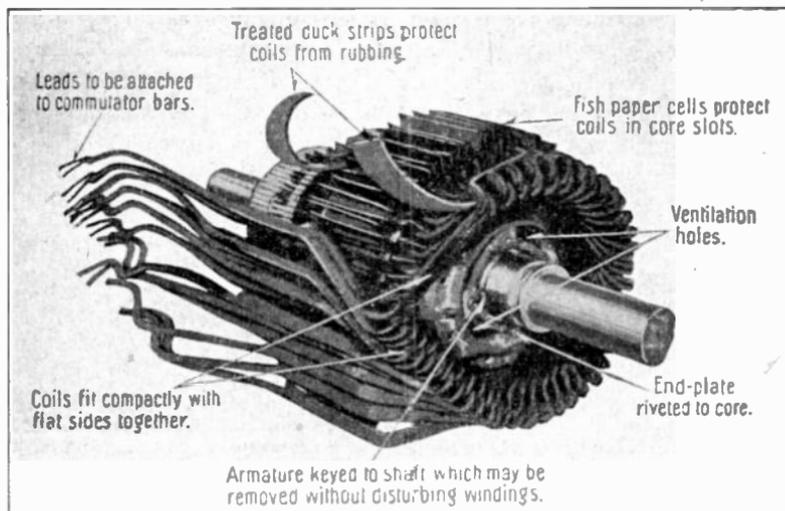
FIG. 276.—Partly wound armature showing method of assembling coils. (*Westinghouse.*)
