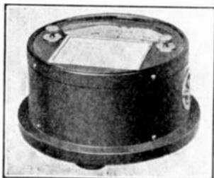
FIG. 203.—Koepsel permeameter.
