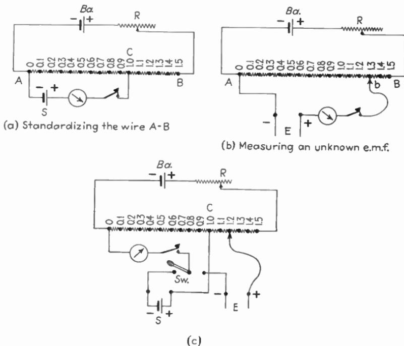
FIG. 117.—Simple potentiometer.
