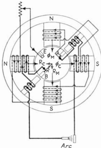
FIG. 354.—Arc-welding generator.
