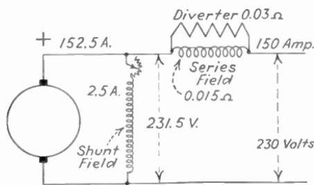
FIG. 338.—Series-field diverter.
