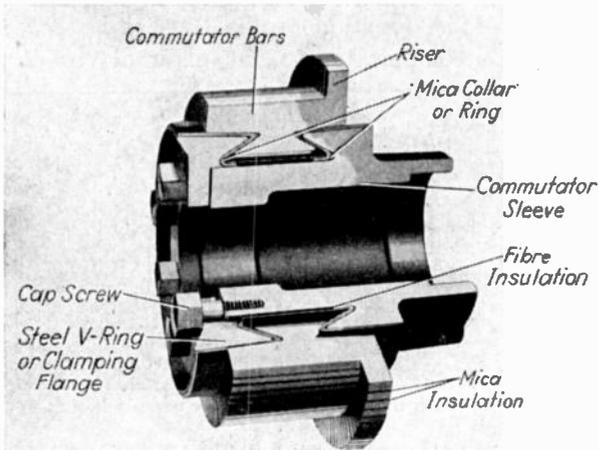
FIG. 286.—Commutator construction. (*Reliance Electric and Engineering Company.*)
