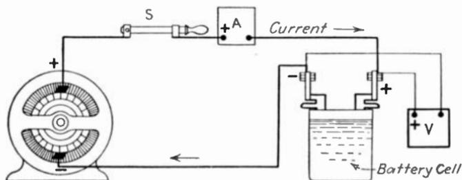
FIG. 33.—Generator charging a battery.
