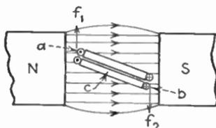
FIG. 84.—Turning forces of a coil carrying current.
