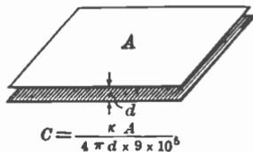
FIG. 233.—Capacitance of a plate condenser.
