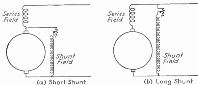
FIG. 335.—Compound-generator connections.
