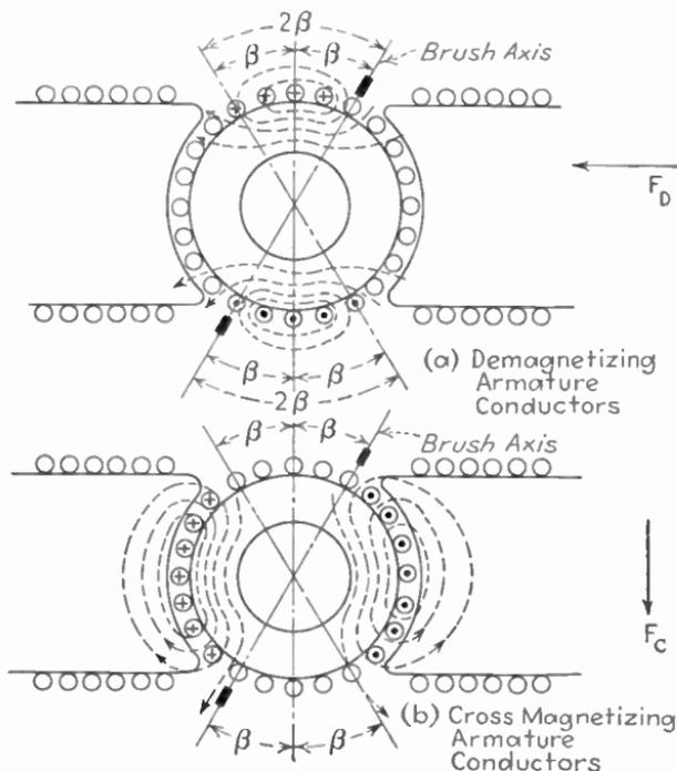
FIG. 301.—Demagnetizing and cross-magnetizing components of armature reaction.
