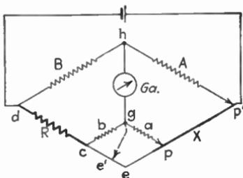
FIG. 110.—Wiring diagram of the Kelvin double bridge.
