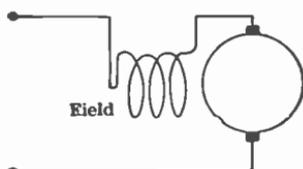
FIG. 368.—Connections of a series motor.
