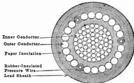
FIG. 428.—Cross-section of a 220-volt, 1,000,000-cir.-mil concentric cable.
