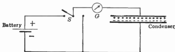
FIG. 227.—Charging and discharging a condenser.
