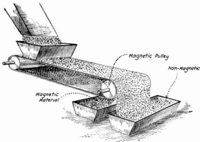
FIG. 178.—Magnetic separator.
