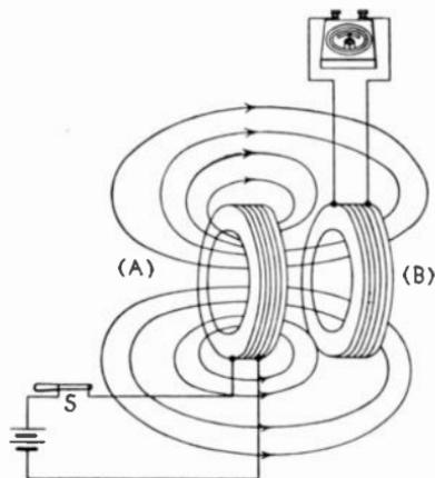
FIG. 215.—Mutual inductance between two coils.
