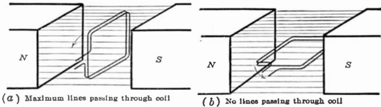
FIG. 246.—Simple coil rotating in a magnetic field.
