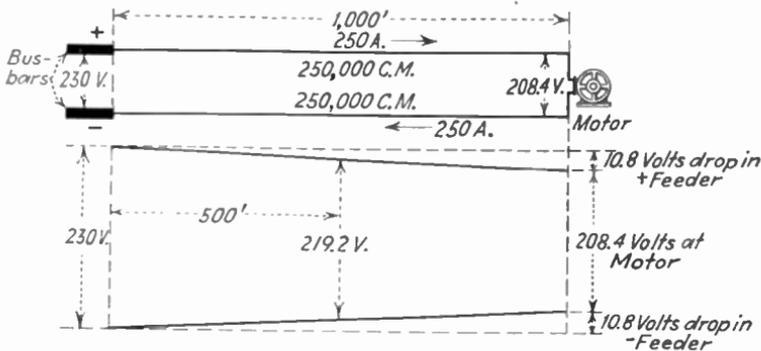
FIG. 28.—Voltage drop in a feeder due to a single load.
