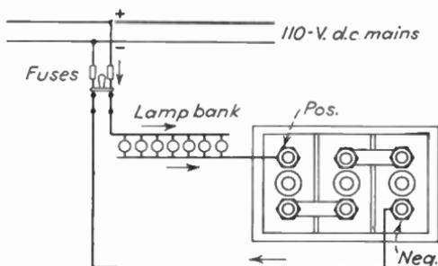
FIG. 74.—Charging a starting battery from 110-volt mains.
