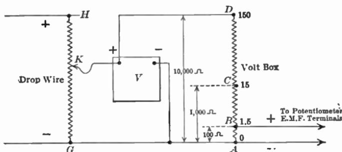
FIG. 122.—Volt-box and drop-wire connections.
