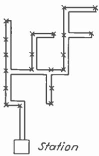
FIG. 437.—Parallel-loop series circuit.
