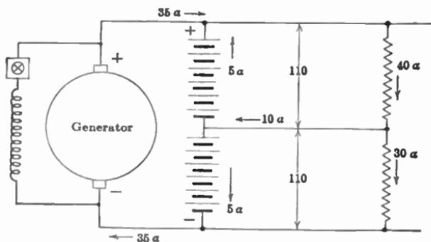
FIG. 423.—Storage battery giving neutral in a three-wire system.
