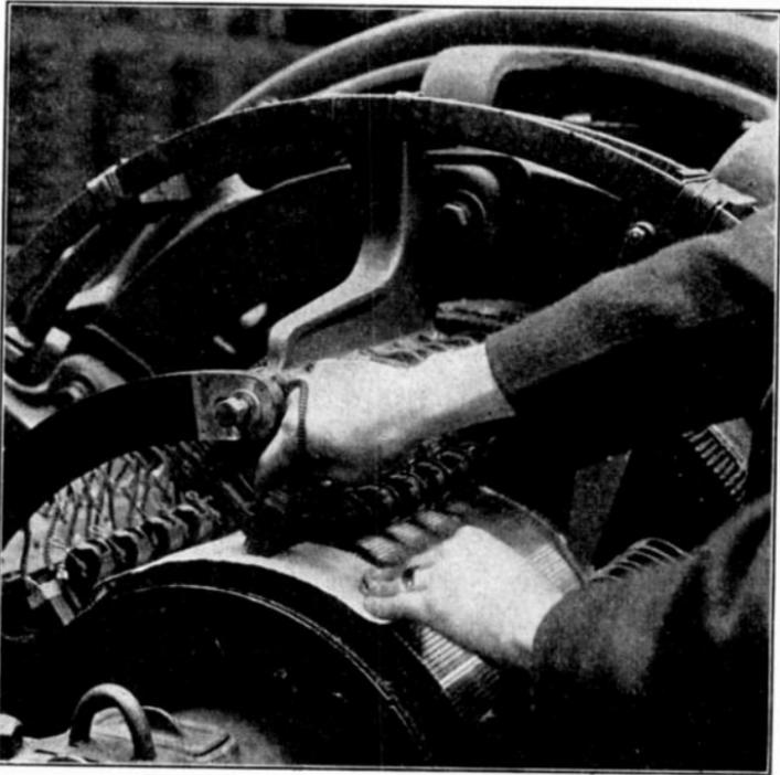
FIG. 320.—Proper method of fitting brushes.
