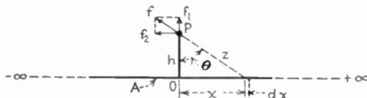
FIG. 235.—Force due charged filament of infinite length.
