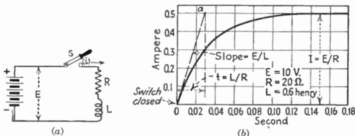
FIG. 209.—Rise of current in an inductive circuit.
