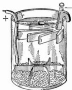
FIG. 56.—Gravity cell.
