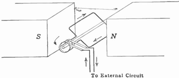
FIG. 250.—Current taken from rotating coil by means of slip-rings.
