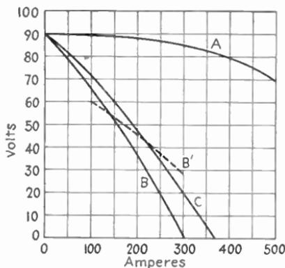
FIG. 353.—Operating characteristics of shunt and arc-welding generators. *A*. Conventional shunt generator. *B*. Steady-state characteristic of welding generator. *B'*. Dynamic or transient characteristic of welding generator. *C*. Steady-state characteristic of welding generator with larger values of current.
