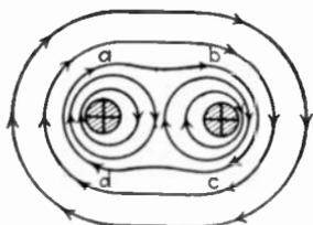
FIG. 162.—Magnetic field about two parallel conductors—current in same direction.
