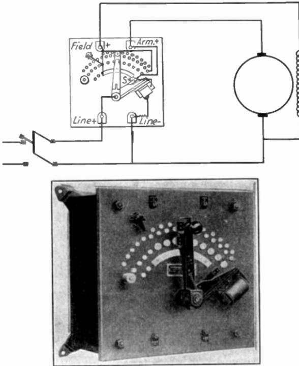
FIG. 376.—Westinghouse starting and speed-adjusting rheostat.
