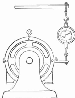
FIG. 398.—Cradle dynamometer.
