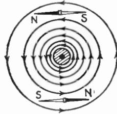
FIG. 159.—Lines of flux surrounding a cylindrical conductor—current outwards.
