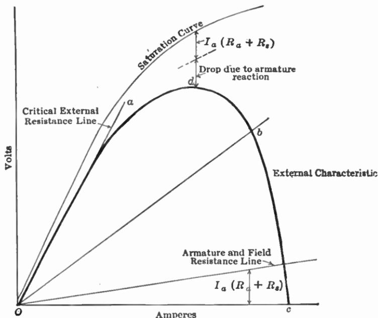
FIG. 345.—Series-generator characteristic.
