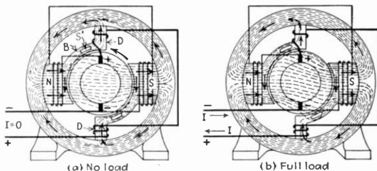
FIG. 351.—Magnetic flux distribution in diverter-pole generator.
