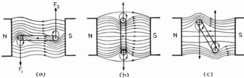
FIG. 360.—Torque developed at different positions of a coil.
