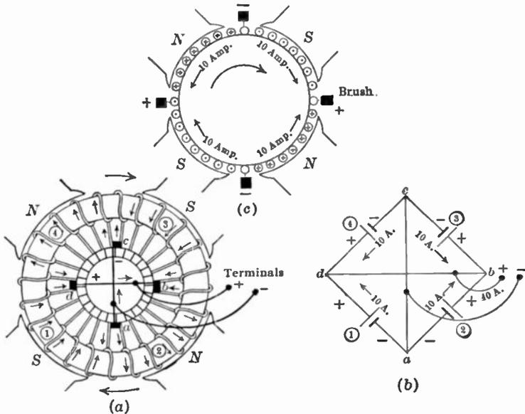
FIG. 262.—Four paths in parallel through an armature.
