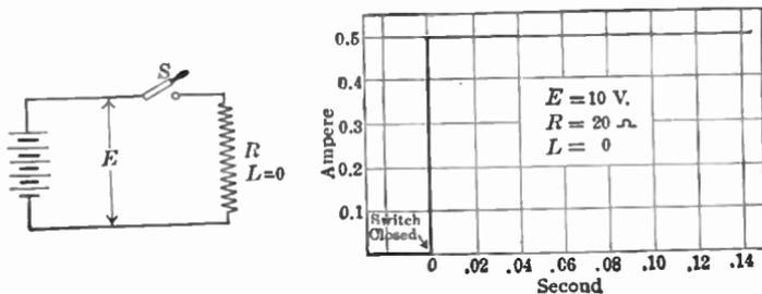
FIG. 207.—Rise of current in a non-inductive circuit.
