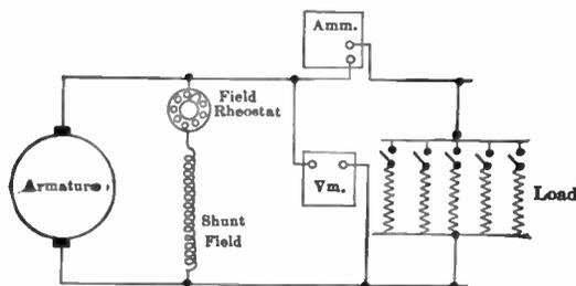
FIG. 296.—Shunt-generator connections.
