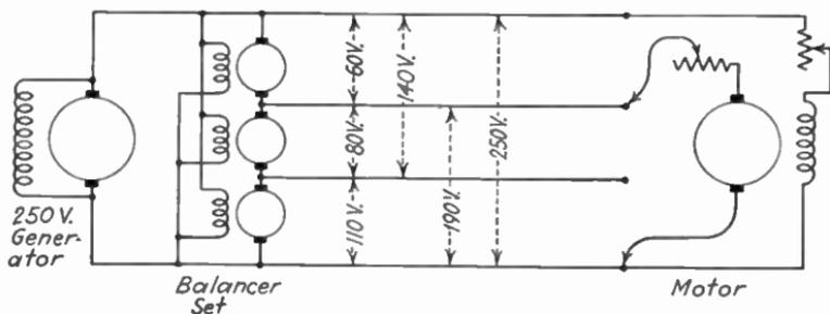
FIG. 382.—Multivoltage speed control.
