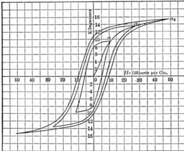
FIG. 194.—Hysteresis loops for three maximum flux densities.
