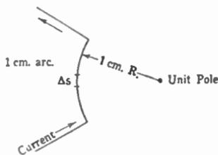
FIG. 12.—Absolute determination of current.
