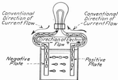
FIG. 1.—Electron movement and conventional current flow.
