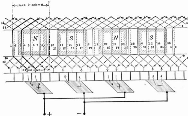
FIG. 259.—Development of a four-pole lap winding.
