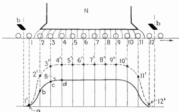
FIG. 288.—E.m.f. induced in conductors between brushes.
