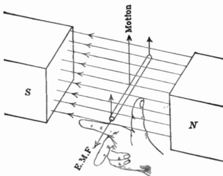
Forefinger along lines of force. Thumb in direction of motion. Middle finger gives direction of induced e.m.f.
