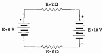
FIG. 20.—Current with two e.m.fs. and two resistances.<sup>1</sup>
