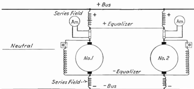
FIG. 411.—Compound generators requiring two equalizers (neutral connection to generators omitted).
