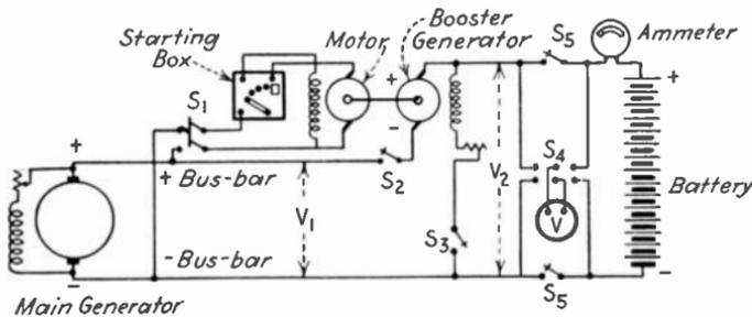
FIG. 75.—Booster method of charging a storage battery.
