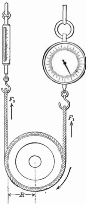
FIG. 391.—Rope brake.
