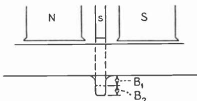
FIG. 322.—Flux density produced by commutating pole alone.
