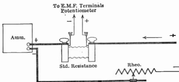
FIG. 123.—Calibration of an ammeter with a potentiometer.
