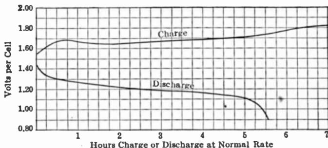
FIG. 80.—Voltage changes during the charge and discharge of an Edison cell during charge with constant current flowing. The state of charge can be approximated at any time by use of an ampere-hour meter or by a charge test fork which indicates from a pilot cell the voltage delivered at a given rate of discharge.
