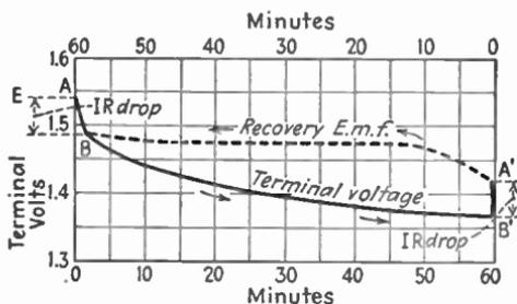
FIG. 54.—Discharge and recovery characteristics of a dry cell.
