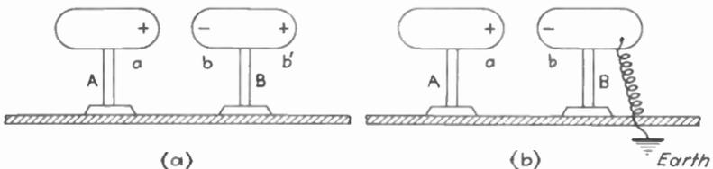
FIG. 222.—Electrostatic induction.
