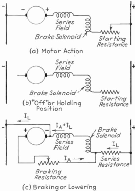
FIG. 387.—Dynamic braking.
