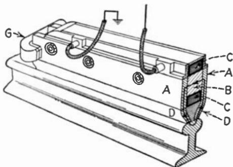
FIG. 179.—Magnetic track brake.
