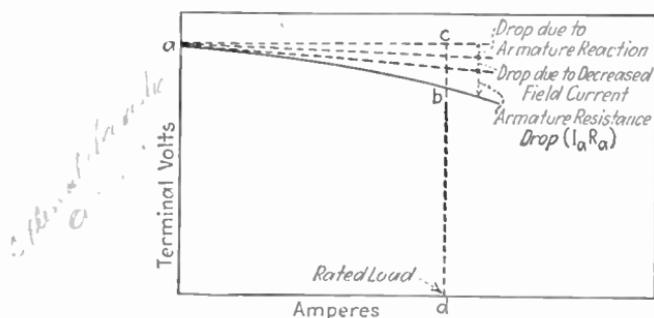
FIG. 329.—Voltage drops in shunt generator.
