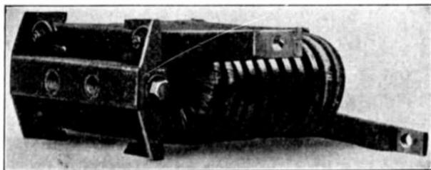
FIG. 325.—Commutating pole and winding.
