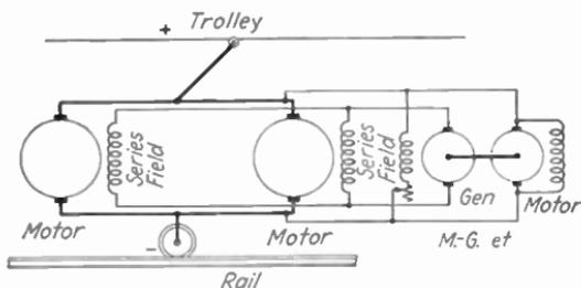
FIG. 388.—Series railroad motors connected for regenerative braking.
