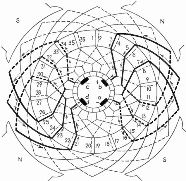
FIG. 263.—Heavy lines show two of the four parallel paths of lap winding.
