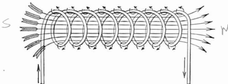
FIG. 168.—Magnetic field produced by a helix or solenoid.
