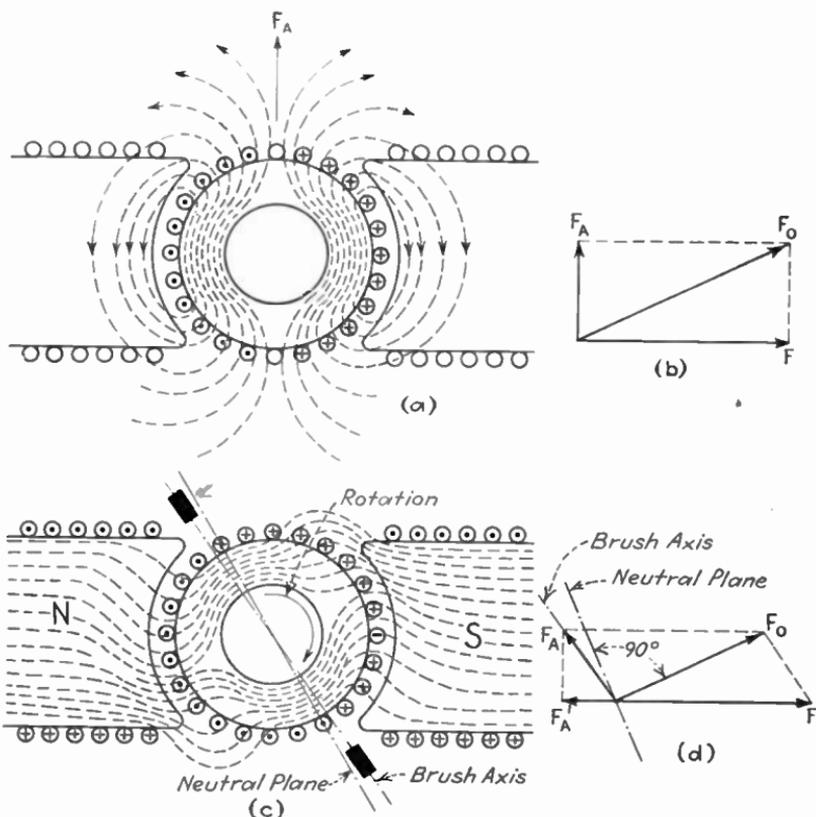
FIG. 364.—Armature reaction in a motor.
