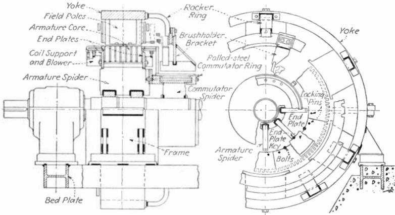
FIG. 280.—A typical, fabricated d.-c. machine assembly. (Westinghouse.)
