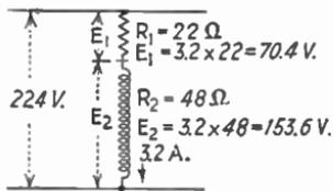
FIG. 21.—Voltage drops across a generator field and its rheostat.
