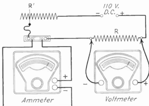
FIG. 101.—Voltmeter-ammeter method of measuring resistance.
