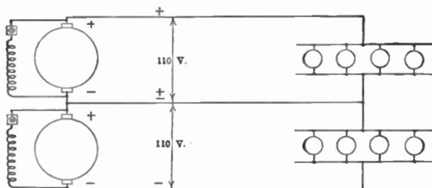
FIG. 422.—Two generators supplying a three-wire system.
