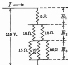
FIG. 26.—Series-parallel circuit.
