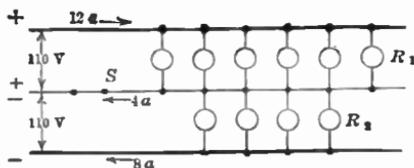
FIG. 419.—Effect on the balance of three-wire system of opening the neutral.
