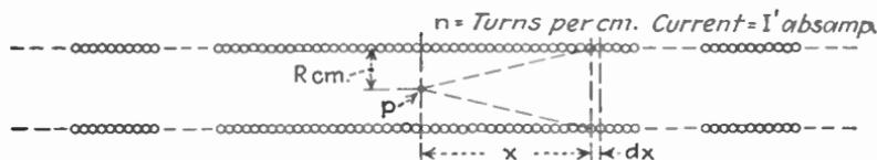
FIG. 170.—Field intensity at center of long solenoid.
