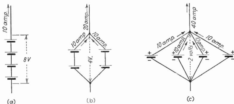
FIG. 261.—Series, series-parallel, and parallel arrangement of batteries.
