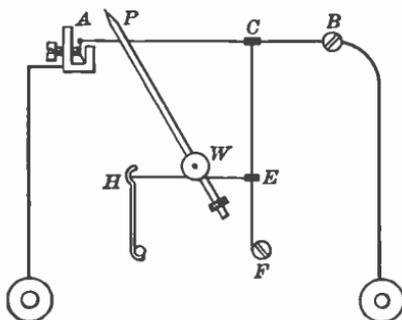
FIG. 99.—Principle of Hartmann and Braun hot-wire instruments.
