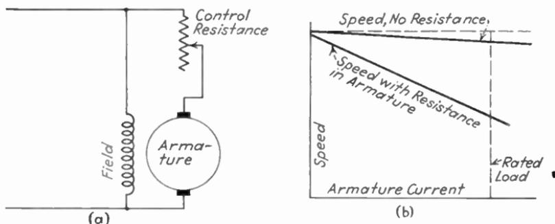
FIG. 381.—Speed control and regulation—armature-resistance method.
