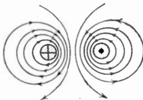
FIG. 163.—Magnetic field about two parallel conductors—current in opposite directions.
