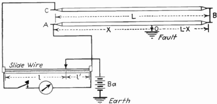
FIG. 112.—Murray-loop test.
