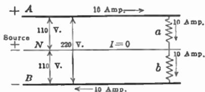
FIG. 417.—Edison three-wire system—balanced loads.
