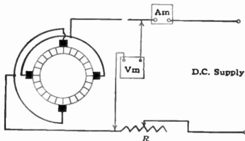
FIG. 394.—Measurement of armature resistance.
