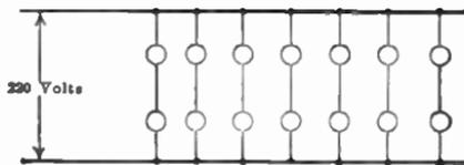
FIG. 416.—Series-parallel system.
