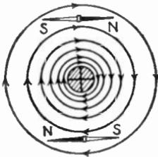
FIG. 158.—Lines of flux surrounding a cylindrical conductor—current inwards.
