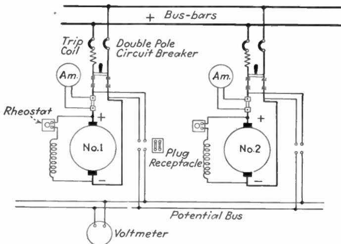
FIG. 407.—Connections for parallel operation of shunt generators.
