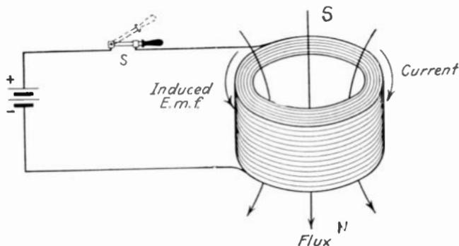
FIG. 206.—Relation of e.m.f. of self-induction to current.
