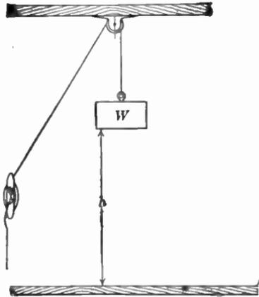
Fig. 211.—Energy of a suspended weight.
