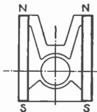
FIG. 150.—Application of straight-bar cobalt-steel magnets to measuring instrument.
