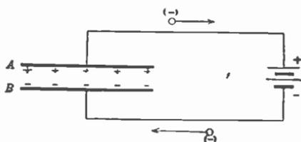
FIG. 220.—Transfer of electrons in condenser plates.
