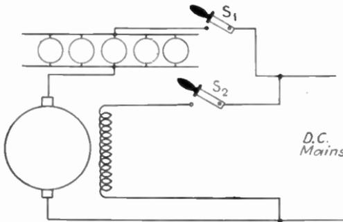
FIG. 363.—Demonstration of counter electromotive force.
