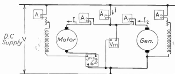
FIG. 403.—Kapp opposition method for determining losses.
