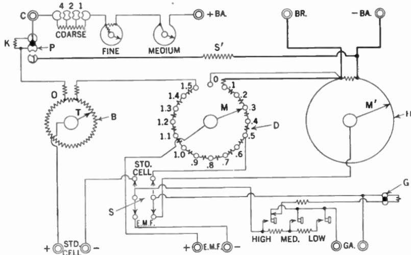
FIG. 118.—Connections of Leads and Northrup low-resistance potentiometer.
