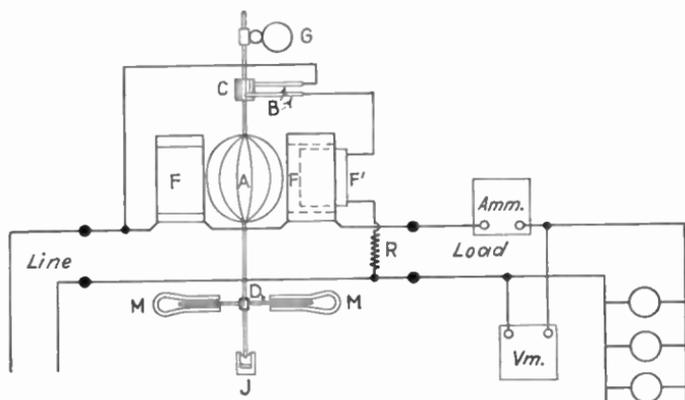
FIG. 128.—Connections of watthour meter.
