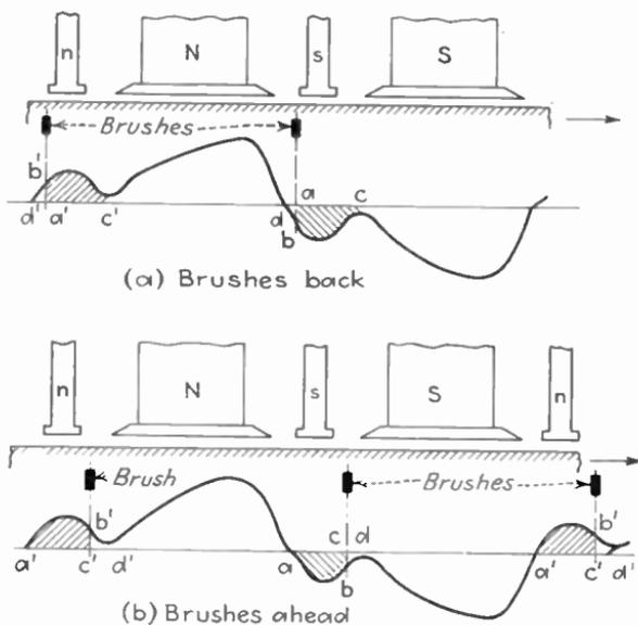
FIG. 344.—Compounding effect of interpoles.
