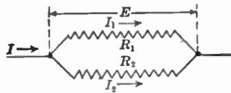
FIG. 24.—Division of current in a two-branch parallel circuit.
