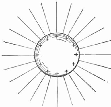
FIG. 225.—Isolated charged sphere.
