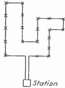
FIG. 436.—Open-loop series circuit.
