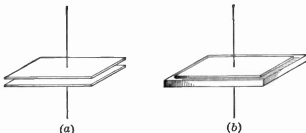
FIG. 229.—Plate condenser having air and then glass as a dielectric.
