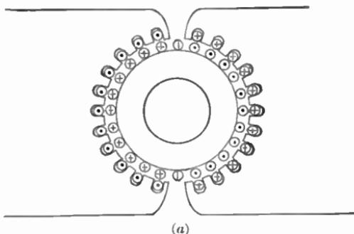
FIG. 309.—Compensation of armature reaction with pole-face conductors.
