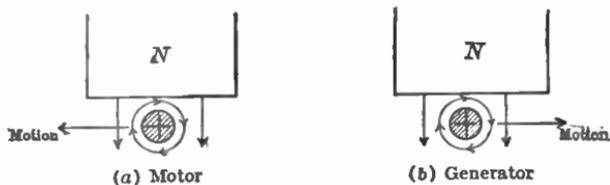
FIG. 357.—Motor and generator action.
