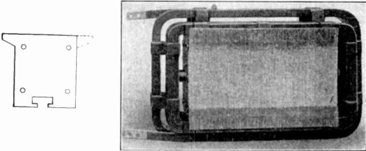
FIG. 282.—Field core lamination, and pole piece assembled. (*Westinghouse.*)
