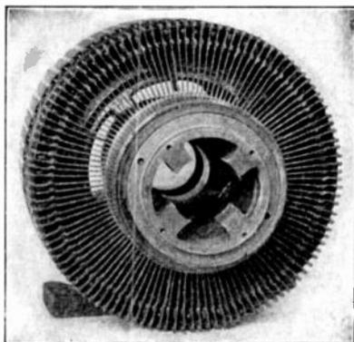
(b) End view of an armature showing spider and commutator. (Westinghouse.)
