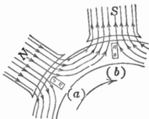
FIG. 396.—Reversal of magnetic flux in armature iron.
