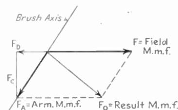
FIG. 302.—Resultant of armature and field m.m.fs.
