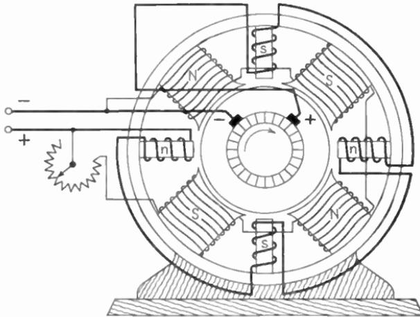
FIG. 324.—Connections of shunt field and commutating poles.
