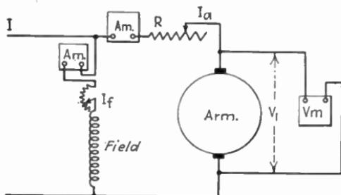
FIG. 400.—Connections for stray-power measurement.
