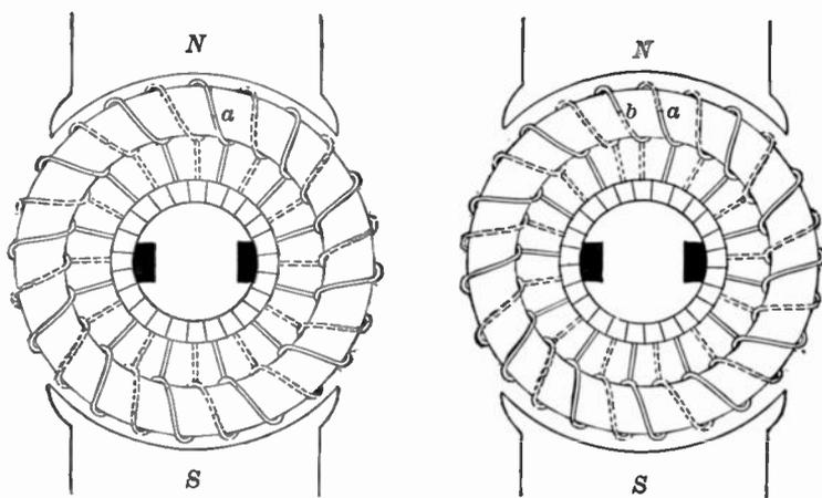
(a) Duplex doubly reentrant gramme-ring winding. (b) Duplex singly reentrant gramme-ring winding.
