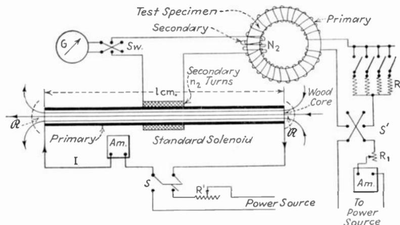
FIG. 199.—Standard solenoid with ring sample and galvanometer.
