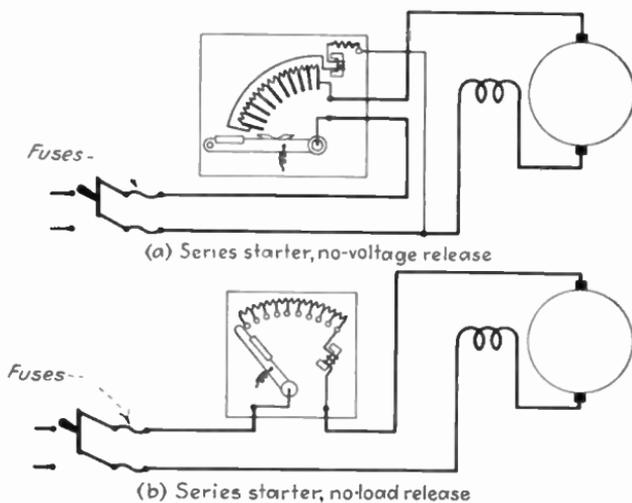
FIG. 377.—Series-motor starters.
