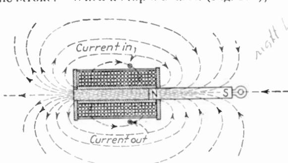
FIG. 171.—Simple solenoid and plunger.
