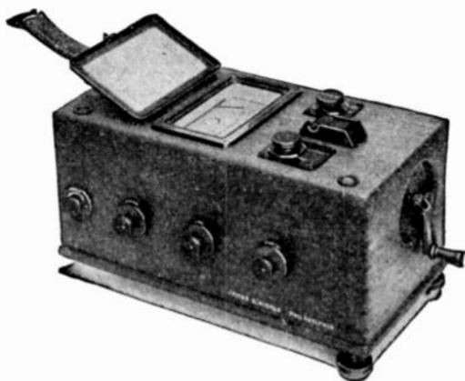
FIG. 105.—Standard high-range megger testing set.
