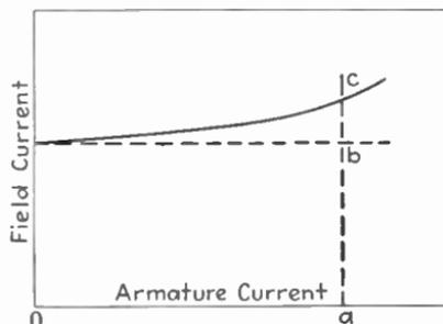
FIG. 343.—Armature characteristic.
