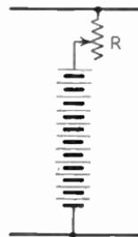
FIG. 433.—Resistance control of battery discharge.
