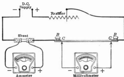
Fig. 102.—Measuring the resistance of a metal rod.
