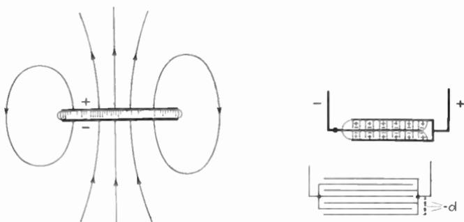
(a) Electrostatic leakage lines of a plate condenser.
