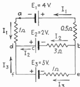
FIG. 45.—Assumed direction of current.
