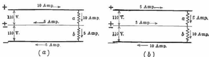
FIG. 418.—Unbalanced three-wire systems.
