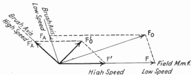
FIG. 384.—Effect of weak field on brush position.
