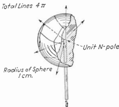
FIG. 138.—Lines of force leaving a unit N-pole.
