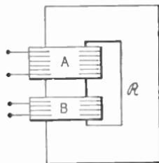
FIG. 217.—Self- and mutual-inductance coils on iron core.
