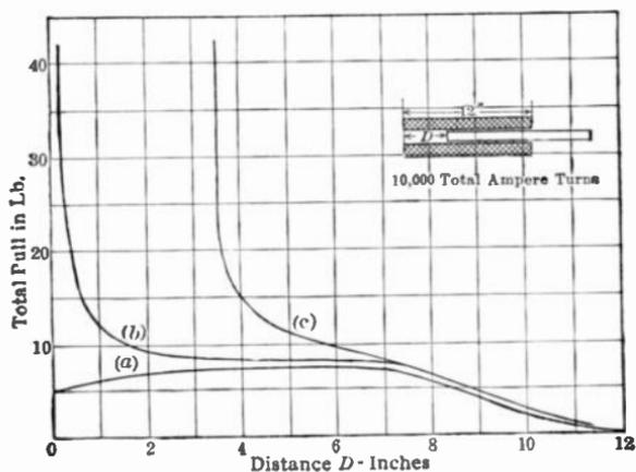
FIG. 173.—Pull of solenoid on plunger.
