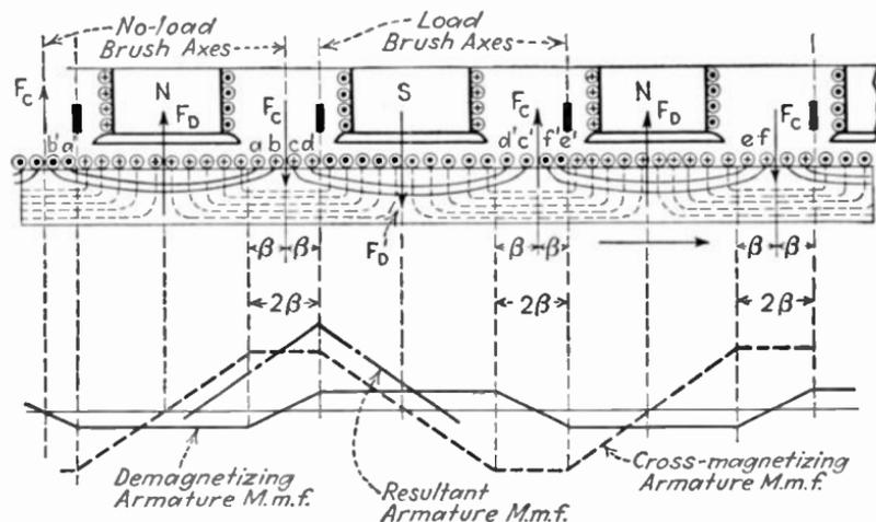
FIG. 307.—Cross and demagnetizing ampere-turns in multipolar generator.
