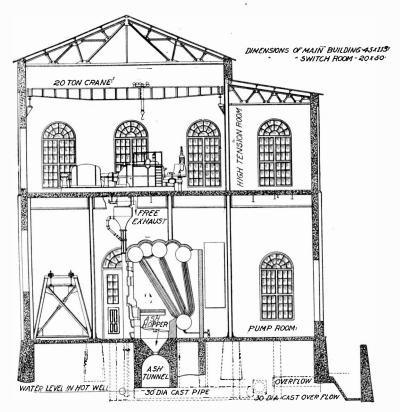
Fig. 53. Double-Deck Turbine Plant
