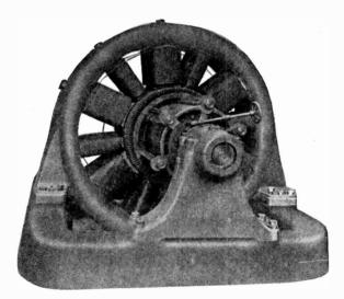
Fig. 42. Regulating-Pole Rotary Converter
