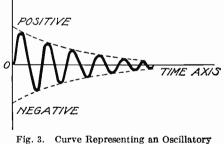
Fig. 3. Curve Representing an Oscillatory Discharge
