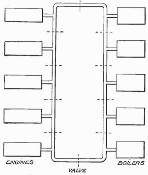
Fig. 2. Diagram of Ring System of Piping
