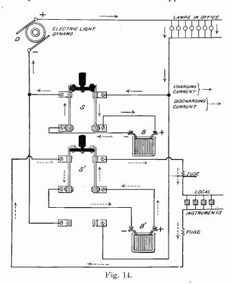
In Fig. 14 is shown a storage cell system fed by a dynamo which is also the source of energy for an electric-light plant. There are two storage cells, one of which, B Fig. 14, is in the same circuit with, and receives the current in the same manner as, the lamps. The other cell, B', is disconnected for the time being from the dynamo, and is represented as supplying the current for a number of sounders arranged in multiple on the lower right. It
