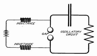
Fig. 34. Thomson Direct-Current Method of Genera ing Oscillations
