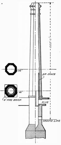
Fig. 7. Good Design of Brick Chimney
