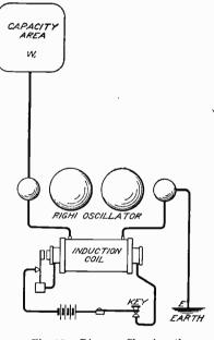
Fig. 15. Diagram Showing the Earthed Oscillator
