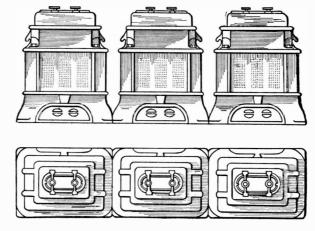
Fig. 18. Three-Phase Air-Blast Transformers. Total Capacity, 3,000 Kw.
