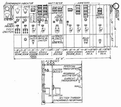
Fig. 25. Standard Switchboard Panel
