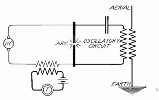
Fig. 8. Transmitter Associated with the Supply Circuit
