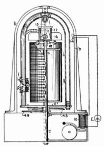
Fig. 7. Telephone Message Recorder.
