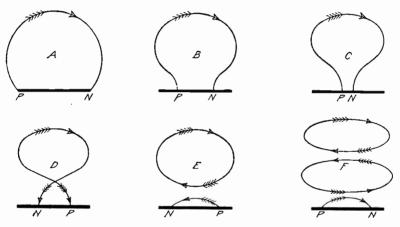
Fig. 5. Formation of Closed Loops of Electric Strain
