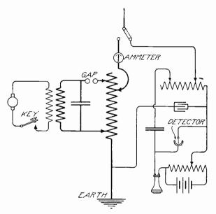
Fig. 66. Massie Sending and Receiving Circuits
