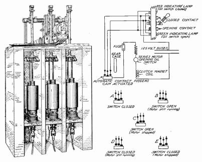
Fig. 29. Form of Oil Switch for High Potentials
