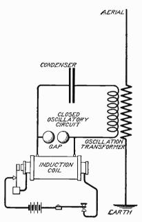
Fig 20. Marconi-Braun Inductive Transmitting Antennae
