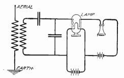
Fig. 49. Receiving Circuit with Audion Detector
