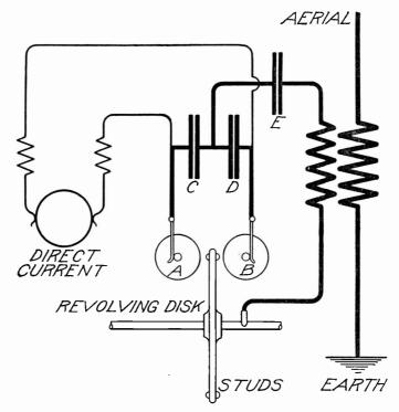
Fig. 33. Disk Discharger for Use with Direct Current
