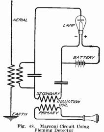
lamp. Instead of passing the rectified uni-directional impulses directly through the telephone, they are passed around the secondary of a large induction coil in series with a condenser, to the primary of which the telephone receiver is connected. Prof. Fleming is authority for the statement that this arrangement, when suitably adjusted, is "one of the best long-distance requivers for electric waves yet devised."
