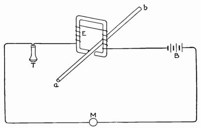
Fig. 1. Illustrating the Principle of the Telegraphone.
