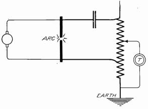
Fig. 11. Transmitter Shunted across a Portion of the Aërial Inductance
