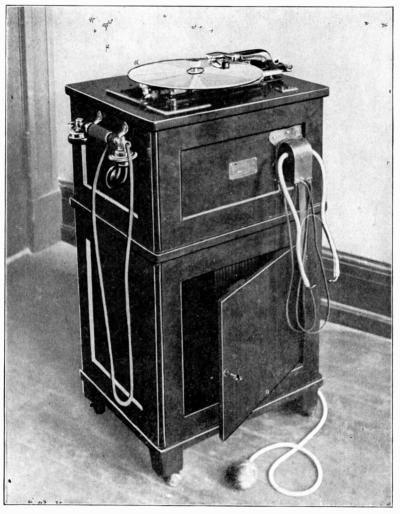
Fig. 4. Disc Type of Telegraphone, with Cabinet.
