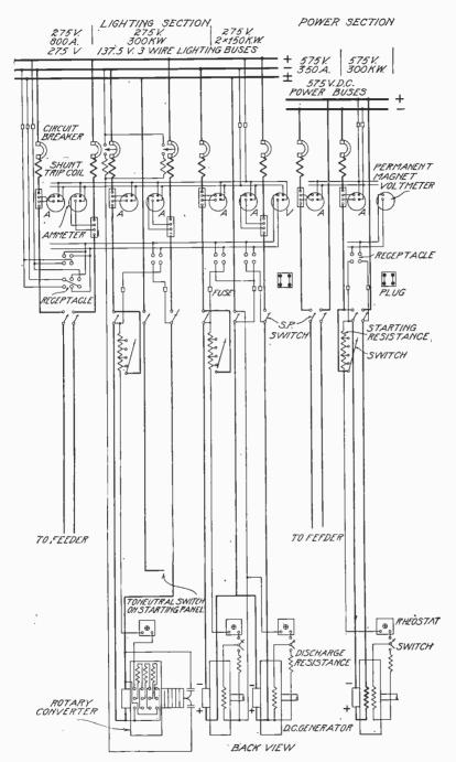
Fig. 39. Wiring Diagram for Standard Switchboard
