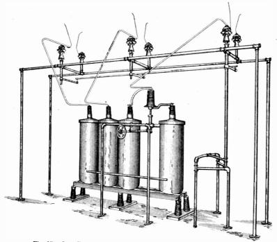
Fig. 37. Installation of Aluminum Lightning Arrester for 35,000 Volts
