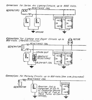
Fig. 32. Lightning-Arrester Diagrams of D. C. Work
