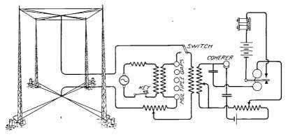
Fig. 63. Lodge-Muirhead Sending and Receiving Circuits
