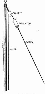
Fig. 41. Single Wire Experimental Aërial
