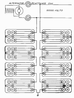
Fig. 33. Connections for 10,000-Volt\_Lightning Arrester
