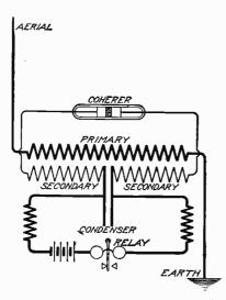
Fig. 19. Marconi Receiver-Circuit with Jigger
