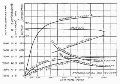
Fig. 13. Efficiency Curves of a 500-H. P. Gas Engine
