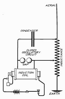
Fig. 21. "Direct-Coupled" Inductive Antennae
