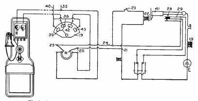
Fig. 8. Connections of the Telegraphone in a Telephone Circuit.
