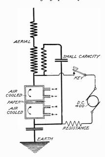
Fig. 61. Von Lepel Oscillation Generator Circuit
