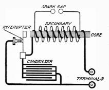
Fig. 23. Diagram of Induction Coil Showing Condenser Circuit
