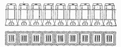
Fig. 19. Single-Phase Air-Blast Transformers. Total Capacity, 3,000 Kw.
