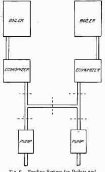
Fig. 6. Feeding System for Boilers and Pumps
