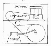
Fig. 49. Diagram of Double-Deck Arrangement of Machines
