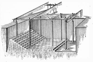
Fig. 44. Foundation for Machines Showing Use of Template and Iron Pipe for Holding Bolts
