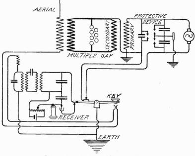
Fig. 65. Stone Sending and Receiving Circuits
