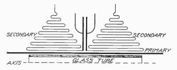
Fig. 18. Diagram of Oscillation Transformer Winding
