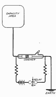
Fig. 16. Earthed Receiving Circuit
