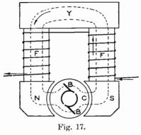
of dynamo. The arrows represent the lines of force between the magnetic poles; and, revolving therein, is shown a single conductor cutting the lines of force at right angles. Now comes the principle which underlies the generation of the electric current by means of the dynamo: If a closed conductor is rapidly revolved in a magnetic field an electric current is set up in the conductor. The collector rings and brushes conduct to the outside circuit the current thus generated.
