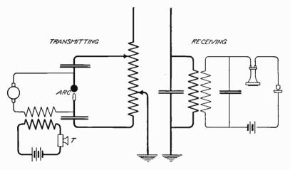
Fig. 17. Circuits of Poulsen System
