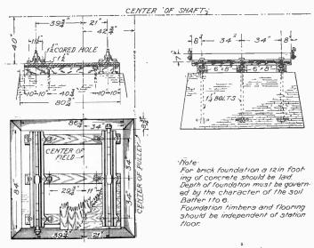
Fig. 45. Foundation for 150-Kw. Generator
