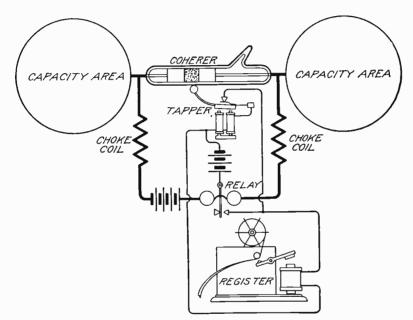
Fig. 13. Early Marconi Receiving Circuit
