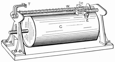
Fig. 2. Early Model of Telegraphone, Wire Type.
