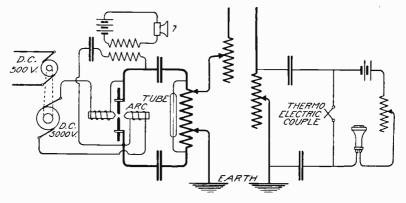
Fig. 20. Circuits of the Collins System
