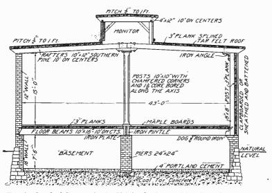
Fig. 43. Standard Construction for Lighting Station. Brick and Wood Construction
