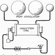
Fig. 12. Early Marconi Transmitter Circuit
