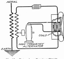
Fig. 13. Heterodyne Receiver Circuit
