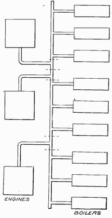
Fig. 5. Arrangement of Boilers and Engines in Very Large Plants
