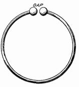
Fig. 6. Hertz Resonator
