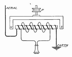
Fig. 51. Shoemaker Magnetic Detector
