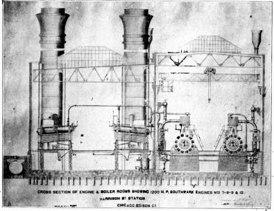
Fig. 7. Cross-Section of Engine and Boiler Rooms, Harrison Street Station.<sup>1</sup>
