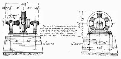
Fig. 46. Foundation for Rotary Converter
