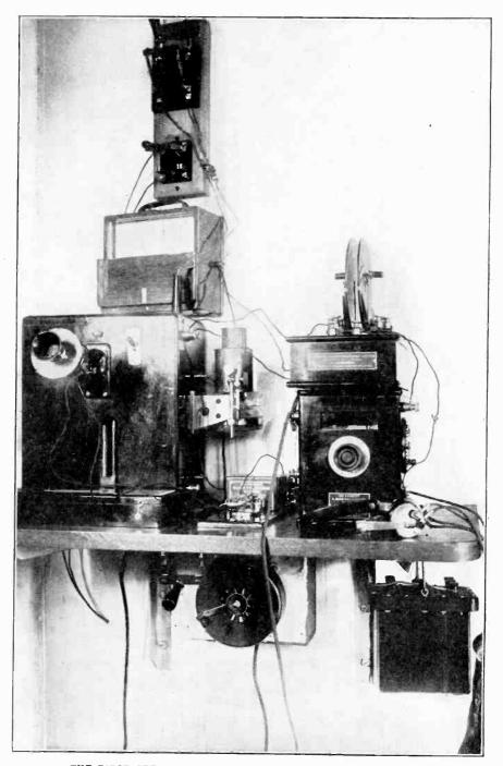
THE FIRST SET DF WIRELESS TELEPHONE INSTRUMENTS FOR THE UNITED STATES NAVY Installed on the Flagship "Connecticut." The "Audion" Receiver with Tuning Device on the Top at Right, the Transmitter on the Left.
