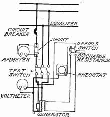
Fig. 21. Wiring Diagram of D. C. Generator Parel
