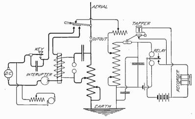
Fig. 60. Circuit Diagram, Telefunken System
