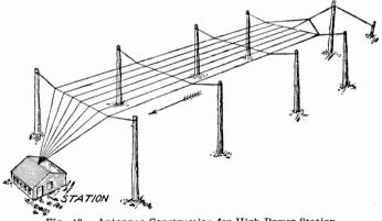
Fig. 42. Antennae Construction for High-Power Station
