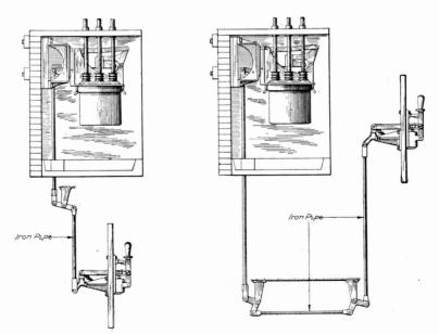
Fig. 28. Four Arrangements of Oil Switch when Mounted at Some Distance from the Panel
