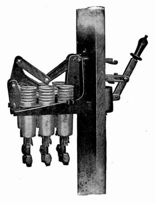
Fig. 26. Three-Phase Oil Switch with Oil Container Removed
