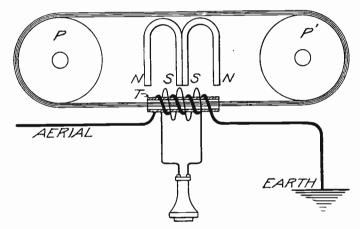
Fig. 50. Diagram of Marconi Magnetic Detector
