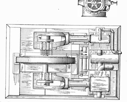
Fig. 54. Space Occupied by Turbo-Alternator Compared with that of Generator and Reciprocating Engine of Same Capacity
