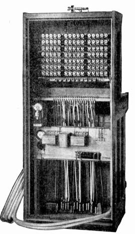
Fig. 148. Rear View of Target Signal, Magneto Switchboard
