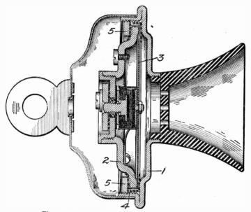
Fig. 44. Automatic Electric Company Transmitter
