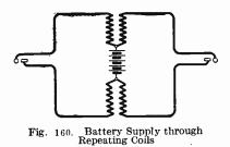
Stripped of all details, such as signals, ringing and listening keys, and operator's equipment, cord circuits of three different types are shown in Figs. 159, 160, and 161.
