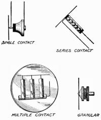
Fig. 9. General Types of Transmitters
