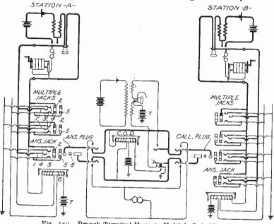
Fig. 180. Branch-Terminal Magneto Multiple Switchboard
