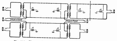
Fig. 226. Phantom from Two Physical Circuits of Unequal Length
