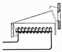
Fig. 23. Electromagnetic Visible Signal
