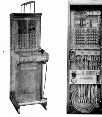
Fig. 142. Upright Magneto Switchboard
