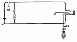
Fig. 156. Direct-Line Lamp with Ballast
