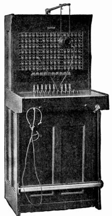
Fig. 147. Magneto Switchboard, Target Signals
