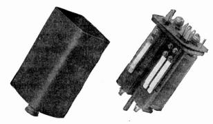
Fig. 208. Kellogg Line and Cut-off Relays
