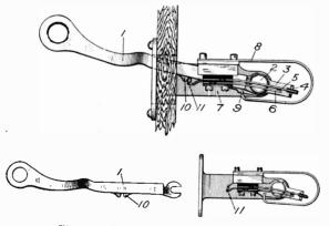
Fig. 77. Removable Lever Hook Switch
