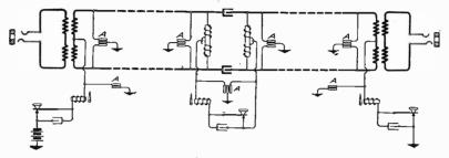
Fig. 232. Simplex Circuit with Waystation
