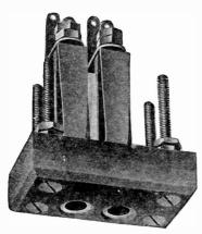
Fig. 119. Operator's Cut-In Jack
