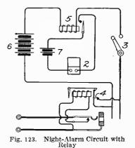
through the relay 5—assuming switch 3 to be closed—and thus cause the operation of the relay. The relay, in turn, by pulling up its armature, will close the circuit of the buzzer 2 through the battery 7 and cause the buzzer to sound.
