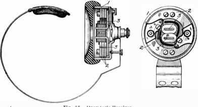
Fig. 57. Operator's Receiver
