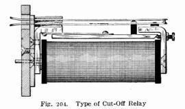
spring underneath two L-shaped polar extensions, one extending up from the rear end of the core and the other from the front end. When energized this armature is pulled away from the core by these L-shaped pieces and imparts its motion through a hard-rubber pin to the upper pair of springs so as to effect the necessary changes in the circuit.
