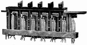
Fig 215. Western Electric Trunk Ringing Key
