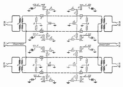
Fig. 235. Phantom of Two Composite Circuits
