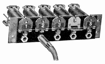
Fig. 101 Strip of Kellogg Drops and Jacks
