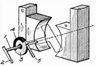
Fig. 69. Pulsating-Current Commutator
