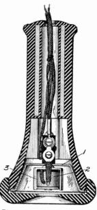
Fig. 52. Automatic Electric Company Direct-Current Receiver
