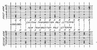
Fig. 229. Transposition of Phantom Circuits
