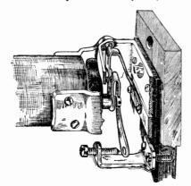
Fig. 108. Code Signal Attachment
