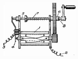
Fig 66. Generator Shunt Switch
