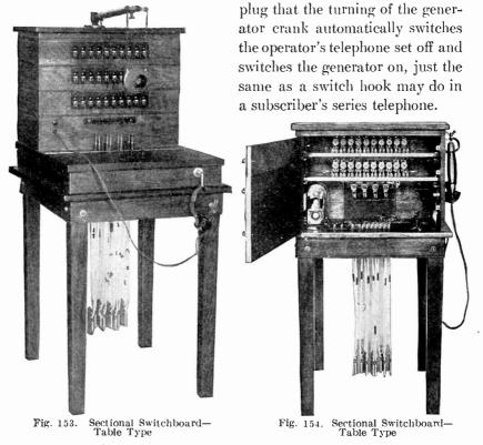
The upright type of sectional switchboard is shown in Figs. 153 and 154, which need no explanation in view of the foregoing, except to say that, in the particular instrument illustrated, ringing and listening keys are provided instead of the jack-and-plug arrangement of the wall type. In this case also, the top section carries an **arm** for supporting a swinging transmitter instead of the hook support for the combined transmitter and receiver.
