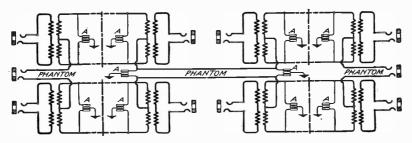
Fig. 228. Two Phantoms Joined by Physical Circuit
