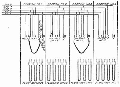
Fig. 178. Principle of Multiple Switchboard
