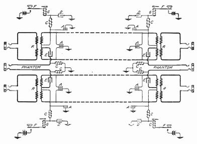
Fig. 234. Phantom of Two Simplex Circuits
