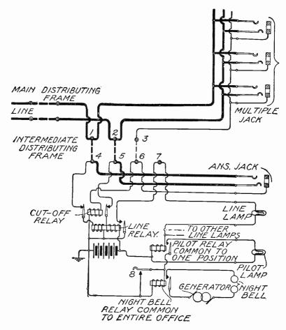
Fig. 190. Line Circuit No. 1 Board
