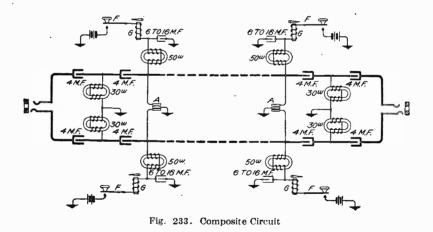
forms two Morse circuits, two wires carrying three services. Each Morse circuit will be seen to include, serially, two 50-ohm impedance coils, and to have shunts through condensers to ground. The 50-
