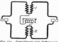
Fig. 134. Cord Circuit with Differential Windings
