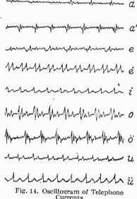
When a current is to be measured by the oscillograph, it is passed through the turn of wire in the magnetic field. While no current is passing, the wire does not move in the magnetic field and its mirror reflects a stationary beam of light. A photographic film moved in a direction normal to the axis of the turn of wire will have drawn
