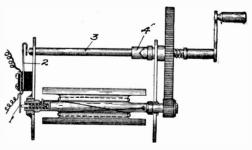
Fig. 67. Generator Cut-In Switch
