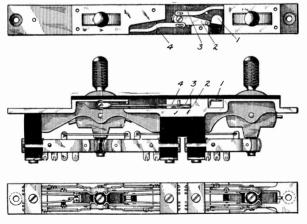
Fig. 114. Horizontal-Spring Listening and Ringing Key
