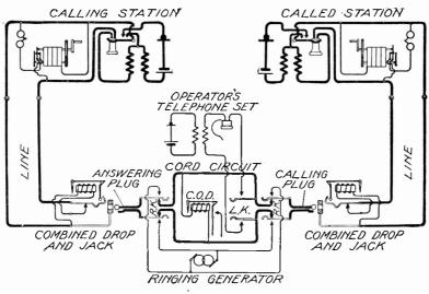
Fig. 121. Circuit of Simple Magneto Switchboard
