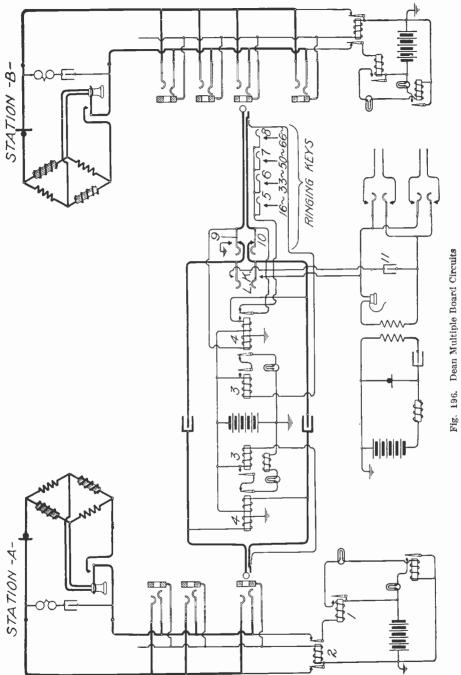
a connection is made with that line by a plug at any position. When an operator makes a test by applying the tip of the calling plug to the test thimble of a busy line, current passes from the test thimble
