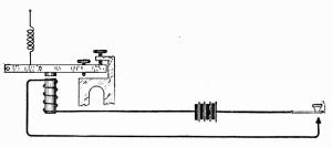
Fig. 15. Telegraph Sounder and Key
