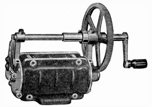
Fig. 64. Generator with Magnets Removed
