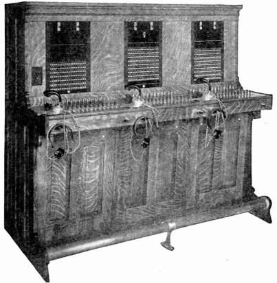
Fig. 177. Three-Position Lamp Board
