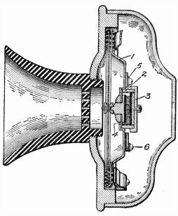
Fig. 42. New Western Electric Transmitter
