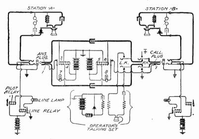
Fig. 162. Simple Common-Battery Switchboard
