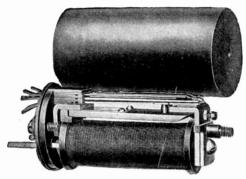
Fig. 216. Trunk Relay
