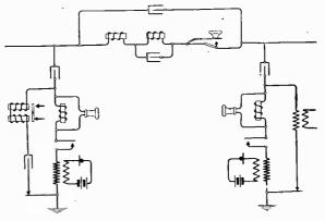
Fig. 238: Railway Composite Circuit
