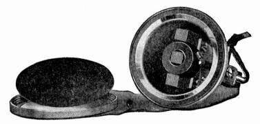
Fig. 56. Working Parts of Dean Receiver
