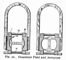
63. It is very important that the space in which the armature revolves shall be truly cylindrical, and that the bearings for the armature shall be so aligned as to make the axis of rotation of the armature coincide with the axis of the cylindrical surface of the
