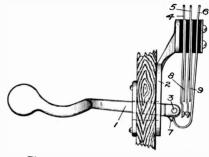
Fig. 76. Short Lever Hook Switch
