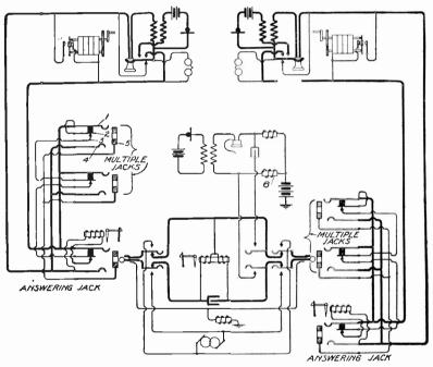
Fig. 182. Monarch Magneto Multiple Switchboard Circuits
