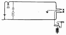
Fig. 157. Line Lamp with Relay
