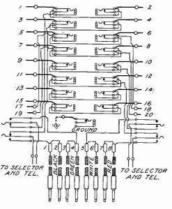
Fig. 262. Circuits of Test Board
