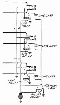
Fig. 158. Pilot-Lamp Operation
