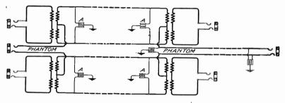
Fig. 227. Phantom Extended by Physical Circuit
