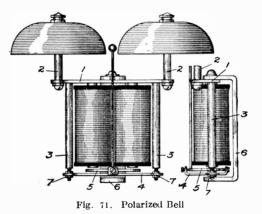
Western Electric bell by means of the nuts 7, by which the yoke 4 is secured to the standards 3. By moving these nuts up or down on the standards the armature may be brought closer to or farther from the poles, and the device affords ready means for clamping the parts into any position to which they may have been adjusted.
