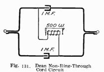
with the Dean Electric Company. It made use of two condensers of 1 microfarad each, one in each side of the cord circuit. The clearingout drop was of 500 ohms resistance and was connected from the answering side of the tip conductor to the calling side of the sleeve conductor. In this way whatever clearing-out current reached the
