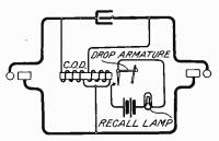
Fig. 138. Cord Circuit with Recall Lamp
