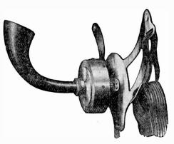
Fig. 47. Switchboard Transmitter
