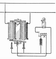
Fig. 236. Ringing Device for Composite Circuits
