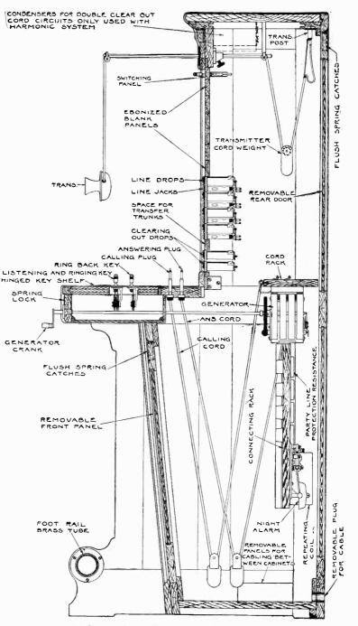
Fig. 145. Cross-Section of Upright Switchboard
