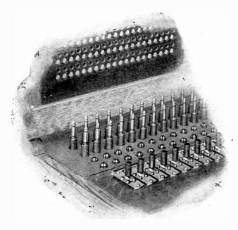
Fig. 175 Details of Lamp, Pluz, and Key Mounting
