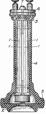
Fig. 49. Single-Pole Receiver
