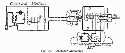
Neither the plug  $P_c$ , nor the ringing key R.K., shown in Fig. 90, is used in this operation. The clearing-out drop C.O. is bridged permanently across the strands 6-7 of the cord, but is without function at this time; the fact that it is wound to a high resistance and impedance prevents its having a harmful effect on the transmission.
