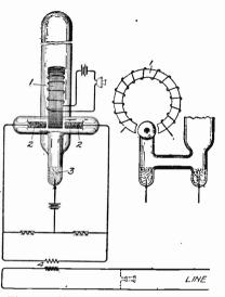
Fig. 37. Mercury-Arc Telephone Relay
